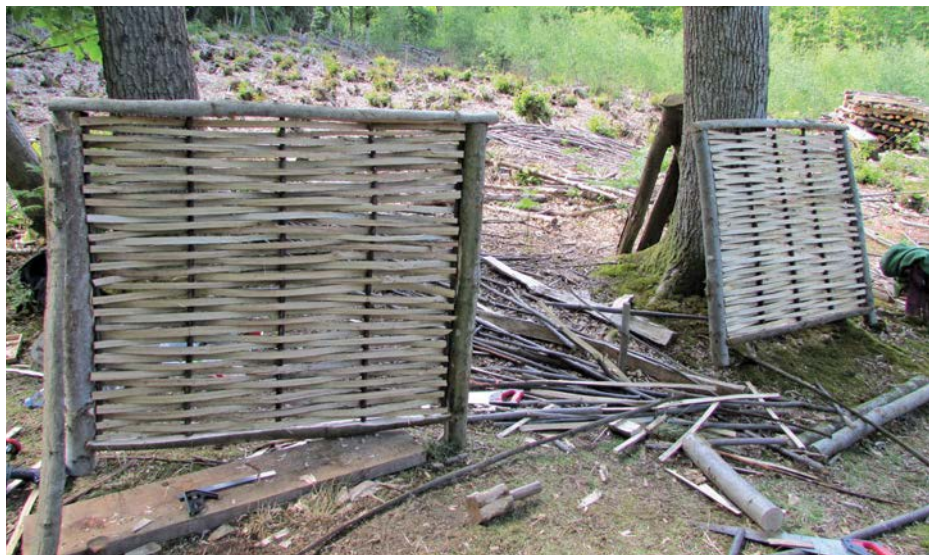
A completed woven panel
