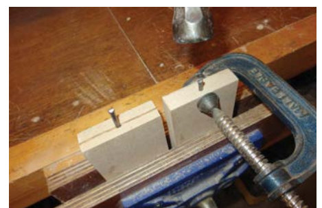
Nails are notorious for causing splits but clamping prevents this quite easily
