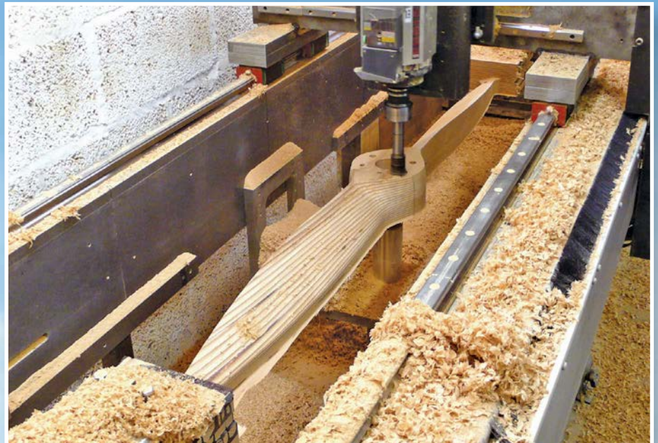
A partly machined blade. Note the step cuts at this stage
