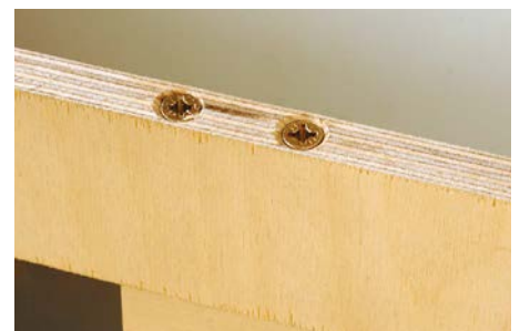
Pre-drilling even in rather thin components can avoid splitting
