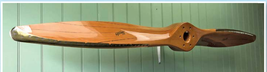
A newly-made vintage style propeller with brass leading edges
