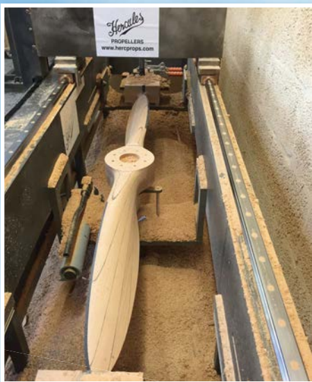
A CNC machined propeller
