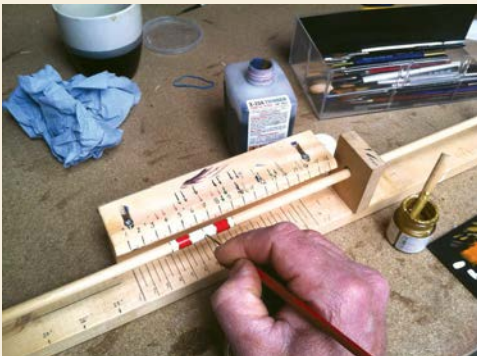
Creasing the arrow shaft
