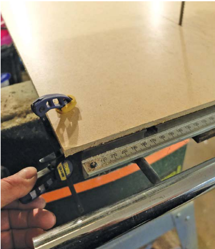
A sub bed gives a smooth surface that won't trap waste. A strip glued along the front edge obviates the need for clamping
