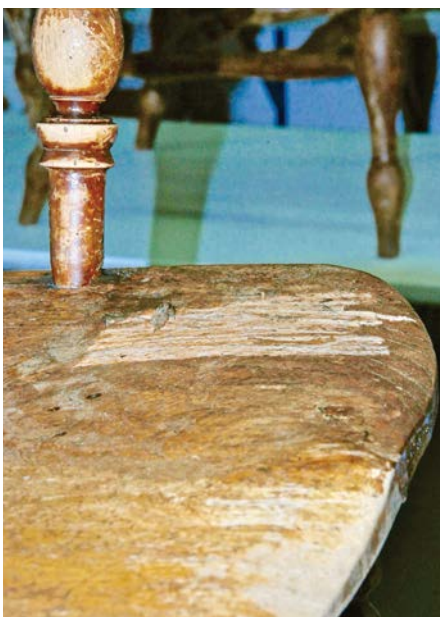
Once the stripper begins to react, the finish will become soft enough to scrape back.
