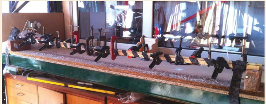
A laminated stave being glued up
