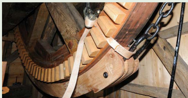
Newly fitted cogs in a restored windmill
