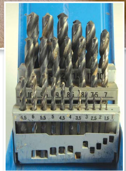
Drill bit shanks in good condition give exact sizing
