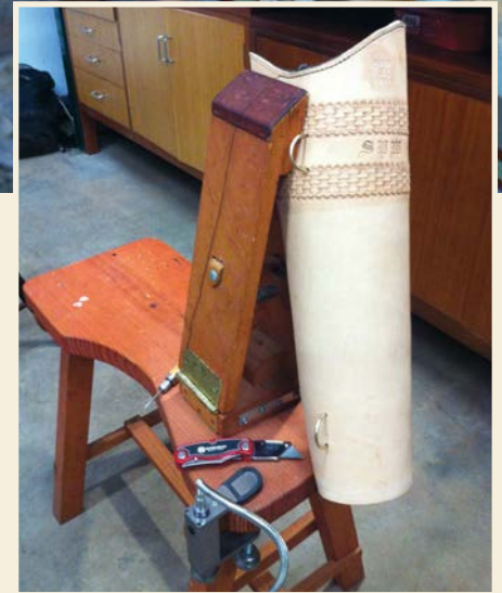
A 'stitching pony' used for holding leather while hand stitching
