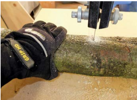
Wet log cutting with a firm grip. The machine casing will fill up with wet sawdust easily
