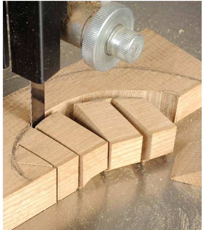
Relief cuts before cutting curves are essential to avoid trapping the blade
