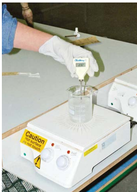
It is important to keep an eye on the temperature of the oxalic acid to avoid it rising above 45°C
