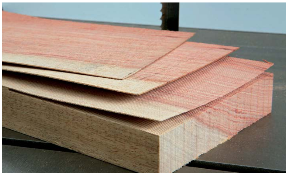
Sawn veneers are possible if you have a high fence and a raker tooth (set left, unset, set right pattern) – note blade marks
