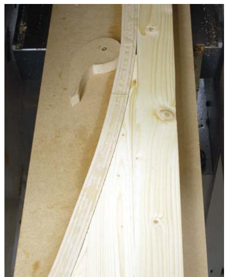
Thin ash strips glued up in a jig to create one of three curved legs for a plant stand
