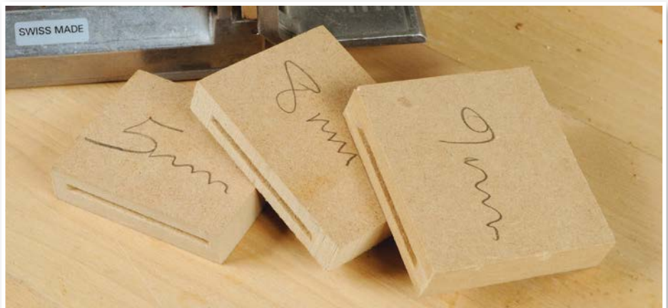
Spacer blocks for biscuit slotting board edges
