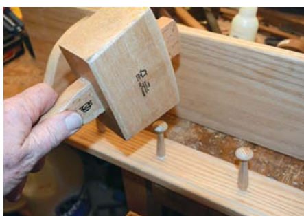
Each peg is tapped home, checking it is standing perpendicular
