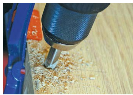
A mitre framing clamp holds the shelf end while dowel drilling
