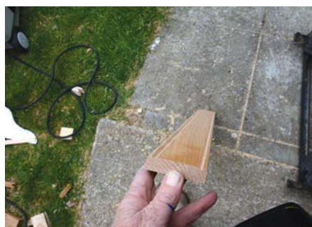
The peg rail has rounded edges and V-grooves done with a router
