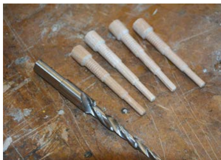
Miller stepped dowels are a very effective method of jointing
