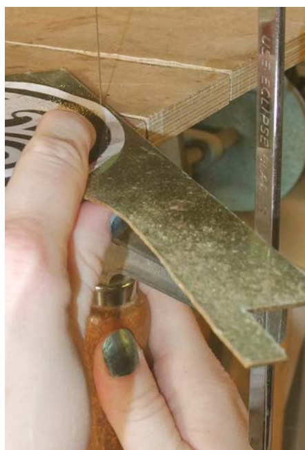
A piercing saw and very fine-tooth metal cutting blade shaping a piece of brass inlay
