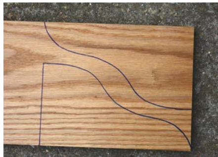
The two shelf ends marked out using a cardboard template
