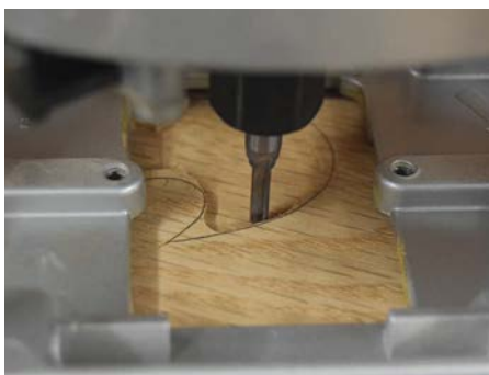
A router and small straight cutter creating a recess for a contrasting wood inlay
