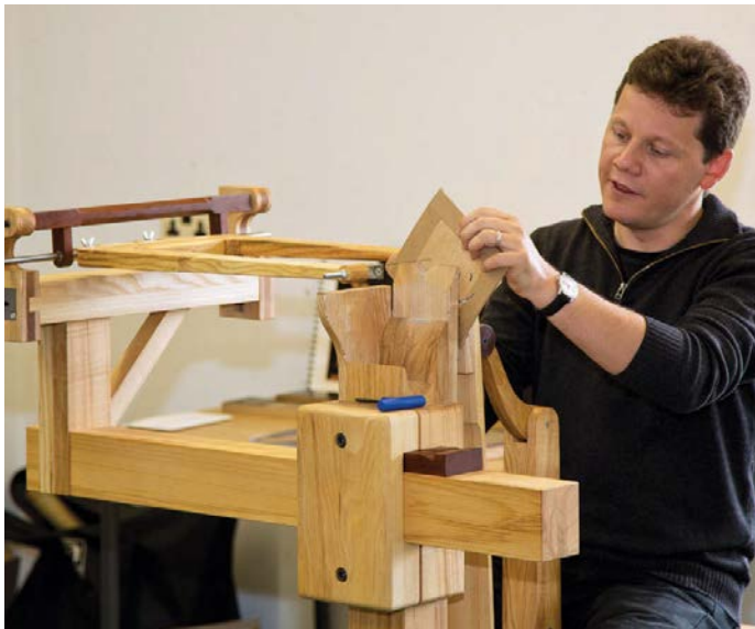
Yannick Chestang, Boulle marquetry restoration expert, demonstrating use of the 'donkey' or 'chevalet'
