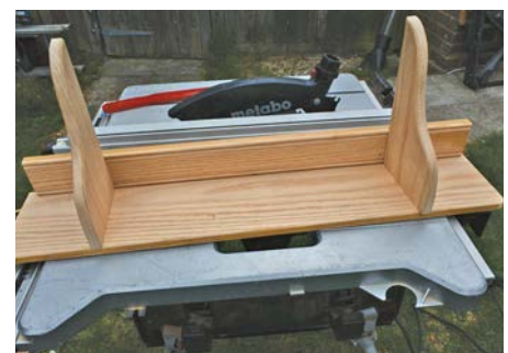
Checking the correct positions for the shelf ends – the peg rail will be cut down
