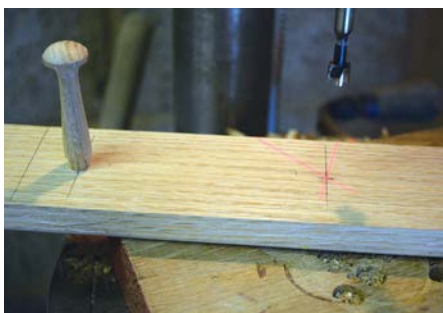
A saw-tooth Forstner bit in a pillar drill is the most precise method
