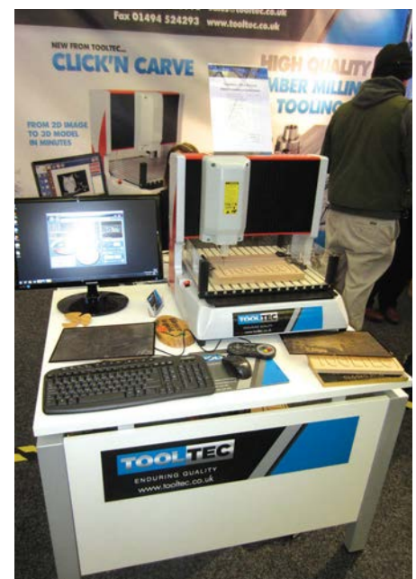
One of many desktop CNC machines which can be programmed to shape, carve or create spaces for inlay
