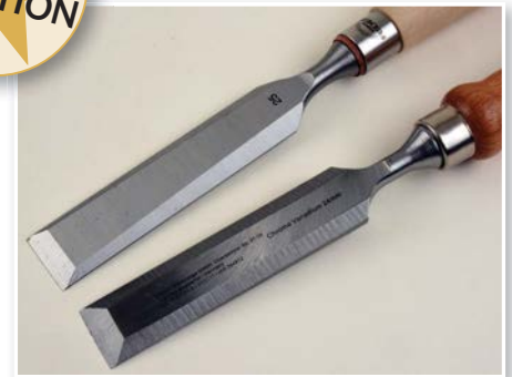
Note the differences in surface grinding, lack of a shock washer and a thinner ferrule on the cheaper chisel
