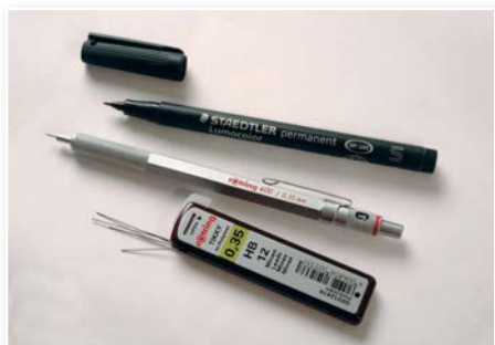
A mechanical pencil and fibre-tip drawing pens are perfectly adequate for most technical drawing work
