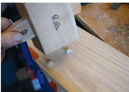
The dowels are glued and tapped firmly into place
