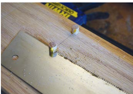
A flush-cut saw takes care of the projecting dowel ends
