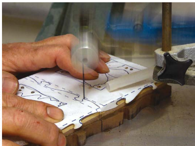
A scrollsaw is the perfect way to achieve controlled fine cuts and follow awkward shapes
