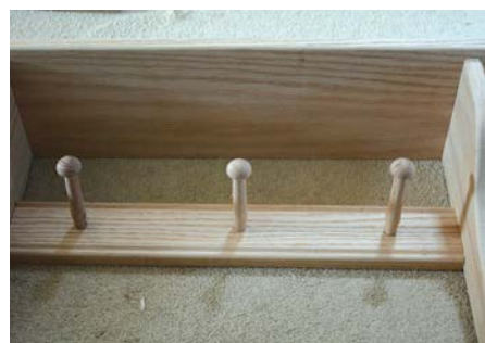
Assessing the correct spacing for the pegs before drilling
