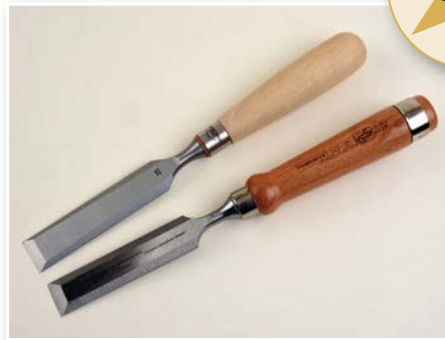
A good quality European-made chisel (top) and a budget Chinese chisel (bottom)
