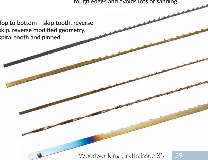
A fine-tooth blade cuts cleanly, minimises rough edges and avoids lots of sanding
