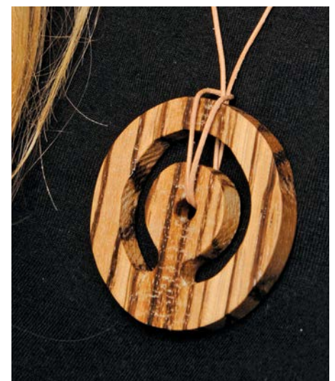
A fine-tooth blade cuts cleanly, minimises rough edges and avoids lots of sanding
