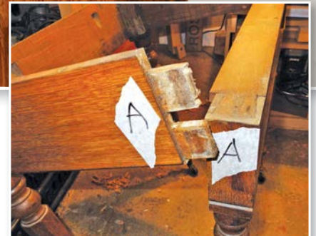
Purely functional twin dovetails connecting a top rail to desk legs
