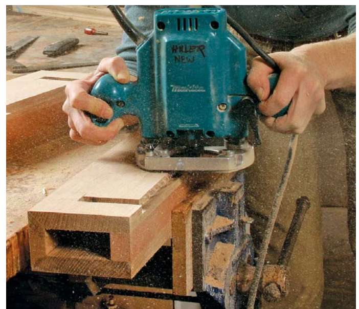
Rout a rabbet for the backboards. A rabbetting bit works well, with the guide bearing running against the side of the column. Stop the rabbet in the shelf dados
