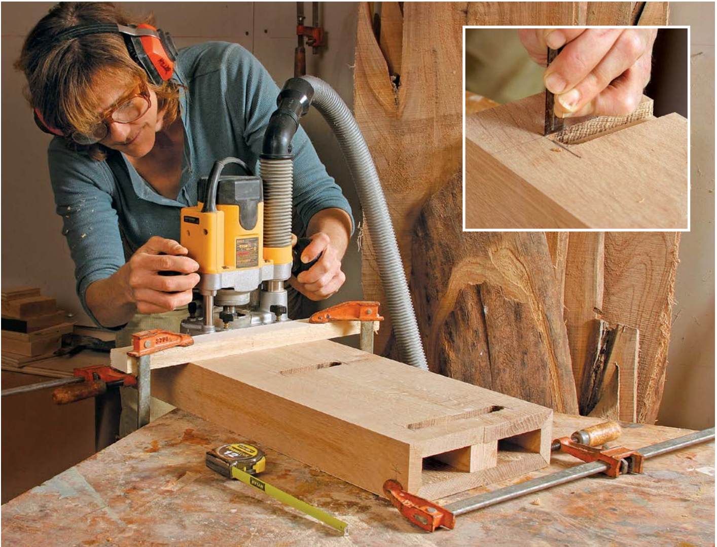
Above: Rout shelf dados while columns are clamped together. Clamp a straight edge to the columns to guide the router
