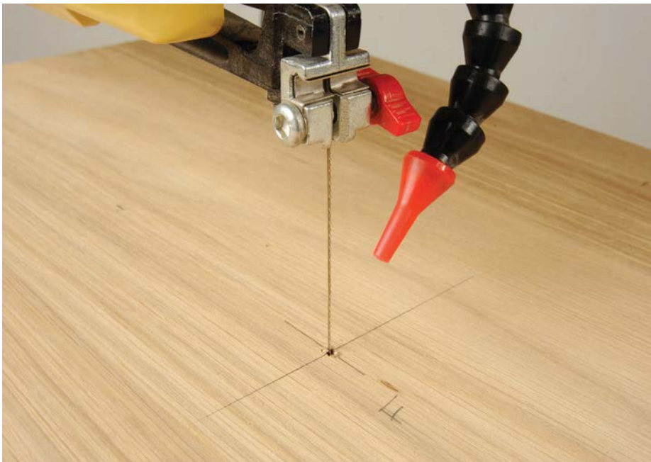
You can make your own sub bed, which gives maximum support for small pieces
