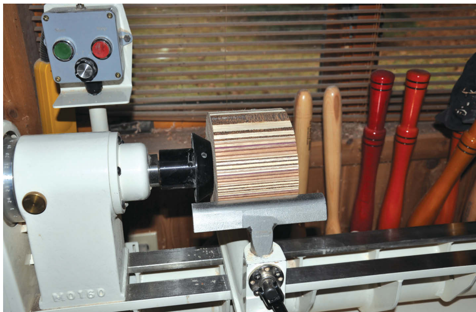
Mount the blank securely before starting
