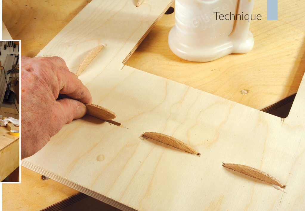
Biscuits give positive location during glue-up as well as creating strong joints
