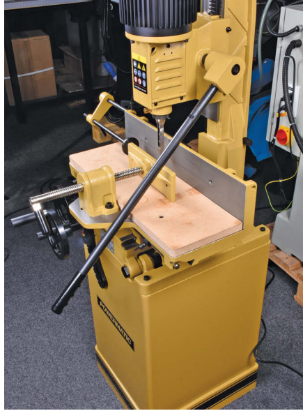
The pull-down lever can clash with the mortiser bed
