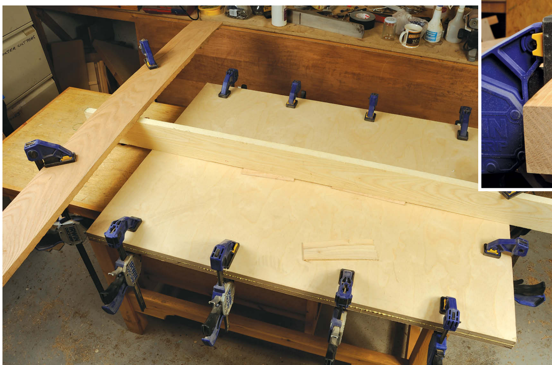
Above: Clamps can wrongly apply pressure so components are no longer perpendicular to each other
