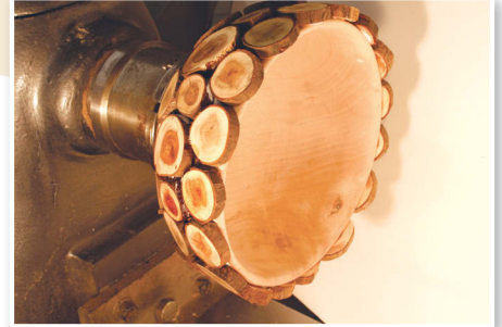
Epoxy resin bonding wood slices to a bowl
