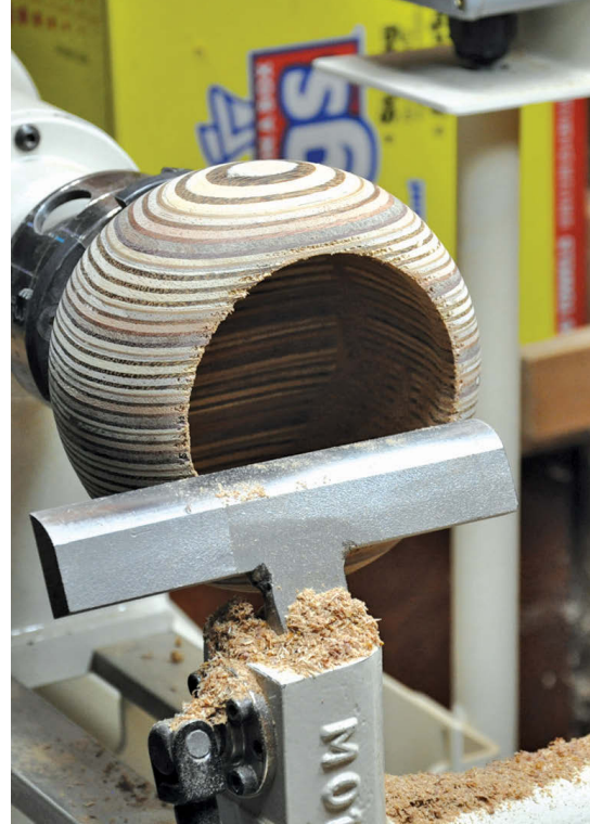
Finish cut the inside nicely and clean up the rim
