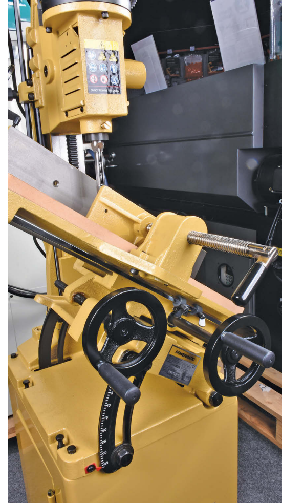
The tilted bed allows for angled mortising
