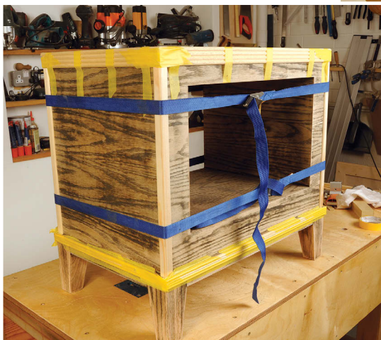
Ordinary luggage straps pressing newly glued corner pieces on to a carcass prior to an overall paint treatment
