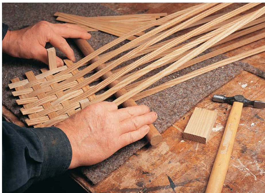
Kevin uses woven ash as an intriguing form of panelling for his hi-fi cabinet
