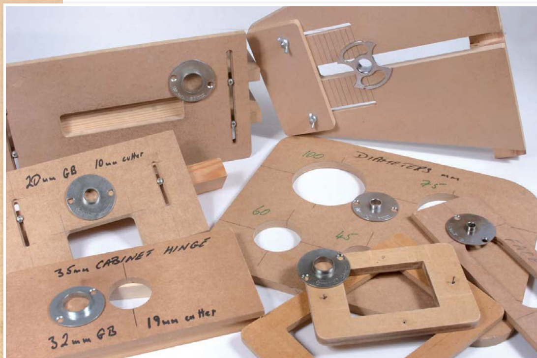
Each jig or template and router will tend to need a different cutter and guide bush combination
