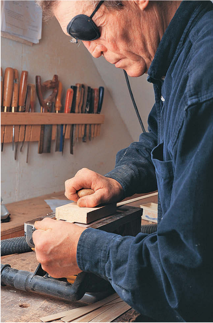
Sanding ash strips on an inverted belt sander using a homemade pressure block to save the fingers
