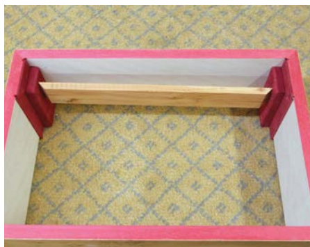
Using test blocks for tray supports to check the length of the tray components
