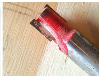
Router cutters get hot and the deposits stick on, but here the muck has come off
