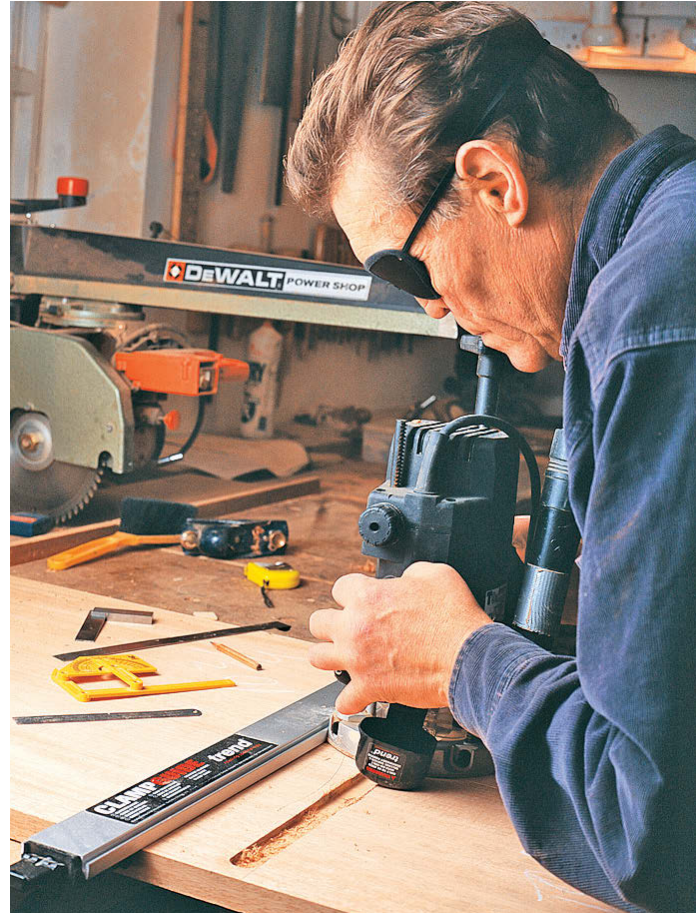
Routing the angled shelf housings using a clamp guide
