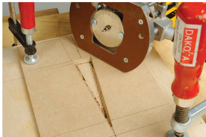
Machining the outline shape with a very small cutter and guide bush
