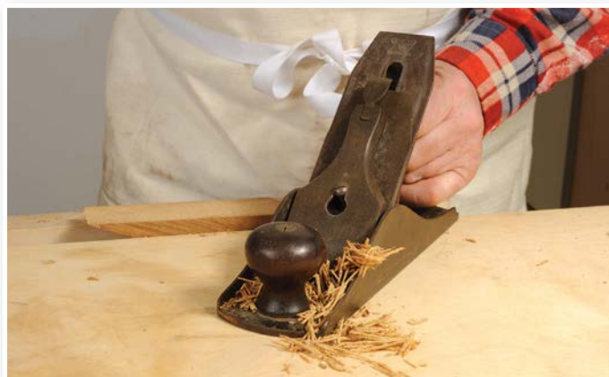
A late 19th-century No.4½ smoothing plane with squat front knob and Sweetheart blade. Sympathetically restored by cleaning alone, no abrasive treatment
