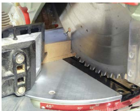
On the mitre saw cutting the half lap joints to the correct width
