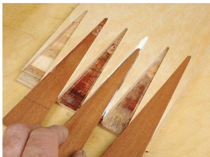
Cut and shaped fingers of contrast wood glued in place
