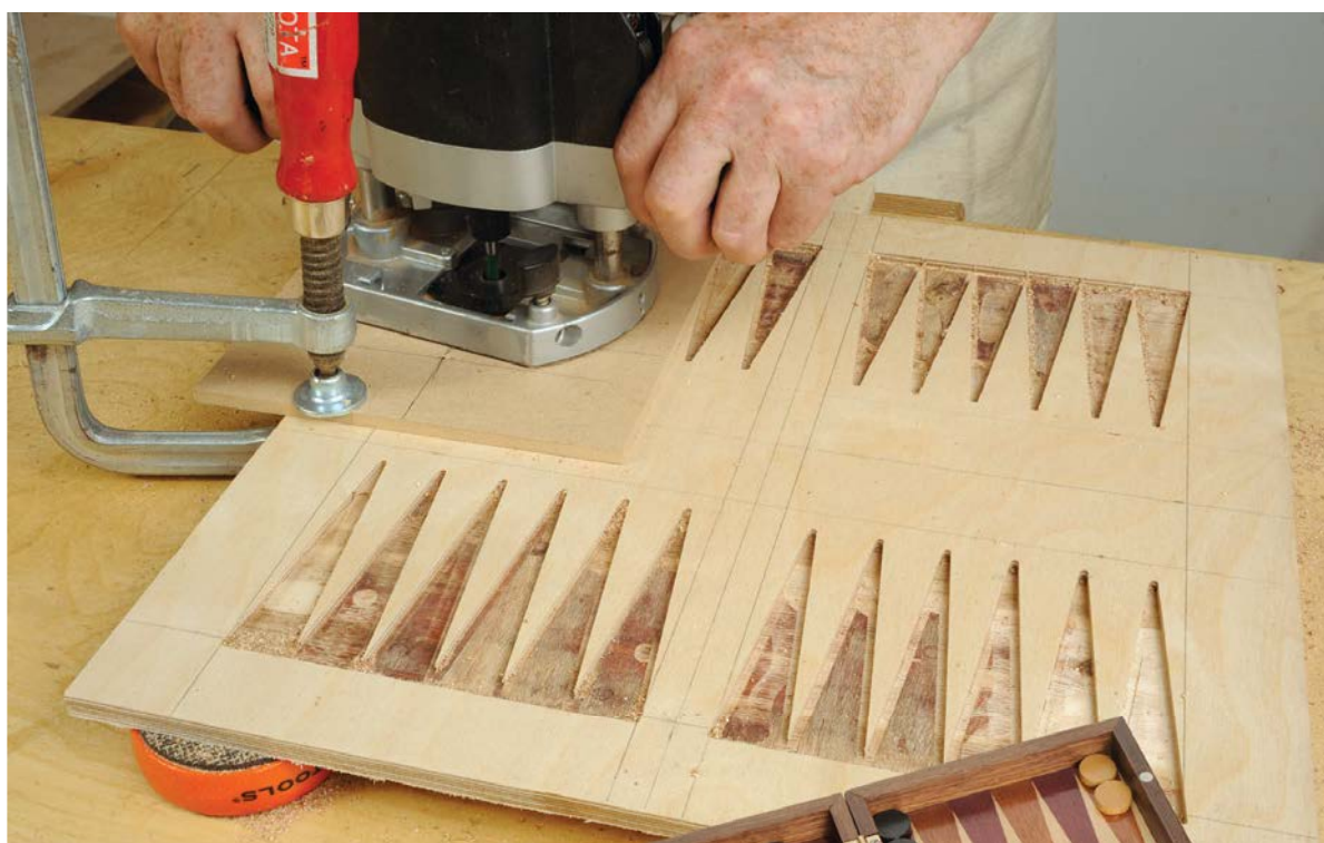
Machining the outline shape with a very small cutter and guide bush
