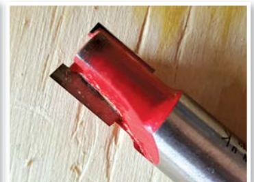
Router cutters get hot and the deposits stick on, but here the muck has come off
