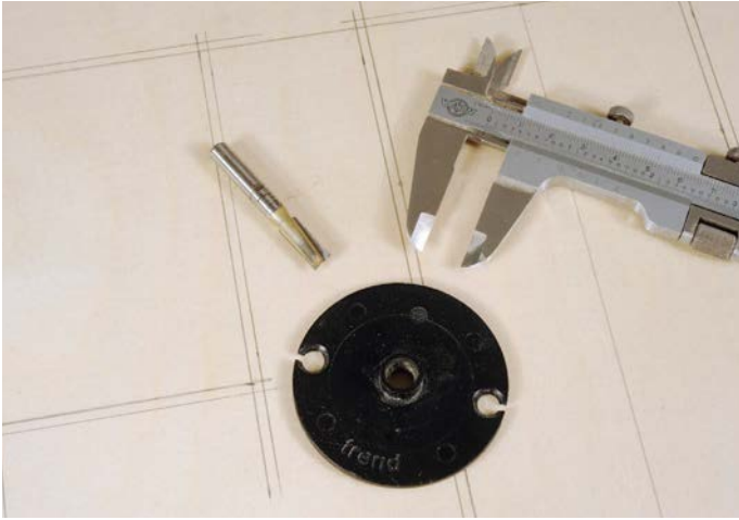
Vernier callipers are an essential method of checking respective diameters when calculating the offset
