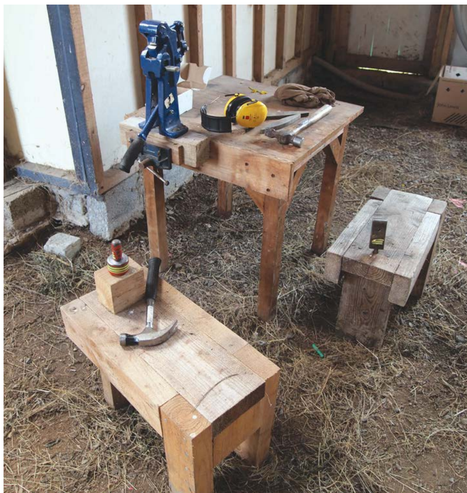
Peening kit: Top left: Table with hand peening machine Bottom left: Peening bench with peening jig and hammer Right: Peening bench with peening anvil.
