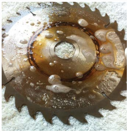
A very gummed-up blade comes up almost like new
