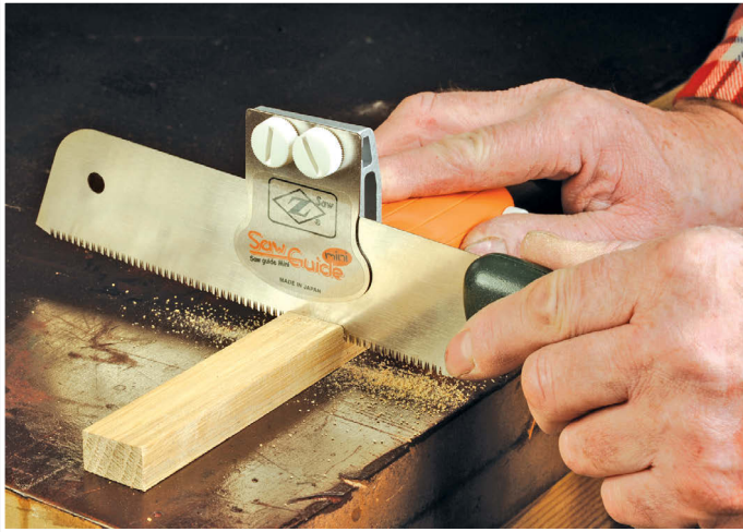
This Z-Saws mitre saw and guide is quick and easy to use and will do perpendicular cuts too
