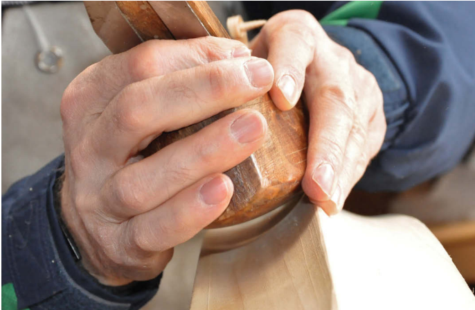
This is one of the modestly sculpted bats where the wooden convex sole planes really come into their own
