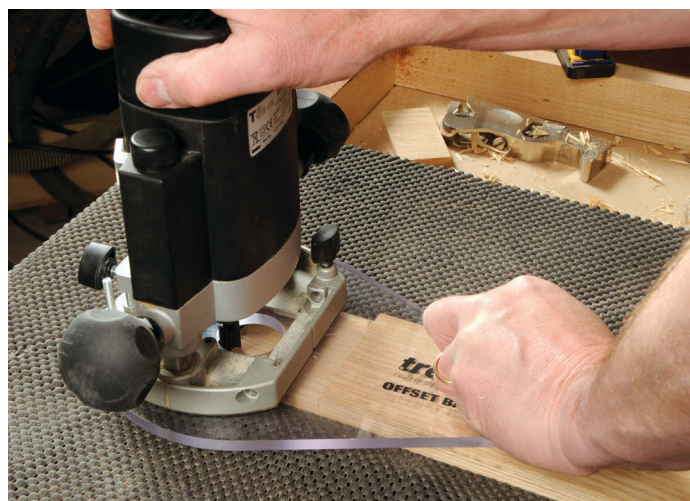
An offset base with a hold-down knob gives control and an even finish when edge machining
