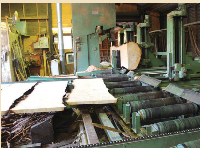
The feed roller moves the boards away
