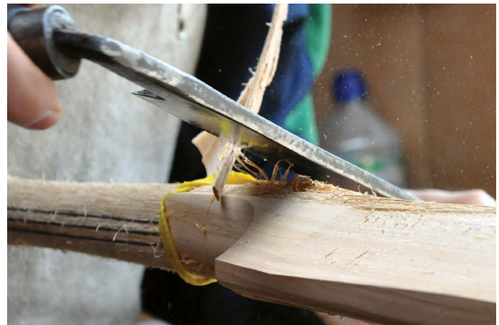
Starting with a CNC machined blank, Robert then uses very traditional tools, such as this drawknife. He changes from heavy 'hogging' cuts to perfect shape refining cuts with incredible speed, flicking from bevel up to bevel down almost unnoticed
