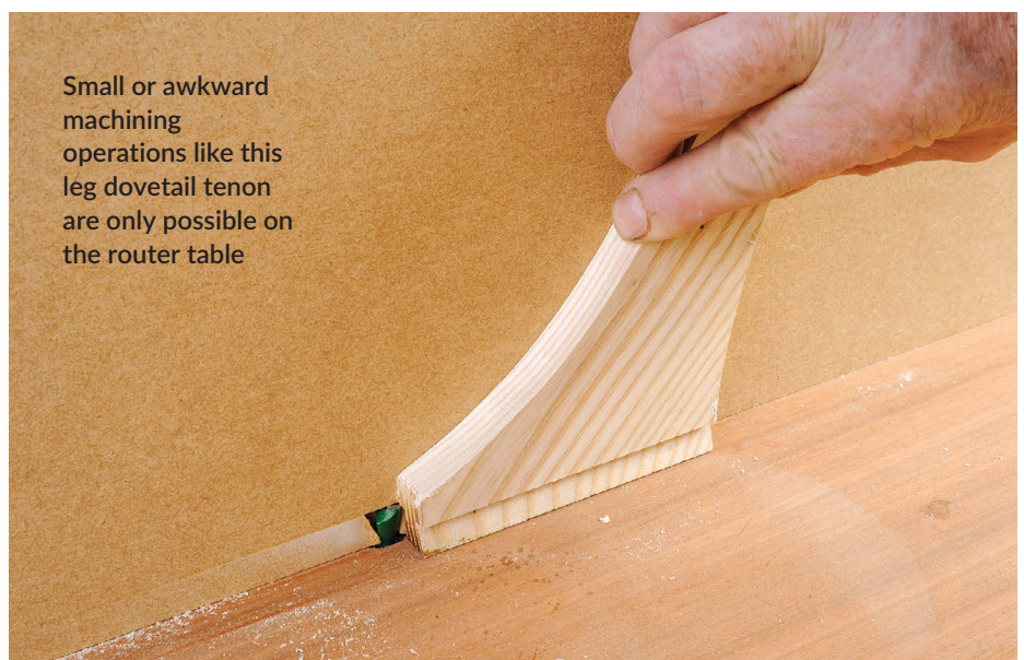
A simple homemade router table clamped in a vice giving excellent control of the work
