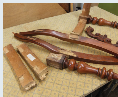
One chair knocked apart with insect damage to the rails and severely damaged tenons
