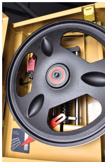
A very solid bandwheel microswitches a tension scale
