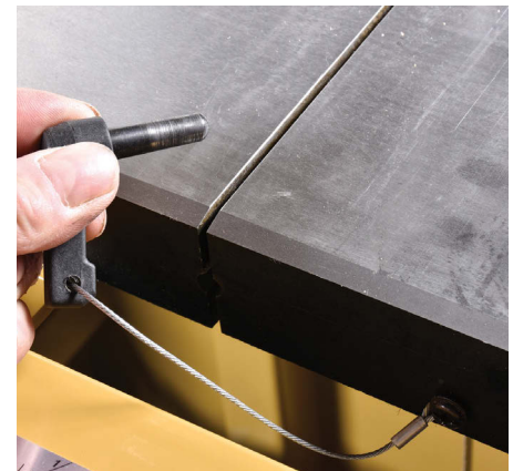
A tapered steel dowel keeps the surface level
