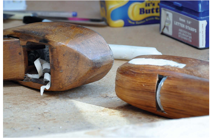
Wooden planes play a large part in this initial shaping and have the advantage of being suitable to modify for a specific profile
