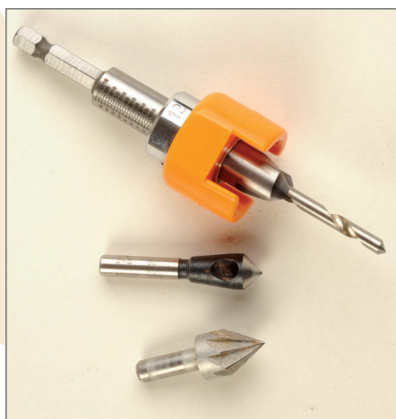
From top: Counterbore; snail and rose countersinks
