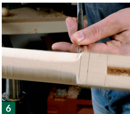
6 Shaping the leg down to start the taper using a spindle gouge
