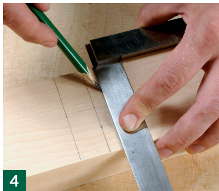
4 Transferring the mortise markings across two leg blanks
