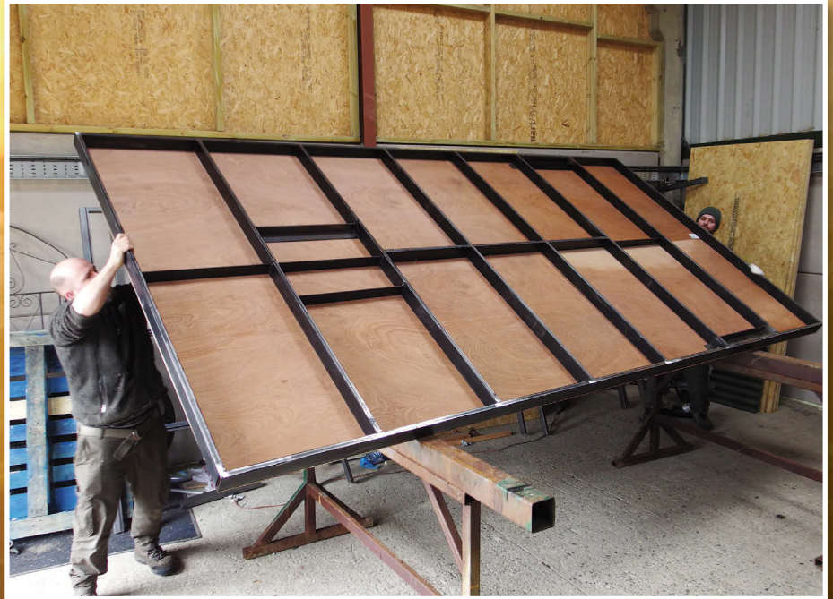
Clockwise from top left: Bare base steelwork after initial welding phase; Dicky and helping hand Chris are flipping the base over relatively easily thanks to the tubular steel construction; the pair of them lining up the rear axle assembly
