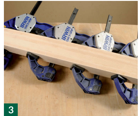
3 Two sets of leg blanks glued up from 28mm sawn stock, two per blank
