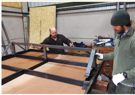
Clockwise from top left: Bare base steelwork after initial welding phase; Dicky and helping hand Chris are flipping the base over relatively easily thanks to the tubular steel construction; the pair of them lining up the rear axle assembly
