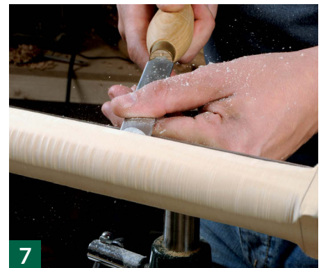
7 Planing the taper with a skew chisel – extra care must be taken near the leg's shoulder
