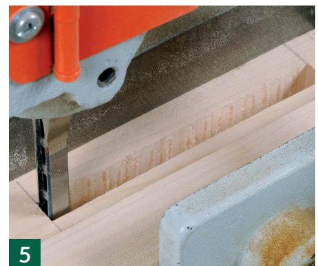
5 Using a chisel mortiser to cut the long thin frame mortises – note the width is greater than the chisel used
