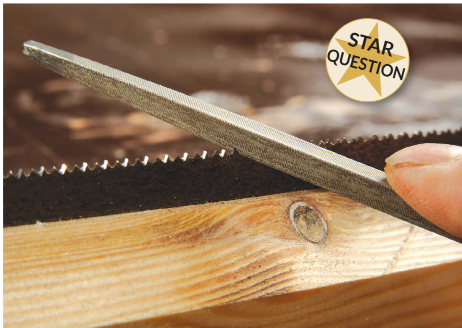
You need a degree of skill to sharpen saw teeth properly
