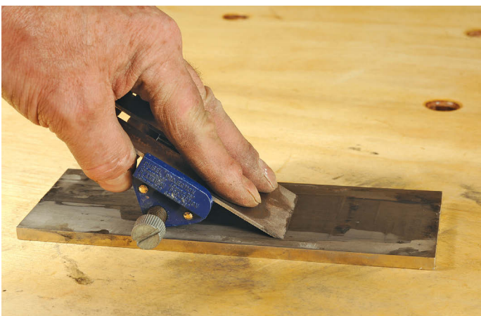
The use of a honing guide gives a much more predictable result as the angle and shape of the bevel will be constant
