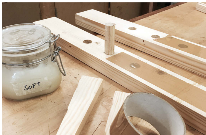
Protect the inside face of the bars with packing tape and beeswax polish
