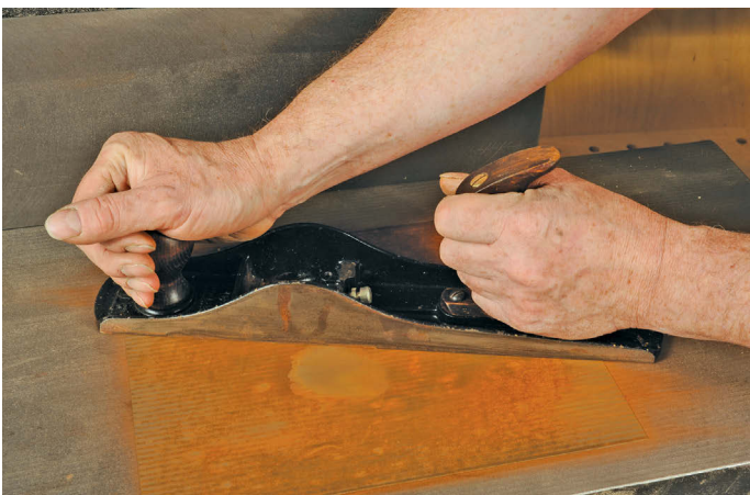
Rubbing down the base of a No.5 jack plane to remove rust and to 'flat' it properly before bringing it back into use
