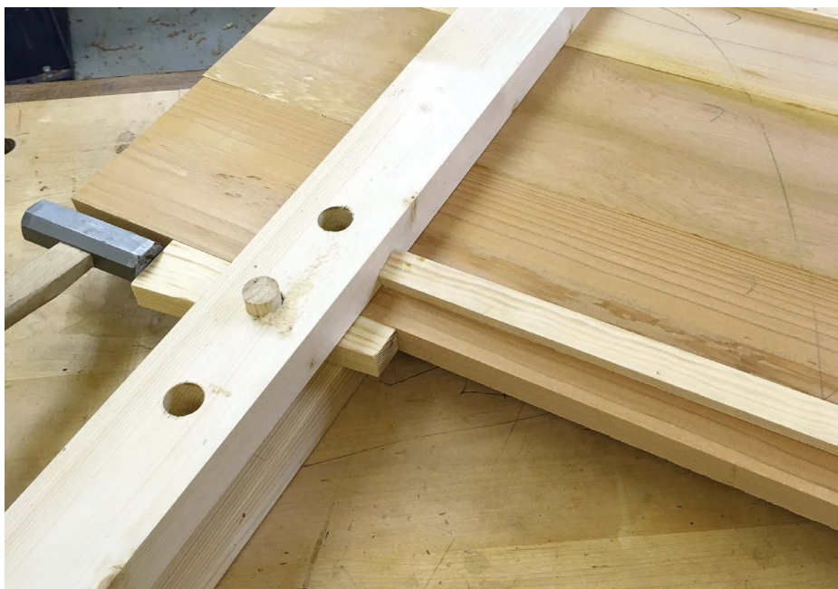
Put a batten between the clamps and drive the wedges towards the centre
