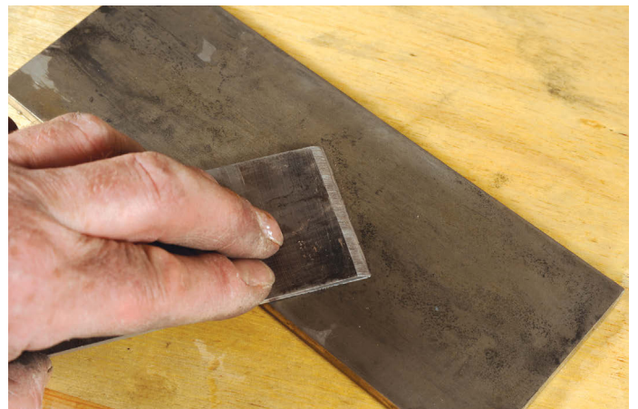
The importance of flattening the back of a plane blade is often ignored. It ensures both edges meet properly at the bevel edge
