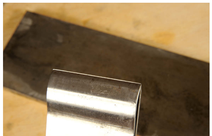
The cap iron has been rubbed on the sharpening stone so there is no gap for shavings between the two irons
