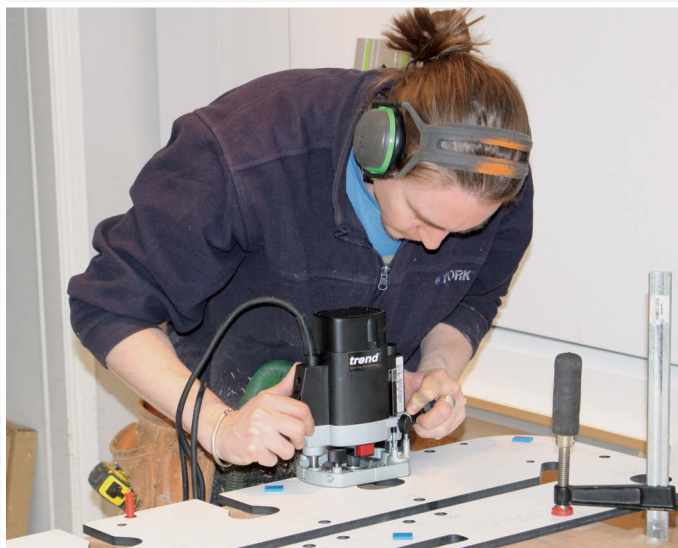
Liam Motyer machining a kitchen worktop joint
