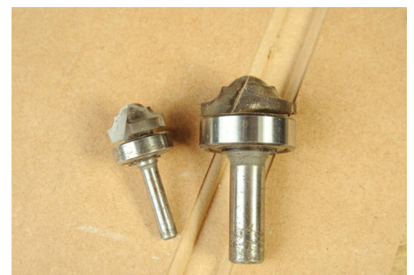
Face mould cutters which need to run around a template for a properly guided and accurate result. Dust is an issue especially with MDF, so extraction has to be fitted to the router
