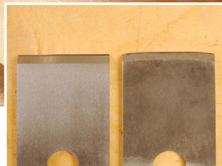
The difference between a straight blade edge and a cambered one for a No.5 jack without any dig-in
