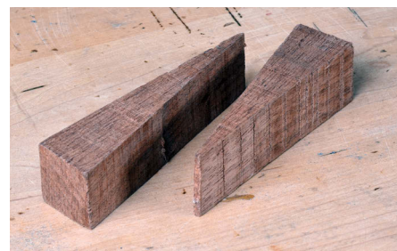
Leave folding wedges rough sawn
