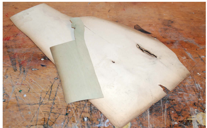
Several weeks in the solution altered colour of the holly veneer to a pale green
