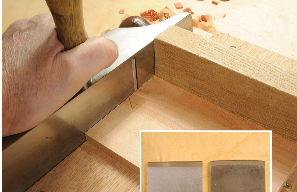
Above: A dead straight edge is needed for narrow edge planing or shooting endgrain for a very accurate result
