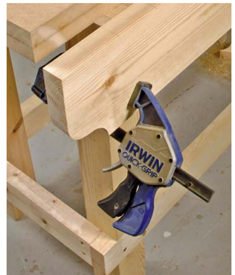
Sometimes just clamping workpieces vertically is enough to be able to work on them
