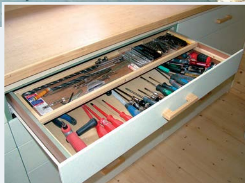
ABOVE: Next a set of drawer boxes constructed from ply with tongue and groove joints and mounted on easy runners
