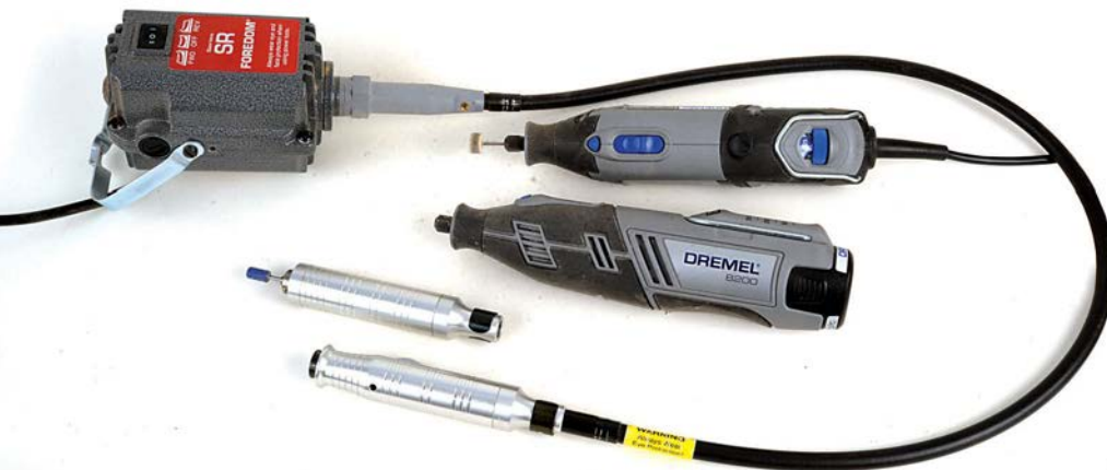
Different types and sizes of rotary carving unit: a suspended motor option with flexible drive shaft and hand-held units which come in various sizes
