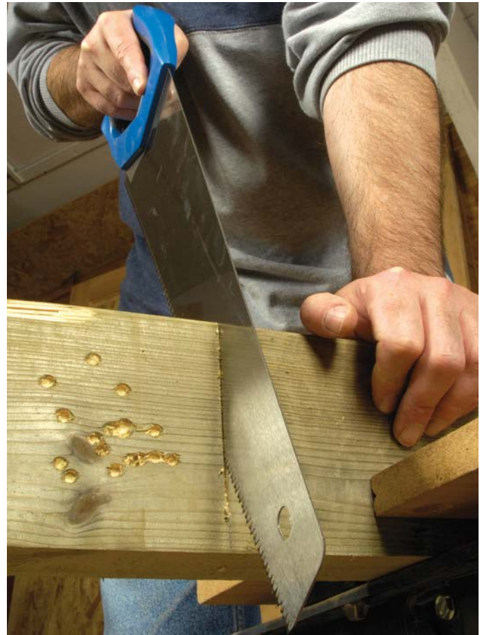
A hardpoint saw is quick and reasonably accurate
