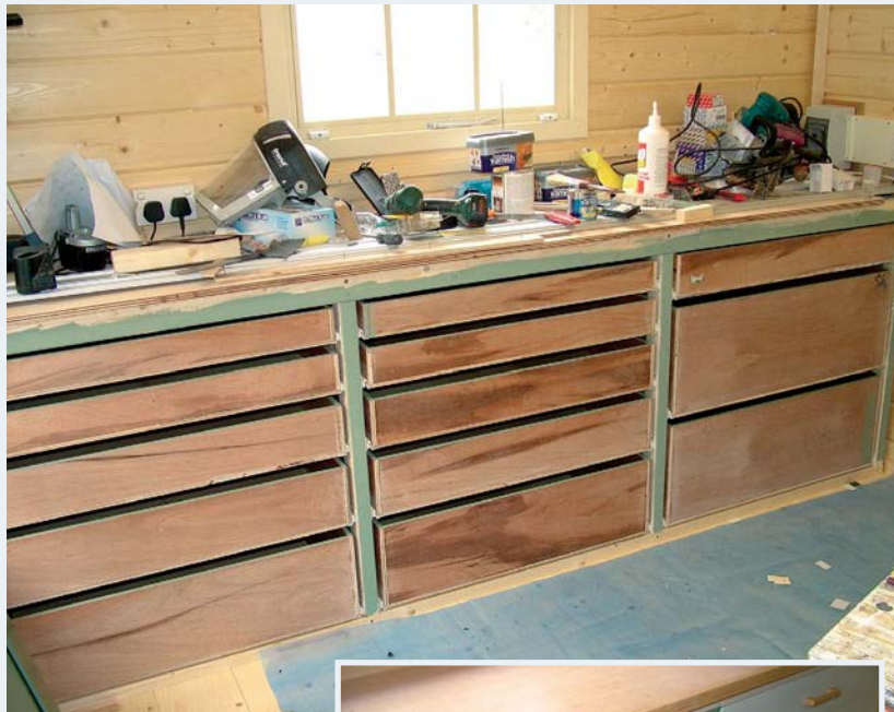
ABOVE: Next a set of drawer boxes constructed from ply with tongue and groove joints and mounted on easy runners
