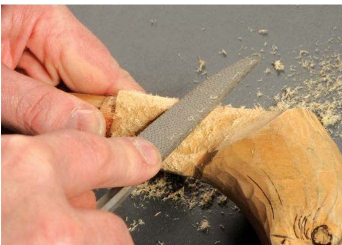
Sometimes a fine tooth rasp is quicker and easier than trying to use a gouge
