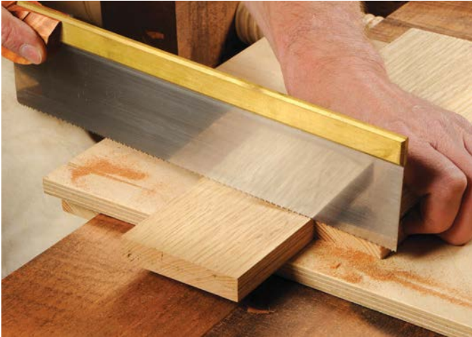
A traditional tenon saw will give very precise fine cuts
