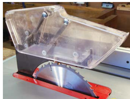
When wood is pushed against the guard it raises upwards like this
