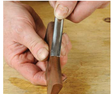
Carving gouges are sharpened using slipstones and then stropped using a special profile covered with metal polish
