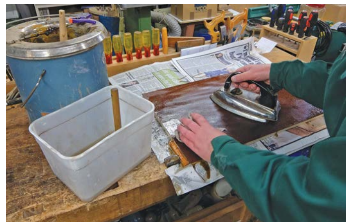
Re-heating the hide glue while hand veneering
