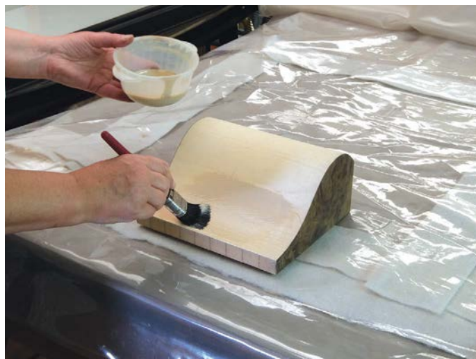
Spreading the aliphatic resin cold press veneer glue ready for the bag press
