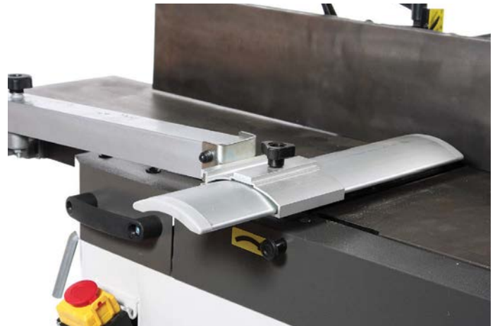
The majority of surface planers are fitted with this standard swinging arm guard. There is normally a height limit which when reached means tall stock will need to be fed alongside the guard in its low down position instead
