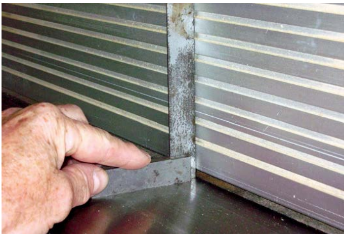
This extruded aluminium fence is unusually flat, many are slightly uneven which makes accurate squaring of stock rather problematic
