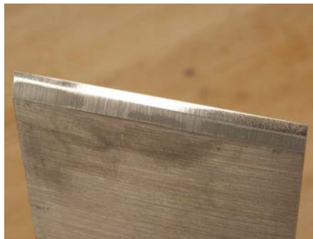
After stropping on leather or a 'short grain' MDF block with metal polish the wire edge will vanish and the edge will get a shine indicating it is sharp
