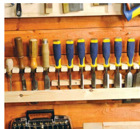
A set of chisels and several gouges that will deal with almost any job
