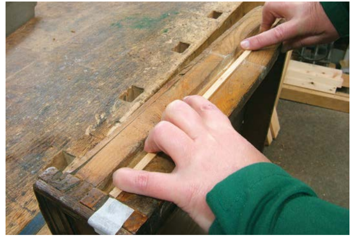
Forming a rub-joint with animal/hide glue
