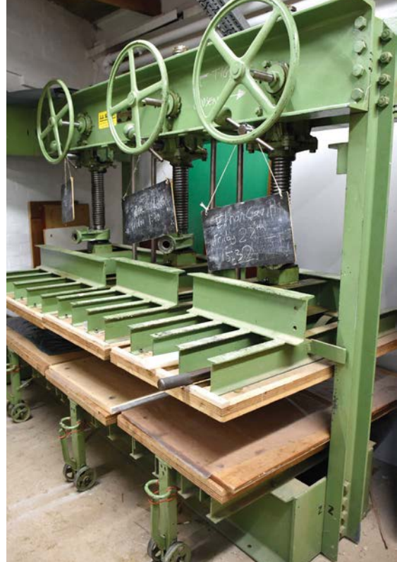
The veneer press showing whose work is being pressed
