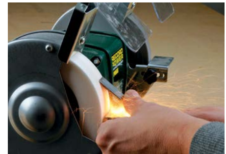
A dry grinder is fine for turning tools but there is a danger of overheating the metal particularly with plane and chisel blades – shown by discolouration of the steel
