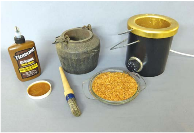
Traditional and electric glue pots with pearl glue and a bridled glue brush and modified hide glue for use cold
