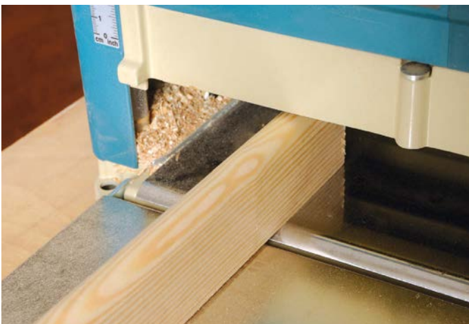
Cabinet thicknessers are really useful but the infeed and outfeed tables may need adjustment accessible underneath, in order to give continuous support while reducing or eliminating 'snipe' or stepping at the ends of the workpiece
