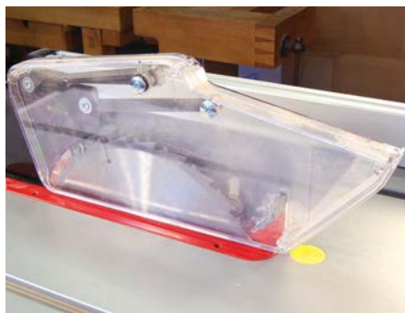
This form of see-through drop down guard is ideal for vision and safety
