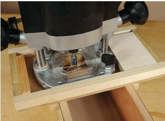
Two blocks dropped in which allow a limited amount of sideways movement so the mortise width can be increased
