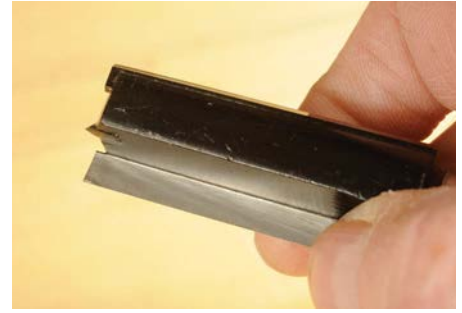
A twin bladed TCT straight cutter, the bottom cutting insert is essential for plunge mortising
