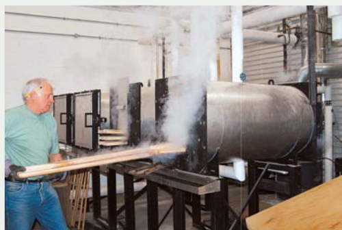
The steam bending process at Ercol, Princes Risborough
