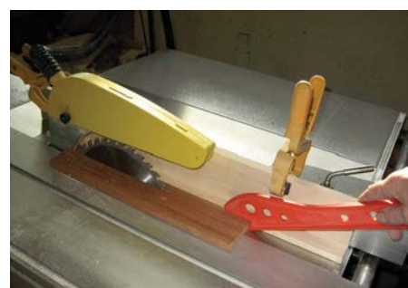
You can make your own sub-fence, which can be located in any position or turned over to give support to small section
