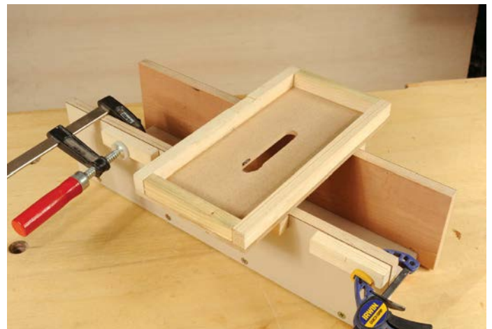
The mortise box with a router tray on top. Note the fillets under the tray and mortise length stops clamped at each end
