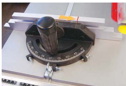
An adjustable and accurate mitre protractor, the arrow has been used to a zero position for the sub-fence
