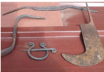
Drawknife, bowl gouge, kilt broach and billhook, all made from scrap
