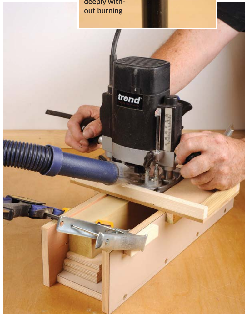
The mortise box in operation; note the support packers so the cutter can have enough plunge depth and extraction fitted as well
