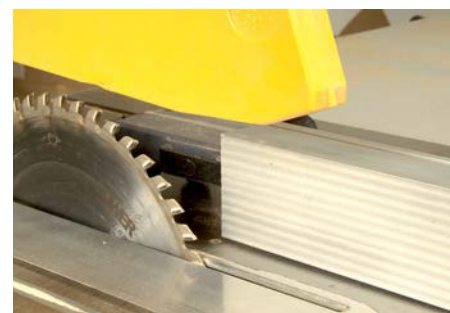
When ripping solid wood withdraw the rip sub-fence to the front of the blade to reduce the chance of timber binding
