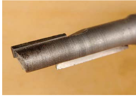
Stagger-tooth cutters have single offset blades, which makes cutting quicker but rougher, however it does allow chippings to escape more easily
