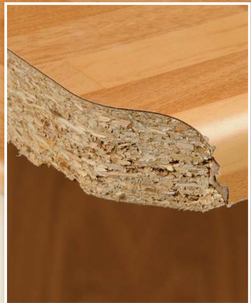
If you machine from the back to the front of the worktop the laminate will breakout
