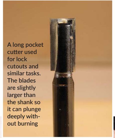
A twin bladed TCT straight cutter, the bottom cutting insert is essential for plunge mortising
