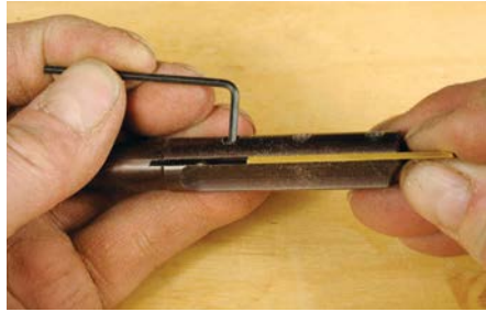
A disposable tip straight cutter. The tips are usually reversible, making it more economic for quantity production work
