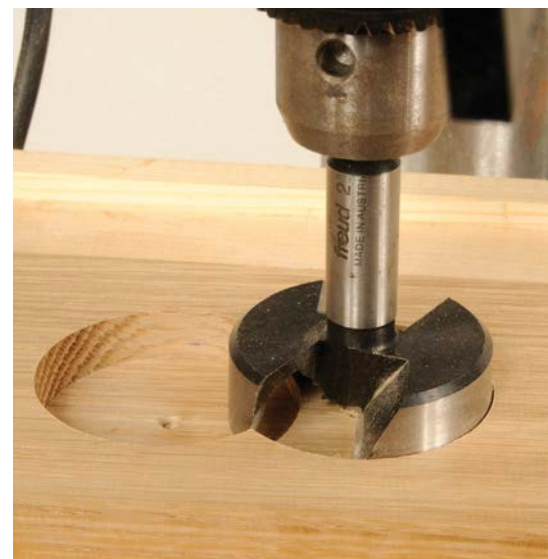
Forstner bits can cut overlapping holes easily due to the cutting action and centre point
