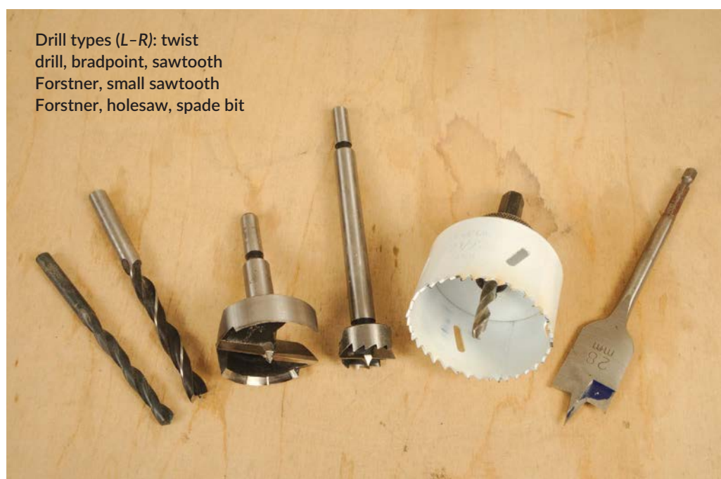
Forstner bits can cut overlapping holes easily due to the cutting action and centre point
