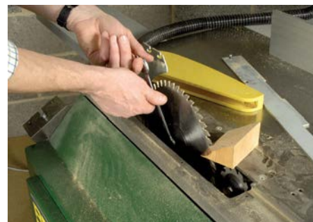
Easy blade changing on a sliding table saw. Note the wedge to hold the blade fast, some machines use an arbor locking rod
