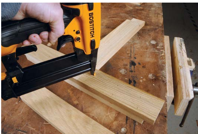
Powered nailers with their own specialised consumables make for fast, repetition fixing
