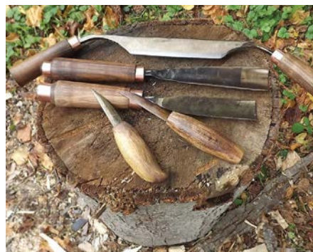
Drawknife, gouges and craft knives fitted with wooden handles and copper pipe ferrules
