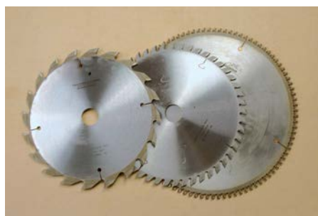
Three different sizes and types of circular saw blade: (L-R) rip/crosscut/triple tip board cut
