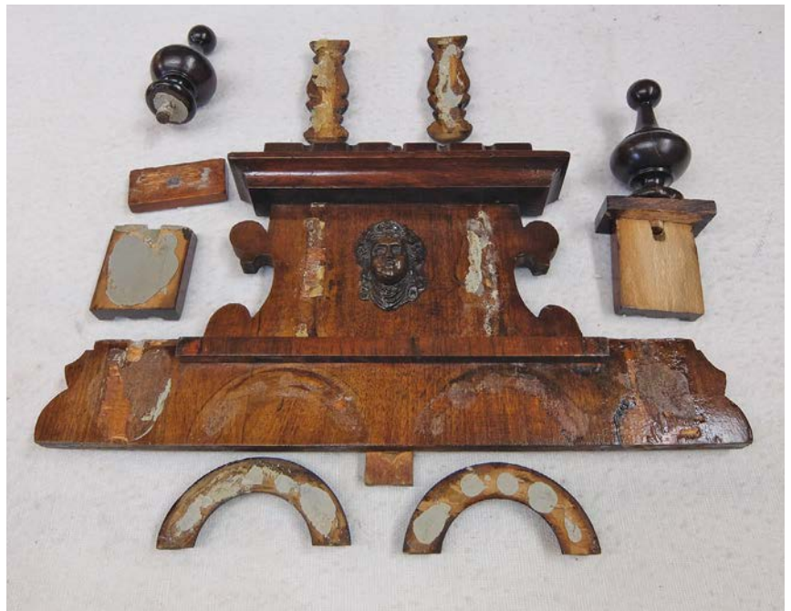
The top pediment with car body filler which glued the applied decoration
