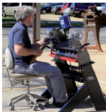
Optional Universal Stand adjusts for the standing or seated turner
