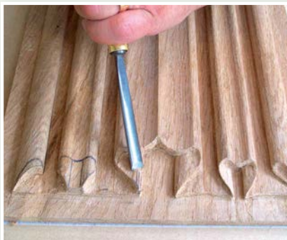
Carving a linenfold panel
