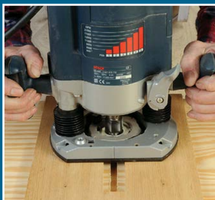
USING A HOUSING JIG
