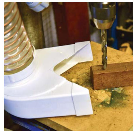
Angled drill press dust collector
