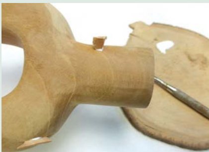
Glue repair wood into hole
