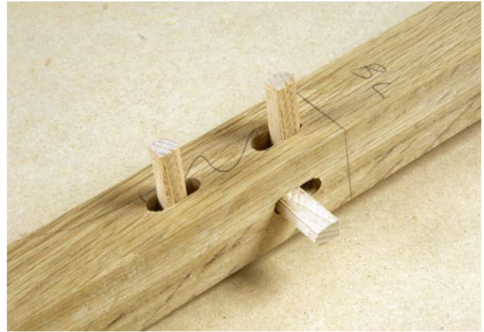
A test joint with mortises offset using split Dominos so they are easy to remove
