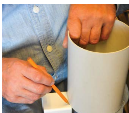
Mark cuts carefully
