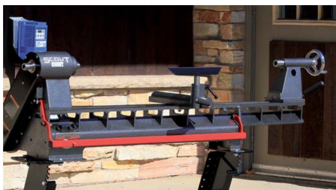
The optional bed extension gives 16" of increased spindle capacity. Used by the headstock, you can turn outboard to 21"
