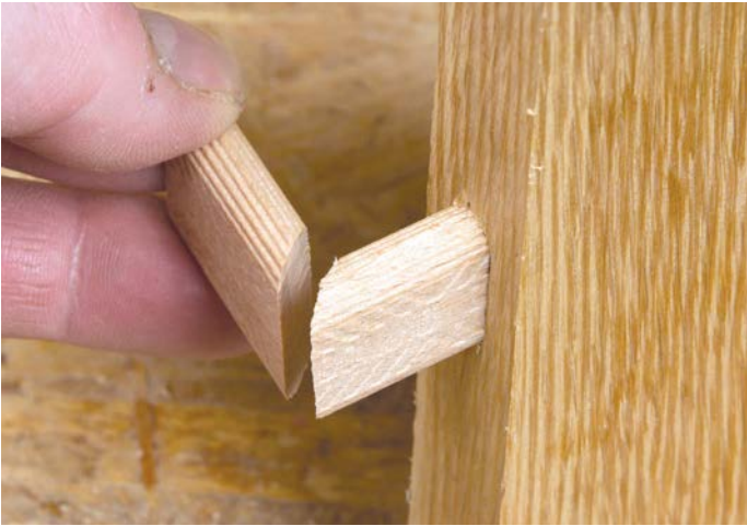
A neat method of making corner leg tenons using Domino components, but being in-line may cause sub-assembly problems
