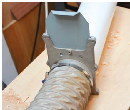
Magnet holds blastgate open/closed
