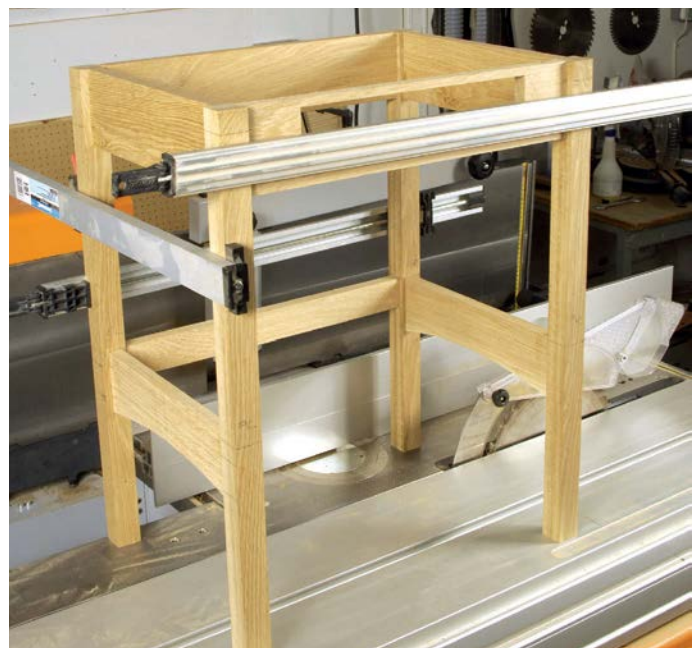
A dry assembly of the overall table minus various infill components to check it goes together properly
