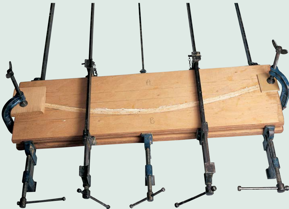
Laminates for the rocker sleds glued up in the jig
