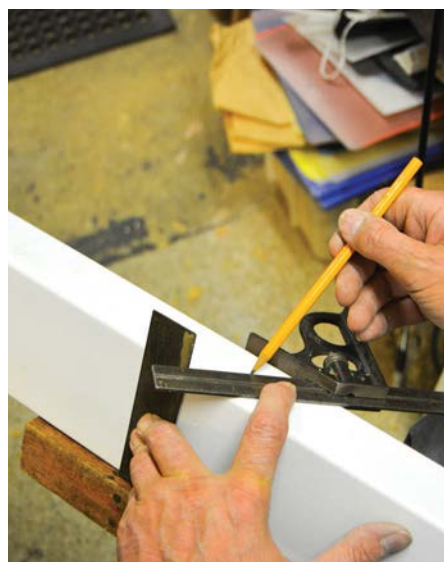
Transfer lines with two squares
