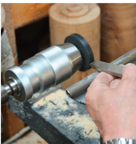
Trim plastic with a trailing scraper
