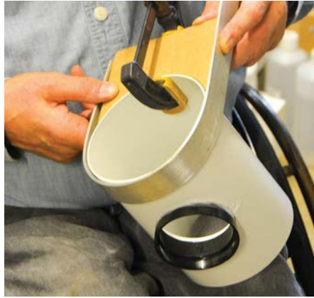
Strap securely, but allow rotation
