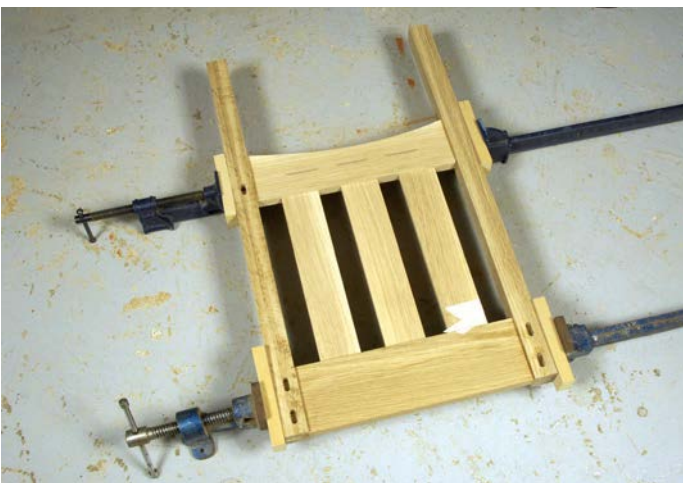
The first sub-assembly, with stub mortises so glue cannot harden at the bottom of the unfilled mortises
