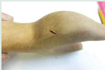
Crack found during carving
