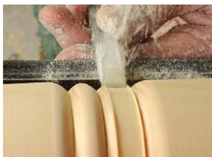
Beading and parting tool cutting a parallel section
