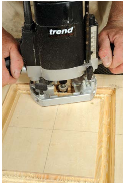
For certain jobs, such as creating a false panel effect, the jig can be a frame so the guidebush only runs against one edge
