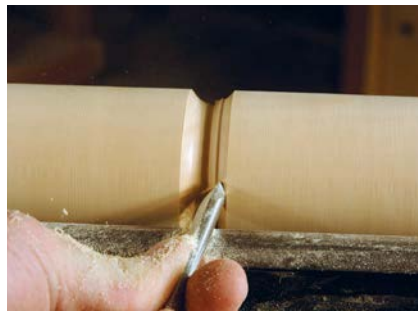
Spindle gouge used for cutting a cove
