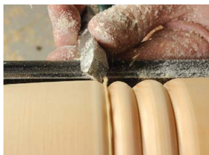
Cutting a series of beads with a beading and parting tool
