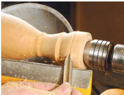
Spindle gouge refining the head of a candlestick
