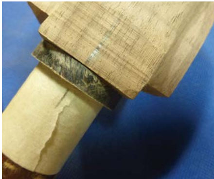
Mark the alignment of the head, spacer and shank where the best fit is achieved
