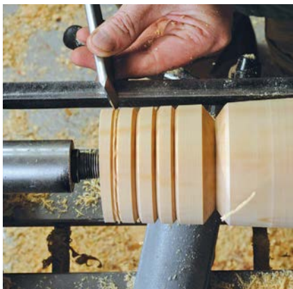
A skew chisel being used to make a V-cut
