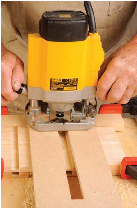
For machining housings or trimming boards a home-made T-square jig with a slot the same width as the guidebush will give easy and accurate machining
