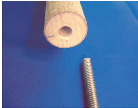
Drill an 8mm hole in the shank
