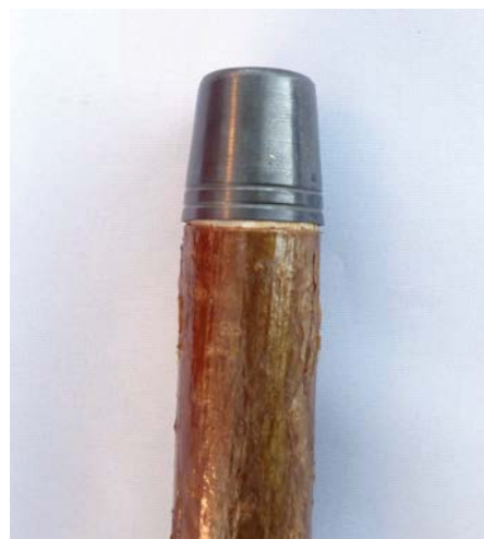
Leave shaping of shank slightly short of the cut mark
