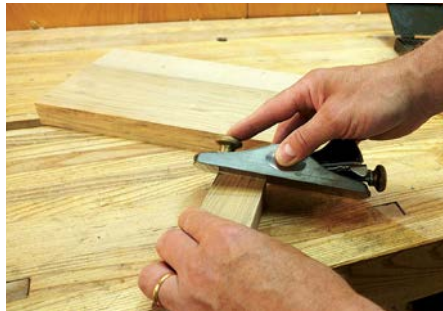
Easing the edges and adding a chamfer
