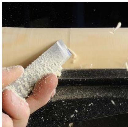
A skew chisel planing smooth the surface of a spindle
