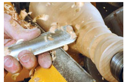
Spindle roughing gouge roughly shaping a spindle
