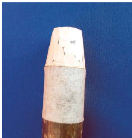
Black marks left by oil residue during manufacture of a ferrule
