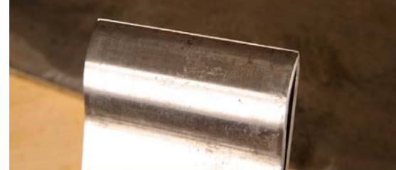
The cap iron is positioned just behind the blade edge so a fine cut is produced and shavings can easily escape
