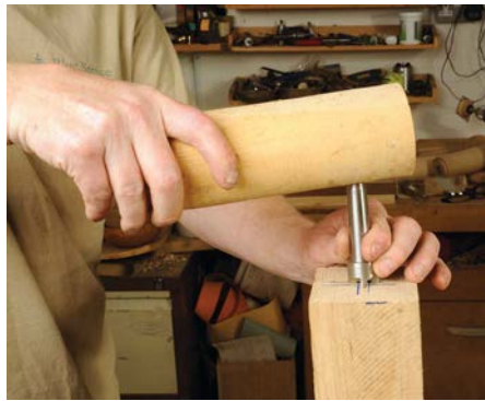
A drive spur driven into a piece of wood with a wooden block/mallet
