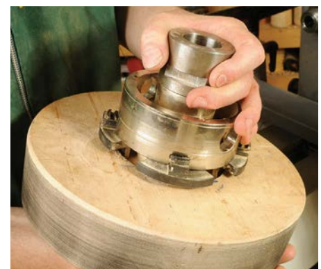
Chuck jaws opening up into a recess
