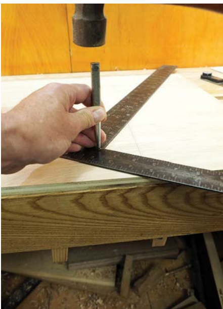
Single sharp blow on the inside corner
