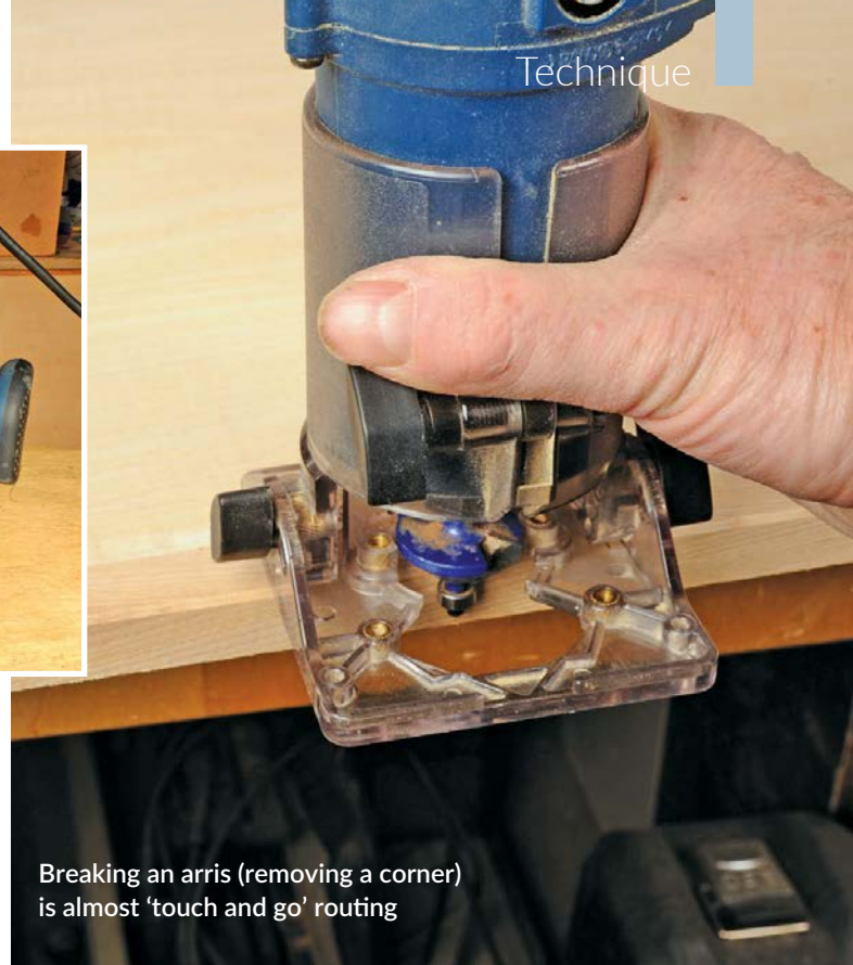
More recently router trimmers have 'grown up', this one is a swap base model turning it into a standard router
