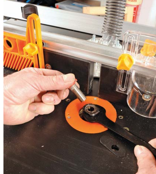
Cutter changing is done above the table
