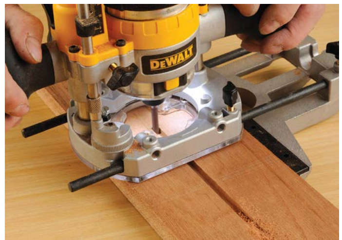
Here the swap base machine is guided by a straight fence for accurate slotting
