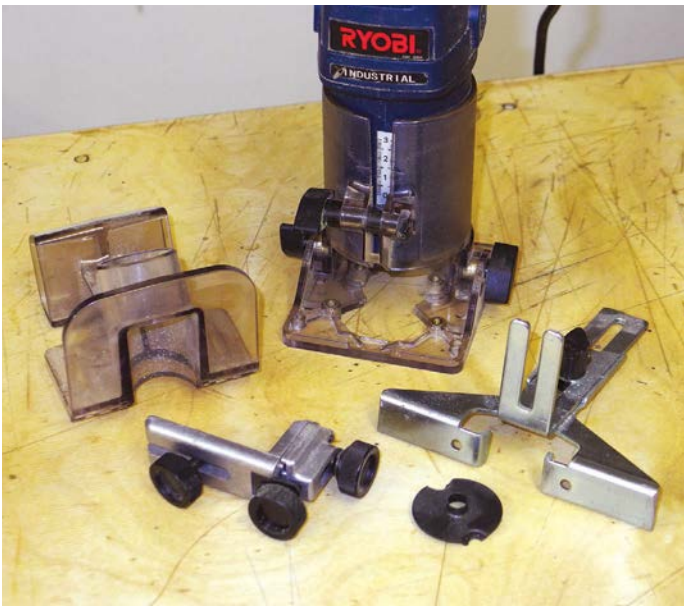
This professional model has everything – fence, roller guide, edge trimming fence and even a tiny guide bush
