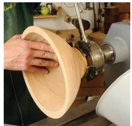
Work about to be held on a spigot
