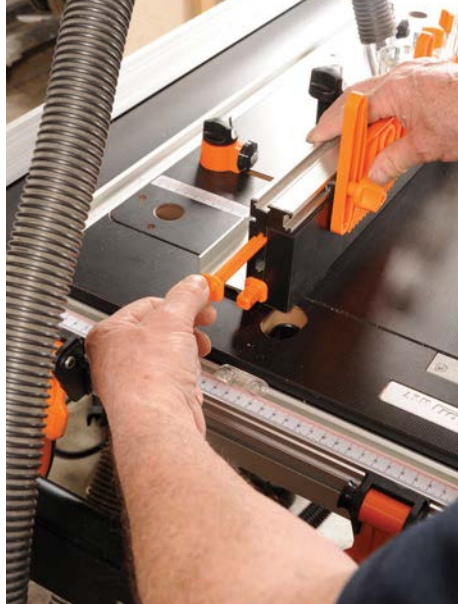
The outfeed fence can be moved forwards by inserting rods
