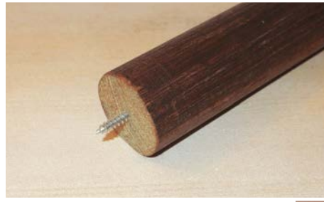
A leg with a de-headed twinfast screw wound into a pre-drilled hole
