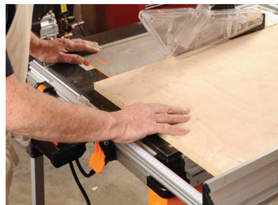
The fence clamps at both ends for sawing
