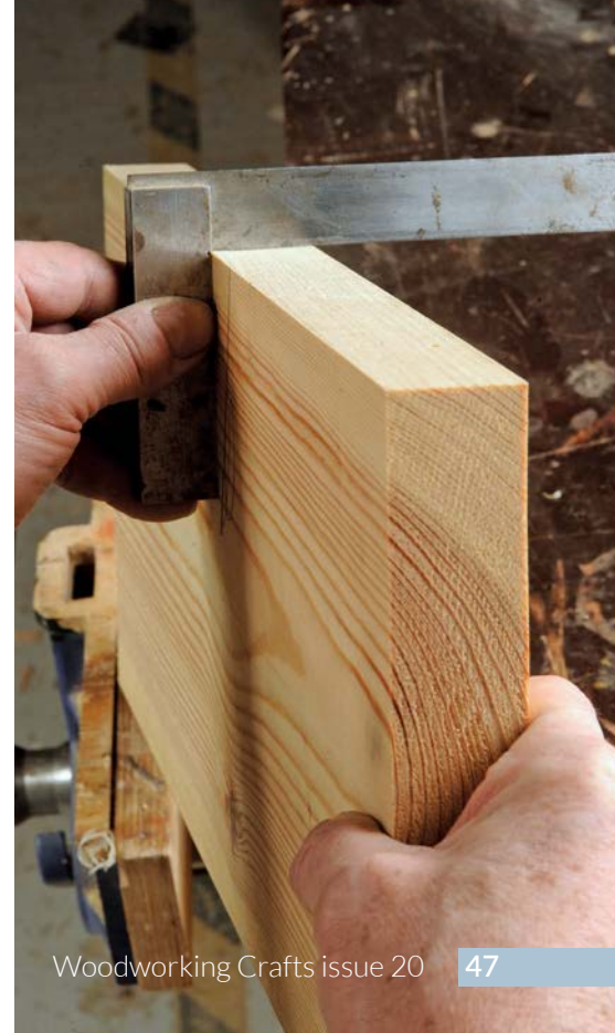
Use an accurate square to check the edge is perpendicular from one end of the board to the other
