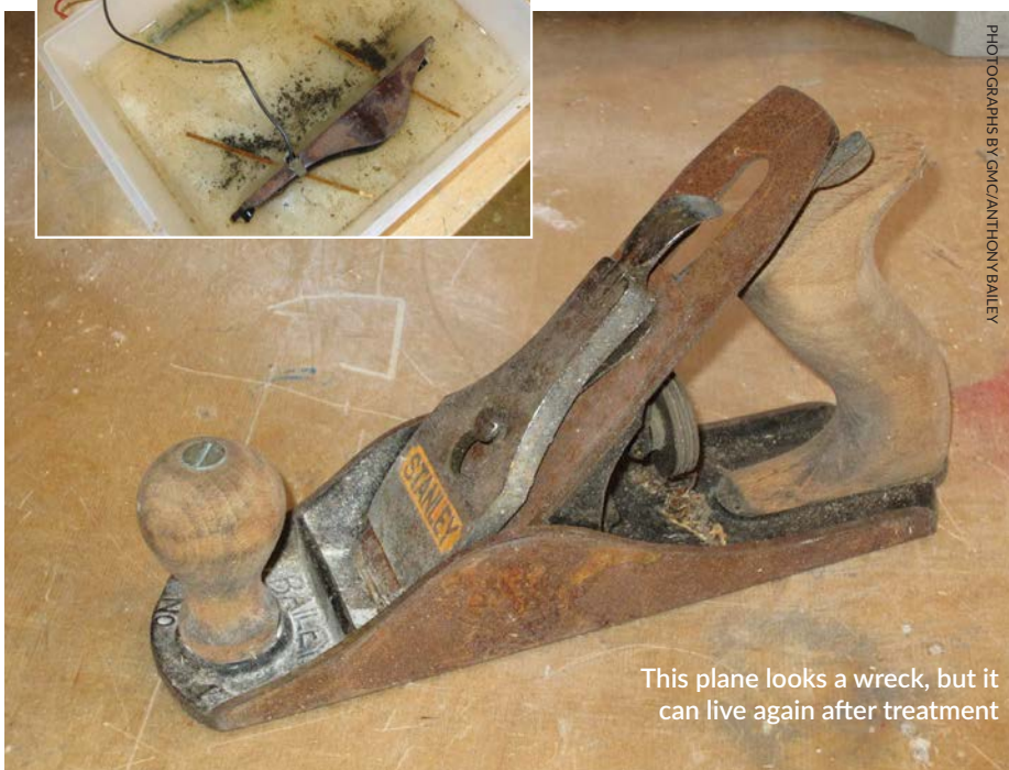
It looks messy but the miracle of electrolysis is removing loose rust and scale from the iron
