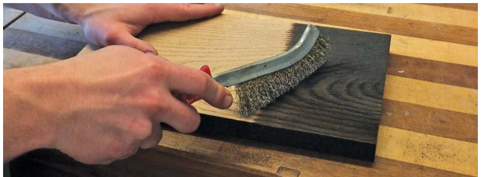
A brass wire brush is great for getting rid of excess and creating a texture
