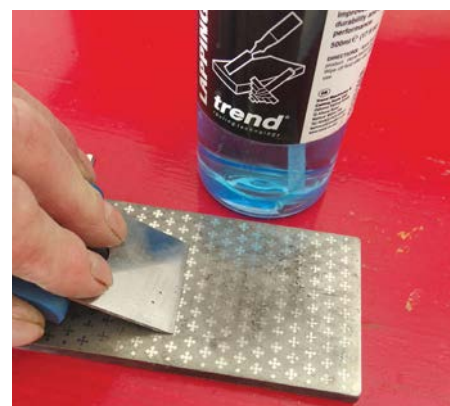
Lapping fluid should always be used with diamond plates
