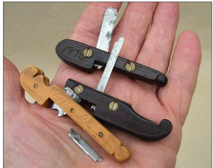
A hand made boxwood miniature scratch stock with a selection of profiled blades
