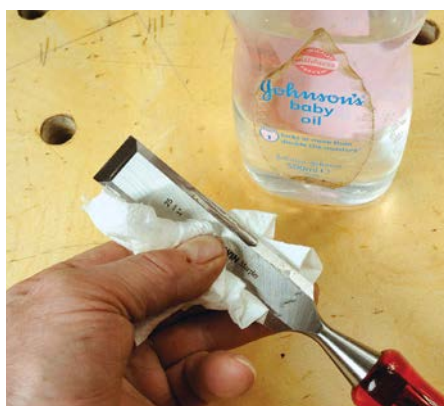
Always wipe tools over with a light oil to prevent rusting
