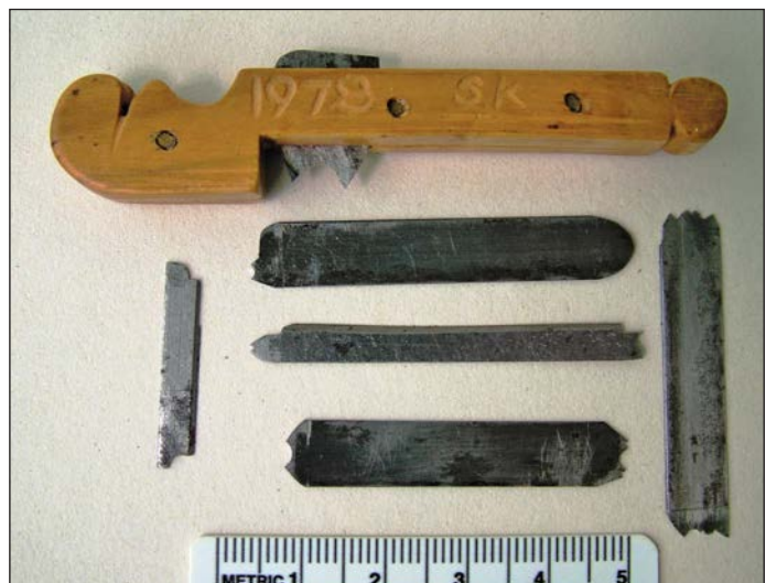
Three scratch stocks made in the early 1970s. It is always a pleasure to make ones own tools and then use them on a project
