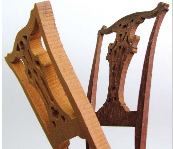
Chippendale style chairs. The back is the integral component and is made in two pieces starting with a strip of long grain glued to one end of the blank for the top rail
