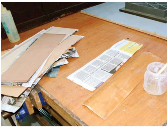
Paper is pressed on to glue covered veneer
