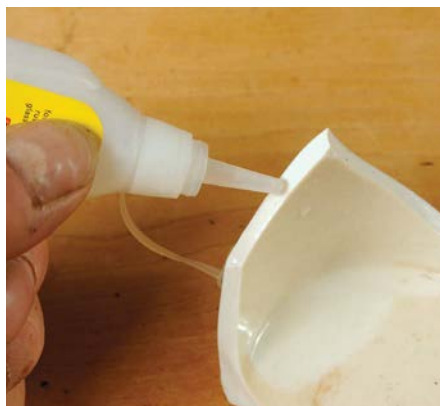
CA glue on ceramic needs water because of porosity
