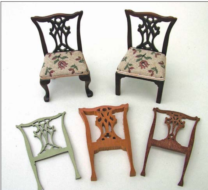
Chippendale style chairs. The back is the integral component and is made in two pieces starting with a strip of long grain glued to one end of the blank for the top rail
