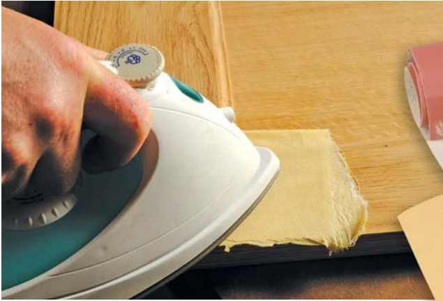
If the wood is dented you can use a steam iron and a sheet of cloth to help remove the dent
