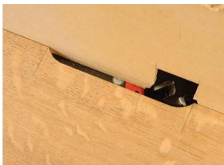
Making the notches is very quick on a router table
