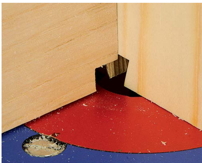
A small cut-out in the stop prevents a build up of waste material and helps with extraction
