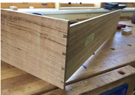
The drawer's back corner has through dovetails
