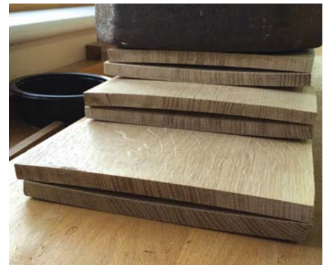
Cupped boards after deeping
