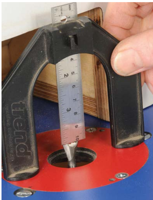
The height required for the dovetail cutter is 12mm. This gauge from Trend takes some of the guesswork out of setting up
