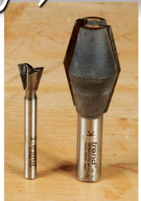
The Trend dovetail shaped cutter is made at 104°, a larger angle than the usual dovetail cutter and it has a 1/4in shank. The matching butterfly spline cutter has a 1/2in shank and is 46mm in length
