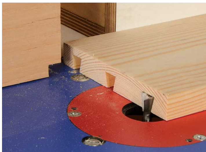
No extra support is required when creating the dovetails while working flat. The fence can be adjusted across the router table after each of the components have been machined at that setting
