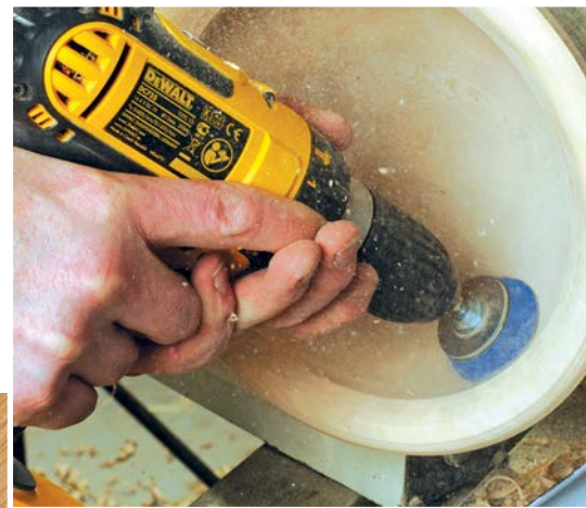
Above: Sanding on turnings is normally done with the work rotating, which is easier and gives a more consistent finish than static sanding
