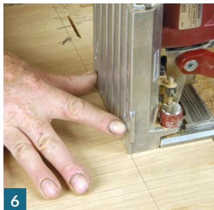
Making the '0' biscuit slots for the carcass bottom
