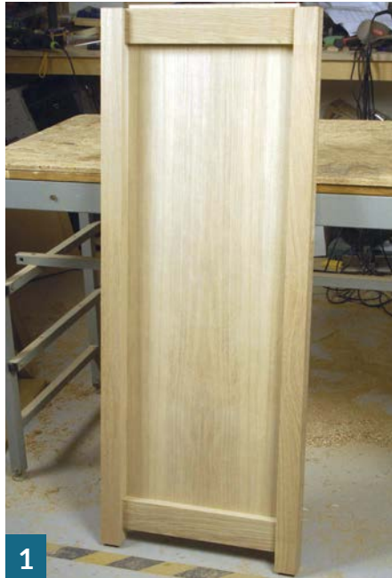
1 The assembled end panel; note the 10mm upstand
