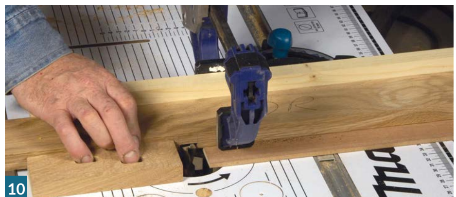
Cutting a drawer stile housing
