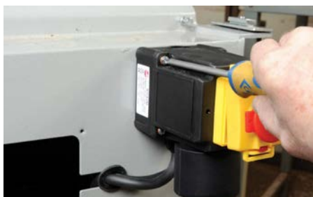
The switch block is flipped out of the casing before screwing in-situ
