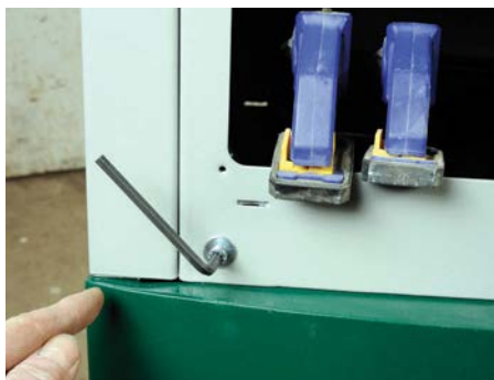
I used clamping to align the Allen bolt holes
