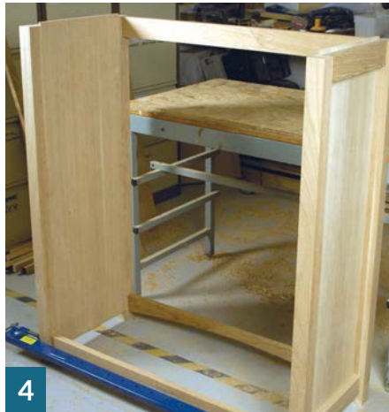
The carcass dry-assembled in order to measure up the drawer rails
