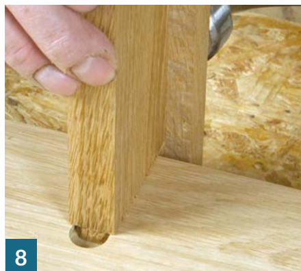
A trial assembly of a housing joint
