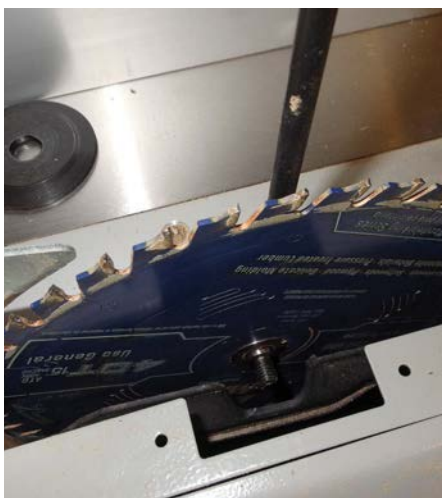
There is a risk of the arbor washer and nut disappearing down the chute
