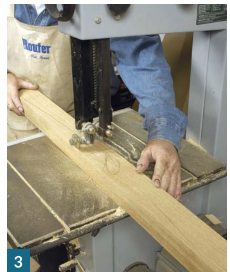
3 Pack-cutting: both lower rails are held together with double-sided tape
