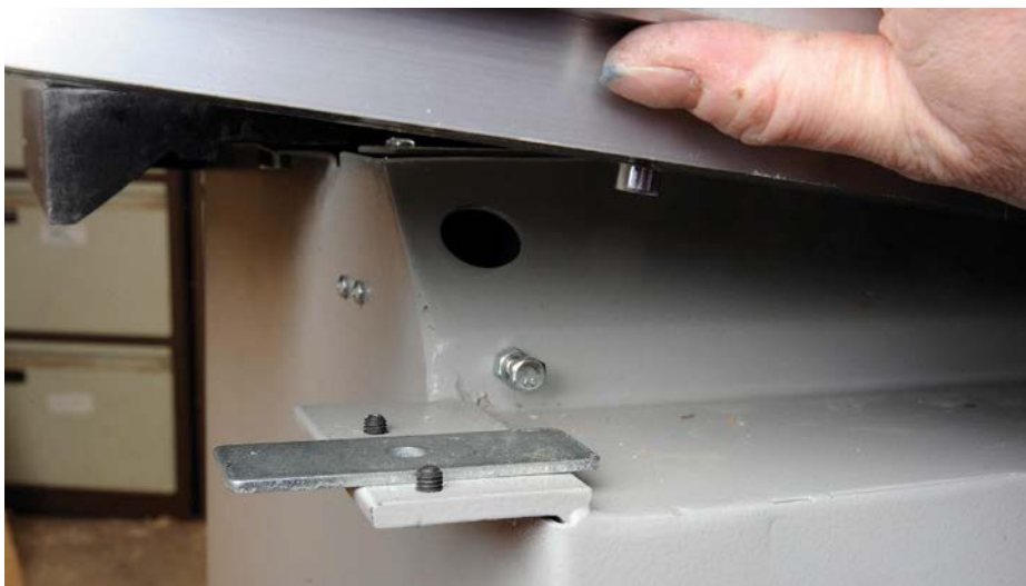
The sliding table sits on adjustable grub screws, the packing pieces in-between not needed
