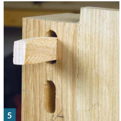
A narrowed-down Domino is easier to extract when test assembling
