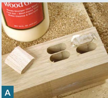
A Fitting Dominos cut in half to make the repair
