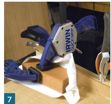
The glued-up carcass bottom and rail; note the block used to keep it square
