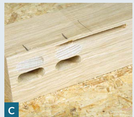
C Almost invisible and strong repair
