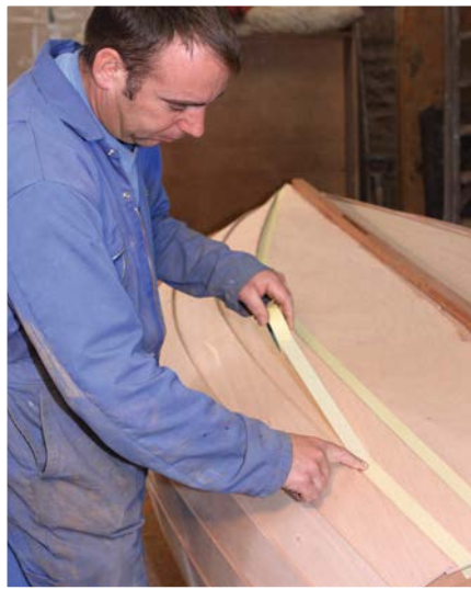
Masking along the pencil lines to keep a clean epoxy line
