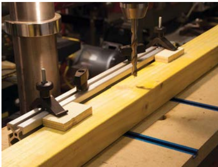
For accuracy and neatness I drilled the holes using my pillar drill
