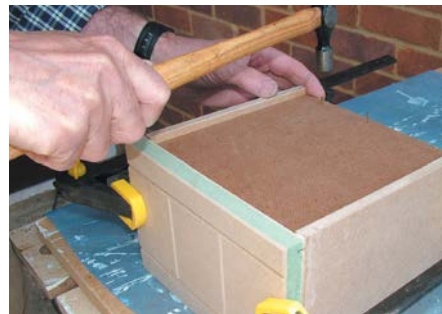
The drawer bottom slides into grooves and is pinned in place to add further rigidity to the drawer box
