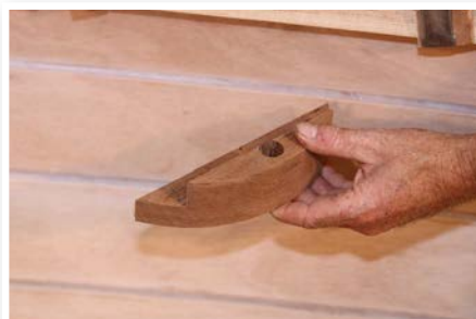
A drilled rowlock chock prior to installation
