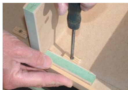
The drawer stops are fixed at this point while good access is available
