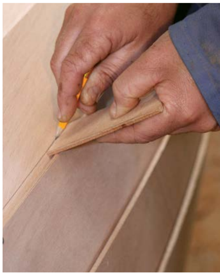
A scribe line to show the limit of the epoxy filler
