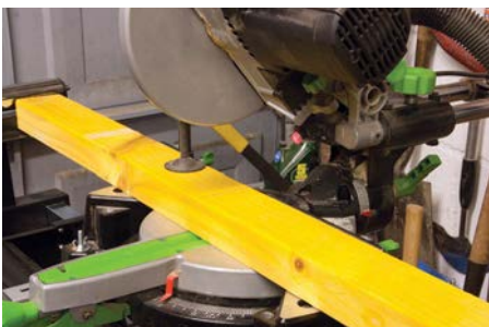
The chopsaw proved invaluable for fast and accurate repeat cutting to length
