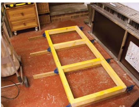
The frame was clamped up square and the pocket screws driven in
