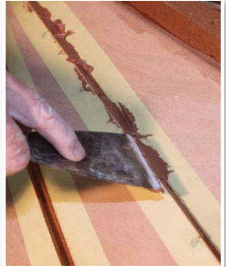
Applying coloured epoxy filler using a broad knife
