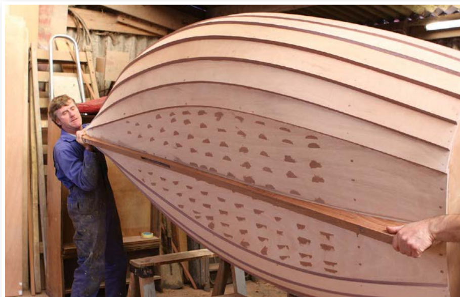
The dinghy has to be turned over to fit the bilge rails
