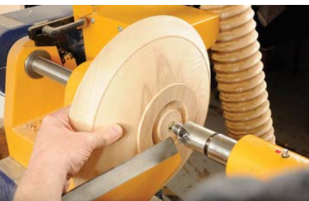
Bring up the tailstock revolving centre to support the work
