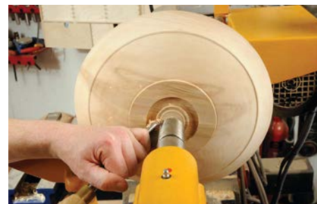
Turning away the majority of the waste wood and cleaning up the base
