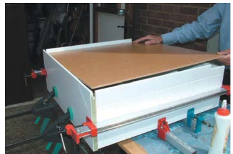
The carcass back fits into a rebate, and helps keep the unit square
