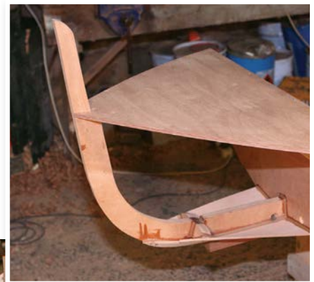
The dinghy starts to take shape with the addition of the transom and aft (rear) bulkhead
