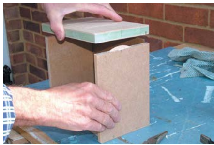
The drawers are a simple box construction with the fronts biscuited on
