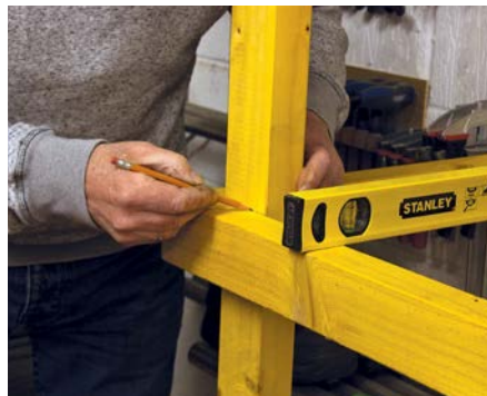
Marking the legs for each position taking account of floor variation
