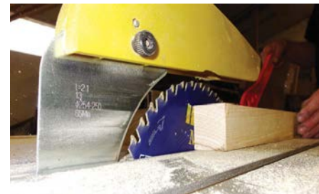
A rip blade is fine for fast cutting in deeper stock
