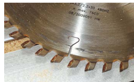
A finer tooth general purpose blade gives a better finish
