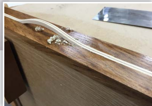
Top: The drawer front routed, awaiting assembly
