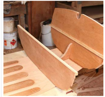
The dinghy starts to take shape with the addition of the transom and aft (rear) bulkhead
