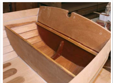
Resin has been applied to the inside of the aft buoyancy tank to prevent future problems with rot
