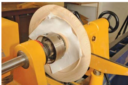
Place the work against the covered friction drive
