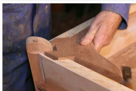
Offering up the breast hook to check the fit
