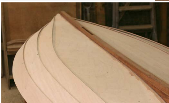
The planks are held in place by a mixture of temporary and permanent fixings, ready for creation of the epoxy fillet joints
