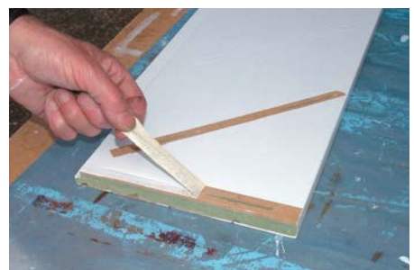
All components are painted before the final assembly, and masking tape used to ensure the mating surfaces will take the glue efficiently
