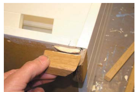
The oak feet of the unit are mitred and biscuited into place
