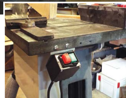
A new motor and modern no volt release switch fitted to this sawtable
