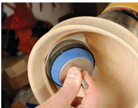
You need to get as much surface contact as possible to ensure a nice even curve without ridges
