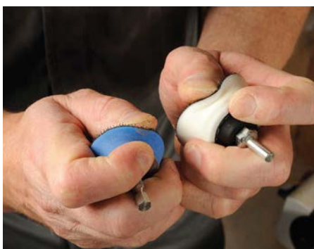
Sanding arbors – which are fitted into a drill – onto which is affixed abrasives, available in various sizes and densities
