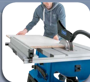
Solid table extension for cutting large boards
