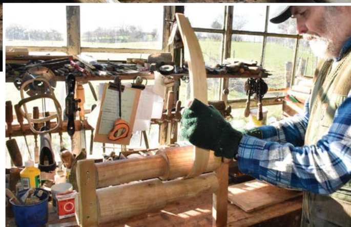
Right: Passing willow boards through the manipulator
