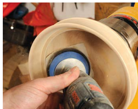
The curved internal profile being power sanded. With any sanding make sure you extract the dust properly
