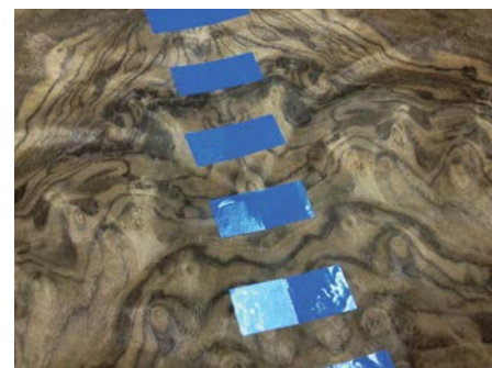
The joints were held with veneer tape
