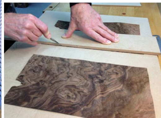
The veneer was cut and jointed together
