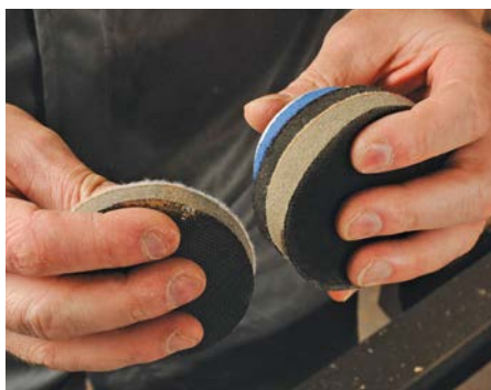
You can buy soft interface pads to fix on to sanding arbors that enable you to alter how the arbor fits against the work
