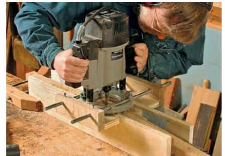
Then cut the mortise with a plunge router.
