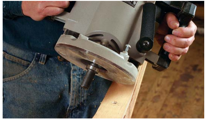
... a shorter bit requires you to flip the jig and make two passes
