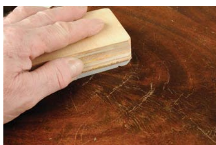
Using a foam-backed fine abrasive to take away the roughness where the grain has raised slightly
