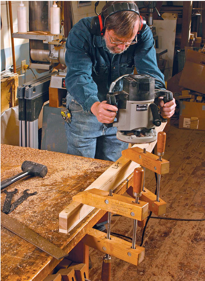
Clamp the jig to a bench to rout the leg shape. A long bearing-guided bit can do the job in one pass...
