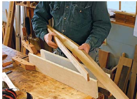
Angle block orients the leg at 85.5°. Set the block against one side of the leg before adding the wedges.
