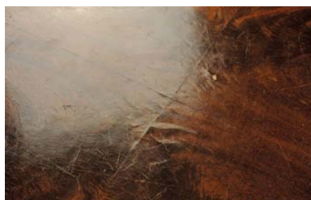
Lifting veneers and a missing fragment
