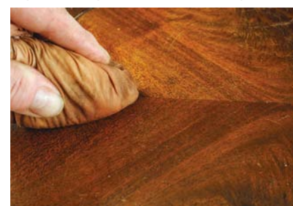
Applying a button polish using a traditional 'rubber' working in circles, figures of eight and finally straight strokes
