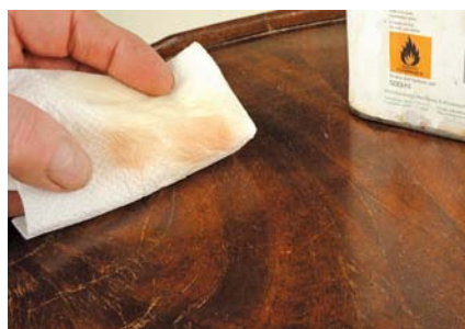
Testing to see whether the finish is French polish or cellulose lacquer – apparently it is lacquer as the reaction was minimal
