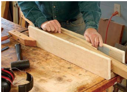
Wedge leg in box for mortising. Adhesive-backed sandpaper prevents the wedges from slipping.
