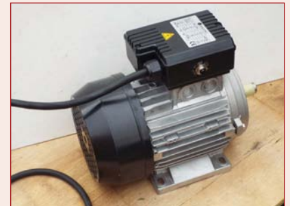
New 2hp motor with built-in reset button on the top box
