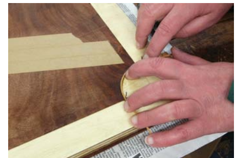
Square white line being shaped to the corner
