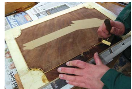
Veneering the cross-banding into place
