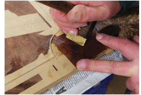
Squeezing the glue out through the joint
