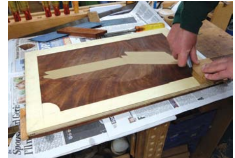
Trimming the corners to a template
