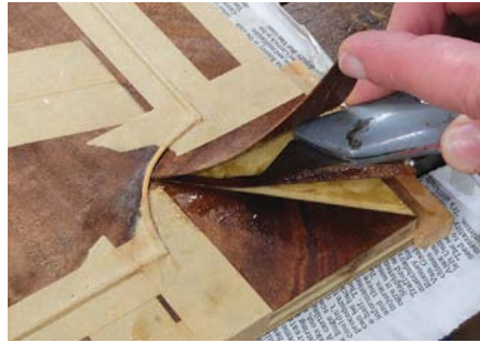
Lifting the top corner piece to remove the waste piece below
