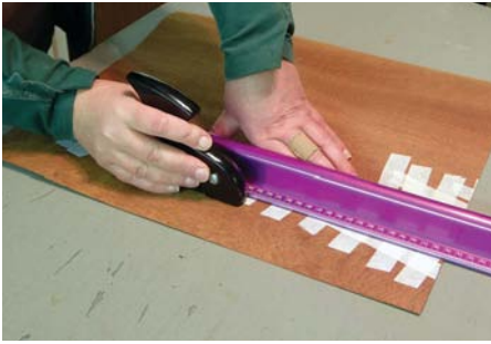
Cutting the counterbalance veneer
