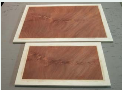
The flame veneer, oversize and pressed into place ready for the edging
