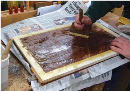
Laying the veneer with the veneer hammer
