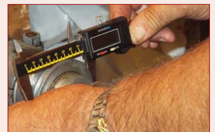
Measuring the machine drive pulley size to calculate the motor pulley size
