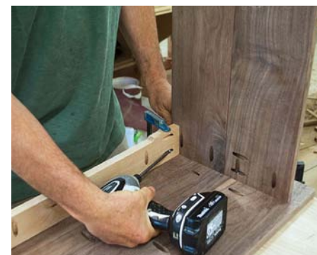
Drive the screws through the skirt into the bench end, starting with the bottom screw, which is backed up by the 1in spacer
