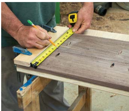
Mark the center of the benchtop in front of the spacer to help align the bench ends
