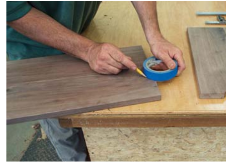
Use a roll of tape to help draw the curve in the bottom edge of the bench end
