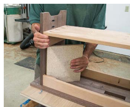
Hold the upper spacer in place as you slide out the lower spacer to keep from scratching the top of the shelf
