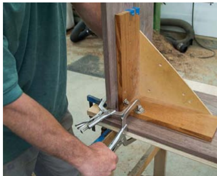
Secure the right angle jig to the bench end with a face clamp, being careful not to cover up the first pocket hole. Then face-clamp the jig to the benchtop
