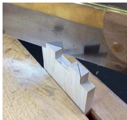
The saw kerf must go exactly corner to corner
