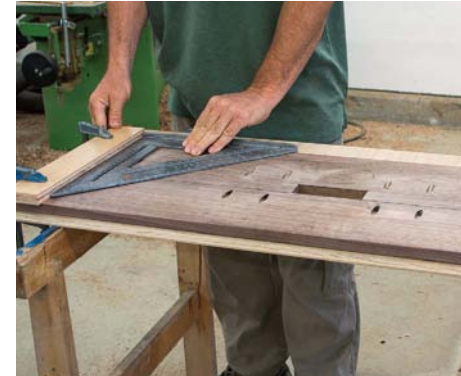
Square up the scrap spacer with the front edge of the bench
