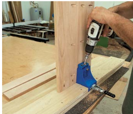
Drill one pocket hole at each end of each slat to attach the shelf to the bench ends
