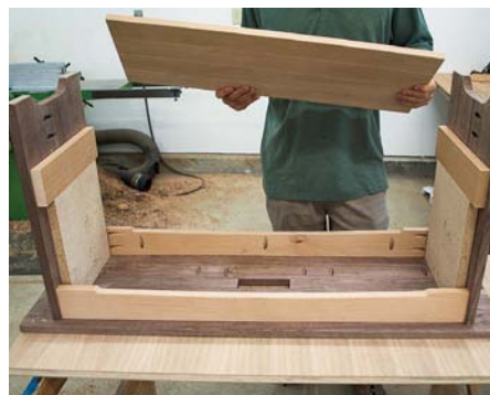
To install the shelf, make a pair of spacer jigs to support it
