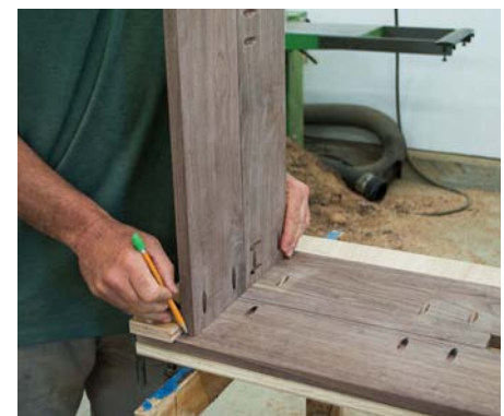
Mark the edge of the bench end, which should be ¾in from the front edge of the top
