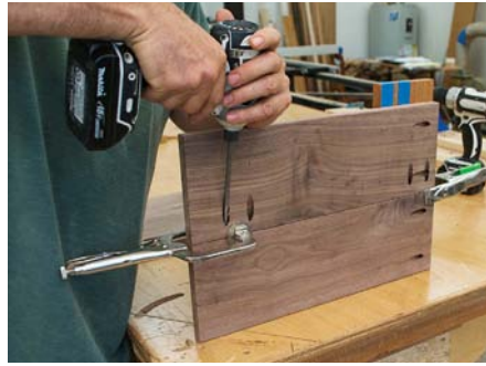
Center a face clamp over the seam between the end pieces as you drive the pocket screws
