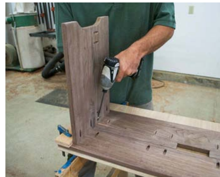
Drive the first screw into the end, remove the right-angle jig, and finish screwing off the end to the top
