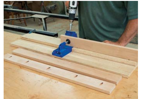
Use the marks on the slats to align them on the jig for drilling
