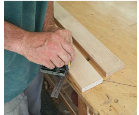
Use a square to mark the 45° start of the curve on the lower edge of the skirt
