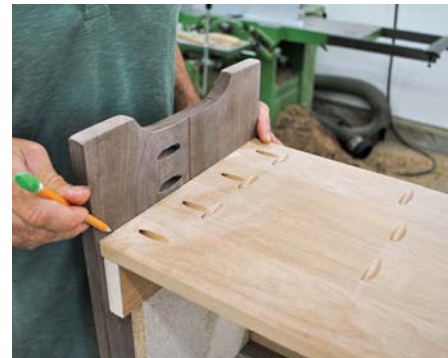
Mark the location of the shelf at the front edge so that you can verify that the shelf did not shift when clamping the right-angle jig in place
