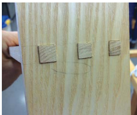
Checking the through tenons are a perfect fit before fitting wedges
