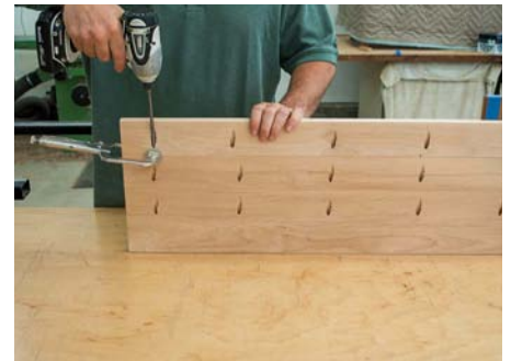
Continue adding the shelf slats until all four are in place
