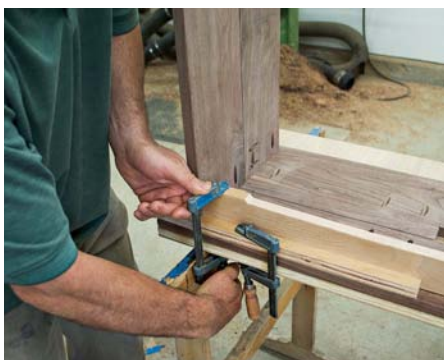
Clamp a 1in spacer to the benchtop, then butt the skirt to the spacer and clamp in place
