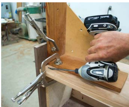
Clamp the right-angle jig to the shelf and bench end so that the first pocket hole is uncovered
