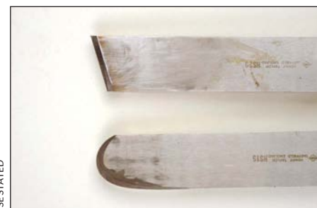
Two 25mm wide scrapers, one skewed angle the other with a French curve
