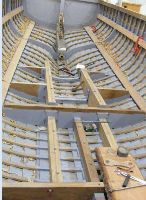
Above left: The ribs rebuilt and in position. Above right: Awaiting deck boarding. Below: Detail of the carvel planking
