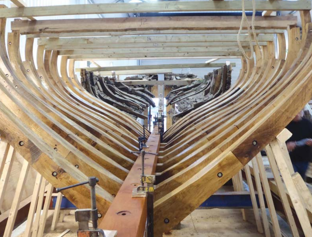
Above left: The ribs rebuilt and in position. Above right: Awaiting deck boarding. Below: Detail of the carvel planking
