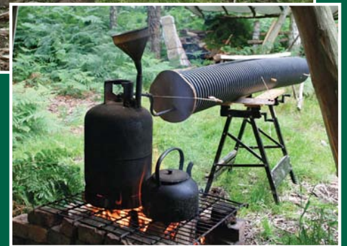
My setup for steam bending
