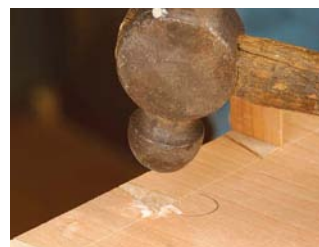
Peen small gaps. Small gaps can be filled by inserting a little glue and then hitting the pin or tail with a ball-peen hammer. Do this before planing the pins flush so that the hammer marks can be removed
