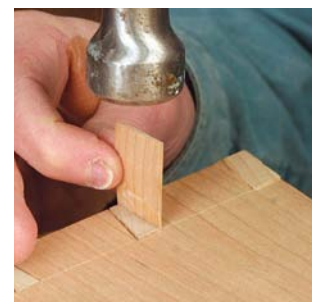
Shim larger gaps. A narrow wedge driven into the gap beside a pin will make an almost invisible end-grain repair
