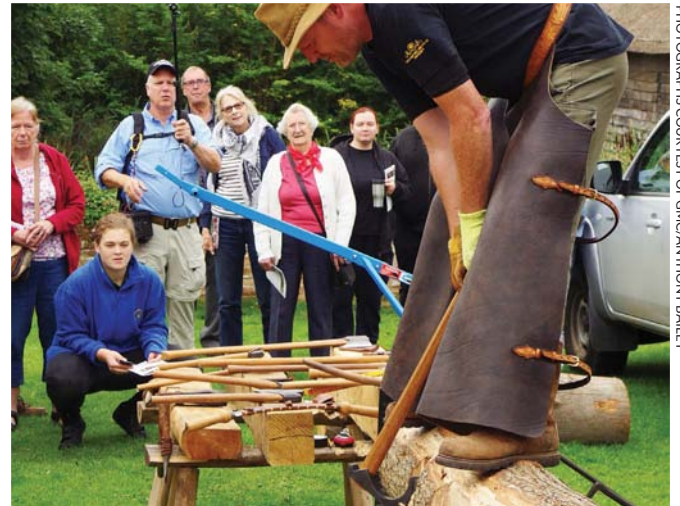
Steve Woodley on top form dividing the trunk side before smoothing with a side axe
