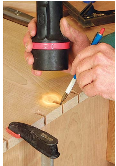
Mark the pins from the tail. With the boards secure, use a sharp pencil to transfer the location of the pins. A torch helps you see into the corners
