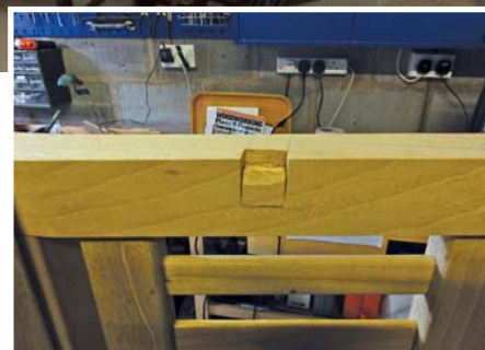
Partway through chopping out the recess to take the arm
