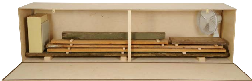
A dehumidifier cabinet is very easy to build and can be made to fit under a bench
