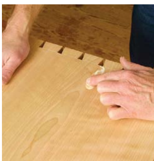
Repair a crack. While flexing the board up and down, force glue into the crack
