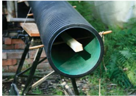
Supports raise the wood to the top of the steam box
