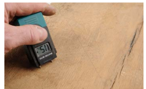
A moisture meter will show the moisture content of wood during drying
