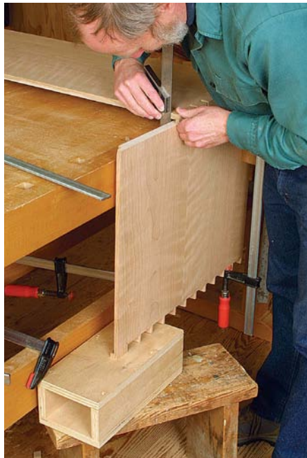
Line up the boards. Before laying out the pins, ensure that the boards are flat and meet at 90°
