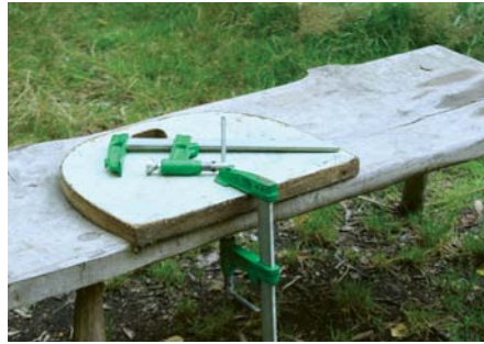
Here I have the second clamp ready to secure the piece of wood when I take it out of the steamer
