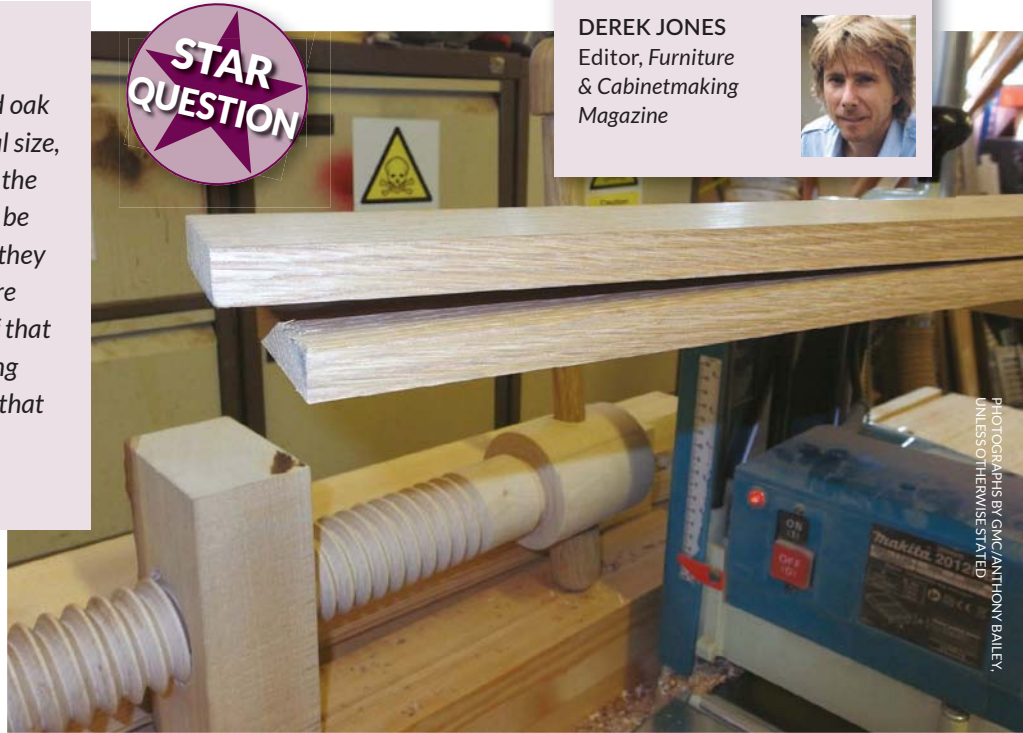
Splitting timber, like oak, down the middle often results in bowed pieces like these
