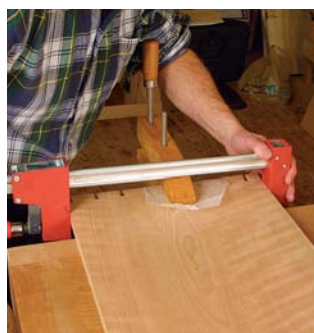
Use one clamp to keep both sides of the crack aligned, with waxed paper between the glue and clamp, then close the crack with another clamp across the board
