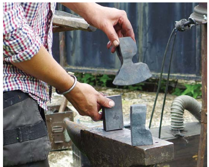
Nic Westermann demonstrating the stages in forging an axe head from a blank piece of steel
