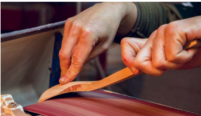
10. Use the belt sander with a coarse grit to shape the spoon's curves
