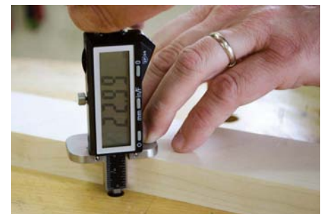
Digital marking and mortise gauges are very easy to read
