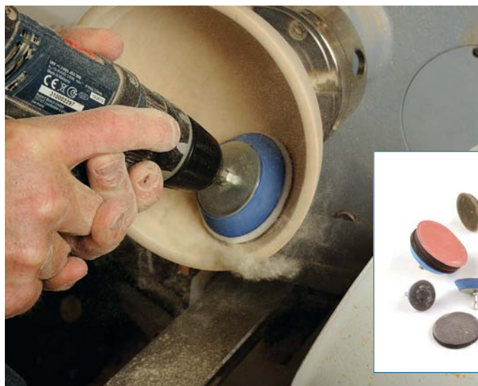
Power sanding a bowl interior Inset: There is a wide range of sanding arbors available
