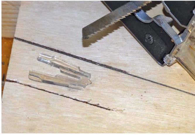
Detail of a cut using the splinter guard compared to a cut without the guard
