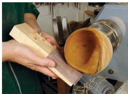
A block with abrasive wrapped around it is great for sanding natural-edges
