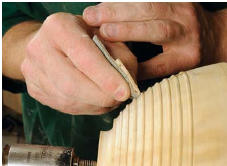
Folded abrasive allows you to access details easily
