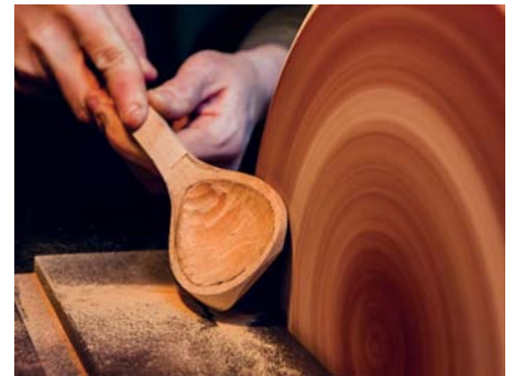
9. Shape the outer part of the bowl on the disc sander
