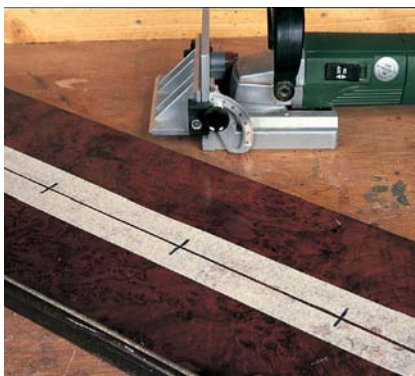
The surface needs to be protected with low-tack masking tape
