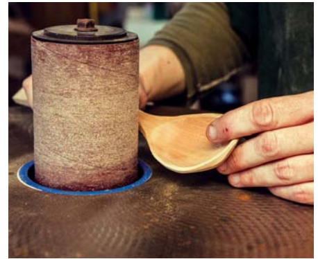
13. The spindle sander gives the spoon its start towards fine sanding and refined shaping
