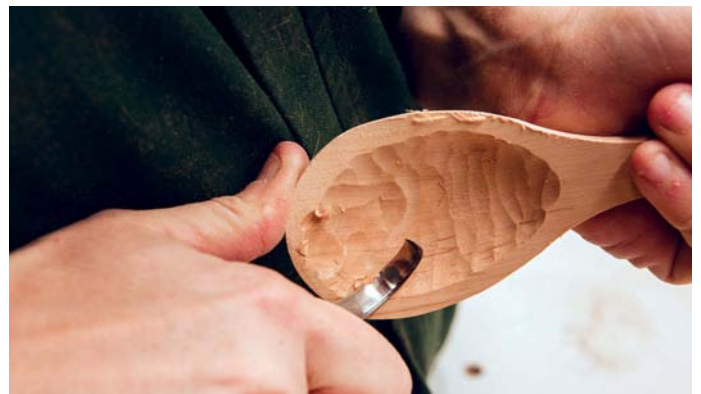
11. Refine the inside of the bowl with a gouge or crook knife
