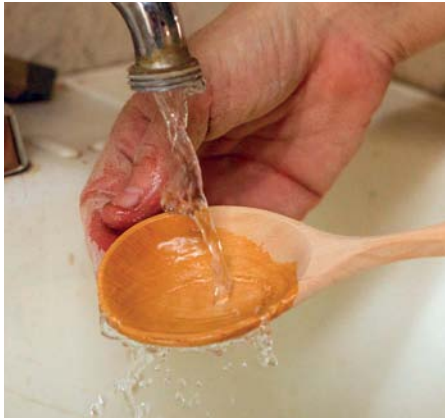
16. Raise the grain between sanding grits by running the spoon under water
