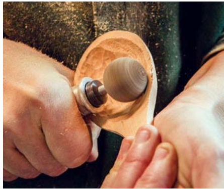
12. A Kutzall grinding burr will easily remove the marks left by the gouge
