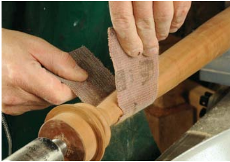
Using the two-handed sanding technique to sand a spindle
