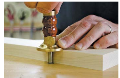
The WoodRiver gauge has a thicker stem and doesn't roll off the bench
