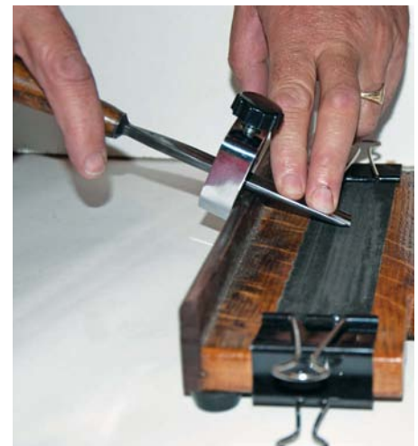
This jig presents an easy, predictable way to sharpen your gouges
