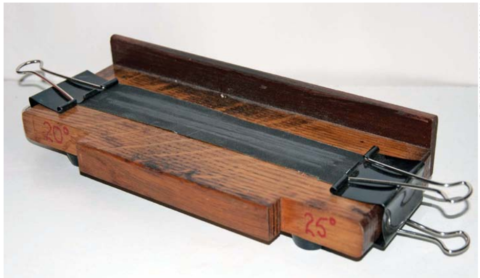
The completed sharpening jig with angle setting recess
