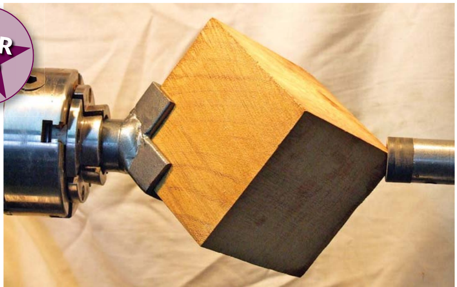
Phillip's driving dog allows him to grip a cube of wood between centres
