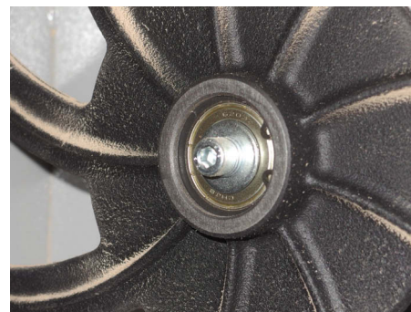
Each bandwheel has a bearing, which is replaceable
