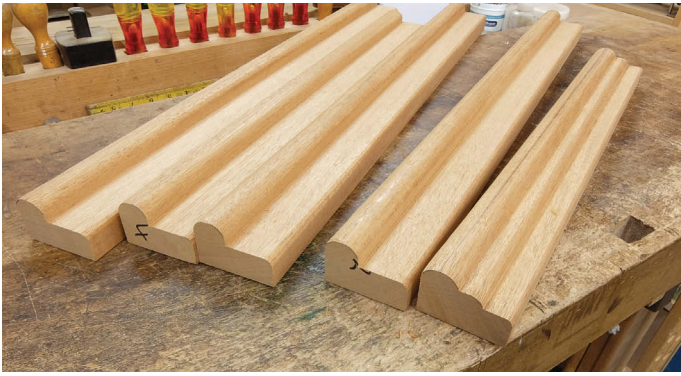
Four sections of moulding awaiting their cover piece, left, and the complete section, right
