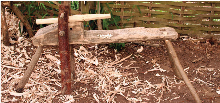
A different shaving horse design with one piece body. It's good for travelling with a shorted body and less parts to transport
