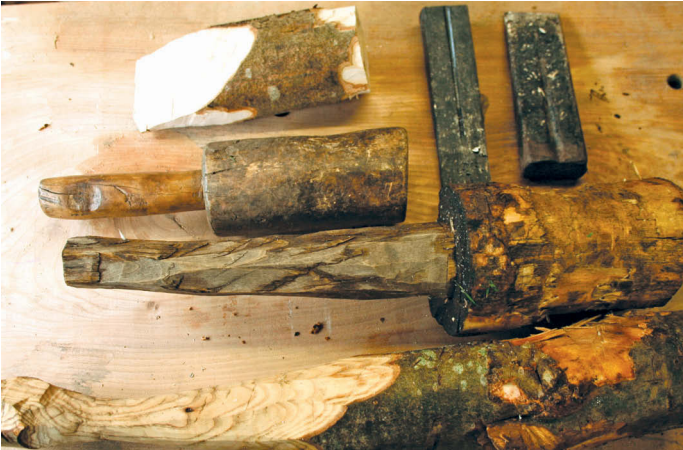
Clockwise from top: a wooden glut; two metal wedges and three mallets – note the tapered handle of the bottom one
