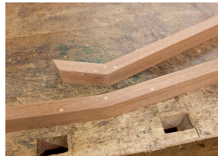
The two sections of curtain track glued and pegged
