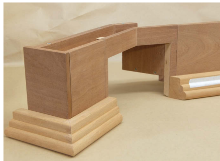
The moulding fitted around the section to the right of the lintel
