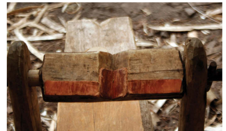
The top bar of the shave horse can be modified to suit what parts you are working. The flat surface and groove reduce sideways movement of billets and the leather reduces slippage
