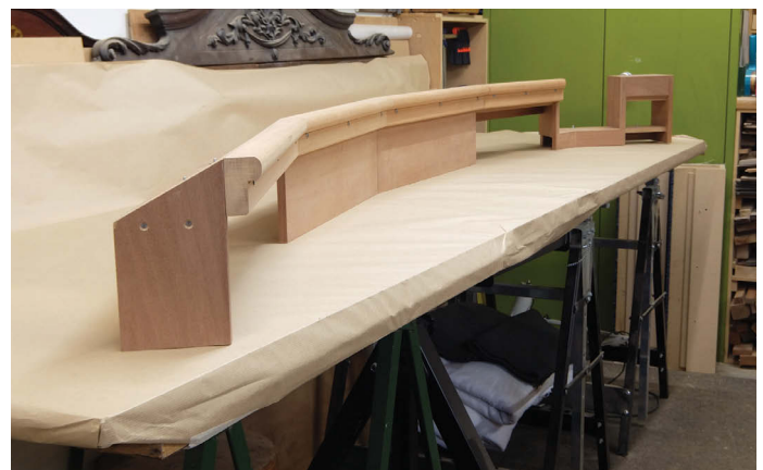
The four sections fitted with the machine screws visible
