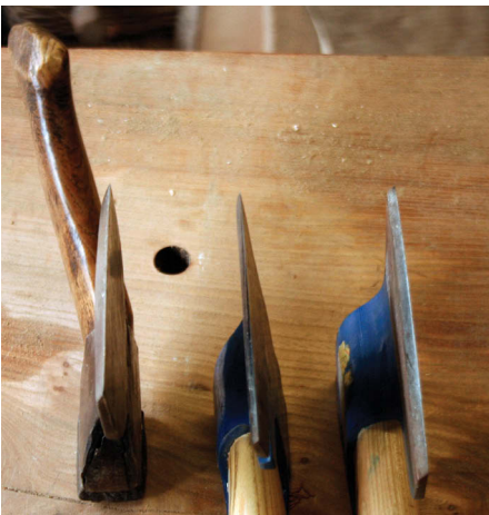
Three side axes: one left-handed with a cranked handle
