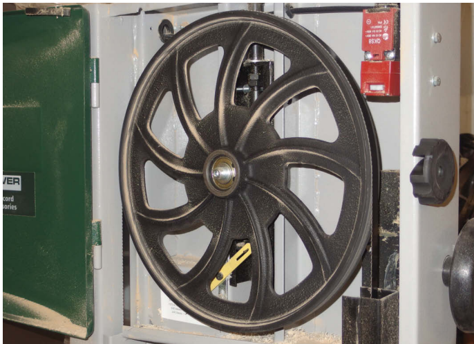
A typical upper bandwheel – note the curved spokes
