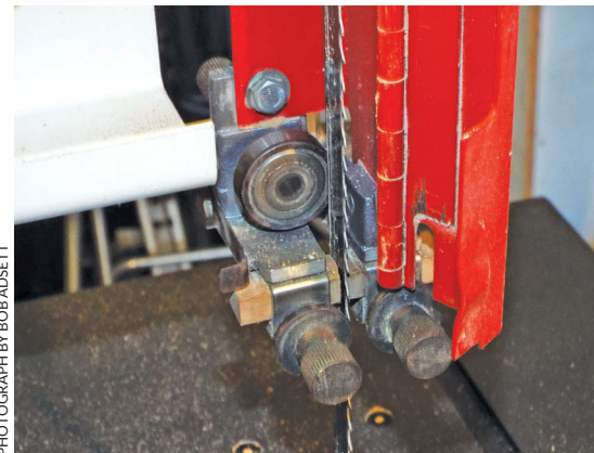
Older machines sometimes had wooden guide blocks
