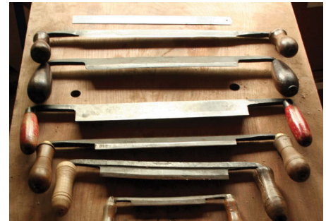
A series of drawknives – note the variety in size, different shapes of blade and handles
