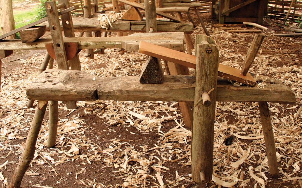
Traditional shaving horse. The wedge has three sides of different lengths so can be turned for adjusting for different sized billets
