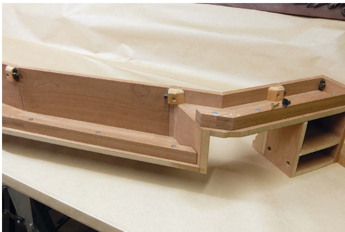
The lintel section – upside down and from the back – showing the clips and blocks to hold the loose panels
