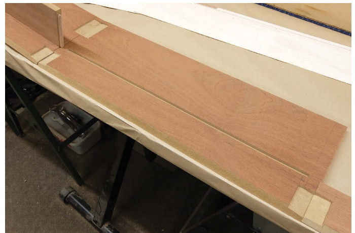
Section 3 – centre, section 4 to right and section 2 to left, showing the dovetail keys to join the sections
