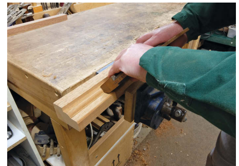
Cutting the middle section and changing the angle of the plane to flatten the quadrant
