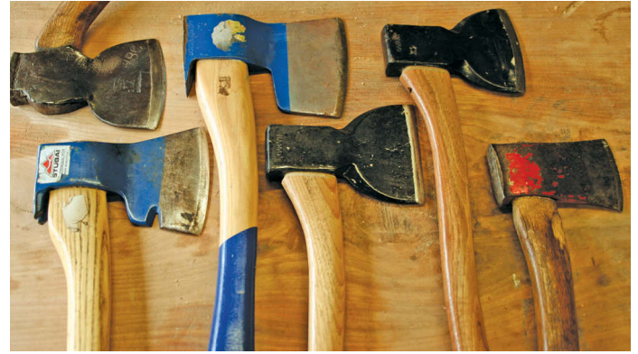
Axes for splitting and shaping. The first five are side axes; a left-handed at the top; two blue Austrian axes; two Kent pattern side axes – note the curved reground blade, which works better, and a simple splitting axe for cleaving
