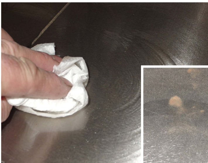
Oiling the cast-iron – left – avoids rust prints – below
