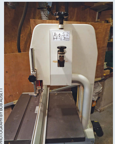
The rigid tubular steel arm on the back of a Kity 613
