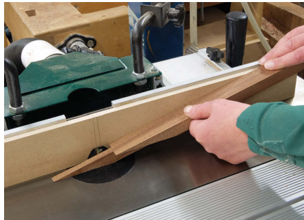
The first half of the finger joint being cut
