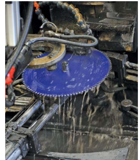
One of the grinding machines shaping the teeth
