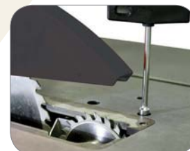
Height & side setting of the scoring blade conveniently accomplished with the tool provided.
