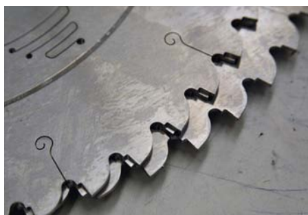
Blade detail, left to right: noise reduction slots; tension ring; expansion slots; tooth gullet and seat for tips
