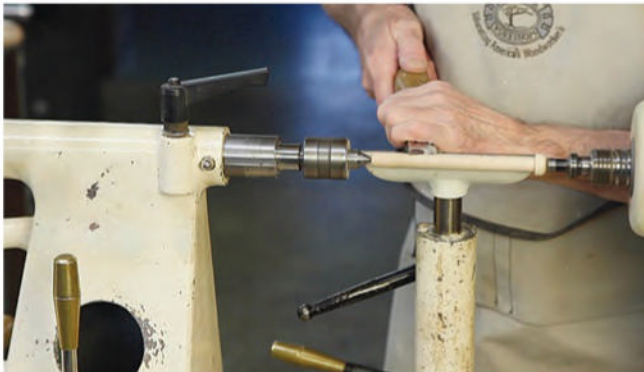
Most of the trunnion shaft needs to be turned at least 1/32" under 1/2" for a sloppy fit in the handle so the handle will rotate on the pin even when soaking wet and swollen. The last 1" has a 1/2" diameter to be a slide fit with the hole drilled in the main cylinder.
