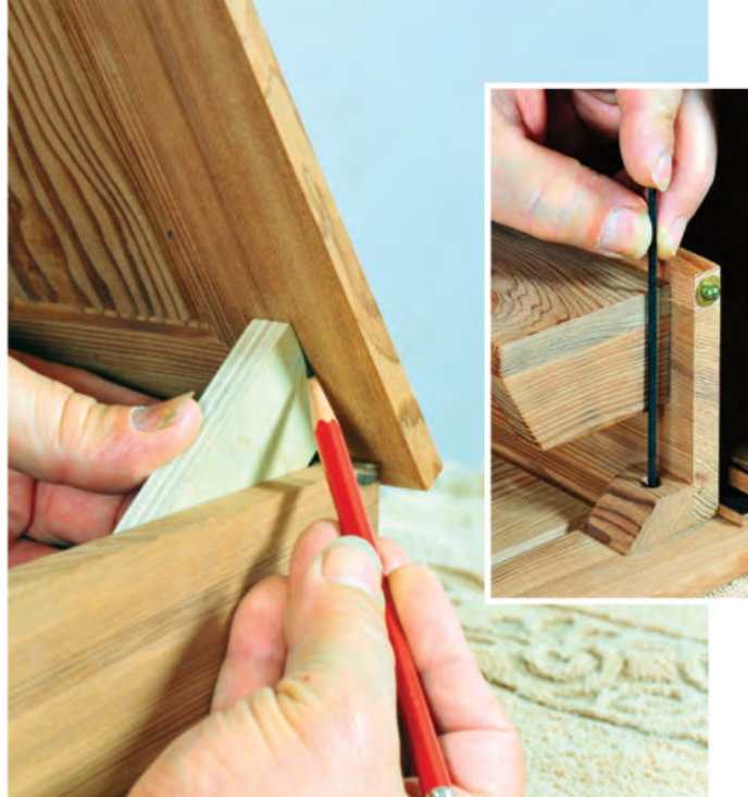
To prepare for mounting the bottle lifting mechanism, the inside edges are marked on the underside of the lid. The mechanism is then positioned between the lines and the holes are marked for mounting screws (inset).
