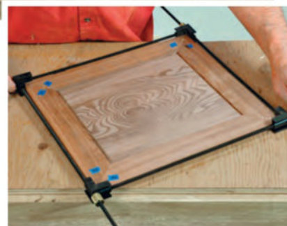
The author used a quick-release frame clamp to draw the mitered corners of the lid's frame together. After spreading glue into each biscuit and its corresponding slot, the frame members were assembled around the raised panel and each corner of the clamp tightened (inset).
