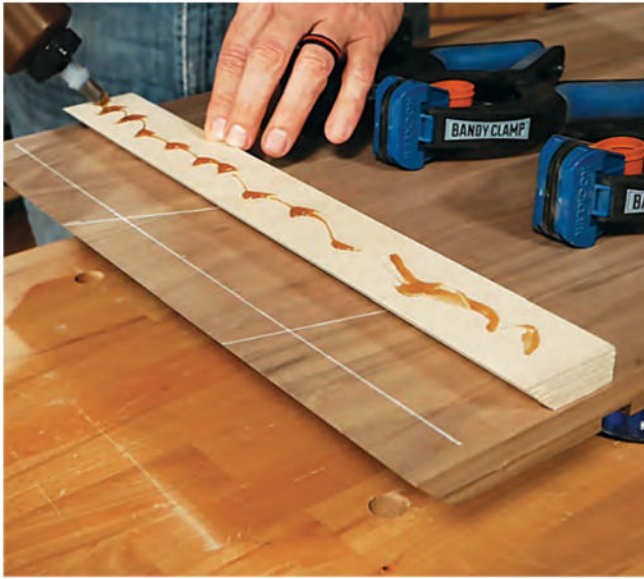
A thin bead of liquid hide glue attaches the temporary clamping cauls to the carcass components. These cauls will then be easy to break loose without damaging the wood. Simply scrub away the dried glue.
