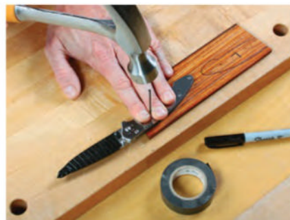
Trace the scale shapes and mark the screw hole locations with a finish nail or drill bit. Wrap the blade with thick tape first to protect yourself.
