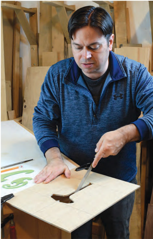
Shape the ginkgo leaf template with flat and round files. Make sure the stem portion of the design is at least 7/16" wide.
