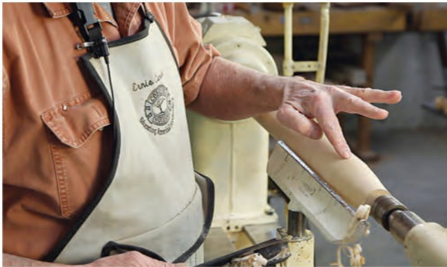
The French baguette pin tapers, starting 4" from each end, to about 1" in diameter. You should be able to set a ruler down and have it touch everywhere on this straight taper.
