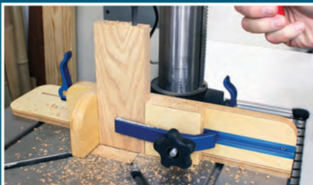
For more holding strength, install a hold-down clamp underneath the star knob on the sliding stop. For wider workpieces, flip the sliding stop and hold-down clamp as needed. Because the hole for the star knob is offset on the sliding stop, the blue hold-down clamp can be flipped 180 degrees to accommodate differently sized stock. When drilling shallow holes, you can remove the hold-down to speed up your drilling.
