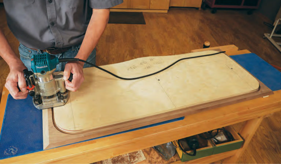
Plowing the track that the tambour doors will slide in requires a template to guide the cut. Screw the template in place for routing.
