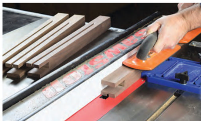
Reset the rip fence for a centered cut on the legs, and make one stopped groove in each leg. A featherboard and push pads help control the cut.
