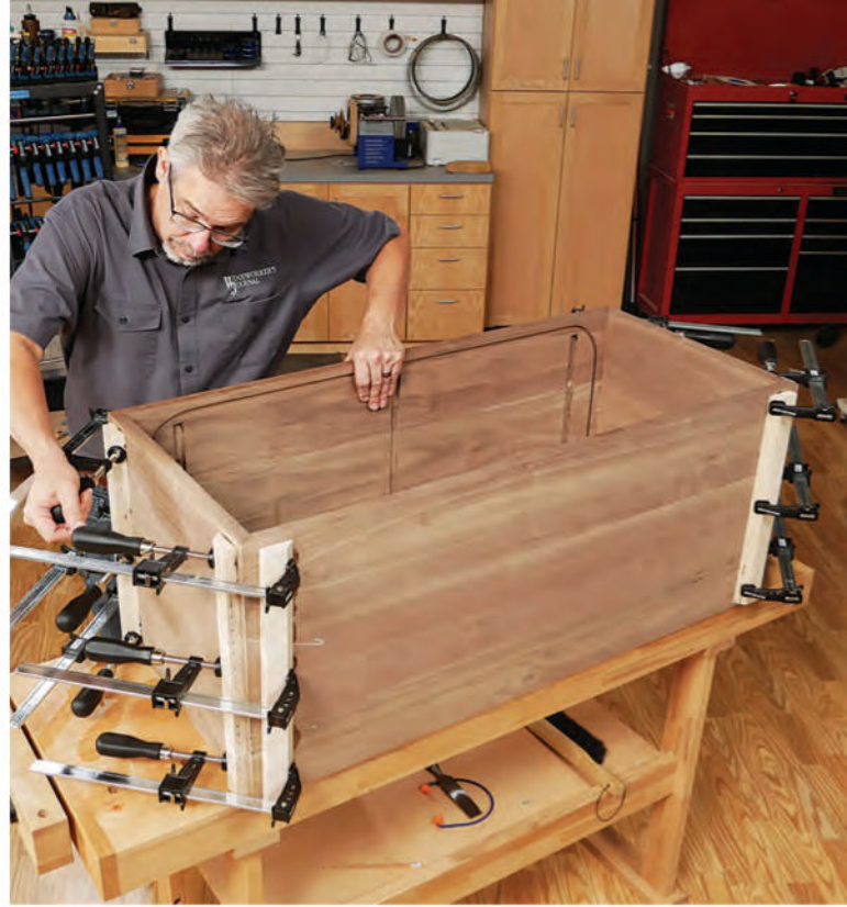
Managing the glue-up of a large carcass requires careful preparation. Here, the author dry-assembles the console to test-fit the corner joints and to practice the clamping order and procedure.
