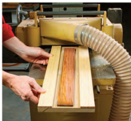
Resaw and plane down a piece of attractive stock for the two knife scales. Tape it to a carrier board to keep the wood flat as it gets thinner.
