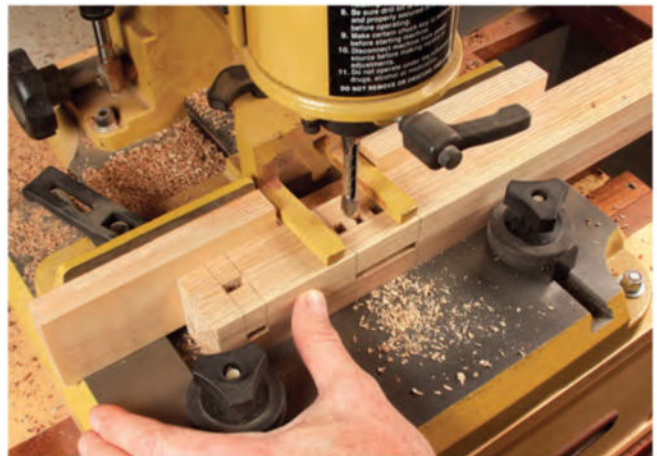
While the author used a hollow-chisel mortiser to chop the rail and apron mortises in the legs, you could also use a Forstner bit in a drill press, a router and straight bit or a chisel and mallet. Choose your favorite method.
