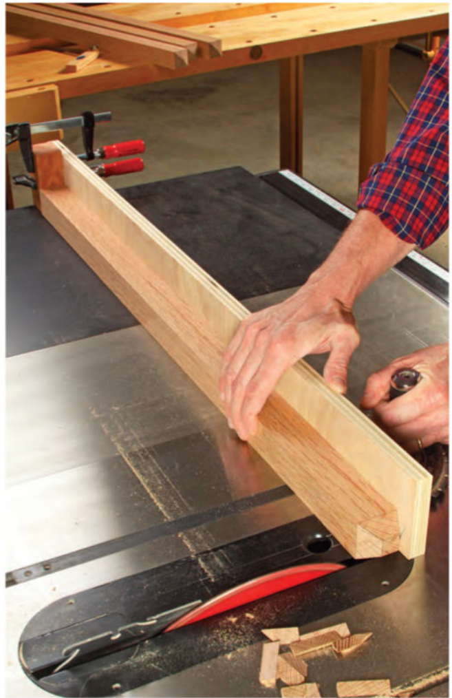
A stop block and long fence register the legs precisely with the blade for making four beveled crosscuts that create the top pyramid detail.
