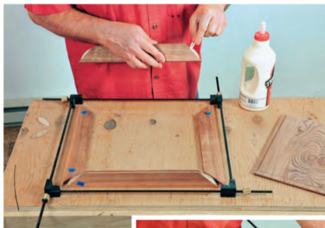
The author used a quick-release frame clamp to draw the mitered corners of the lid's frame together. After spreading glue into each biscuit and its corresponding slot, the frame members were assembled around the raised panel and each corner of the clamp tightened (inset).
