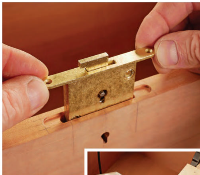
Installing the lock hardware involves cutting deep and shallow mortises for the lock body and selvedge plate. Most of the deep mortise was drilled out first with a doweling jig (not shown). A slotted router jig (inset) cut the selvedge mortise.
