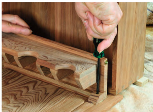
Once the lifting mechanism was operating smoothly, it was glued and screwed to the underside of the lid. The dividers between the notches keep bottles from shifting sideways inside the box.
