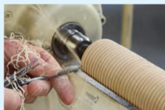
Scraping grooves into an American rolling pin turns it into a pasta cutter. Careful layout and tool presentation are critical to getting even spacing for good cutting.
