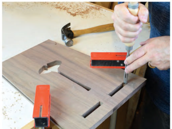
Chisel the corners of the four through mortises square. Make these cuts into the outside faces of the panels to reduce the chances of chipping the mortise edges. That damage would show after final assembly.
