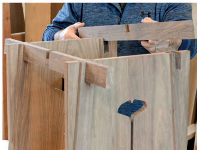
Test-fit the stretcher rails in the legs' bridle notches. The stretcher rails project 31 5 / 16 " beyond the legs, so make sure to center the rails for the next step.
