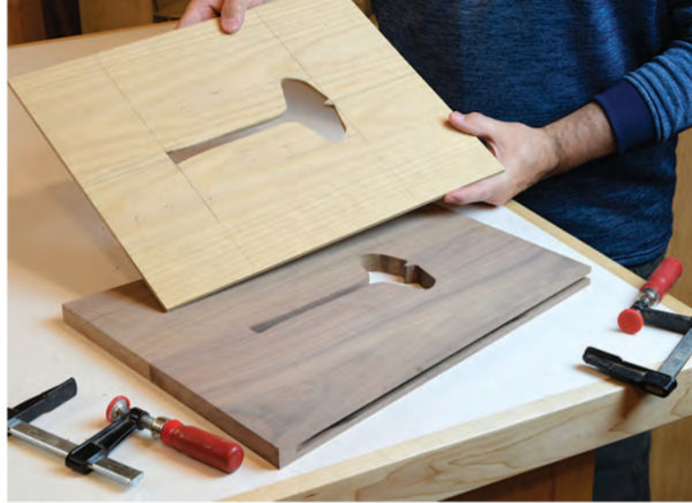
Start with a 7/16" bushing installed in your handheld router to rough out the inner waste material in several clockwise passes. Then switch to a 3/8" guide bushing with the same router bit for a final cleanup pass. The resulting shape needs very little sanding.
