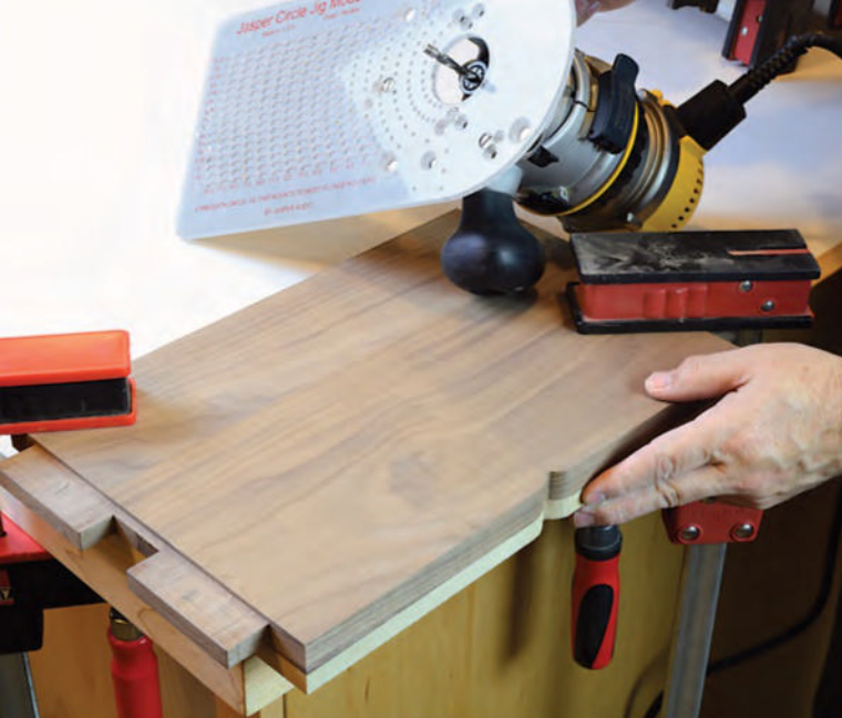
The shelf receives a V-notch detail on both long-grain edges. Here, a template is clamped beneath the shelf and the shape is routed with a 1/4"-diameter flush trim bit.
