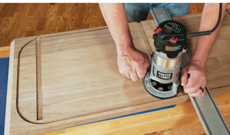
Cut three dadoes into the top and bottom panels to house the vertical dividers. Where the dadoes interrupt the tambour track, small fillers will be added to allow the doors to slide smoothly.
