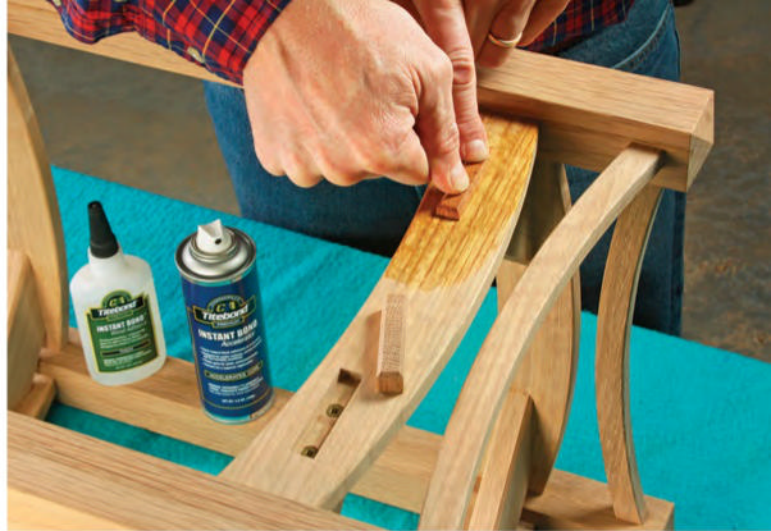
Chamfered faux tenons hide the screwheads and lend a classic Arts & Crafts detail here. CA glue is more than strong enough to secure these parts in their mortises. A spritz of accelerator shortens the glue's cure time to just seconds.
