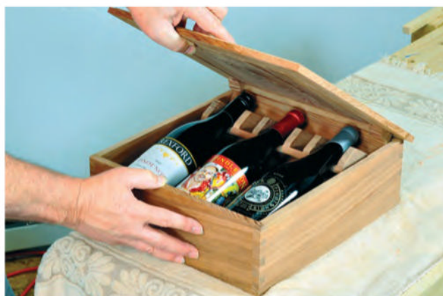
The author tested the operation of the lifting mechanism (temporarily screwed in place) with three bottles. With the lid fully open, he marked the position of the bullet catches and used a Dremel tool to create divots.
