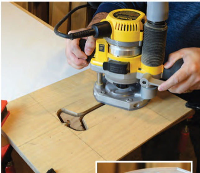
A plunge router removes the waste inside the leaf cutout in a multi-step process. The author used two guide bushing sizes and a 1/4" spiral bit.
