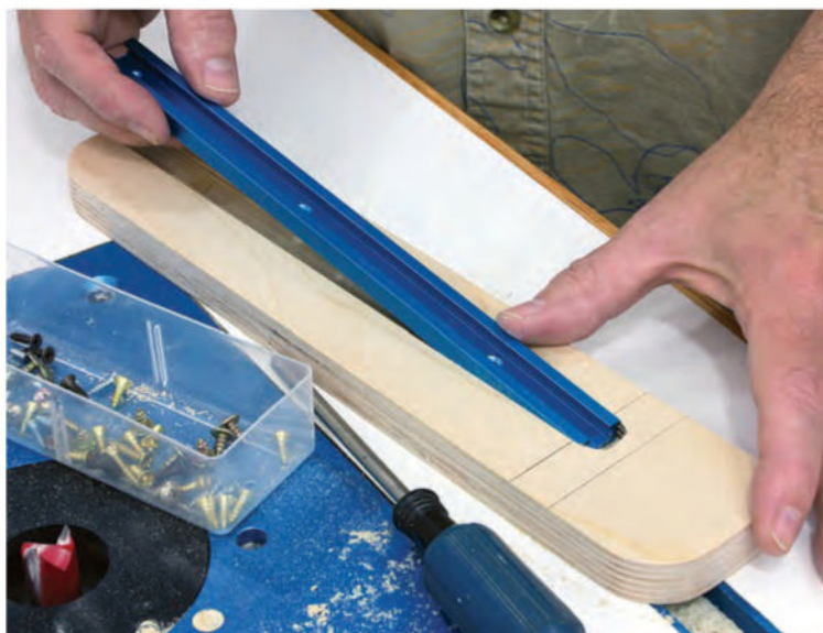
By routing the dado slightly long, the end of the T-track is neatly hidden underneath the fixed stop — a nice touch. The T-track is held in place by screws driven in through prepared countersunk holes.
