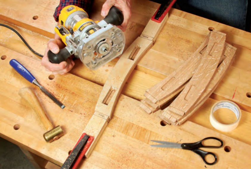
While an apron is still taped under its template, the author mills two 1/4"-deep stopped mortises with a plunge router, 1/2" O.D. guide collar and 1/4" spiral bit. The offset between the collar and bit creates mortises that are 1/2" wide and 2 1/4" long.
