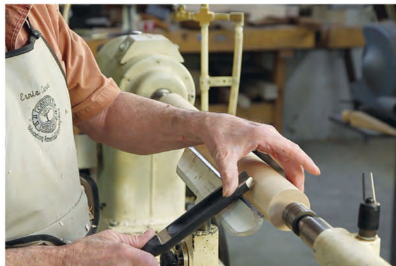
Use a spindle roughing-out gouge to bring the blank nearly round, then lightly touch the back of the piece with your fingers while holding the tool with your thumb. Sweep side-to-side to feel when the flat spots disappear.
