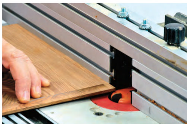
The top curved portion of a finger pull bit was used in the router table to raise the lid's book-matched panel. Each side of each edge was routed so as to reduce the panel's edge to about 1/8" thick.
