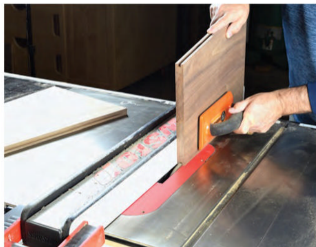
Form stopped grooves in the side panels with a 1/4"-wide dado stack. Note the clamp on the rip fence here, which acts as a stop block.
