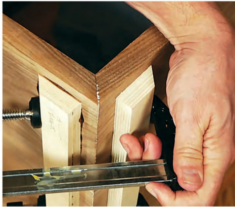
A combination of glued-on cauls and alignment biscuits turn this challenging assembly job into a very manageable task.
