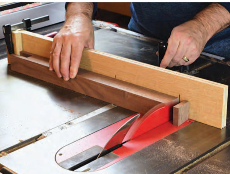
Now slide the leg down the auxiliary fence and set a stop block to trim all four legs to the same length. Keep their orientation the same for this cut.
