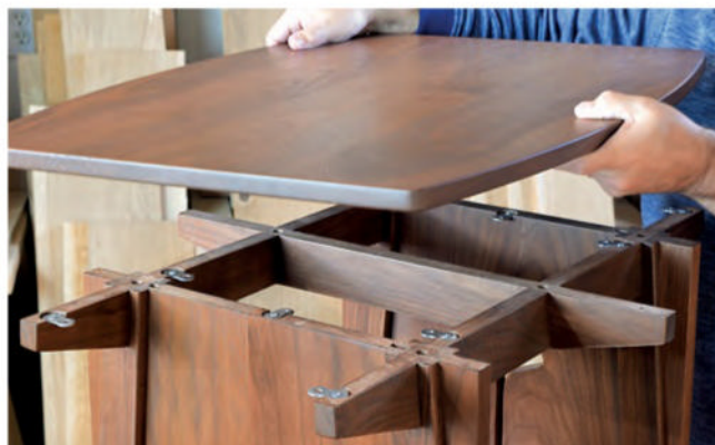
The solid-walnut top is attached with figure 8 fasteners to allow for seasonal movement. Three screws through the cross rail offer additional anchor points.
