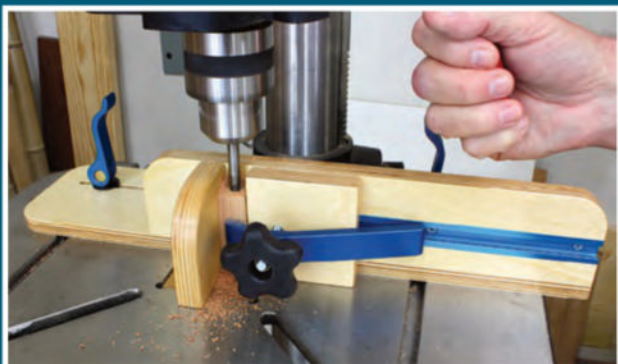
For more holding strength, install a hold-down clamp underneath the star knob on the sliding stop. For wider workpieces, flip the sliding stop and hold-down clamp as needed. Because the hole for the star knob is offset on the sliding stop, the blue hold-down clamp can be flipped 180 degrees to accommodate differently sized stock. When drilling shallow holes, you can remove the hold-down to speed up your drilling.
