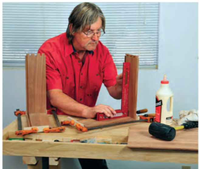
The box sides were assembled in two stages: The front and right side were first glued together, then back and right side. After glue-up, the author checked to make sure that each of the subassemblies was square.
