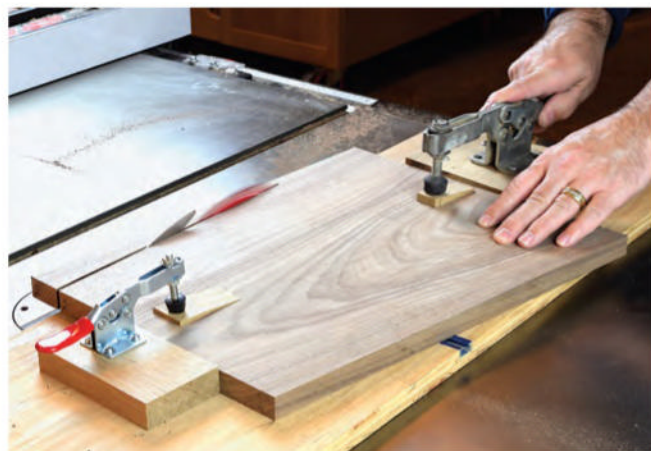
A shop-made tapering sled handily slices the side panels to their 5-degree tapers. This one is guided by a wooden strip riding in the miter slot.
