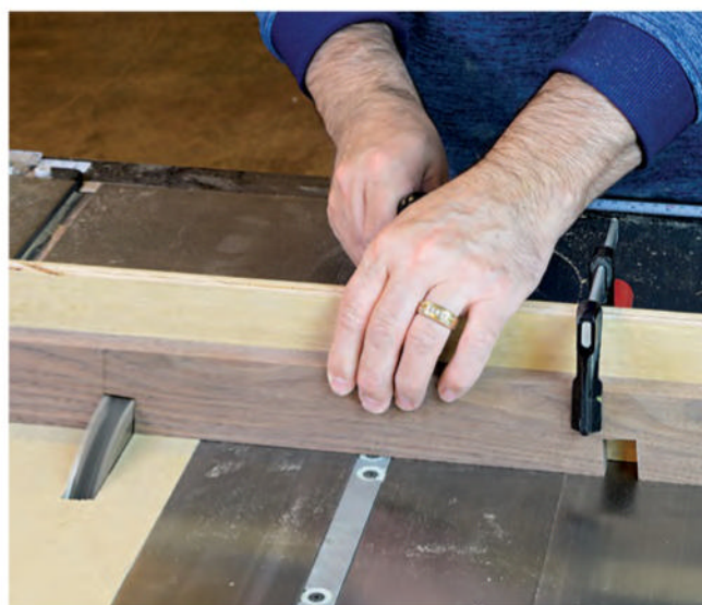
Tilt a dado blade to 5 degrees to cut opposite-facing notches in the cross rail. Use a full 3/4" dado stack plus a .004" shim to ensure the parts will come together without a wrestling match.
