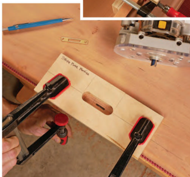
A shorter-slot mortising jig made quick work of routing a shallow recess in the lid for the lock's strike plate. Notice the dark rectangular marker imprint of the lock's bolt: it helped make locating the strike plate easier.
