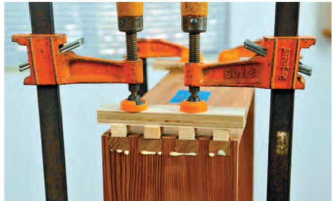
Small pine blocks cut from scrap were arranged to provide clamping pressure to the tail portion of the joint. A light coat of glue applied to all joint surfaces produced only a small amount of squeeze-out.
