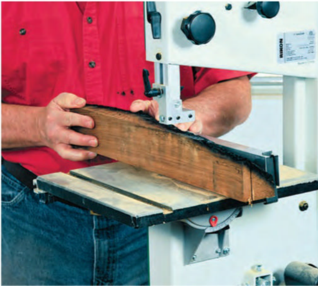
For the presentation box, the author resawed stock that he cut from an old-growth redwood stump on his property. After hand-sawing, each piece was surfaced and edged with a jointer and thickness planer.
