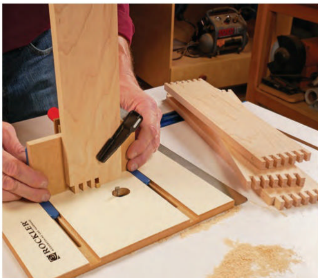
The author opted to make the chest's removable storage tray from maple. He used 1/4" box joints to provide a contrasting geometry to the chest's dovetails. They form rock-solid connections for this application.
