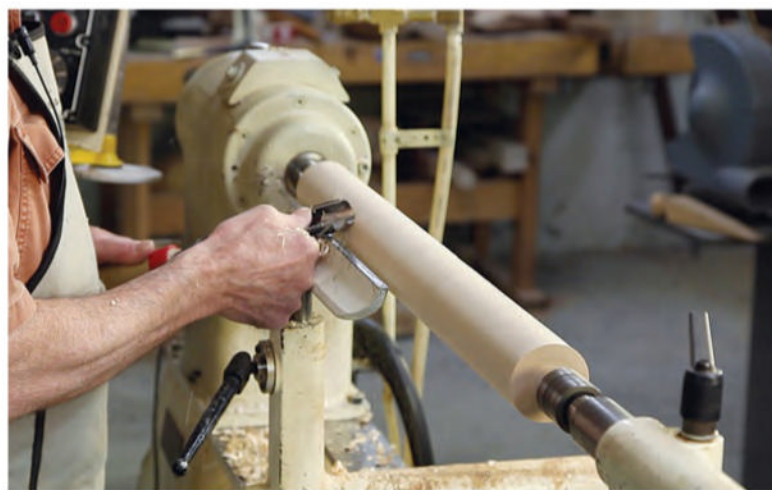
Holding the spindle roughing-out gouge at about a 30-degree angle to the work and pushing sideways (maintaining the angle) will give you about as good a finish as that left by a skew, with none of the danger of a catch.
