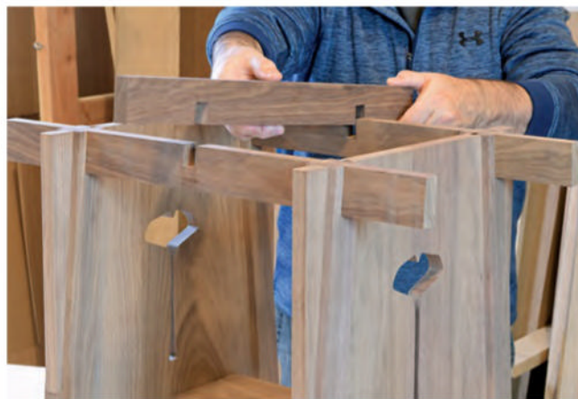
Due to the fact that the rail joinery is angled, the parts won't drop right together. You may need to use a clamp, reversed as a spreader, to gently flex the stretcher rails apart to ease the half-lap joints into place.
