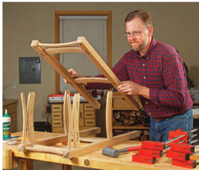
Glue up two side assemblies for the plant stand framework first. When their joints dry, join them to the remaining top rails and aprons to complete the frame. Remember that top rail and apron curves face one another.
