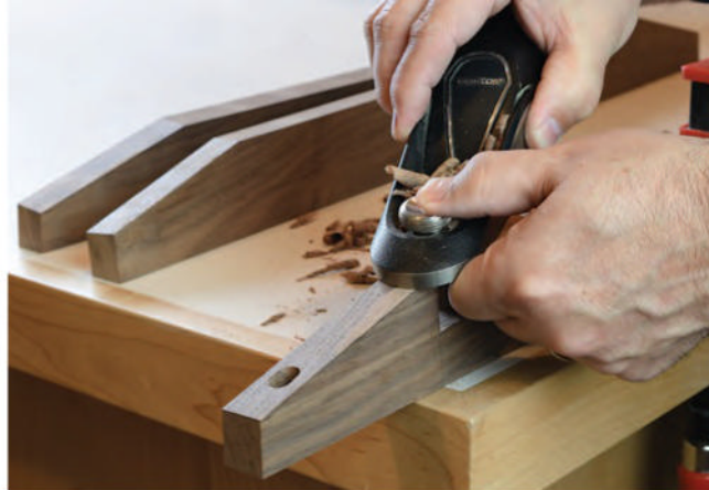
Tidy up the tapers on the ends of each rail by making repeated passes with a block plane. Hold the plane at a skewed angle while making these smoothing passes to minimize tearout.
