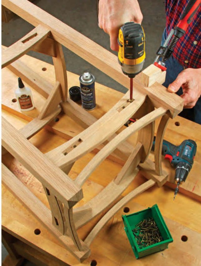
A simple way to install these corner braces is with pairs of screws countersunk into the stopped mortises. The author held the braces in place with CA glue and a clamp before drilling and driving the screws home.
