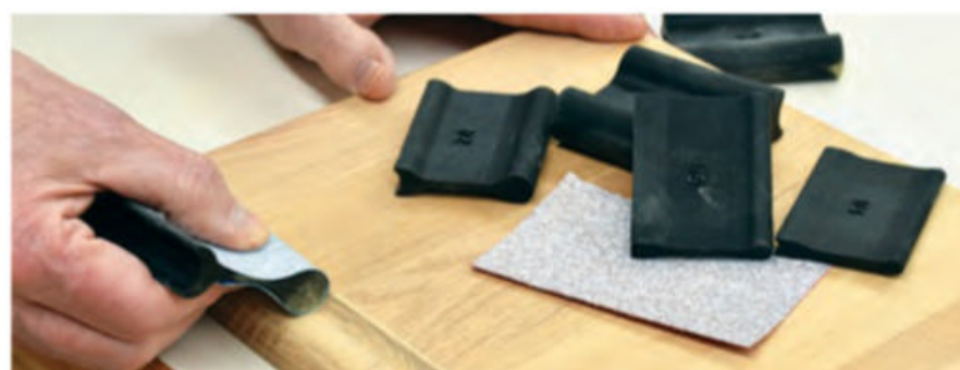
Contour sanding grips, like these from Rockler, are an effective alternative to a powered contoured sander and will help keep profiles crisp.
