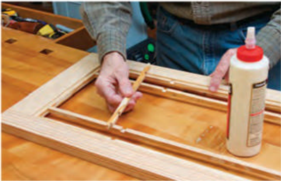
Continue the grid assembly with the inside vertical strips and, finally, the two inside horizontal strips. Glue these joints together and use small clamps if needed. Assemble the rear grids as stand-alone units; just be sure they fit into the frames easily.
