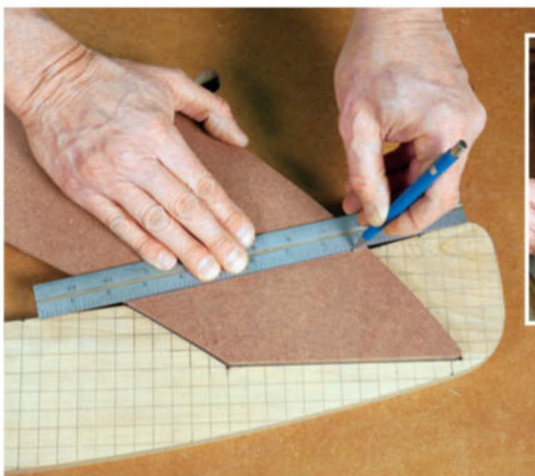
Set the back leg template into position on the rocker template and draw a line on the back leg template where the parts cross to create the leg blocking shape. Cut out two of them from scrap (inset).
