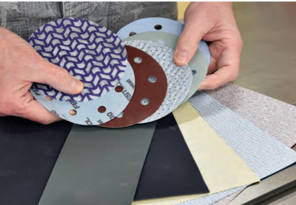
There is an enormous range of types and grits of sandpaper in both sheets and discs. The most commonly used in woodshops is aluminum oxide, but ceramic-based abrasives are becoming more popular.
