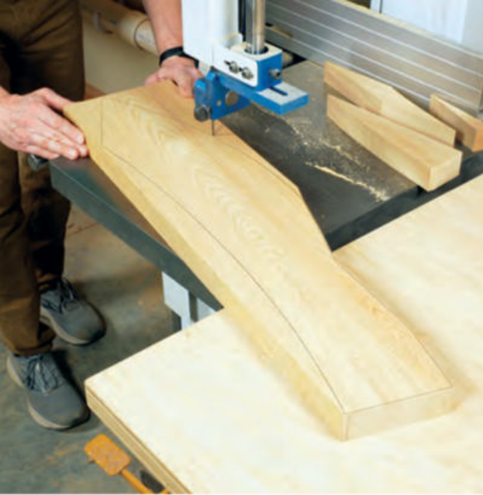
Use the chair templates to trace the part shapes onto your project workpieces and cut them out. The author rough-cut his chair parts slightly larger than the template tracings in order to prepare them for template-routing.
