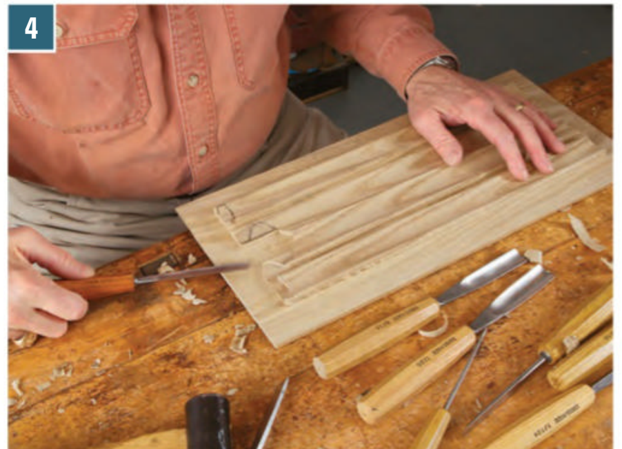
4 Carve the center section first, with the very center brought down to the base of the field and the edges carved to create the illusion of folded cloth.
