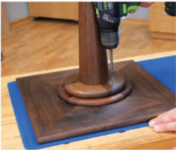
If the top surface of your pedestal stand's top will be visible, drive #8 x 1 1/2" screws through the upper discs from below to install it in order to hide the screwheads.
