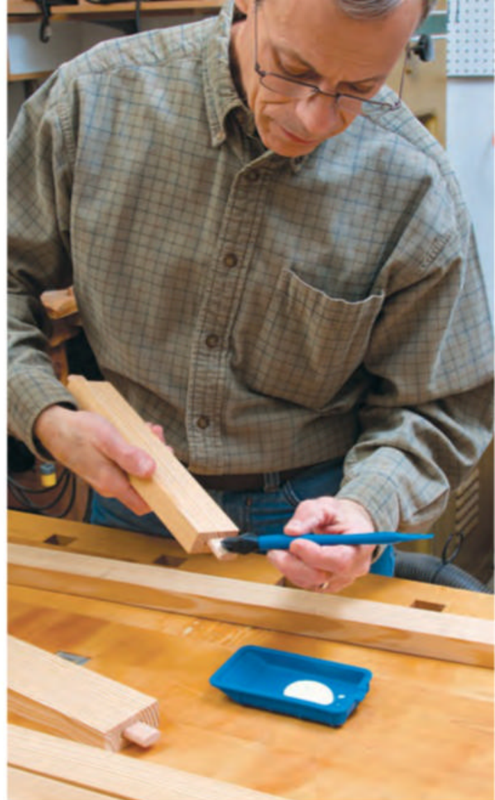
When assembling the frames, spread glue evenly inside the mortises and on the tenons. A silicone brush works well here and can be easily cleaned because glue won't adhere to it.
