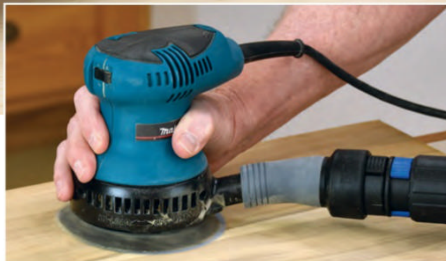
Although not suited to hogging off massive amounts of wood, a random orbit sander excels at most other shop-sanding chores and leaves a swirl-free surface.
