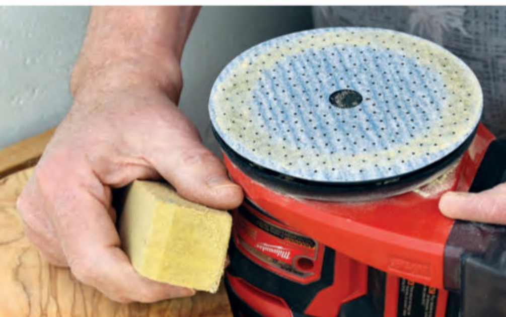
If a sanding disc still has plenty of abrasive but becomes clogged, a gum-type cleaning block can bring it back to life. Here, the author has cleaned just the center of a fully-clogged disc to show how well it works.
