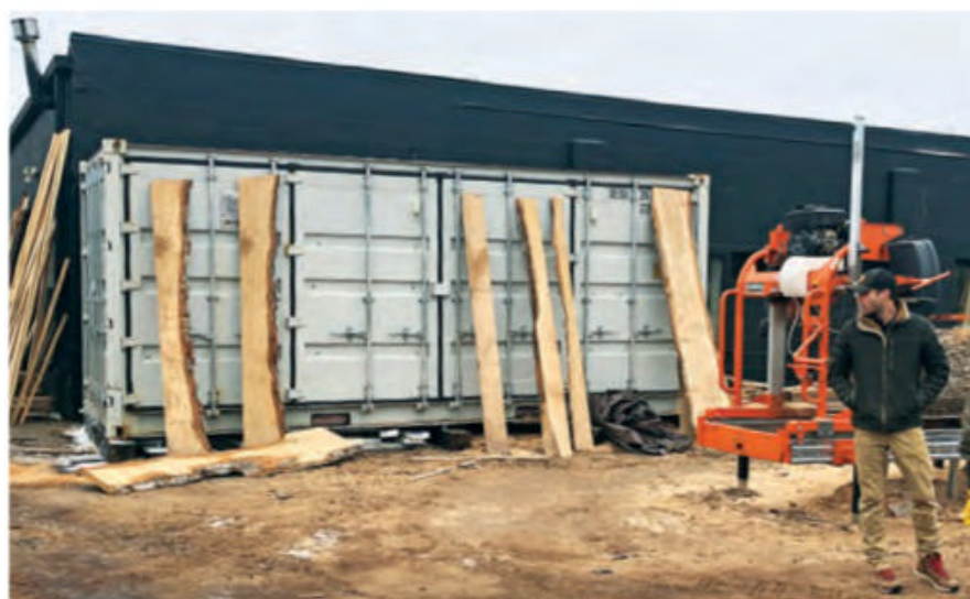
McLean and Hughley assembled Nyle L200PRO dry kiln unit bands in a shipping container to adhere to moisture removal schedules. The heat treatment cycle sterilizes the salvaged wood.
