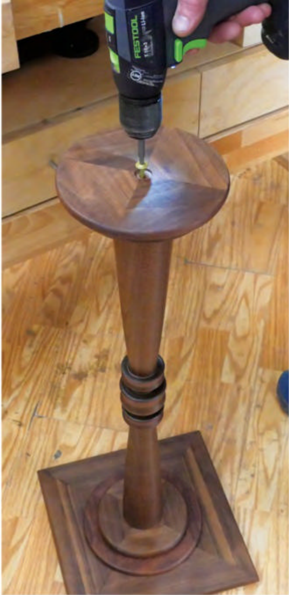
Install the top two discs on the pedestal with another 4" lag screw, just as you did for the base and bottom discs.
