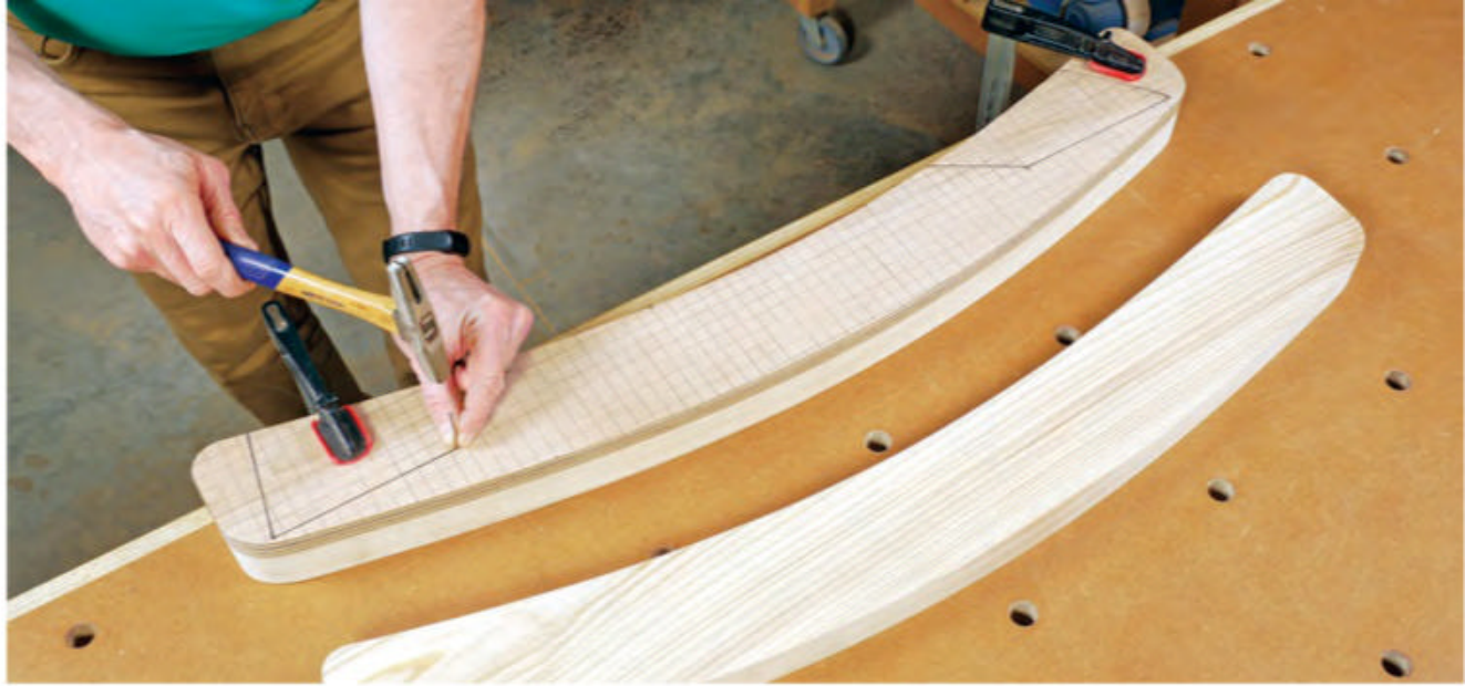
Clamp the rocker template to each rocker workpiece with their edges flush, and tap a long, thin casing nail through each of the template's four drilled holes to mark the leg positions on the rockers.
