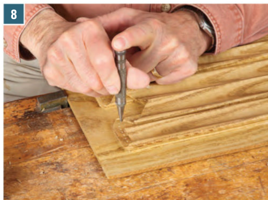
8 The author uses an automatic center punch in each of the pinpricks, but with careful use, a regular center punch works just as well.
