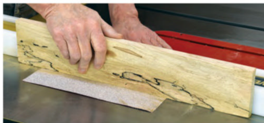
Narrow workpiece edges are often difficult to sand with a machine. A low-tech solution is to sand the piece against your table saw table using the rip fence as a side support. It will keep the workpiece edge square.
