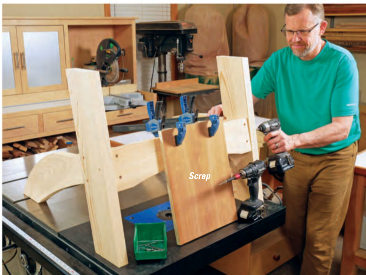
Begin assembling the chair frame by screwing the front cross brace to the back legs. Then raise this subassembly up, hold it upright with a clamped scrap and fasten the front legs to the back legs.
