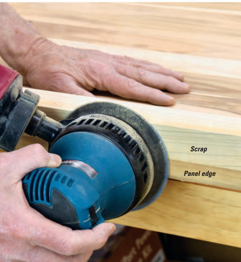
It's not easy to balance a sander on the edge of a panel. A straight piece of scrap clamped flush with the edge widens the surface area, helping to keep the edges of the panel square and flat.
