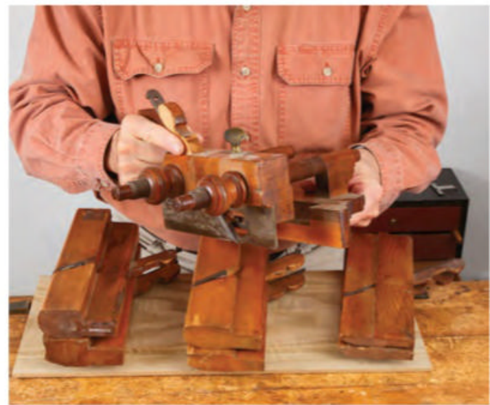
Hand planes with curved irons are key to producing a linenfold panel by hand. They are easily found at yard sales and antique stores.
