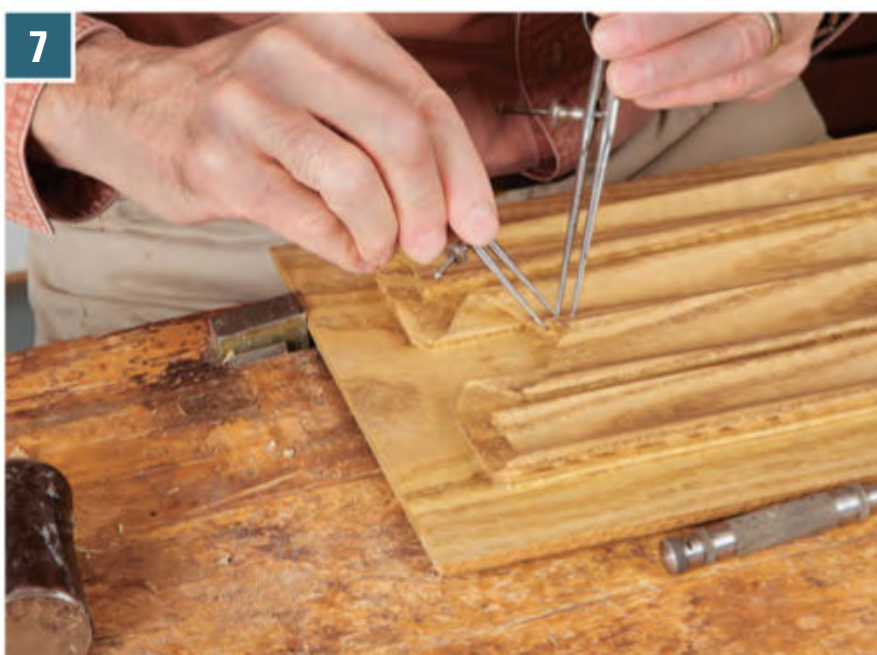
7 Use dividers to lay out pinpricks at a uniform spacing and a set distance from the edge. This will mimic stitching, evoking a "hem."
