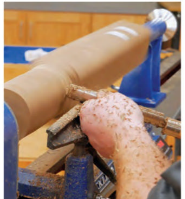
Mount a square blank for the pedestal between lathe centers and turn it into a round cylinder. A spindle roughing-out gouge, like the one shown here, is the best tool for this task.
