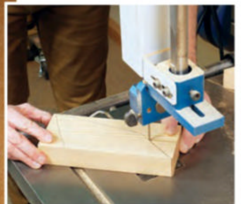
Set the back leg template into position on the rocker template and draw a line on the back leg template where the parts cross to create the leg blocking shape. Cut out two of them from scrap (inset).
