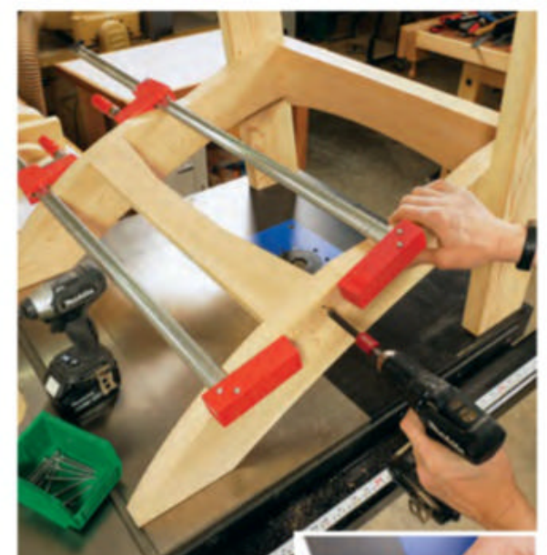
Mark each back leg's top edge 1" behind where the rearmost seat slat will attach (inset). Locate the front edge of the lower back brace flush with these marks before fastening the back legs to it with pairs of #8 x 2 1/2" screws.
