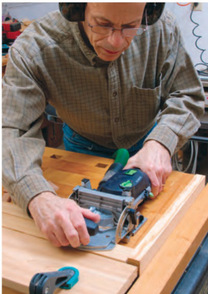
A Festool Domino is a quick way to make strong mortise-and-tenon joints for the shutter frames. Dowels, plate-joining biscuits and pocket-hole screws are good alternative joining methods.
