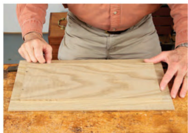
A raised field will become the "folded linen" area of the panel. You can raise the field on the table saw or with hand planes.
