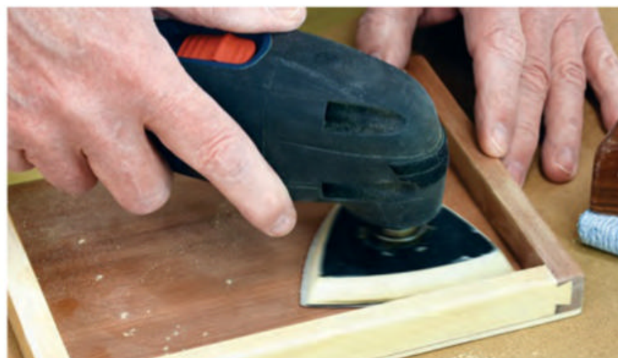
A detail sander, or an oscillating tool with sanding attachment as shown here, easily gets into the tightest corners.
