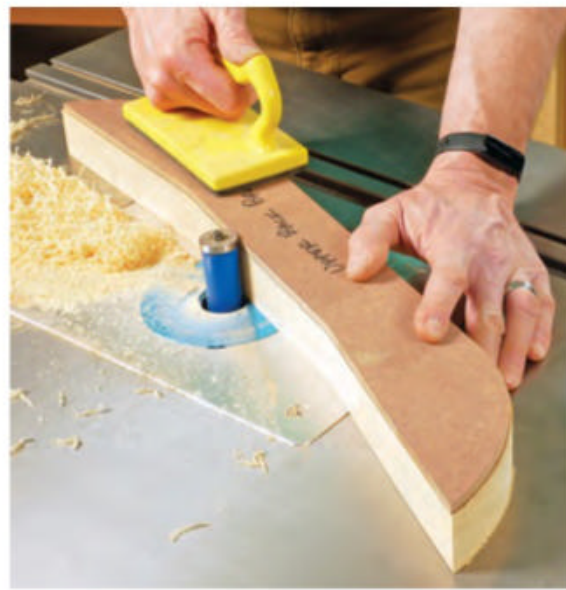
Here, the pilot-bearing on a long flush-trim bit follows the edge of the hardboard template to rout the chair workpiece to an exact match. Alternately, you could sand the parts to final shape instead of template-routing them.
