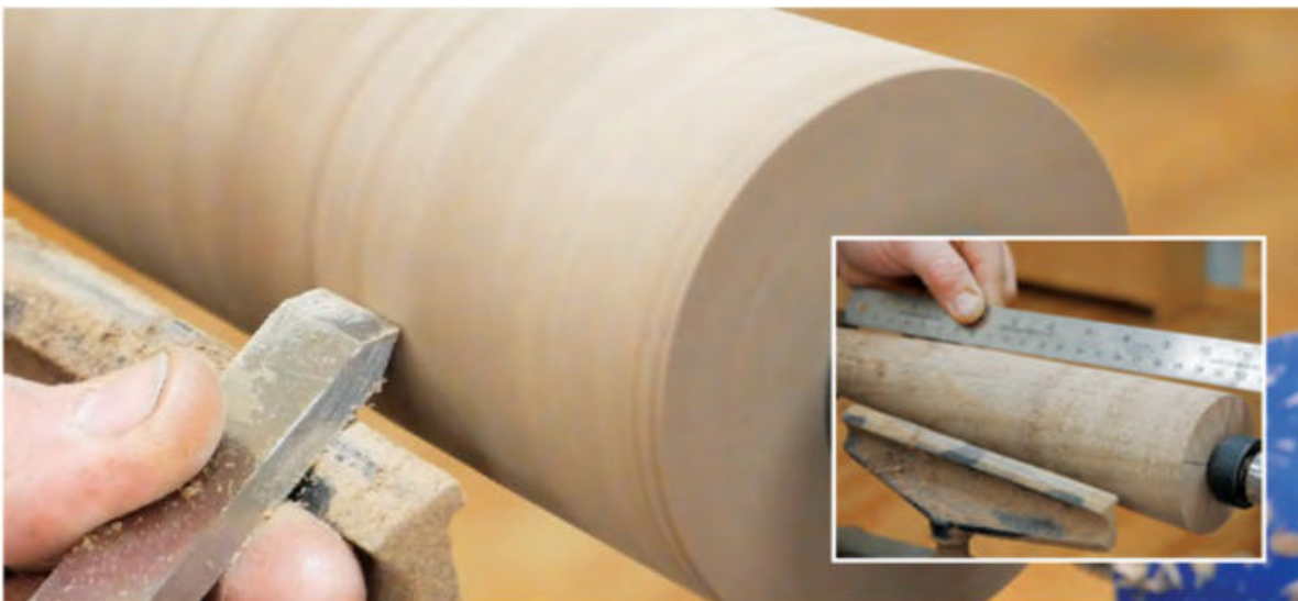
Turn the long tapered areas of the pedestal to shape using a spindle roughing-out gouge or a skew chisel. Try to keep the tapers as flat as possible. A long rule (inset) will reveal any high or low spots.
