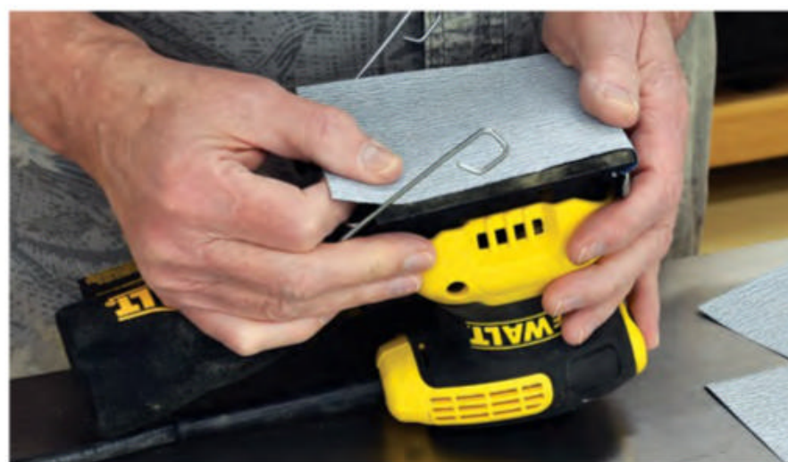
While quarter-sheet sanders have a few drawbacks, such as no hook-and-loop option for abrasives, the sandpaper is very economical. Less aggressive than other sanders, they’re also a good choice for finish sanding.
