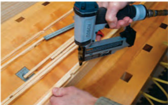
Use a pin nailer to attach the vertical perimeter strips first, then the horizontal strips. There's no need to glue the strips, and it's unnecessary to fill the pin-nail holes because they're almost invisible.
