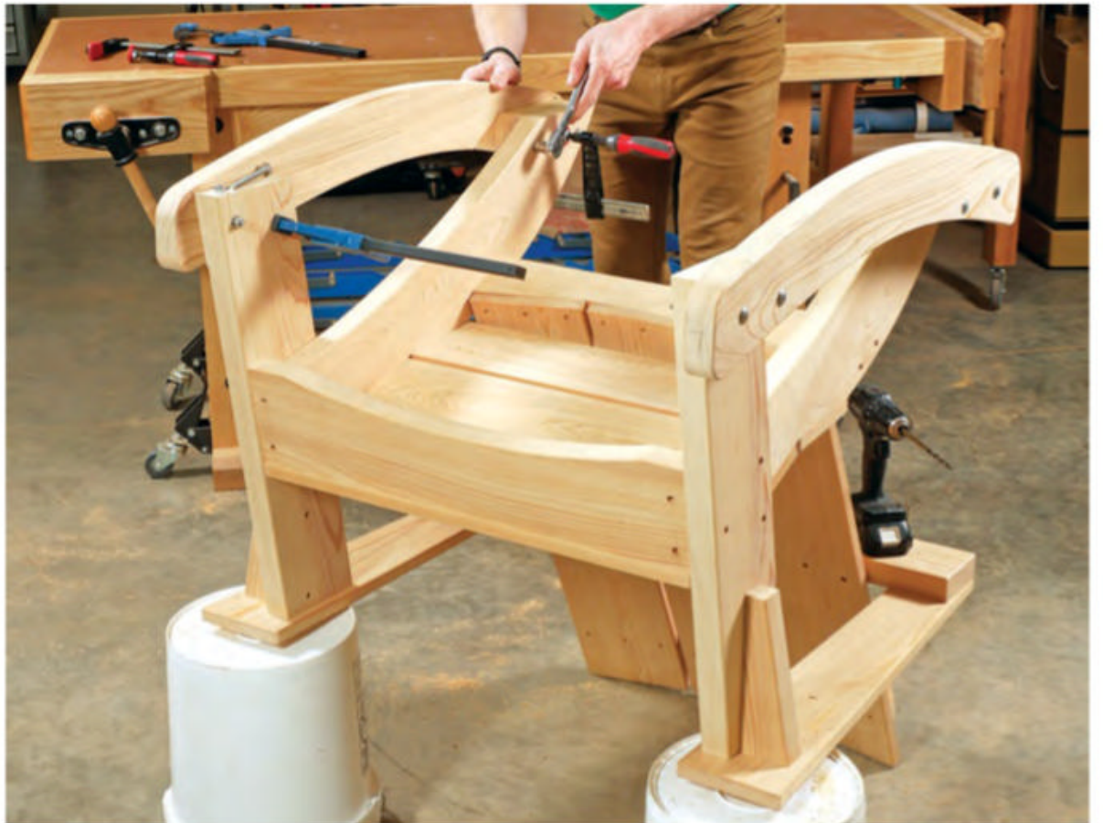
Align the nail marks on each rocker with the corners of the legs and clamp them in place. Install the rockers with carriage bolts, washers and locknuts. Use two bolts per leg driven into pilot holes.
