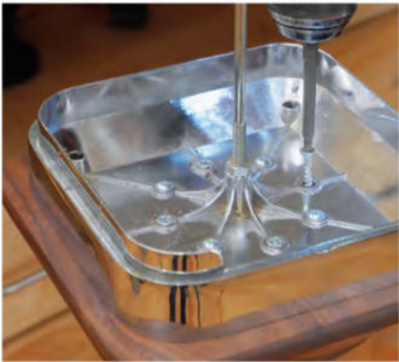
The author mounted the candy machine's metal base and top panel to the stand's top disc by driving #8 x 1" screws down through the parts.
