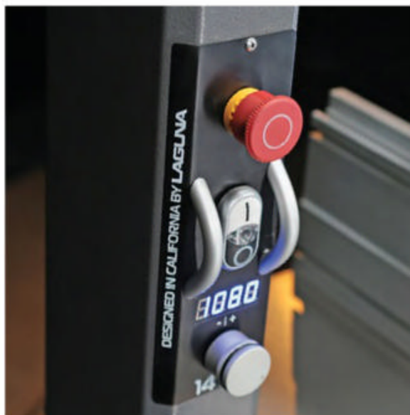
Blade speed can be adjusted on the fly with the twist of a dial. Digital readout reports the speed.
