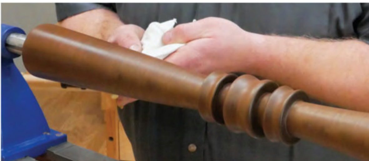
Hard wax oil or a shellac-based friction polish applied on the lathe are two quick finish options for this project's pedestal. Or wait until after final assembly and spray it with an aerosol finish instead.
