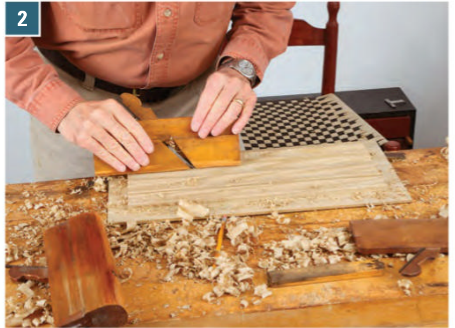
2 Use the rounding plane to radius the outside edges of the field and either side of the grooves to make them look like rolled linen.
