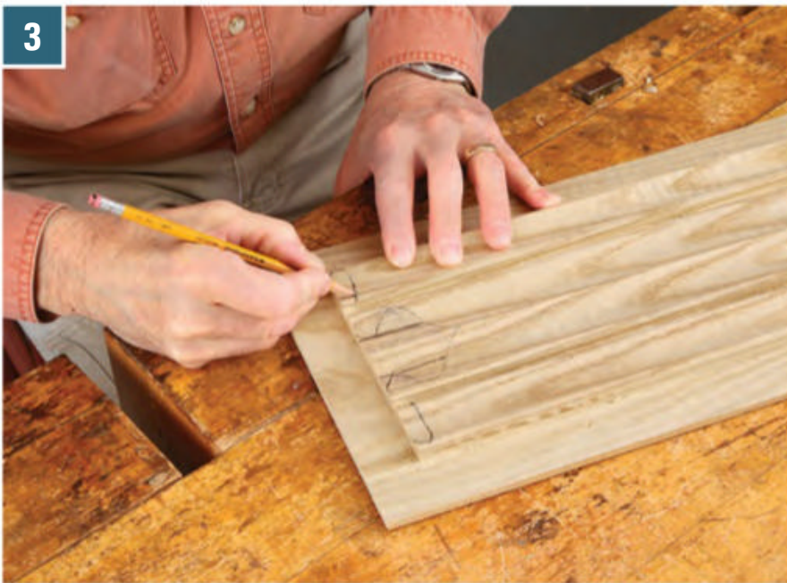
3 After the field is in the correct contour, the author uses a pencil with a soft lead to sketch in the lower and upper "folded cloth" details.
