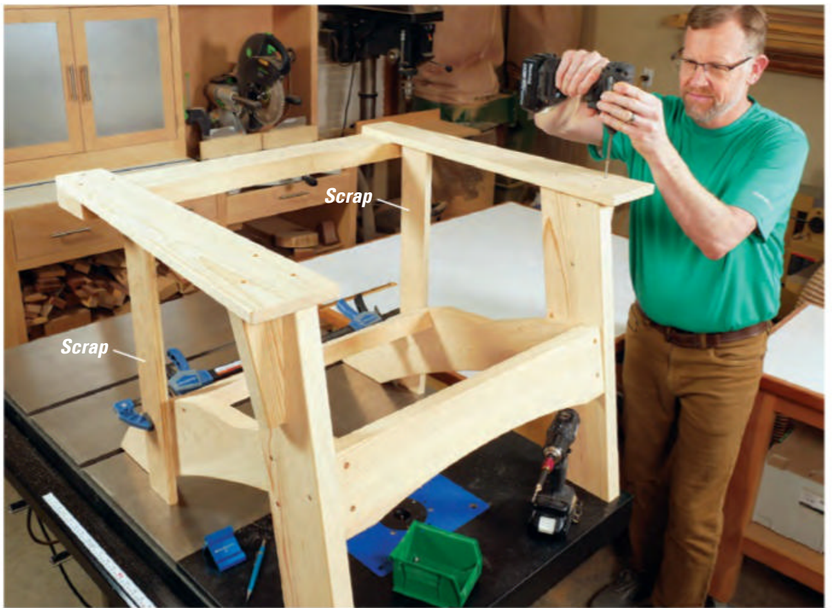
Attach the arms to the top ends of the front legs and arm braces using three screws per arm. The author created a subassembly of the middle back brace and arms first, held up with a pair of scraps.
