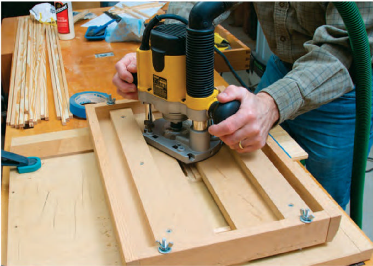
Use a plunge router and 3/8" straight bit to cut the dados in the lattice strips. Set the fences in the router carriage to work with your router's base. In this case, twisting the router between the fences produced the least amount of friction and the best stability and accuracy.
