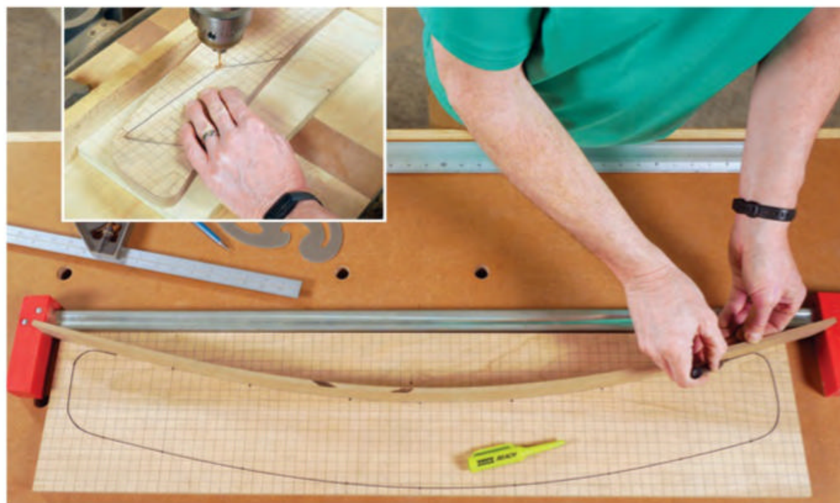
Use the gridded Drawing on page 24 for plotting points onto a plywood scrap to create the rocker shape. Here, a flexible batten squeezed inside a long clamp creates a fair curve to connect the points. Draw the legs onto the template as well and drill 1/8" holes through their corners (inset).
