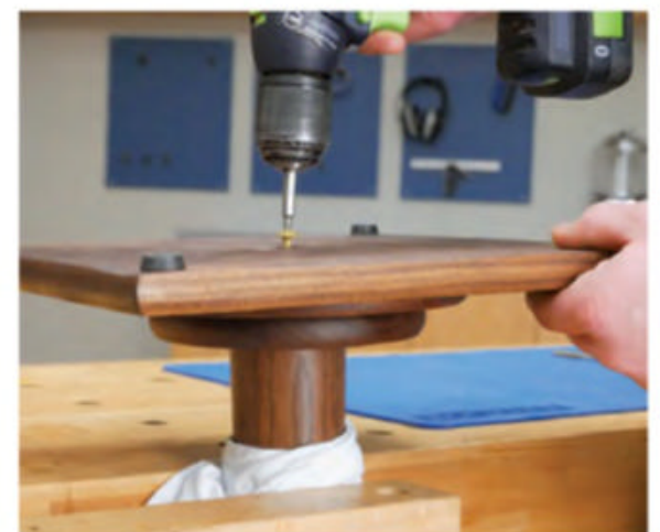
Install rubber feet on the base, then attach the base and bottom discs to the pedestal with a 4” lag screw. Counterbore the screwhead.
