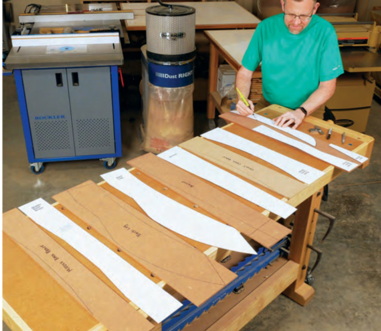
Rockler's white cardboard templates work fine for tracing part shapes directly onto the chair workpieces and then cutting them out. But the author used them to make a set of 1/4" hardboard templates instead for template-routing. This way the hardboard templates can be used over and over again.
