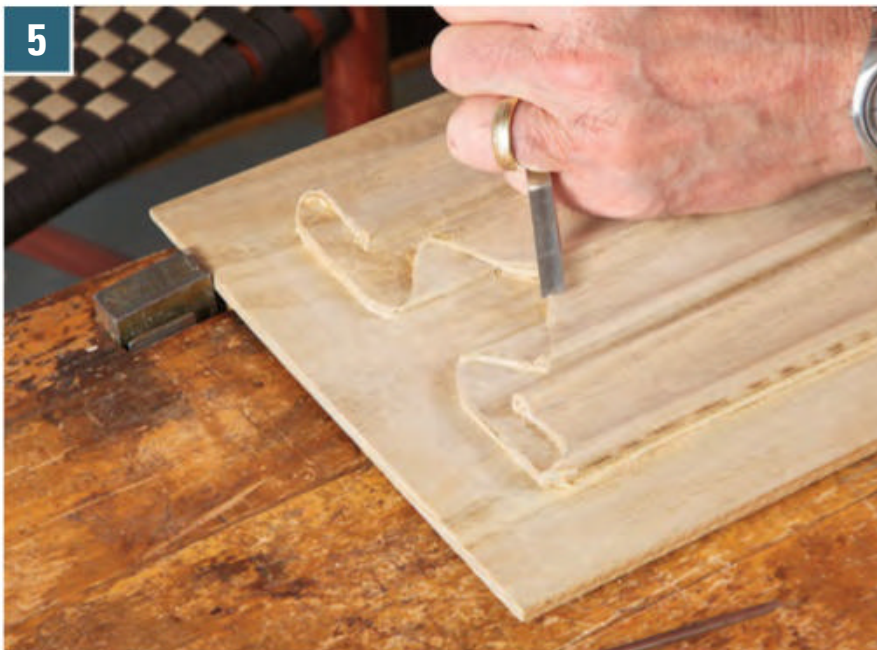
5 Putting a very slight chamfer (or bevel) on all of the edges enhances the illusion of a thin piece of cloth.
