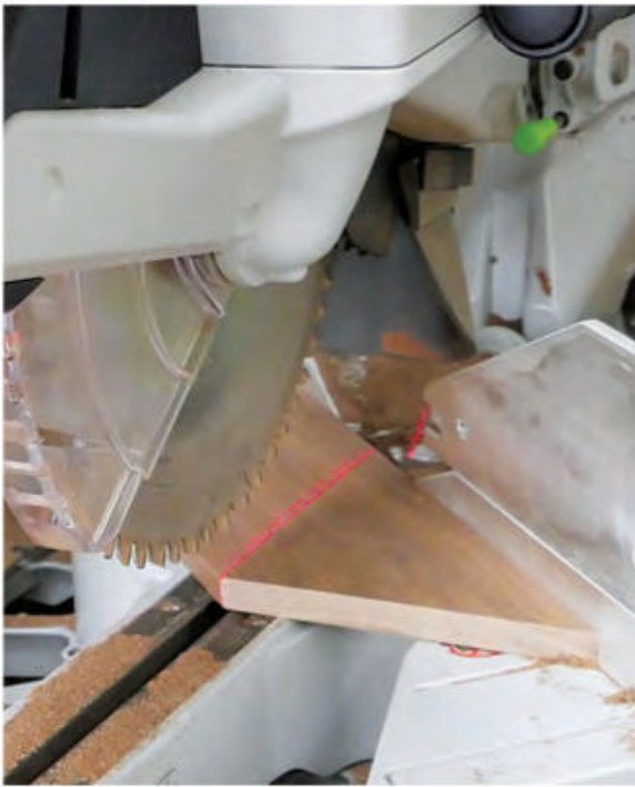
After ripping and crosscutting sections for the discs, base and large top (if you're making one), carefully cut each into a 45°-45°-90° triangle. The author used a miter saw for this process.
