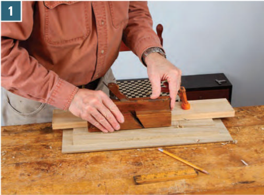
1 Clamping a scrap piece of wood to the panel helps to get the hollow plane running true with the length of the field.
