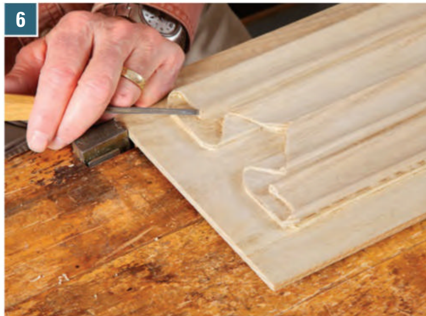
6 Using an 11-2 gouge like a drill at the final roll of the edge enhances the illusion. (A small twist drill will work just as well.)
