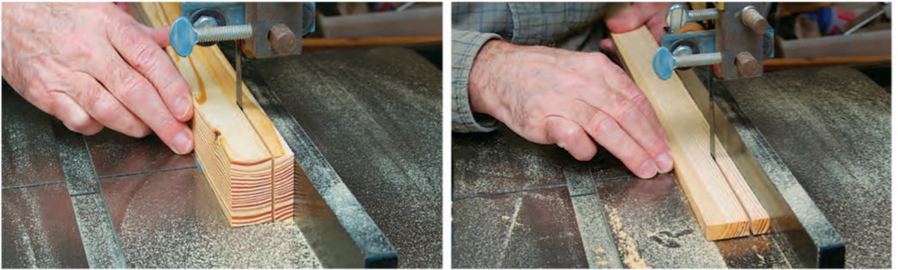
Photo at left: To use a hand saw to make the 3/8"-square lattice strips, rip pieces slightly less than 1/2" wide from larger stock. (The piece shown is roughly 2" x 2".) Photo at right: Next, with the hand saw fence at the same setting, make the second cut. Use a planer to clean up the strips and mill them to exactly 3/8" square. You could also make the strips on a table saw, but there would be more waste, due to the wider saw blade kerf.
