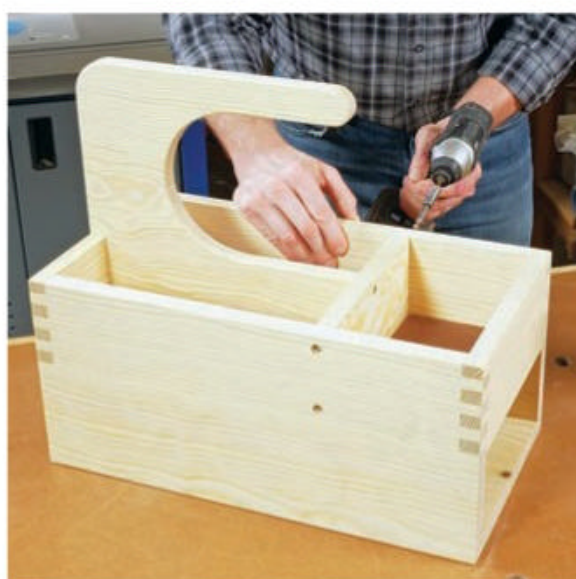
Fasten the upper divider to the front end of the handle with a couple of #8 x 2" countersunk screws. Then attach the handle/divider assembly to the carcass with more screws.
