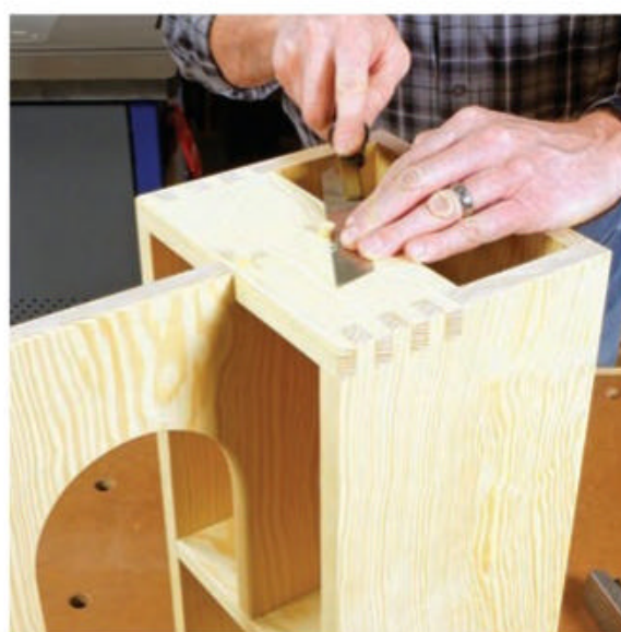
Wood plugs aren't necessary for shop projects like this, but they do make evidence of screws less noticeable. Install them with glue, then saw off the excess and sand the areas flush.
