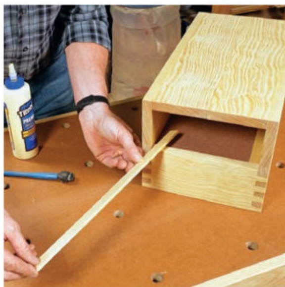
Glue a pair of 1/4"-thick scrap drawer guides to the bottom face of the deck panel. They'll prevent the drawer from tipping down excessively when it's opened. If they're initially flat, the guides don't need to be clamped in place.
