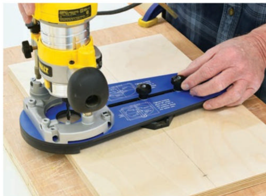
Attach the jig's pivot base to your workpiece, aligning it with your grid lines. With the jig arm placed on the pivot pins and the router attached to it, adjust the router bit to your marks and tighten the locking pivot knobs.
