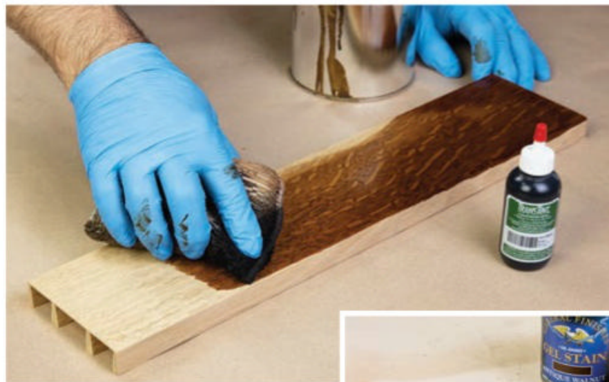
The author uses a two-stage coloring process: dye first (above), followed by gel stain (inset). He applies a barrier coat of dewaxed shellac after dyeing the wood to seal it in. The final topcoat is satin lacquer.
