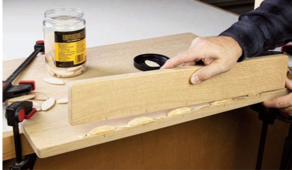
Attach the backsplash to the top panel with glue and #20 biscuits, dowels or some variation of loose tenons. Leave the back edge crisp where it intersects the backsplash for a nice tight joint.
