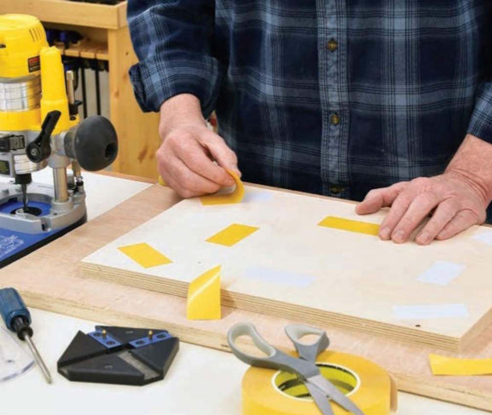
For securing the workpiece to a sacrificial surface underneath, double-sided tape is your friend. It will hold the work steady without marring it.
