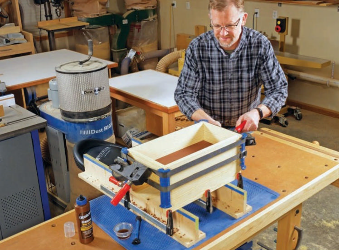
Glue up the carcass with the deck and bottom panels installed. Rockler's blue 1/2" Box Joint Cauls (item 34974) and a pair of strap clamps are an effective way to press the joints' pins and slots together snugly. Hide glue, used here, makes squeeze-out easy to clean up with water and a sponge.
