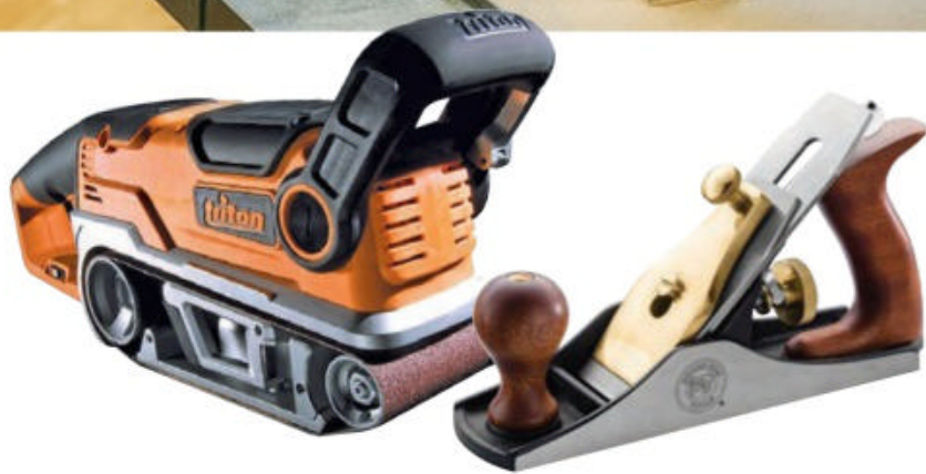
Once a resaw cut is completed, the roughsawn faces can then be smoothed in a surface planer. If you don't own one, however, a belt sander or bench plane can do the job by hand, too.
