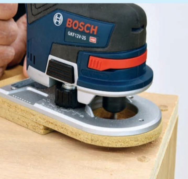
With the bit set just shy of the main workpiece, slide it over the plugs in a clockwise circular motion until the waste is removed.
