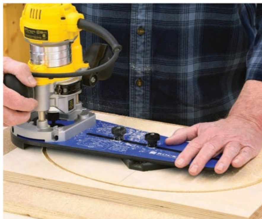
When everything is secure, plunge the router bit into the work about 1/8" and rotate the router to begin the cut. Make subsequent passes, resetting the depth each time until you've cut through the workpiece.
