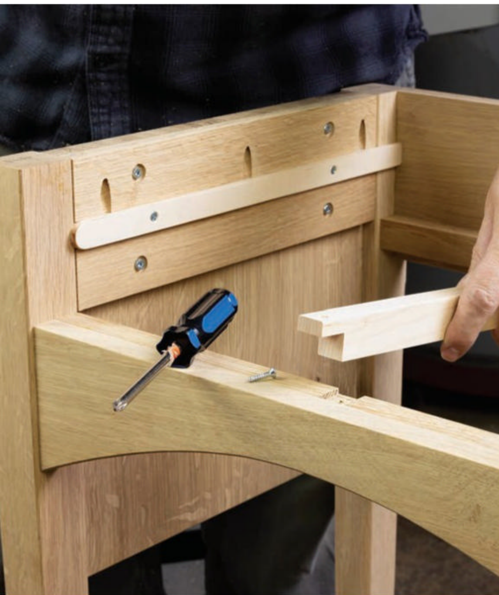
Install the center slide into the 1/16"-deep notches in the top edges of the cleats and secure it with a pair of wood screws, one driven through each of the slide's tongues.
