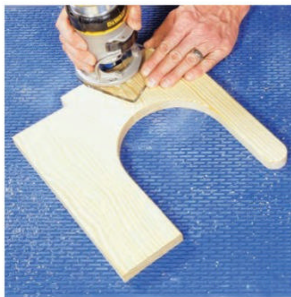
Saw the handle to shape and sand it smooth. Then ease the sharp edges above the carcass area with a 1/8" roundover bit in a handheld router, as shown here, or with sandpaper, to make it more comfortable to grip.
