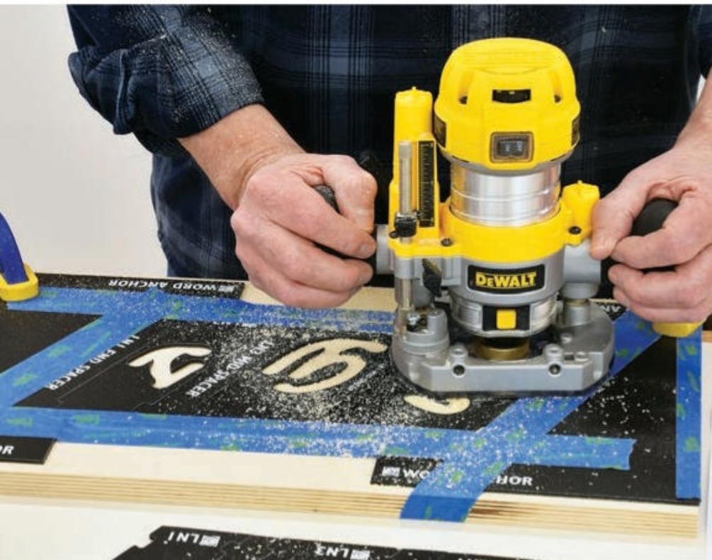
Carefully insert the collar of the bushing into the first letter template, plunge the bit and simply follow the template to rout each letter in turn.
