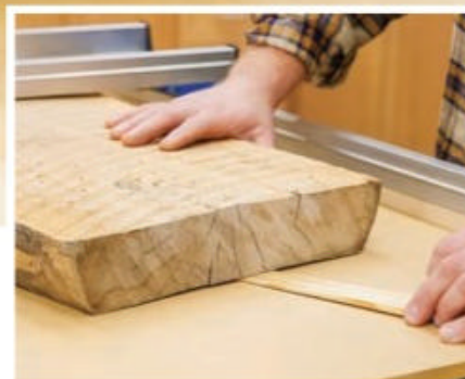
While this Slab Flattening Jig is intended for slabs up to 1¾" thick, it can be raised higher with spacers for thicker slabs, as the author did here (above). Be sure to shim and secure the slab (inset) so it won't shift during routing.
