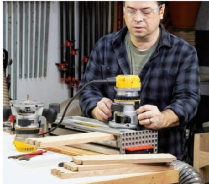
Attach the backsplash to the top panel with glue and #20 biscuits, dowels or some variation of loose tenons. Leave the back edge crisp where it intersects the backsplash for a nice tight joint.
