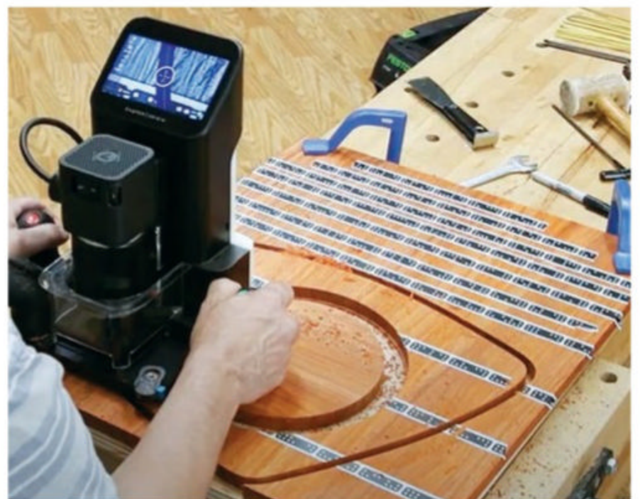
Whether you see it as a handheld CNC or a router with a GPS system, Shaper Origin vastly expands the scope of what a woodworker can do.
