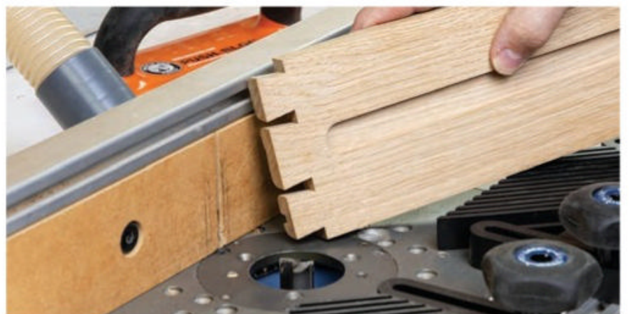
Rout a 1/4" deep stopped-groove in the drawer sides with a 3/4"-diameter bit capable of making plunge cuts. Reference the top edge toward the router fence for both cuts so these grooves match on both drawer sides.
