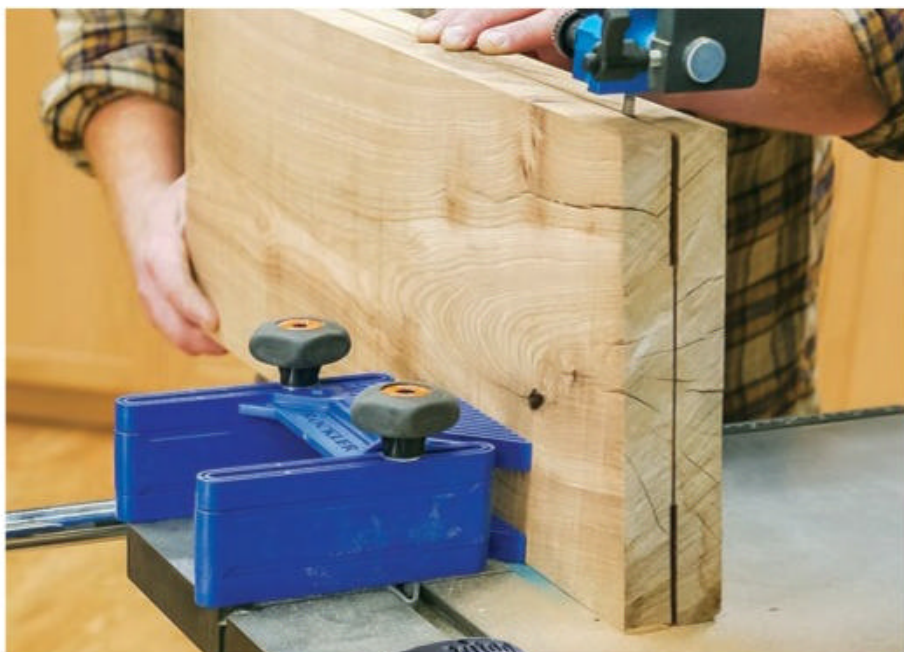
Even though the rip fence on this Laguna band saw isn't in view (the tall workpiece obscures it), it's supporting the opposite face of the slab section to help guide the cut along the line the author marked on top of the workpiece. A tall featherboard presses the slab against the fence to also help keep the cut on track.
