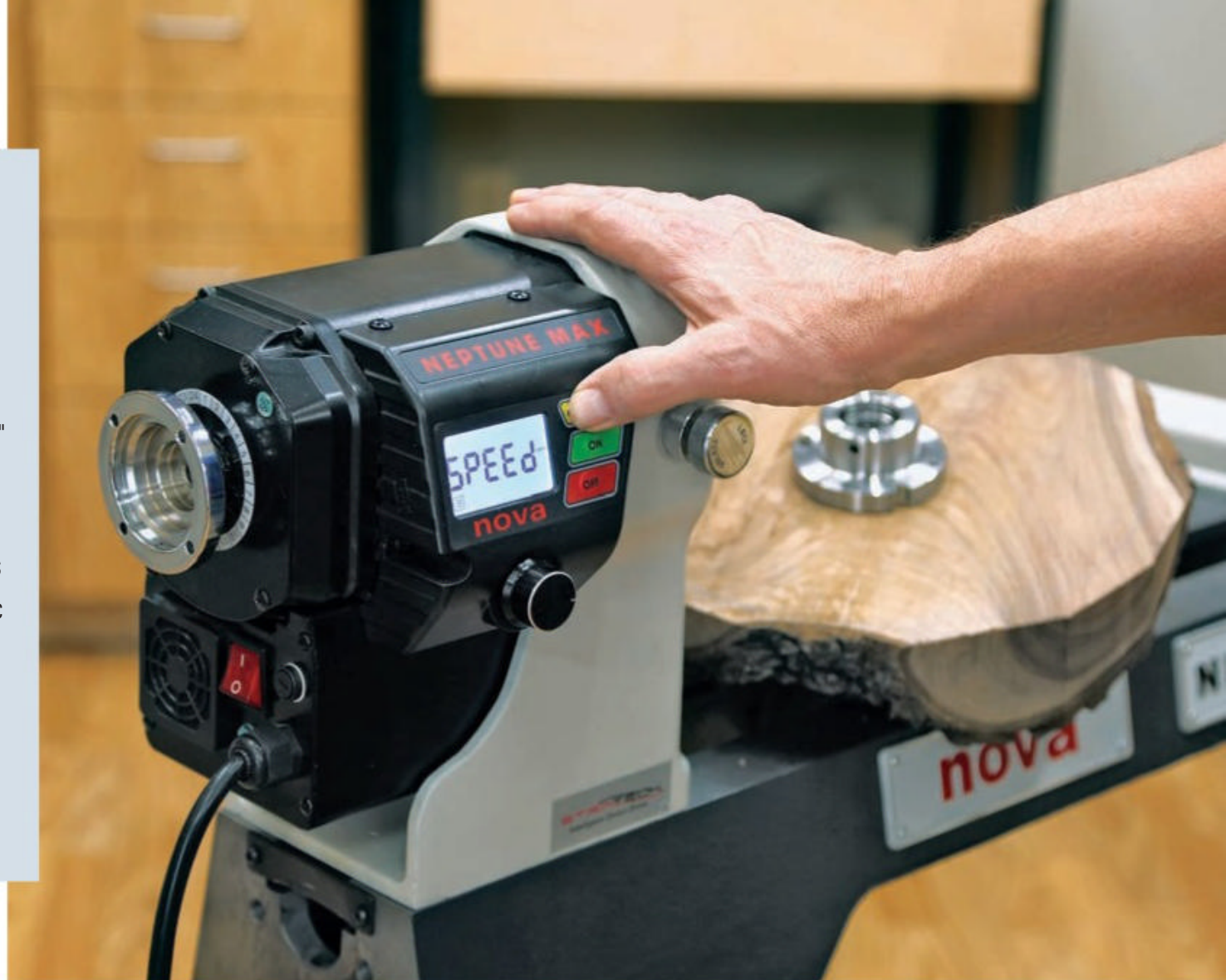
The Neptune's high-tech DVR programmable motor is paired with an icon-based HMI control screen that provides accurate and exacting control to the user.
