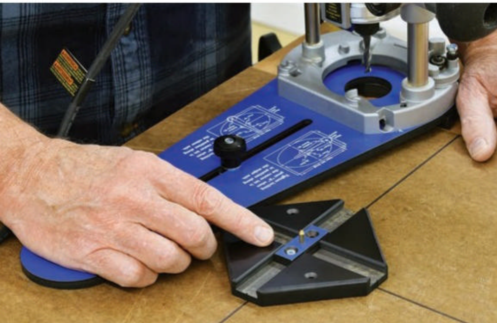
Routing a circle is the same process as an ellipse, but you only use one centered pivot pin and rotate the arm around a single set radius.
