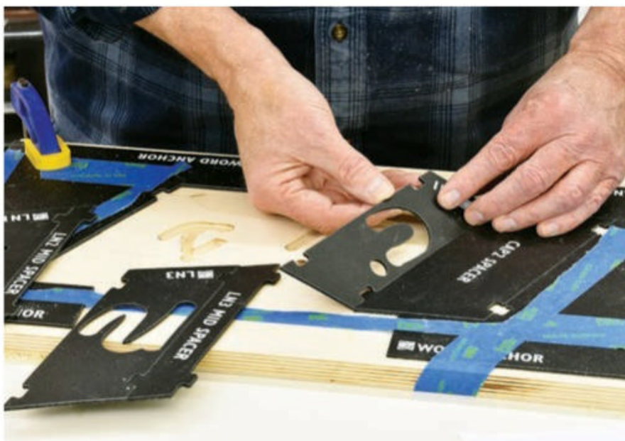
Being careful to leave the end word anchors in place, remove the letter templates from the first pass and insert those for the second pass. Tape them down securely and rout the new templates as before.
