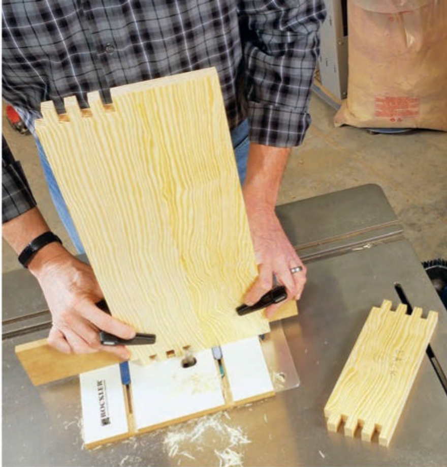
Mill 1/2"-wide x 3/4"-deep notches on the ends of the carcass front and back, and a mating pattern into the top ends of the carcass sides, to form interlocking box joints. Be sure to test your setup on scrap stock first.
