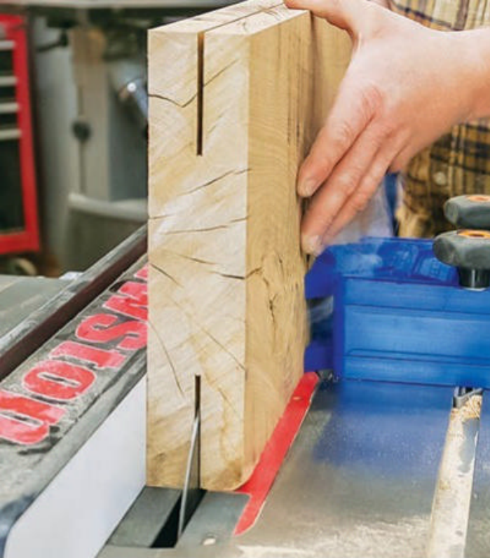
Starting an ambitious resaw cut at the table saw is one way to reduce the amount of material that a modestly powered band saw must then cut through. Square both workpiece edges first.
