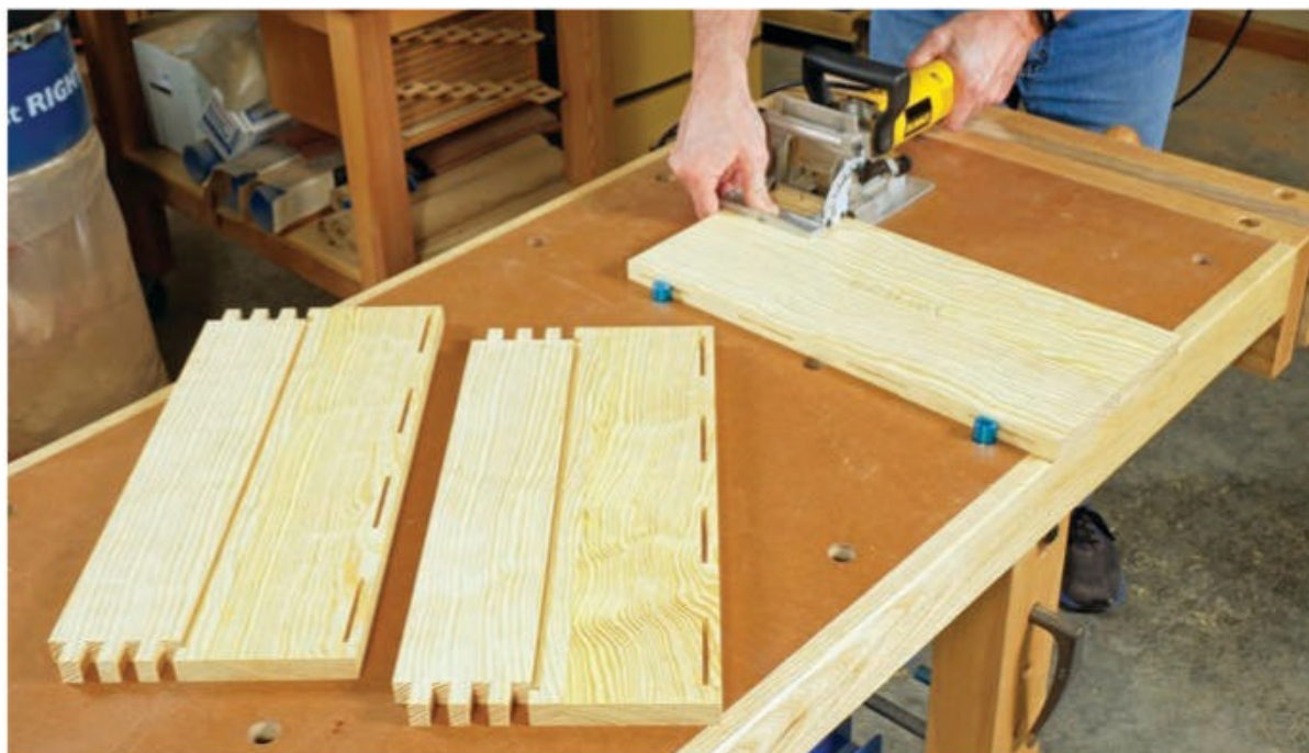
While the author opted to use #20 biscuits to attach the bottom panel to the sides, other joinery options would be fine choices too, including nailed or screwed butt joints or loose-tenon variations.
