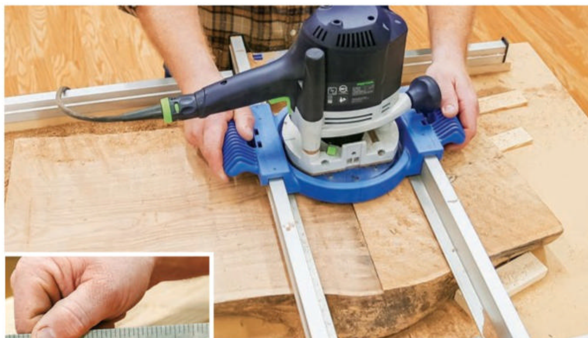
With the router set to remove about 1/8" of material thickness, flattening a slab involves sliding the router carriage back and forth slowly in side-by-side passes from one end of the slab to the other. You'll be left with a dead-flat surface (inset).
