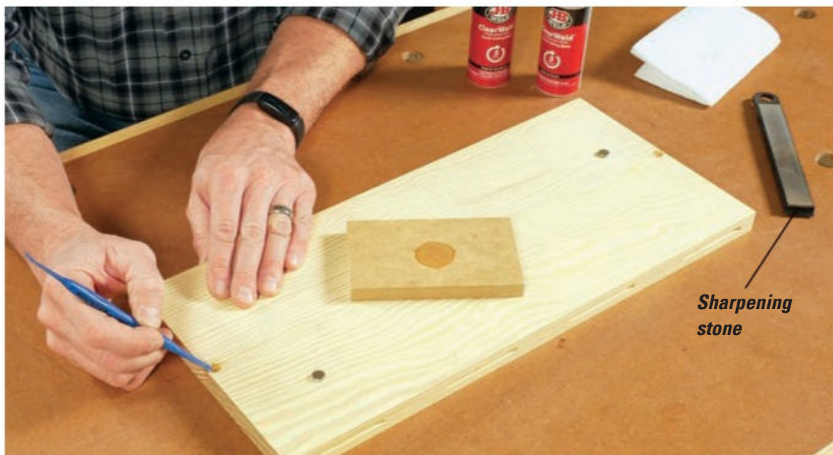
A pair of 3/8"-dia. rare-earth magnets, set flush with the top face of the bottom panel near both ends, will provide half of the drawer "catch" feature. Rough up the bottom surface of the magnets with a fine-grit sharpening stone or sandpaper before installing them in their holes with 5-minute epoxy.
