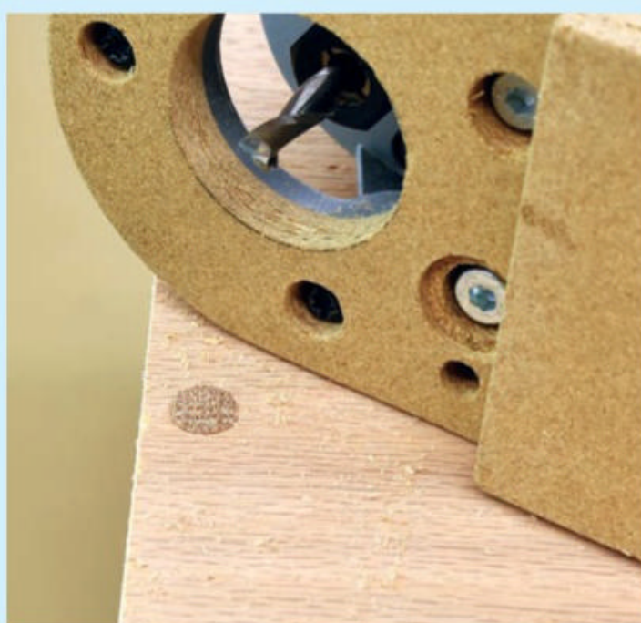
Once leveled, the tiny amount of the plug still above the surface can be quickly sanded smooth. Here, the author has shaved the plug to less than 1/32" proud.
