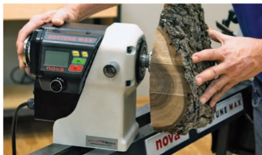
The headstock can slide across the full length of the bed and rotate 360 degrees. Outboard turning is one of the "big" lathe features on this model.
