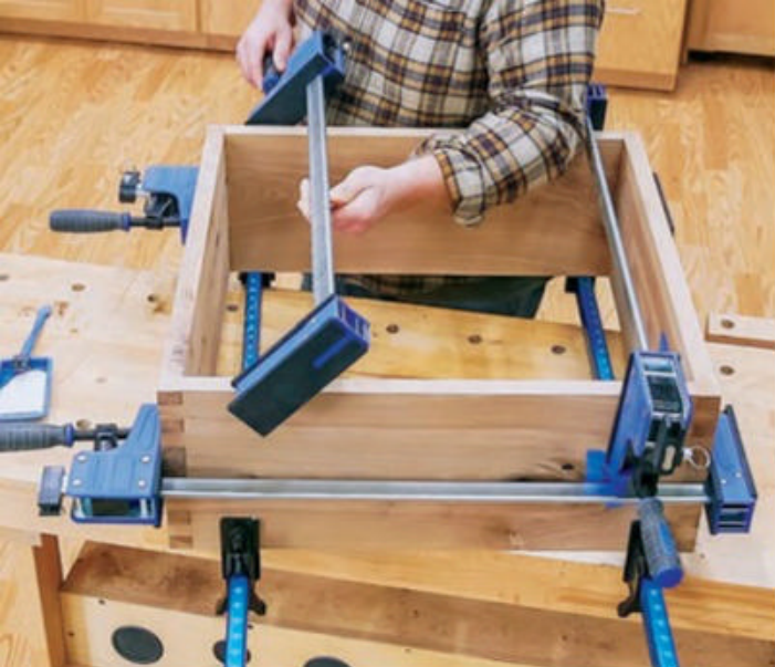
Assemble the bookcase's carcass with glue and plenty of clamps so the joints close fully.
