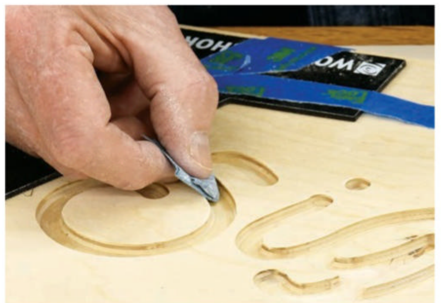
With the second pass complete, remove all the letter templates and use folded sandpaper to smooth and refine each letter. There typically will be a bit of burning or fuzz left behind, depending on the wood species and bit.
