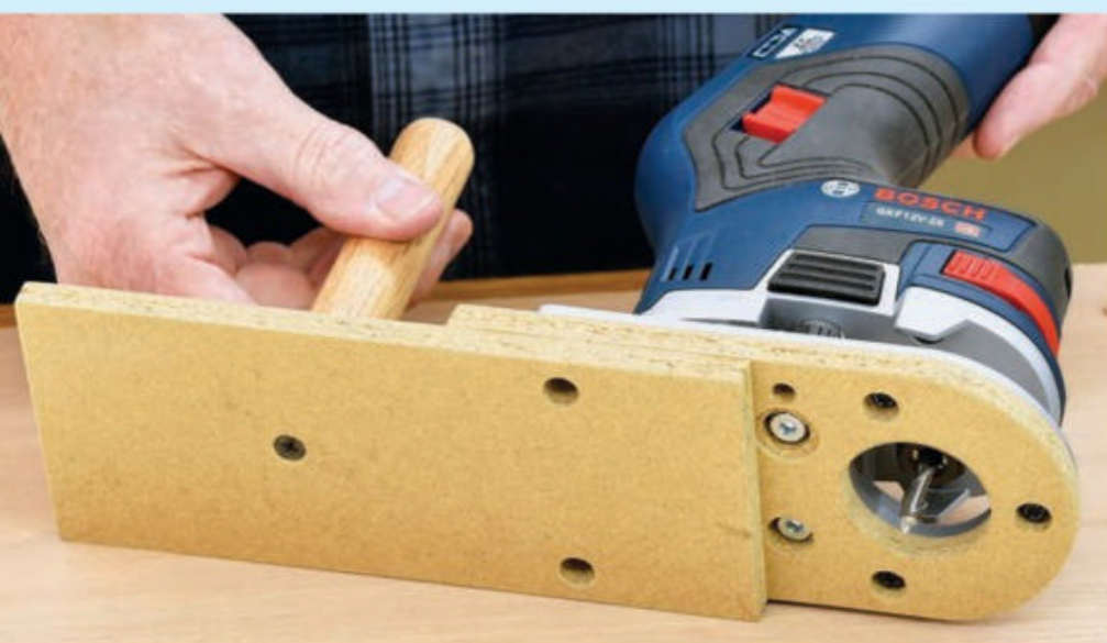
An easy-to-make subbase suspends the collet and bit above a work surface, allowing you to adjust the depth to shave a perfect amount off plugs, tenons, box joints or anything else you need to level.
