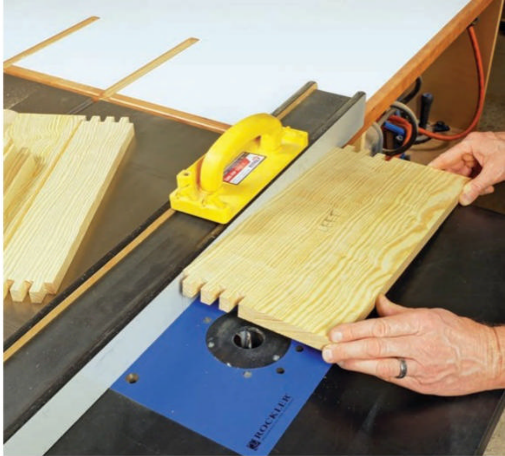
Plow 1/4" x 1/4" grooves along the inside faces of the carcass front, back and sides for the deck panel. Mark the cutting limits of the router bit so you can start and stop the groove cuts in the side panels accurately.
