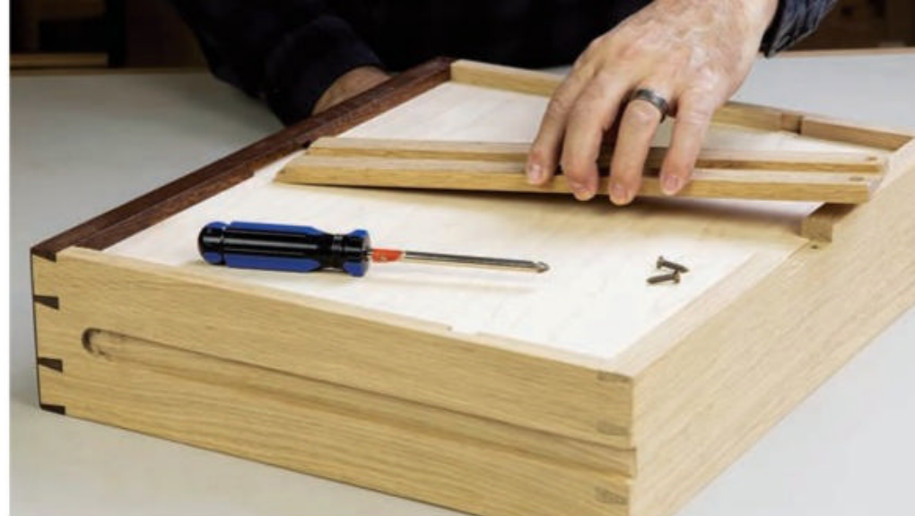
Insert the center track's tongue into the mortise below the drawer bottom in the drawer front, and drop it into the notch in the back of the drawer. Two screws at the rear secure the track to the drawer.
