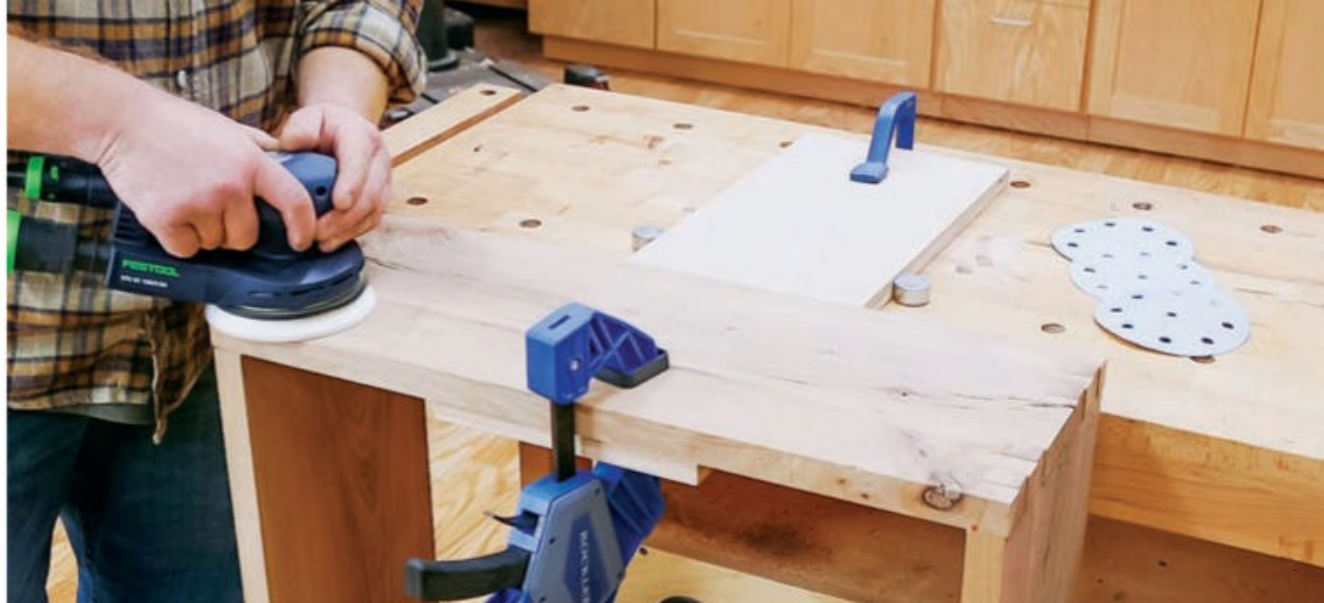
Flatten the protruding pins of all four joints with a sharp hand plane or with 60-grit sandpaper in a random orbit sander. Work up through the grits from there to 220. To avoid scratches, don't skip grits.
