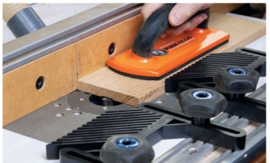
Lower the bit height to 1/16" and make a through groove in the filler strips with the same router table setup. This shallow groove will register the drawer slides in the perfect position, without trial and error.
