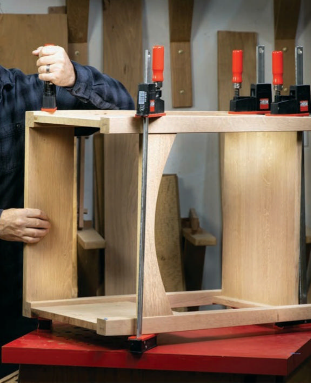
Bring the two side subassemblies together with the front rail, back rail, and shelf to complete the framework. The top edge of the front rail should be positioned 4" down from the tops of the front legs.
