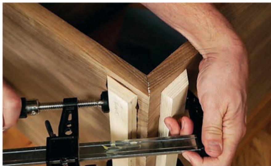
Clamping miter joints can be tricky, especially when glue is behaving as a lubricant before it sets. A pair of angled glue blocks, installed on each joint member with hide glue, can provide improved clamping surfaces.
