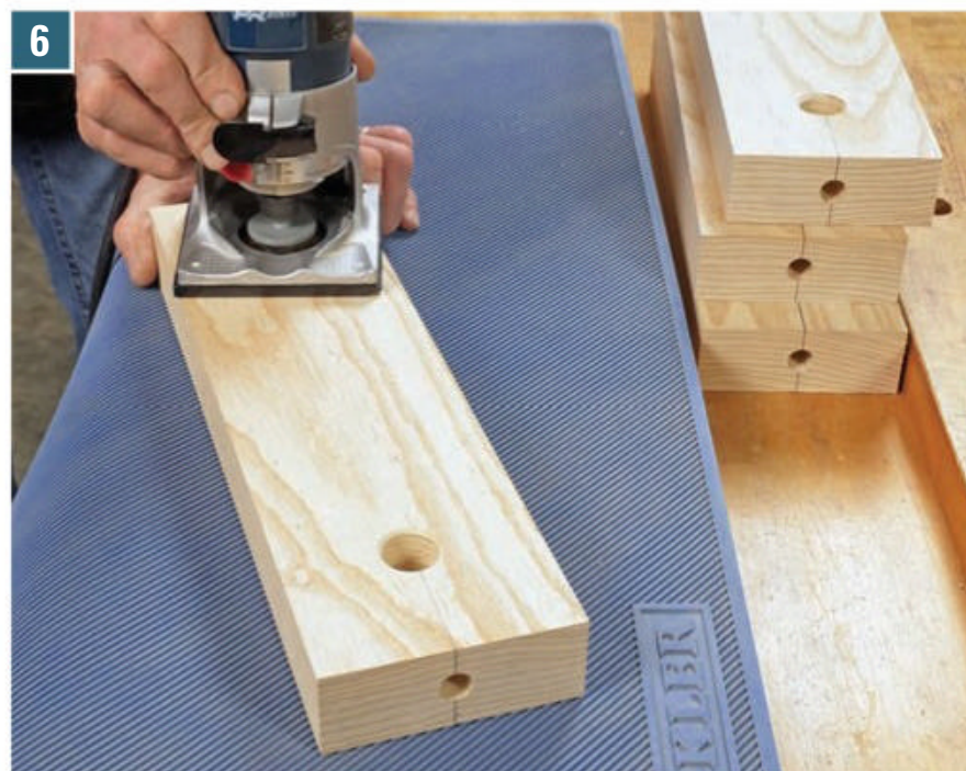
6 While this step isn't mandatory, easing the rims of the cross-dowel holes with a chamfering bit in a router is a good idea, because it creates a tidier-looking joint and removes any rough edges left by the Forstner bit.
