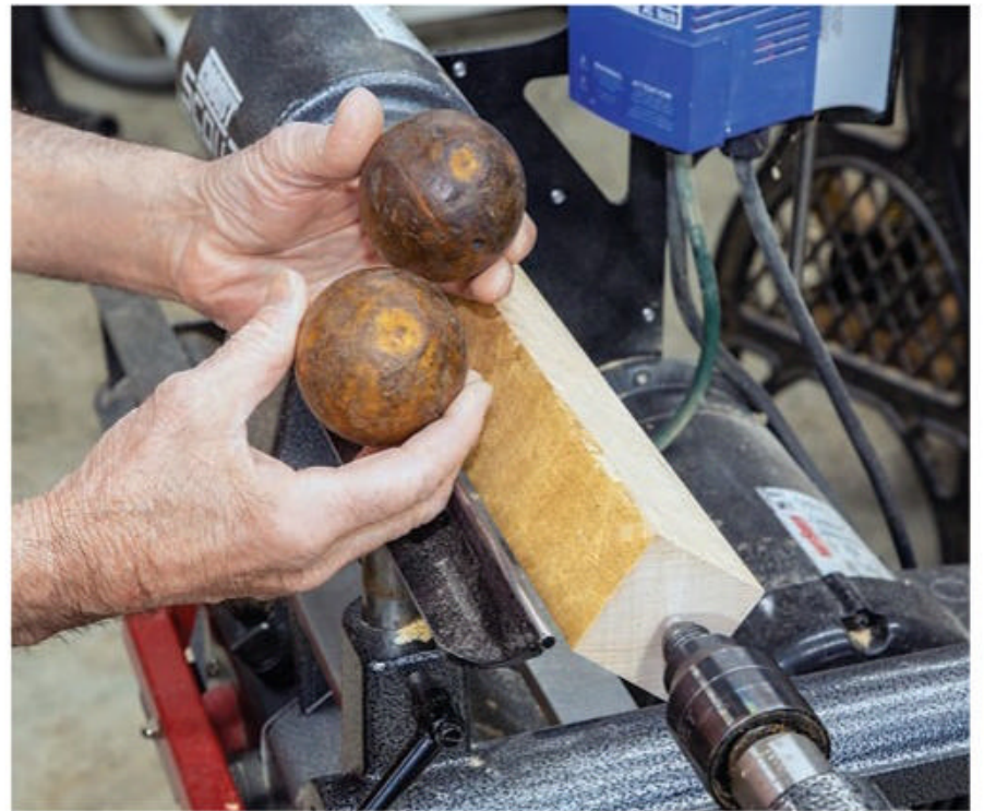
The antique wood balls are more lumps than orbs. Turned between centers, they have flat spots where they once were held in the lathe. The arc between the center points was likely turned by eye.
