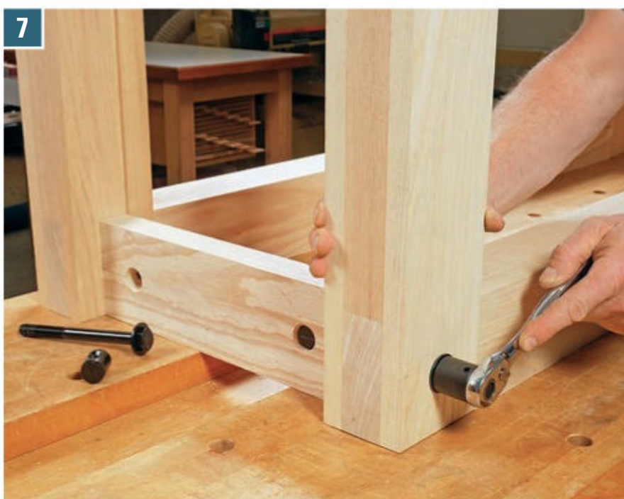
7 Insert the bolt and washer through the leg, and slip the cross dowel into its hole in the rail or stretcher. Align the parts so the bolt can engage the cross dowel. Tighten the hardware with a socket or a wrench.
