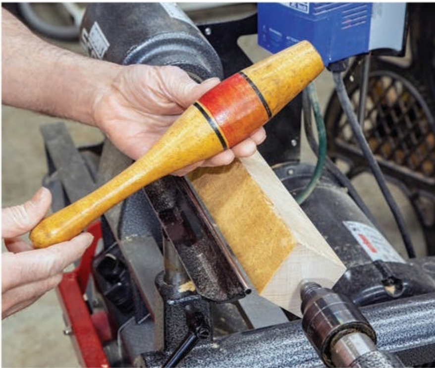
The author's antique pins were probably turned from green, or more likely, poorly seasoned wood. The telltale sign is that the pins have dried oval in cross section, which can be felt by turning them in hand.
