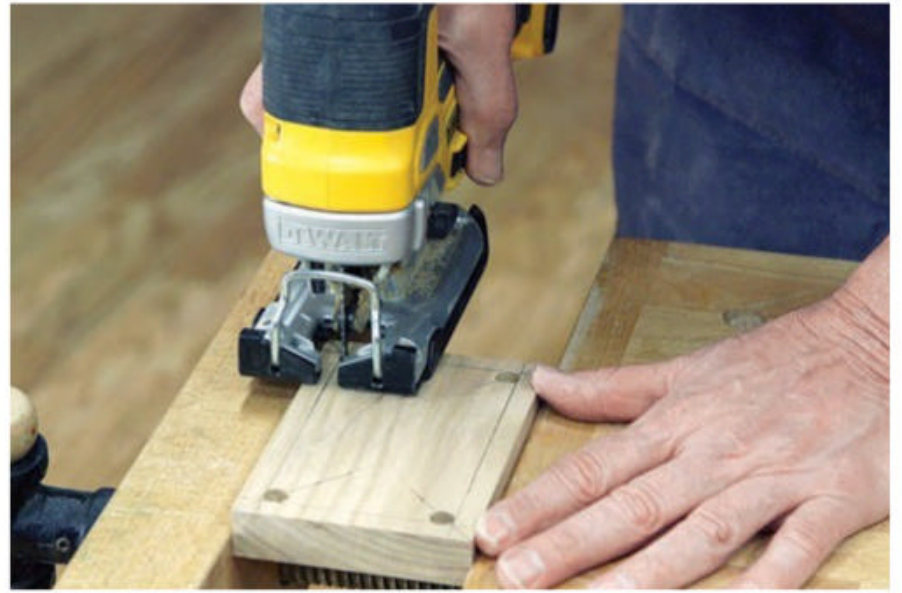
Cut from hole to hole in the block to remove the center section of the bit holder block. A good way to safely secure the block as it is cut is to use a bench vise. A handheld jigsaw is just the tool for the job.
