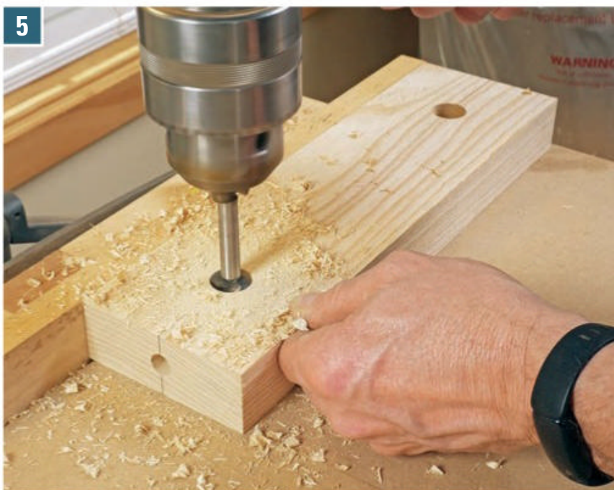
5 Bore a 7/8"-diameter hole through the rail or stretcher at the center point marked in the previous step to house the cross dowel. Use a backup board beneath the workpiece to ensure the bit will exit it cleanly.
