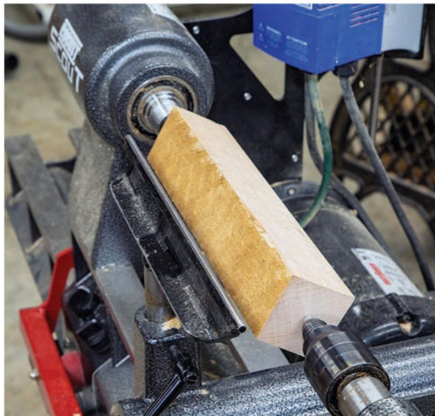
An 8/4 plank of hard or soft maple, ash, hickory, beech or birch will yield billets for pins with no lamination required. Crosscut the lumber into 12" lengths, then rip the pieces into square blanks. Mark their ends with centers so you can mount the pin blanks between drive and live centers.
