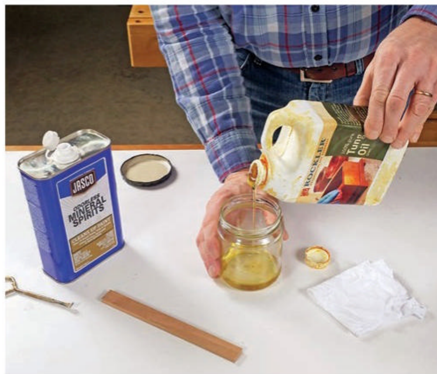
Tack cloths for cleaning wood that will be finished with an oil-based topcoat can be made by dampening a clean rag with a mixture of boiled linseed or tung oil and mineral spirits.
