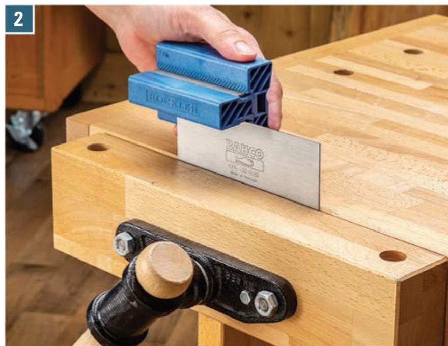
2 Flipping the sharpener over switches it from filing to honing — the second step of the sharpening regime. Super-fine diamond grit removes filing marks on the edge and sharpens its corners.
