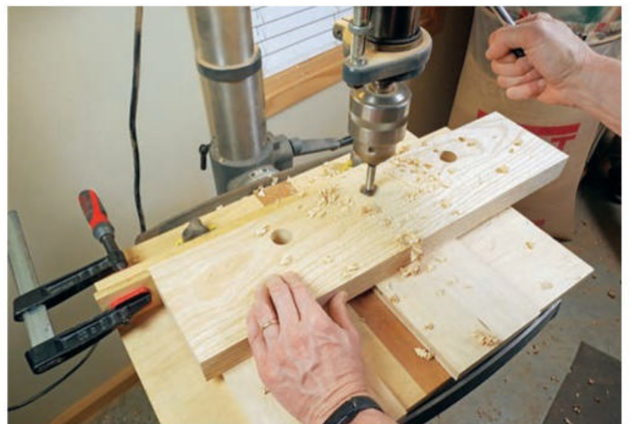
Use a 1 1/8"-diameter Forstner bit to bore holes through both wooden tail vise faces for the guide rods and center screw. Register each drilling position with a stop block so the holes line up exactly on both vise faces.
