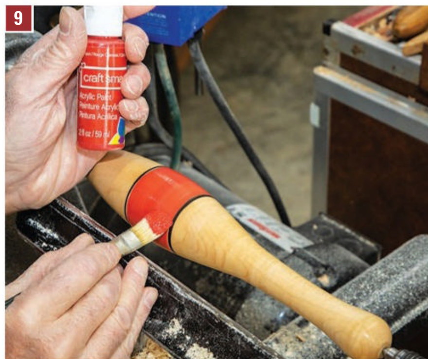
9 Acrylic paint, available at craft and art stores, is perfect for this embellishment. It sticks to shellac, dries quickly and forms a tough finish. Fill in the area between the pinstripes with your favorite color.
