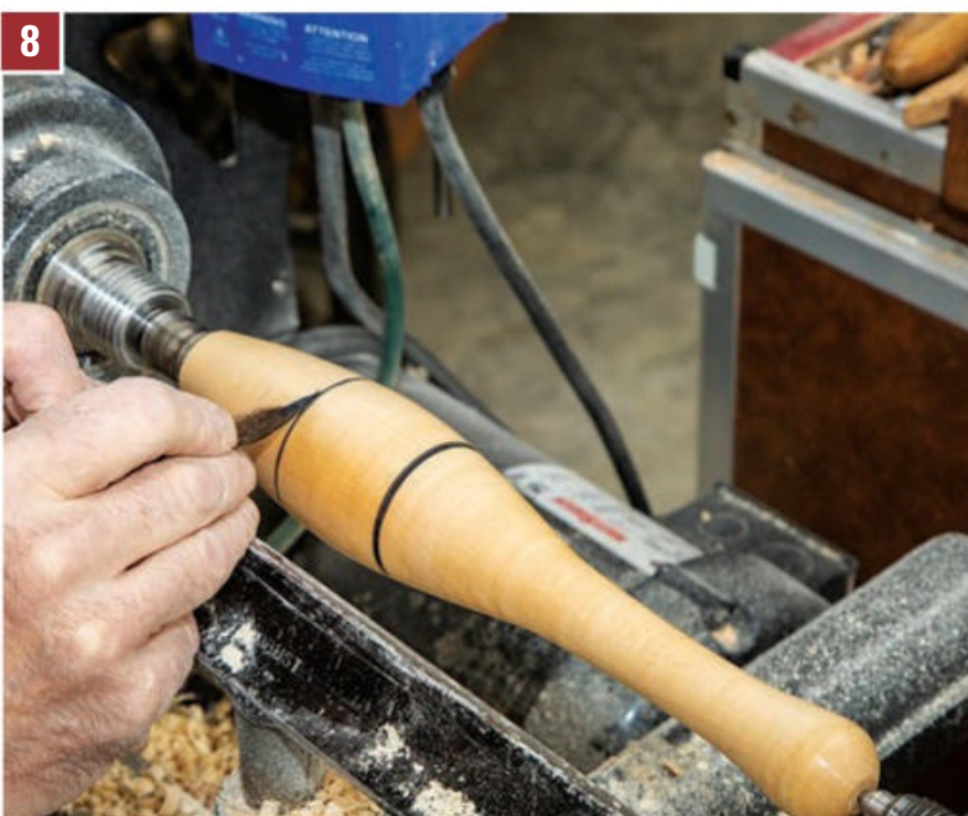
8 Placing the tool-rest an inch or so away from the bowling pin provides a helpful rest for steadying your hand when painting both pinstripes. The author located the second stripe at the pin's largest diameter.
