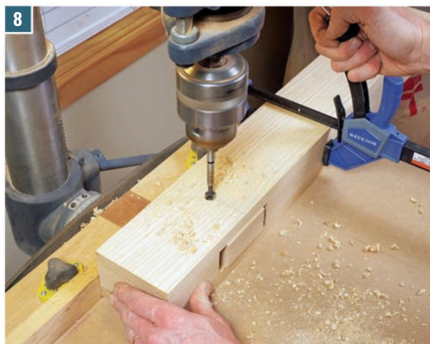
8 Drilling Variation, Step 1: If you don't have a doweling jig, you can still install this hardware. Drill the bolt hole through the leg at a drill press, if at all possible. It's imperative that this hole runs through the leg squarely.
