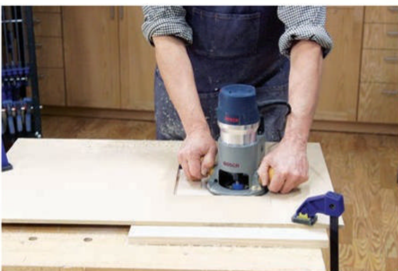
Locate the recessed tray section of the base using a template made of 3/8" MDF or something similar. The author sized his template's opening so the rim of the router base could be used as a contact edge against it. Clamp the template securely in place and use a 1 1/4"-diameter bowl-carving bit to form the tray. The bit forms gently curved edges that flow down to a flat recessed area.
