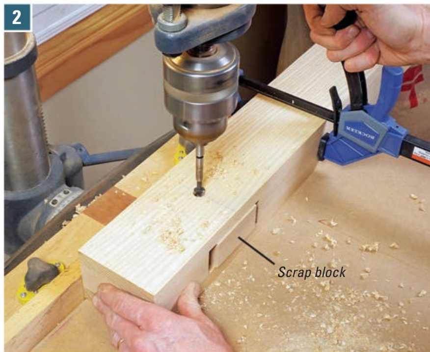
2 Chuck a 1/2"-diameter twist, brad-point or Forstner bit in a drill press, and bore the bolt hole all the way through the leg. In this photo, the leg mortise is filled with a scrap block to prevent tearout inside the mortise area.
