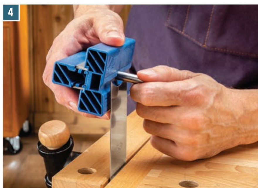
4 The angled fence held against the scraper's face in Step 4 tilts the burnishing rod about 10 degrees past square. When it's pressed along the scraper's edge, the rod turns the burr downward to complete it.
