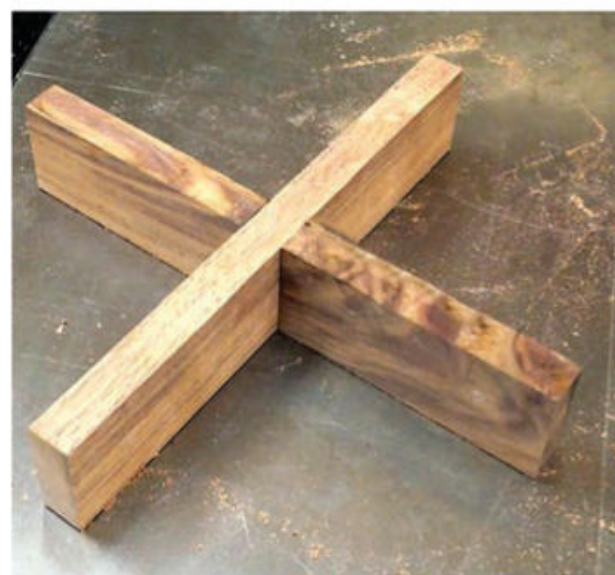
Clamp the supports (pieces 2) together and cut 3/4"-wide x 1"-deep notches at their centers. It's best to cut the notches a little narrow and short so that you can then sneak up on a final tight fit with a file.
