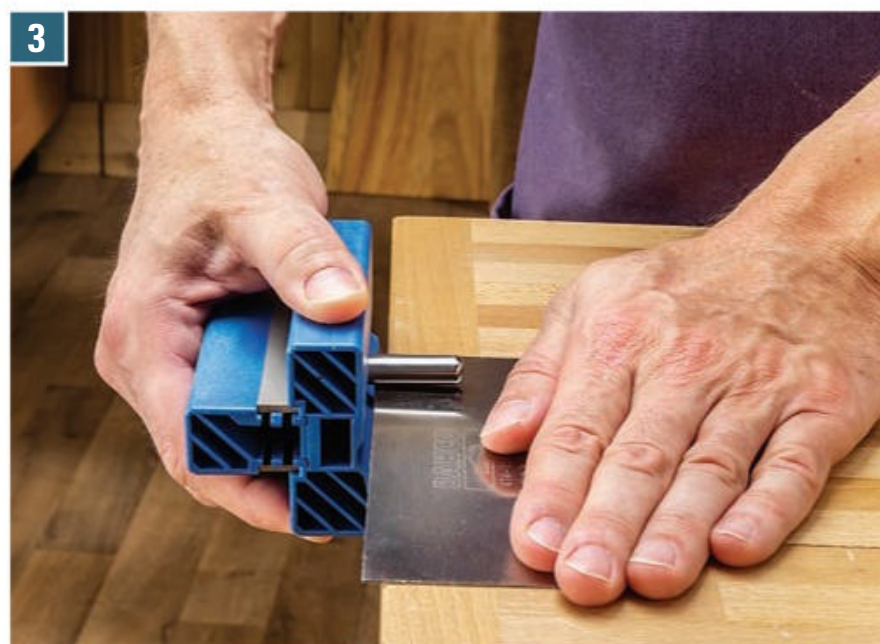
3 A hardened-steel burnishing rod is used next for Step 3, to draw the scraper's corners out into burrs that extend beyond its edge. A few passes along the corner, pressing down with moderate pressure, is all it takes.
