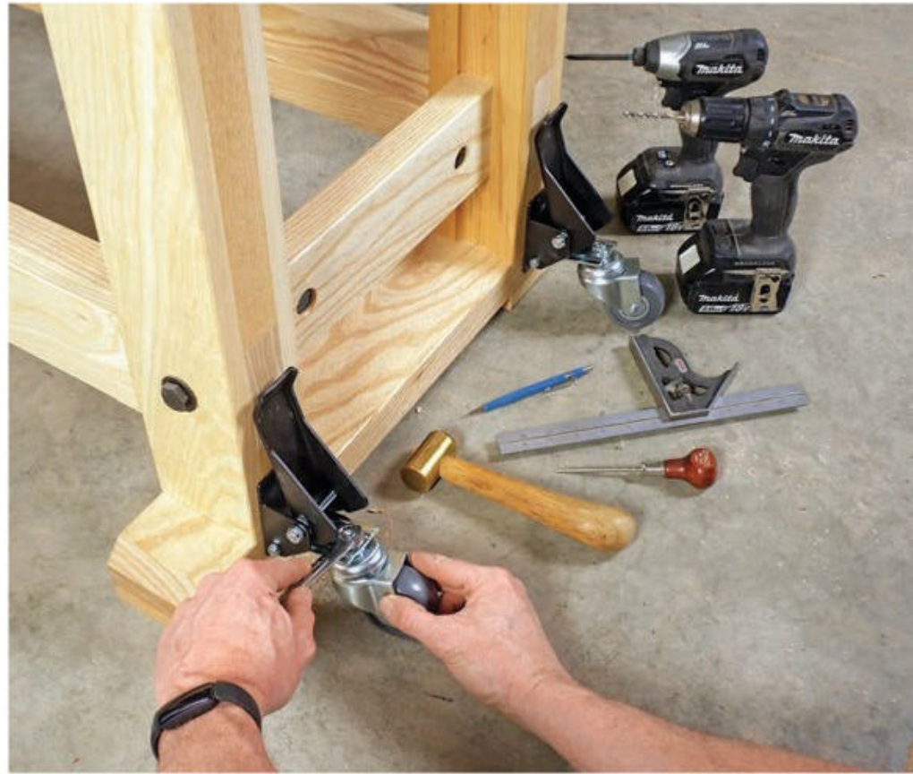
Rockler's heavy-duty workbench casters flip up or down with a foot lever. They make it easy to park this bench wherever it's needed or roll it out of the way conveniently without lifting or straining.
