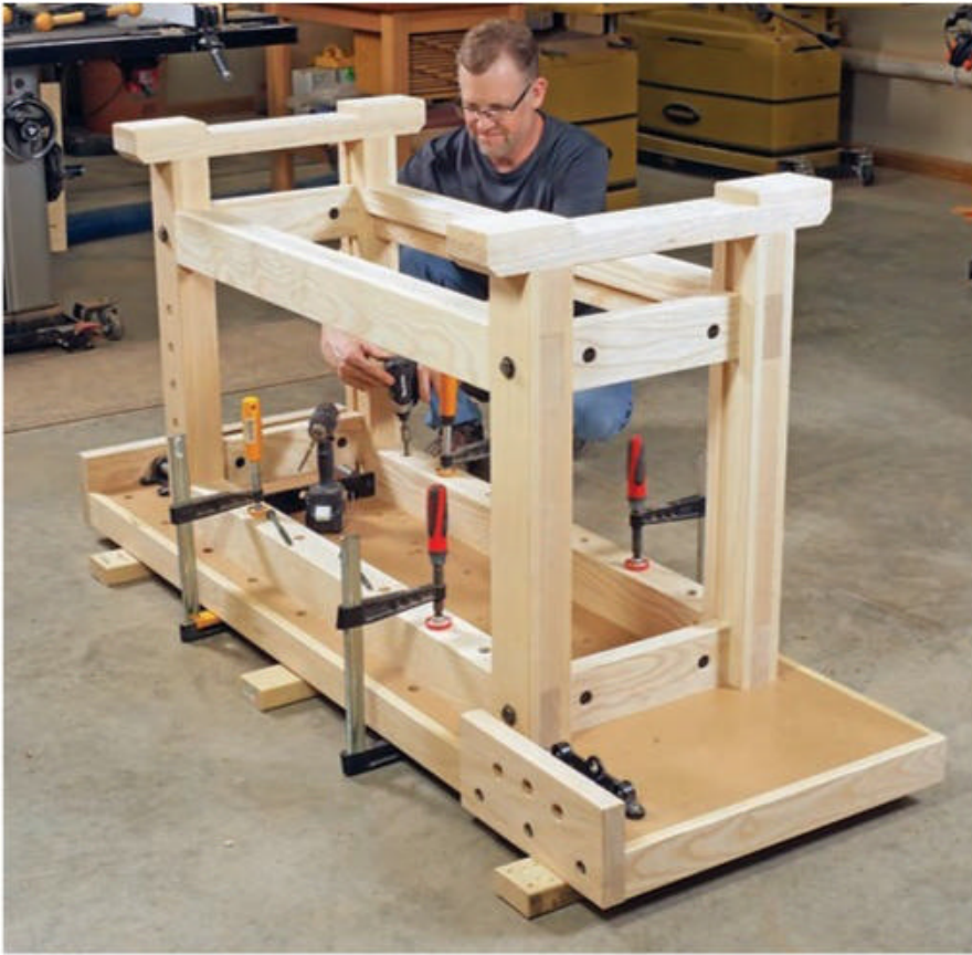
Set the benchtop down onto scraps on the floor. Position the base frame over it, checking carefully that the bench dog holes aren't obstructed and the tail vise moves freely. Fasten the components with 6" lag screws.
