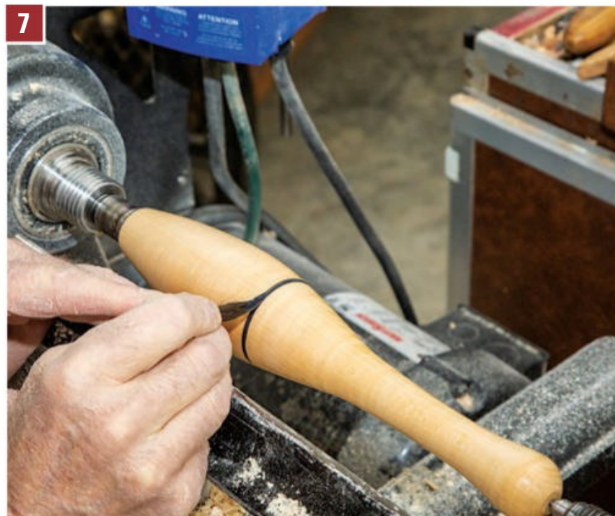
7 Clear shellac makes a durable, quick-drying topcoat that's easy to apply to the pins with a brush, then burnish smooth with shavings. Once it dried, the author set the lathe to a slow speed and in reverse. He used a stripping brush to apply a thin pinstripe just above the pin's large diameter.
