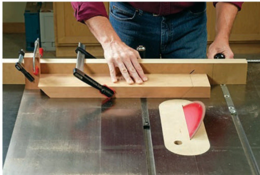
Closed forms created with miter joints will require that each workpiece is cut to precise length or width. When possible, use a stop block clamped to a fence (here on a table saw miter gauge setup) to control part lengths.
