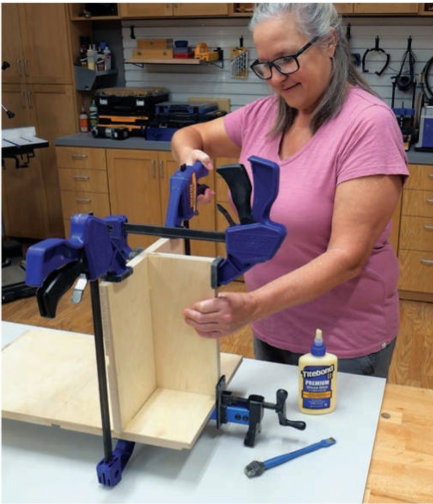
Dry-fit the pieces together to confirm the parts are all correct. Then glue and clamp subassemblies of the dog steps in manageable groups, a few parts at a time. Check routinely for square as you proceed.
