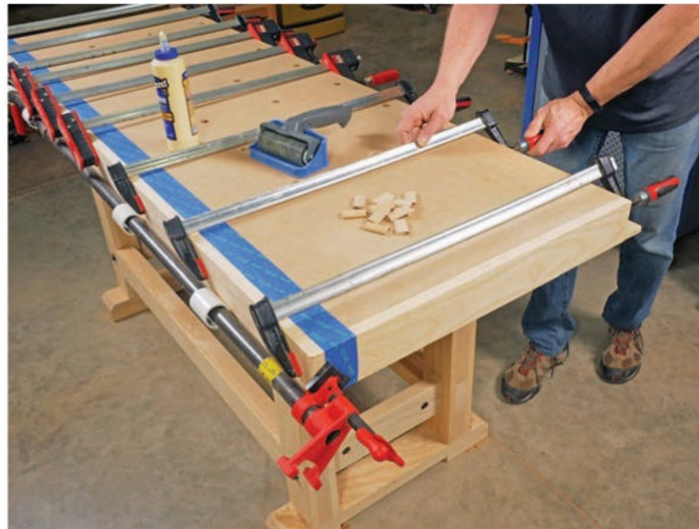
Lots of clamps is the name of the game for attaching the edging pieces to the MDF core. Strips of painter's tape can prevent glue squeeze-out from sticking to the MDF.
