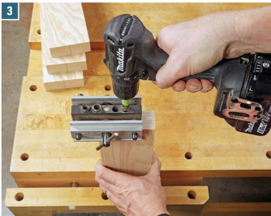
3 Mark the bolt hole location on the end of the rail or stretcher. Then use a doweling jig to drill it carefully, making sure the hole penetrates straight into the workpiece and deep enough to intersect the cross-dowel hole.
