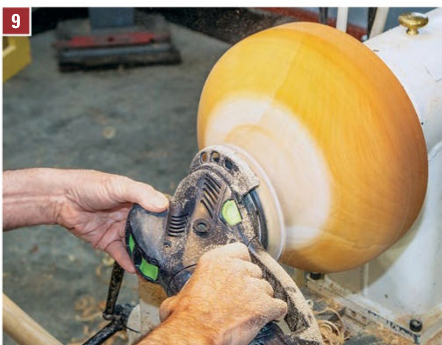
9 Sand the bottom and outside to 220-grit as was done on the inside, being careful to remove all traces of tearout. Power-sanding with a random-orbit sander is a fast method, but hand-sanding will also yield good results.
