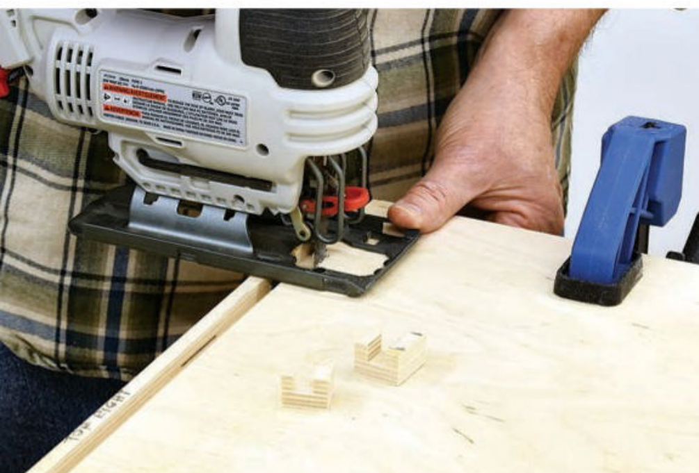
Using a jigsaw or handsaw, cut the exit holes for the four leaf supports. Use a fine-cutting wood blade or even a metal-cutting blade and set your saw's orbital action to zero to prevent splintering.
