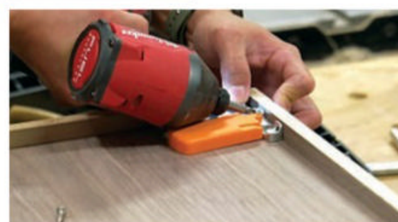
The author adjusted his banded plywood drawer faces with playing cards to achieve an even gap all around before attaching the drawer faces to the boxes with screws and metal drawer pulls.
