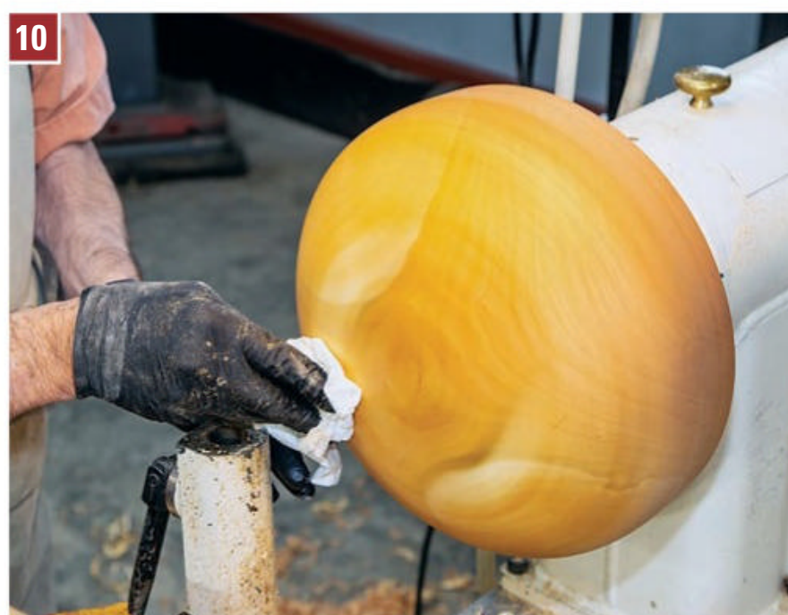
10 It will take three or more coats of finish to bring the sheen to a level that Hawaiian culture demands. Subsequent coats can be done off the lathe or on the lathe if you have a vacuum chuck.
