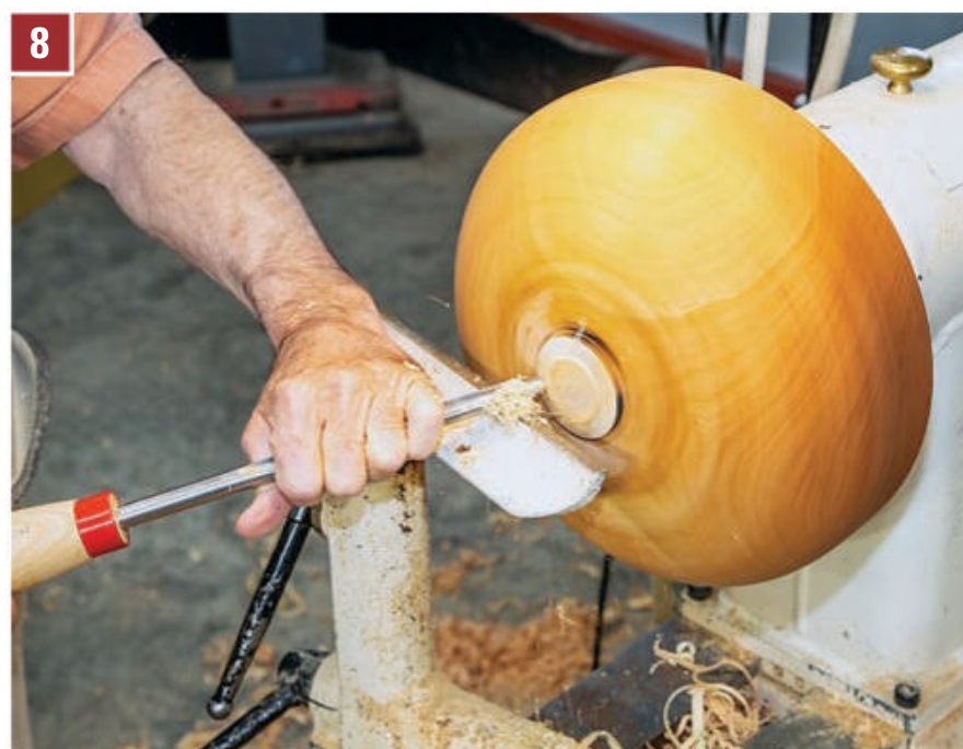
8 Reverse the bowl onto either a jam chuck or a vacuum chuck. Turn the bottom to a very uniform, convex shape, and bring the wall of the bowl to a constant thickness from the rim to the center of the base.
