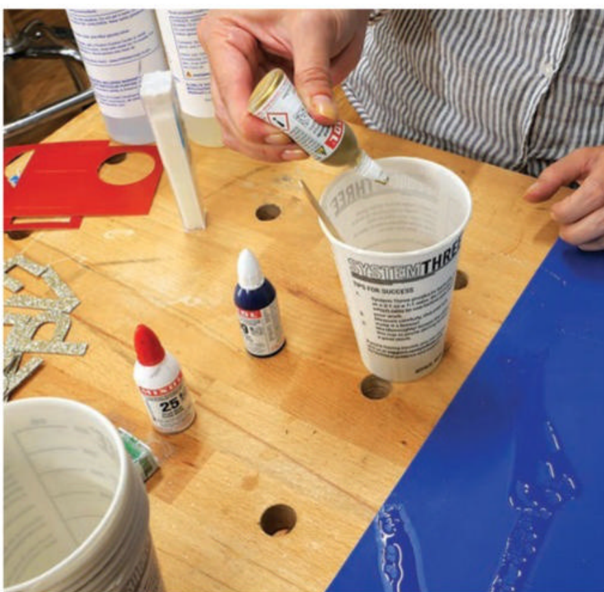
A variety of colorants can help to create dynamic pours, too. Be sure to mix the colorant thoroughly into the resin to achieve an even tint.
