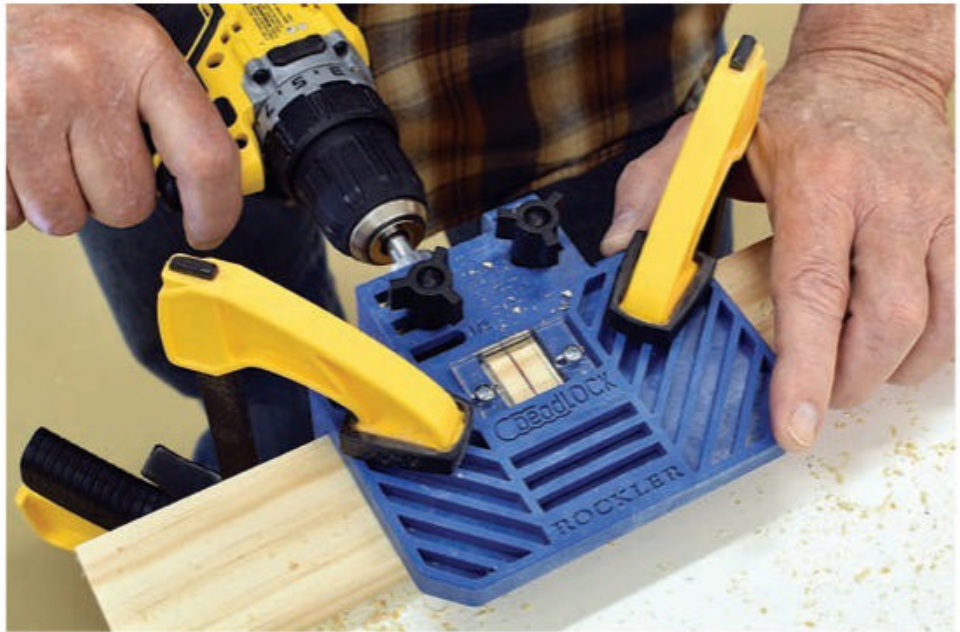
The Beadlock jig can be used in various orientations to suit different joint applications. Notice here how the alignment line is visible through the jig's window, making it easier to register the jig accurately before drilling.
