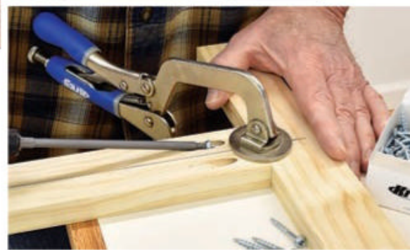
Deluxe pocket-hole jigs have a built-in clamping system for securing workpieces, plus extensions for supporting long parts. After the holes are bored into one workpiece and the joint is clamped together, special self-drilling screws complete the assembly (inset).
