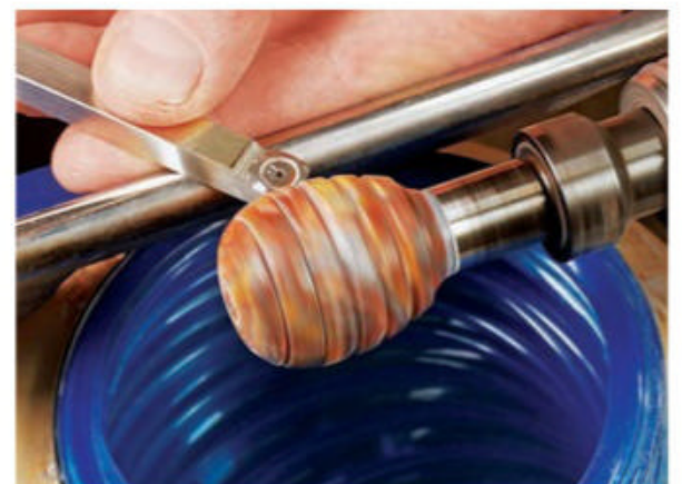
Score a series of shallow lines in the knob to establish the limits of each cove. Widen these lines into V-notches with the corner of a square cutter to begin the bead-making process.
