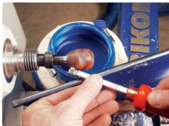
Turn the cylinder into an ovoid that resembles a guitar pick or hot-air balloon. Square- and round-edge cutters make quick and easy work of this shaping process.
