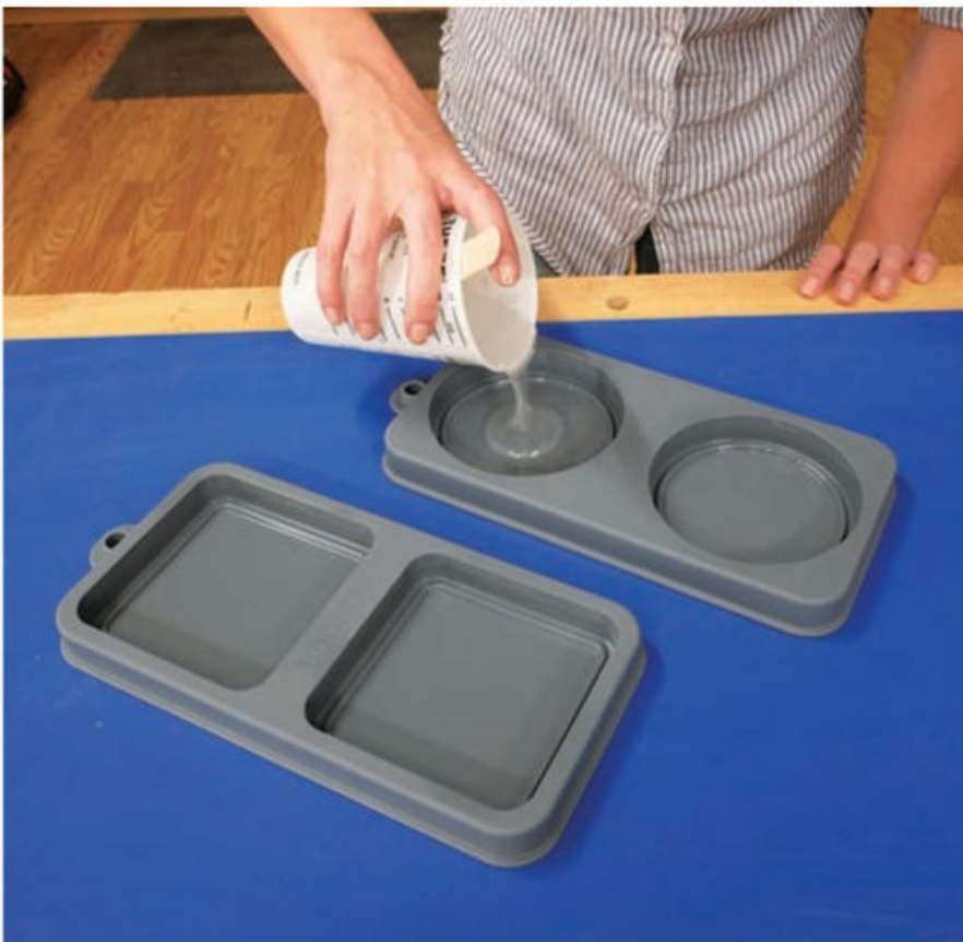
For this set of coasters, the author poured a thin layer of resin into the molds, deep enough to fill the lower lip.
