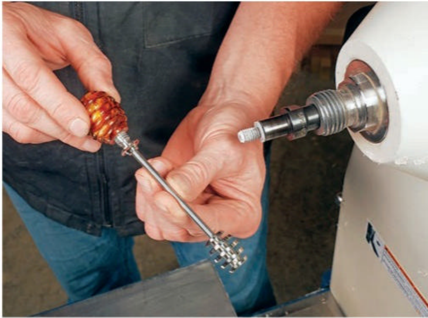
Buff the knob to a glossy sheen with a liquid scratch remover such as Novus #2. Then carefully unscrew the knob from the mandrel and blow out any dust inside the threaded hole. Screw it onto the honey dipper.
