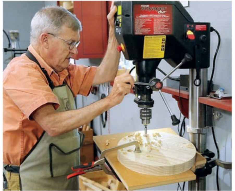
Bore a 1"-diameter through hole for each leg socket with your drill press table tilted to 11 degrees. The author used a Fisch Wave Cutter Forstner bit. A backer board helped to align these holes and minimize tearout.
