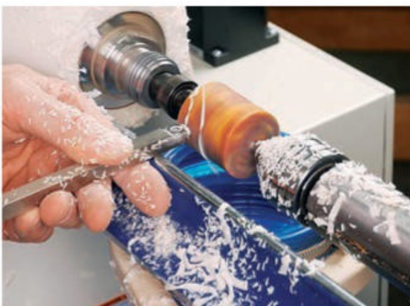
Rough the blank into a 1¼"-diameter cylinder with a carbide-insert turning tool. The author’s tools were equipped with Easy Wood Tools negative-rake cutters for turning composites.
