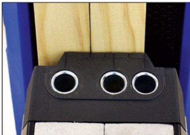
Depending on the size of the workpiece and number of holes desired, line up the workpiece with the appropriate registration lines when clamping up stock in a pocket-hole jig.
