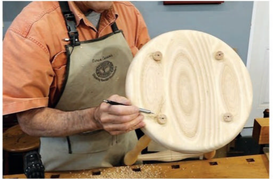
Adding wood wedges to the leg tenons will lock them in place. Arrange these wedges by penciling a line across the center of each leg tenon. Draw the lines perpendicular to the seat's grain direction.
