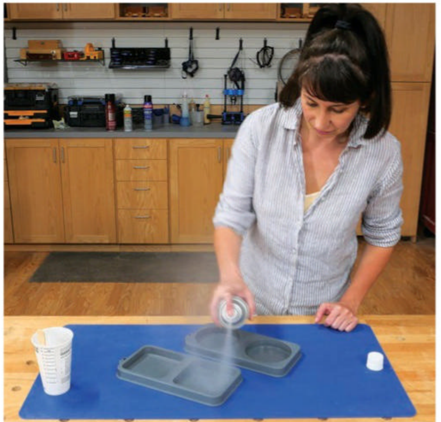
Spraying Rockler's silicone molds with a mold release isn't imperative, but it will help make the coasters easier to pop out when they cure hard. It will also help to protect the molds over time.
