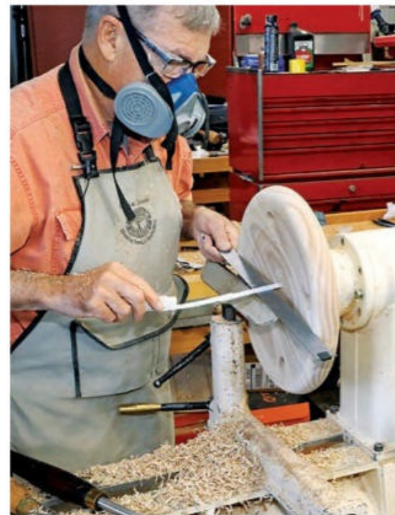
After rounding over the seat's top and bottom edges, dish out the top face about \frac{3}{4} " deep for added seating comfort. Check your progress by placing a straightedge across the seat's face and using a ruler to measure the depth.
