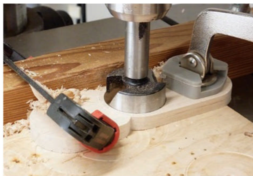
Before drilling the candle holes, stabilize the fragile end of the piece being drilled by butting it against the matching curve of a bottom side piece (E). Adjust the drill press to the correct speed for the bit size.
