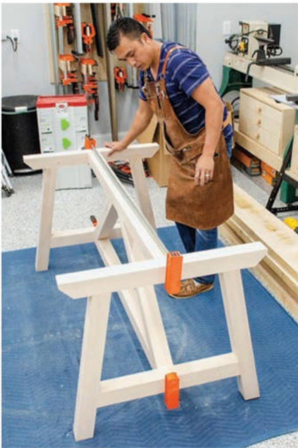
Once the Beadlock mortises are drilled, glue up the table's two trestle subassemblies. Notice that each joint receives two 1/2" Beadlock tenons and the use of clamping cauls across the leg/lower cross support joints.
