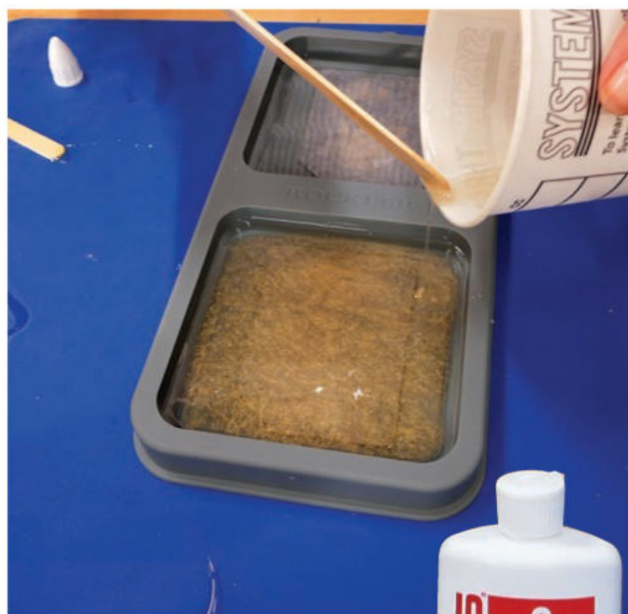
Mica powder (above) can add sparkle to a coaster. Once the resin cures, buff it to a glossy finish with Novus #2 Fine Scratch Remover (Rockler item 58280; $8.99).
