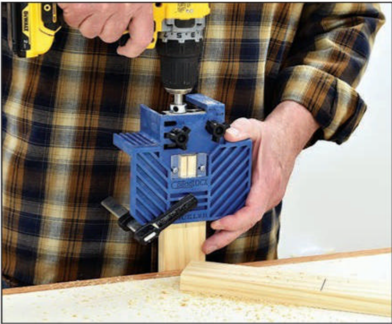
Like a doweling jig, the Beadlock loose-tenon system uses a drill to create a mortised joint. A hardened-steel drilling guide inside the jig enables a series of overlapping holes to be drilled.
