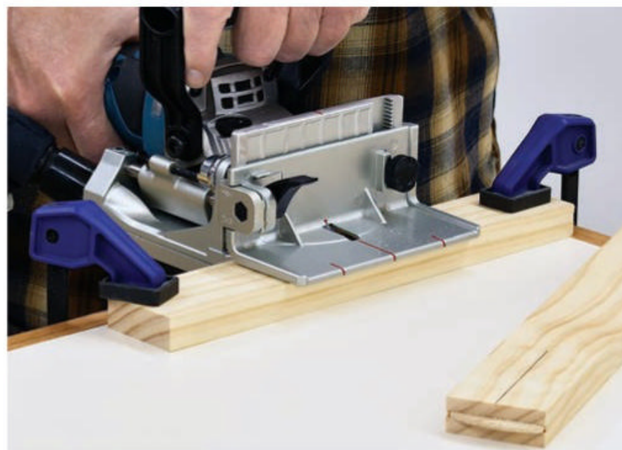
With the workpiece secure and the biscuit joiner's fence in place, slide the body of the tool forward into the wood to cut a concave biscuit slot.
