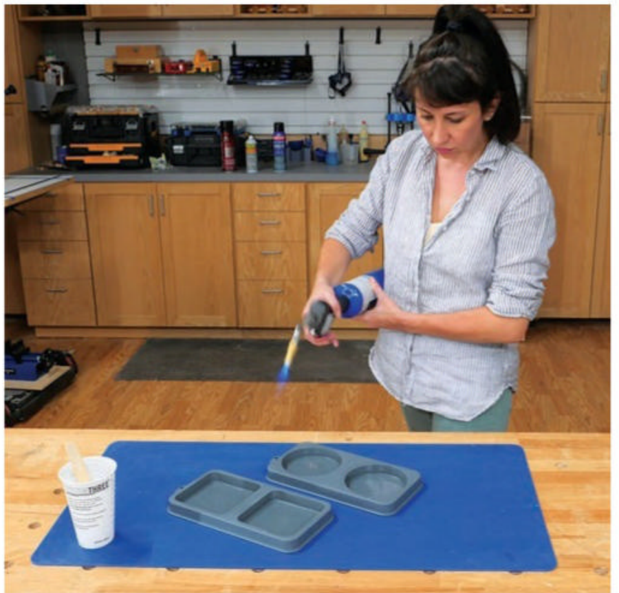
Bubbles can form in the newly poured resin. They're easy to remove, either with a quick pass of a torch or by misting with isopropyl alcohol.
