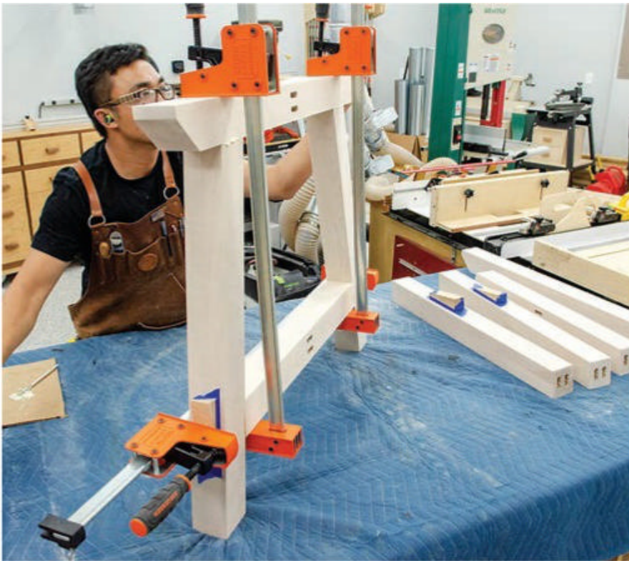
Once the Beadlock mortises are drilled, glue up the table's two trestle subassemblies. Notice that each joint receives two 1/2" Beadlock tenons and the use of clamping cauls across the leg/lower cross support joints.
