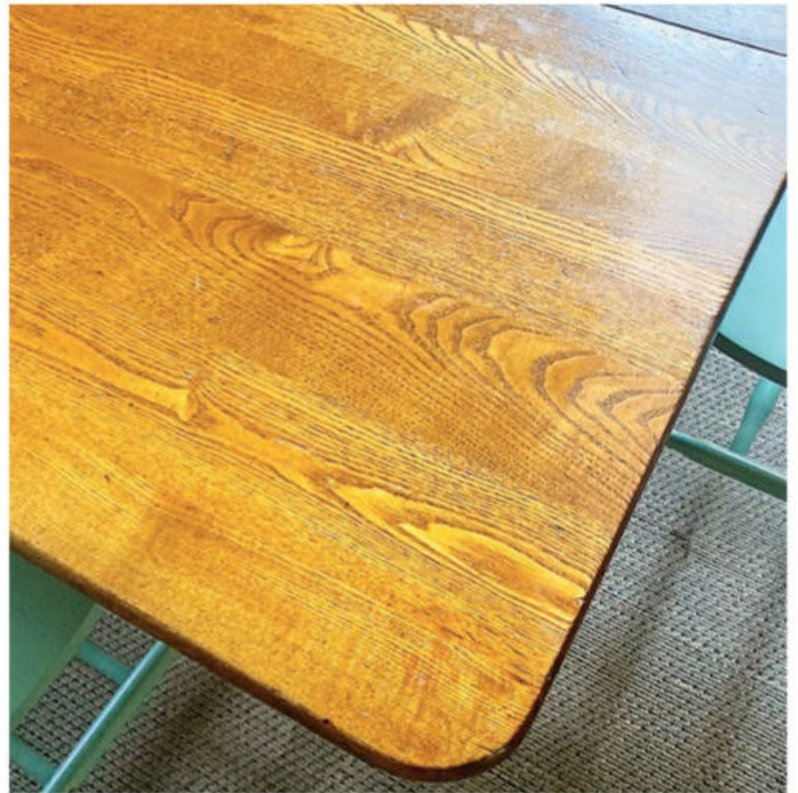
Vintage oil/varnish finishes can begin to turn gummy as they age. On this table, it has resulted in a soft finish that becomes sticky when heated by warm coffee cups and cookware. Refinishing will improve durability.
