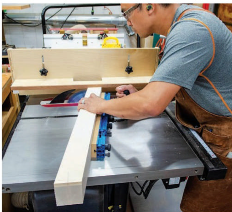
Angle-cut the part ends at 10 or 40 degrees, depending on the component. The author made these cuts with the appropriate template secured to the top of the workpiece with double-sided carpet tape.
