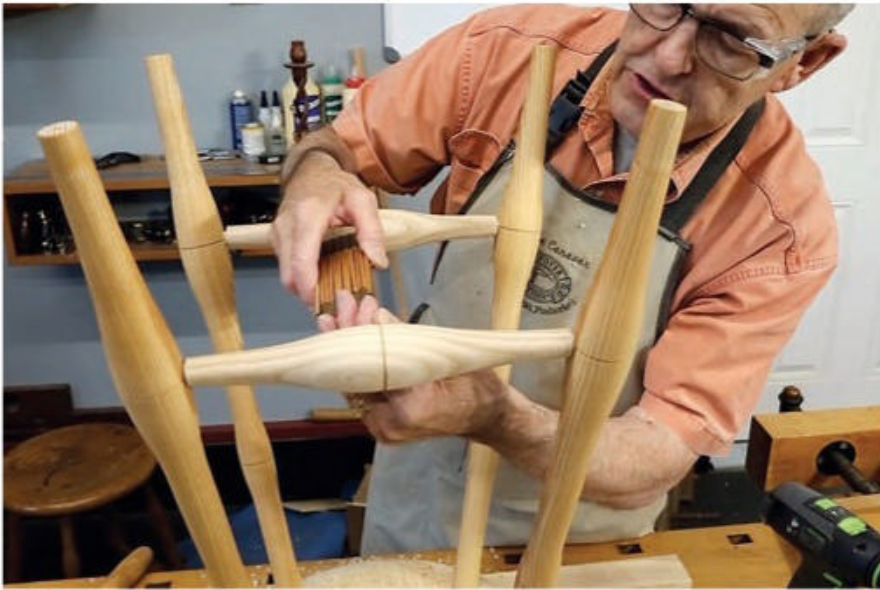
Dry-fit the side stretchers between the legs, then measure the distance between their bobbins at the grooves. The center stretcher's length is this span plus 1\frac{9}{16} ". Cut a billet and turn it to shape with a centered bobbin.
