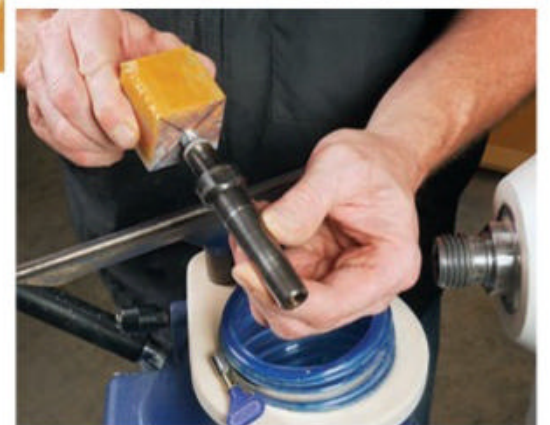
Bore a centered hole into one end of the blank using a 19/64" or 5/16" twist bit. Then carefully cut threads for the honey dipper with a 3/8"-16 tap. This enables the blank to mount to Rockler’s #62683 turning mandrel (inset).
