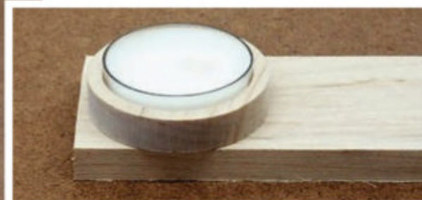
Determine the overall candle hole depth on scrap wood that will make the tea candles easy to insert or remove (left). This depth, minus 3/8", sets the shallow hole drilling depth (inset).
