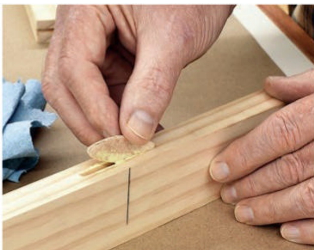
Apply glue to the biscuit and into the slot, then slide the biscuit down into place.
