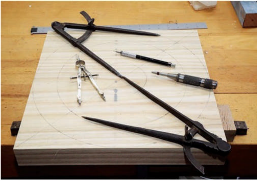
Find the center point of the seat blank's bottom face with two diagonal lines, then use a compass to draw three circles at the center point to mark the seat's outer rim, leg socket locations and your faceplate's diameter.
