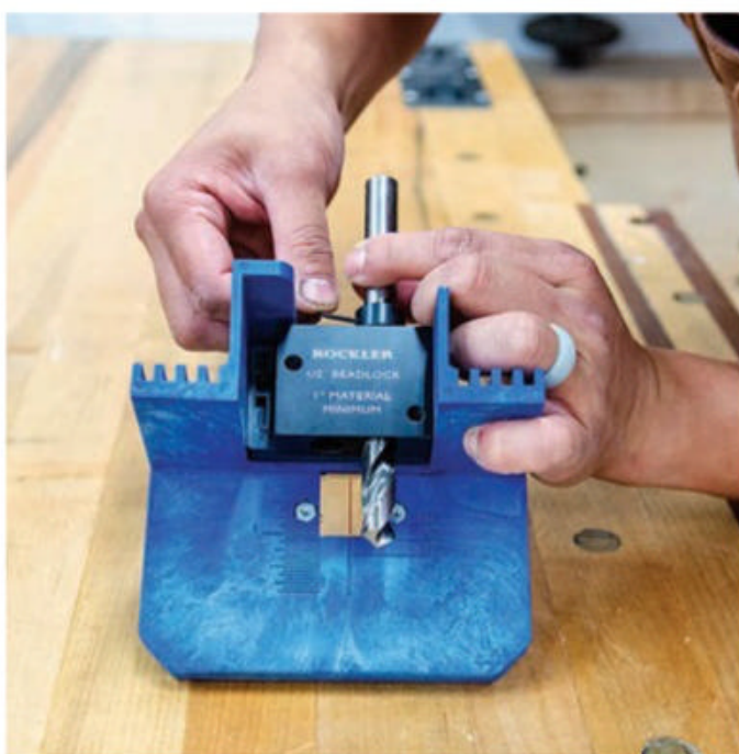
Angle-cut the part ends at 10 or 40 degrees, depending on the component. The author made these cuts with the appropriate template secured to the top of the workpiece with double-sided carpet tape.
