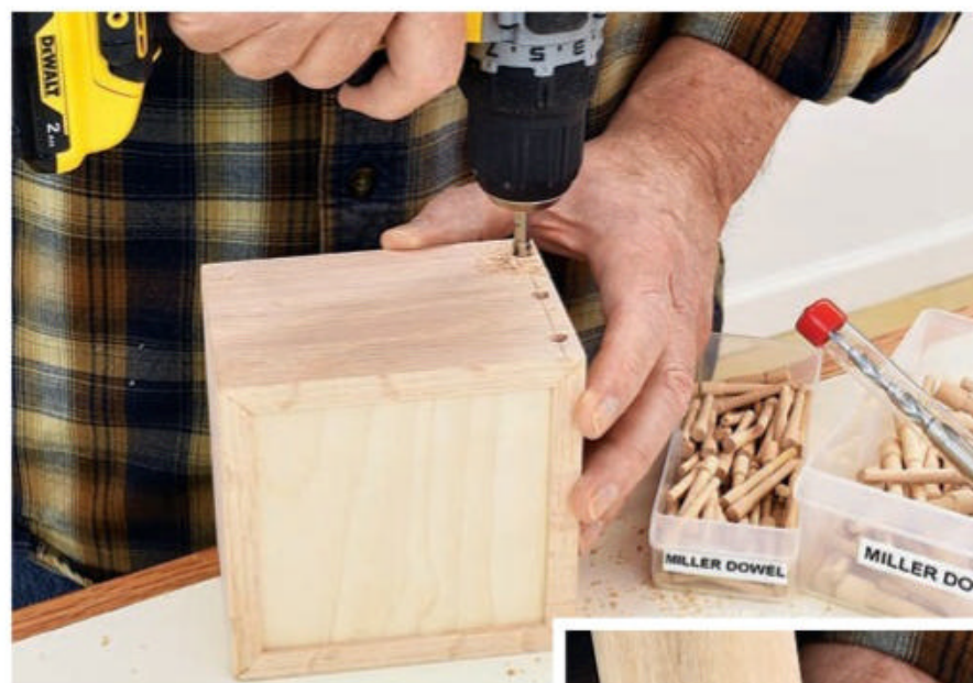
Doweling can also be done after a project is completed to add both strength and a decorative flair. Here, the author adds Miller dowels to a finished box.
