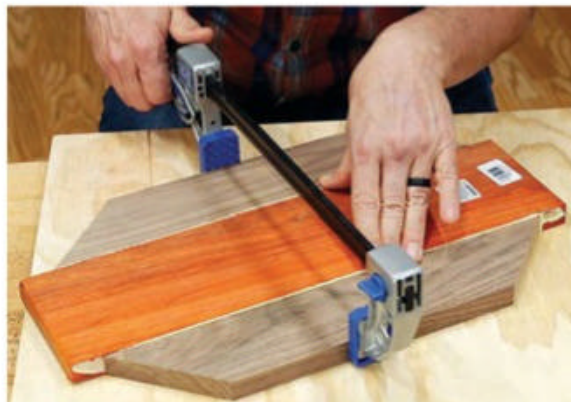
Use three clamps to glue the tray components together. The center paduk board extends past the outer walnut boards by 1" on each end.
