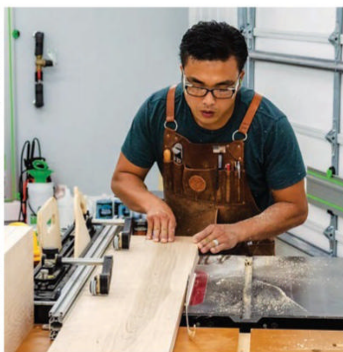
After planing his maple tabletop boards to 1 1/4" thick (left photo), the author flattened their edges and brought them into parallel on the table saw using a glue-line ripping blade (inset). He reports that the sawn edges require no further dressing on the jointer to be ready for glue and clamps.
