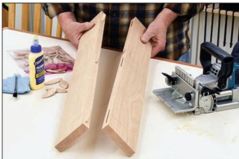
Biscuits used for edge joints align workpieces perfectly and keep them from slipping while being clamped.
