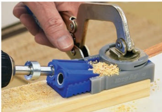
The simplest and most economical pocket hole jigs clamp to the workpiece. This also enables them to retrofit to already-assembled projects, if needed.
