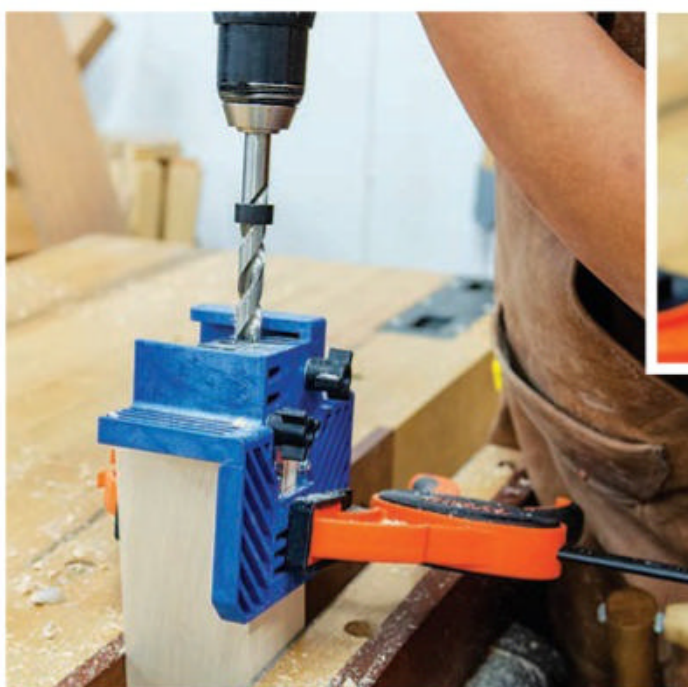
Drilling \frac{1}{2} " Beadlock joints involves boring two holes at the jig's "A" position and a third hole at the "B" position to create the overlapping, three-hole mortise pattern (inset). The author drilled each mortise \frac{1}{4} " deep to fit 2\frac{1}{2} "-long precut Beadlock tenons (left, center photos).
