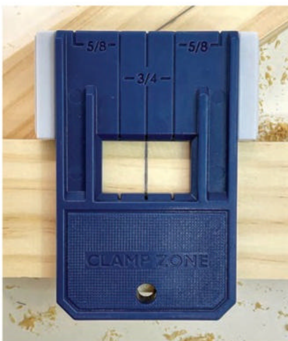
Alignment is critical for dowel joints. Make sure the jig is positioned carefully and square to the workpiece before clamping it into place.
