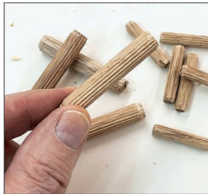
Dowel "pins" for joinery incorporate grooves or spirals that allow glue to spread evenly when they're driven in.
