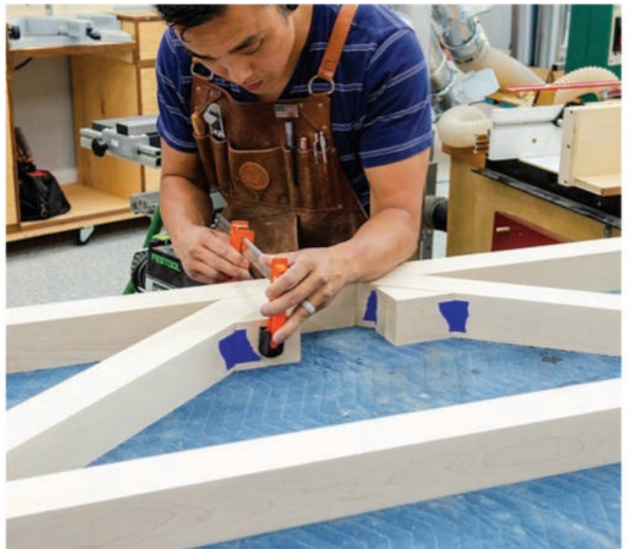
Assemble the long stretchers and diagonal braces to form a third table base subassembly. Here again, the author employed clamping cauls at the top and bottom ends of the diagonal braces to bring these joints together.
