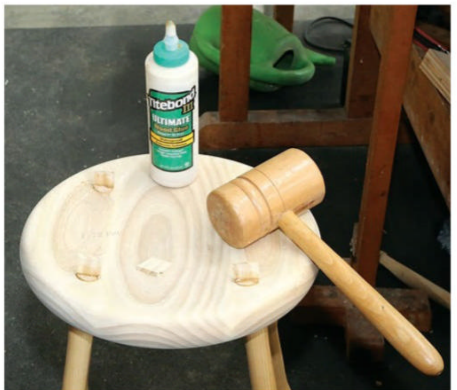
Saw slots in the leg tenons, assemble the chair and drive a wedge into each tenon. Use a slow-setting glue such as Titebond III or 90-minute epoxy to provide ample working time for this assembly process.
