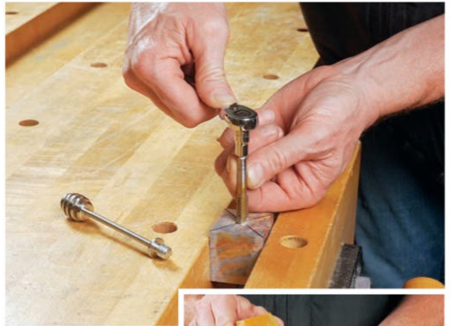
Bore a centered hole into one end of the blank using a 19/64" or 5/16" twist bit. Then carefully cut threads for the honey dipper with a 3/8"-16 tap. This enables the blank to mount to Rockler’s #62683 turning mandrel (inset).
