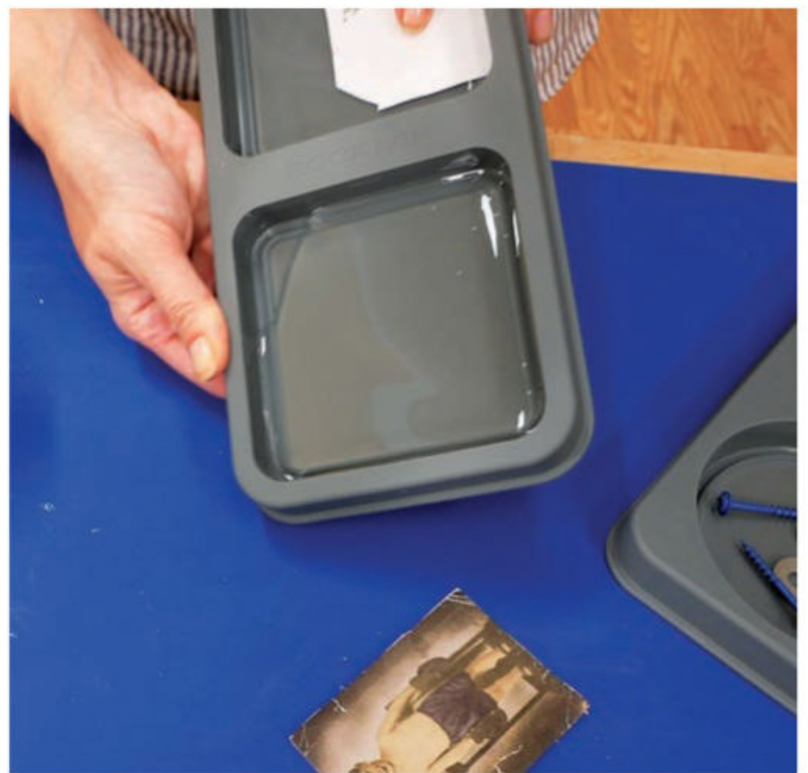
Gently tilt the mold if needed to spread and level the liquid resin, and be aware that the epoxy will begin to harden quickly. Don't dally!
