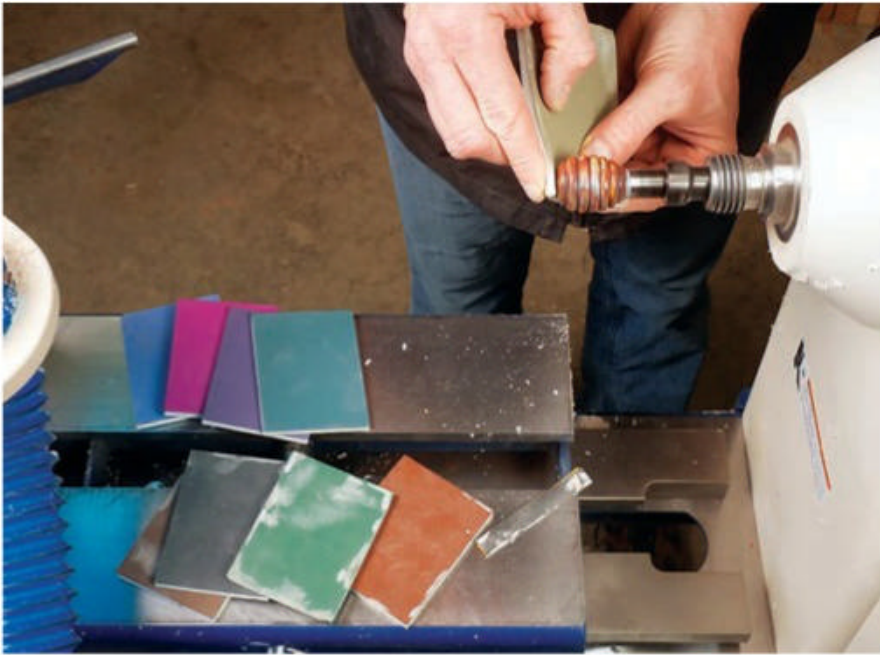
The author used a set of color-coded, foam-backed micro abrasives to sand away all evidence of tool scratches. Light pressure is all that's required here. Sanding up through the grits takes just a few minutes.
