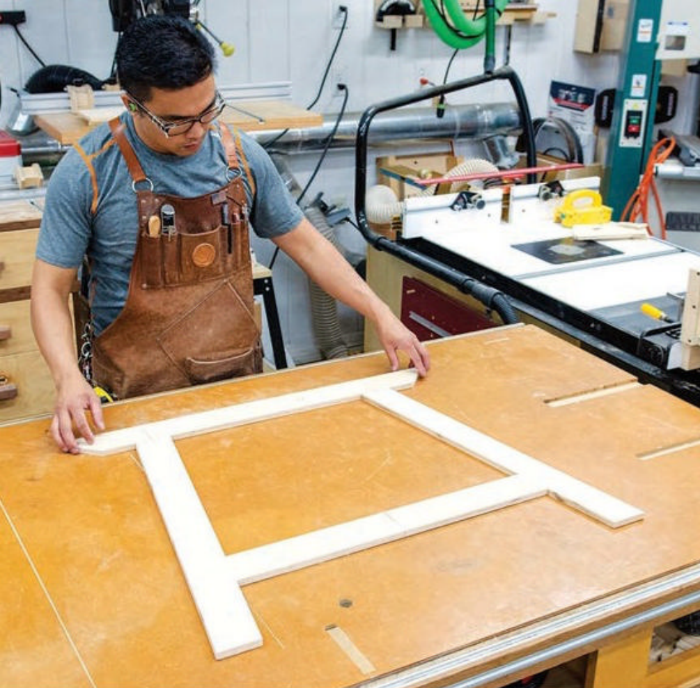
The author arranged his leg and upper and lower cross support templates on a large work surface in order to check their alignment and to extend Beadlock layout lines across each joint.
