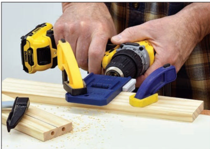
You don't always need a vise to use a doweling jig. Clamping the wood and jig directly to a bench or worktable is fine — and sometimes easier.
