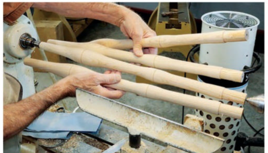
Shaping the four legs is straightforward spindle turning using a roughing out gouge and either a spindle gouge or a skew. The goal is to create four legs with matching profiles and a 1"-diameter, 2"-long tenon on top.
