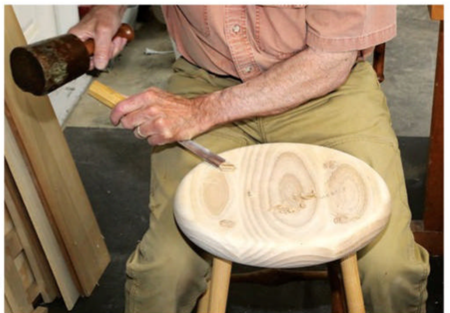
The author used a fishtail gouge to trim the protruding tenons flush with the seat. Tap the chisel around the circumference of each tenon to score it, and work inward, being careful not to chip out the end-grain fibers.
