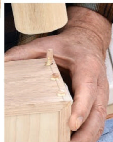
Doweling can also be done after a project is completed to add both strength and a decorative flair. Here, the author adds Miller dowels to a finished box.
