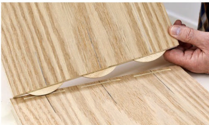
Biscuits can also be used in corner joints for building casework such as cabinets, consoles, boxes and shelves.
