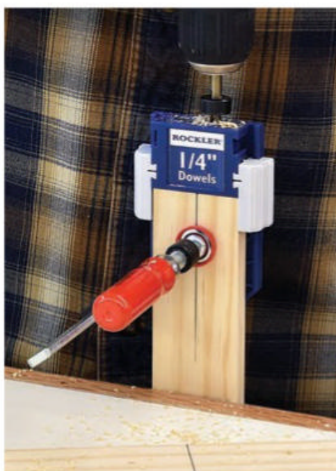
With the doweling jig set and clamped, a few quick plunges with a stopped drill bit creates half the joint.
