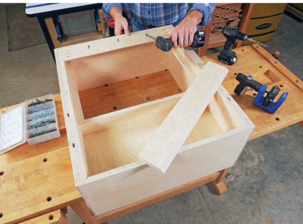
Install two French cleats with their bevels facing inward and down. One fits inside the upper back of the cabinet (being installed here). Position the second cleat so its non-beveled edge is 9" up from the cabinet bottom.
