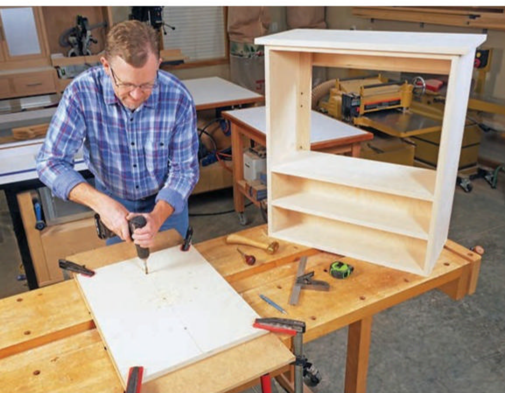
Drill a series of pass-through holes for the charger power cords in the upper back panels with a 3/8" brad-point bit. Clamp the panels together before drilling the holes along their adjacent edges to minimize tearout.
