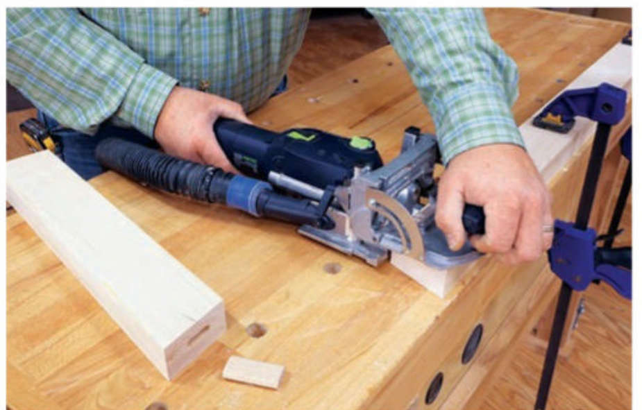
Mill mortises for loose-tenon joints that will attach the front angled ends of the supports to the back edges of the uprights. Festool Dominoes are a sturdy choice, but other options like Rockler's Beadlock tenons could also work.
