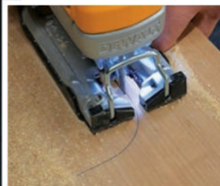
The bottom (Piece 2) has a large foot recess to cut away. Lay out this shape using the Drawing on page 37. Common shop supply containers like cans or glue bottles can provide the curves you need to draw the shape easily. Cut the recess with a jigsaw (inset).
