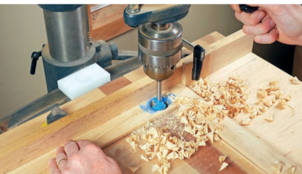
Rockler's JIG IT Hinge Cup Drilling Jig (white in photo) makes it easy to position a drill press fence accurately for drilling hinge cup holes in the door stiles. Bore these holes 12.7 mm deep with a 35 mm Forstner bit.
