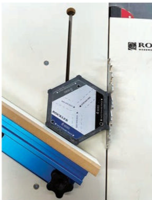
Cutting precise 30-degree angles on the ends of the hexagon segments is crucial for these shapes to fit together. To do it, the author used Rockler's Perfect Miter Setup Blocks (right) to dial in her crosscut sled fence setting.
