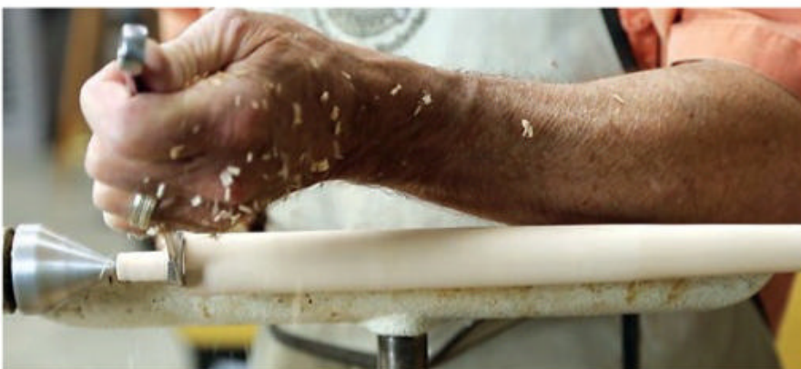
Use a beading and parting tool to cut the tenon, checking its diameter with an open-end wrench. When the wrench's jaws just drop over the tenon, you'll know the tenon is very close to fitting the mortise.
