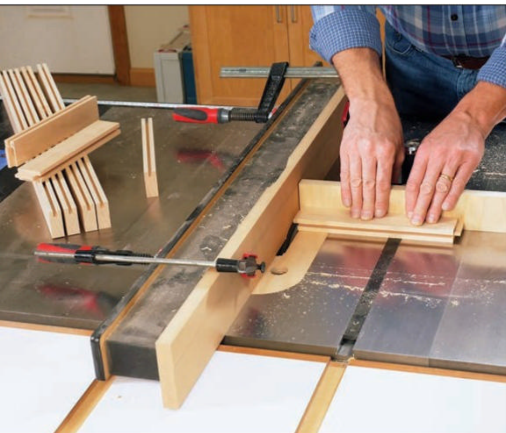
Plow 3/8"-deep, centered grooves along the edges of the door rails and stiles. Make the groove width match the thickness of the acrylic you'll use for the door panels. The author's grooves were just shy of 1/4" wide at 0.22".
