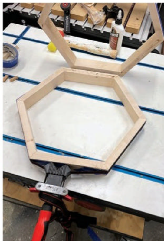
The author constructed a simple three-part ramped jig from scraps (top left, center) in order to position and hold each hexagon segment against her Beadlock jig (bottom) for boring mortises in the part ends. Her jig enabled the beveled ends of each workpiece to sit flush against the Beadlock jig while hand-holding them. Once these mortises were bored, she assembled the parts for both hexagons with 3/4"-long Beadlock tenons. Band clamps pulled the joints together securely while the glue dried (top right).
