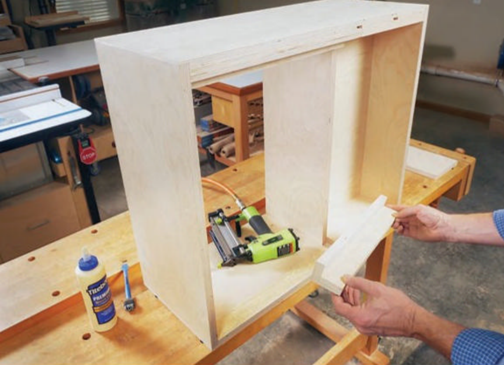
Fasten the upper blocking pieces to the cleats with glue and screws to form a pair of L-shaped subassemblies. Install these inside the cabinet above the lower blocking and so the cleats face forward.
