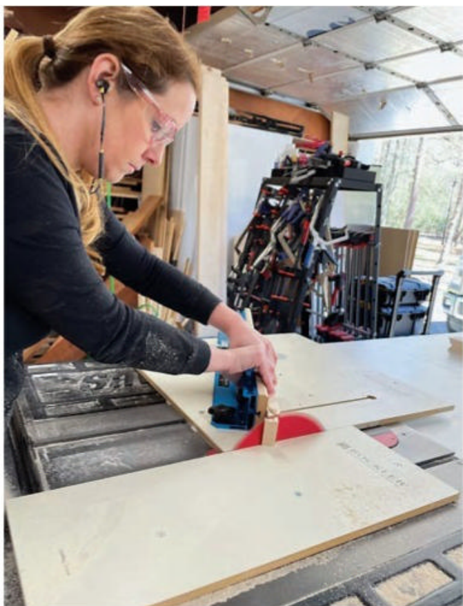
Cutting precise 30-degree angles on the ends of the hexagon segments is crucial for these shapes to fit together. To do it, the author used Rockler's Perfect Miter Setup Blocks (right) to dial in her crosscut sled fence setting.
