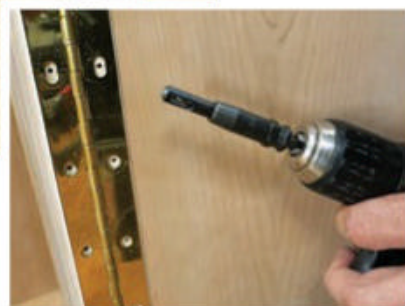
Mounting and aligning doors on piano hinges is a fussy but achievable task. A self-centering drill bit (inset) makes installing the hinges' many screws easier.
