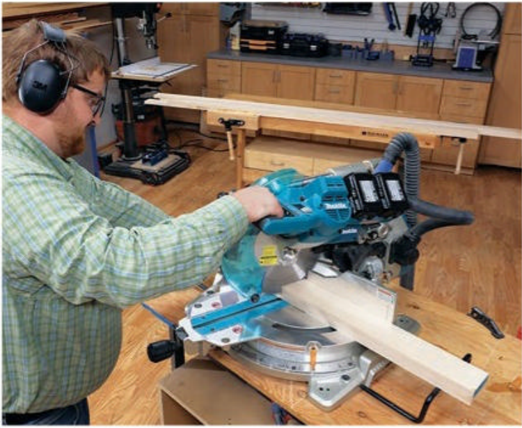
Miter cut the 36"-long blank for the two supports in half with the saw swiveled to 15 degrees. This cut forms the supports' angled front ends. Crosscut the opposite end of each support square to bring these workpieces to their final length.
