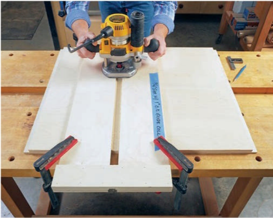
Mill a pair of 1/4"-deep dados across the inside face of the carcass side panel workpiece for the shelves. The author used a shop-made, slotted routing jig, 1" O.D. guide collar and 3/4" straight bit for this operation.
