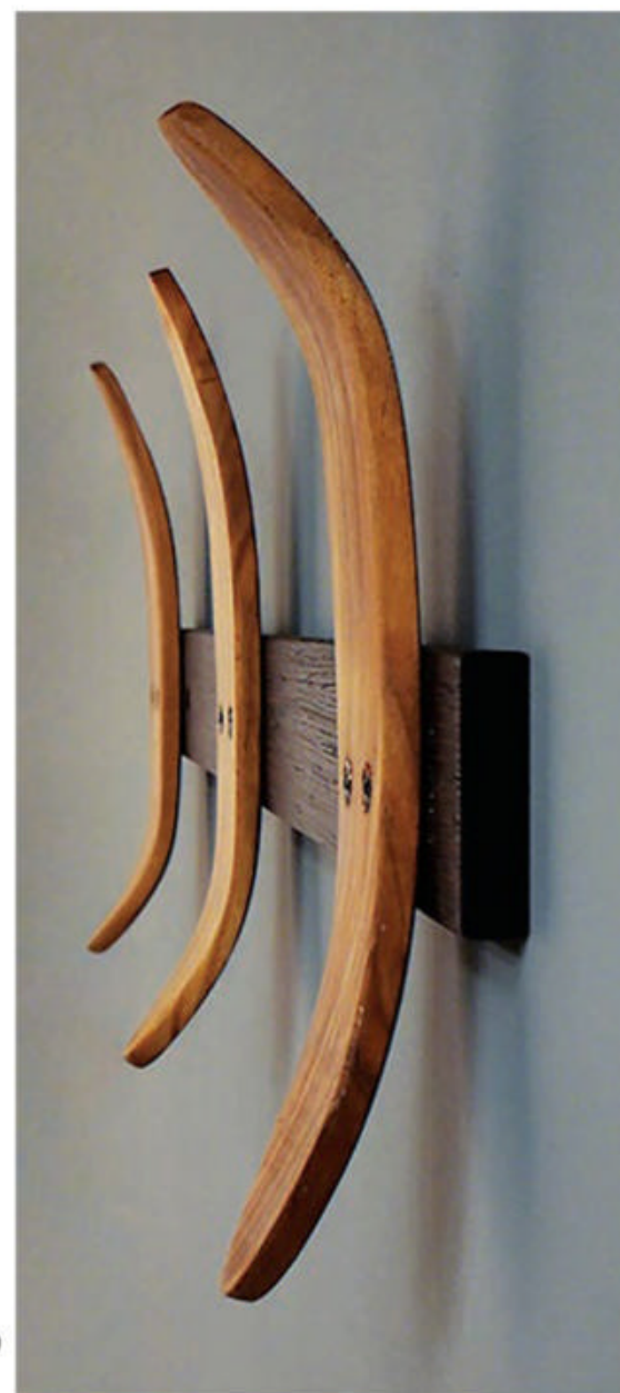
Riving spindle blanks from green wood (above) prevents distortion as the spindles dry. Lumber with 20 to 30 percent moisture content steam bends well for making curved projects such as these coat hooks (below).
