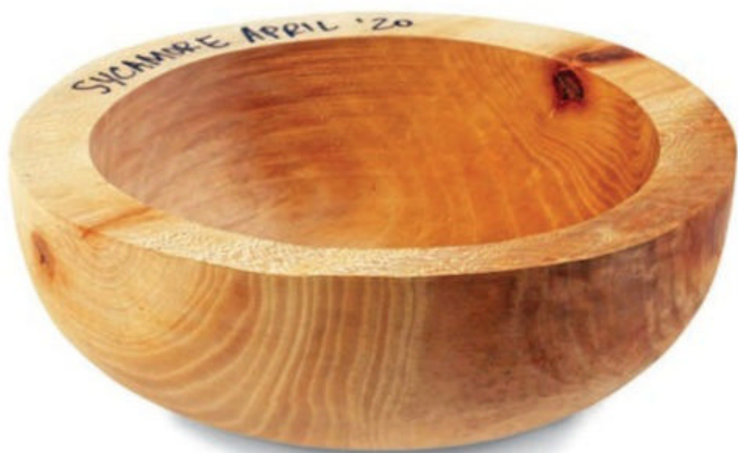
This thick bowl blank was rough-turned from a green sycamore log, packed in a bag with wet shavings and set aside for a year. That enabled it to dry slowly and avoid checking. When it's turned to its final shape, the bowl will remain round (mostly).
