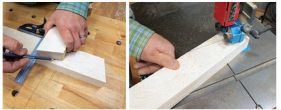
Make a mark at 67\frac{5}{8} " on the inside edge of each upright (top). Then use the 15-degree end of a support and a combination square to lay out the upright's top back angled edge (bottom left). Cut these edges to shape (bottom right).
