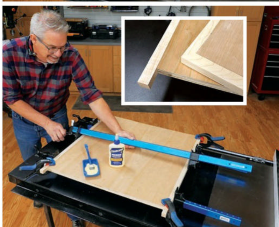
Secure the edging to the plywood panels by gluing and clamping it in place. Miter-cut this trim to detail the top and doors. The back- and side-panel trim is just cut flush to the plywood (inset).
