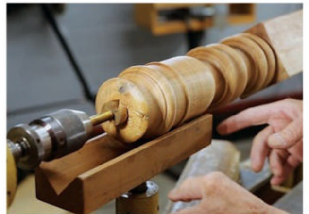
When mortising heavy turnings, the author uses a V-block jig mounted in his lathe's banjo to properly align the turning with the drill bit and support it.
