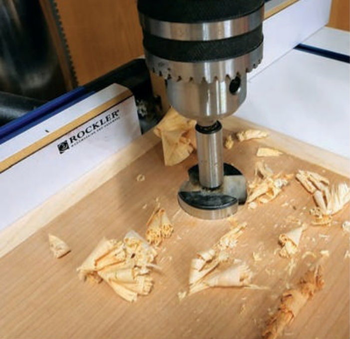
Boring the holes for the inset door pulls is best done on a drill press, so the Forstner bit can drill straight down, evenly into the plywood.
