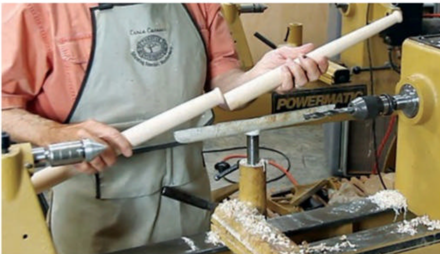
Once the outer profile of a jointed spindle is turned, decide which portion of the spindle will be mortised and which will receive the tenon. Here, the shorter portion will be mortised.
