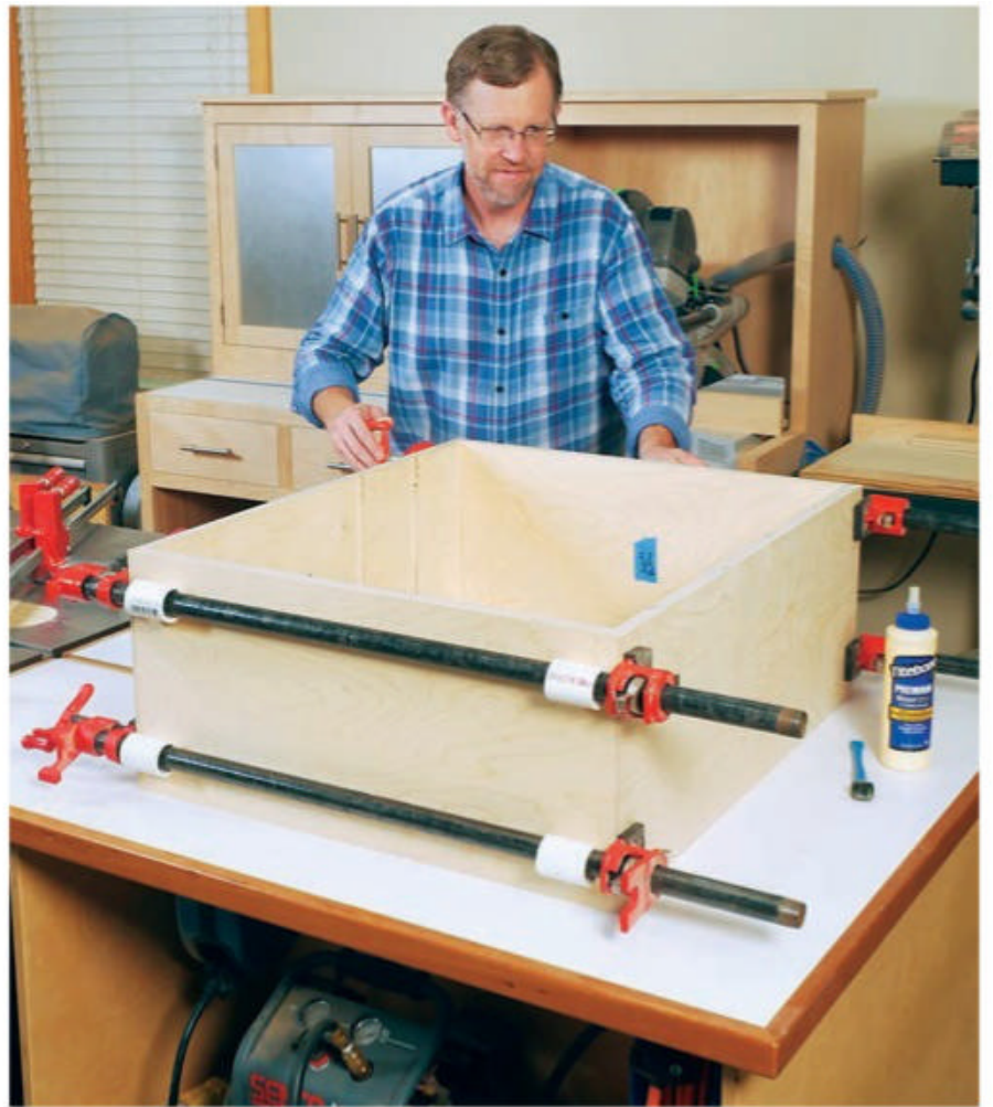
Spread glue along the rabbets of the side panels, fit the top and bottom panels into place and clamp the assembly together. Tighten the clamps enough to close the joints, but be sure the assembly remains square.
