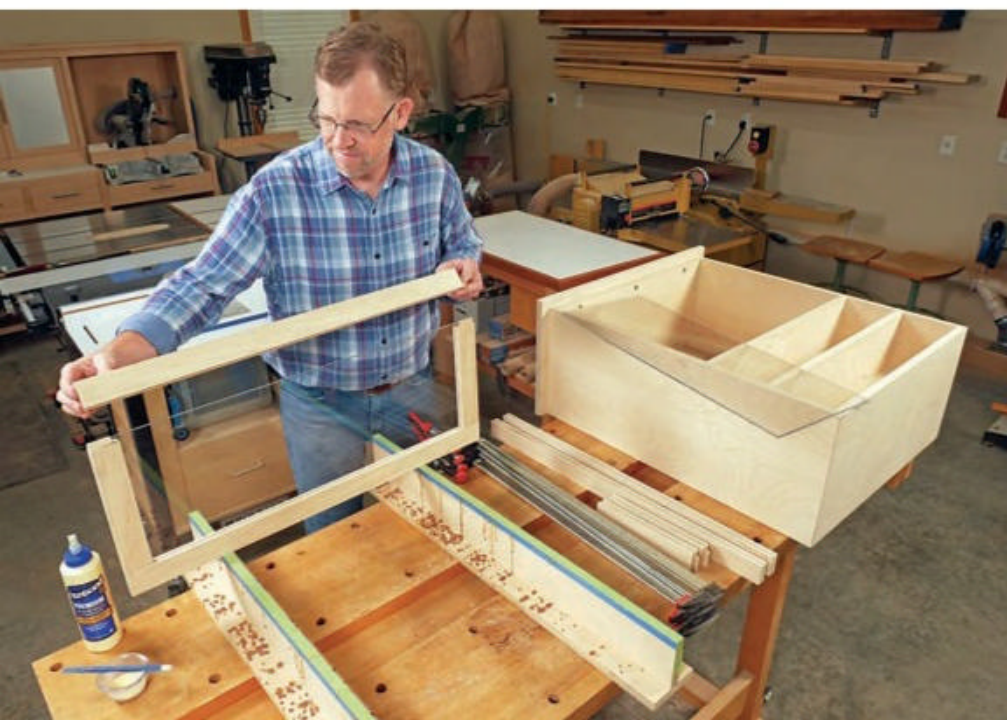
After you've cut clear panels for the doors and checked their fit in a dry assembly of the door frames, spread glue on the rail tenons and assemble each door with its clear panel in place. Clamp the frame joints together.
