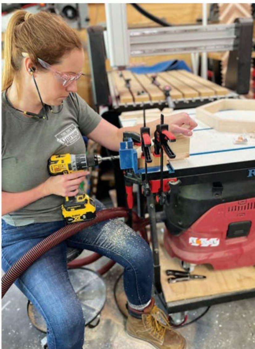
The author constructed a simple three-part ramped jig from scraps (top left, center) in order to position and hold each hexagon segment against her Beadlock jig (bottom) for boring mortises in the part ends. Her jig enabled the beveled ends of each workpiece to sit flush against the Beadlock jig while hand-holding them. Once these mortises were bored, she assembled the parts for both hexagons with 3/4"-long Beadlock tenons. Band clamps pulled the joints together securely while the glue dried (top right).
