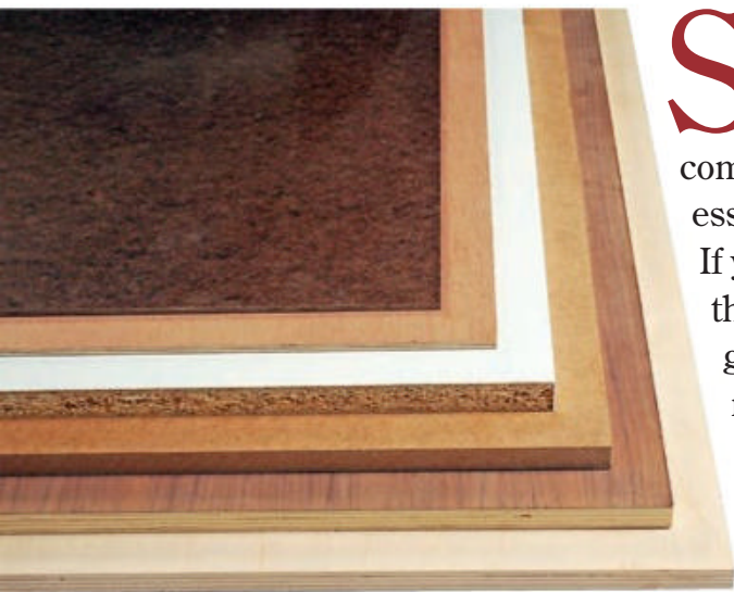
Six worthy sheet goods for woodworking include, from bottom to top: Baltic birch, veneered plywood, MDF, melamine board, lauan plywood and tempered hardboard.
