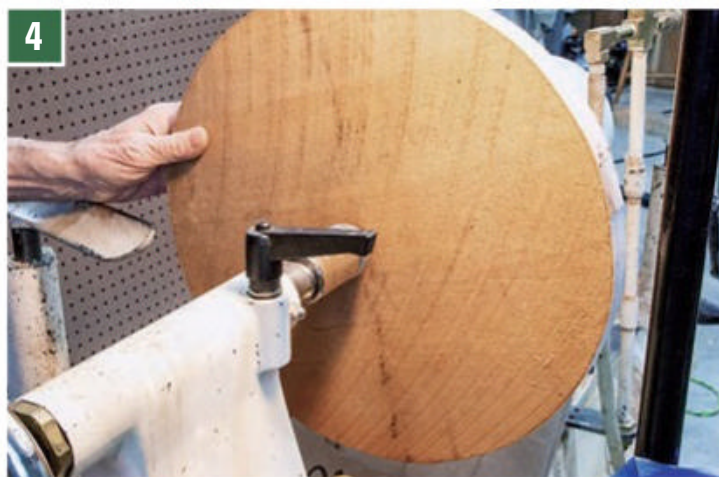
Mount the faceplate and glue block on the lathe, and scrape the block absolutely flat. Then spread wood glue on its face and cover it with a layer of brown craft paper or grocery bag (left). Spread glue on the paper and press the tray blank against it with the tailstock (right), picking up the original center layout mark.
