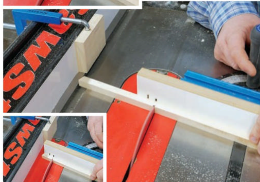
Cut the ends of the panel top and bottom pieces to 12 degrees. Swivel your miter gauge to that angle, and trim one end of the square-edged strips to shape. Then use a step-off block on the rip fence to set the long bottom and short top part lengths.
