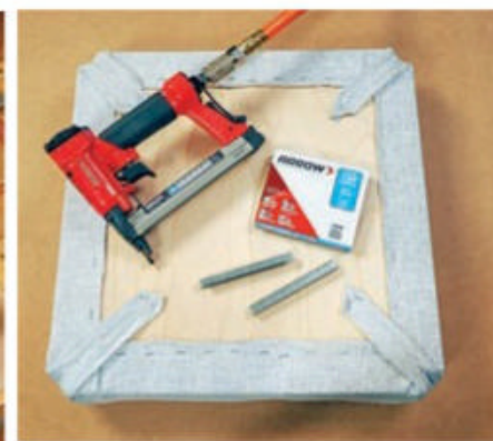
Upholster the chairs with 2"-thick foam and the seat covering of your choice. Arrow's PT50 pneumatic stapler (inset) was up to task for driving 3/8" staples into tough Baltic birch ply without a single misfire.
