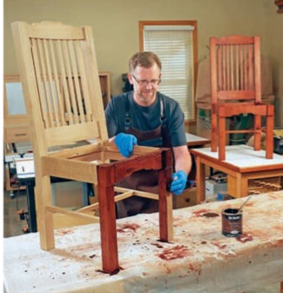
Red mahogany stain enhances the figure of this quartersawn white oak and evens out color differences between the lumber (left). Once stained, the author topcoated his chairs with aerosol shellac to build up a film layer quickly (right), followed by satin lacquer to subdue the initial glossy sheen.
