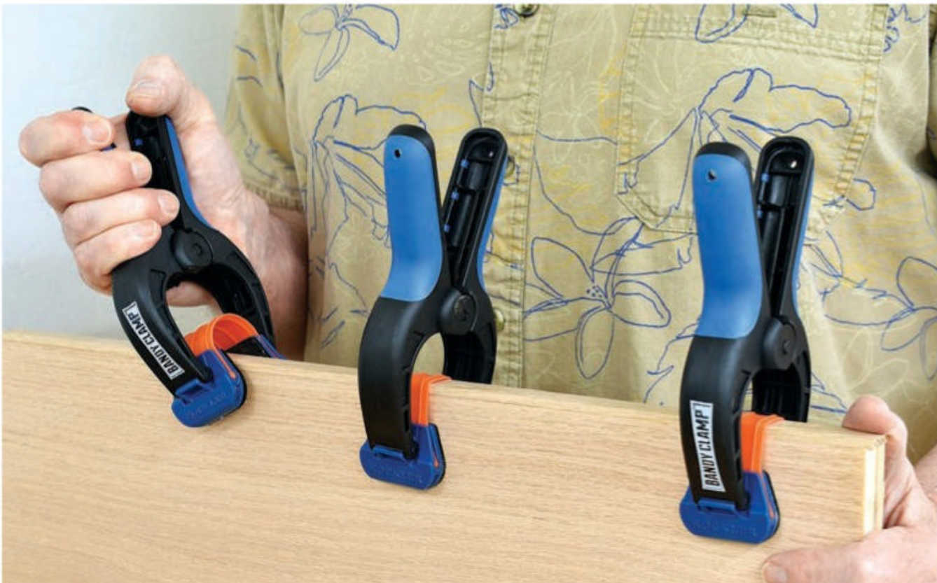
Rockler's Bandy Clamps have a stretchy inner band that applies pressure at a right angle to the clamping force.
