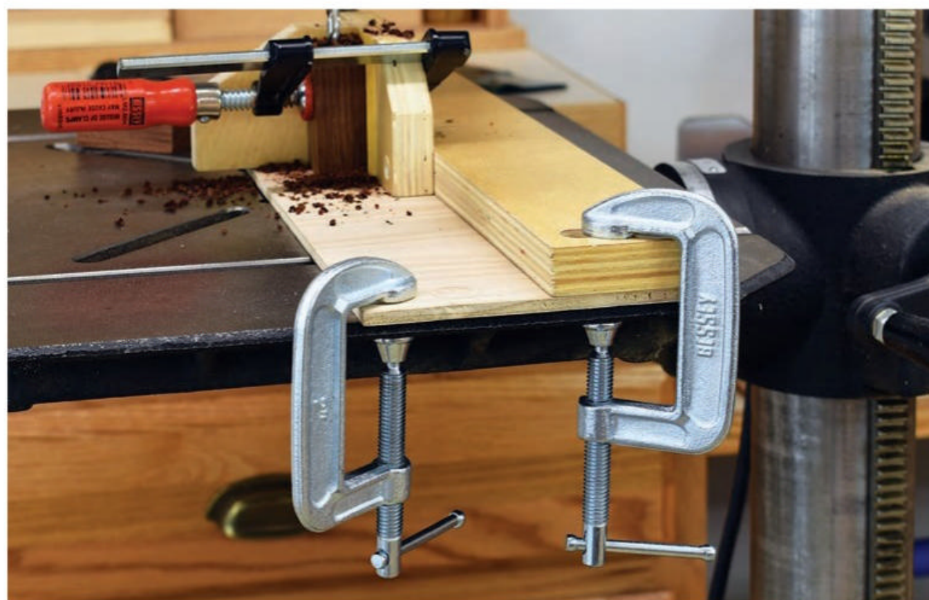
While not ideal for joinery, C-clamps excel as hold-downs for jigs and fixtures. Here, they're securing a jig for pen blanks to a drill press table.
