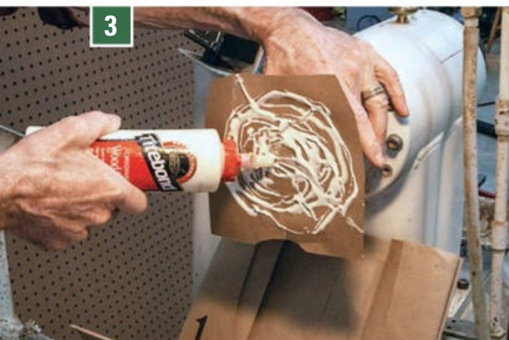
Mount the faceplate and glue block on the lathe, and scrape the block absolutely flat. Then spread wood glue on its face and cover it with a layer of brown craft paper or grocery bag (left). Spread glue on the paper and press the tray blank against it with the tailstock (right), picking up the original center layout mark.
