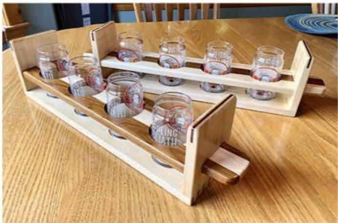
Beer Paddles “My ash and cherry beer paddles are assembled with box joints and through tenons that form handles on their ends.” – Brian Kise
