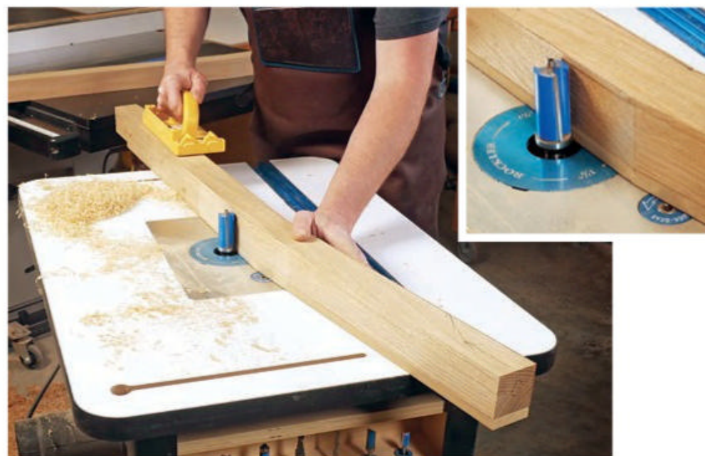
A 2"-long pattern bit (inset), set to full height, will trim most of the leg's edge to final shape with the template attached (here, it's on the bottom). After the first pass, set the bit higher to reach the remaining waste.
