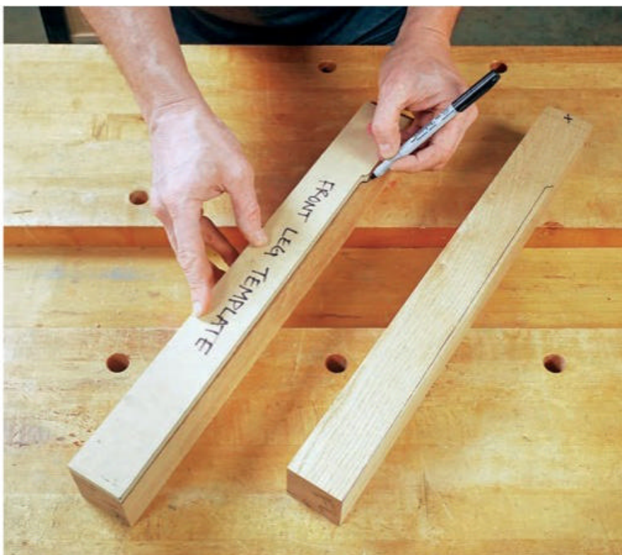
Make and use a rigid template to trace the cloud lift profile onto the front leg blanks. Notice the extra length the author leaves at the top of each leg — it supports the end grain when drilling the seat rail mortises.
