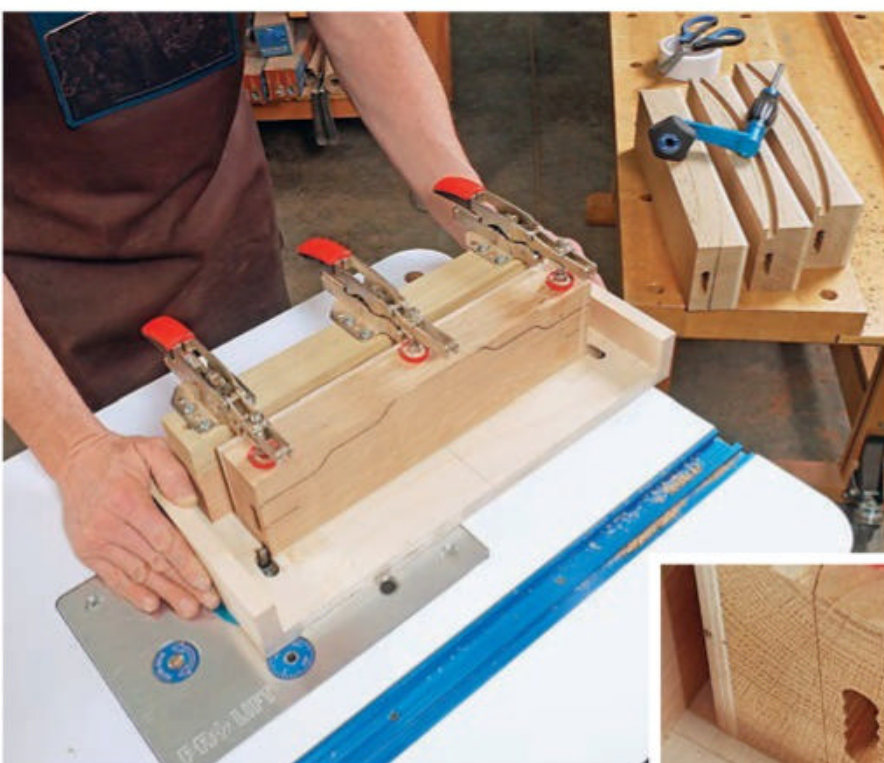
Mill the 1/2"-deep curved grooves in the crest and back rails with a 3/8"-dia. bit (inset). With each routing pass, move the jig side-to-side so the guide bushing can follow the curved opening in the jig's base.
