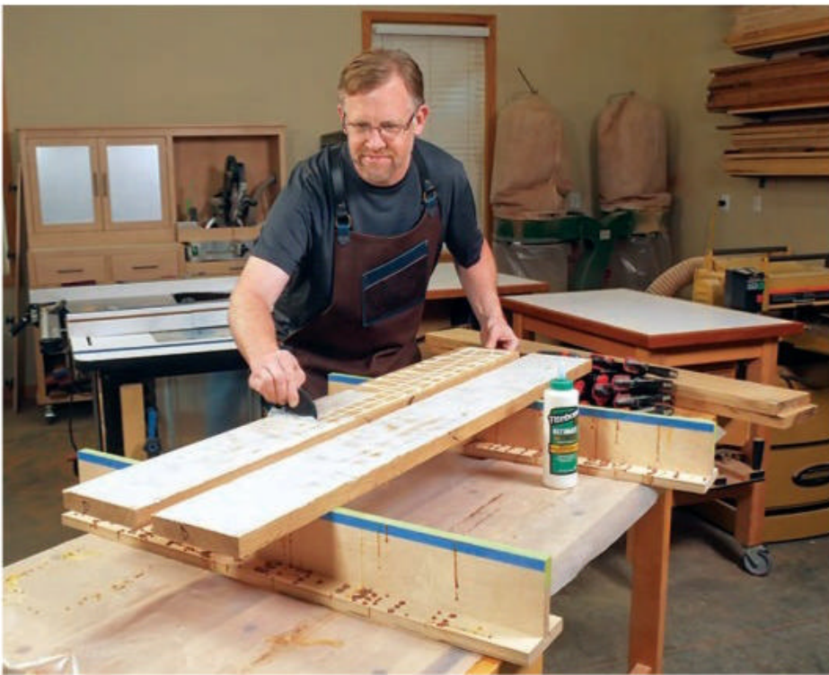
Glue up a pair of blanks measuring 6" x 46" for each chair you plan to build. These laminated blanks will yield both a back and a front leg. The author started with 5/4 stock here, planed to 1" thick, to create their 2" thickness.
