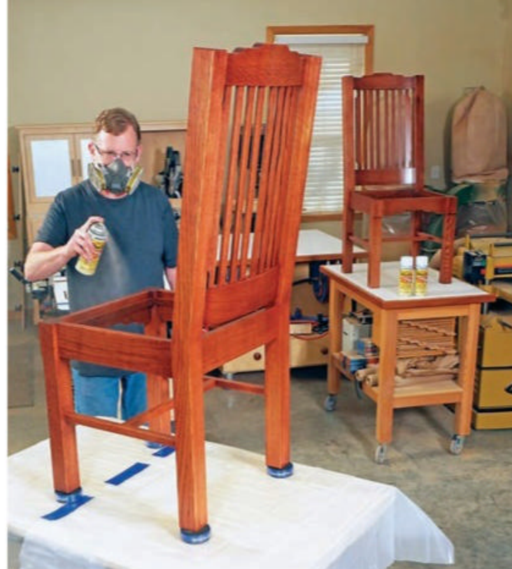
Red mahogany stain enhances the figure of this quartersawn white oak and evens out color differences between the lumber (left). Once stained, the author topcoated his chairs with aerosol shellac to build up a film layer quickly (right), followed by satin lacquer to subdue the initial glossy sheen.
