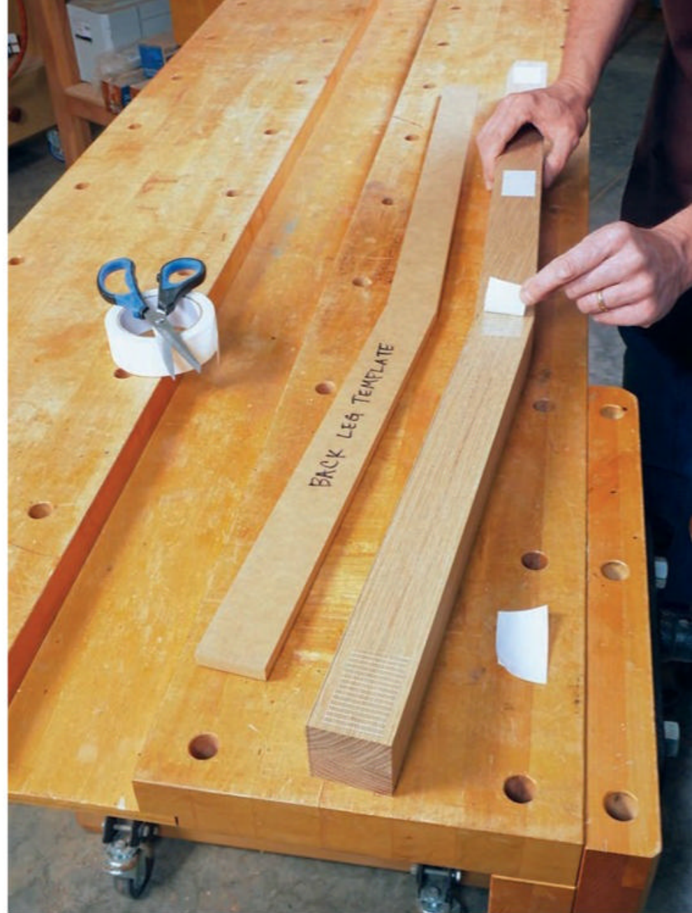
Rough cut the back legs to size, and create a rigid template from MDF or sheet stock. Secure the template to each back leg for template routing using several short strips of double-sided tape.
