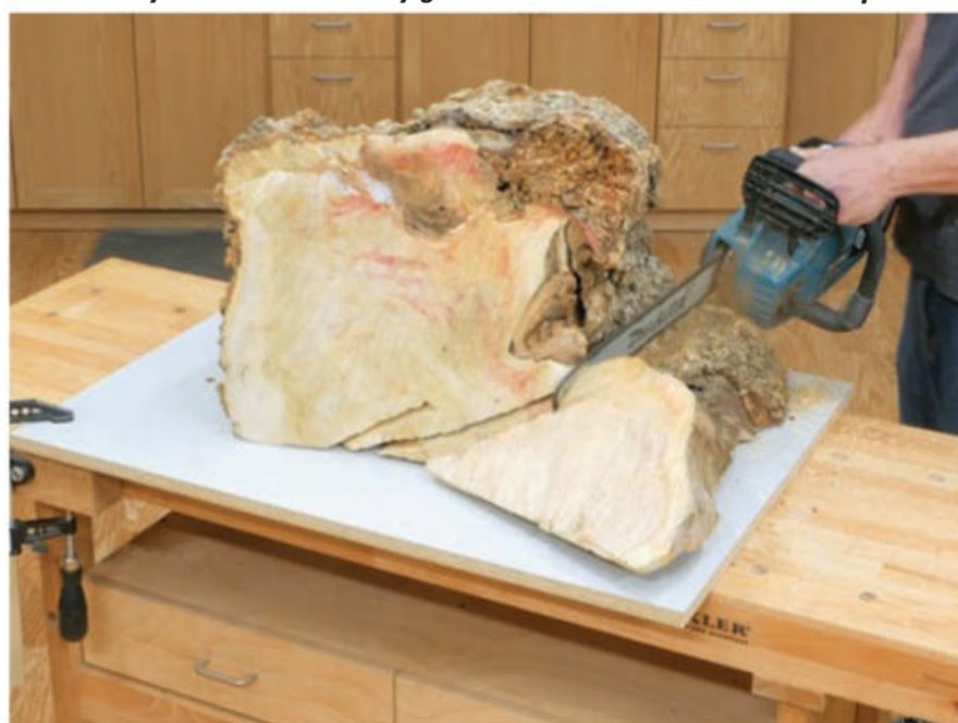
Trimming with a chainsaw started the process of harvesting the parts. Careful planning ahead made it possible to yield several turnable pieces.
