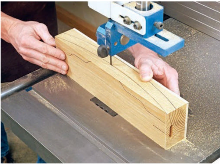
Cut the broad curves of the crest and back rails in one pass so you can save and reattach these offcuts for the routing and sanding steps. Notice the plywood backer piece here, which will keep back offcut in one piece.
