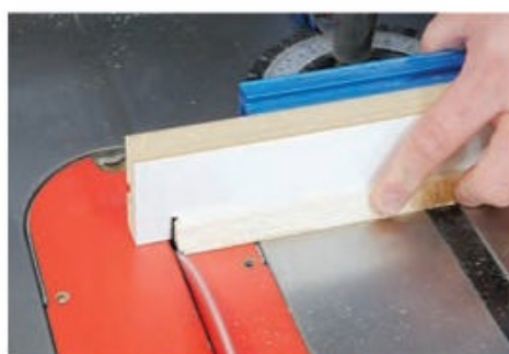
Crosscut the six bevel-edged strips into 12 side pieces for the shade panels. With a miter gauge set square to the blade, trim them each 11" long, making sure to square their ends (inset). The author used a flip stop on his miter gauge to set these part lengths.
