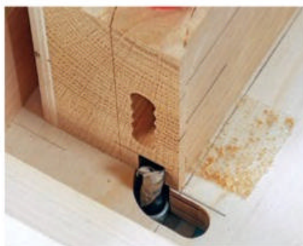
Mill the 1/2"-deep curved grooves in the crest and back rails with a 3/8"-dia. bit (inset). With each routing pass, move the jig side-to-side so the guide bushing can follow the curved opening in the jig's base.
