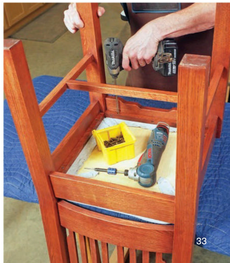
Finish up this ambitious dining chair project by attaching the upholstered seat to its cleats with several countersunk 1 1/2" wood screws per cleat.
