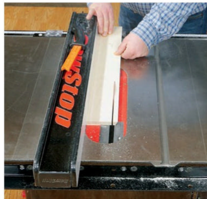
Reset the blade to 90 degrees, and adjust the rip fence so the beveled offcut will be \frac{1}{2} " wide. Rip this strip free to form two panel sides. Repeat for the other edge.
