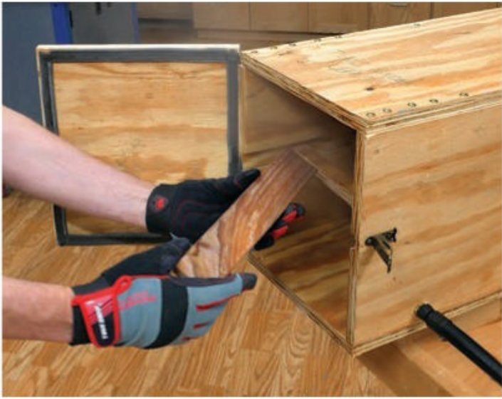
Take care when removing stock from the steam chamber — it is very hot. Note the slat inside the chamber to hold the stock in the middle of the steam.
