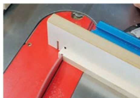
Cut the ends of the panel top and bottom pieces to 12 degrees. Swivel your miter gauge to that angle, and trim one end of the square-edged strips to shape. Then use a step-off block on the rip fence to set the long bottom and short top part lengths.
