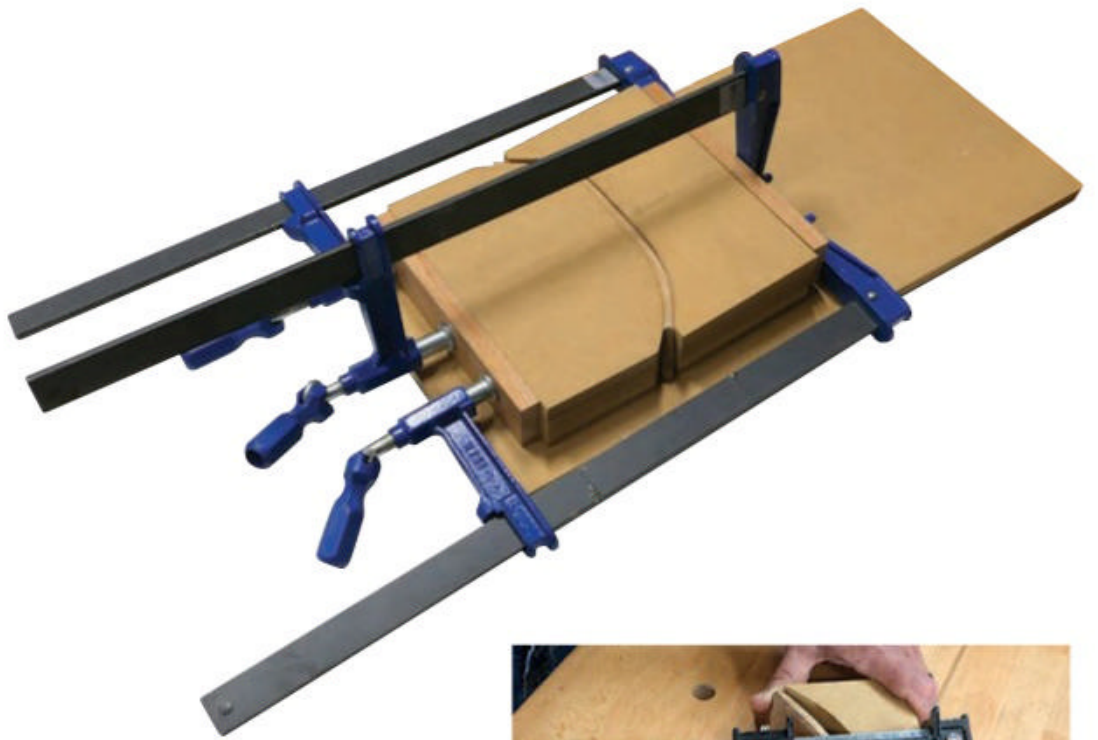
Once bent, leave the coat hook in the forms for one hour (above). Then transfer it to a cooling form (right). It should remain in the cooling form at least overnight.
