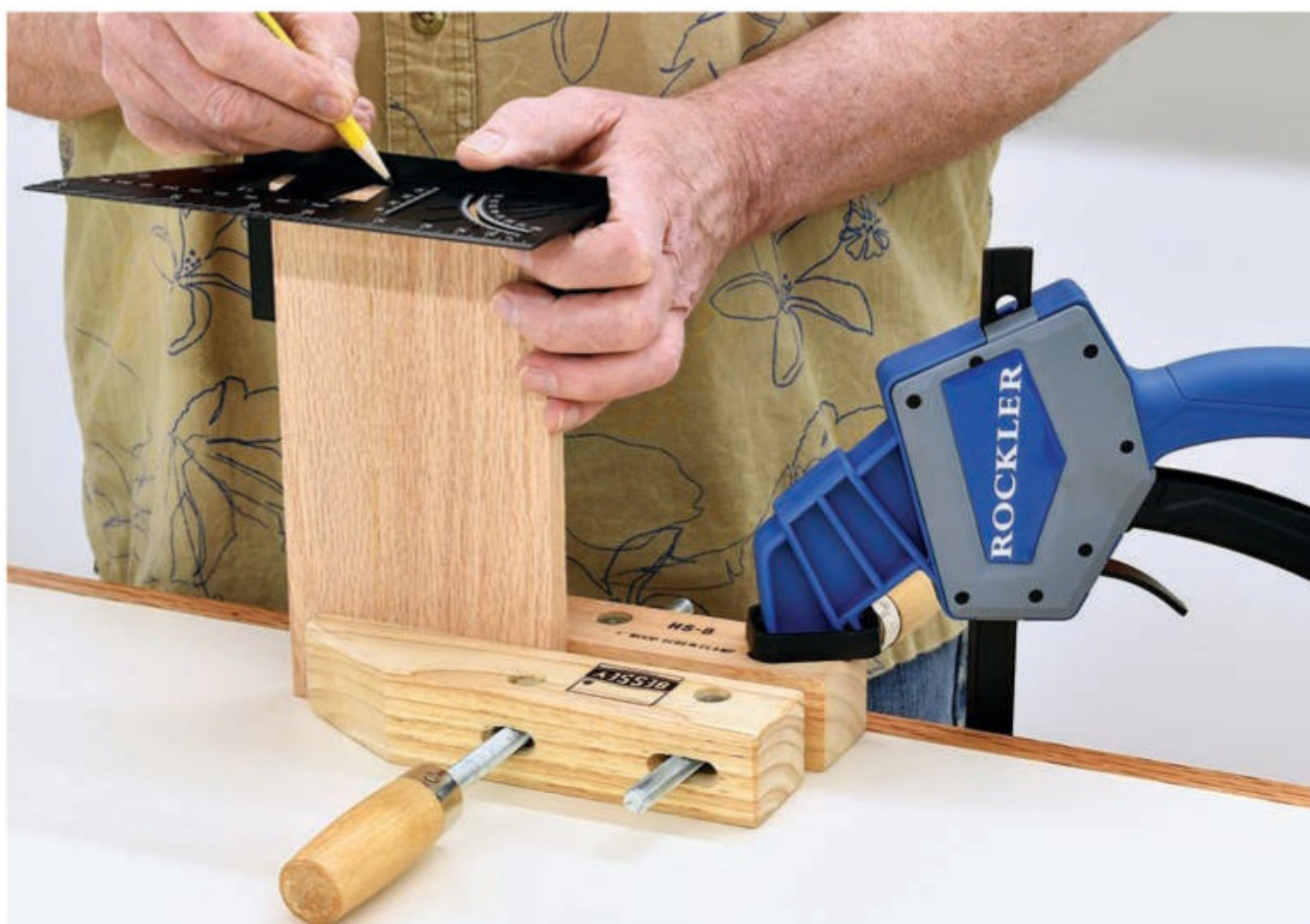
A wooden hand screw (flat on table) not only clamps things together but also can function as a use-anywhere vise. Here it's being held in place by a Rockler quick-action clamp that tightens by pumping a single handle.
