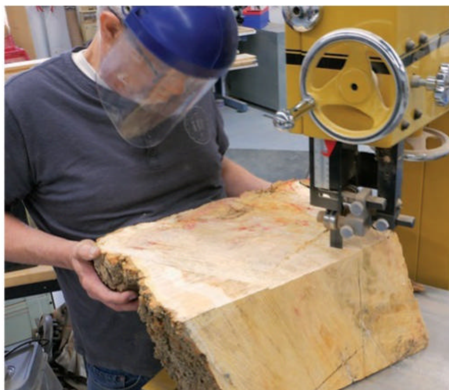
Next stop was a large band saw to further break down the box elder into mountable and turnable blanks.
