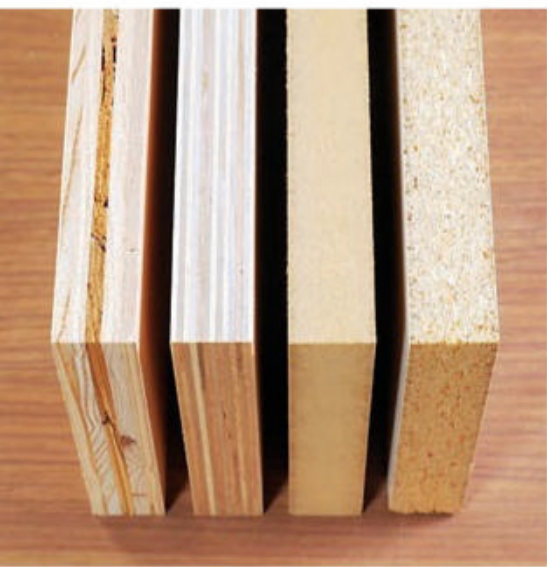
Core compositions of sheet goods will vary. From left to right, they might consist of thin solid lumber laminations, even thinner veneer layers, wood pulp or coarser wood particles.
