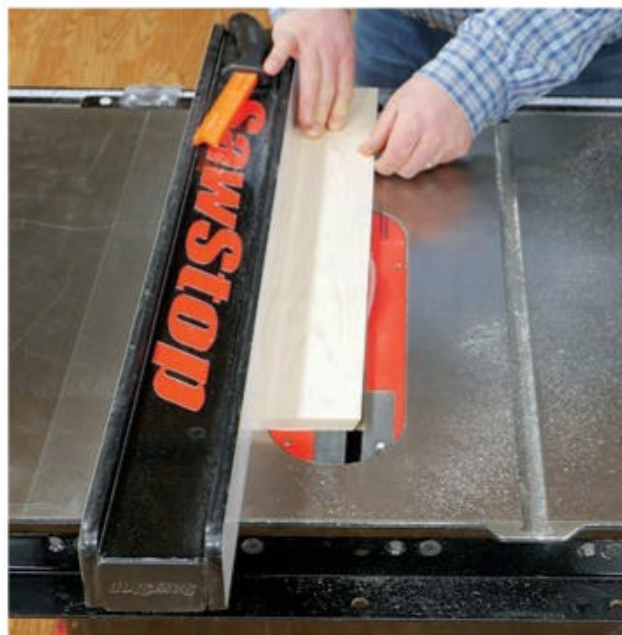
Make sides for the shade's six panels by first bevel-ripping both edges of the maple workpiece to 29 degrees.
