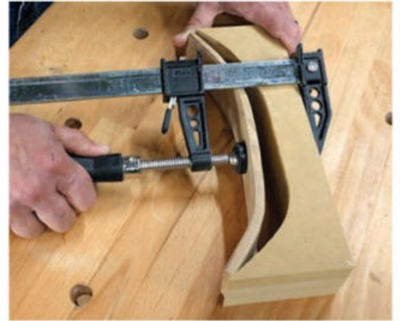
Once bent, leave the coat hook in the forms for one hour (above). Then transfer it to a cooling form (right). It should remain in the cooling form at least overnight.
