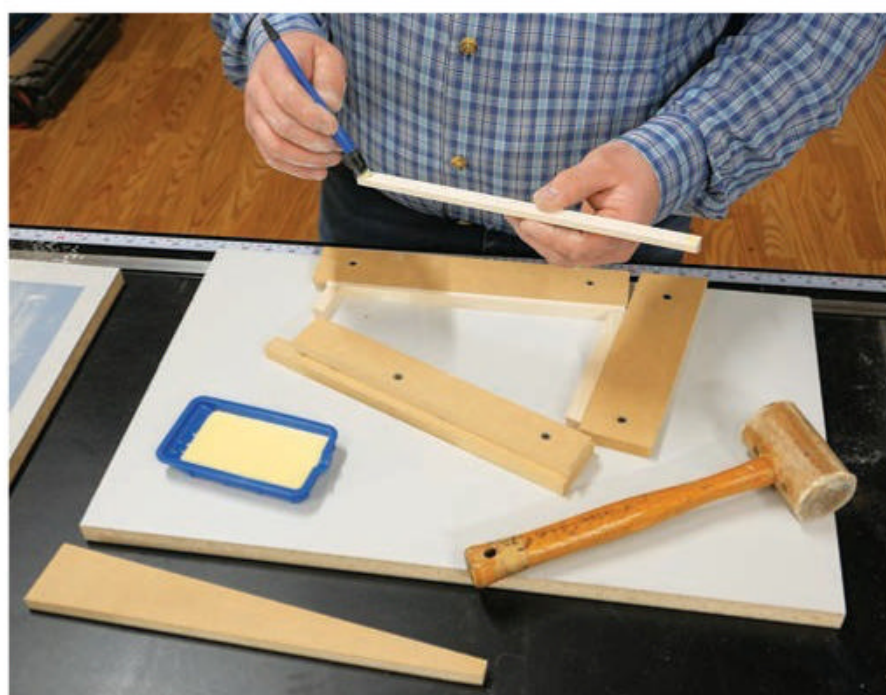
Spread glue on the part ends, and insert the panel workpieces into the jig. The bevels on the panel sides should engage the jig's inner beveled edges.
