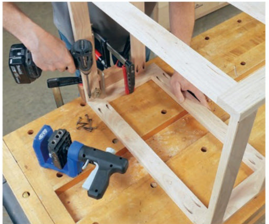
After you've assembled the longer rails and legs into two frames, connect these frames with the shorter rails to complete the base. The bottom short rails are located 2" up from the bottom ends of the legs.
