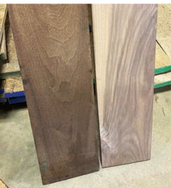
Dark outer surfaces on the walnut sample (above left), might be hiding lighter sapwood areas underneath. “Skip planing” (left), will reveal at least some of the actual figure and color you can expect. This maple board attests to it here.
