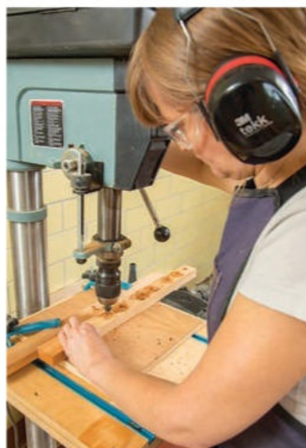
Drill countersunk pilot holes through the cross braces at the screw locations you’ve marked (left photo). Attach these braces to the aprons with pocket screws, then drive in the screws that attach the braces to the slats.
