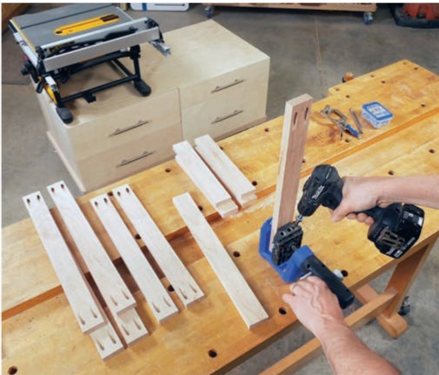
Pocket-hole joints are a simple means of assembling frameworks like this router table base. Use a commonly available pocket-hole jig to bore a pair of holes on the inside faces of all the long and short rails.
