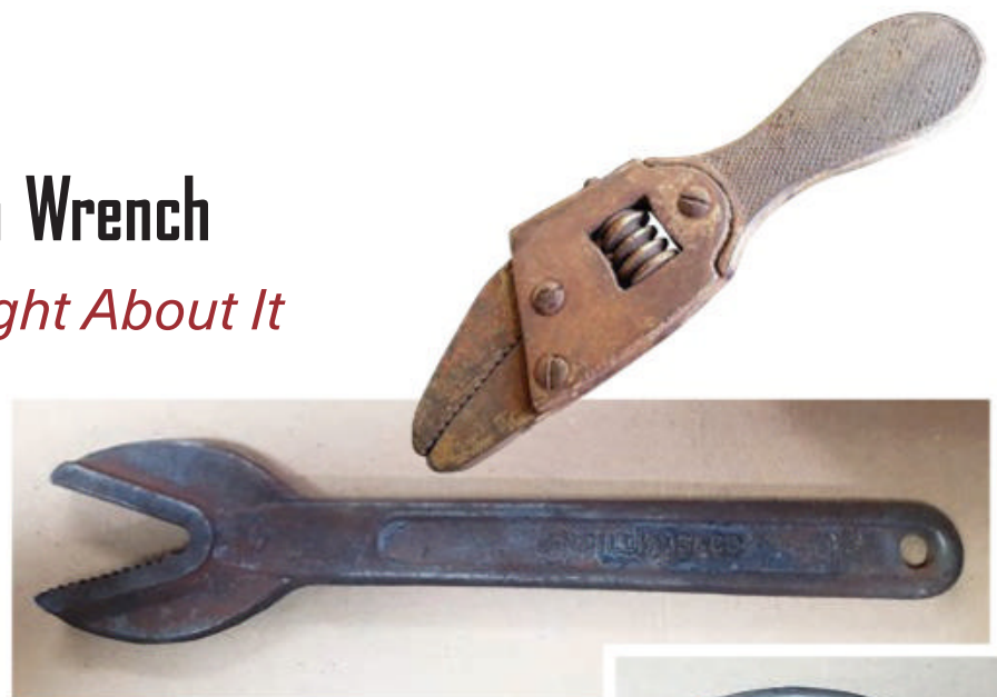
Denny Mandeville's fixed-jaw "fitzall" wrench (above) was handy in the days before standardized fastener sizing. The smooth jaw registered against a nut's flat, and the toothed jaw engaged its corners (inset). Pat Graser's wrench (top photo) is an adjustable version of the same basic style.
