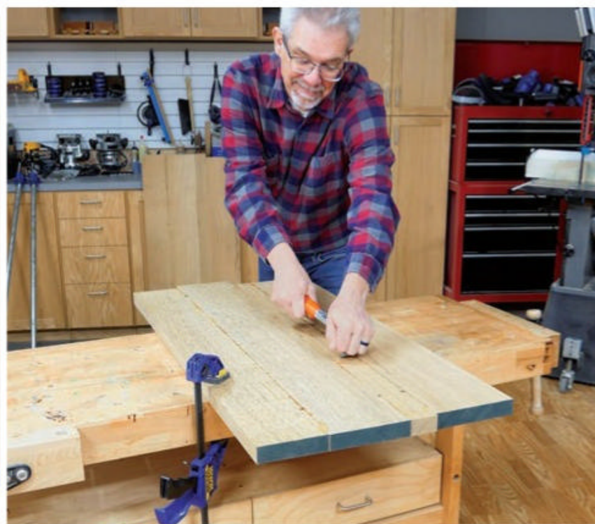
Taking time to select the nicest-looking stock for the tabletop was an early step in the process. The author placed the most highly figured wood in the center of the panel and the less showy stock on either side of those planks. To make the assembly process more manageable, he glued up the top in two sections, then flattened and sanded them smooth.
