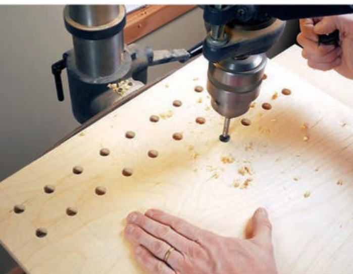
The author dedicated the shallow drawer to router bit storage. It's large enough to stow 90 router bits with shank holes spaced 2" apart.
