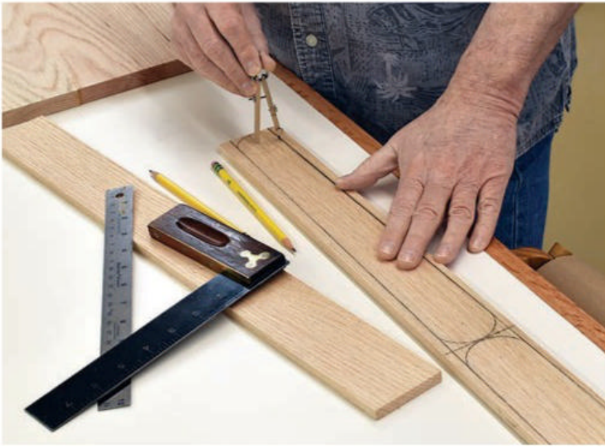
Follow the Drawings to lay out the arm components for cutting. There is a continuous taper that runs through both upper and lower arm sections.
