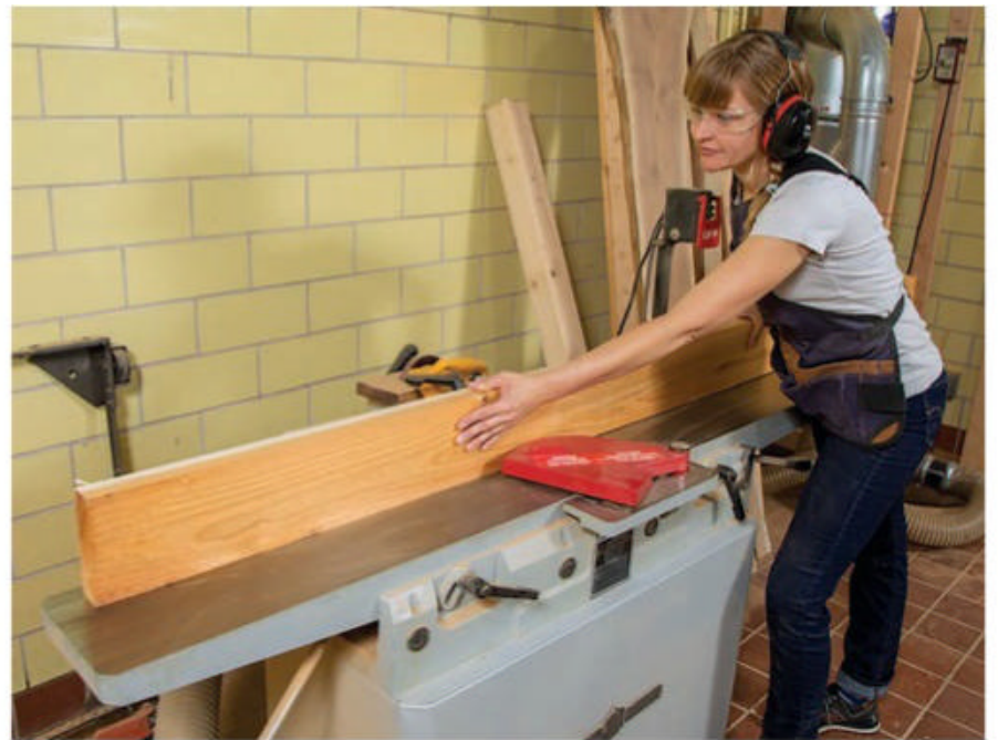
After the author planed her stock to 1½" thick, she flattened one reference edge on the jointer. This will allow you to rip the bench's workpieces to width, yielding parts with straight, parallel edges.
