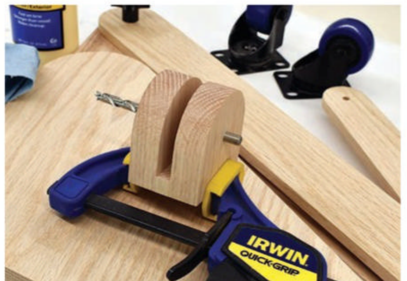
Glue the 3/8" spacer to set the opening for the mounting swivel, and clamp up till dry. A 1/4" drill bit aligns the two pieces.
