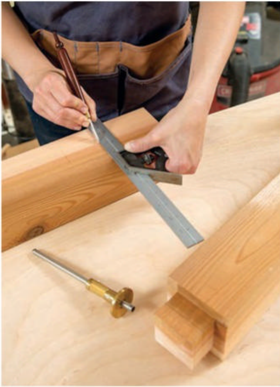
A combination square makes quick work of laying out the top and bottom layout lines for the leg mortises. The author used a marking gauge to scribe the mortises' side layout lines instead.
