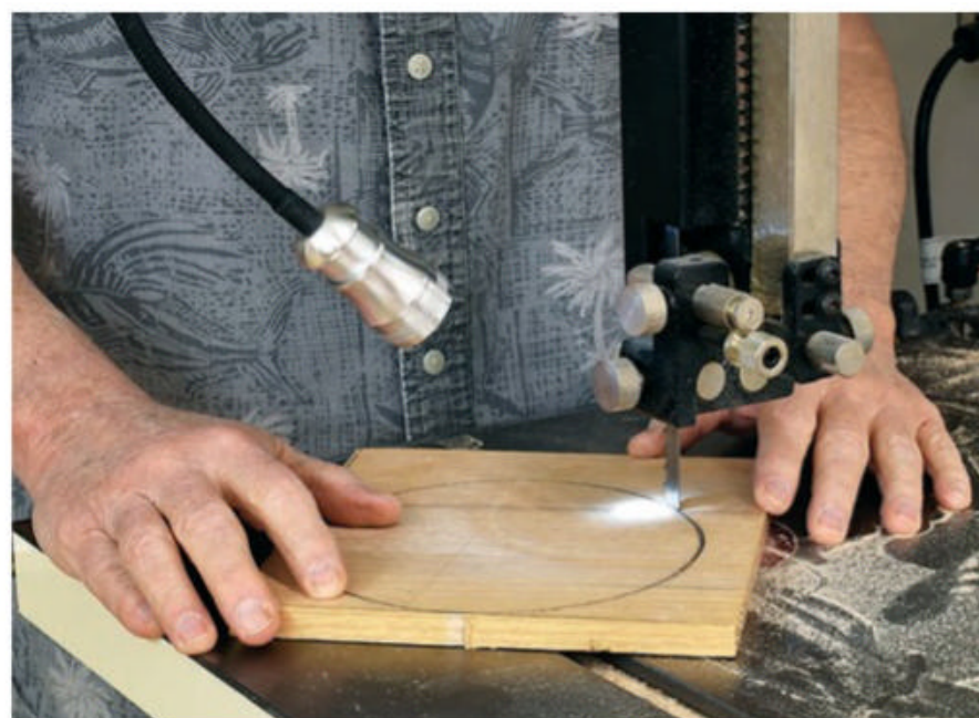
A dedicated adjustable light mounted to this band saw makes following a cut line simpler, and the blade is easier to keep an eye on.
