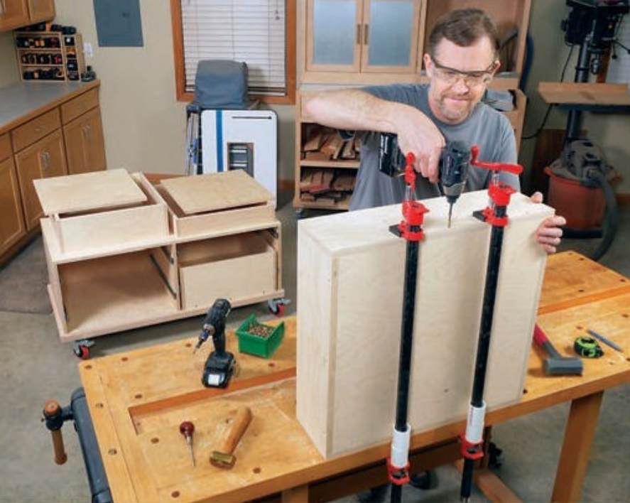
These drawers are easy to assemble with butt joints and counterbored screws, and they'll be plenty strong. All the drawer components are 3/4" plywood, including the bottom panels.
