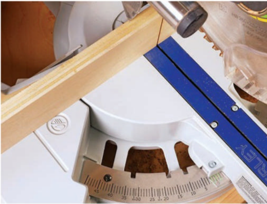
The long line and “no hands” symbol embossed into the table near the rim of this miter saw’s protractor scale marks the “danger zone.” Anything inside this area is too short to be held in place by hand for cutting.
