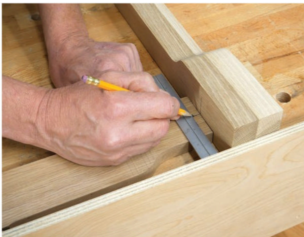
Position the aprons on the legs so the top edge of the center cloud lift is aligned to the top ends of the legs. The author checked his measurements using a straight-edge on a workbench.
