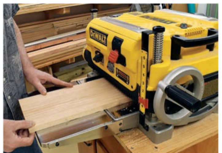
Plane solid stock to 3/8" for the articulated arm, inner base and light mount plate components.
