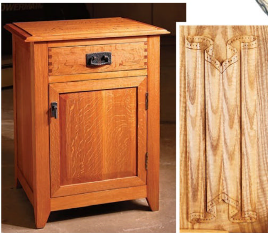
Beautiful quartersawn white oak displayed in the frame-and-panel cabinet (left) versus an expertly carved flatsawn white oak panel (right).
