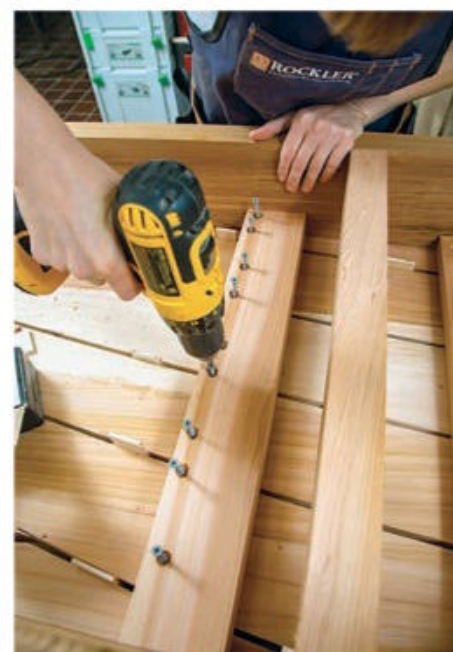
Drill countersunk pilot holes through the cross braces at the screw locations you’ve marked (left photo). Attach these braces to the aprons with pocket screws, then drive in the screws that attach the braces to the slats.
