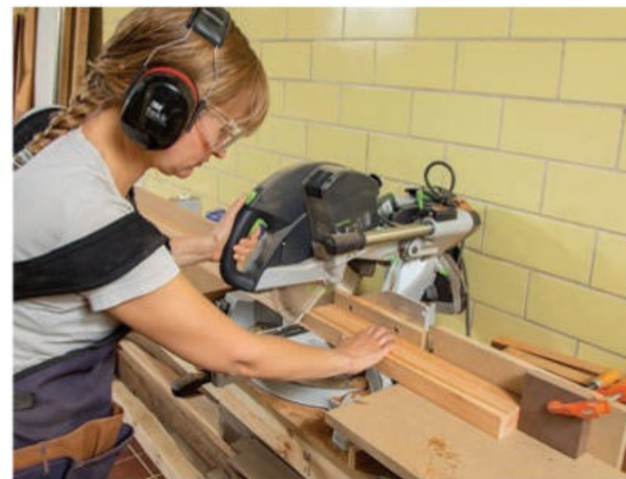
Here the author uses a stop block, clamped to her miter saw station’s fence, to set the length for cutting multiple same-sized parts. It’s an efficient and accurate sawing strategy.
