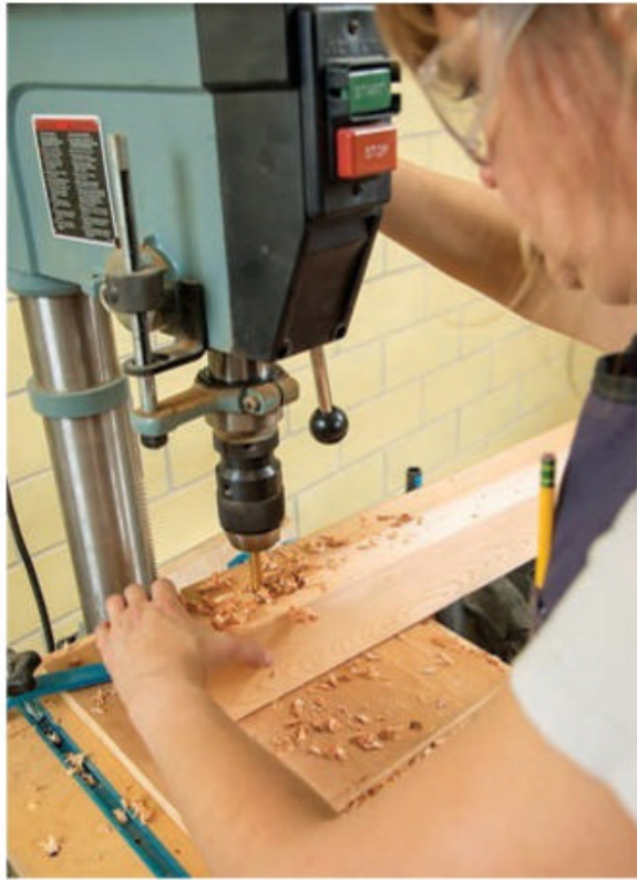
You can hog out most of the waste inside the leg mortises at the drill press with a large Forstner bit. A series of overlapping plunge cuts will take care of most of this stock removal.
