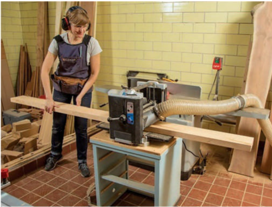
Roughsawn cedar timber like this will require some initial surfacing to smooth its faces and reduce its thickness to 1½" for many of the parts. Flatten one face on a jointer before planing the other face parallel to it.
