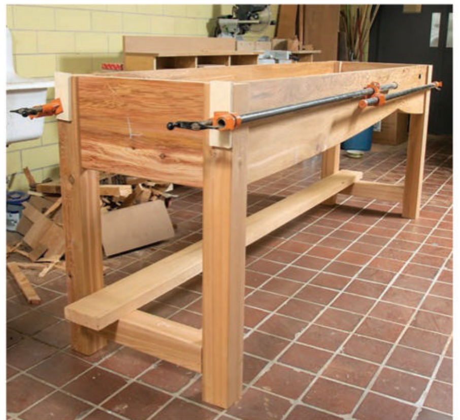
Pairs of interlocked pipe clamps helped the author hold the front and back aprons in place before she drove 2 1 / 2 "-long pocket screws through them to secure the joints. Scrap blocks prevented marring by the clamp heads.
