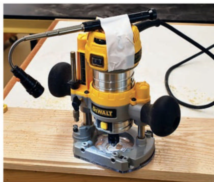
Taping a small utility light to a router is a quick fix that works wonders for lighting up the bit area.
