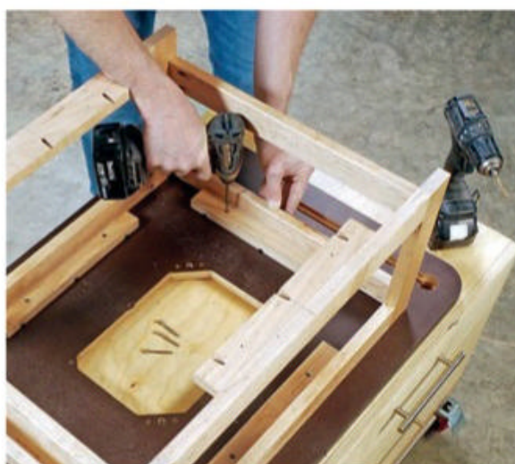
Attach the router table base to the tabletop by driving pairs of countersunk 1½" screws through the top cleats and into the bottom face of the tabletop.
