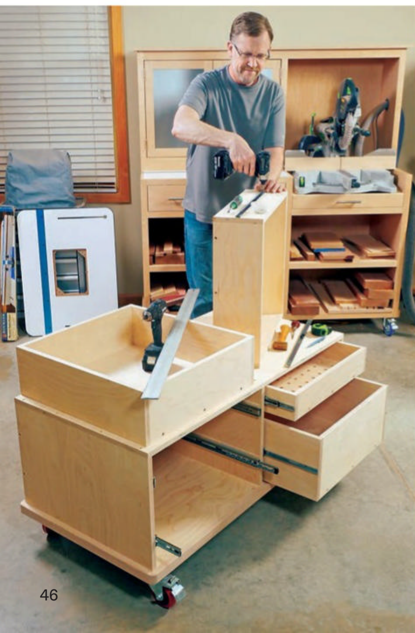
The author dedicated the shallow drawer to router bit storage. It's large enough to stow 90 router bits with shank holes spaced 2" apart.
