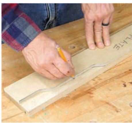
Transfer the shape of the aprons from the template to the workpieces. Then cut the aprons out on the band saw, staying just outside the lines.
