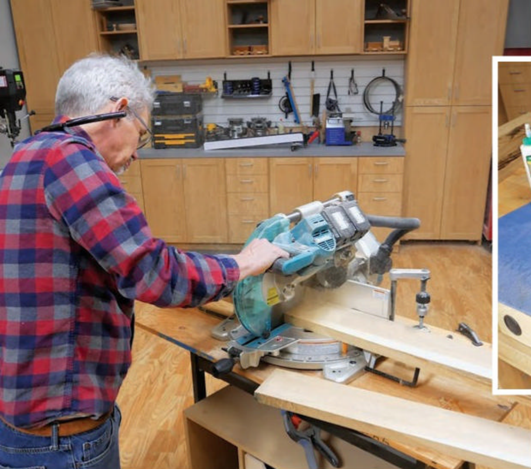
Crosscutting and ripping stock for the legs was the author's first step. He cut enough to glue up five leg blanks. At this time he also selected the stock for the tabletop and cut those pieces to length.
