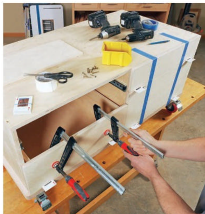
Stacks of playing cards make handy spacers when positioning the drawer faces on the drawer fronts. Double-sided tape holds the faces in position for clamping.
