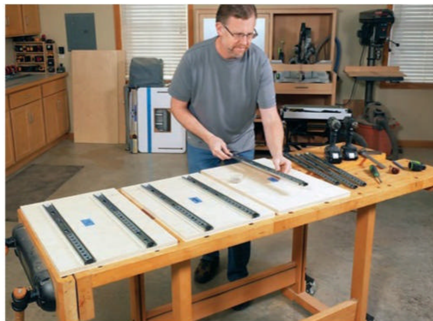
Install the "cabinet" side components of the drawer slide hardware on the carcass side and divider panels before continuing the construction process, while these workpieces are still loose and can be laid flat.
