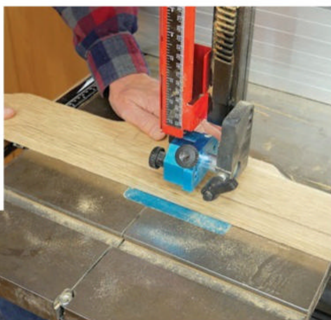
All of the quartersawn white oak was purchased as 1 1/4" thick, surfaced two sides and in random width and length. To make the aprons, the stock was resawn to 3/4" thick at the band saw against a point-style fence.
