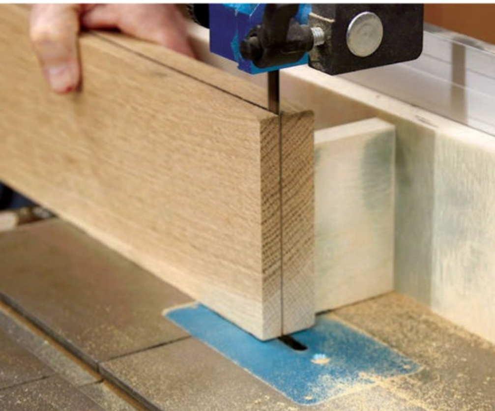
All of the quartersawn white oak was purchased as 1 1/4" thick, surfaced two sides and in random width and length. To make the aprons, the stock was resawn to 3/4" thick at the band saw against a point-style fence.
