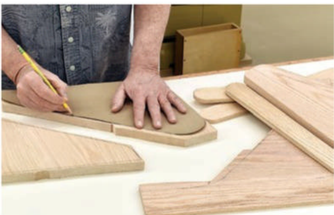
The three base components — two 3/4" thick and one 3/8" — get identical profiles from a single pattern. However, the thinner middle component has an extended "neck" for attaching the articulated arm.
