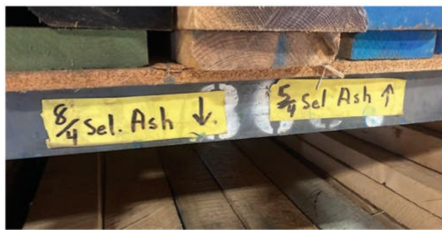
Roughsawn lumber is shelved and sold by its quartered thickness. Here, 8/4 ash (about 2" thick) will have a finished thickness of about 1 3/4", and 5/4 ash (about 1 1/4" thick) will plane down to about 1" smooth.
