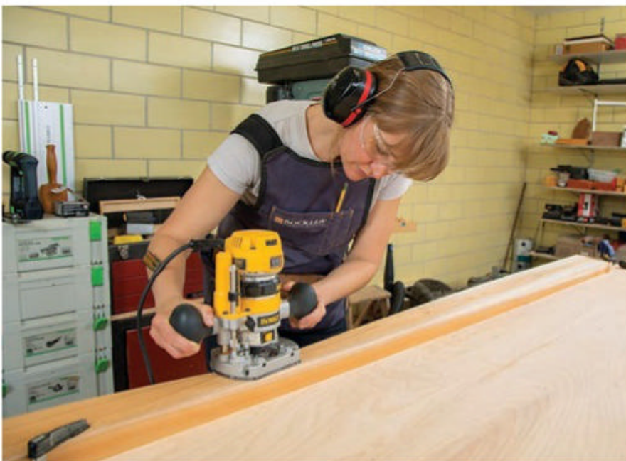
Cedar is prone to splintering along its edges. To safeguard against injury and make the potting bench more enjoyable to use, break any sharp part edges with a router and 1/8" roundover bit, a file or a sanding block.
