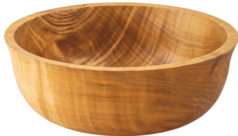
Small salad bowl turned from curly maple by the author. It is 7¾" dia. by 2¾" deep with a 1/2" wall thickness and a slight Revere flair at the rim.
