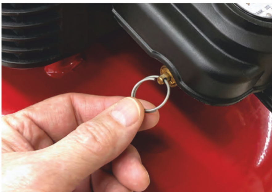
Although designed as a safety feature, an air release valve also serves as a means to quickly empty the tank.
