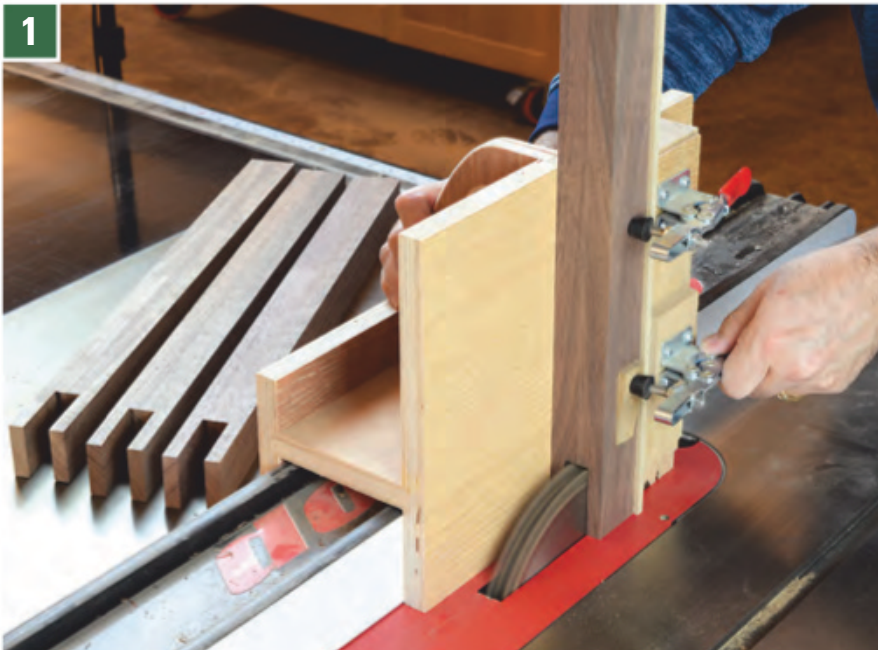
Using a tenoning jig and dado blade, form a 2"-deep x 3/4"-wide notch in the top of each leg. Cut from both sides of the leg to center these bridle joint notches.
