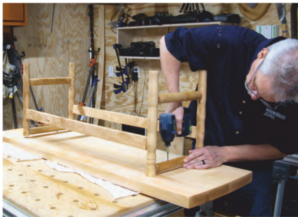
The undercarriage attaches to the seat with 2½" screws. On each upper stretcher, one of the through holes that accommodates the screws is elongated to allow the seat to expand and contract across its width seasonally.
