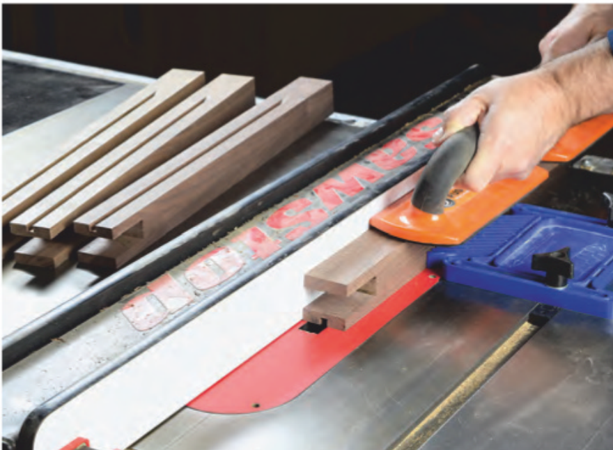
Reset the rip fence for a centered cut on the legs, and make one stopped groove in each leg. A featherboard and push pads help control the cut.
