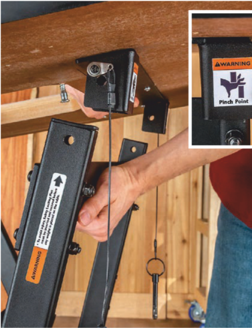
The stand's front table bracket with angled sockets attaches beneath the tabletop. It captures the top front legs that hold the table upright.
