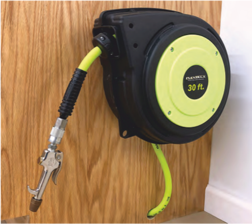
With a centrally located compressor and a versatile retractable hose reel, you can use an air tool almost anywhere in the shop. Typical reel lengths run from 15 to 100 ft.
