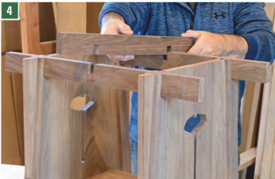
Since the rail joinery is angled, the parts won't drop right together. You may need to use a clamp, reversed as a spreader, to gently flex the stretcher rails apart to ease the half-lap joints into place.
