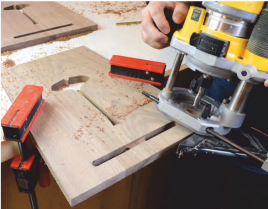
A router equipped with an edge guide and 1/2" spiral downcut bit handles the mortises. After the through mortises are cut from the outside face, flip the panel over and extend the mortises on the inside face (shown here).
