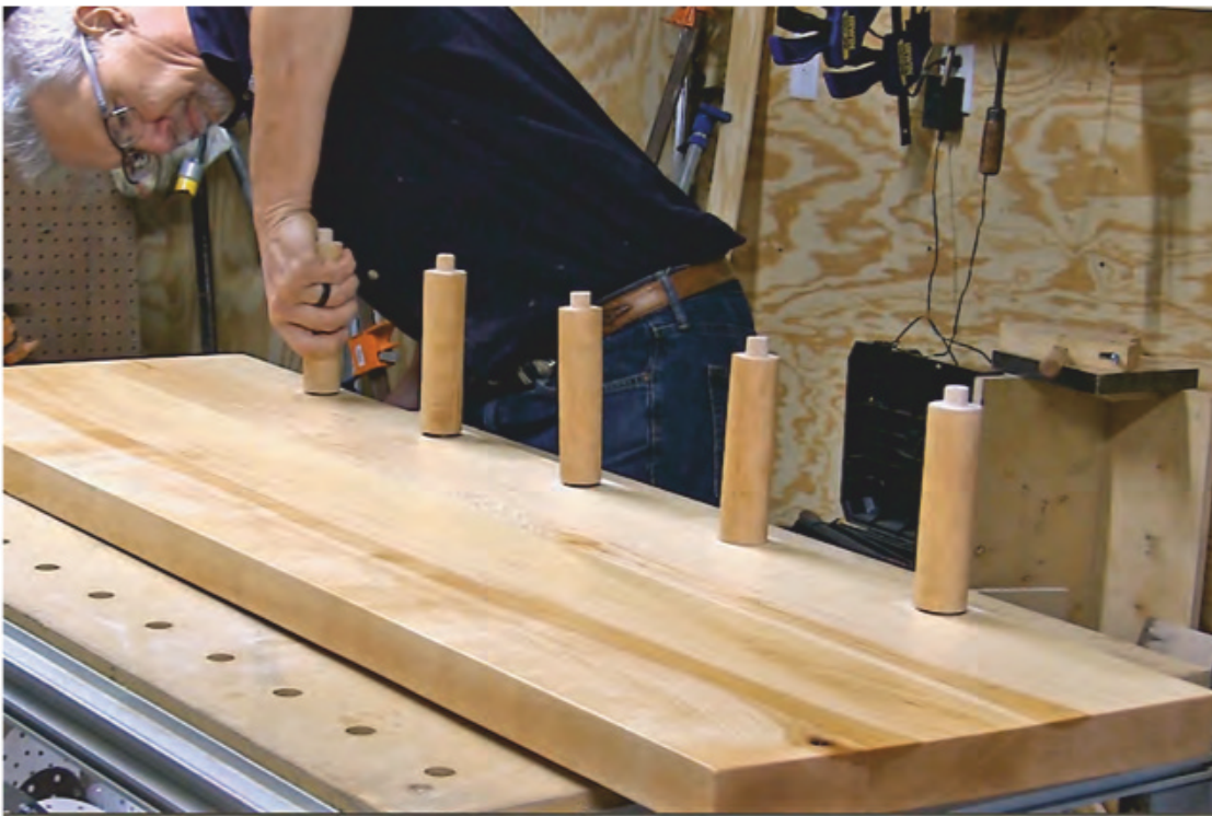
As with any woodworking project, a dry assembly before gluing and clamping is a must. Here the author found that the spindles' tenons needed a little adjustment before they fit properly.
