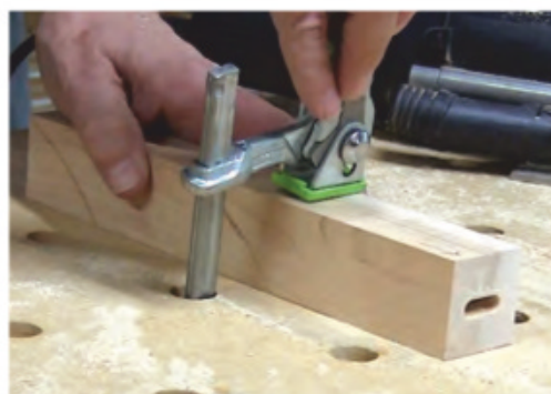
Before turning the spindles, the author used a Festool Domino machine to form mortises on the legs and stretchers. See the Drawings for mortise location details.
