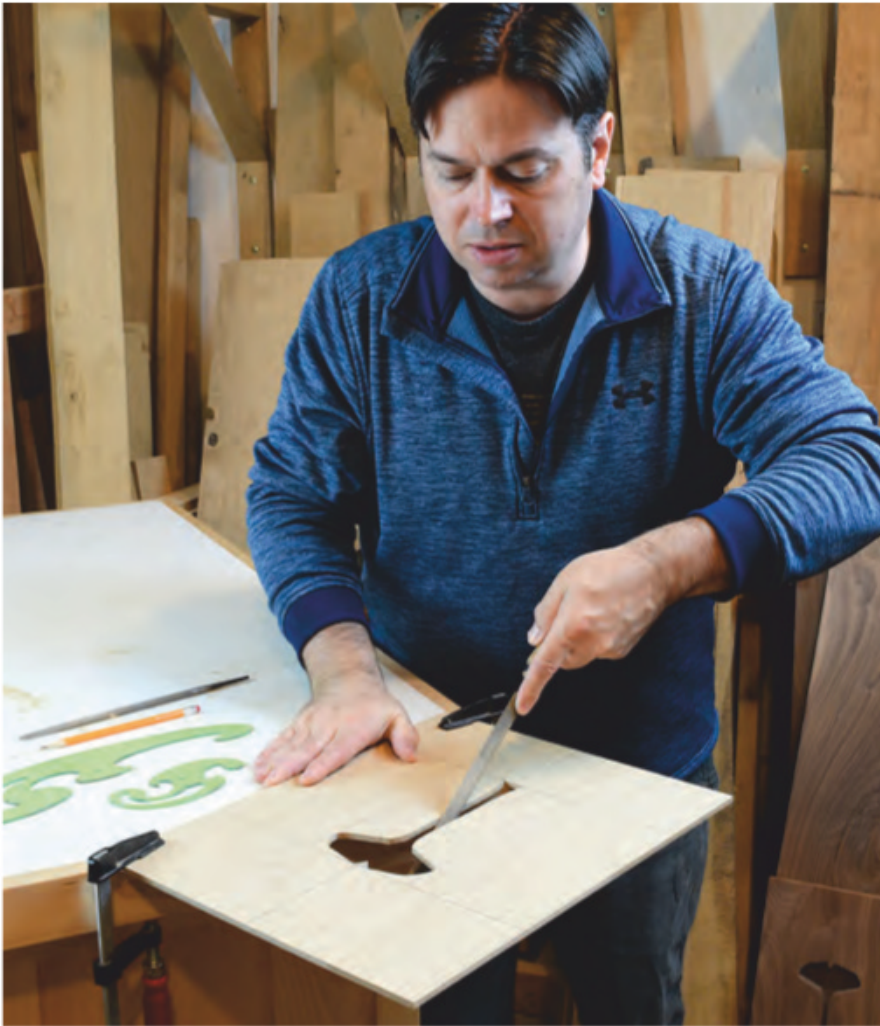
Shape the ginkgo leaf template with flat and round files. Make sure the stem portion of the design is at least 7/16" wide.
