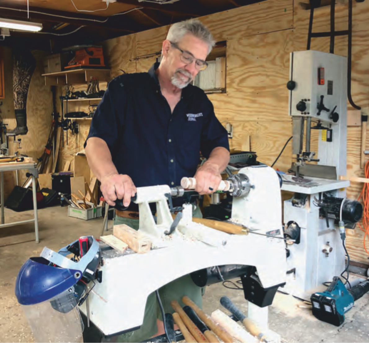
With the blank preparation completed, it was time to get busy turning the various spindles for the undercarriage and those that support the backrest. The spindles that join the backrest to the seat have 5/8"-long tenons turned to 11/16" diameter.
