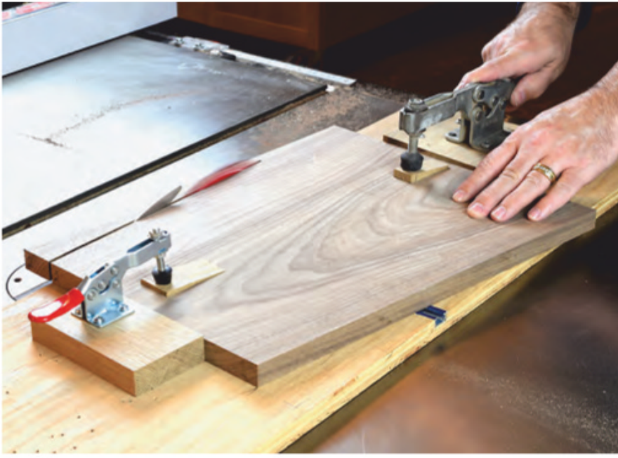
A shop-made tapering sled handily slices the side panels to their 5-degree tapers. This one is guided by a wooden strip riding in the miter slot.
