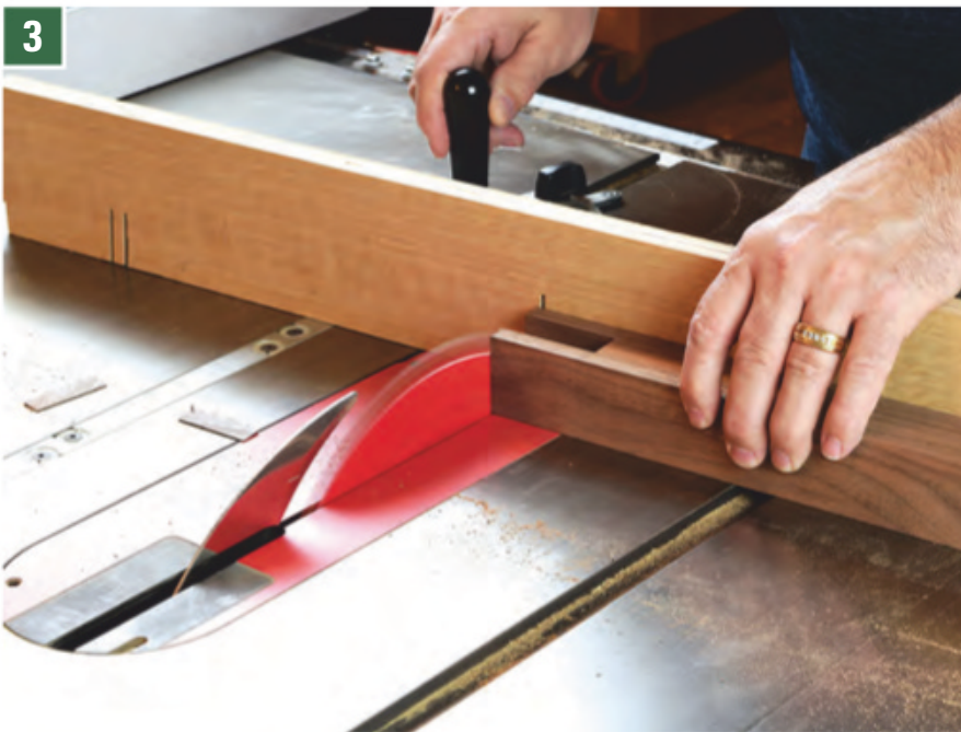
With the miter gauge swiveled to 5 degrees, trim the top ends of the legs. Remove just enough material to create the required angle.
