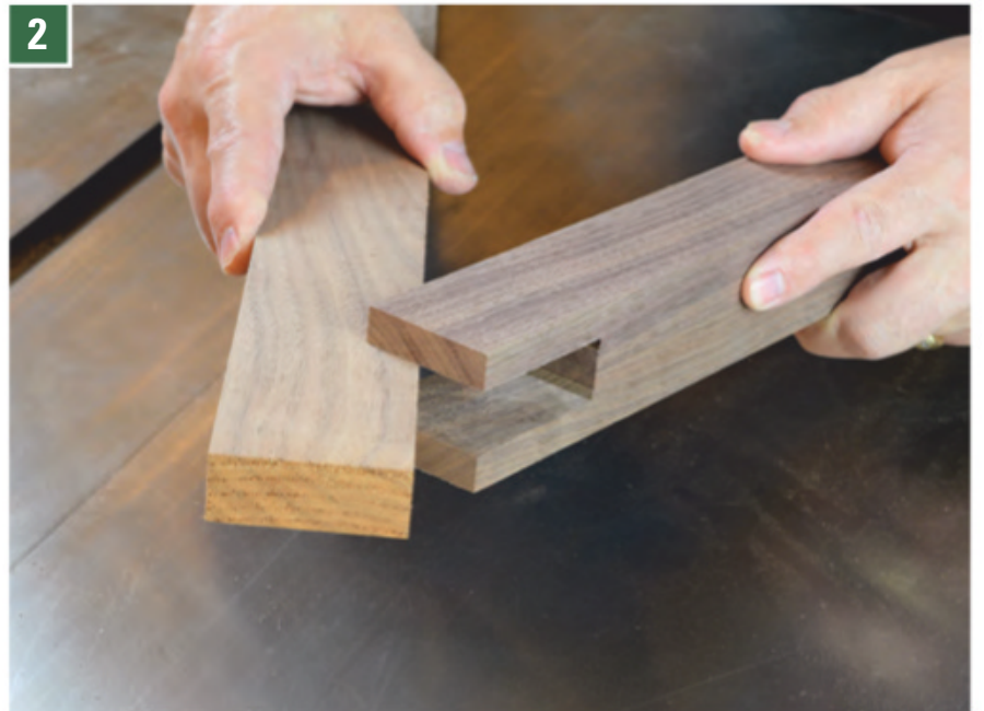
Plane a test board to 3/4" thick, and use it to gauge the width of the leg notches. Incrementally adjust the rip fence as needed, and make more passes until the test board eases into the notch.
