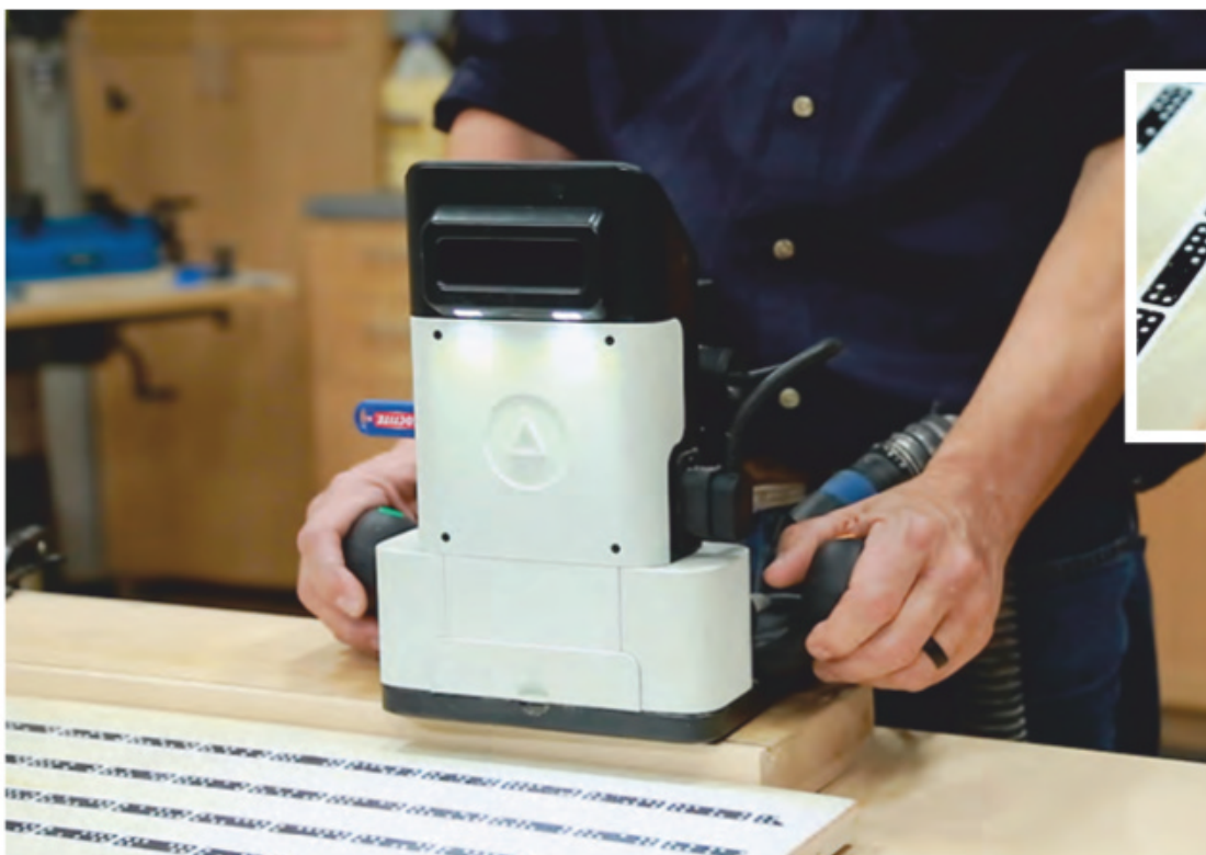
To enhance the Asian influence of this project, a simple bamboo motif (inset) was carved onto the face of the backrest. These mirror image carvings were easily done with a Shaper Origin CNC.
