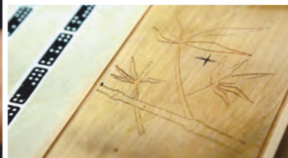
To enhance the Asian influence of this project, a simple bamboo motif (inset) was carved onto the face of the backrest. These mirror image carvings were easily done with a Shaper Origin CNC.
