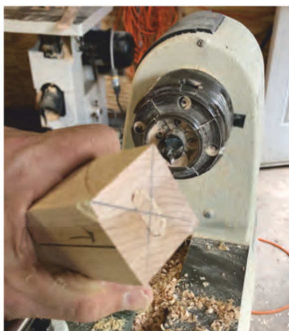
The short stretchers needed a Domino mortise in each end. That made mounting them between centers difficult. A Domino was put into each mortise and cut flush to solve the problem.
