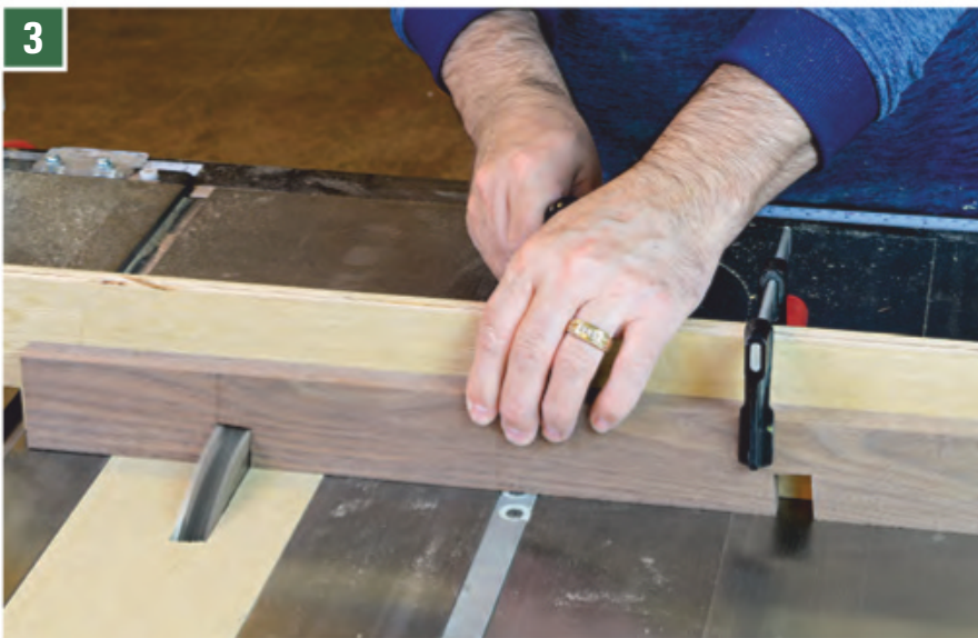
Tilt a dado blade to 5 degrees to cut opposite-facing notches in the cross rail. Use a full 3/4" dado stack plus a .004" shim to ensure the parts will come together without a wrestling match.
