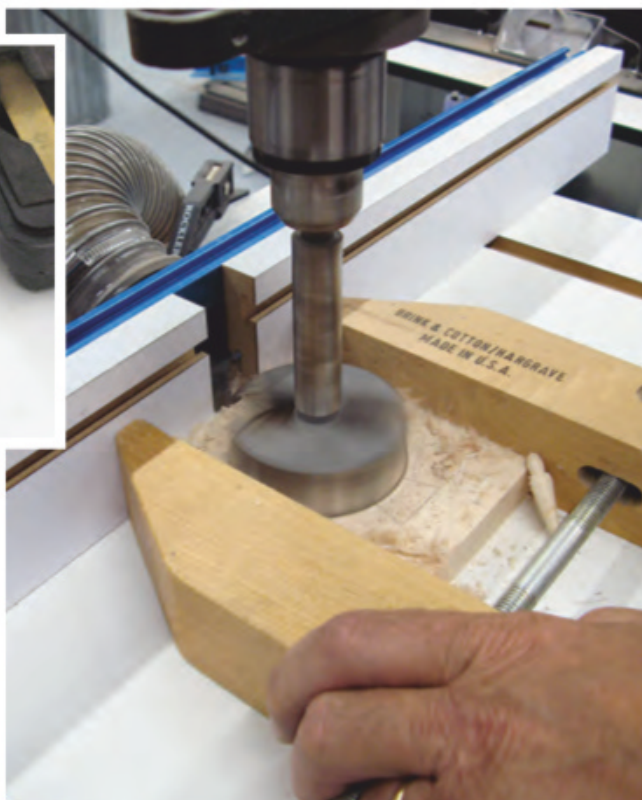
To drill a 7/16"-deep recess in the body for the clock's quartz works, the author used a 5/16" brass setup bar (above) to dial in the Forstner bit's depth of cut, then clamped the workpiece in a large wood screw to hold it securely for drilling (center). After the large hole was bored, he switched to a 5/16"-diameter brad point bit to drill a through hole at the centerpoint (far right).
