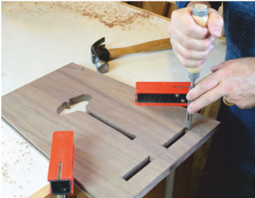
Chisel the corners of the four through mortises square. Make these cuts into the outside faces of the panels to reduce the chances of chipping the mortise edges. That damage would show after final assembly.
