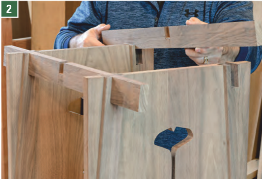
Test fit the stretcher rails in the legs' bridled notches. The stretcher rails project 3 15/16" beyond the legs, so make sure to center the rails for the next step.
