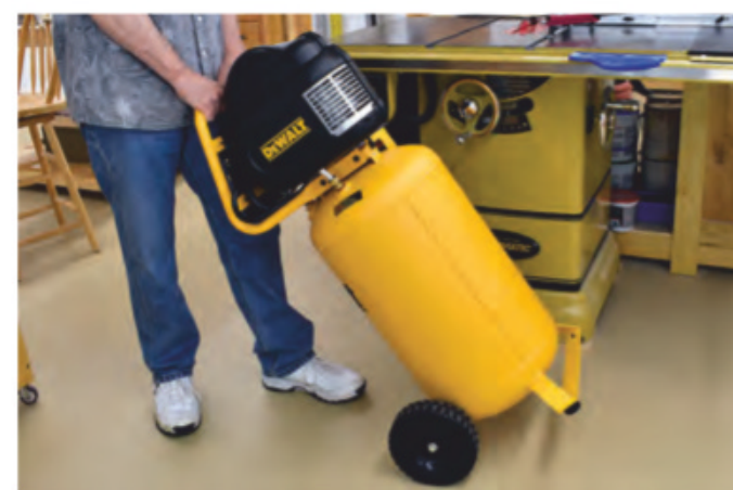
In spite of a vertical air compressor's top-mounted bulk, wheels allow it to be moved around the shop with relative ease.
