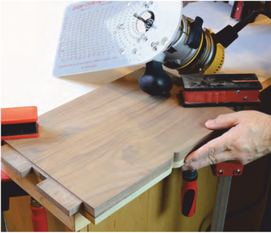
The shelf receives a V-notch detail on both long-grain edges. Here a template is clamped beneath the shelf, and the shape is routed with a 1/4"-dia. flush trim bit.
