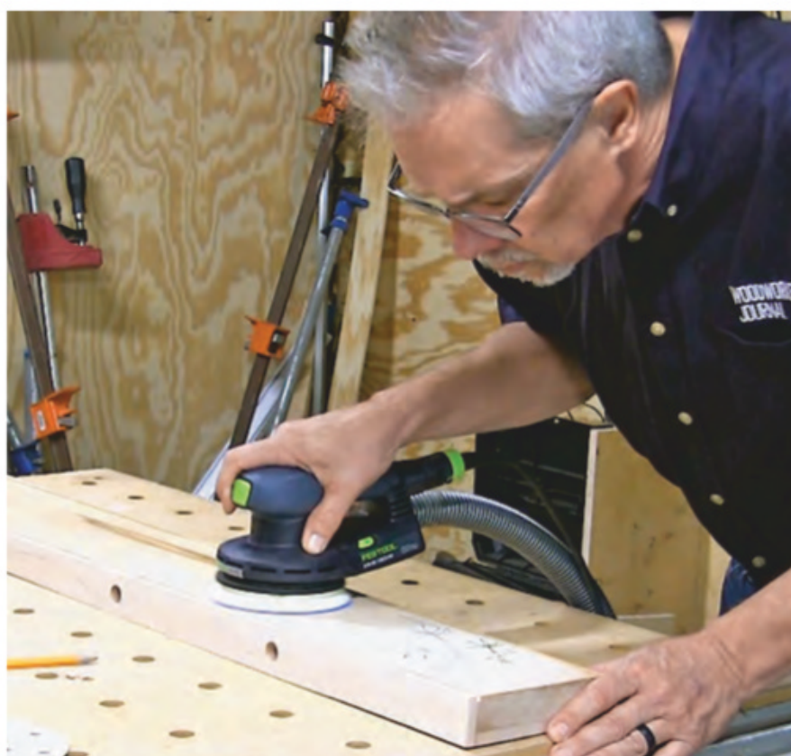
After the excess and overflow of the green epoxy was sanded away, the surfaces of the backrest and seat were smoothed up to 400-grit.
