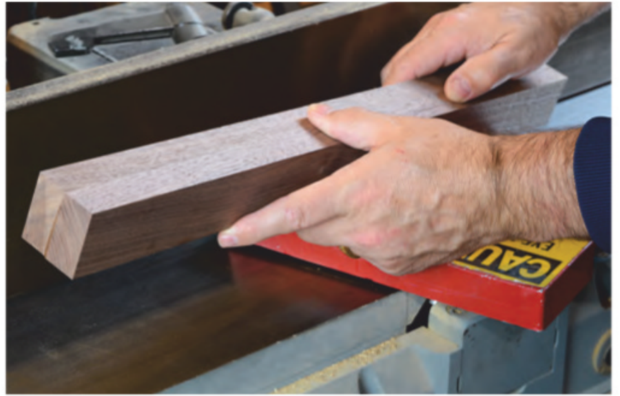
The author created 1 \frac{3}{4} "-thick leg blanks from two strips of 7/8"-thick stock glued together. He then planed the flattened blanks to 1 \frac{5}{8} " square.
