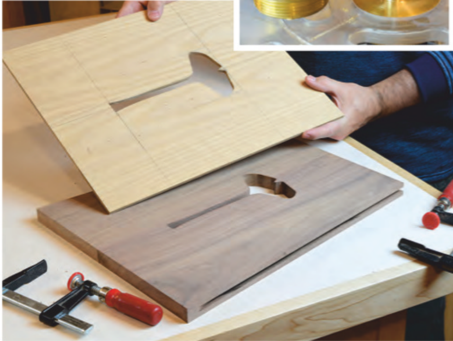
Start with a 7/16" bushing installed to rough out the inner waste material in several clockwise passes. Then switch to a 3/8" guide bushing with the same router bit for a final cleanup pass. The resulting shape needs very little sanding.
