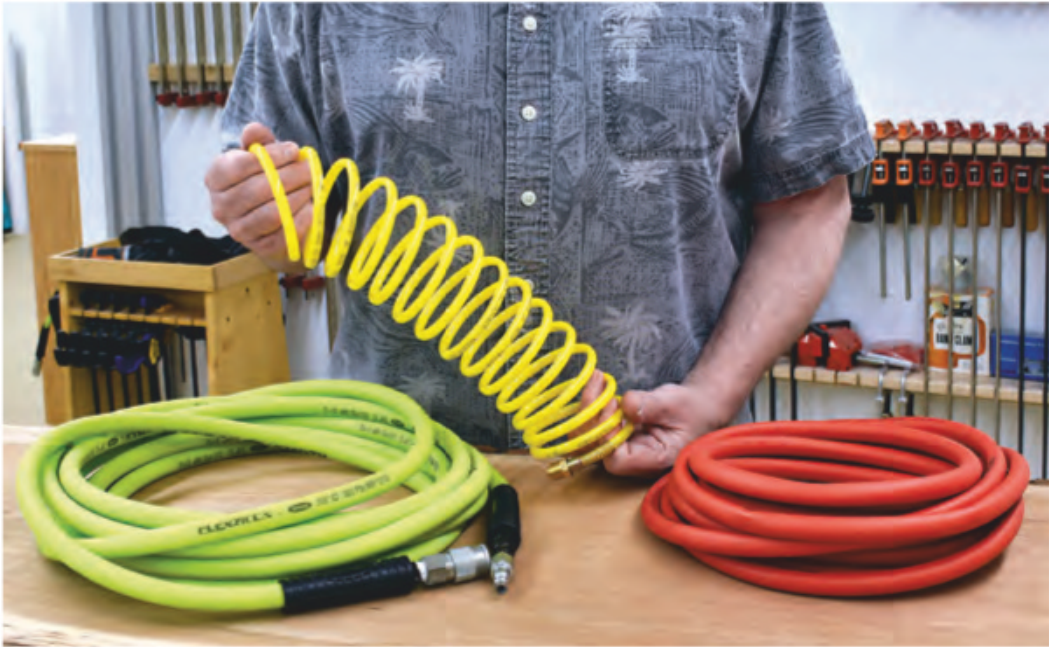
An air hose is essential. From left, choices include an extremely flexible hybrid polyurethane hose, a retractable spiral hose and a conventional rubber hose.
