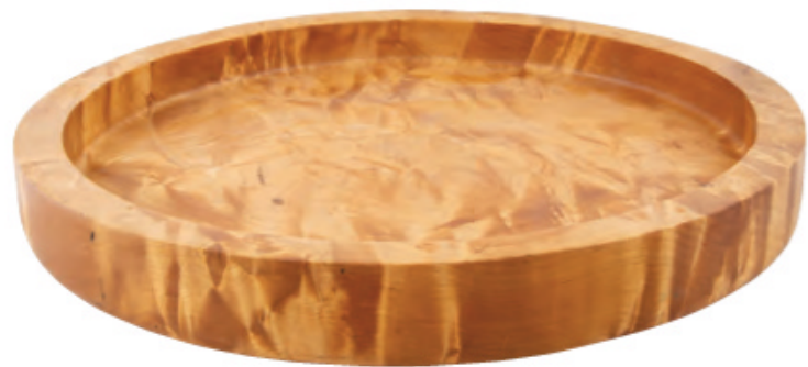
This 14"-dia. x 2"-deep sushi platter was turned by the author in 2003 from an exceptional piece of quilted hard maple. To evoke this Japanese design, he used straight walls with a square rim.
