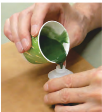
The carved bamboo designs were filled with colored epoxy resin. This "inlay" procedure could not have been easier. Mixol colorant was added to the prepared resin, which was then flowed into the carving with a glue syringe. It cured completely in 24 hours.
