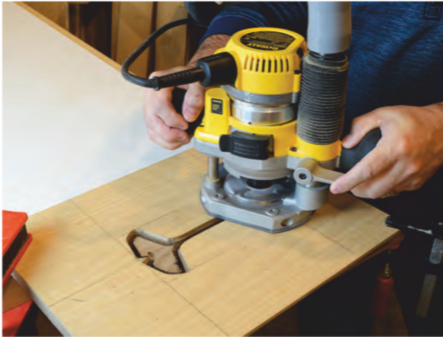
A plunge router removes the waste inside the leaf cutout in a multi-step process. The author used two guide bushing sizes and a 1/4" spiral bit.
