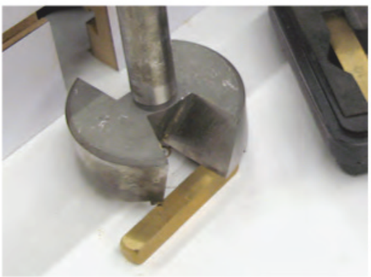
To drill a 7/16"-deep recess in the body for the clock's quartz works, the author used a 5/16" brass setup bar (above) to dial in the Forstner bit's depth of cut, then clamped the workpiece in a large wood screw to hold it securely for drilling (center). After the large hole was bored, he switched to a 5/16"-diameter brad point bit to drill a through hole at the centerpoint (far right).
