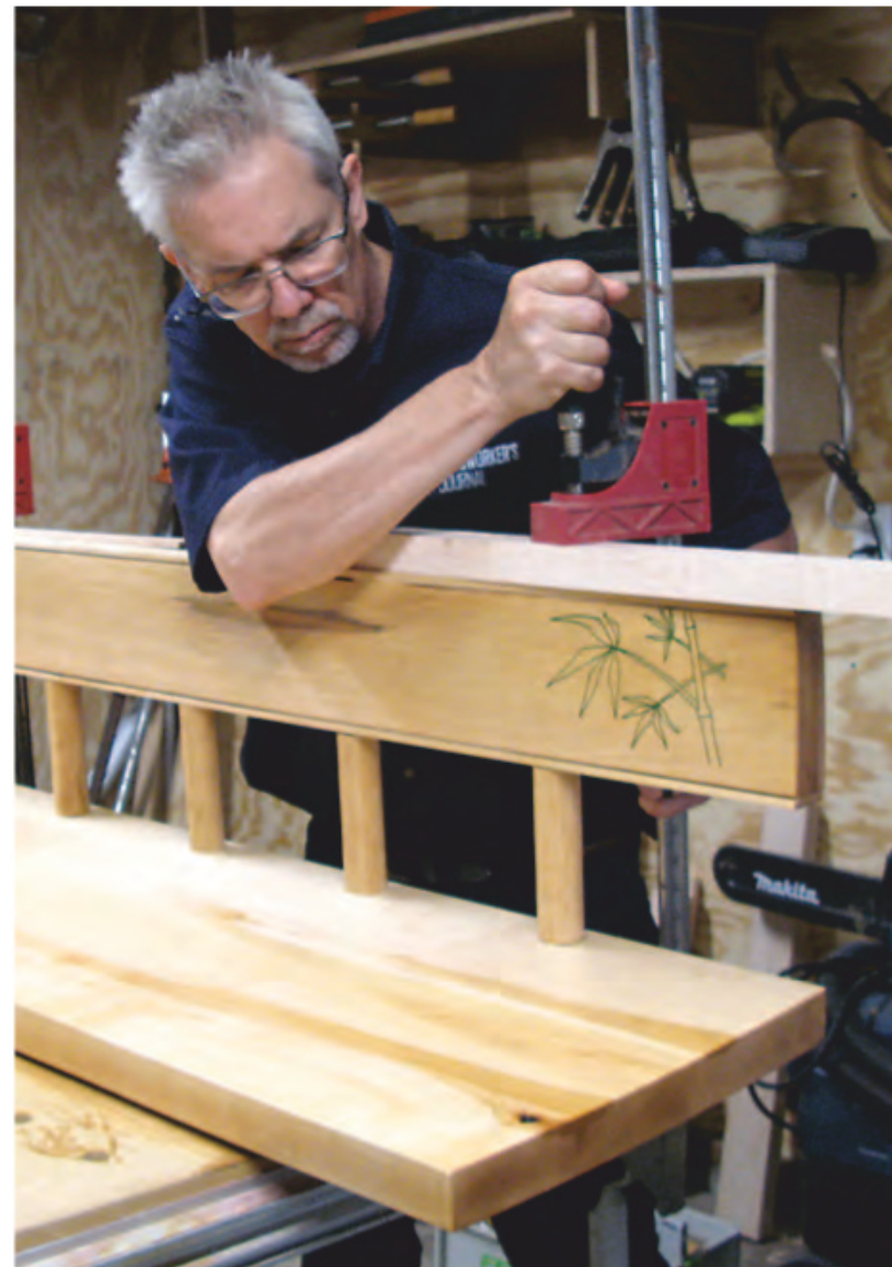
Once the dry fit was successful, it was time to glue and clamp the bench together. The tenons and spindle shoulders provide significant glue area.
