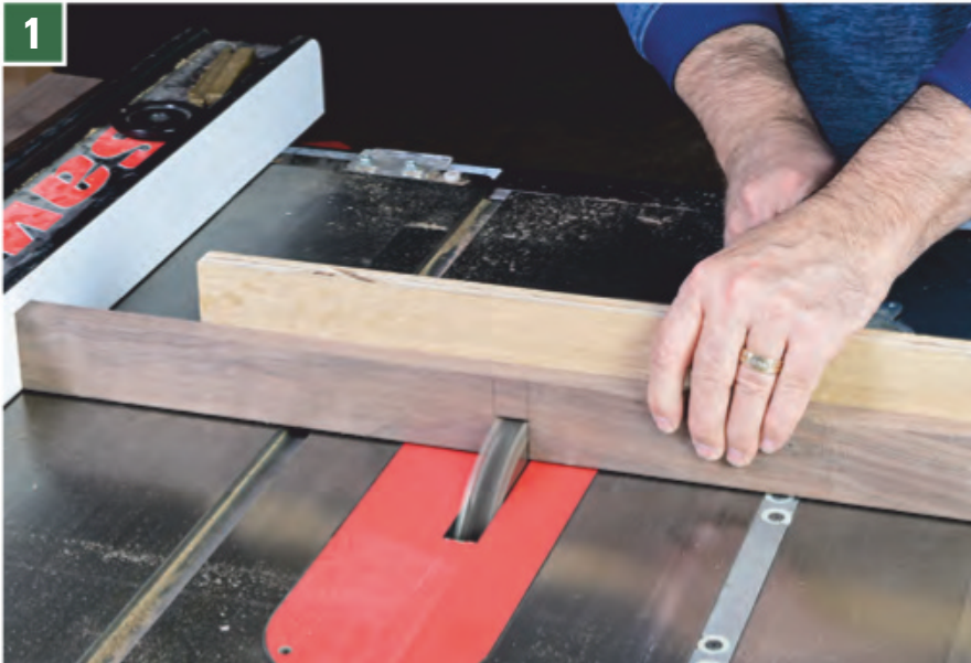
Make a centered notch in the stretcher rails with a dado blade. Since the edge of this part receiving the notch has already been angled, it's important to hold the rail flat against an auxiliary fence.
