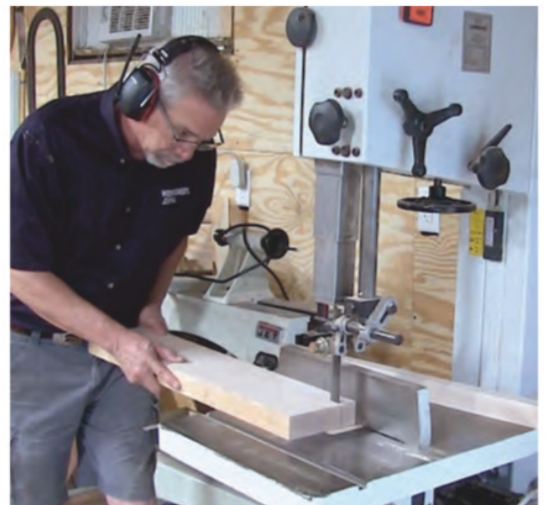
The stock remaining after making the seat and backrest was then cut to width on the band saw and to length on a miter saw. These blanks will be turned into the various spindles.
