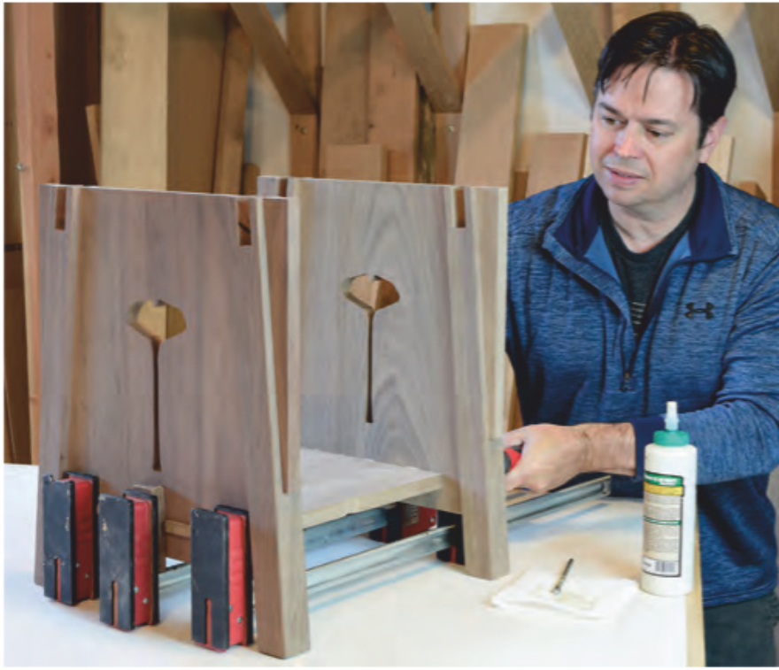
Clamp the side assemblies together with the shelf using parallel clamps. The middle clamp bears on a wooden block to direct pressure between the tenons. Use just enough pressure to close the joints.
