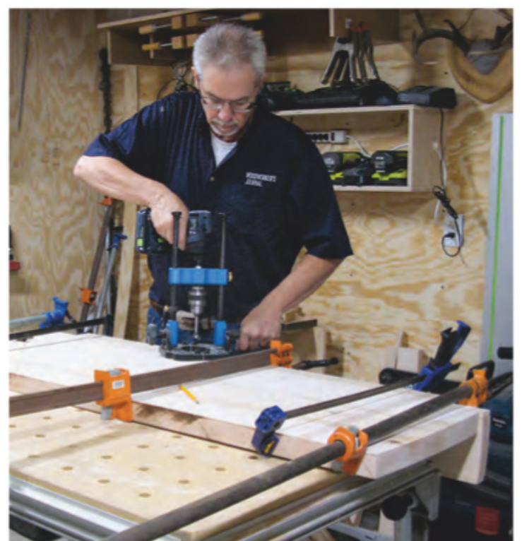
Without a drill press in his home shop, the author used Rockler's Portable Drill Guide to bore 11/16"-diameter holes for the spindles. The guide handled the task easily.
