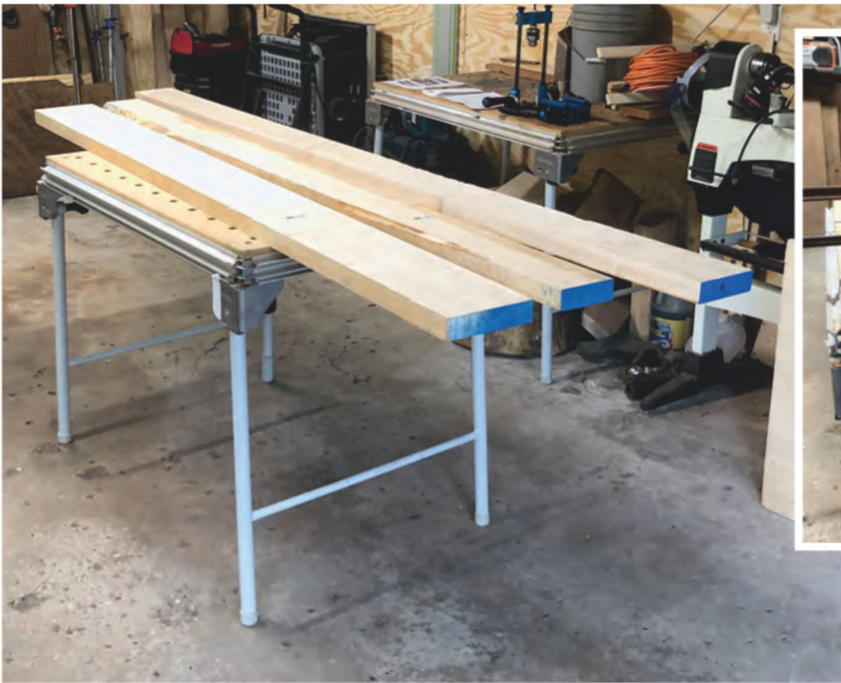
Starting out with 1 3 / 4 "-thick maple lumber, the first step was to glue up a blank for the bench's seat. Thick joints like this require extra time to cure.
