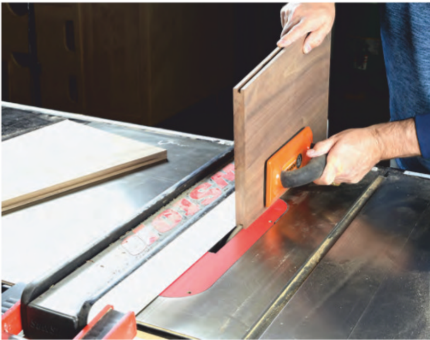
Form stopped grooves in the side panels with a 1/4"-wide dado stack. Note the clamp on the rip fence here, acting as a stop block.
