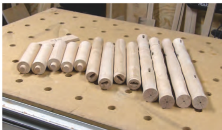
Thirteen spindles of various lengths and shapes are required for this bench. All of them were sanded to 400-grit while still on the lathe to prepare them for a Watco Oil finish.
