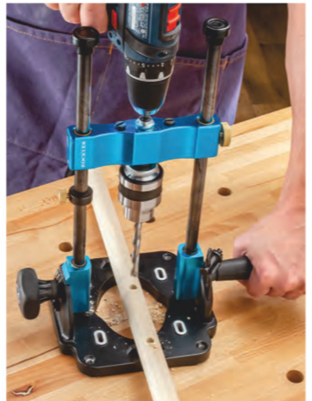
V-notches in the base can hold round workpieces, such as dowels, for drilling centered holes.
