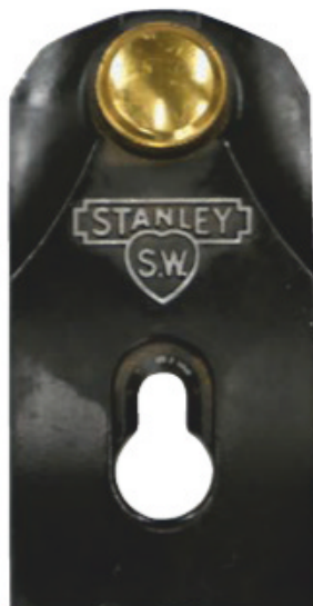
Lever caps are an integral component of both the Bailey and Bedrock plane configuration.
