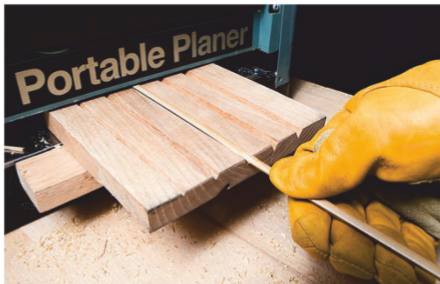
The author uses a heat gun to bend bamboo and get rid of its nodes (photo above). Running the bamboo strips through a planer in a special shop-made jig (photo below) progressively turns them into the tapering triangular strips needed to construct the fly rod.
