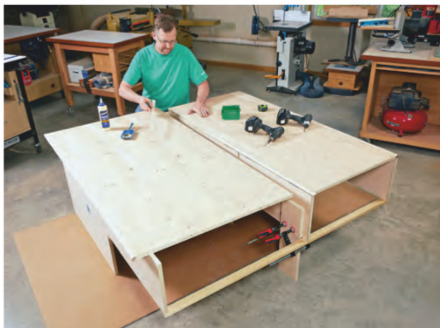
Install the wide and narrow back panels with the carcass facing down. A glued spline, being inserted here, reinforces and aligns the back-panel's mating seam. Prevent the carcass from tipping forward by clamping a scrap in the upper cabinet area to act as a temporary leg against the floor.
