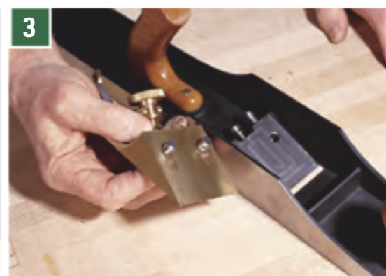
3 A Bedrock frog (above) ingeniously connects the blade assembly firmly to the body. A Bailey frog is not as robust.
