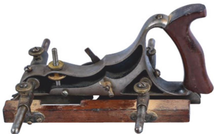
Molding planes were manifold when plane bodies were mainly made of wood. They reached their zenith with the advance of the combination plane.
