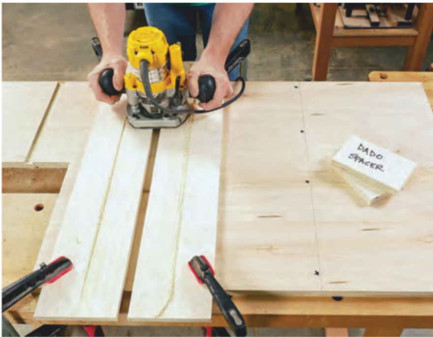
The author used a short piloted mortising bit and a pair of scrap fences to sandwich a couple of spacers of the project plywood in order to create exact-fitting dados in the uprights.
