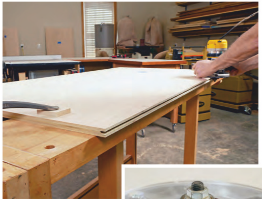
Rout a 1/4"-wide x 1/2"-deep spline slot along the full length of the mating edges of the wide and narrow back panels. A piloted slot-cutting bit (inset) makes the task simple and quick.
