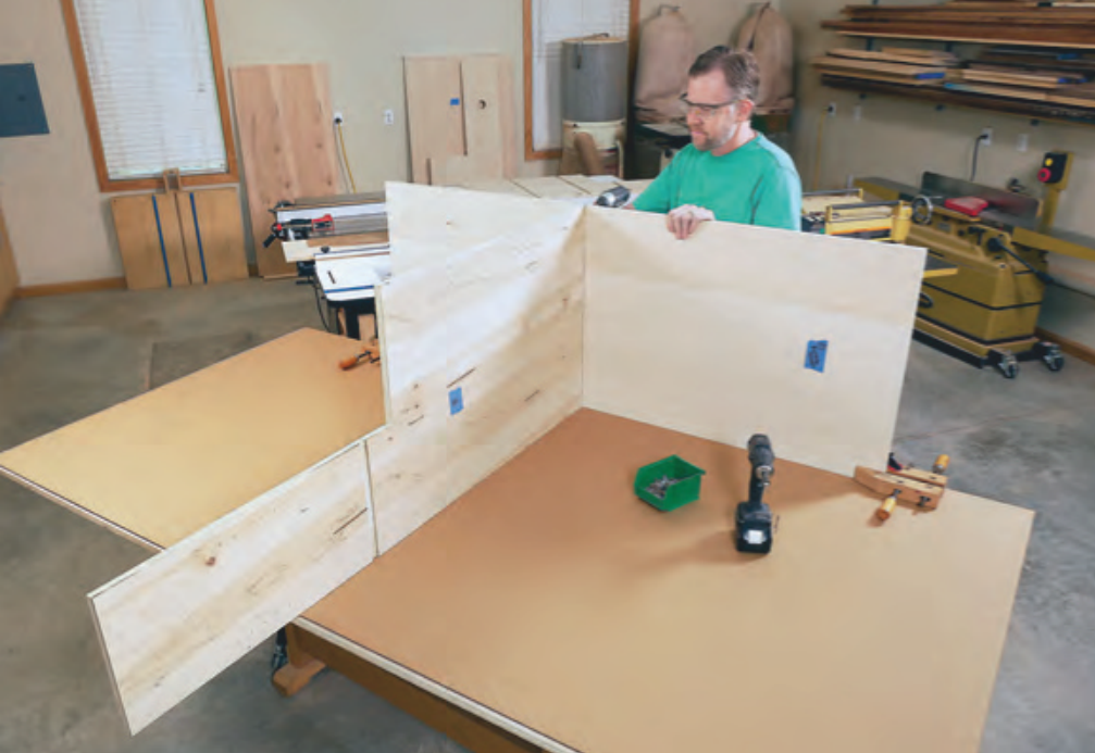
On a large, flat work surface, attach the bottom panel to the uprights with 2"-long countersunk screws. Notice how a pair of wooden hand screws can help to keep the bottom panel upright during this construction step.
