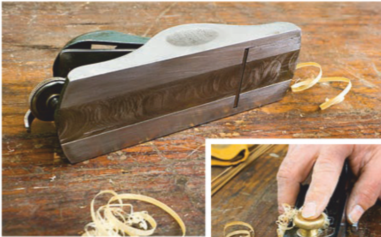
The author created a rod-making plane by routing a .003" groove in the sole of a block plane with several passes on his router table.
