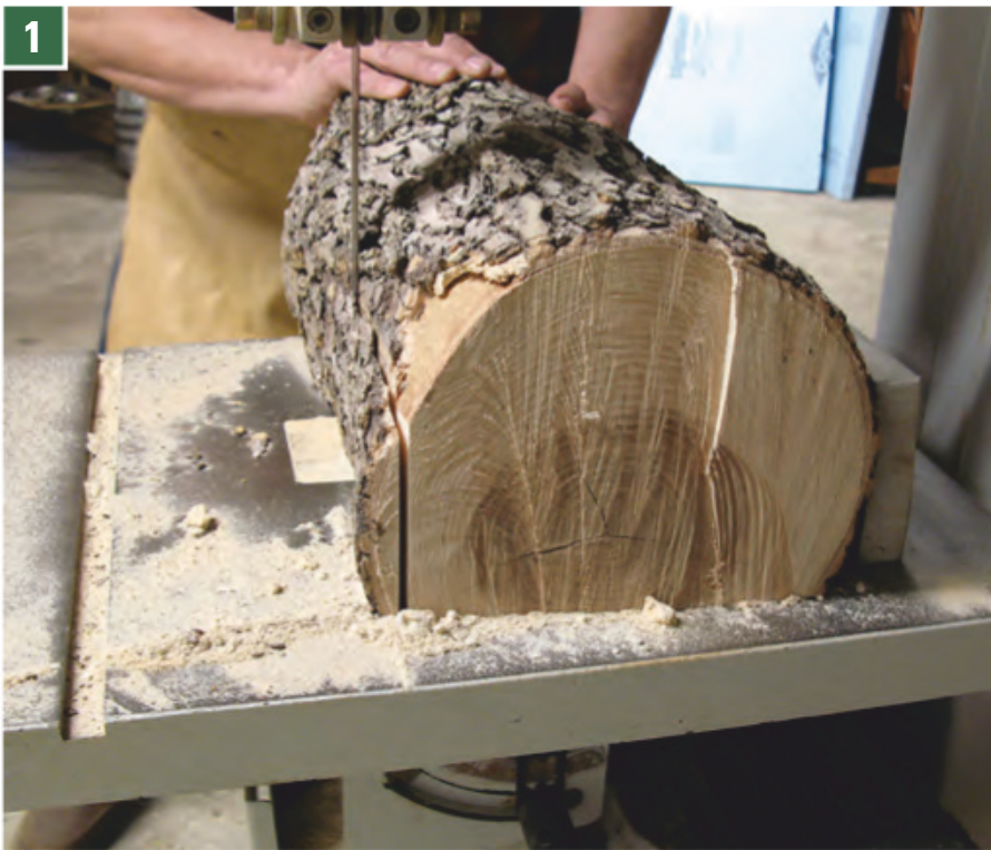
1 After one flat surface is formed, turn that face down and cut another flat surface at 90 degrees to the first. If the bole of the log is straight along its length, you can guide it using the band saw fence. If not, reuse the fixture.
