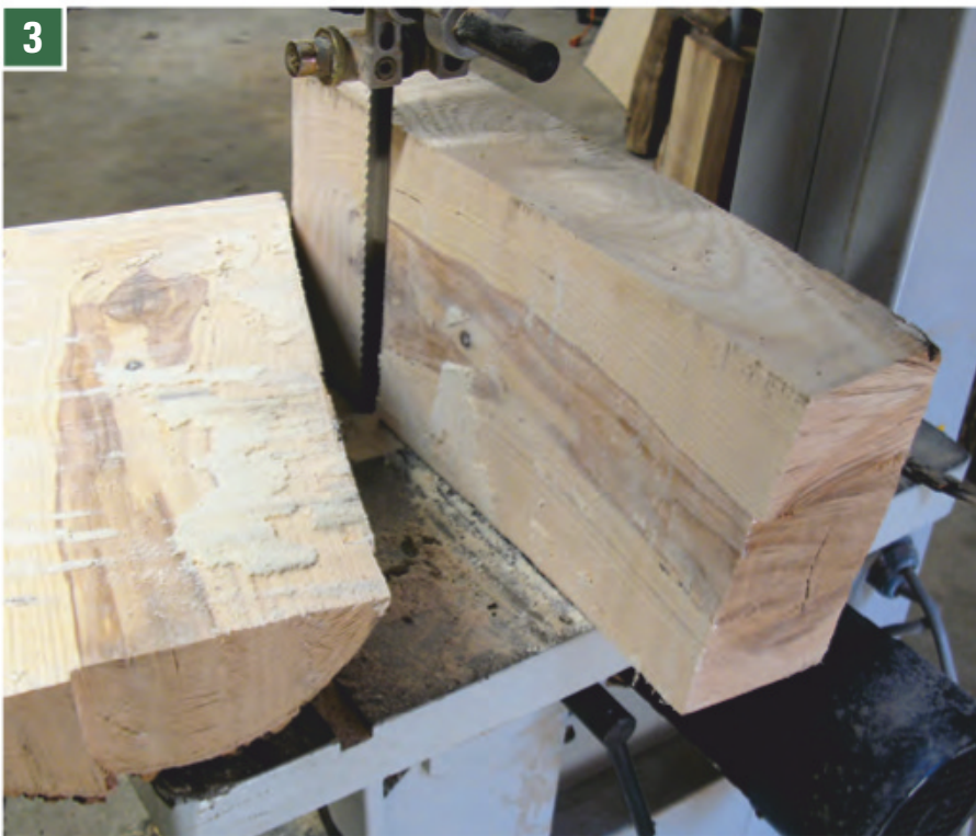
3 The rectangular blank is completed with a fourth cut. You need to think about how deep you want your bowl to be before you make this cut. In this case, the drop from the log is still thick enough to make a turning blank.
