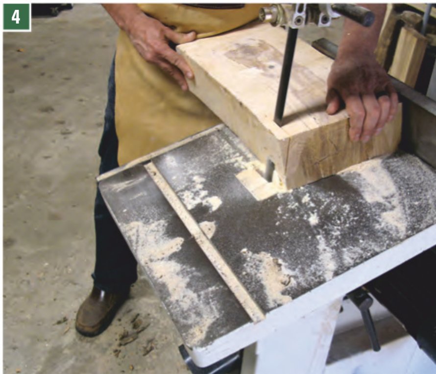
4 The last step on the band saw is refining the edges and ends of the newly formed blank. Here the author angles the sides of the blank. Next he will cut the curves onto the ends of the lumber. Then it's on to power carving.
