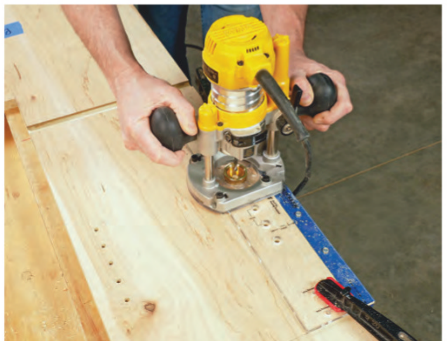
Drill or rout two rows of shelf pin holes in the upper cabinet area of uprights A and B. Here, a guide collar and straight or spiral bit in a plunge router take the place of a drill/driver to produce tearout-free holes.
