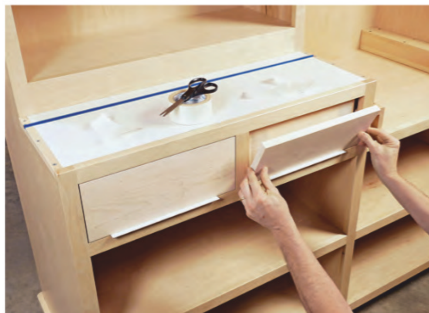
Scraps of plastic laminate provide about 1/16" of clearance for positioning the drawer faces in the face frame. Double-sided tape holds them in place temporarily before the drawers are opened and clamps are installed.
