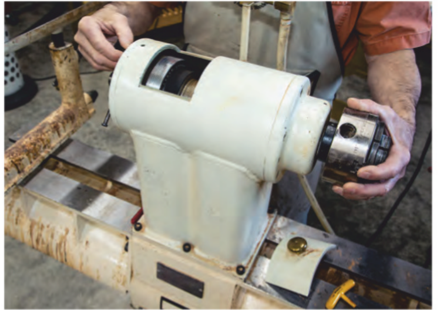
The author's Oneway 2436 has 48-position indexing. While this is certainly a beneficial feature, don't fret about too few indexing positions. You can get around the limitation in various ways, such as using dividers.
