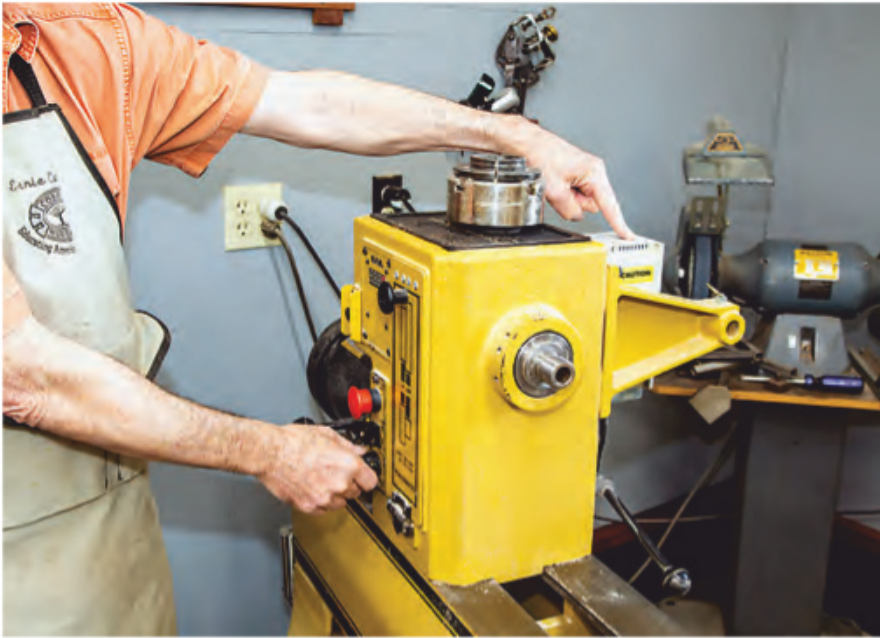
This Powermatic lathe has electronic speed control with a VFD (being pointed to) at the back of the headstock. The author is adjusting the speed with a potentiometer on the face of the headstock.
