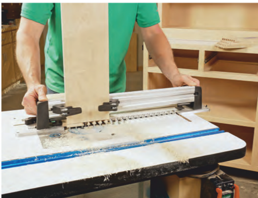
Half-blind dovetails will form rock-solid connections for the front corners of these drawers. The author milled them on his router table using a Leigh RTJ400 "template down" style dovetail jig.
