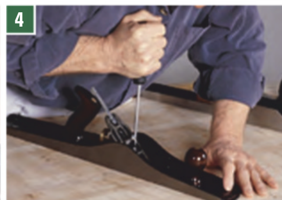
4 Adjust the frog to support the blade securely. The mouth opening should be set at 1/32".
