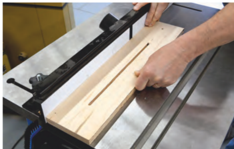
Install a 5/16" straight bit in a router table. Set the bit height to 1". Place the adjustable post on the router table with the top hole on the left side, and fit the router bit through the top hole. Position the router table fence up against the edge of the workpiece. Then turn on the router and feed the board along the fence to cut a slot from the top hole to the bottom hole.
