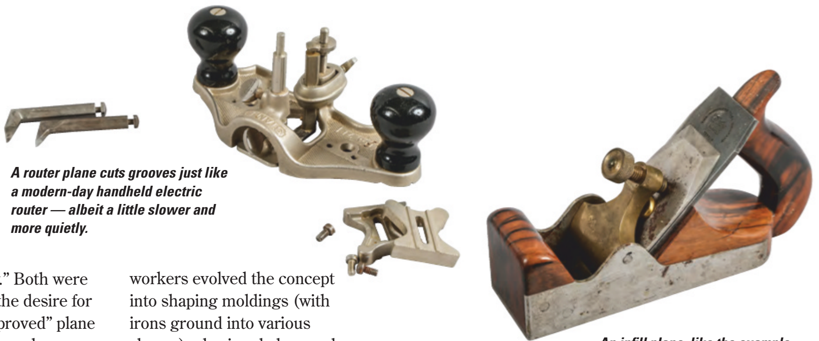
An infill plane, like the example above, has a metal body filled with wood. Manufacturers such as Spiers and Norris produced planes of exceptional quality and beauty.
