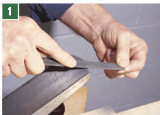
1 To make your plane less likely to mar the wood’s surface, file a substantial chamfer on the toe and heel of the plane’s sole.
