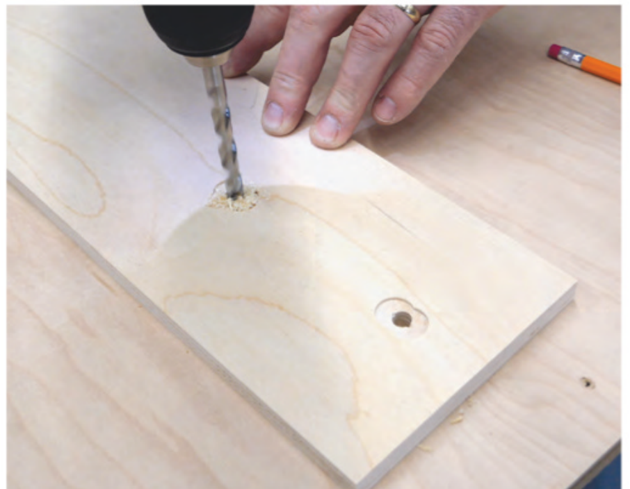
Drill 5/16"-diameter T-bolt holes through both base post pieces. Drill the holes through the back base post first, centering the holes in each bolt head recess. Then use the back piece as a template for drilling the holes through the front base post.
