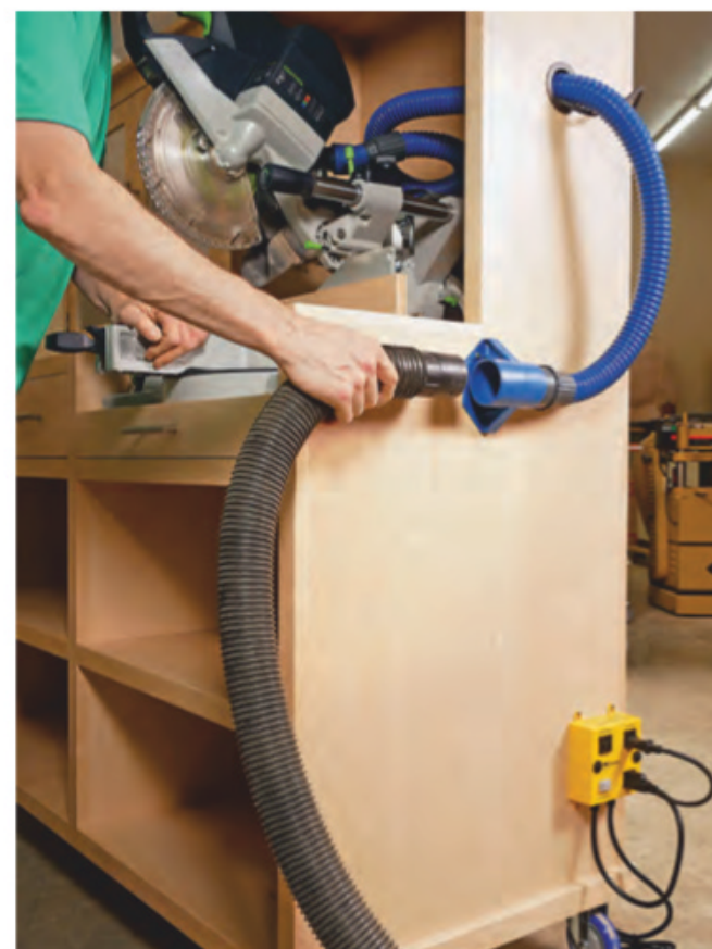
Various Rockler Dust Right components connect the saw to a shop vac hose. An iVac switch automatically activates the vacuum when the saw starts.
