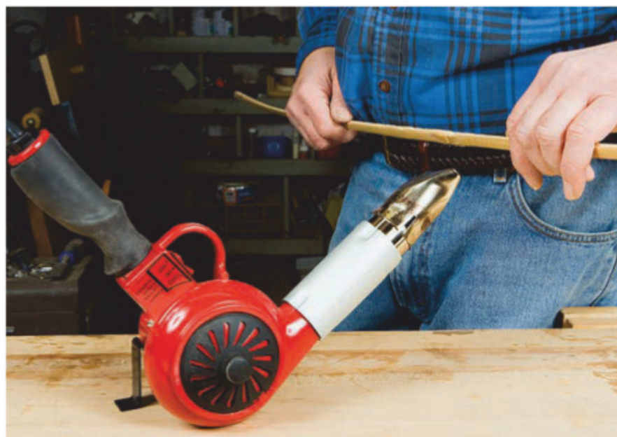
The author uses a heat gun to bend bamboo and get rid of its nodes (photo above). Running the bamboo strips through a planer in a special shop-made jig (photo below) progressively turns them into the tapering triangular strips needed to construct the fly rod.
