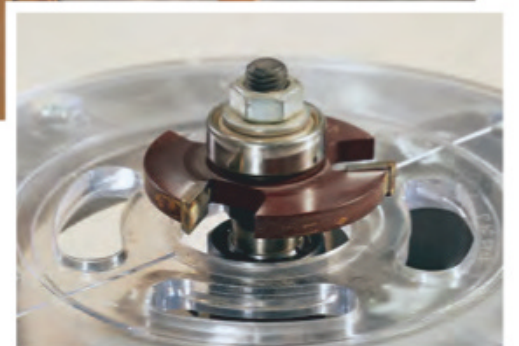
Rout a 1/4"-wide x 1/2"-deep spline slot along the full length of the mating edges of the wide and narrow back panels. A piloted slot-cutting bit (inset) makes the task simple and quick.
