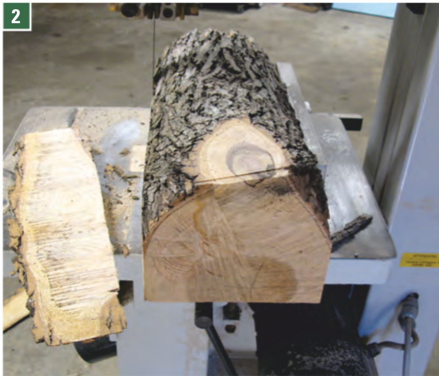
2 Spin the log around and cut a third flat surface onto it. Try not to remove too much material, as the blank gets narrow in a hurry. This is a dusty process, so dust collection is a good idea. Consider wearing a respirator, too.
