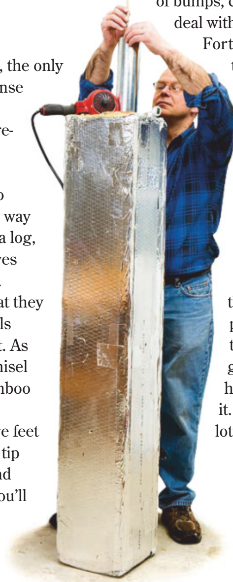
Using a shop-made "bamboo cane kiln," our author demonstrates one of the many steps required to create a bamboo fly rod.
