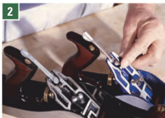
2 The old-style blade controls are more strongly made than the stamped metal version today.
