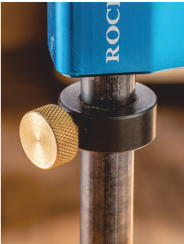
An integral depth stop with knurled brass knob (left) sets the drilling depth for repeatable drilling. The Guide offers 9 5 / 16 " of capacity from the end of the chuck to the bottom of the base (right).
