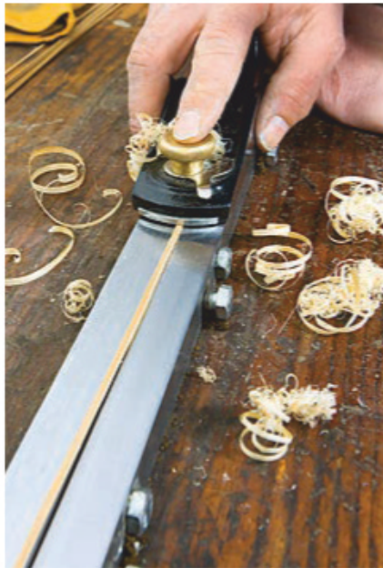
The author created a rod-making plane by routing a .003" groove in the sole of a block plane with several passes on his router table.
