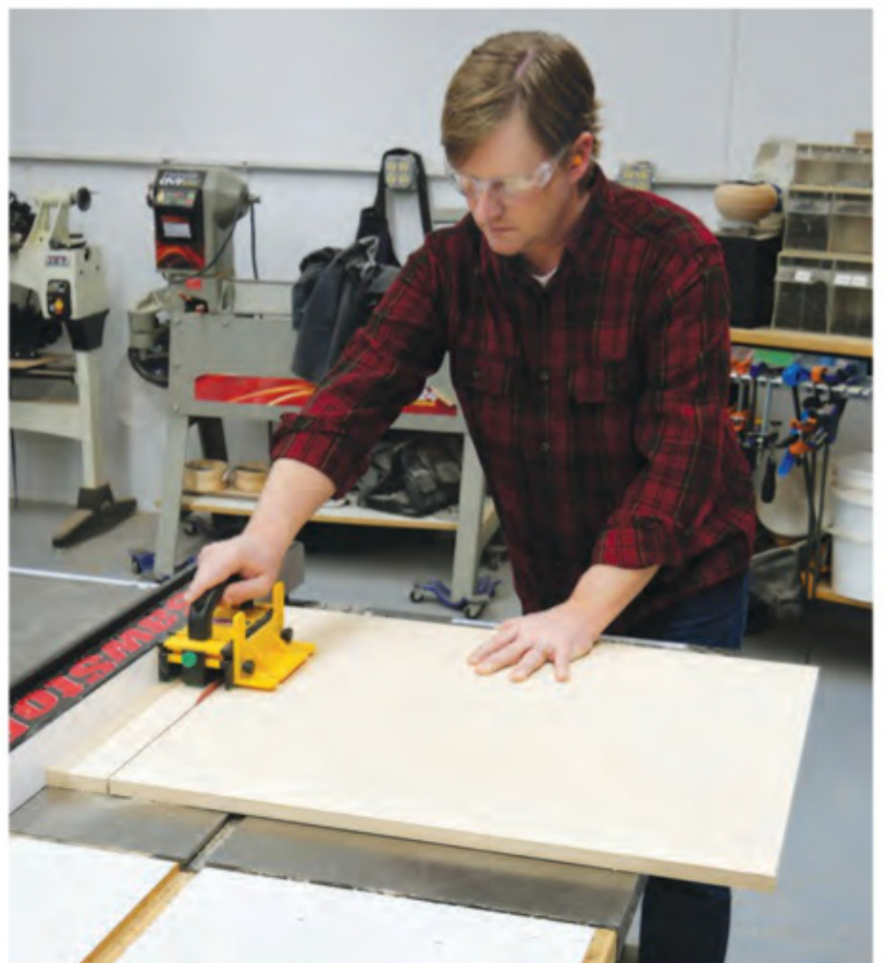
Crosscut a 2 3/4"-wide strip off the end of each panel first, following the Plywood Cutting Diagram, above. These become the sides of the case. Then rip a long strip for the case's top and bottom pieces.
