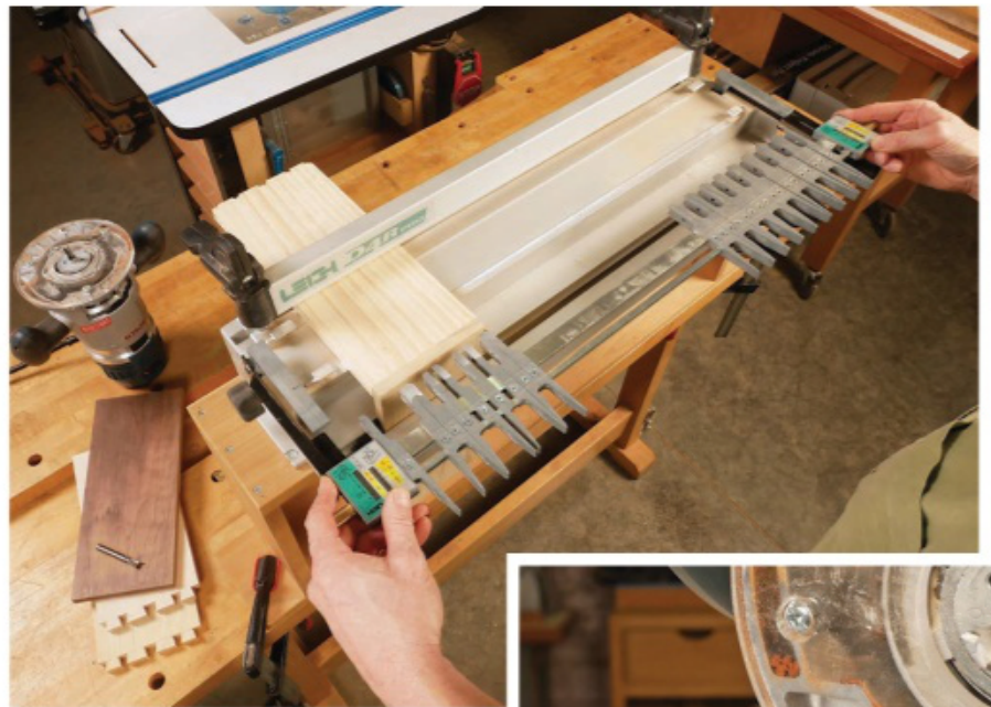
Once the tails of a through dovetail joint are routed on an adjustable template (inset), flipping the template over resets the jig for cutting the mating pattern of pins and tail sockets on the pin board.
