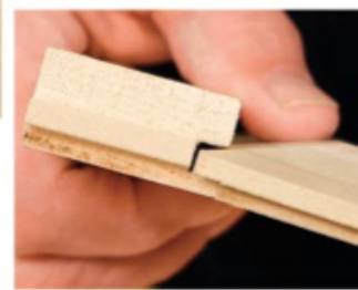
4 A shallow rabbet milled around the back face of the door panel fits its edges to the frame grooves and brings the back faces of the parts flush (inset).
