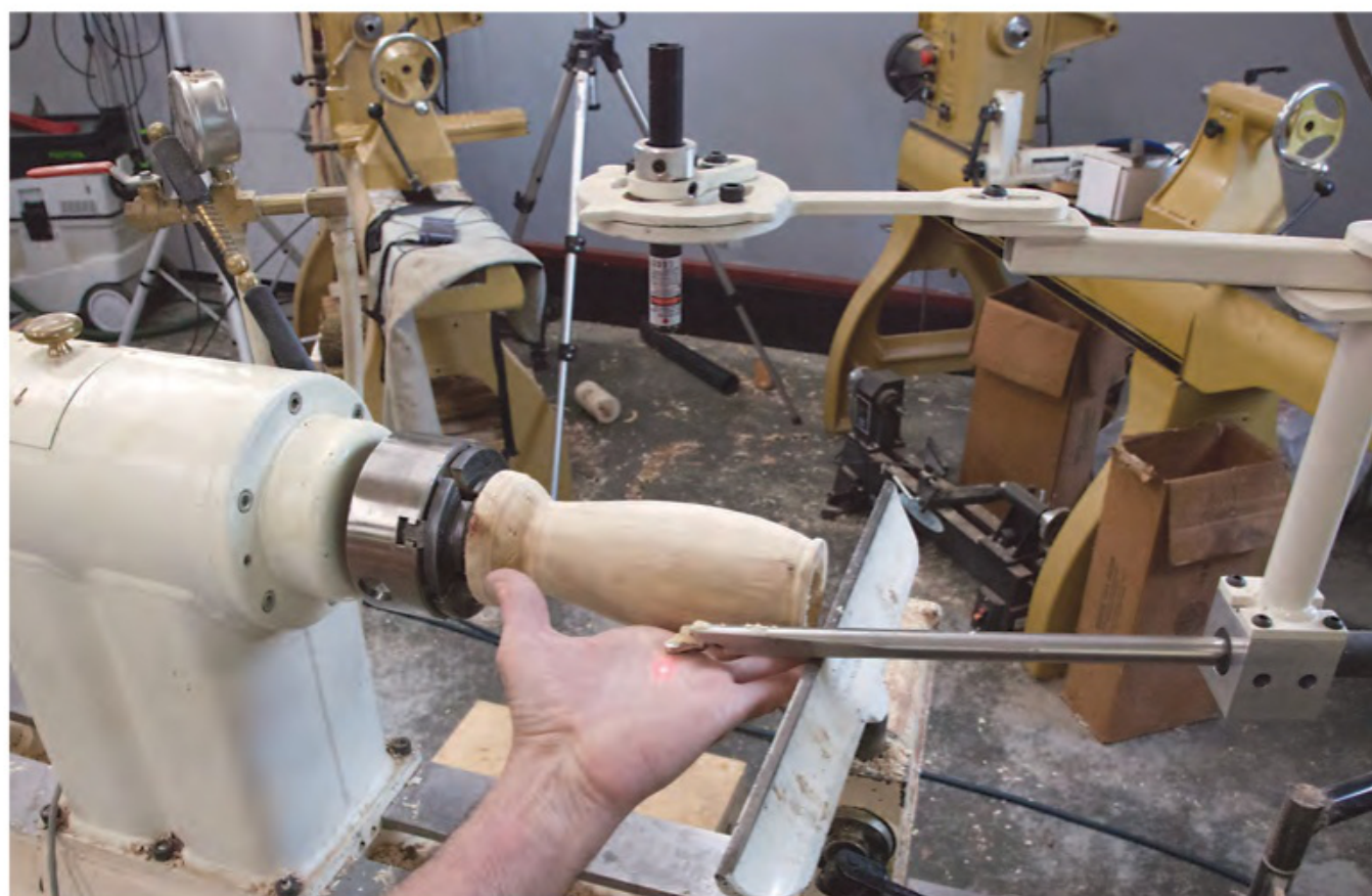
The laser beam's offset from the edge of the boring bar (reflected on the author's hand) indicates the wall thickness the setup will cut. The laser can be adjusted left or right as desired for turning thinner or thicker walls.
