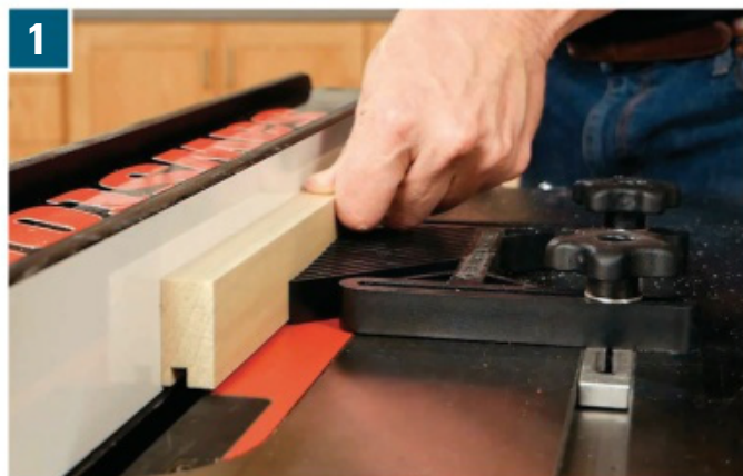
1 Plow a 1/4" x 1/4" groove along one edge of the door's stiles and rails, using a table saw and dado blade. Locate this offset groove 1/8" from the back part faces.
