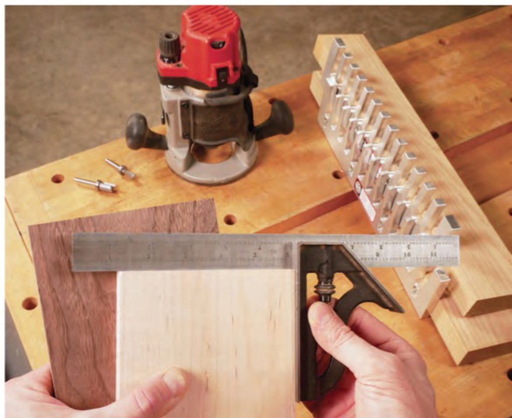
You'll better your odds for dovetailing success if you begin with workpieces that are flat, of uniform thickness and with edges and ends that are precisely square. Prepare your stock carefully.
