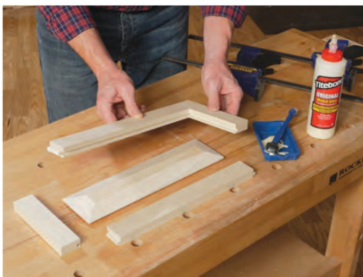
Assemble the drawer's raised panel framework with glue and clamps. Be careful to only glue the tongue-and-groove corner joints; the panel must be able to float freely in its grooves.
