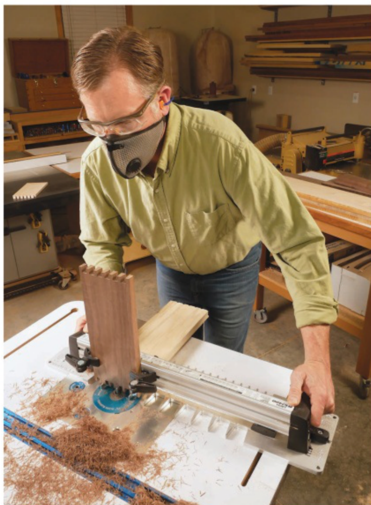
The RTJ400 Dovetail Jig from Leigh Industries is a "top down" variation on the fixed-template concept: here, workpieces clamp above the template, which is fed over a router table. In this photo, through dovetail pins are being cut.
