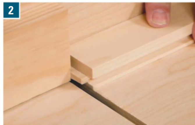
2 Raise 1/4"-long tongues on the ends of the rails to fit the frame grooves. A stop, clamped to a crosscut sled, ensures that the tongues will all be the same length.
