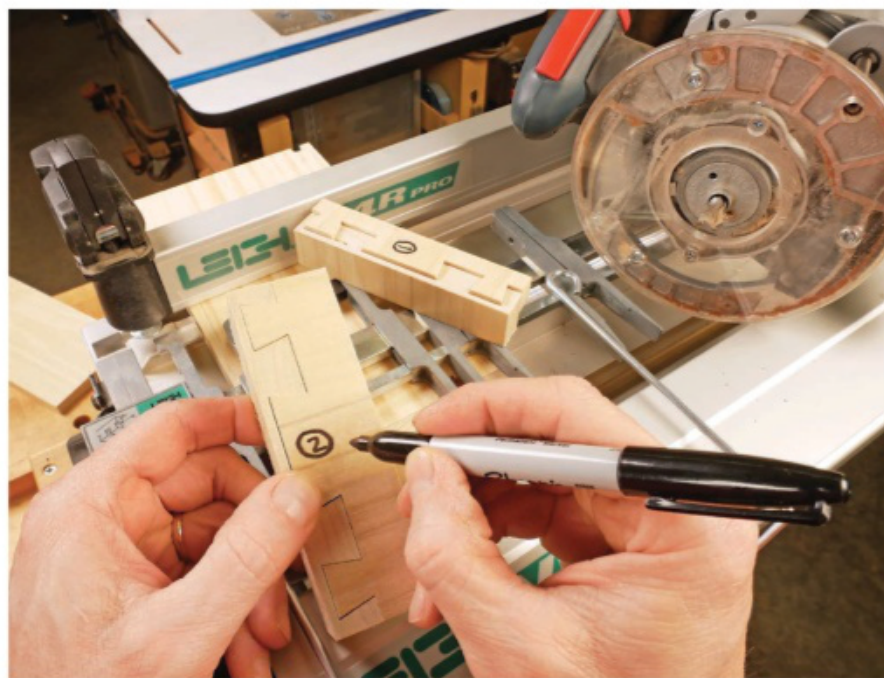
Fine-tuning the settings on a dovetail jig can be time-consuming. Bit depth, stops on the jig and template adjustments all can impact how joints fit together. Mark the order of the test joints to keep track of your progress.
