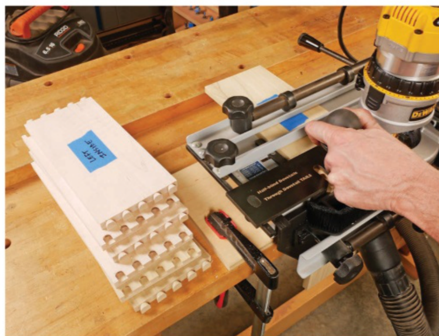
Once a dovetail jig and router bit (or bits) are properly set up, you can machine dovetails quickly and easily for one drawer or a production run of as many drawers as you need.
