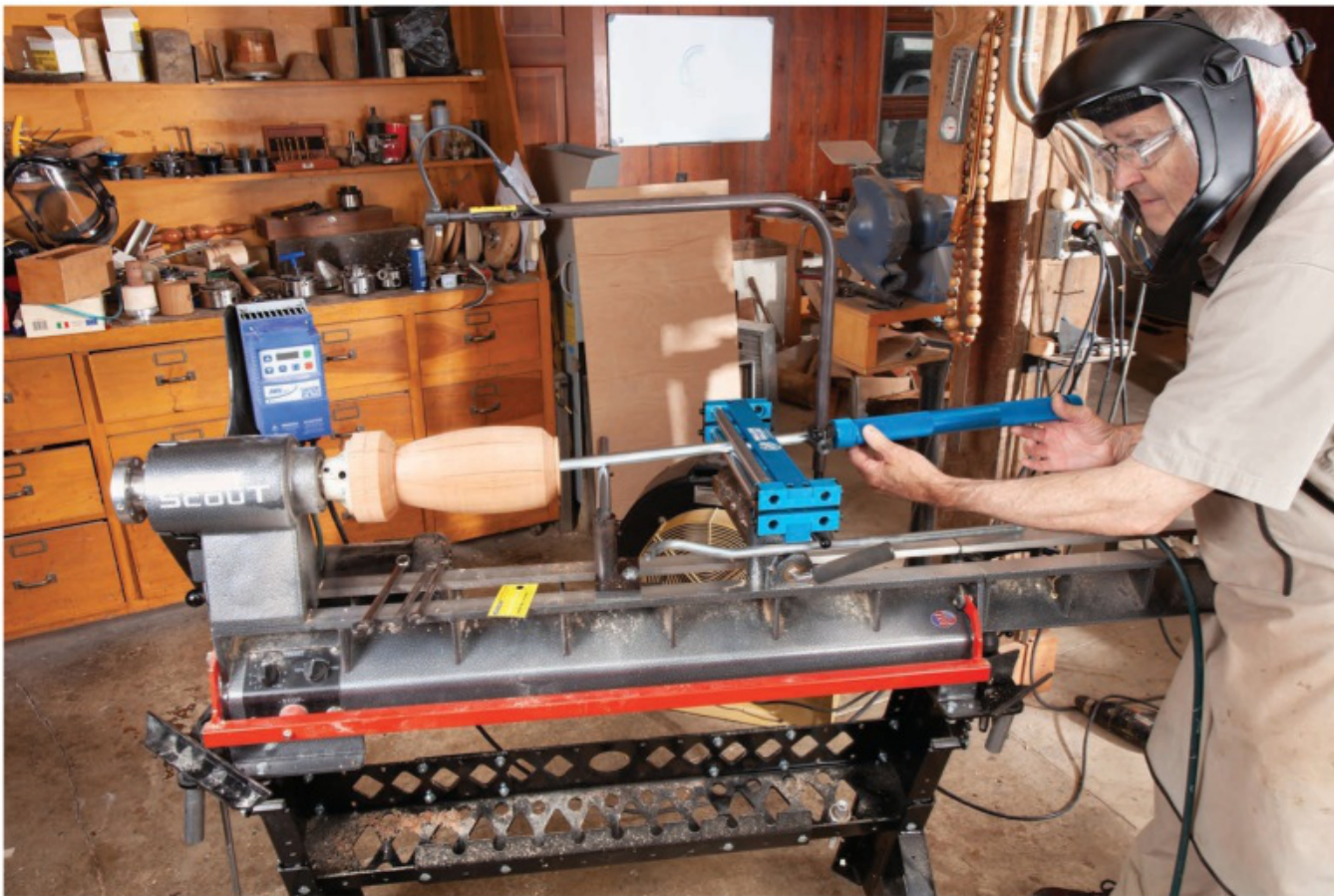
This blue Carter Products Hollow Roller Vessel Turning System is mounted to a Robust Scout benchtop lathe.
