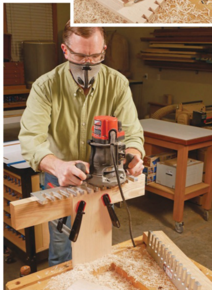
All it takes are a pair of aluminum or phenolic templates, piloted dovetail and straight bits and two backup boards (inset) to mill through dovetails using a Keller & Company dovetail jig system.
