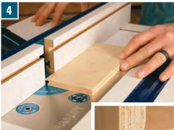
4 Reset the bit's projection using the other end of the setup block to cut a deeper profile into the ends of the drawer backs. Make test cuts and adjust the bit accordingly. The drawer back fits correctly when its thin outer tongue overlaps the end of the drawer side (inset).
