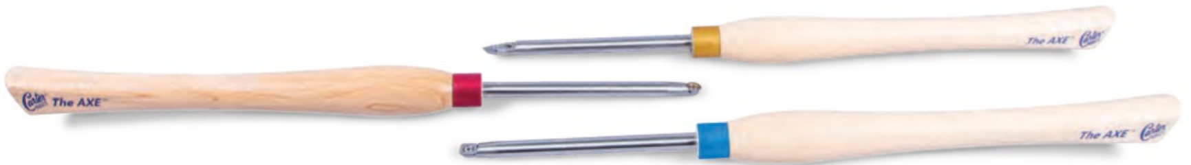
Carter Products Axe boring bars have flat-sided handles — similar to an axe — to help provide a more secure, comfortable grip. Their shafts accept replaceable carbide inserts.
