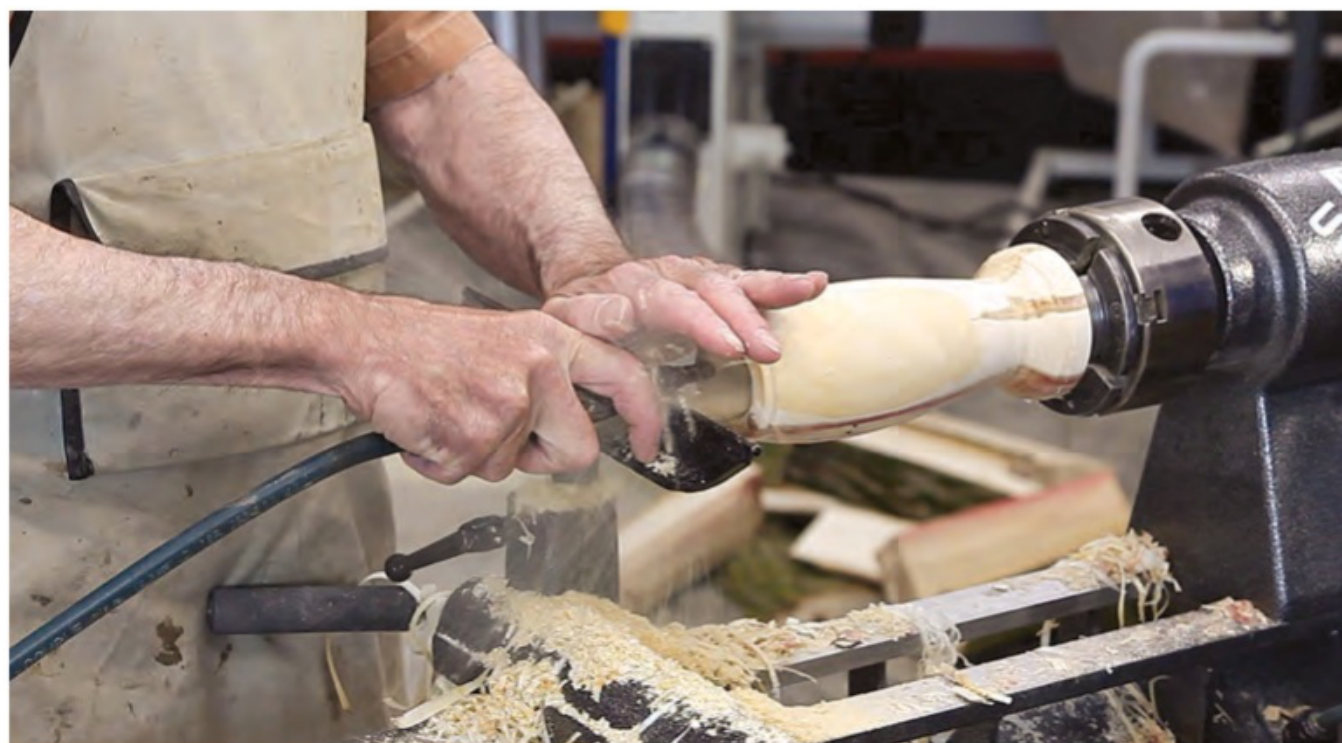
A blow nozzle with a cross hole is a safe way to clear accumulated swarf from inside a hollow form.
