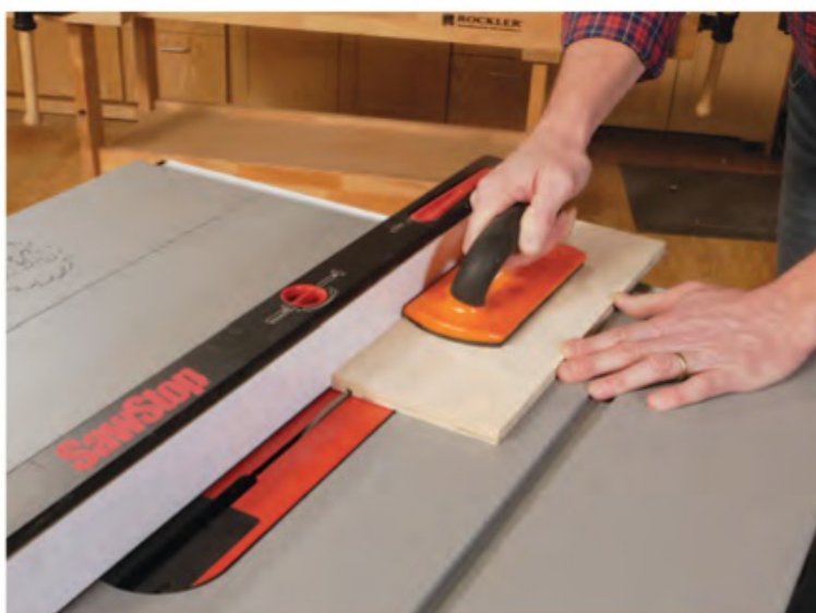
Cut a 1/4"-deep groove along the inside face of the drawer sides, front and back, to house the drawer bottom. Size the width of these grooves to match the bottom panel's thickness.
