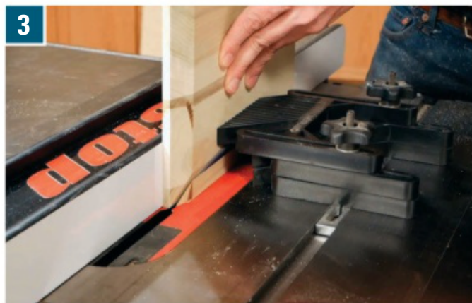
3 With the saw blade tilted 20 degrees off of vertical, bevel-cut the door panel's ends and edges to create its field area. Use a tall featherboard to support these cuts.
