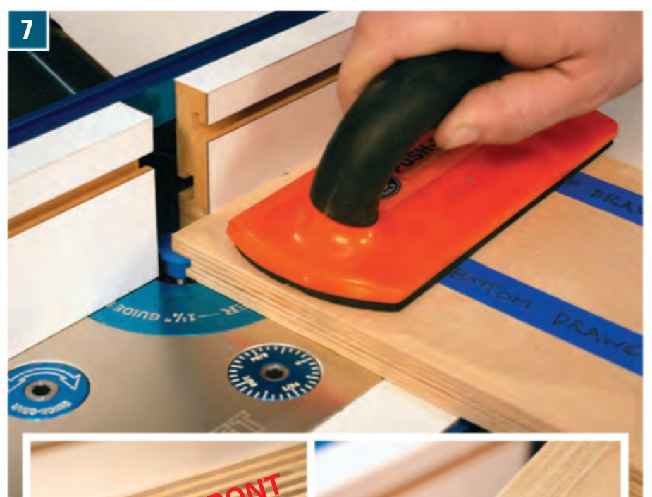
5 Rout the drawer lock profile across both ends of the back panel — the face against the router table will become the inside back face of each drawer. We made these cuts into a double-wide blank of 1/2" plywood to improve stability during routing and to help speed up the process. Once the joints are cut, you can rip the panel to form both drawer backs.
