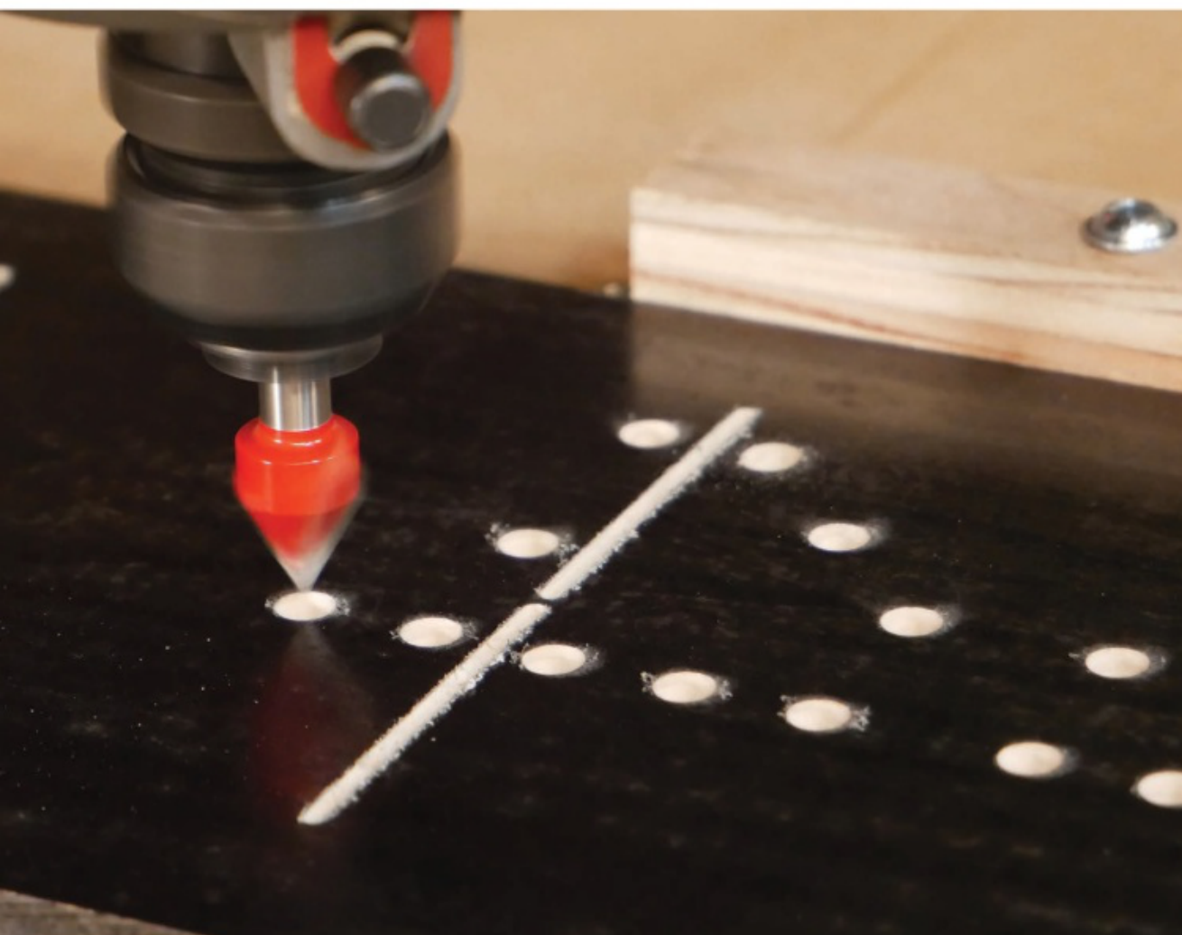
There are two engraving programs required to make a complete set of 28 dominoes. The dot patterns will be different from each other. A CNC router makes quick work of drilling the many holes.
