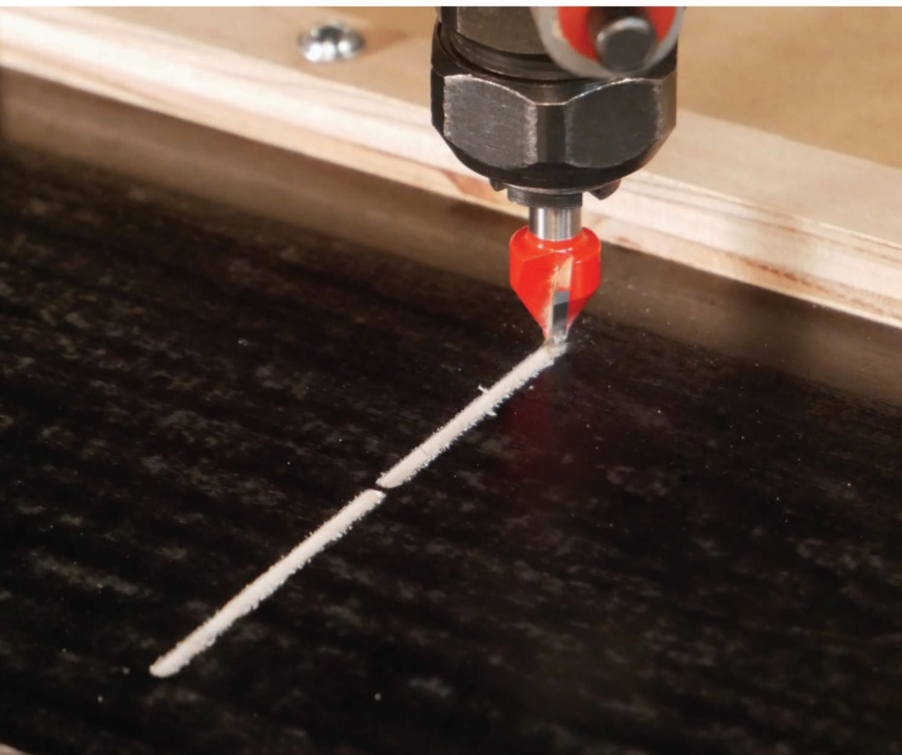
Using a V-bit, the divider lines are engraved into the surface of the domino stock. Here, the maple stock is painted black so that the routed lines are easily seen. The paint is non-toxic when cured.
