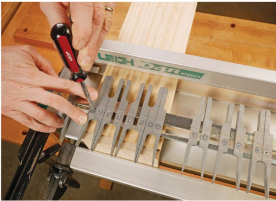
Adjustable-template dovetail jigs feature pairs of metal fingers that create tail cuts on one end and pin cuts on the other. You can alter their spacing and pattern by loosening set screws and sliding them left or right.
