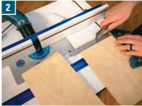
2 To prevent chipping the plywood veneer on the faces of the drawer side workpieces during routing, score them 3/8" in from both ends of one face with a sharp knife or razor blade several times before routing.
