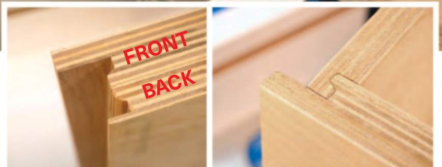
7 The drawer face blank receives a deeper profile cut that forms a long tongue to overlap the drawer sides and drawer slides (right inset). Make shallow passes, resetting the fence further from the bit to lengthen this tongue. Continue routing until the length of the inside face of the drawer front matches the inside face of the drawer back (left inset).
