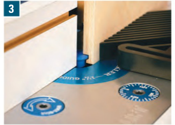
3 After making test cuts on scrap, rout the drawer lock profile into the drawer side blanks with the panels oriented vertically against the fence. Install a featherboard on the router table to keep the panels pressed firmly against the fence.
