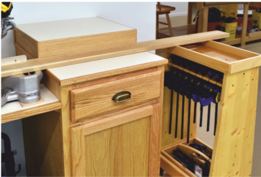
Always support the ends of long stock. The author's clamp/tool caddy, designed to be the same height as his miter saw's table, does double duty as a workpiece support.
