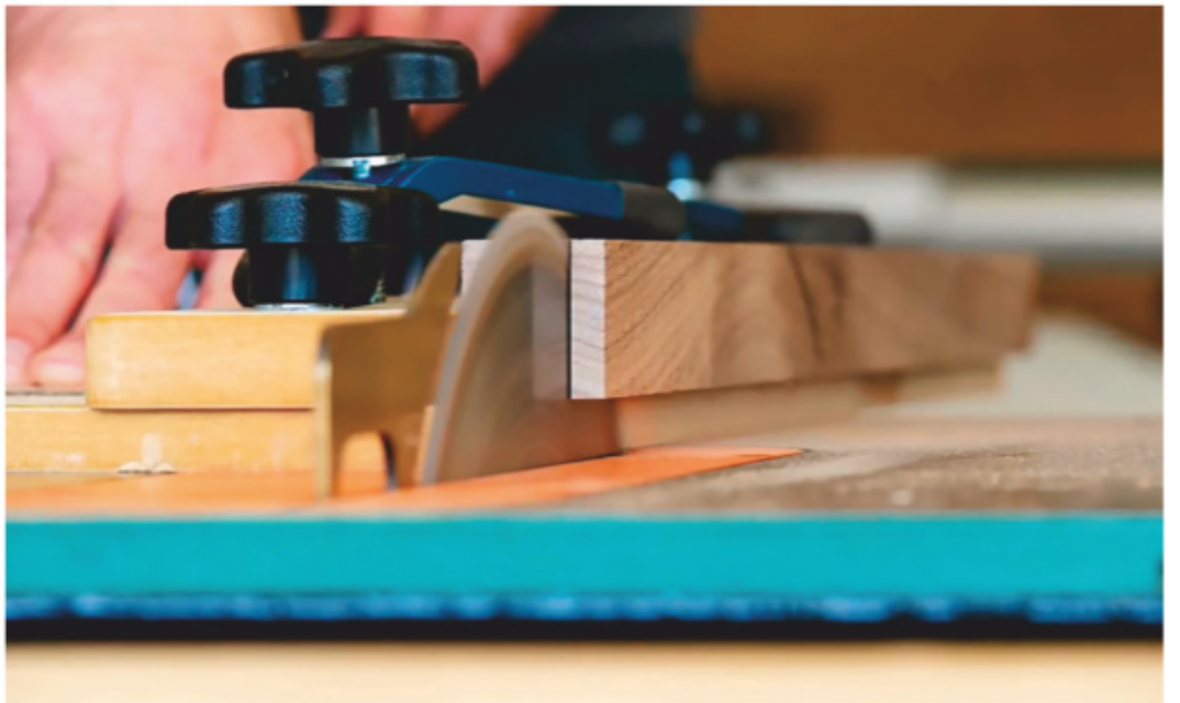
The tapers on the inside edges of the legs are started by marking the leg blanks at the top and bottom, then connecting the marks. With that done, step to the table saw and set up a tapering jig to accurately slice the angle that forms the taper.
