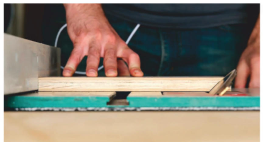
Here the author uses a table saw to machine the 45° angle along the bottom edge of the carcass sides. It also sets the length of the sides.
