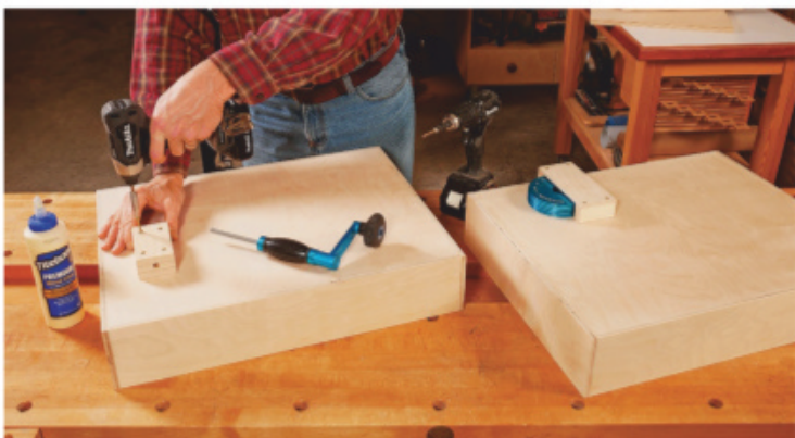
A few parts attached to the bit racks can add storage options for bit insert rings and a router lift adjustment wrench.
