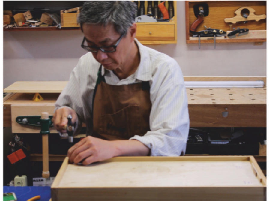
After the finish dries, nail or screw the back panel into place. Notice how the rabbeted depth leaves room for recessing a pair of hanging cleats.
