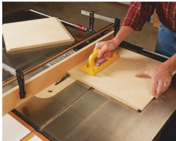
Form 3/4"-wide, 3/8"-deep rabbets along the ends of the cabinet's top and bottom panels with a wide dado blade.
