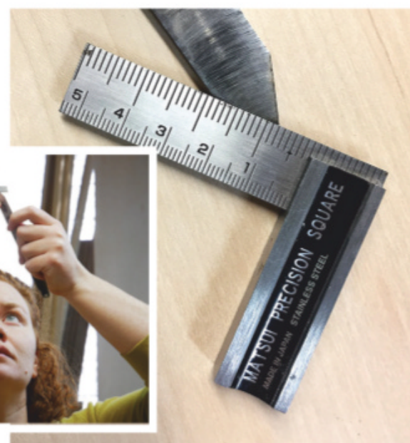
Ensure the flatness of each side of the blade tip using a small square or straightedge.
