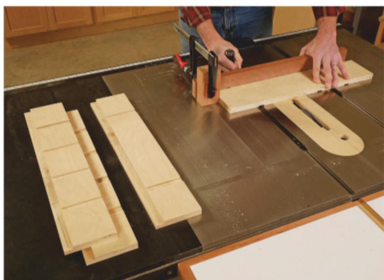
Cut four 1/8"-deep dados across the bit rack sides for storage shelves. Set the dado positions using a clamped stop block.
