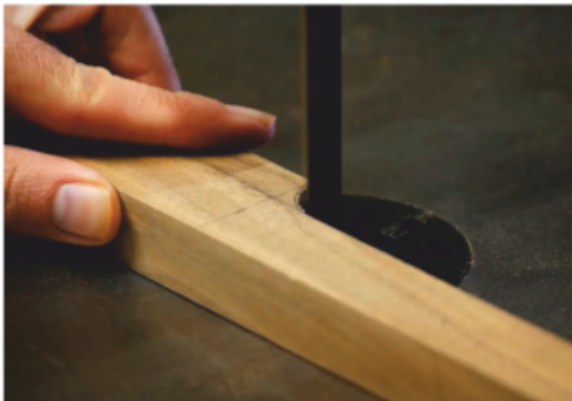
Even a band saw blade that's too wide to cut such tight radii can still do the job if you nibble away the waste and sand the curve smooth.
