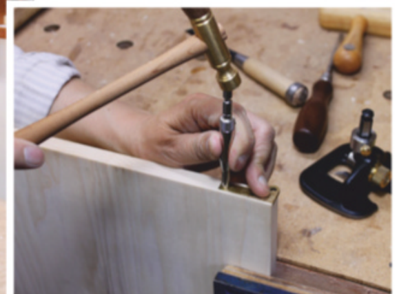
Mark for the hinge screws with a self-centering Vix bit, and drill their pilot holes. The author bores them by hand.
