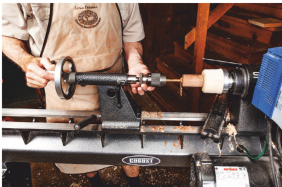
Using a drill mounted in the tailstock quill to drill a piece mounted in a chuck or on a faceplate is the most common lathe drilling task.
