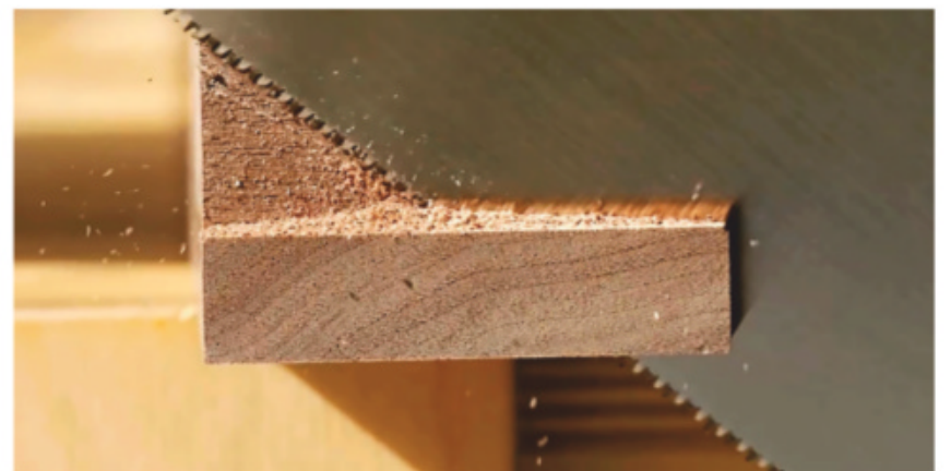
The author used a hand saw to trim the cross braces to match the angle of the legs, then he sanded the joint flush and smooth.
