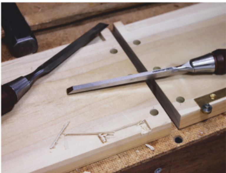
A palm router will get the mortises cut in no time, but careful chisel work keeps one in tune with Krenov's methods.
