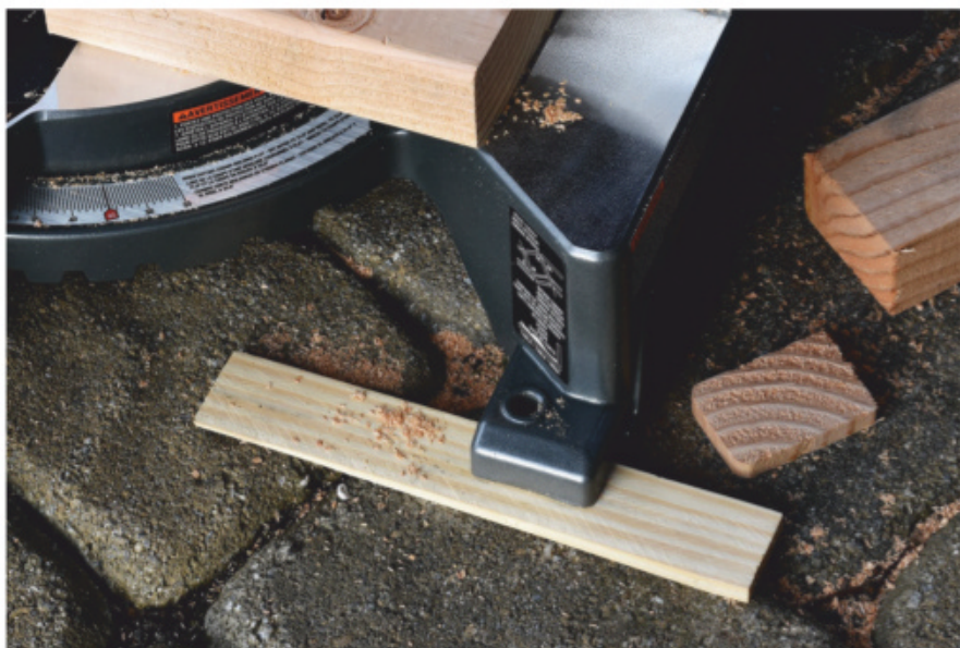
The saw should always sit without wobbling, no matter where you use it — even on the ground. The author keeps a couple of cabinet shims in his pocket to firm up the saw's footing when using it outside the shop.
