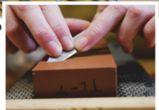
Hone the edge on an extra-fine water- or oilstone until you achieve a mirror polish.
