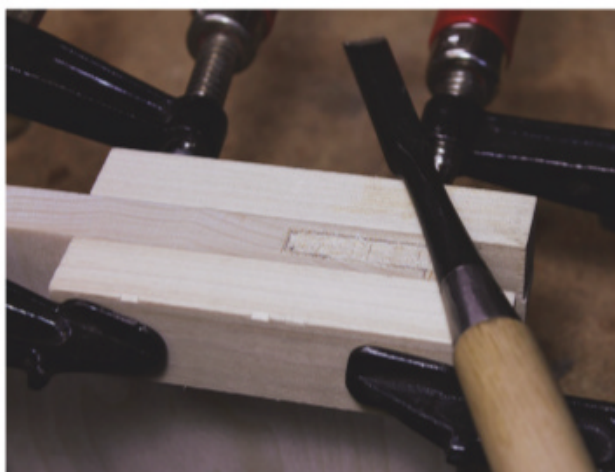
When chopping, always finish the cross-grained end first to avoid splitting the wood.
