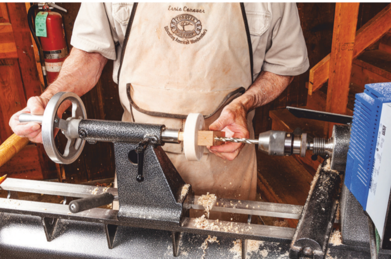
Here, the author is cross drilling a 1"-square blank, using a drill pad. Another option for cross drilling round bars on perfect center, every time, is to make a second pad with a "V" centered in the block.
