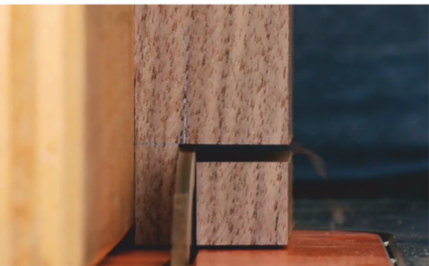
The author used a two-step cut to form rabbets on the ends of the drawer front. The drawer sides are glued and nailed into these rabbets.
