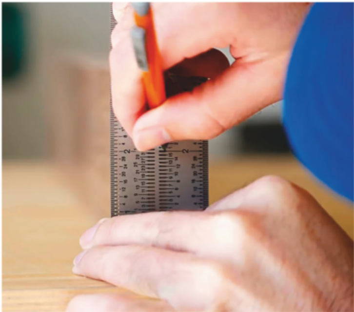
The tapers on the inside edges of the legs are started by marking the leg blanks at the top and bottom, then connecting the marks. With that done, step to the table saw and set up a tapering jig to accurately slice the angle that forms the taper.
