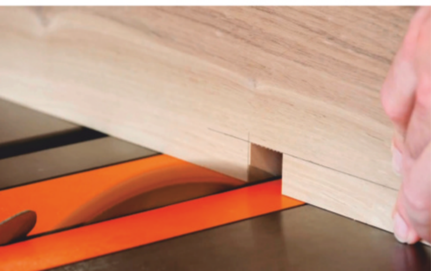
The "drawer pull" is created by removing a hand-sized notch in the top edge of the drawer front. It's an elegant and simple "non-hardware" solution.
