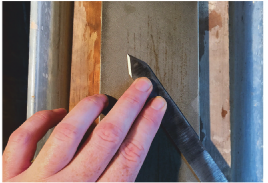
Flatten the back of the blade on a diamond-coated sharpening stone. You want the back of the blade area to display consistent markings.
