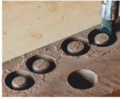
A tapered plug cutter was the tool of choice for making plugs from the offcuts of the project.
