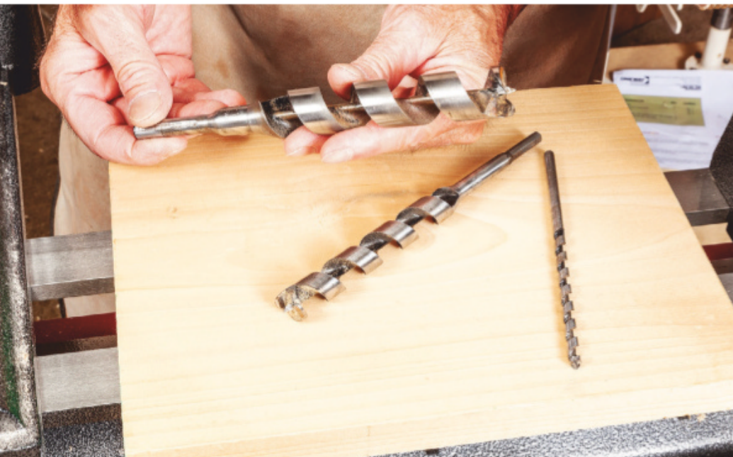
Auger bits tend to be the most expensive type of bit, but they drill deep holes quickly and require less clearing.
