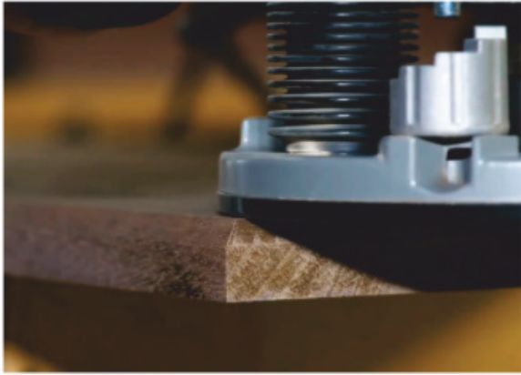
Use a handheld router and a piloted chamfer bit to shape the bottom edge of the carcass top. It adds a nice shadow line.
