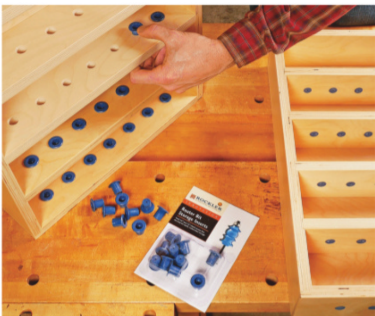
Rockler's new plastic Router Bit Storage Inserts simply press into 5/8"-dia. holes and can hold either 1/4" or 1/2" bit shanks.
