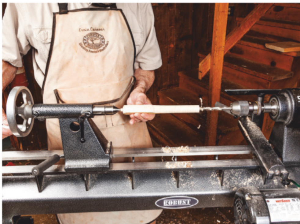
Mounting the drill in the headstock spindle and pushing the part into it with the tailstock ram is the best way to drill this blank for a tool handle on the center axis.
