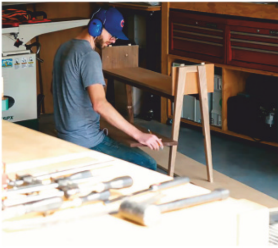
Before gluing the top in place, fit the shelf into the dados that were formed earlier. It is secured with screws hidden by shop-made plugs.
