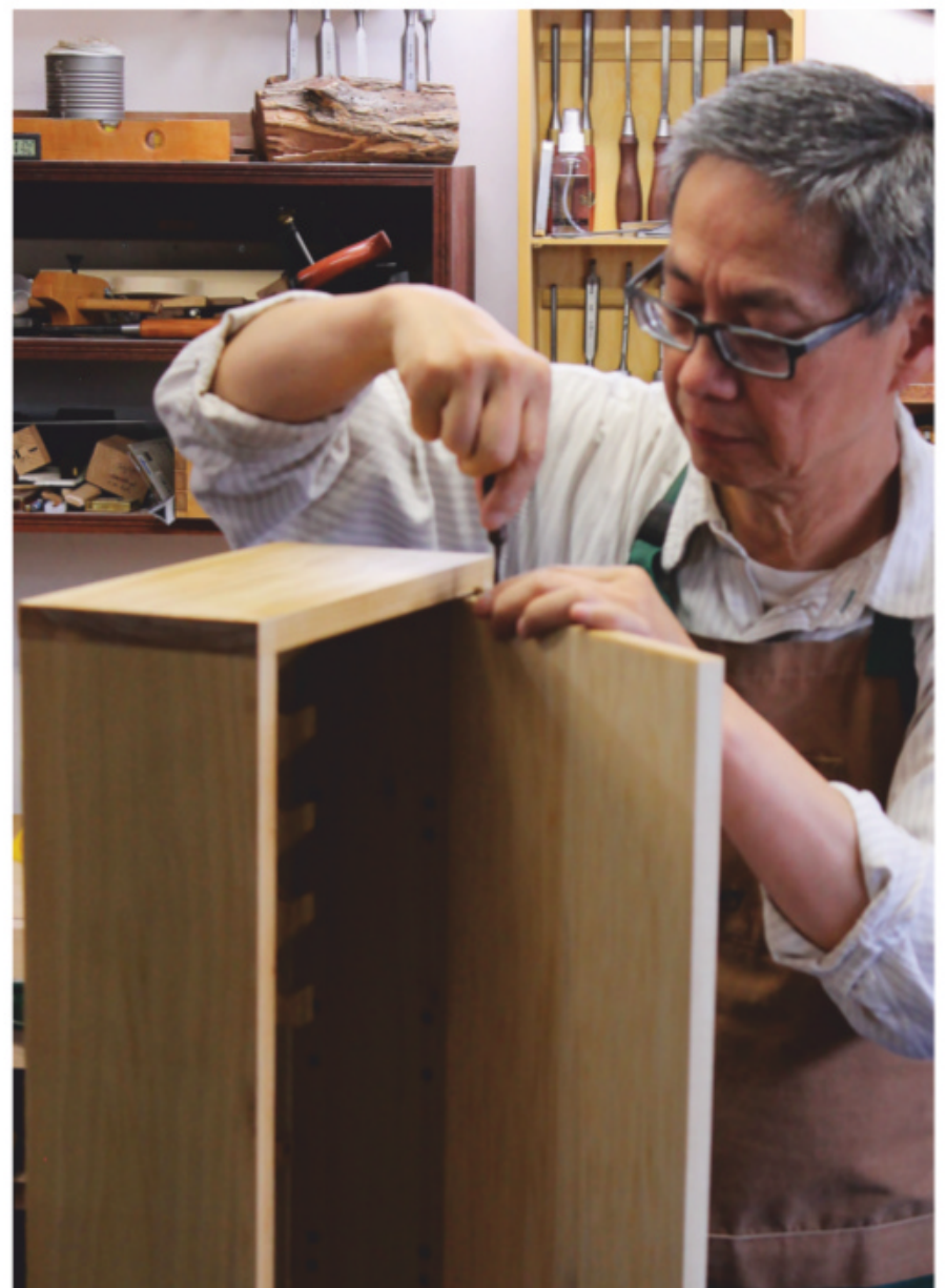
Install the bottom door hinge to the carcass, followed by the top hinge.
