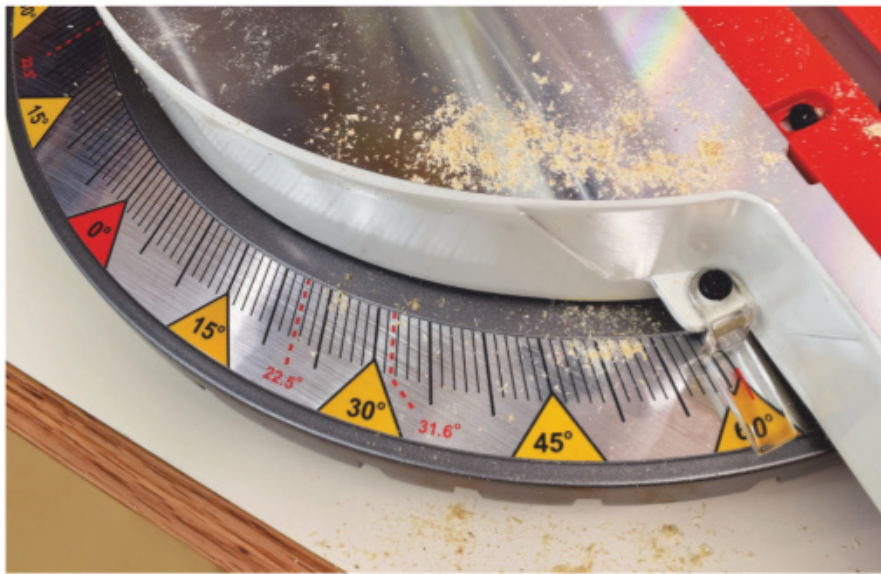
A good miter scale will include easy-to-see markings plus positive stops for the most common cutting angles.
