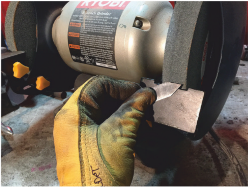
Set the guide on the bench grinder to 25° and remove material in small passes, taking care not to overheat the blade. Cool it often with water.
