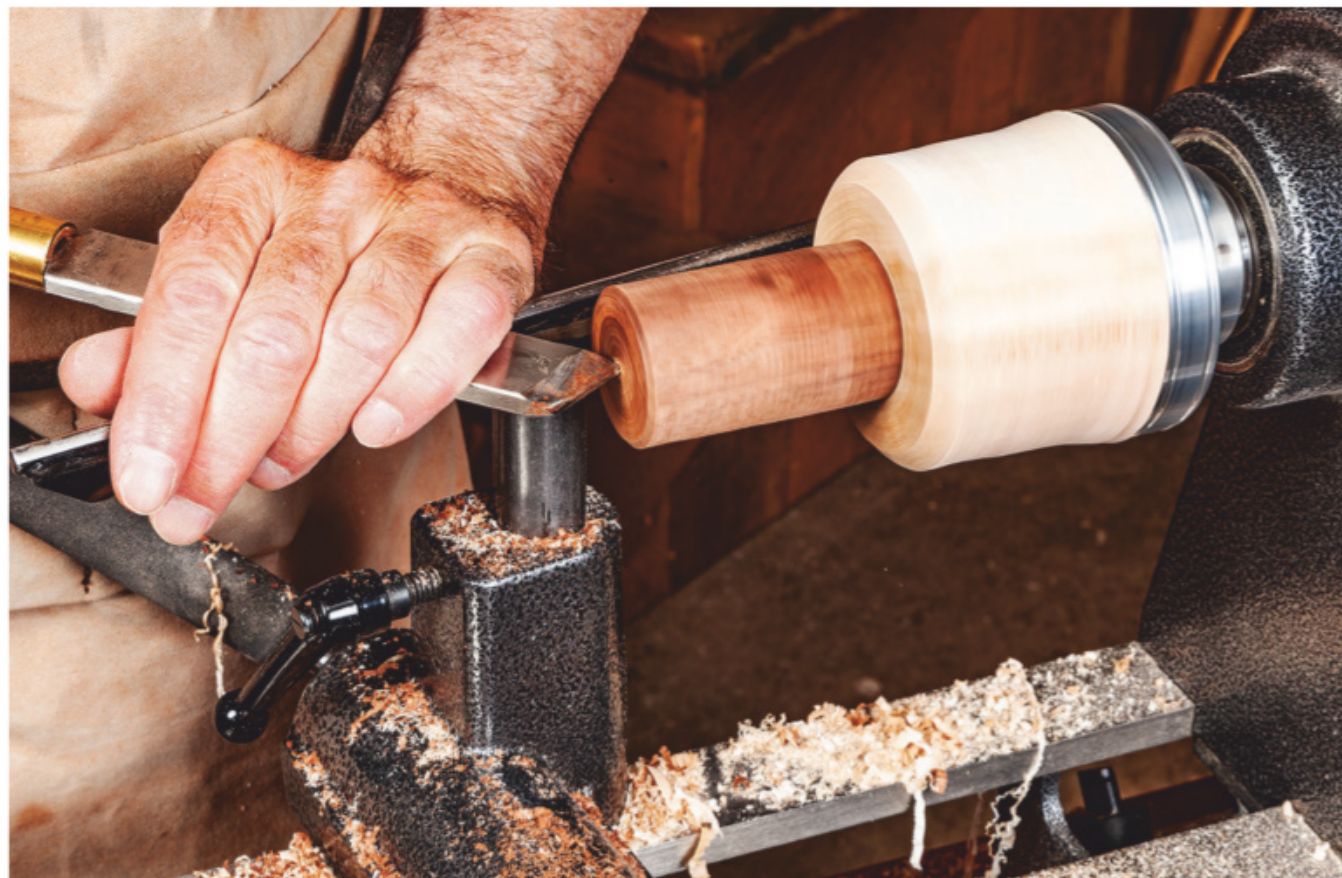
When drilling in a lathe, use a skew to turn a dimple on exact center to ensure the drill has a clean start.
