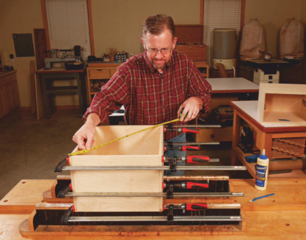
Assemble the drawer components all at once with glue and clamps. Check for matching diagonals to ensure the box is square.
