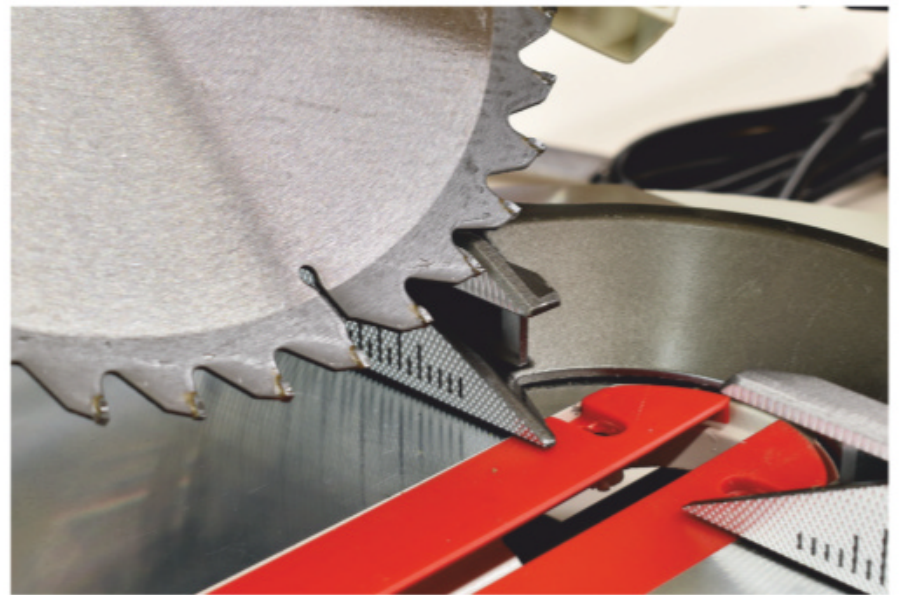
Two-part fences are a wonderful feature on high-end saws, but be sure to pull the movable top portion out of the blade path when making bevel cuts.
