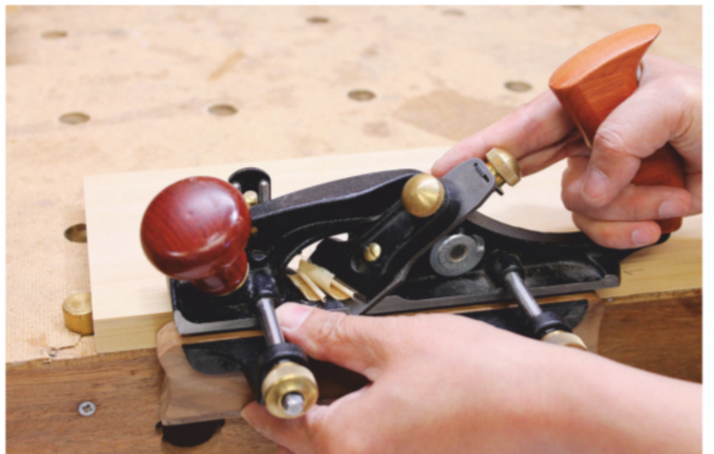
Hold the fence tight to the work and extend your index and middle fingers forward to prevent tilting the plane as you push it.
