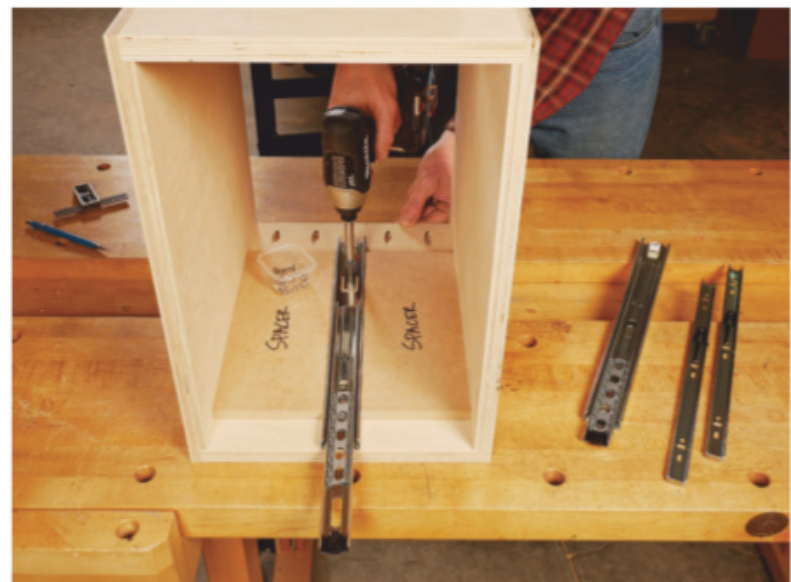
Scrap spacers ensure that the drawer slides are centered and parallel inside the cabinet.
