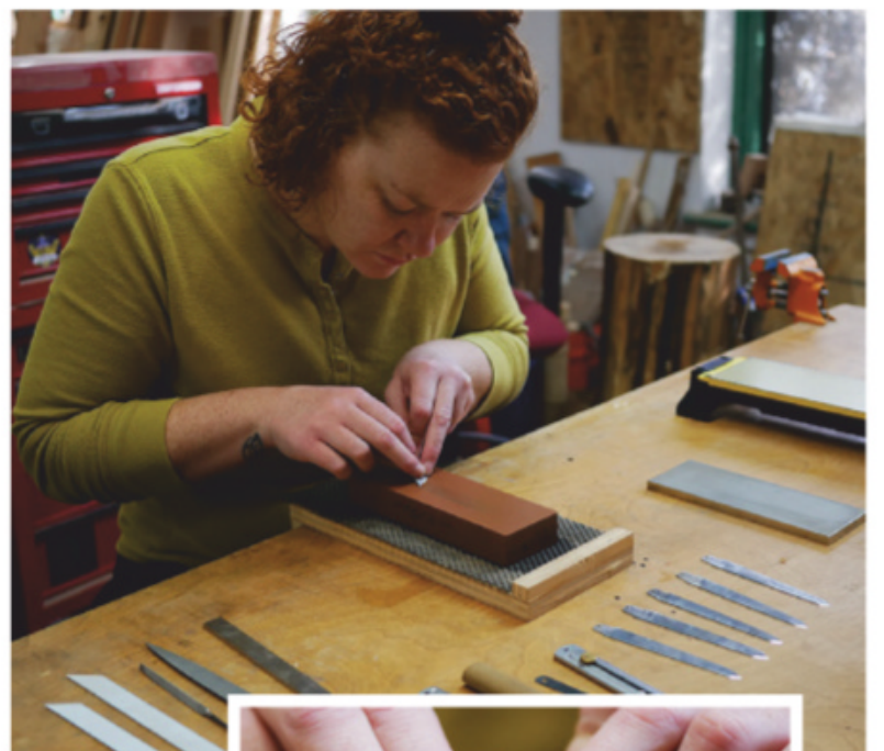
Sharpen each side of the blade’s edge until a burr forms. Start with a diamond stone and work down to an extra-fine water- or oilstone; there should be no burr on the final finish.
