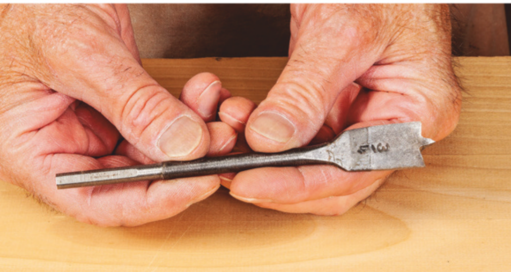
Carbon steel spade bits are available in 1/16" sizing at very reasonable pricing. They are the author's least favorite bit option for lathe drilling.
