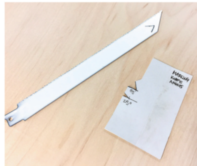
You can trace an existing knife's blade and grind angle onto a cardstock template.
