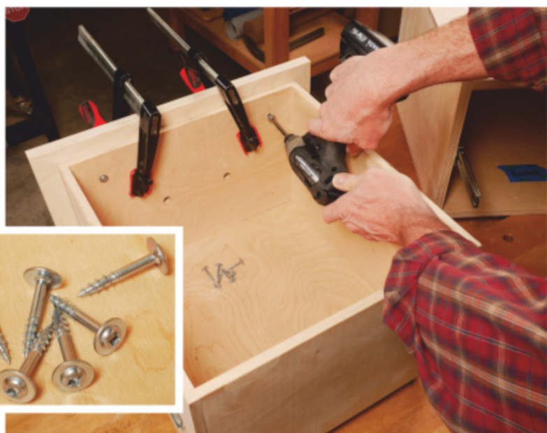
Washerhead screws are designed for installing drawer faces. Driving them through oversized holes allows for final adjustment.
