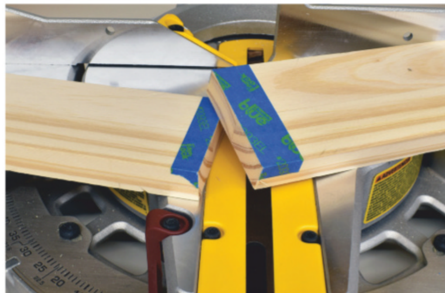
Masking tape on the underside of workpieces helps to prevent tearout.
