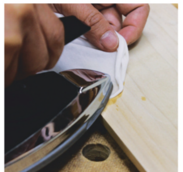
Remove any dents with a clothes iron and wet rag — a step that should be done before final surface planing or sanding.
