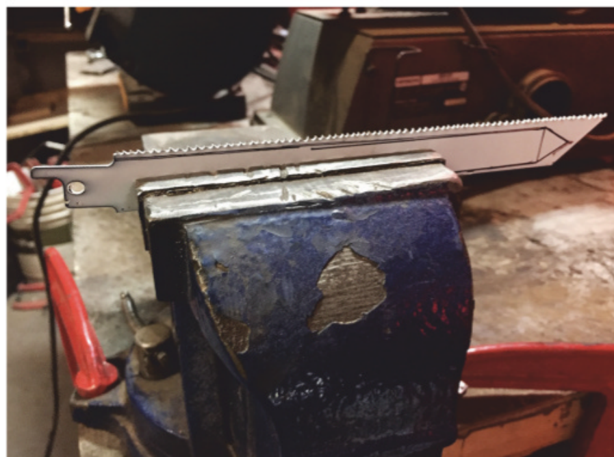
Clamp the saw blade you start with securely into a vise while you are removing the teeth and paint from it.
