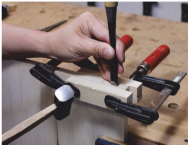
A pair of scrap blocks clamped to the door support the thin mortise walls during chiseling.
