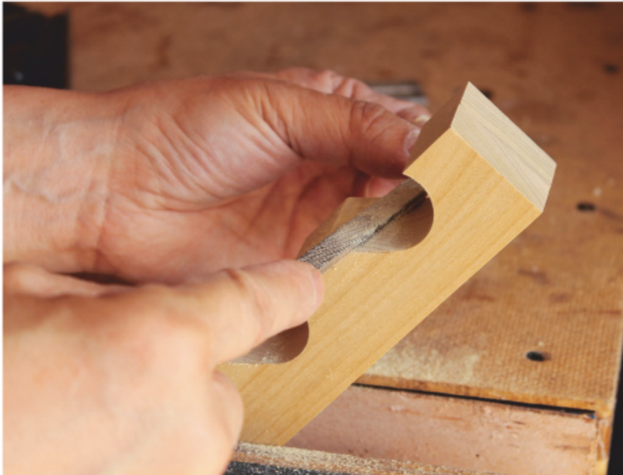
Clamp the spokeshave holders together, and rasp or hand-sand them to a uniform shape. This small detail will give your work a neat look.
