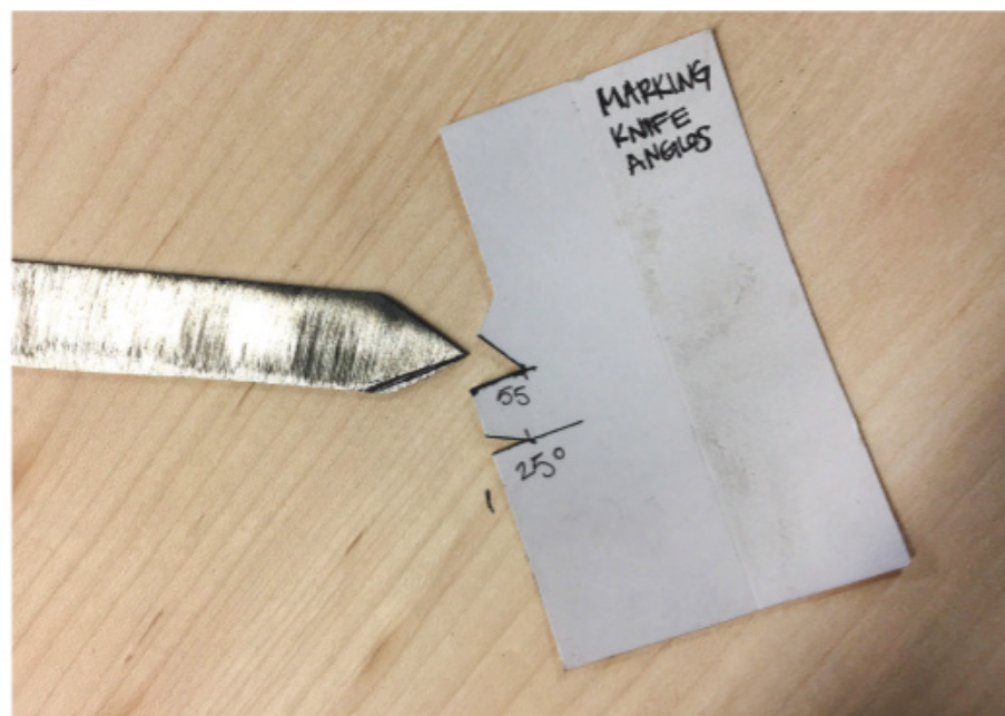
Check the accuracy of the blade angle often against the cardstock template.
