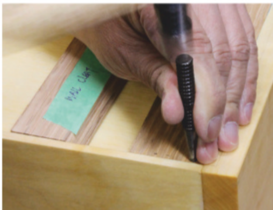
Nail or screw a French cleat to the side rabbets so the cabinet's weight will be supported by the side panels, not the top.
