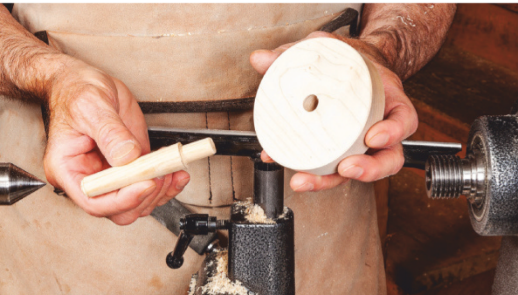
The author chose a durable hardwood (maple or oak are good choices) to build this drill pad by turning a Morse taper with a 1/2" tenon on the end and gluing it into a disk of wood.
