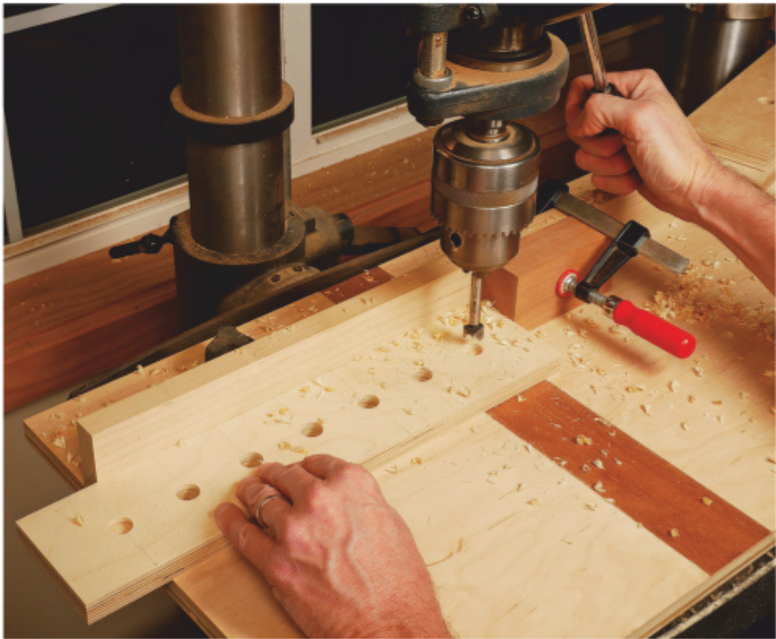
Bore holes for router bit inserts into the shelves. The author recommends a 2" spacing, which allows for seven bits per shelf.
