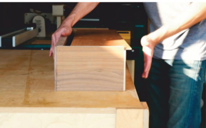
The drawer bottom slides into the grooves prepared for it. Then nail the drawer bottom to the bottom edge of the drawer back with pin nails to secure it.
