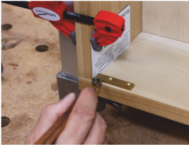
Set and scribe the carcass hinge slightly away (1/32" here) from the hinge side wall. A plastic gift card makes a handy spacer.
