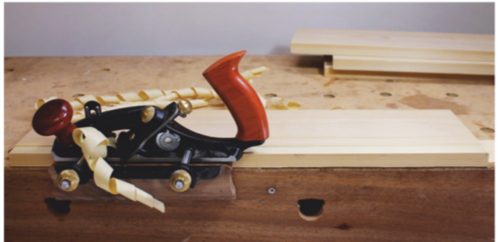
Begin at the far end with short forward strokes, extending them progressively until eventually you are making full-length strokes along the edge.
