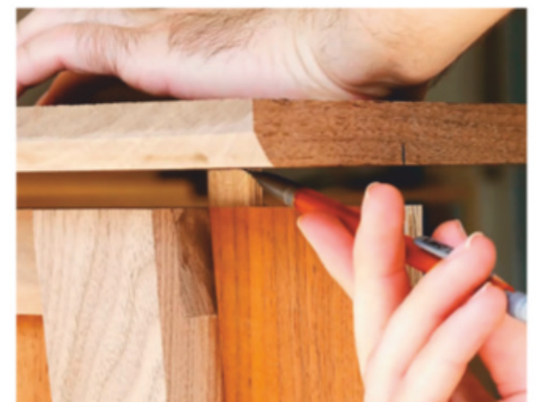
You can attach the top to the carcass with Domino joints. Dowels are another perfectly suitable way to join the top to the project.
