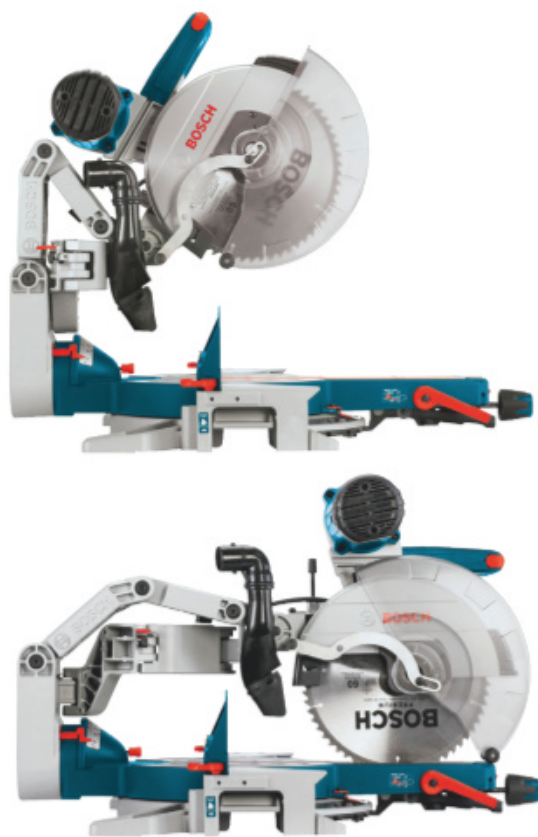
Instead of rails, Bosch's Model GCM12SD 12" dual-bevel "axial-glide" miter saw uses cantilevered arms that allow the cutterhead to move through a full range of motion when cutting.
