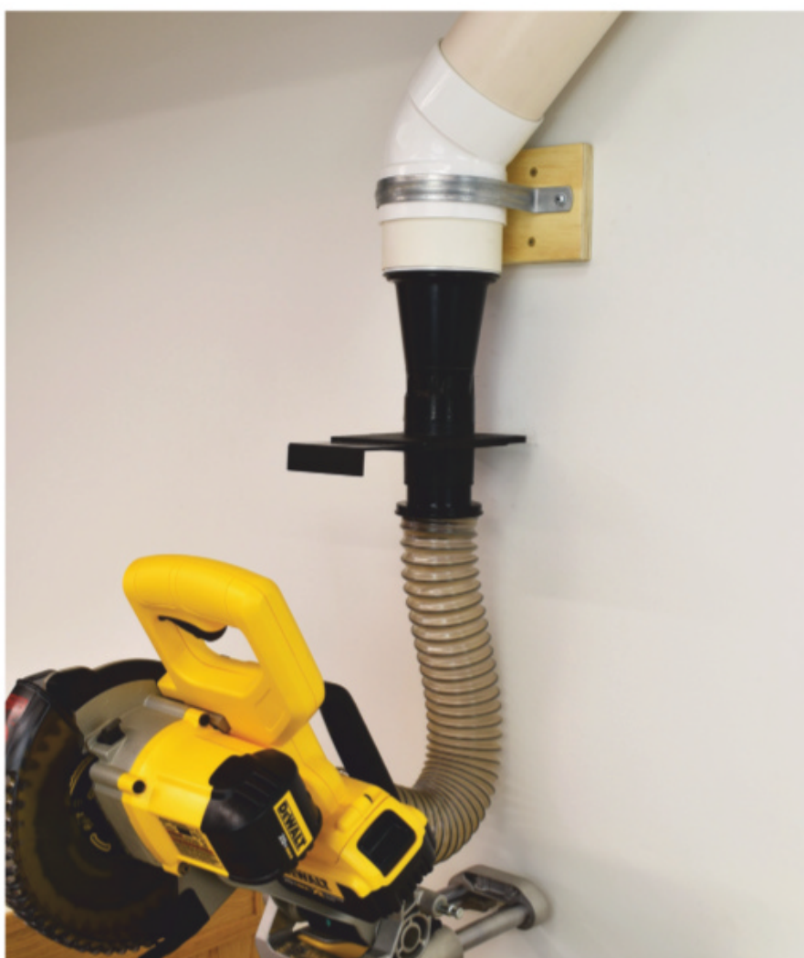
Miter saw dust is difficult to catch, but a dedicated collection hookup maximizes the amount of dust and debris kept out of the air and off your work area.
