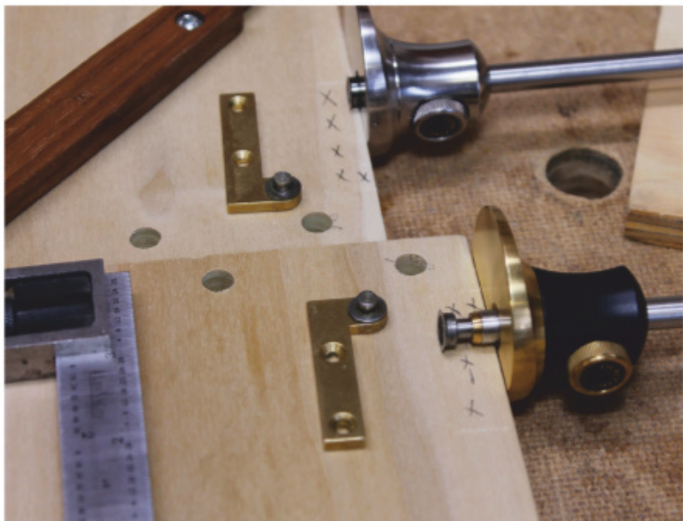
The marking gauges, previously set for the door hinge leaf, are re-used to mark the mortises on the carcass.
