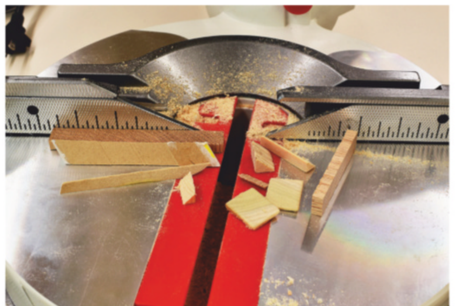
Cutoffs small enough to fall through the throat plate opening will quickly build up in there. Clean it out regularly so the blade doesn't send these small pieces flying.
