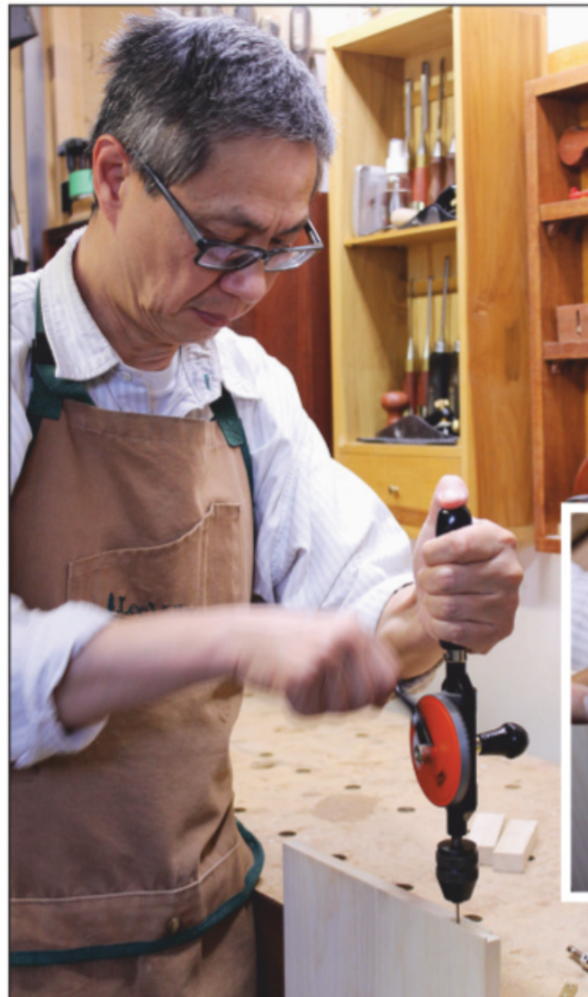
Mark for the hinge screws with a self-centering Vix bit, and drill their pilot holes. The author bores them by hand.
