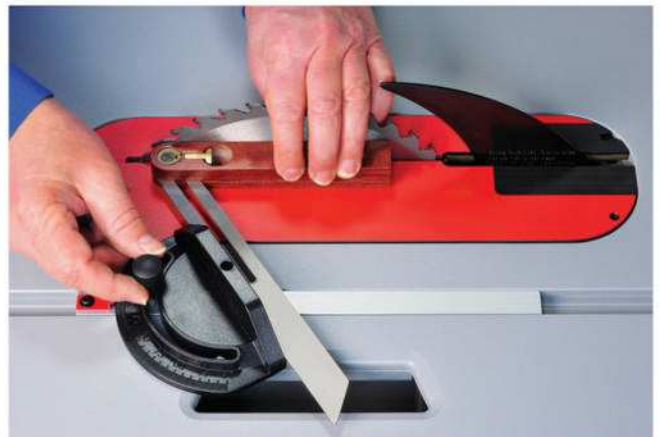
The author uses a sliding bevel gauge that's been set to the desired miter angle to adjust the angle of the head of a miter gauge relative to the saw blade.
