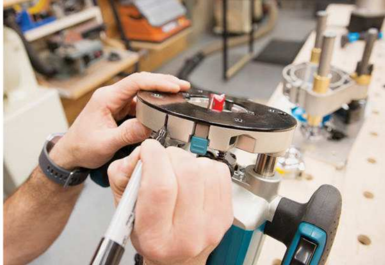
Drawing a witness mark on the router base can help ensure that the offset distance between the bit and the edge of the base remains the same during routing. Unless the base is perfectly centered, this distance can vary.
