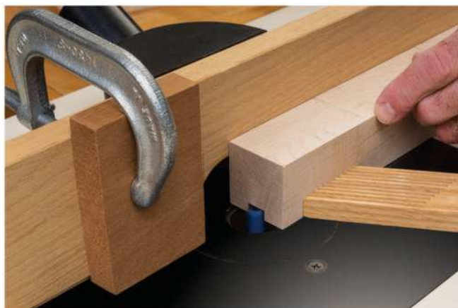
Rout the stopped grooves in the stiles on a router table fitted with a 1/2" straight bit. A stop clamped to the fence prevents cutting too far, and a featherboard keeps the workpiece traveling against the fence.
