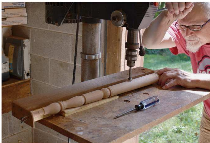
Before locking the post's rotation, sight the post to see that the bit's lead point will enter the mortise halfway across the post's diameter. Then, move jig and post side to side for proper alignment.
