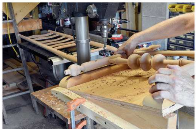
Reversing the jig's position allows you to drill the side-rung mortises in the front ladder. The 2 x 4s are necessary here so that the turned ornamentation in the front stretcher clears the jig's deck.
