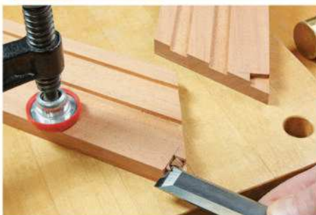
Miter cut the ends of the sides to 30°. A crosscut sled with a hold-down clamp handles these short pieces safely. Chisel the top grooves square.
