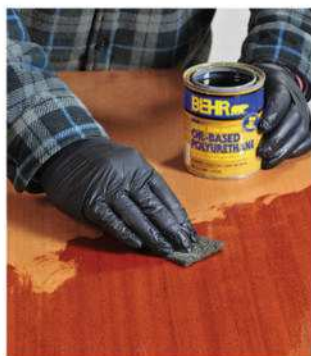
Scrub unreduced polyurethane varnish liberally onto the wood with a fine nylon abrasive pad, then wipe off the excess.
