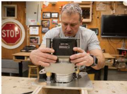
Rockler's Pro Lift accepts full-size router motors as well as smaller diameter models when retro-fitted with accessory adapter collars.
