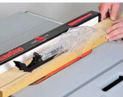
A table saw's blade guard, splitter and/or riving knife and anti-kick-back pawls all serve to protect the user from harm during cutting.
