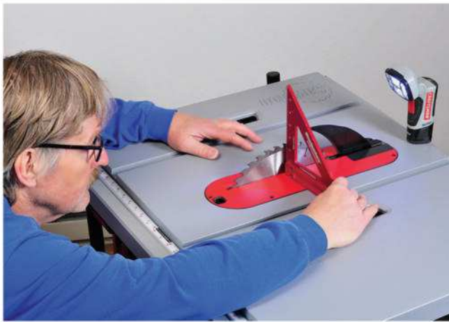
When adjusting a table saw blade for a square cut, the author uses a flashlight to shine light on the gap between a handheld speed square and the saw blade itself.
