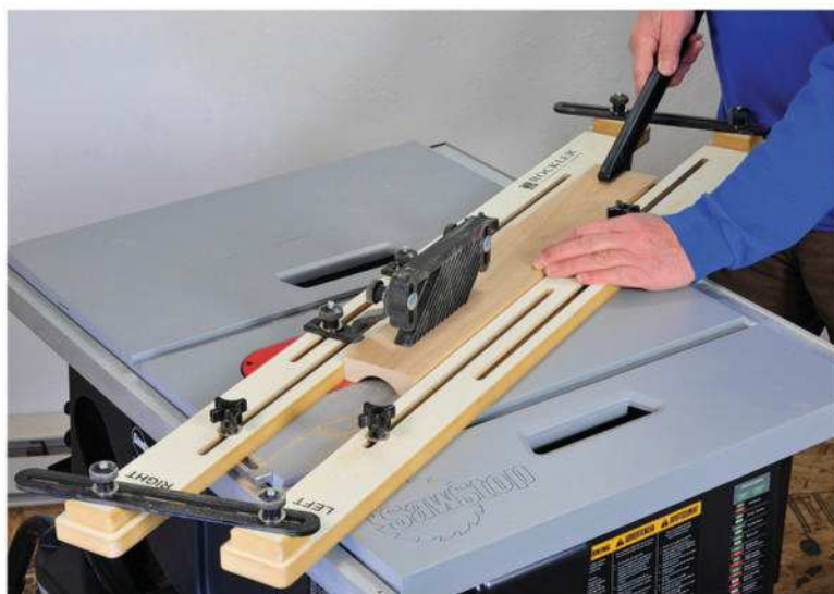
Using a special fence jig, stock is run at an angle over the top of the blade, thus cutting an arc-shaped hollow cove in a series of shallow passes.
