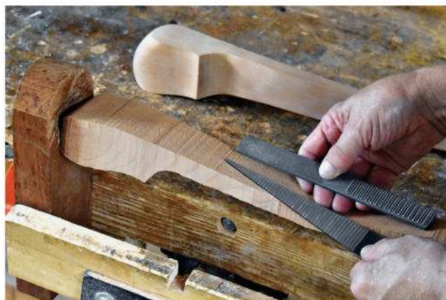
The tool in the author's left hand is a planemaker's float, for the clean, quick removal of wood. In his other hand is a sharp four-in-one rasp.
