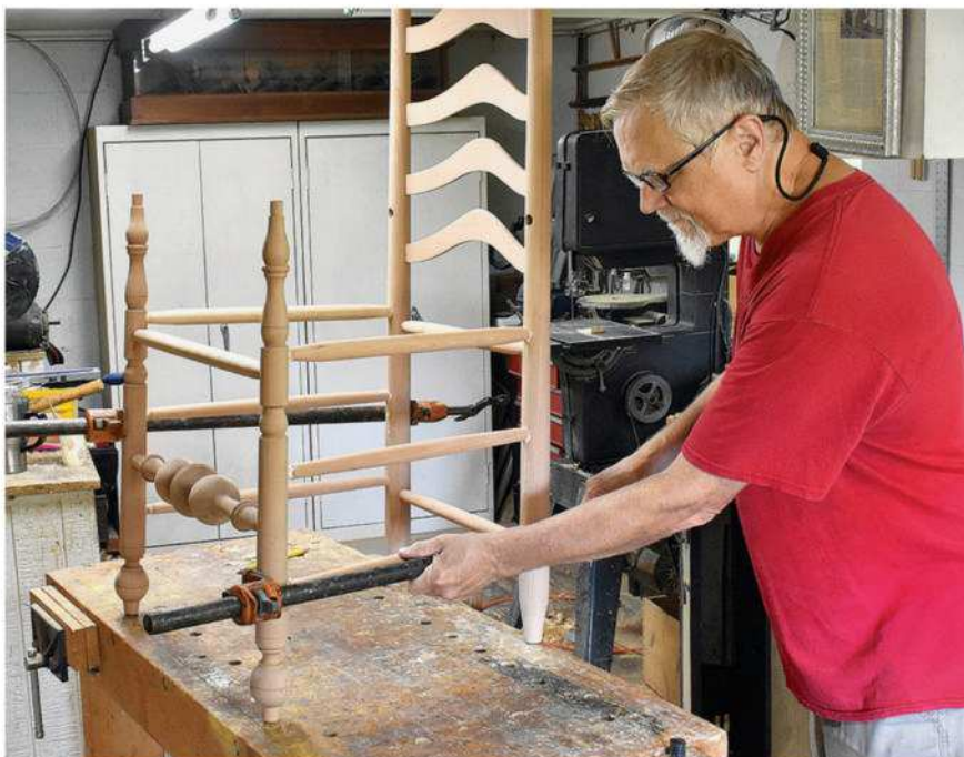
Once the side-rung mortises have been drilled, assembling the chair frame is simple. Chairmaking is a bit complicated, but with a good plan and careful marking, it is eminently achievable.
