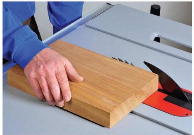
For safety's sake, always adjust the height of a table saw blade so that the saw teeth only protrude about 1/4" above the thickness of the stock being ripped or crosscut.
