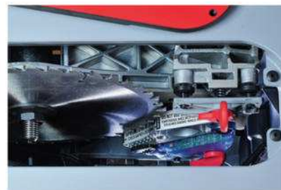
The SawStop mechanism is a protective device built into SawStop brand table saws.
