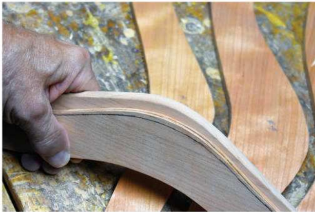
In the pair of slats held here, the rear slat has been radiussed. The front slat has not, but it does have radius guidelines sketched in. The radii on these slats disappear at the ends, where they will later enter the posts.
