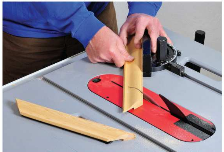
A standard miter gauge fitted in a table saw's miter slot is just right for cutting mitered corners on moldings used for small picture and mirror frames.
