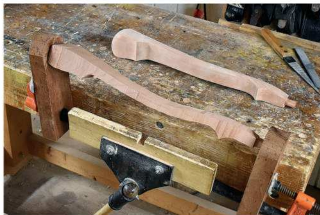
When shaping the arm blank, the author secures it between a pair of puppets mounted on a pipe clamp, which is mounted in a vise.
