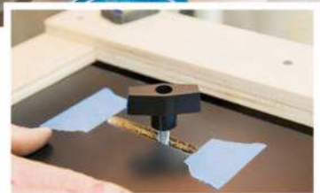
A pair of elongated slots cut through the table on either side of the router lift provide for through bolts and knobs to attach a router table fence. This way, the fence can slide back and forth.
