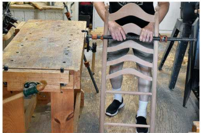
Clamp one back post to your bench, mortises up. Insert all rungs and slats, followed by tapping the other post into place. Then squeeze together the pipe clamp and slat so that tenons pop into their mortises.
