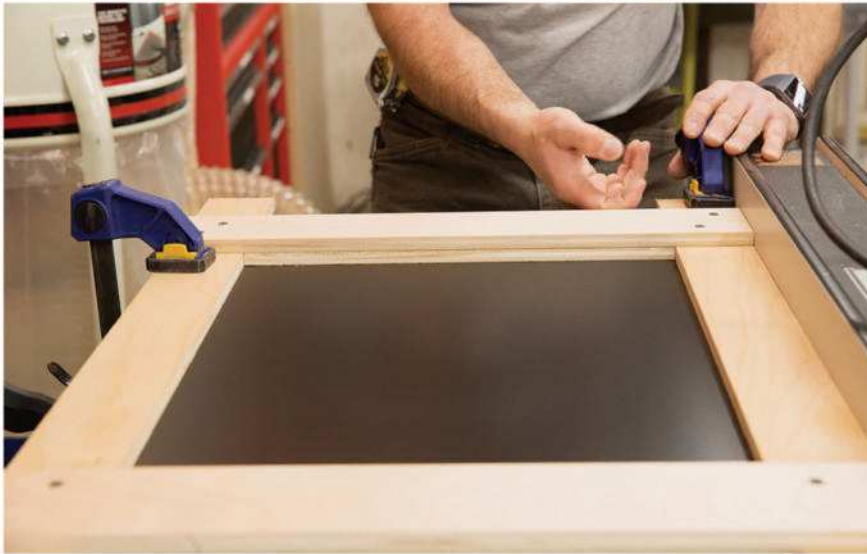
A pair of overlapping strips and screws secure the four 1/2"-thick plywood pieces of the template at its corners. It's crucial that this template is made accurately, because the router base registers off of it directly when cutting the router plate opening.
