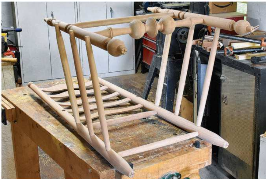
Years ago, when working with an early side-rung mortise jig, the author discovered that the angle of the jig's deck was incorrect. He then discovered that chair frames assembled with this error stayed together even without glue, and he has incorporated that error into his process ever since.
