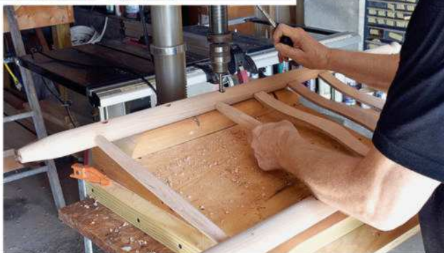
With the jig in this position (high side closest to the drill-press post), drill side-rung mortises into the back posts. The two short lengths of 2 x 4s screwed to the jig raise the posts so the back slats clear the jig's deck.
