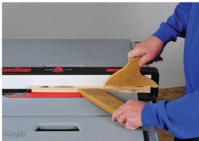
When cutting small or narrow workpieces, use a push stick to feed the stock forward and a featherboard to help it bear against the rip fence.
