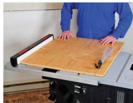
Small- and medium-sized pieces of plywood and other sheet goods are easy to cut, even on compact jobsite table saws, using the saw's standard rip fence.
