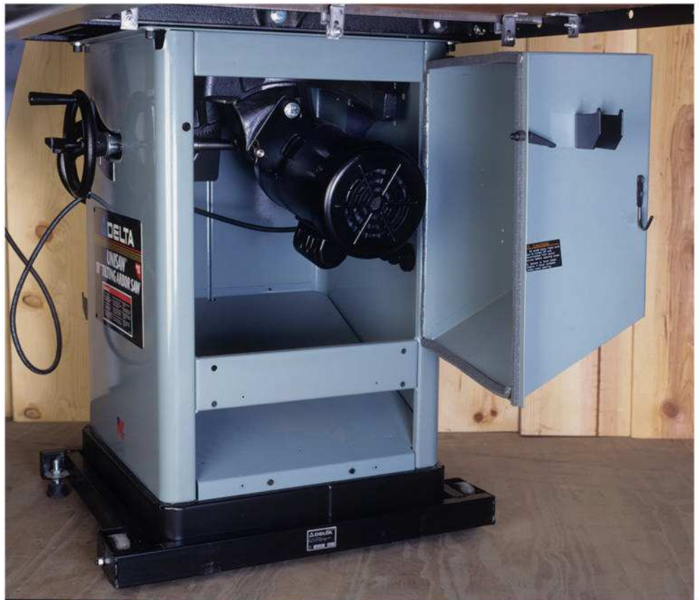
All of a cabinet saw's heavy-duty components — motor, belts and pulleys, saw arbor and trunnions (that allow the arbor to tilt) — are housed inside a sheet-metal base that also supports the saw table.
