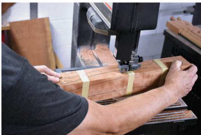
With the offcuts reattached to the blank using masking tape, rotate the arm 90° and saw the blank in the adjacent plane.
