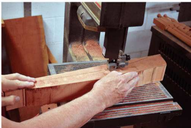
Cut out the arm pattern on one side of the blank, taking care to save the offcuts — you will need to reattach them to complete the arm.
