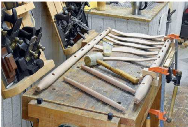
It's essential to have all your materials prepped before beginning the back ladder glue-up. In fact, if you're a chairmaking first-timer, you might want to enlist an extra set of hands.
