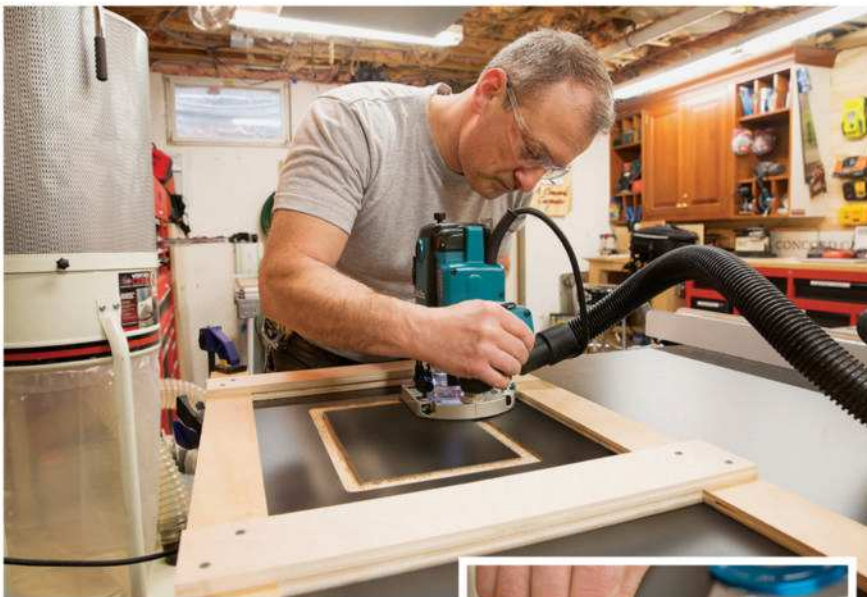
A 3/4"-dia. straight bit enabled the author to match the corner radii of his router lift plate. With the cutting depth set to match the thickness of the plate, he routed down in clockwise passes. Then, adding 1/2" spacers to the template, he reset the router for removing the center cutout and forming a rabbeted ledge. A scrap straightedge helped check for a flush fit (inset).
