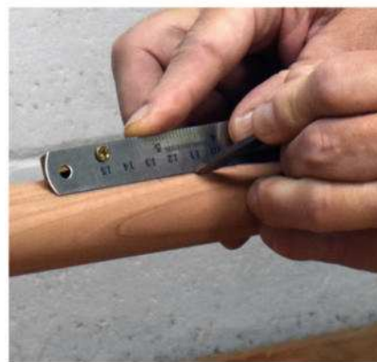
This little jig makes it easier to hold a straight-edge in a consistent alignment when scoring the limits of the slat mortises with a marking knife.
