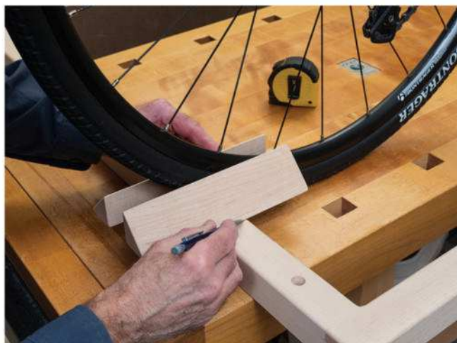
Use your bike's tire to establish the distance between wheel braces, then mark the braces' position on the frame or the brace platform and measure the gap.
