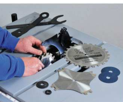
Dado blades are used to cut grooves, dadoes and other joinery. The width of cut is determined by the number of chipper blades and shims set between a pair of outer saw blades.
