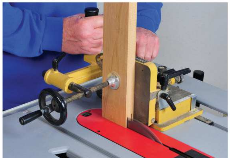
Cutting tenons on frame members used for mortise-and-tenon joinery is done with a dedicated jig that firmly supports the stock as it slides past the saw blade.
