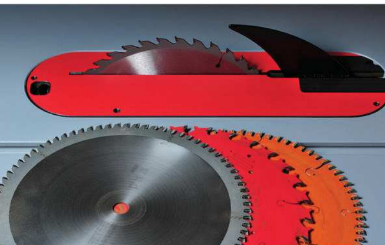
General-purpose carbide-tipped saw blades (rear) are great for everyday use, but for specialized tasks, choose special blades: (left to right) cross-cut, rip and melamine/plywood.
