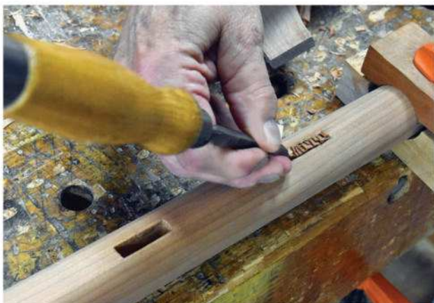
At left, the author chops out the slat mortises with a mortise chisel. In the photo above, notice that the slat mortise angle allows the two ends of the bent slat to mate with the two back posts (one present, one not). The relationship between the slat mortise angle and rung mortise angle is critical if the back ladder is to come together properly.
