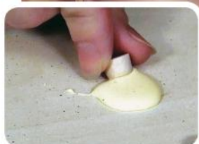
Glue wooden plugs into the counterbores to hide the screws, and sand flush when dry.
