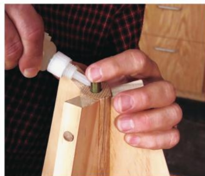
Slip the threaded rod into the hole in the leg connector, leaving enough of it exposed to attach the socket base, then glue it into place.
