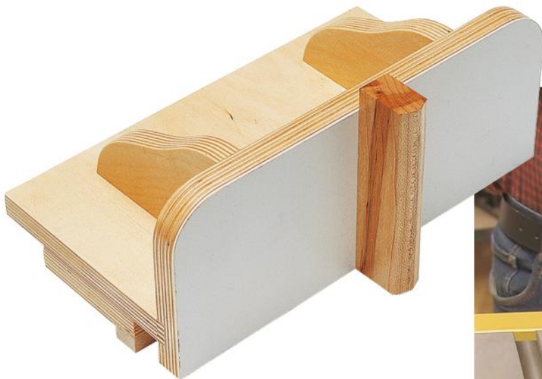
A point fence, like the adjustable shop-made version above, is the key to being able to adjust for blade drift as you resaw.
