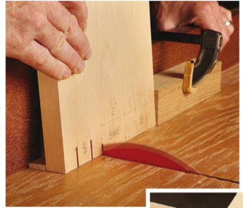
With the box joints carefully marked out, remove the waste from the seat and back. Note the spacer behind the cherry stock: it helps keep the piece tipped back properly at the 5° angle during cutting.
