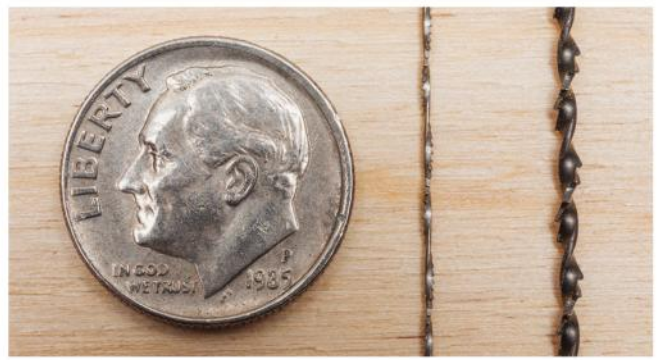
It requires considerable practice to use spiral blades like these, but they are invaluable when working on projects with limited access.
