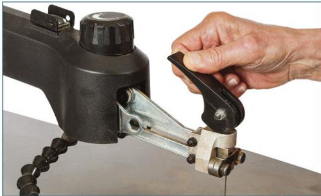
This scroll saw features a lever that clamps and tensions the blade in a single operation.
