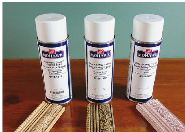
First, make samples like these for comparison. Left to right: Van Dyke brown wet glaze, Van Dyke brown breakaway glaze and white breakaway glaze.
