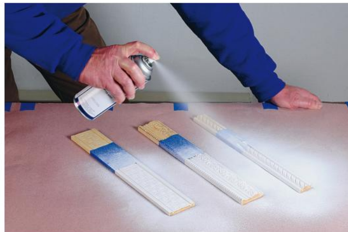
To see the difference the background makes, prepare glaze samples by sealing half of each with shellac and half with white paint.
