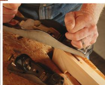
The walnut splines that join the arms and legs are both structural and aesthetic in nature. A jig (left) was specifically made to slice the spline openings into the arms and legs. The spline grain (top) must run across the joint to strengthen it. Once the glue cures, trim and plane the splines flush, as needed (bottom).
