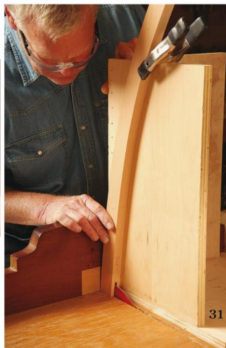
Pattern-routing the rockers is the best way to get identical pieces, once they are cut to final length. The rockers and legs connect with bridle joints, with an open mortise cut into the rockers. Our author used a shop-made variant on the classic table saw tenoning jig (right) to make the mortises.
