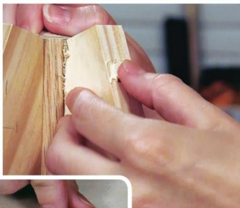
Glue wooden plugs into the counterbores to hide the screws, and sand flush when dry.
