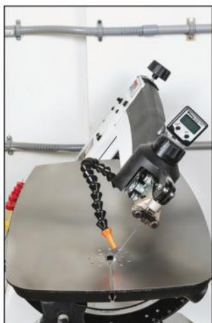
This saw makes bevel cuts by tilting the arm and blade. The saw table remains level.
