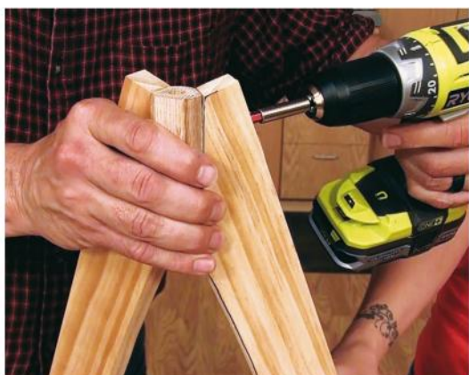
Slip screws into the pilot holes, then apply glue to both mating surfaces before driving the screws securely home to attach each of the legs to the faceted connector.
