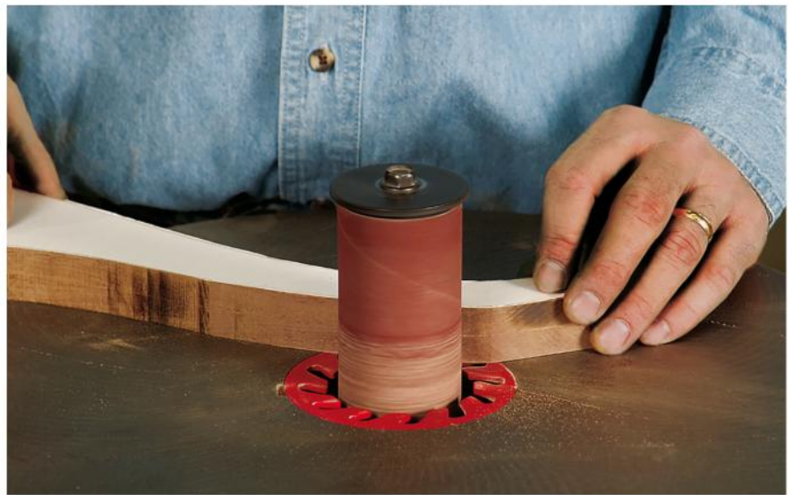
The author used a spindle sander to complete the shaping of the legs and to remove any saw marks from the leg's edges.
