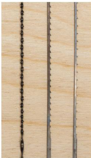
The three basic types of scroll saw blades are, from left to right: spiral, skip tooth and reverse tooth.
