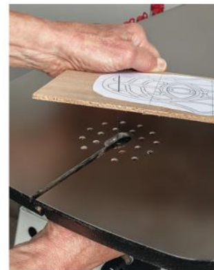
"Bottom feeding" (inserting the blade from under the workpiece) is possible on all scroll saws.
