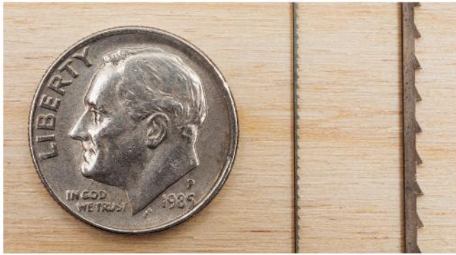
Scroll saw blades are typically 5" long and vary in width. Even the largest, however, are tiny when compared with blades used on other tools.
