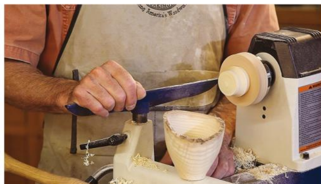
Part off at an angle so as to undercut the base. Hand sand the base, apply finish and admire your newly minted art.
