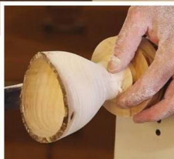
To find the cutoff point, place the eraser of a pencil against the bottom and place your thumbnail even with the high point. Now, with the pencil outside, sight with your nail against this high point and cut below the eraser.
