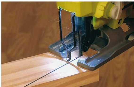
Use a jigsaw to cut along your marked lines. Start with the short cut on the upper leg, and save this triangular cutoff for later. Next, make the long cut to finish the leg.
