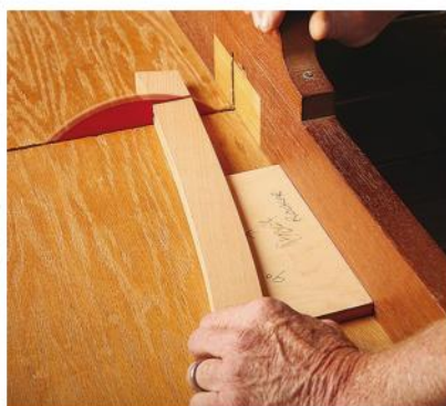
Pattern-routing the rockers is the best way to get identical pieces, once they are cut to final length. The rockers and legs connect with bridle joints, with an open mortise cut into the rockers. Our author used a shop-made variant on the classic table saw tenoning jig (right) to make the mortises.
