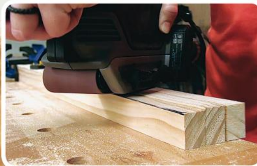
As you sand, be careful to keep the belt sander perpendicular to all three legs. Check your progress often and continue until the three pieces match.
