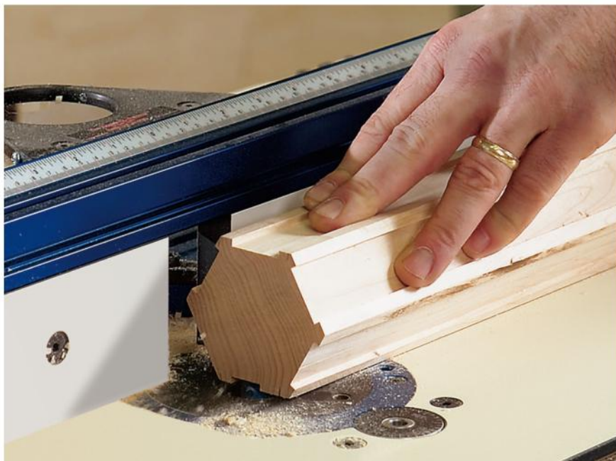
The two-step plowing technique for the grooves in the hexagon (make one pass, flip the workpiece end-for-end and make a second, widening pass without moving the router table fence) is a sure way to keep the opening in the exact center of each facet.
