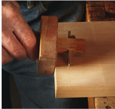
The author scribed a line with his cutting gauge to prevent tearout as he cut the box joints for the seat and back pieces.
