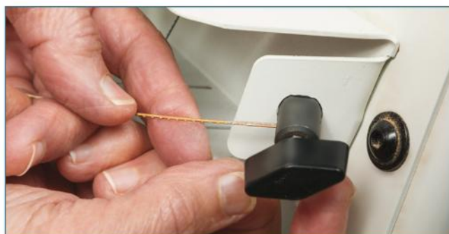
You can easily tighten the lower blade clamp of this saw by hand, but placing it into a built-in holder is required before insertion or removal.
