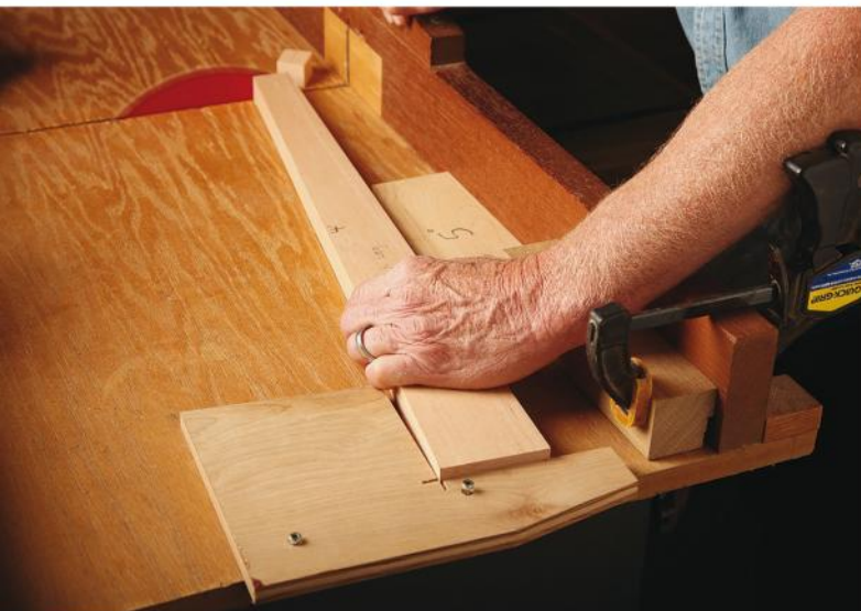
Raising the tenons on the ends of the legs requires a few cuts that must be made accurately. The author used more shop-made jigs and fixtures to machine the tenons. He used scrap lumber to test each cut for accuracy.
