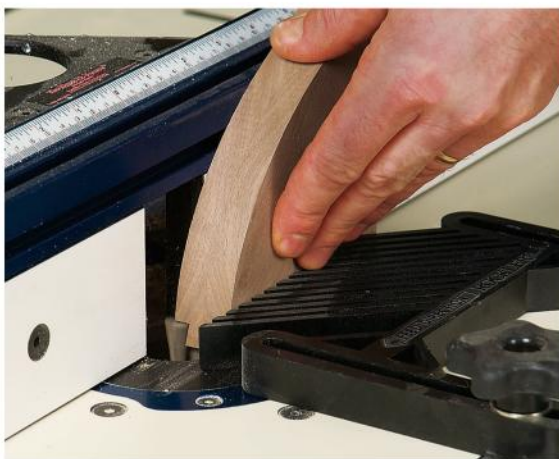
As for the dovetails on the legs, creeping upon on their final width — cutting in multiple passes and making slight adjustments to the fence — helps to prevent tearout of the grain.
