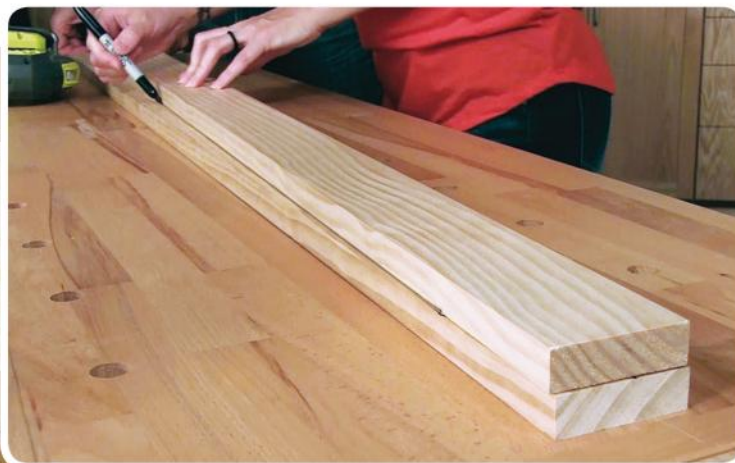
Make a mark 1" from the edge at the bottom of the leg, as shown at left. Align a straightedge from this mark to the one you made earlier, and draw the long cut line between these two points, as shown in the photo above.
