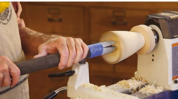
The author uses his Thompson Tool Handle, wrapped in foam rubber with sandpaper taped to it, as a safer sanding option for the interior of his natural edge bowl.
