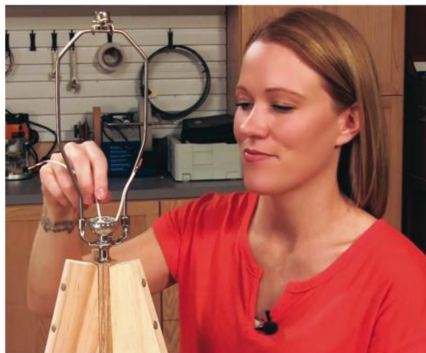
Thread the lamp cord up through the leg connector and socket base from underneath. Separate the ends of the cord, knot it, and secure the wires to the socket screws. Then reassemble the socket.
