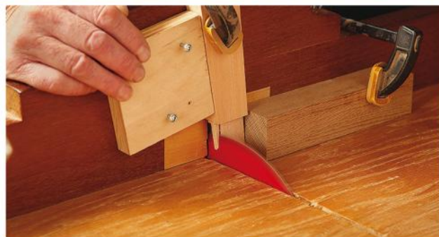
Raising the tenons on the ends of the legs requires a few cuts that must be made accurately. The author used more shop-made jigs and fixtures to machine the tenons. He used scrap lumber to test each cut for accuracy.
