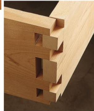
With the box joints carefully marked out, remove the waste from the seat and back. Note the spacer behind the cherry stock: it helps keep the piece tipped back properly at the 5° angle during cutting.
