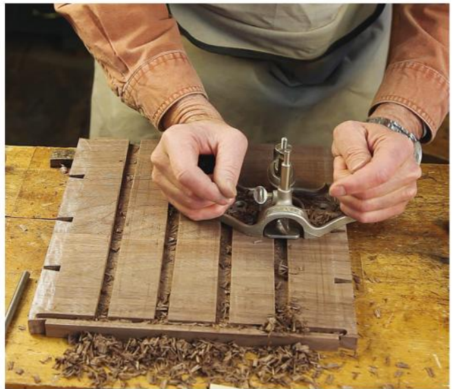
He then removed the waste with a router plane. You could also do this job using a chisel instead.
