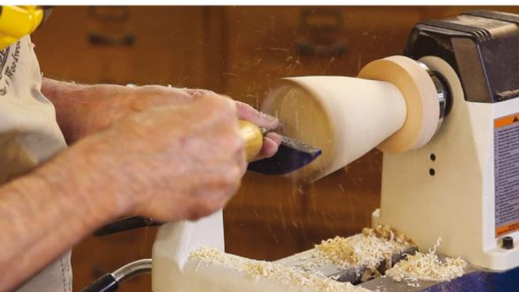
If your gouge skills are tentative, scraping past the uneven rim and then picking up the cut with a bowl gouge is the answer.
