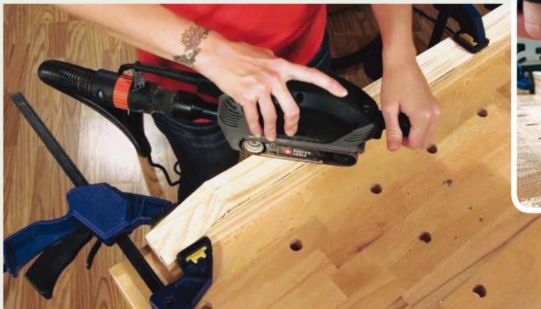
As you sand, be careful to keep the belt sander perpendicular to all three legs. Check your progress often and continue until the three pieces match.
