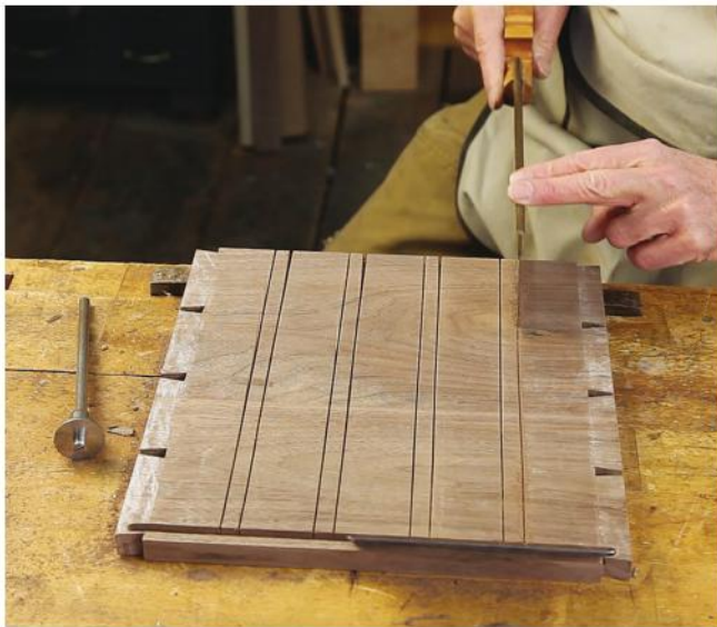
Sawing dados: the author chose to cut the dados in the side panel of the carcass by hand, first back sawing the edges with a carcass saw.
