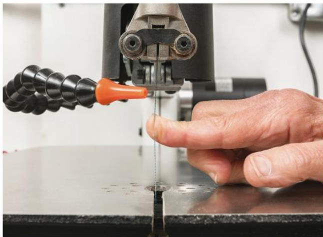
Tensioning a blade correctly is more of an art than a science. The author finds degree of deflection an adequate indicator.
