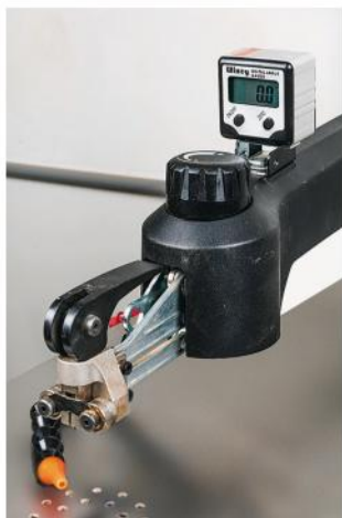
An aftermarket digital readout can provide more accuracy than a scroll saw's angle gauge.
