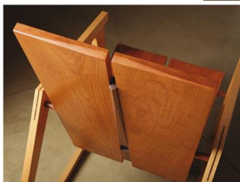
Although small, the walnut seat and back center pieces are key to this chair's design. Tapered to keep the back and seat in a proper relationship, they also have edge detailing that provides shape and shadows. The "disappearing chevron" shape in the back center is shaped with a combination of grinders and spokeshaves. Note in the center photo here that the top edges of the cherry back pieces are shaped with details that complement the disappearing chevrons. In modern furniture, it's often these small details that make the difference.
