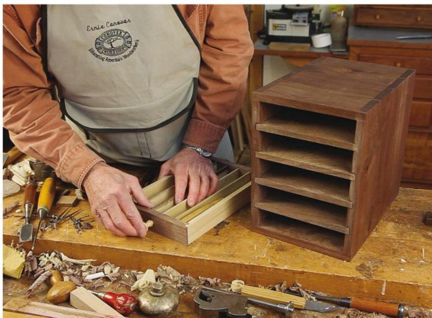
You can see the completed joinery at the edge of the finished drawer, shown here receiving its partitions and a hand-turned knob.
