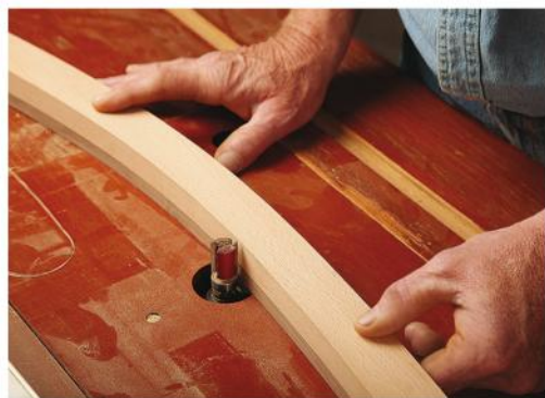
Pattern-routing the rockers is the best way to get identical pieces, once they are cut to final length. The rockers and legs connect with bridle joints, with an open mortise cut into the rockers. Our author used a shop-made variant on the classic table saw tenoning jig (right) to make the mortises.
