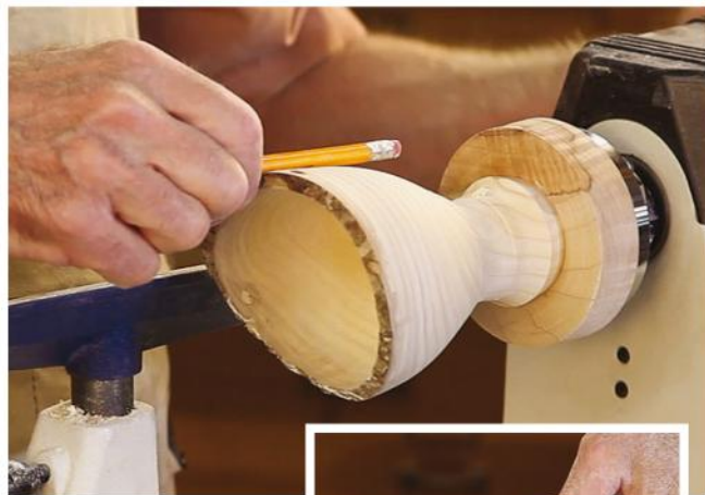
To find the cutoff point, place the eraser of a pencil against the bottom and place your thumbnail even with the high point. Now, with the pencil outside, sight with your nail against this high point and cut below the eraser.
