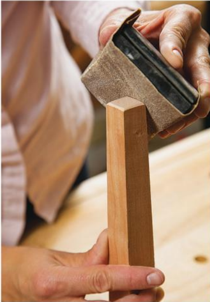
Chamfering the feet helps prevent scratching and snags. For even more protection, cover the feet with adhesive-backed felt pads.
