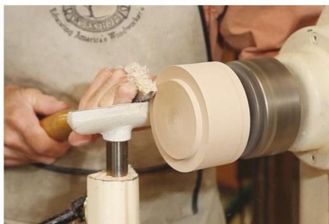
Chuck the lid and turn a tenon that is a press fit with the canister opening.
