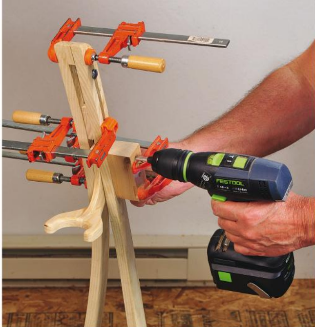
A guide block, made on the drill press by drilling two 5/16" holes 1" apart into scrap block, guides a cordless drill's bit as it bores holes for dowels through both legs and the guitar hanger upright.
