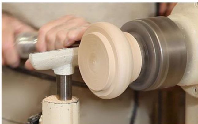
The lid is a lopsided bead, steep toward the tenon and lazy to the top. The near side in the photo should only go to where the outside of the canister meets the tenon's shoulder.
