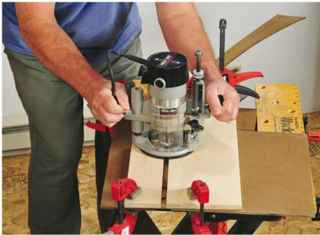
Use two scraps of 1/2" ply to guide a bushing-fitted router to create a 3/8"-wide guide slot at the top of the leg template. The scraps are positioned parallel to one another and 1/2" apart — the O.D. of the guide bushing.
