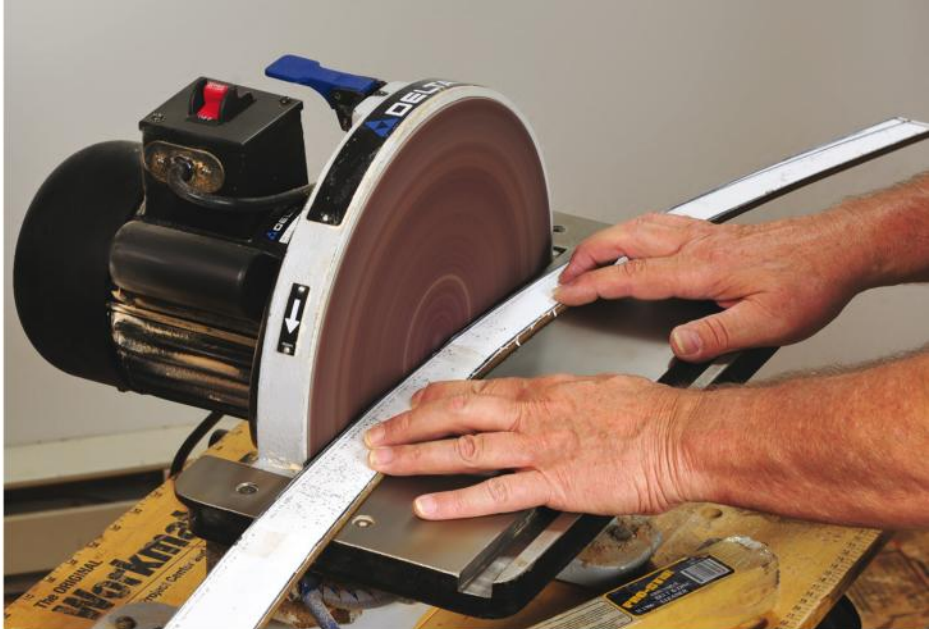
Use spray adhesive to glue the paper pattern atop a piece of 1/4" hardboard, then saw the template to rough shape, trimming it to final shape using disc and drum sanders.
