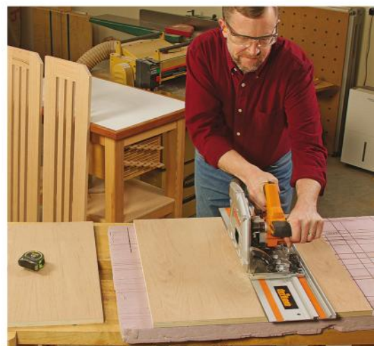
Cut the four shelves to size from a 2 x 4-ft. oak plywood "handy panel." Guide your circular saw with a clamped straightedge, or use a track if your saw has one, to ensure that these cuts are straight.
