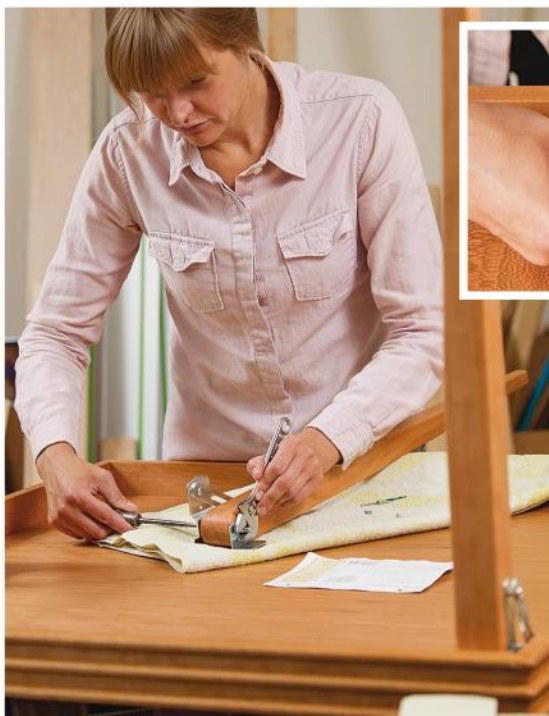
Use a wrench and screwdriver to attach the bracket's top bolt with the locking nut. After marking the screw hole locations on the aprons, drill their pilot holes. Be careful not to drill through the aprons — wrapping the drill bit with masking tape can serve as a simple and prudent depth stop.
