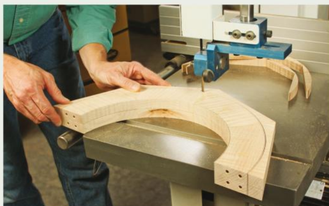
A band saw will make quick work of cutting two subassemblies of four segments into semicircles. Gang them up with double-sided tape.
