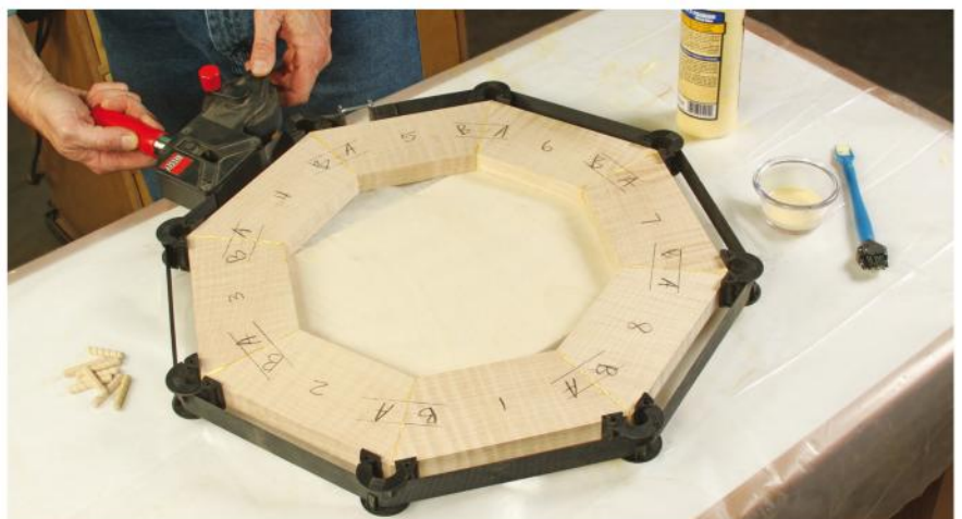
The initial cost of a band clamp will be forgotten the first time you need to clamp an irregular frame like this together. It's the perfect solution. Spread glue onto the joint surfaces, insert the dowels, and tighten the clamp to close the joints. The band applies even pressure to every joint simultaneously.
