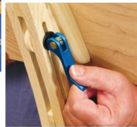
After cutting the bracket arm to shape, glue and clamp the five bracket pieces together (above). A 1/4 " bolt set through the leg slots and bracket hole secures the music holder via a cam clamp (right).
