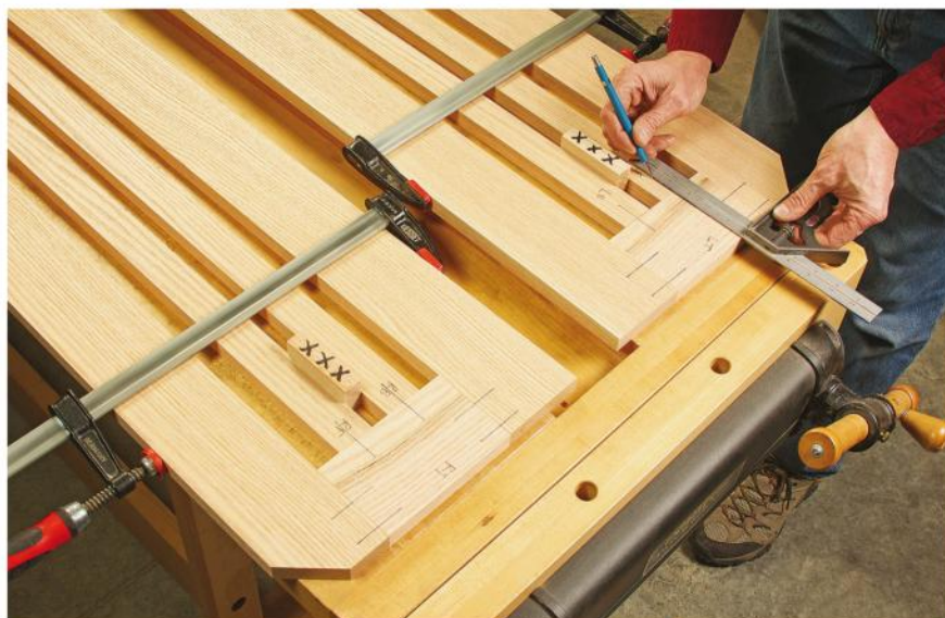
Mark the side assemblies for single dowels that connect the stiles and rails. Center the dowel joints on the stiles. Scrap blocks inserted between the stiles can help hold their spacing for marking.
