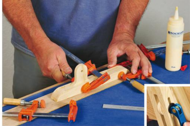
After cutting the bracket arm to shape, glue and clamp the five bracket pieces together (above). A 1/4 " bolt set through the leg slots and bracket hole secures the music holder via a cam clamp (right).
