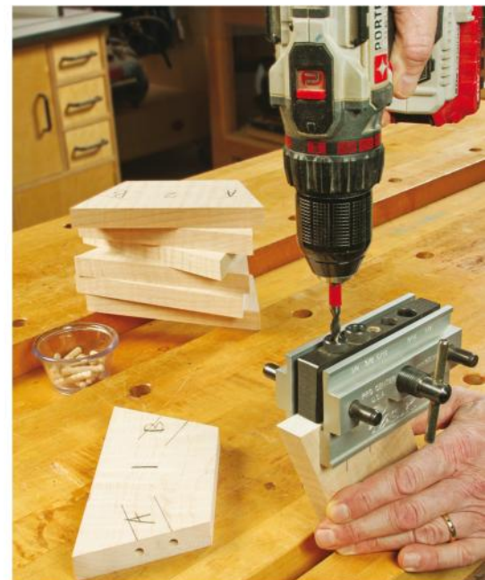
Reinforce the miter joints with a pair of 1/4" dowel pins. Position them 1/16" from the inside corner of the frame segments and 7/8" apart.
