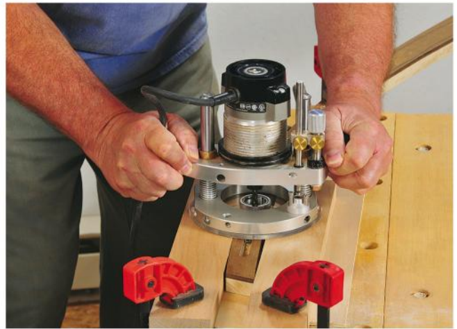
A 3/8" O.D. guide bushing guides the router in the template guide slot as a 1/4" slot is routed. This slot accommodates the bolt and cam lock that support and allow adjustment of the stand's music holder.
