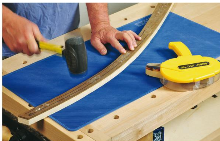
In preparation for pattern routing, the leg template shown here is temporarily attached to the rough-cut stock using adhesive transfer tape. Pounding with a mallet increases the strength of the tape's bond.
