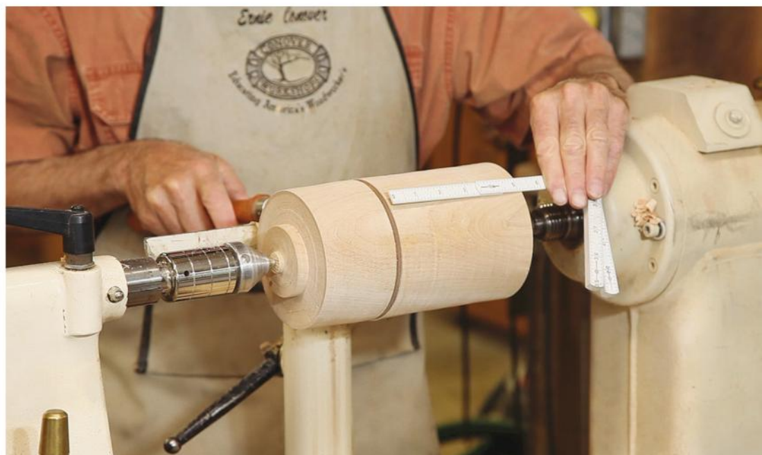
The author's stub tenons are 3/8"-long by 2 1/2" diameter: the optimal outside holding diameter of his Oneway Stronghold chuck. Adjust your tenon dimensions according to your chuck. Here, he is parting the lid away, leaving the canister height 5 1/8" above the tenon.
