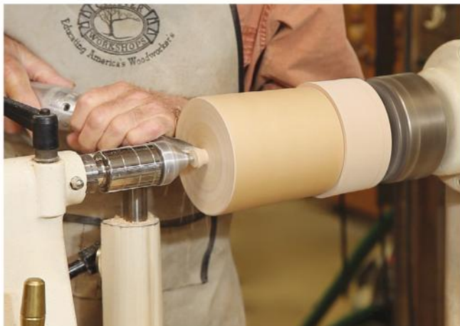
The bottom of the canister is turned by pinning it against the lid. The bottom should be slightly undercut to a small chucking nubbin which can be chiseled and sanded away later.
