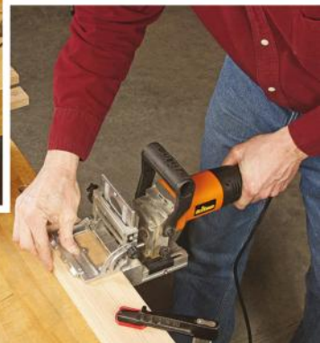
Bore dowel holes at your layout lines in the legs, rails and stiles. When drilling holes in the ends of the narrow stiles, it's helpful to clamp all four together (see inset). One of two bits must be removed from the Triton Duo Dowel Jointer, shown here, to drill single holes in the stiles and rails.
