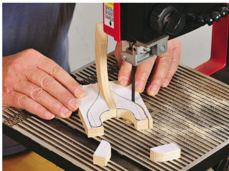
Two rectangular blanks for the guitar hanger's prongs are first glued to the sides of the upright piece, then cut to shape on the band saw. Their edges are rounded and shaped with rasps and rifflers, then sanded smooth.
