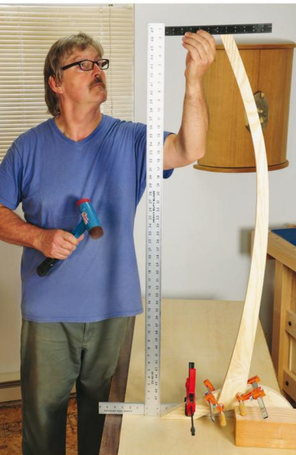
With a leg and foot clamped together and set on a flat table (left), position a sheet rock square against the back edge of the foot and use a rule to confirm the alignment of the leg. The distance to the top of the leg should be 6 1/4"; if it's not, the angle of the leg can be tweaked slightly. Scribe the edge of the leg's lap joint with a sharp knife (top), before routing the joint to a depth of 1/4" using a straight bit in a router (above), then trimming it with a chisel.
