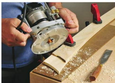
With a leg and foot clamped together and set on a flat table (left), position a sheet rock square against the back edge of the foot and use a rule to confirm the alignment of the leg. The distance to the top of the leg should be 6 1/4"; if it's not, the angle of the leg can be tweaked slightly. Scribe the edge of the leg's lap joint with a sharp knife (top), before routing the joint to a depth of 1/4" using a straight bit in a router (above), then trimming it with a chisel.
