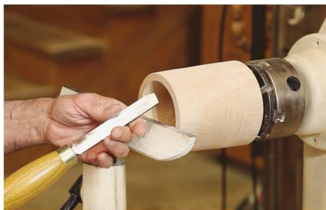
The lion's share of the hollowing can be done with the spindle gouge, but you'll need large square-end scrapers to finalize the side wall and bottom.
