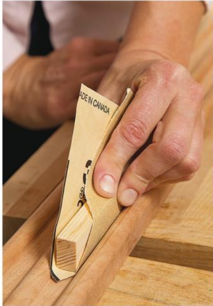
The author used a 1/2"-thick piece of wood to sand effectively between the apron beads. Sand all the way up to 220-grit.
