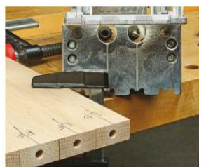
Mark the side assemblies for single dowels that connect the stiles and rails. Center the dowel joints on the stiles. Scrap blocks inserted between the stiles can help hold their spacing for marking.
