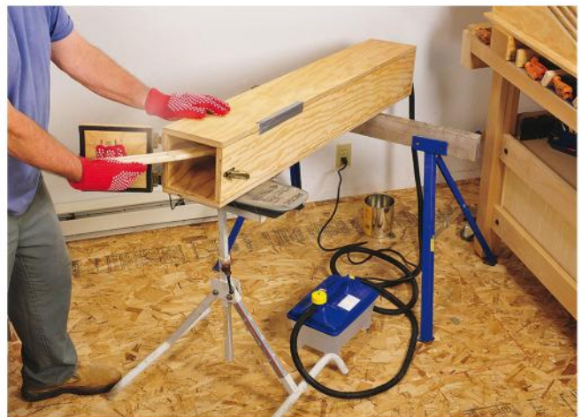
A steam generator supplies steam to a 4-ft.-long plywood steam box. Steam each of the stand's ash legs for 45 minutes before quickly removing them and clamping to the form. Wear oven mitts to protect from burns.
