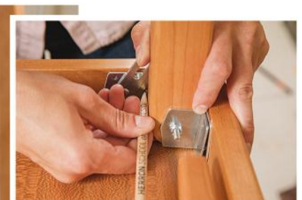
Use a wrench and screwdriver to attach the bracket's top bolt with the locking nut. After marking the screw hole locations on the aprons, drill their pilot holes. Be careful not to drill through the aprons — wrapping the drill bit with masking tape can serve as a simple and prudent depth stop.
