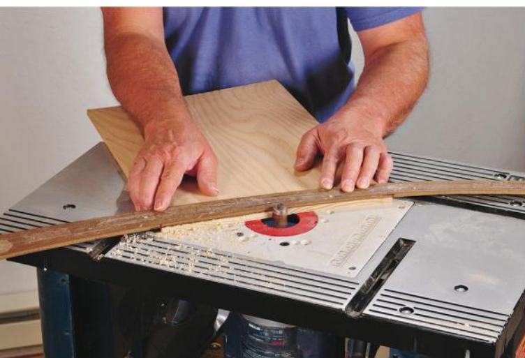
Use a section of the concave side of the leg template to shape both curved side edges of the music holder. The pattern routing process is the same process used earlier to trim the legs and feet to shape.
