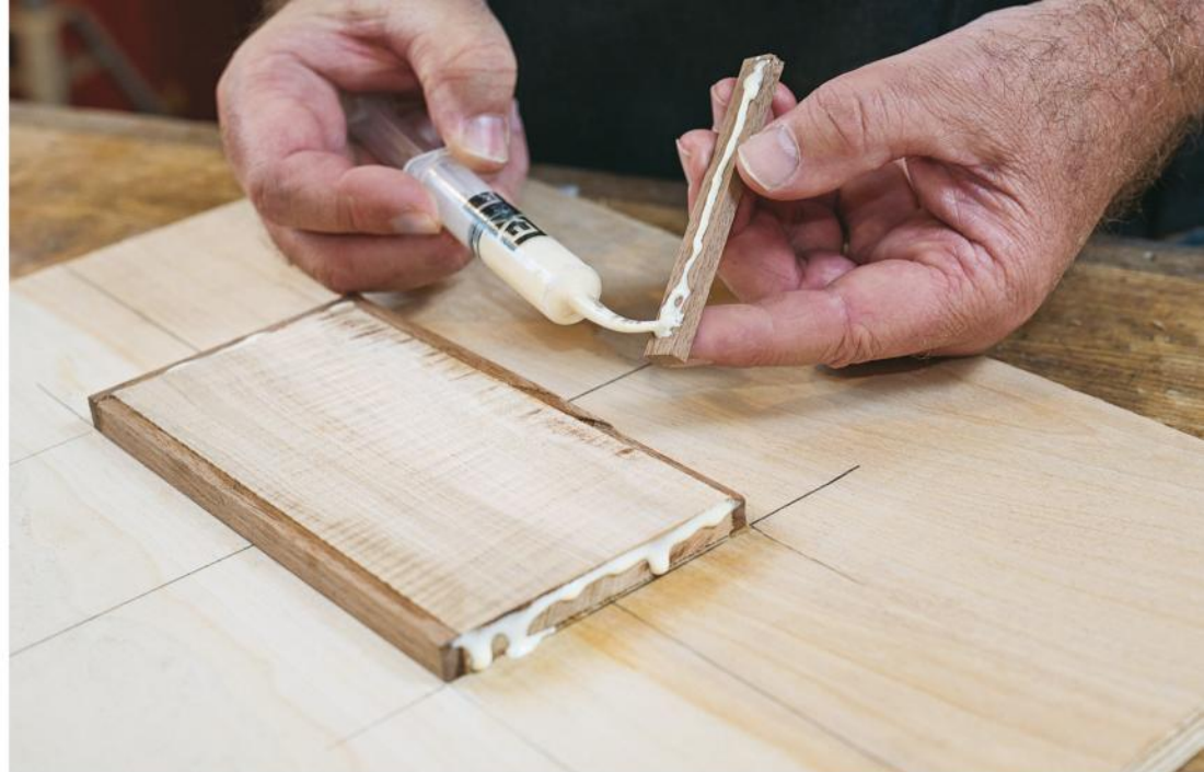
Once you've trimmed the surrounding strips to the exact length so there are no protrusions, glue the thin strips around the center panel. A glue syringe allows a more exacting method of glue application.
