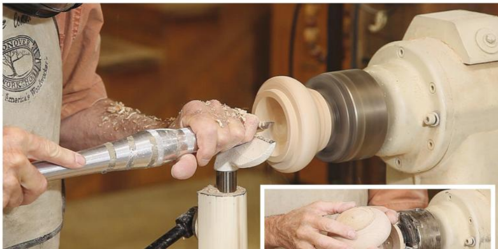
Hollow out the center of the tenon to reduce weight and give a refined look. After parting off, the top of the lid can be turned to shape in a jam chuck or simply sanded to a gentle domed shape.
