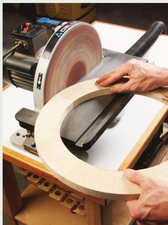
After gluing the half circles together, refine the outer rim on a disc sander and smooth the inner rim on a drum sander.
