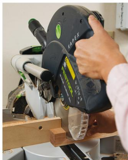
Crosscut the legs to length on the miter saw, but make sure you use a stop for precision. The legs need to be accurately cut for the table to sit level.
