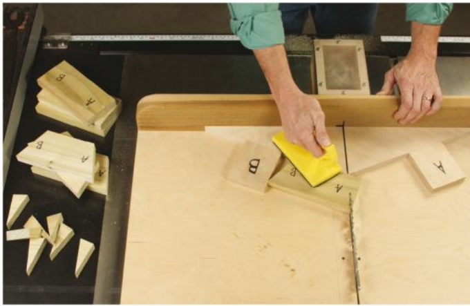
Cut eight test pieces to width and length first, and mark them with A and B ends. Hold each segment against the A stop and miter-cut one end to 67.5°, then set the mitered end against the B stop to angle-cut the opposite end.
