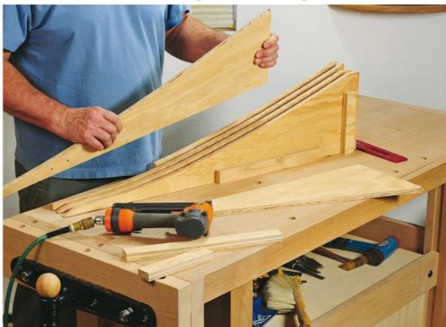
Before steaming begins, build a bending form from scraps of 1/2"- or 3/4"-thick plywood. Nail 3/4"-thick spacers between the sawn segments to make the form 6 1/2" wide, then nail the assembly to a plywood baseplate.
