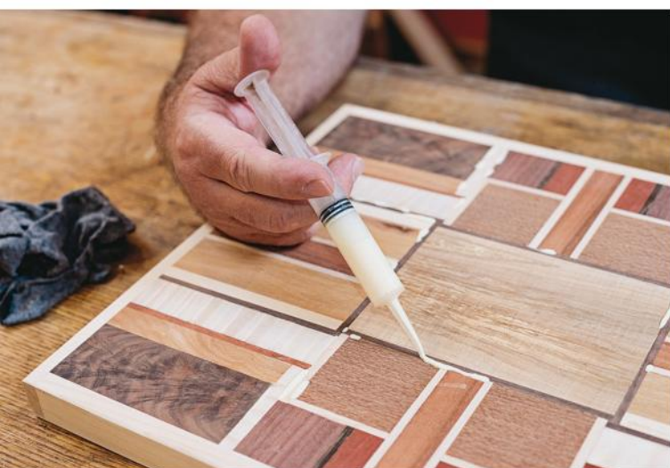
Inject glue into small cracks, wipe off the excess glue, and lightly sand over the glue-filled crack to hide the gap with fine sawdust.
