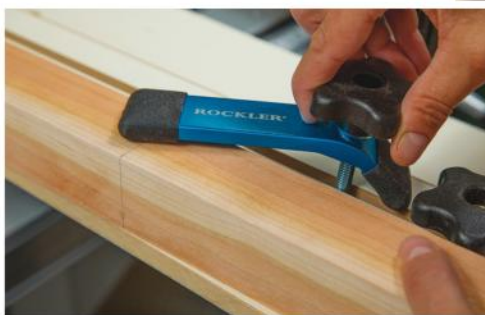
The author adjusted the tapering jig with a leg in place, according to her pencilled layout. Have the blade cut to the waste side of the layout line. After fine-tuning the setup, slide the jig forward to create the tapered rip cut, then flip and re-clamp the leg in the jig to taper an adjacent leg face.
