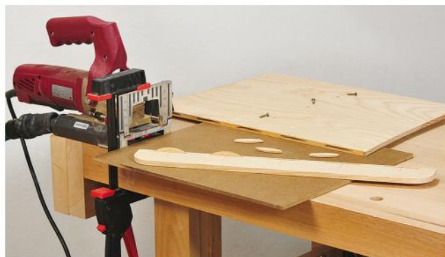
Use a biscuit joiner to plunge cut slots for the five #0 biscuits that reinforce the joint between the music stand's music holder and ledge. Three countersunk holes in the holder will be used to join the holder to its bracket.
