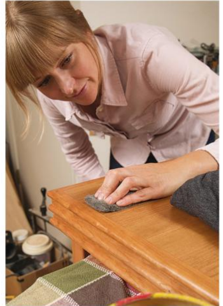
After the finish cures, apply a coat of paste wax for a bit of extra protection as well as to make the table's surfaces silky to the touch.
