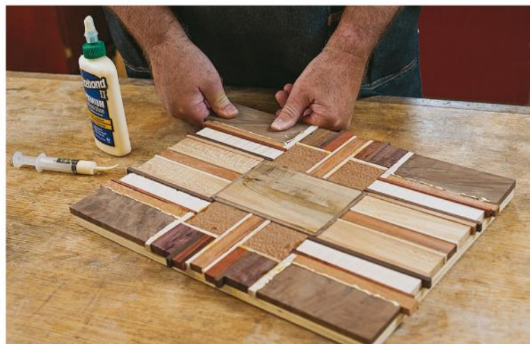
Working from the center of the project to the outside edges, glue pieces of wood to the plywood base, keeping the design symmetrical.
