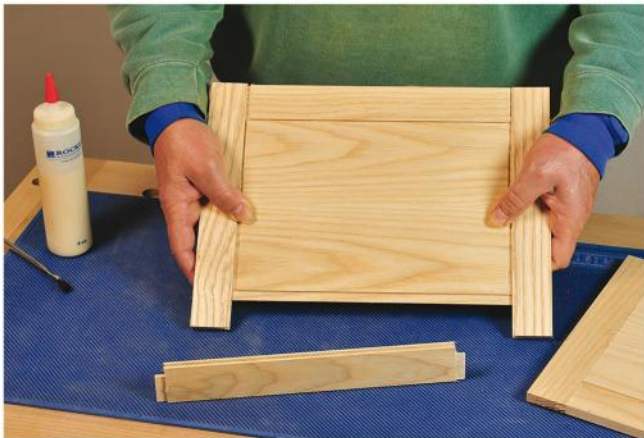
Cut a rabbet all the way around the top edge of the lid panels to slip into grooves cut in the lid frame members. This positions the top surface of the 1/4"-thick panel flush with the top of the frame.
