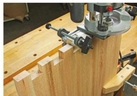
The 4556's clamps hold it securely on the edge of a panel for handheld routing. It also cuts the widest joint pattern of any jig here, at 1 9/16".
