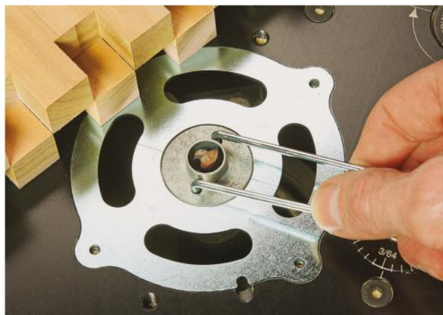
eBush's elliptical shape around the bit allows you to improve the fit of joints in thousandths of an inch by turning the collar left or right.
