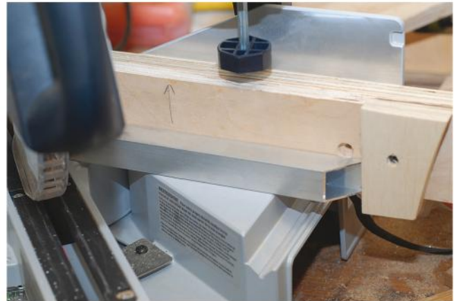
Stop blocks on the miter saw fence ensure that you'll cut the rails and stiles of the leg assemblies to the same length.
