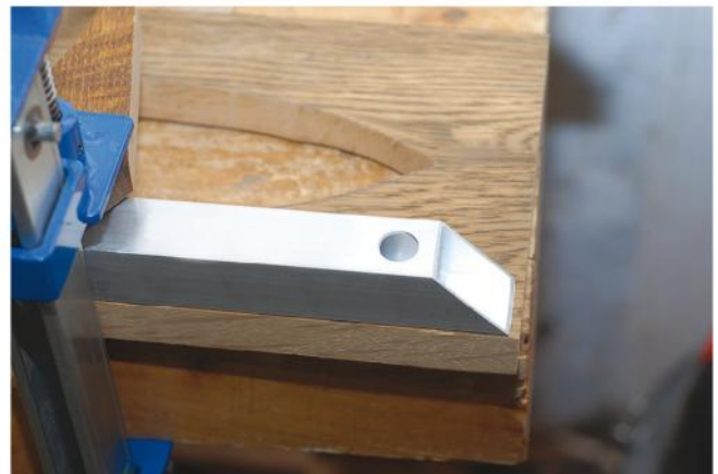
Drill a hole large enough to fit your screw heads through the bottom wall of the top rail tubing in each leg assembly.
