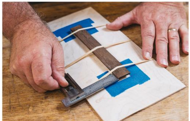
A combination square works nicely to center the lift/spacer onto the lid. Mark the location with painter's tape and use rubber bands for clamps.
