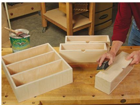
Ease the sharp corners created by the folding joints with a sanding block. Then sand the rest of the bare wood before topcoating the project surfaces with your favorite finish.
