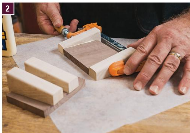
2 With the bevel edges facing up, glue and clamp an end assembly between a pair of legs, keeping the top edges and bottom surfaces flush.
