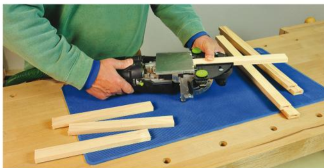
The author used Domino joinery for the members that join the basket's frame. He used a guide with the Domino machine to plunge-cut mortises for loose tenons in the ends of the frame rails.
