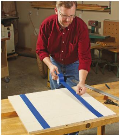
Cover four penciled layout lines on the back of the cabinet panel with painter's tape to support the fragile veneer along these fold lines.
