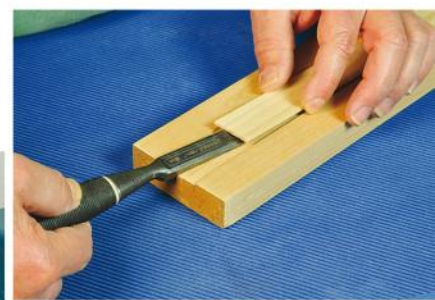
Apply adhesive transfer tape or carpet tape to the carrier board to keep the thin wood weaving strips flat during thickness planing. After planing, pry the strip up with a chisel.
