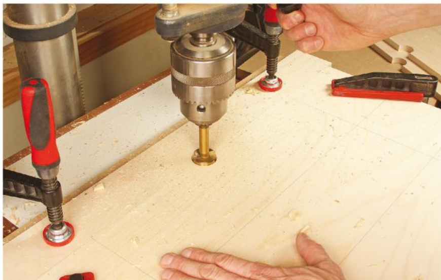
Bore a half circle into one edge of each drawer blank with a 1/4"-dia. Forstner bit to form a finger pull. Clamp the workpiece against a scrap of the same thickness first, to act as backup fence.
