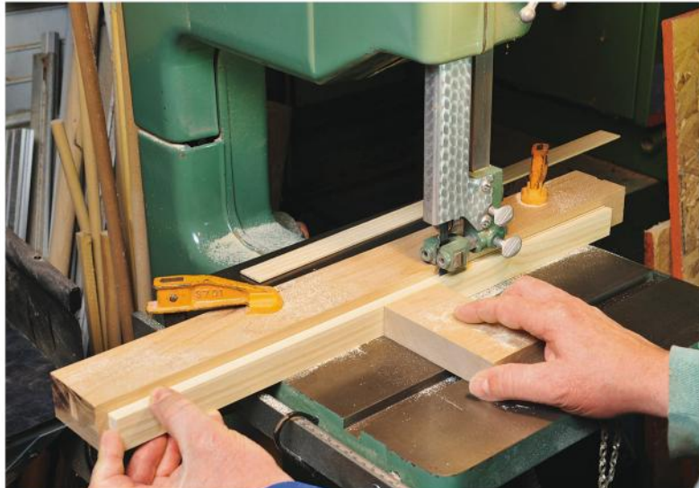
A thick, straight board clamped to the band saw table creates a stable fence used to guide workpieces past a wide resaw blade. The thin strips that are sawn with this setup are used to weave the picnic basket's lightweight side panels.
