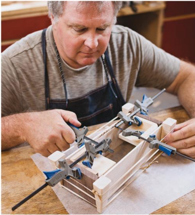
Rubber bands make excellent clamps for assembling a pair of sides between the end assemblies. Corner braces and small clamps help ensure a square finished assembly.
