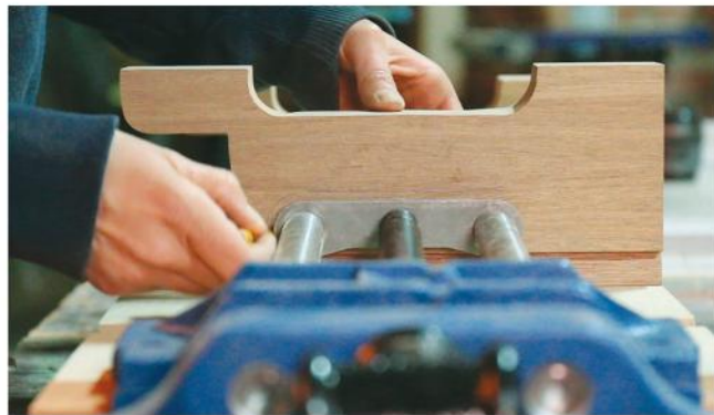
You'll need to drill holes through the leg closest to the end vise in order for its posts and threaded rod to pass through. Mark and drill carefully.
