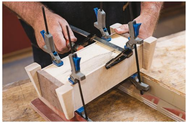
Cut the box bottom to fit snugly inside the rabbet bottom edge of each side piece. Check the fit, and glue and clamp it in place.
