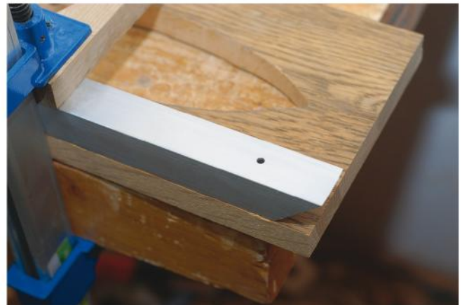
Drill a pilot hole wider than the threads of your screws in the upper rail of each leg assembly. The author used a 3/16"-dia. drill bit here.
