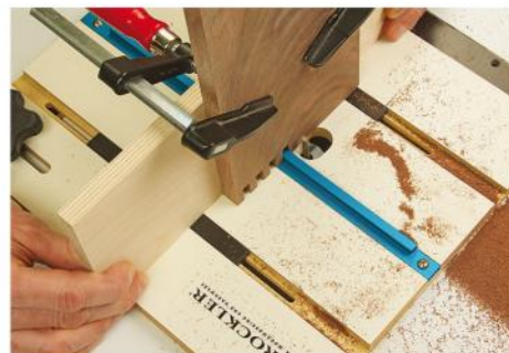
Built-in stops in the bottom of the backer sled slots keep the sled from sliding too far; they prevent the bit from cutting through the sled's back plastic face.
