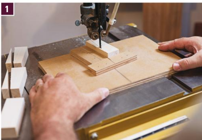
1 For identical taper cuts on each box leg, a band saw sled fitted with two angled cleats works perfectly for consistent taper cuts.
