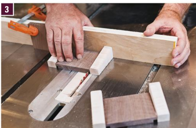
3 Using a miter gauge with a sacrificial fence and stop, cut a pair of grooves through the end assembly to house the box sides.
