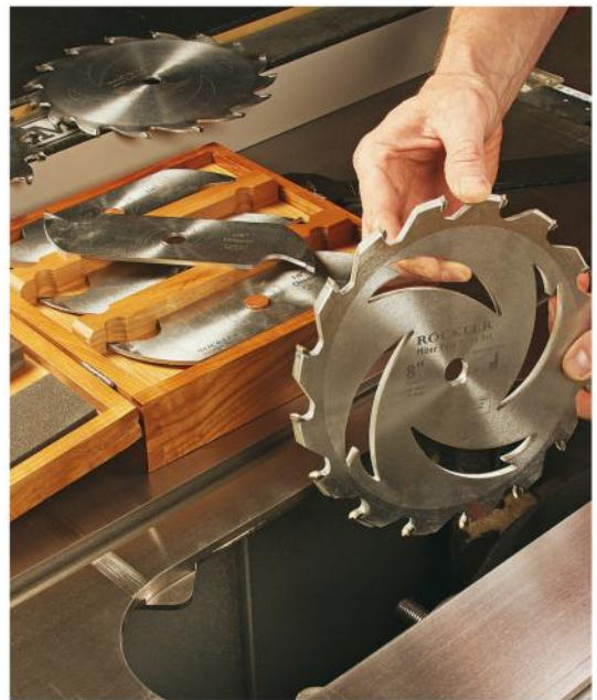
The Miter Fold Blade's specialty blade, in tandem with the kit's stacked dado blade, cuts an interlocking, hinged miter joint. Load the parts to the correct cutting width required.
