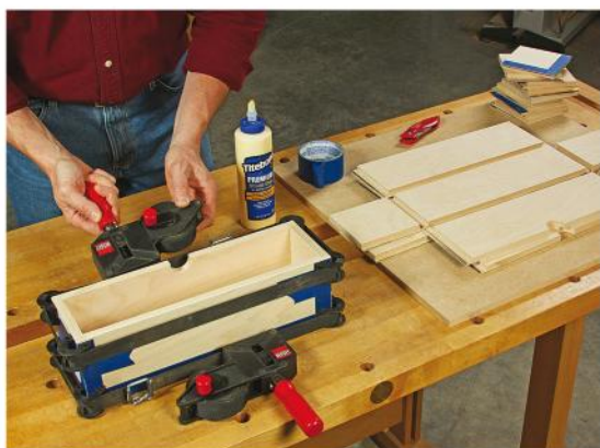
With the exception of there being no divider dados, building the drawers involves the same cutting, gluing and clamping strategy as the cabinet carcass — only with smaller panels.
