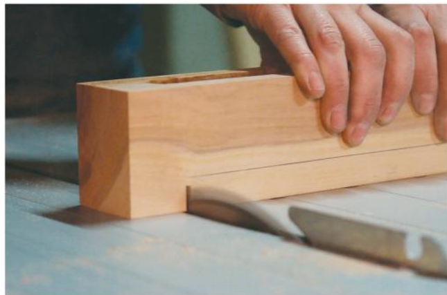
The outer end of the breadboard holding the vise will need some retrofitting, too. The author cut a vise recess with her table saw.
