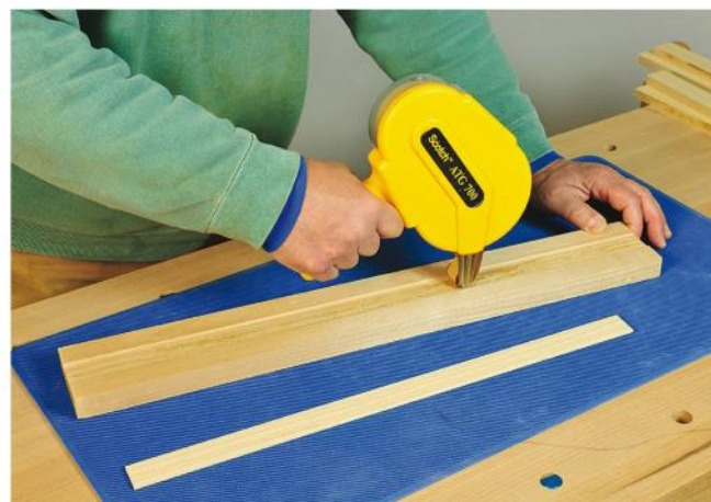
Apply adhesive transfer tape or carpet tape to the carrier board to keep the thin wood weaving strips flat during thickness planing. After planing, pry the strip up with a chisel.
