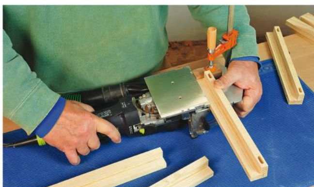
All the corner stiles have mortises plunge-cut near the ends. Here, the author properly spaced the mortises from the ends of the stiles with a stop block clamped to the Domino machine's flip-down fence.
