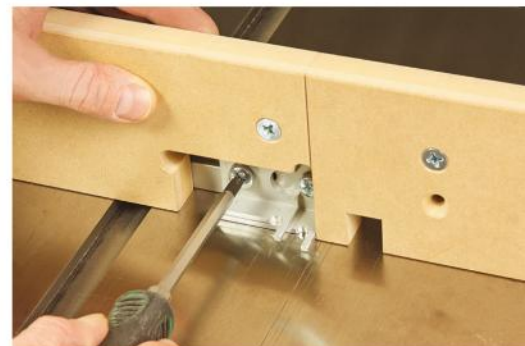
A pair of metal pins fit inside slot cuts to register the joint during machining. A screw on each pin sets their spacing.
