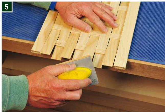
5 Chamfer the ends of the wide horizontal weaving strips with a sanding block. This makes them easier to slip into the narrow stile grooves in the next step.
