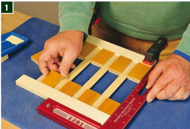
1 Blocks cut from scrap plywood keep the narrower vertical weaving strips properly spaced as they are glued into the bottom rails. Glue the top rails on after weaving the sides.
