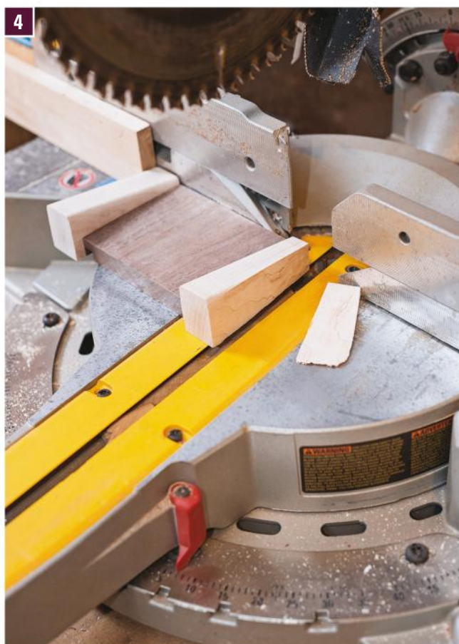
4 Angle the blade, set up a stop on the miter saw fence, and miter-cut the outside edge of each leg on each end assembly.
