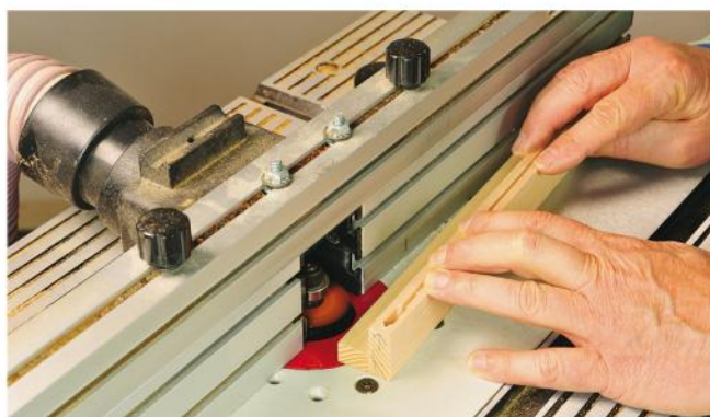
Plow a groove in the edges of the picnic basket's frame members with a slot-cutting bit in the router table. The ends of the weaving strips slip into these narrow grooves when the basket's sides are woven.
