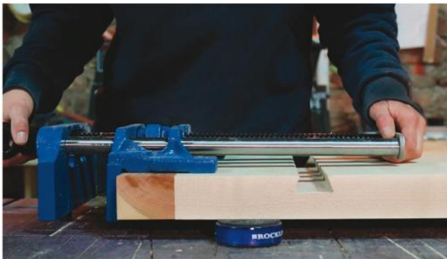
Position the vise on the end of your inverted benchtop where you want it and mark its location, plus any modifications that might be necessary.
