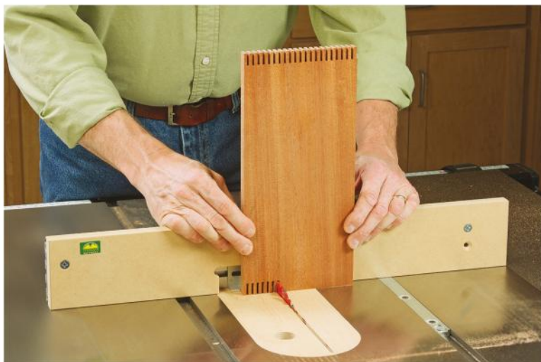
A pair of metal pins fit inside slot cuts to register the joint during machining. A screw on each pin sets their spacing.
