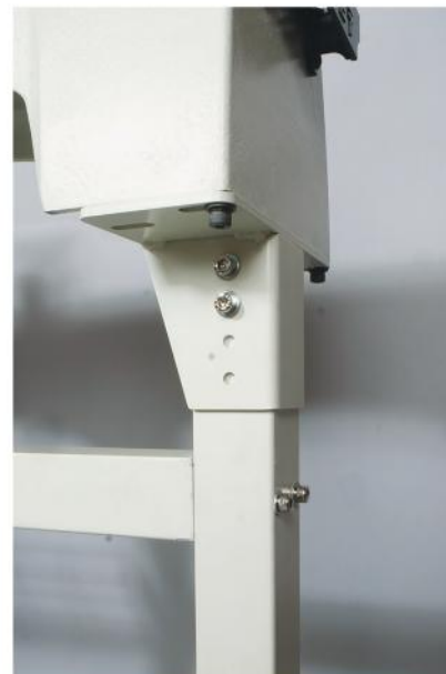
The JET had the best stand, with very heavy-gauge metal, more than adequate height adjustment and quality fasteners — many plated. All holes lined up perfectly.
