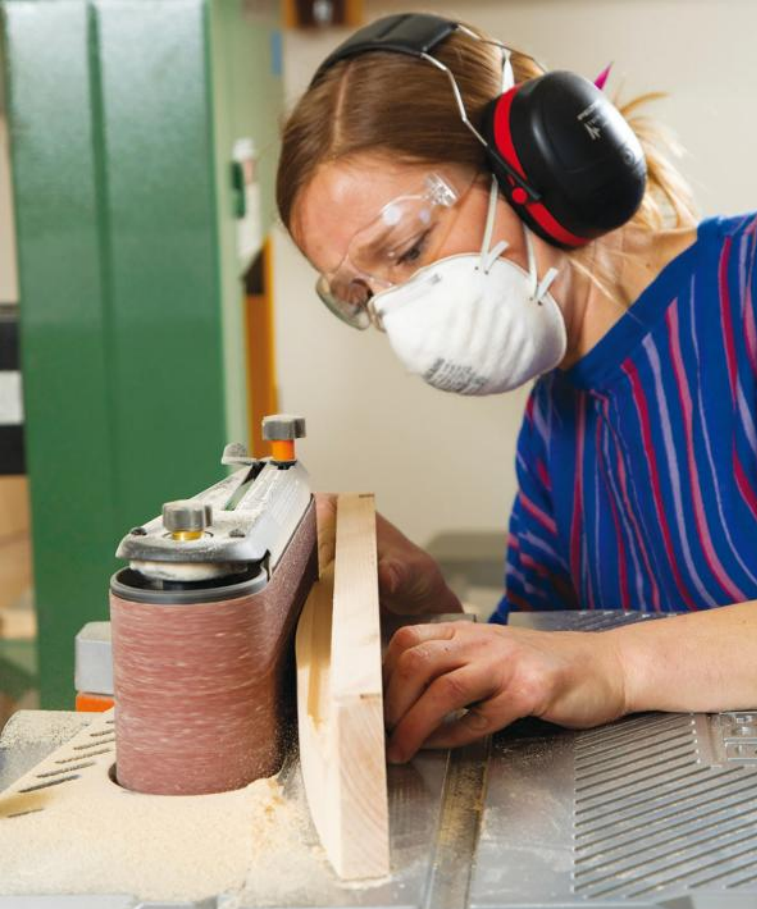
A benchtop sander with a horizontal belt made it easy to smooth the outside curved faces of the top and bottom tray end pieces.
