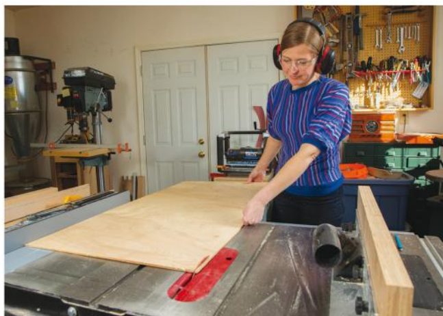
Dry-assemble the top and bottom trays so you can be sure to cut the bottom panels to the correct fit. Quarter-inch plywood was used here.
