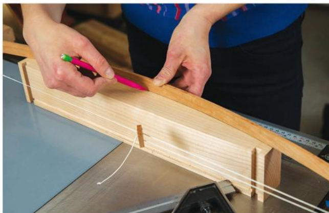
A curve bow can set the broad arch shapes you'll cut into the ends of the top and bottom trays — but wait to make these cuts until after you shape the top tray handles into the tray ends.
