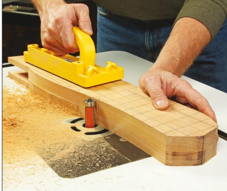
Use your "master" seat support and seat back to template-route their shapes onto the other two sets of seat frame parts. A piloted flush-trim bit makes part duplication like this easy.
