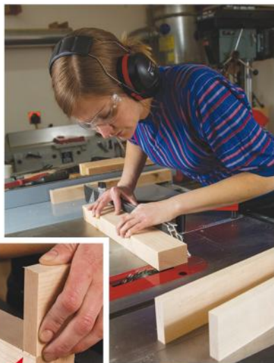
The author verified the position of her tray dados by nicking the first cut (top) and referencing it against a side piece (inset).
