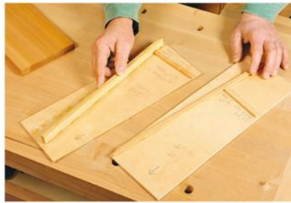
The tall fence strip on the second stave cutting jig (left) angles in the opposite direction than the fence on the first jig (right).
