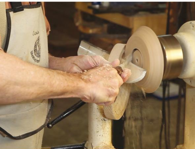
The three roof rings are parted out of a single piece of wood. The parting tool is guided into the piece at a 45° angle. When their order is reversed, they stack up nicely.
