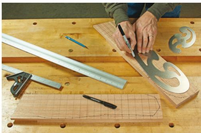
On a pair of gridded workpieces, plot points and draw the profiles for a seat support and seat back. A large French curve makes it easy to connect these dots with smooth, flowing lines.
