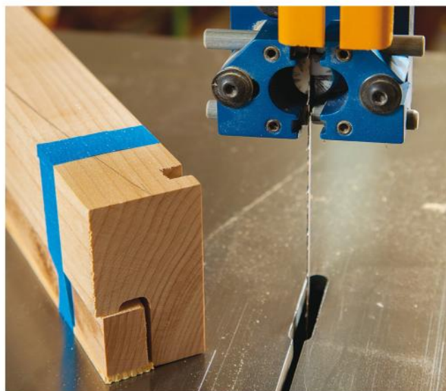
Tape the offcuts you made from the rabbeted handle cutouts back into place before hand-sawing broad arches into the top tray's end pieces.
