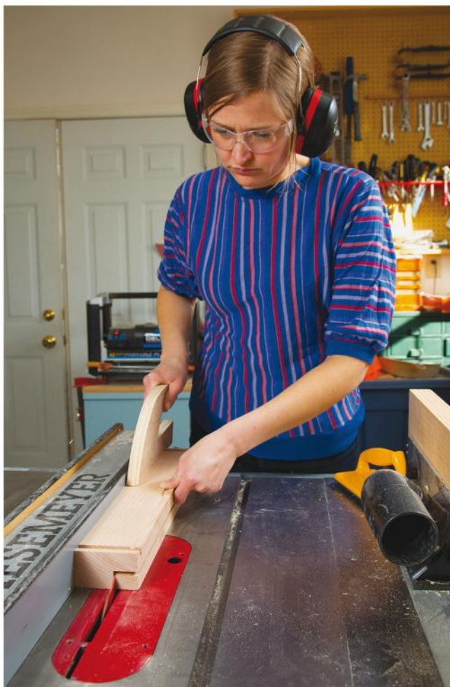
The top tray handles begin as large rabbet cutouts in the tray end pieces. Make these with two table saw cuts, and save the waste pieces.
