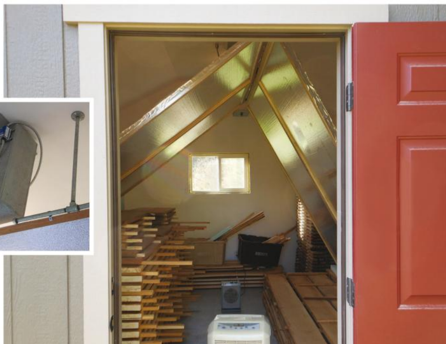
Here the author's kiln is set up with the baffles in place and the electric heater and dehumidifier in the aisle between the wood stacks. A fan is also in place over the conduit baffle frame (inset).
