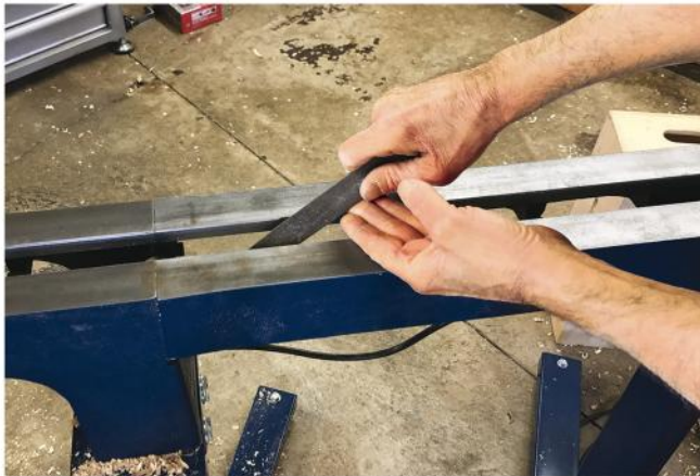
All of the lathes in this review had a sharp edge on the bottom corner of the bed ways. The author used a file to smooth this out.
