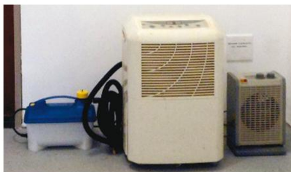
A dehumidifier, a 1,500-watt electric heater with a tip-over shutoff switch and a steam generator — very common home center and Rockler supplies — are used to control lumber drying.
