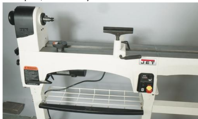
The JET's DC speed controller was nicely placed, easy to use, and had digital readout. The tool basket allows for storage of chucks and faceplates without collecting chips.
