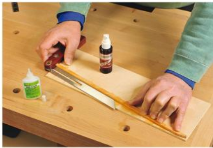
A spray-on CA accelerator quickly sets the glue applied to the "fence" strip on the first tapered stave cutting jig.
