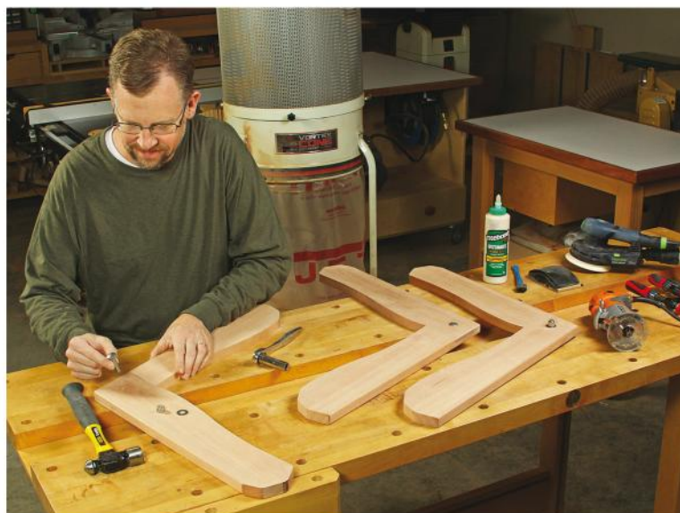
Glue and clamp the three seat frames together, and sand the joints flush. Ease the bottom sharp edges if you wish. Then reinforce each lap joint with a stainless or galvanized carriage bolt, washer and nut.
