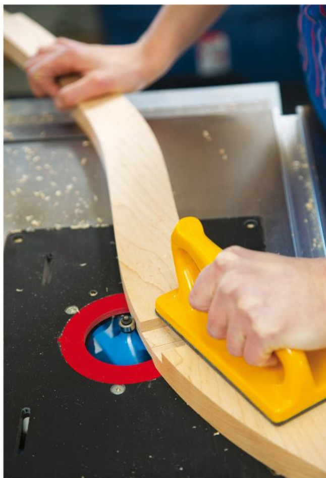
The author eased the long, sharp outside edges of the legs at her router table using the Rockler Table Edge/Handrail Router Bit. Be careful of grain direction.
