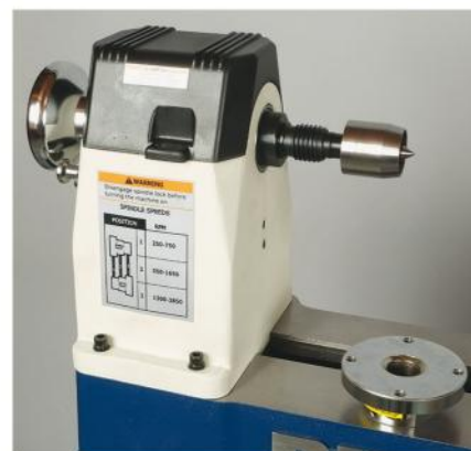
Like many of the lathes, the RIKON's exterior sports a spindle speed chart.
