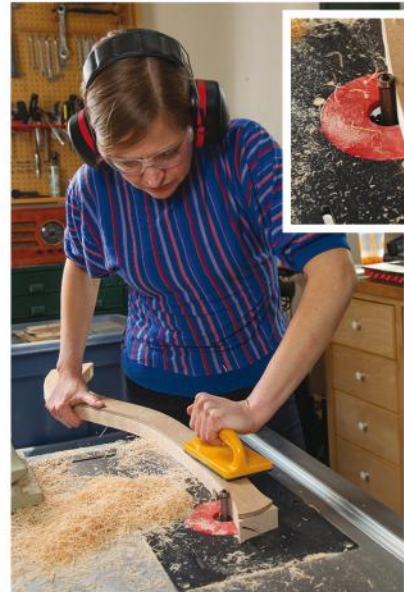
Follow your directional arrows (inset) to avoid routing against the grain, and don't rout around the ends of the feet, or they can chip.
