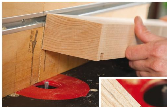
Since the tray bottom grooves are cut face-down and must terminate at the corner joint dados, mark your router fence (top) so you can start and stop them accurately.
