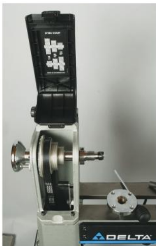
The DELTA DC speed controller had a chart which gave an accurate prediction of speeds at a given number and pulley groove setting, but our author would have liked to have seen a digital readout.
