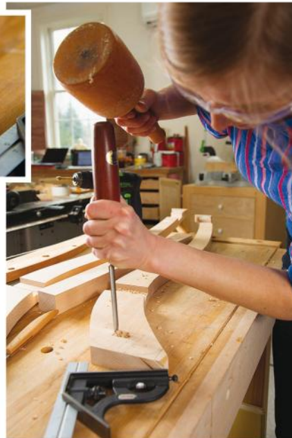
Work carefully when squaring up the mortises, and try to keep your chisel perfectly perpendicular, cutting a tiny bit outward.
