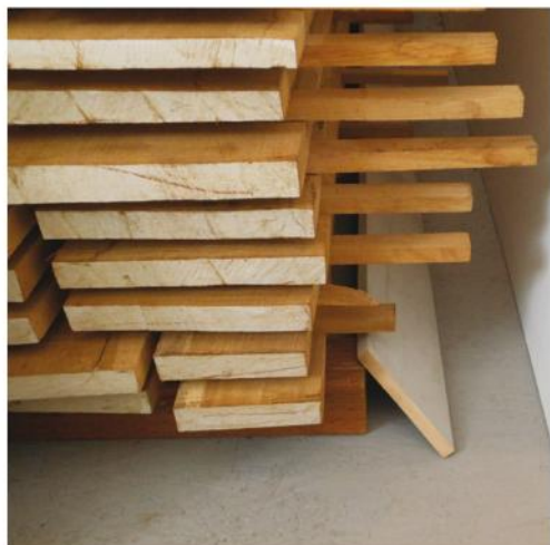
The kicker board stops airflow from predominantly going under the stack of lumber. The angle of the board helps direct the flow up toward the stacked lumber.
