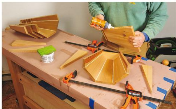
Once the small bottom piece is set into its slot in the planter staves, glue and clamp the back in place, using a pair of wedges as cauls.
