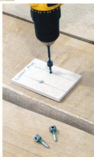
It is possible to use moisture meter probes that you secure to lumber within the stack, which will give you readings otherwise difficult to get.
