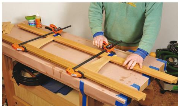
The author used loose tenons, secured with polyurethane glue, to join the planter box frame's risers and rails together.
