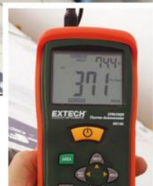
Here the author measures the airflow and effectiveness of his baffles with an Extech AN100 anemometer. Around 350 feet per minute is a good air speed.
