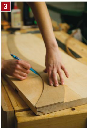
3 Use your template, lined up carefully with the ends of the leg blanks, to draw two leg shapes per blank, nested together.
