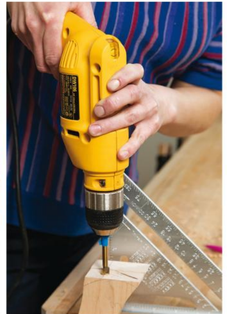
When drilling the legs for casters, be mindful of what the grain on the feet is doing. Move their position, if needed, to avoid weak, short grain.
