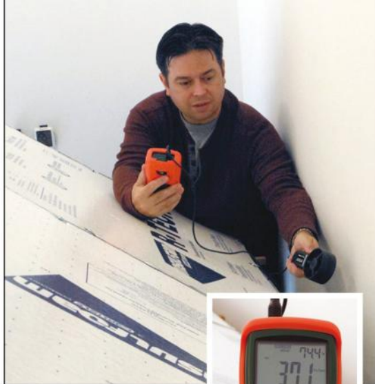
Here the author measures the airflow and effectiveness of his baffles with an Extech AN100 anemometer. Around 350 feet per minute is a good air speed.
