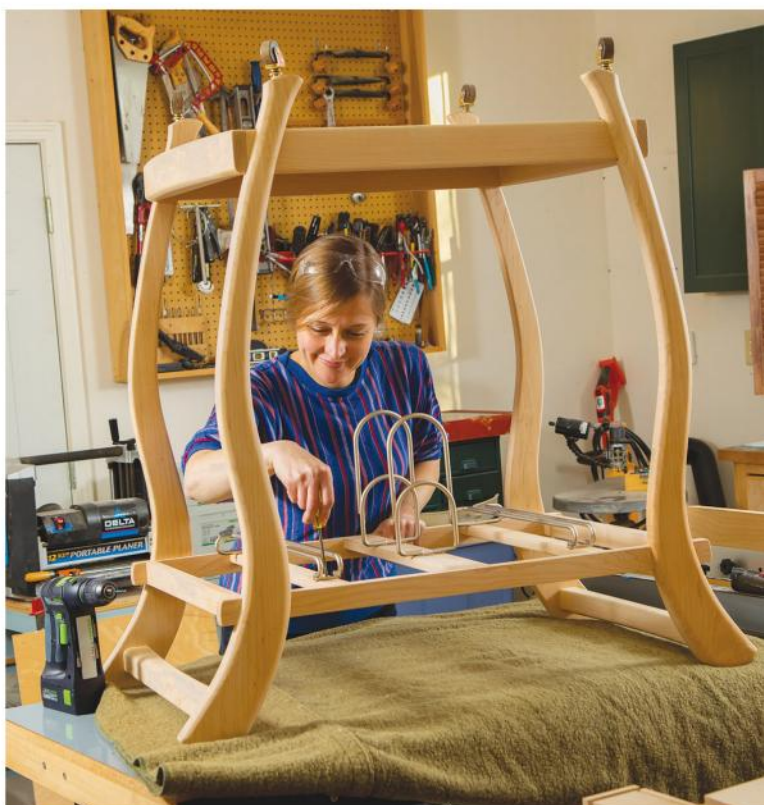
Attach the cart's stemware and bottle holders to the top tray cross support bars with short screws driven into pilot holes.
