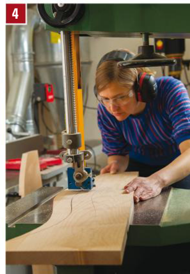
4 Cut out the four legs with a band saw or jigsaw, sawing just to the waste side of your penciled layout lines.
