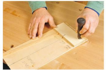
The third stave jig, which is used to cut staves in half, has a handle to make guiding the jig past the saw blade a safer process.
