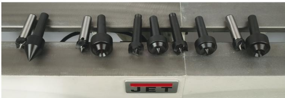
Almost all of the live centers supplied with the lathes in this review were nearly identical, indicating that the components likely came from the same manufacturers (a common industry practice).
