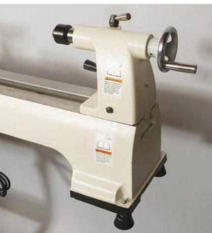
The Steelex's surface-ground bed shows attention to quality.
