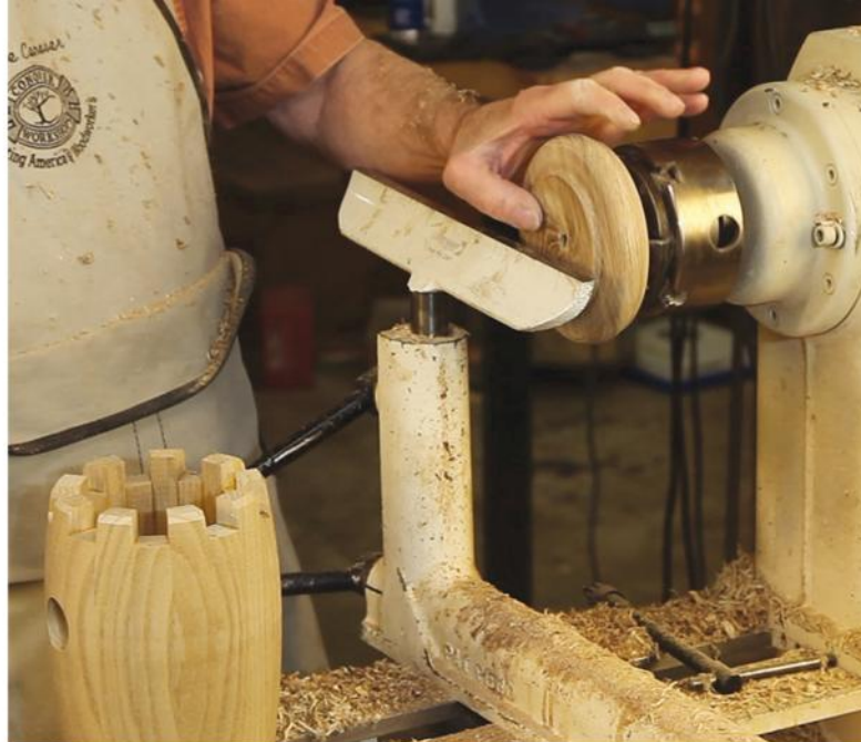
The floor is turned on a screw chuck. It has a tenon that loosely fits the inside of the walls and sports a 3/8"-wide bead on the outside.
