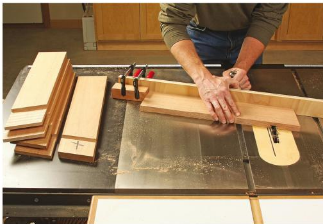
Cut angled half-lap joints on the back ends of the seat supports and seat backs. A long auxiliary fence attached to your table saw's miter gauge, and a clamped stop block, can help register the inside ends of these joinery cuts.
