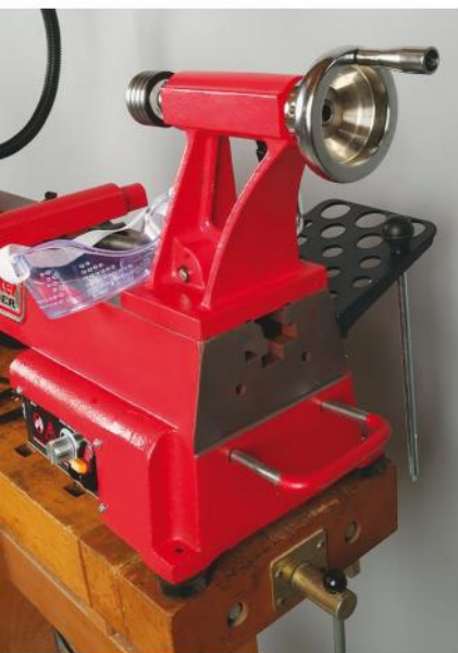
The lifting handles on the Turncrafter Commander made it easier to move on and off a bench.
