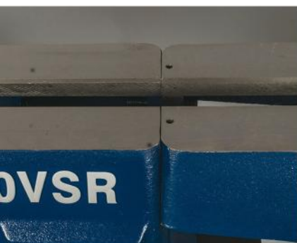
Two grub screws in RIKON's extension bed allow for easy alignment.
