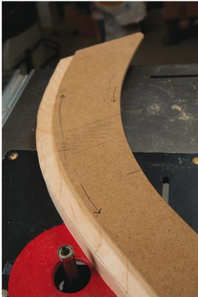
The sharp curves of these legs could chip out if you rout against the grain. Study the grain and mark your template with arrows.
