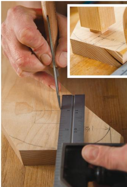
Mark a 1 1/8" x 1 1/8" mortise on all four legs to house the cart's two handles. Position these mortises 1 1/2" down from the top ends of the legs.
