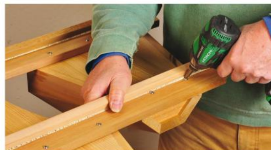
Washerhead screws driven through the back of the frame rails secure both the bottom and top of each planter box.
