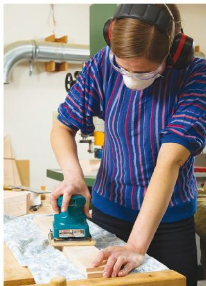
A thorough job of sanding will help your first coat of finish lie down more smoothly. Sand to 220-grit, as a general rule.
