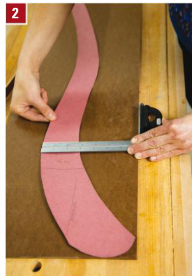
2 Position your paper pattern on the MDF using the dado layout lines to register it squarely. Trace the template and cut it out.
