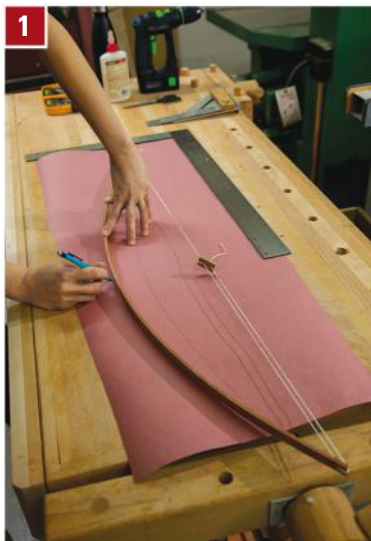
1 A flexible length of scrap and string formed a helpful curve bow when the author laid out the leg shape from scratch.
