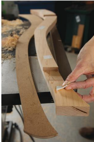
The author did some of her template routing on the legs with the template mounted on top, then taped it underneath to finish up.
