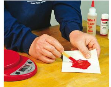
The next step is to add an equal amount of Part B to the colored Part A. A scale helps you be exact.
