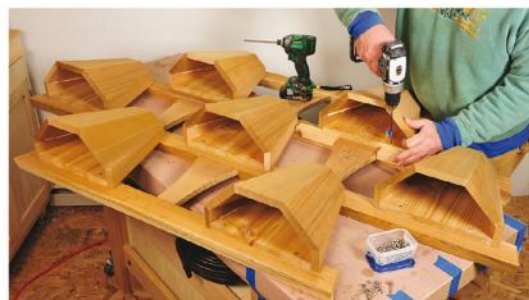
Stainless steel (the author's choice), brass or bronze screws are good options for this project; avoid regular zinc-plated screws, as they will rust.
