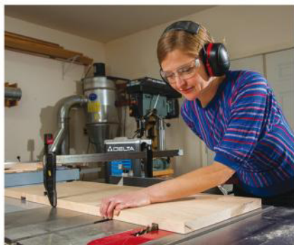
Mill pairs of dadoes across your leg blanks. Clamp the blanks to your miter gauge's fence to keep them from shifting laterally during cutting.
