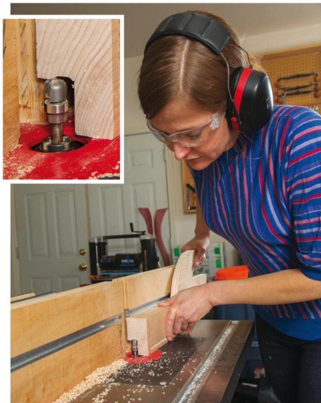
The author used a 1/4"-radius dish-carving bit with a shank-mounted bearing (inset) to form a finger recess in the top end of the rabbeted cutout on the top tray end pieces. Note: these end pieces still have flat faces.
