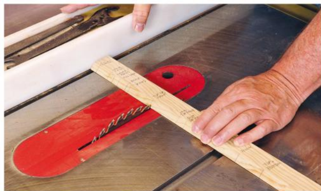
A story stick that identifies all crucial project measurements is especially great for setting table saw rip fences and fence stops on crosscut saws.
