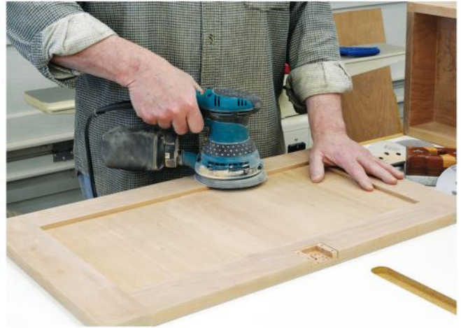
Give the completed door a good sanding, working your way up through the grits. Also, sand the center stile flush with the panels.
