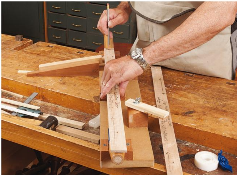
For his drilling fixture, the author glued V blocks to a base and secured them with drywall screws through a hole at the edge. The clamping arms are secured with 1/4"-20 threaded rod epoxied into the block.
