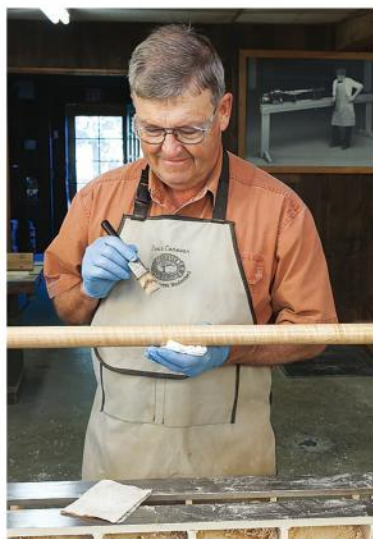
If you've chosen a clear finish, it is easiest to apply several coats in the lathe.
