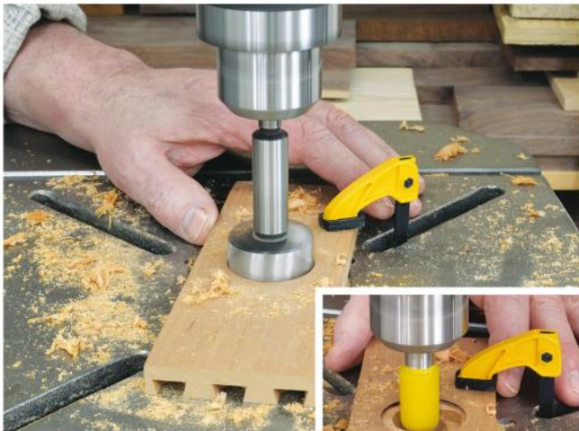
A large Forstner bit makes the initial round mortise for the flush pull. Do a test cut in scrap, and set the drill press depth stop appropriately. Finish the drawer front mortise by rounding out the bottom to accept the rounded back of the flush pull.
