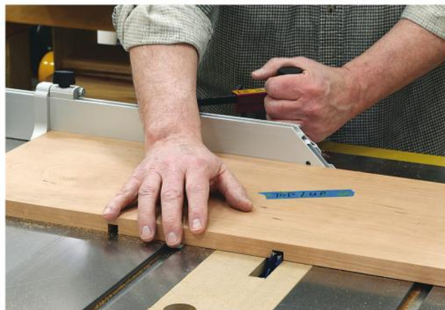
The 1/2" sides of the center module go into 3/8" x 1/2" dados cut into the inside faces of the desk top and bottom components.
