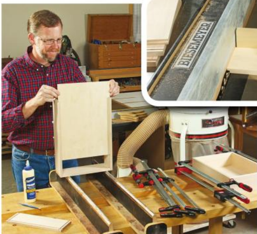
These light-duty drawers have rabbet-and-dado corner joints made at the table saw with a dado set (see inset).
