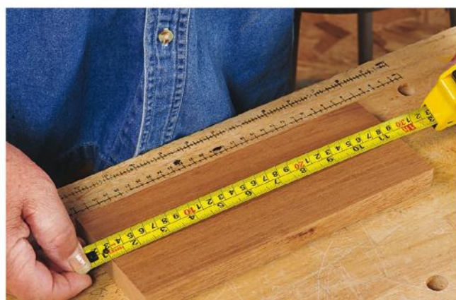
The "classic" method to avoid inaccuracy caused by a tape measure's sliding end stop is to measure by aligning the 1" mark with one edge of the workpiece, then add one inch to the resulting measurement.
