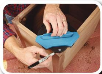
Trace the large outer corner radii of the carcass with a template or a compass, then shape them with a spokeshave. It's easy and enjoyable hand tool work.
