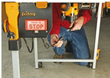
An onboard power switch plugs into both a wall outlet and power tools, to give you easy on/off control from the Workcentre's infeed end.
