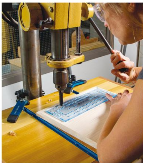
Double-sided tape keeps the template secure during the drilling process. The author recommends frequently cleaning the chips from the drill bit.
