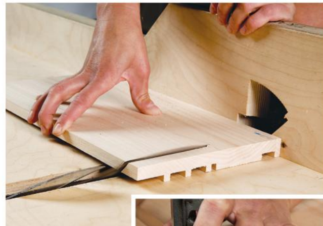
The author marked the game box's corner miters to 45°, using the chessboard top as a reference (inset). She cut the miters on a crosscut sled for best control and accuracy.
