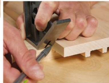
The author marked the game box's corner miters to 45°, using the chessboard top as a reference (inset). She cut the miters on a crosscut sled for best control and accuracy.
