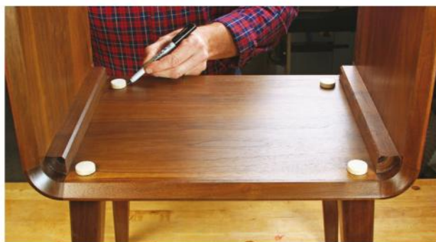
A chamfer around the carcass face reduces its perimeter edge to a thin, clean detail. Several deepening passes help to avoid bit burn marks.
