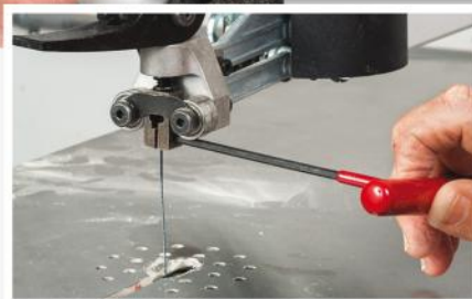
In assessing the JET 22" Scroll Saw's blade change capabilities, the author used features like a built-in wrench (left photo, above), a cam lever that secures and tensions the blade (right photo, above) and set screws for the upper clamp (photo at right).
