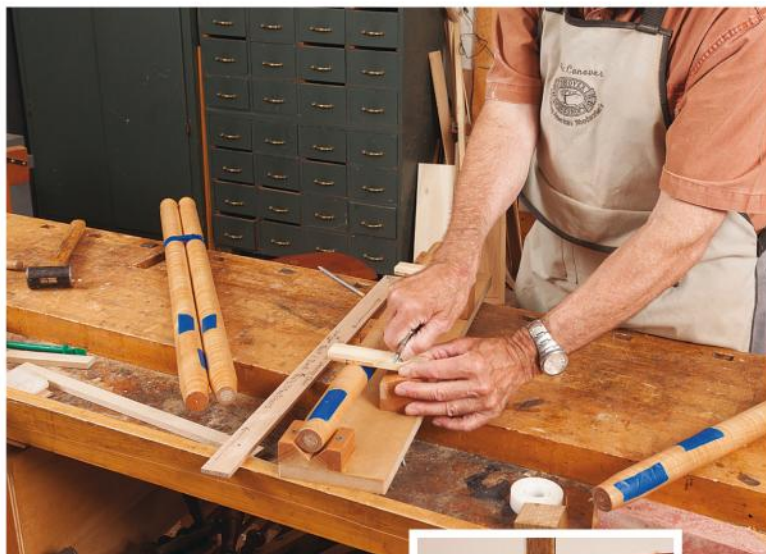
Locating the borings that will accept the tenons of the stretchers and rails is key to this project. The author bundles a group of four legs for each chair as he marks them. To do this accurately, he created a fixture to aid both marking and drilling. (See the next page.)
