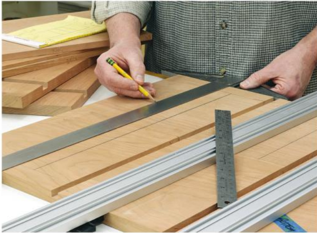
Clamp up component pairs with inside faces upward, then pencil in guide-lines for routing dados for the dividers. A T-square ensures accuracy.
