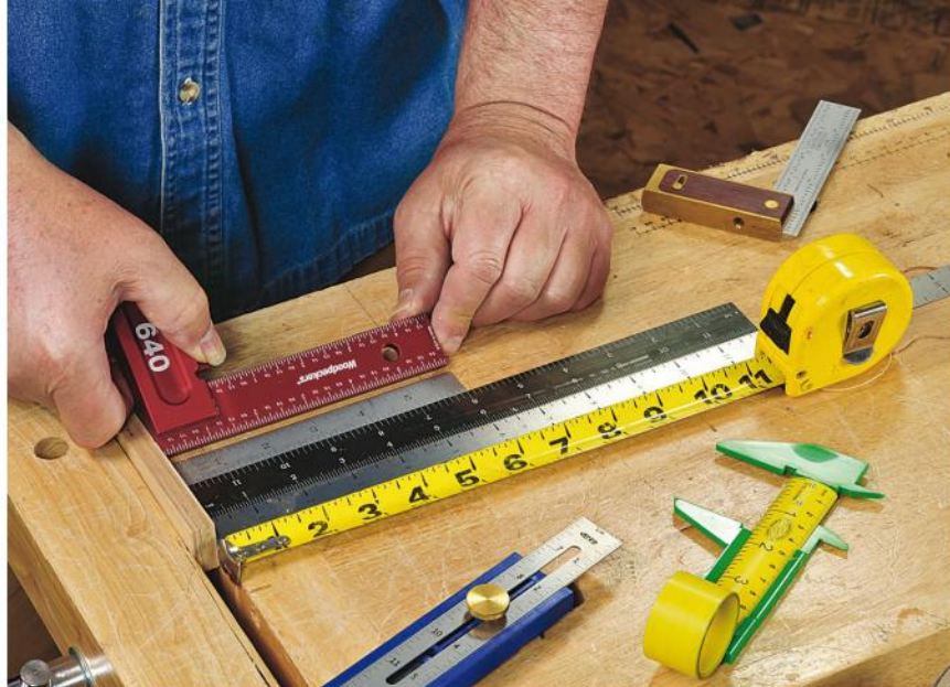
Think the graduations on the scales of your measuring tools all match perfectly? A comparison test will reveal that's not necessarily the case.
