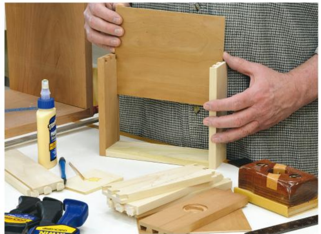
Assemble the two drawers, check for square, and clamp up till dry. In the modern drawer fitting technique, you slide the bottom into a groove cut in the four sides, then attach the final drawer side.
