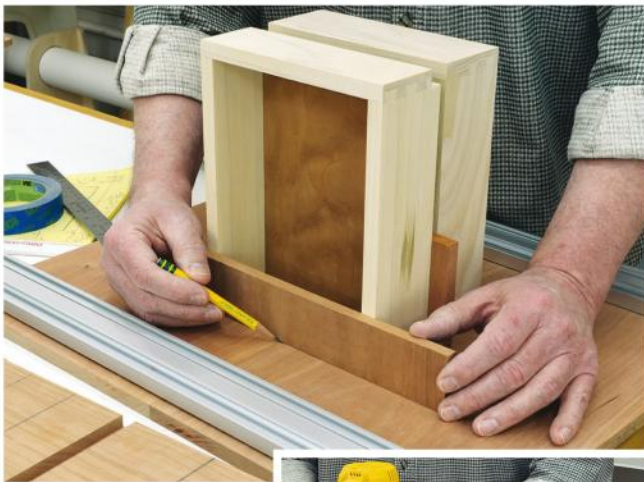
To set up the locations for the dados for the drawer openings, it's easiest to use the drawers themselves as a guide. Note here that the author uses scrap of the same thickness as the drawer shelves as spacers. With the drawer module sides clamped edge-to-edge, rout the dados for the drawer shelves. The clamps not only hold the workpieces together, but are also placed to act as guides for the router.
