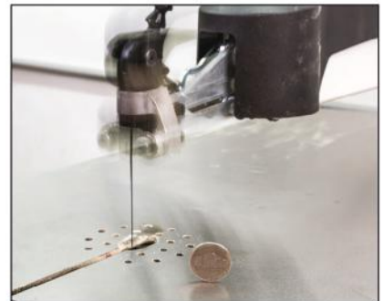
The author's "nickel test" gave her feedback on the scroll saw's vibration.
