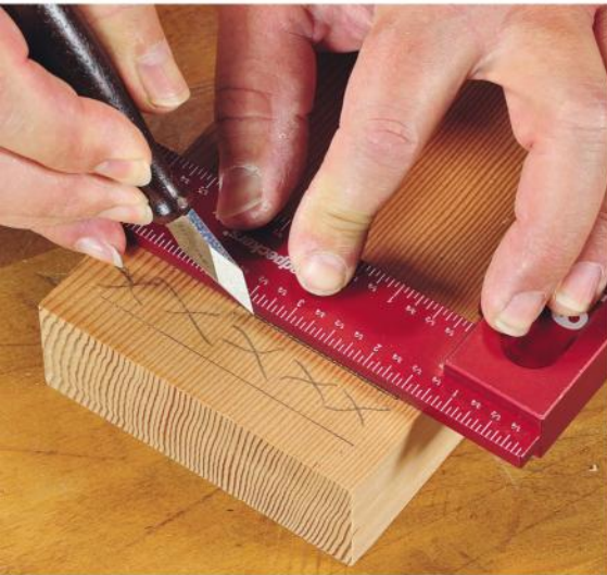
Marking identical joinery across a blank allows you to gang-cut parts with the same dimension.
