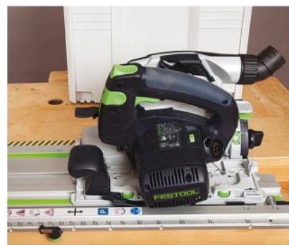
Move the left button under the track to one of the notches calibrated to specific degrees, for exact angle cuts.
