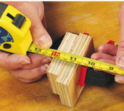
Ganging parts and subtracting their thickness from the length of what you're building can yield lengths of adjacent parts.
