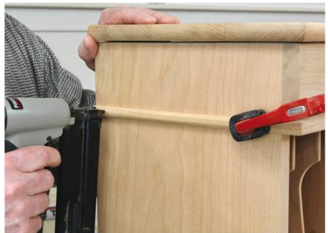
The front trim can be glued into place, since wood movement isn't an issue, but nail on the side trim to account for the cross-grain situation here.
