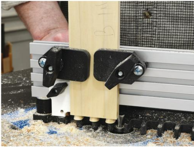
A router table dovetail jig makes fast work of the half-blind drawer dovetails. Although not visible, the drawer front is cut at the same time.
