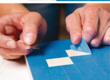
The author used finishing expert Michael Dresdner's process of masking off with tape (see page 82) in order to create the chessboard squares with spray paint.
