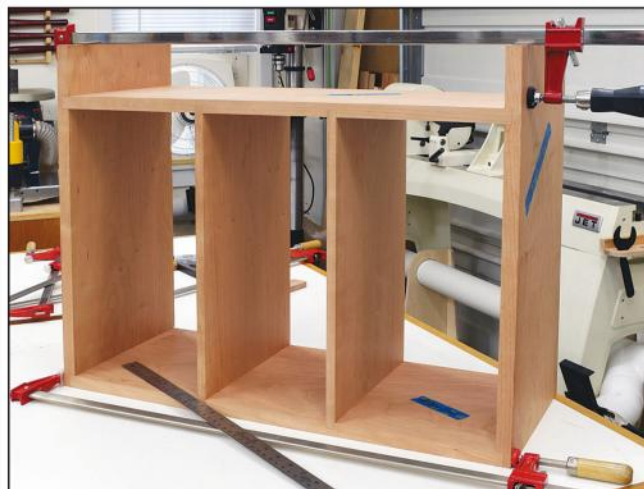
With all rabbets and dados cut, do a dry assembly of the carcass to check all the case joinery.
