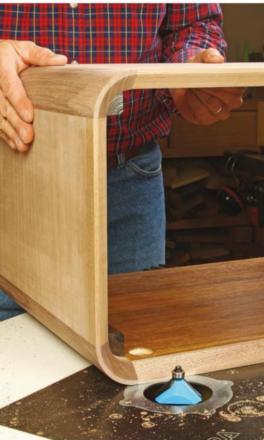
A chamfer around the carcass face reduces its perimeter edge to a thin, clean detail. Several deepening passes help to avoid bit burn marks.
