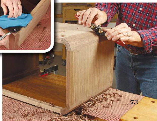
Trace the large outer corner radii of the carcass with a template or a compass, then shape them with a spokeshave. It's easy and enjoyable hand tool work.
