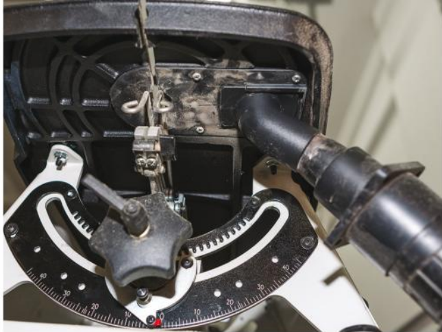
The author used an extra hose fitting (not shown) to reduce suction from the dust collection feature and allow her workpiece to move more freely.
