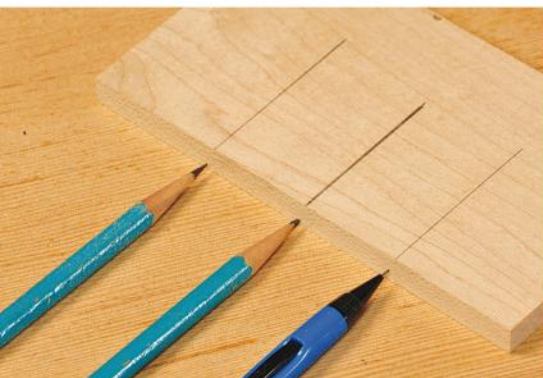
Unless regularly sharpened fastidiously, wood pencils draw a line that gets thicker with each use. A mechanical pencil's line has a fixed width.
