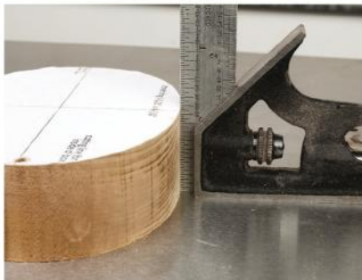
The author used an oval box as a test. The saw cut sides that were absolutely vertical.
