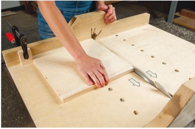
A crosscut sled and clamped stop block ensure that project parts can be cut to lengths that match one another exactly.
