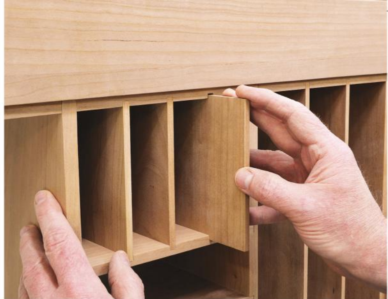
Once carcass assembly is done, give each of the dividers a test fit. Too tight? Ease the fit with a sanding block.
