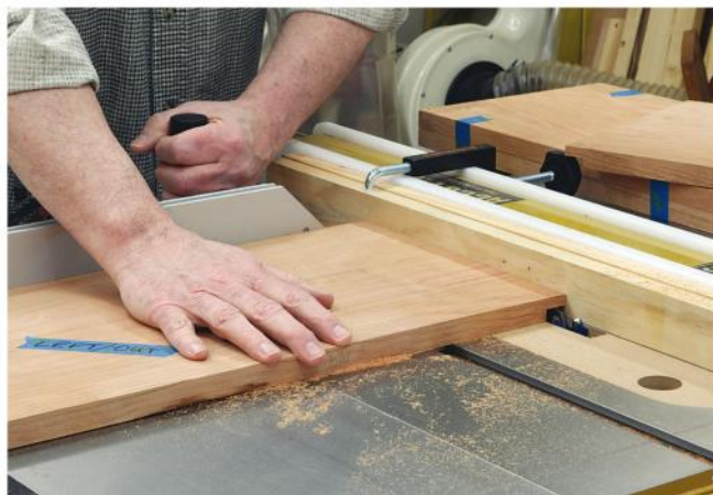
The two sides receive a 3/8"-deep x 3/4"-wide rabbet on the inside bottom edges, and a 3/8"-deep x 3/4"-wide dado 3" from the top.
