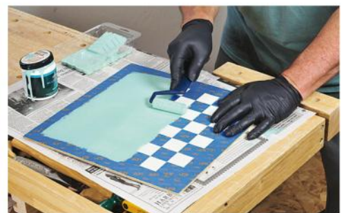
Miniature paint rollers actually work better than brushes on masked surfaces, since they apply paint more evenly and don't scrape across the tape dam.
