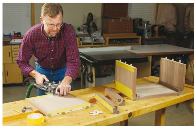
The author used Festool's Domino system to create loose-tenon joints for assembling the nightstand's carcass panels and corner blocking. Biscuits or dowel joints are suitable options, too.
