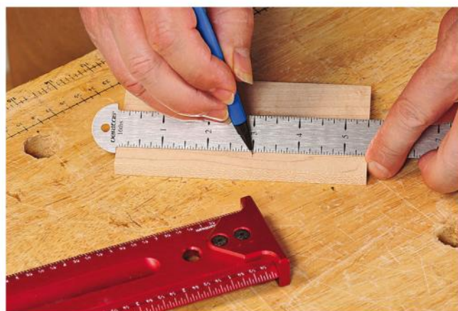
A hook rule's hook precisely aligns zero with the end of the workpiece.
