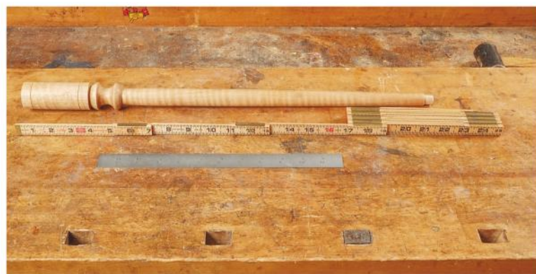
Turn an example of the piece to be the master part. Take measurements for all the turnings from this part, and compare them often. The author prefers wood folding rulers or steel rulers over steel tapes for laying out turnings.
