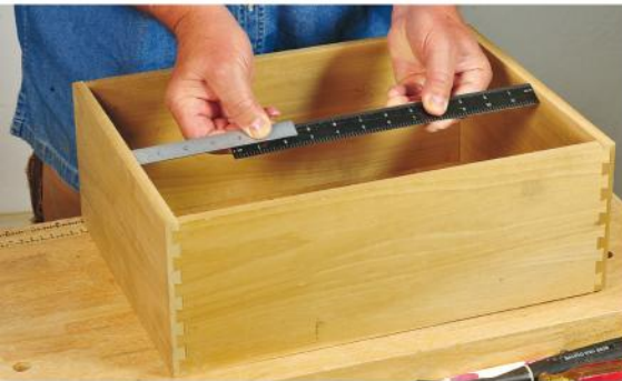
Take an inside measurement with two rules: the measurement equals one rule's full length plus the amount a second rule extends past it.
