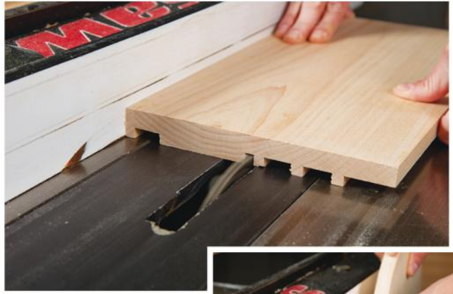
When cutting dados, make sure to hold the workpiece flat against the saw table. On narrow parts, such as shown in the inset photo, use a push stick to keep your fingers clear of the blade.
