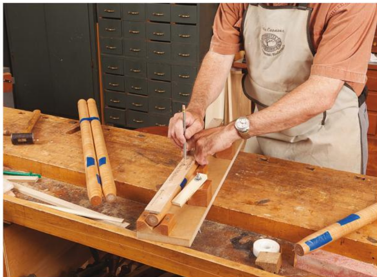
It is worth making some story sticks, even for one chair. By making the story sticks 1 1/16" wide, it is easy to center them on the 1 1/2"-dia. legs.
