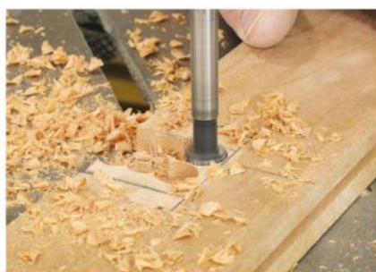
Use a small Forstner bit to clear out most of the waste from the inside of the secondary mortise. Be sure to set the drill press depth stop.
