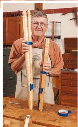
Locating the borings that will accept the tenons of the stretchers and rails is key to this project. The author bundles a group of four legs for each chair as he marks them. To do this accurately, he created a fixture to aid both marking and drilling. (See the next page.)
