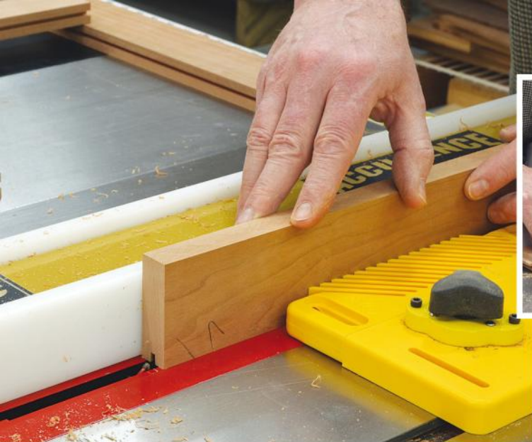
Cut the 1/4"-deep grooves for the frame-and-panel door on the table saw.
