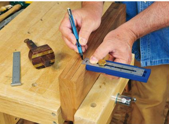
The Kreg Multi-Mark's built-in rule makes it easy to set precisely for marking out joinery, rabbets, hardware mounts, etc.
