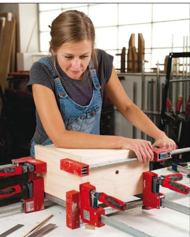
If the game box parts are cut carefully and accurately, gluing and clamping them together at once will be easy work with enough clamps.
