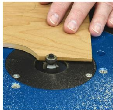
Cut out the profile of the tall dividers on the band saw as here, or with a jigsaw or scroll saw. Round over the straight edges on the fronts of the tall dividers. The short dividers also have their front edges rounded over.
