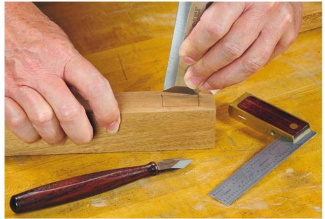
A knife line makes it easier to register the tip of a chisel (or tooth of a hand saw) to the marked line when you're ready to cut the part.
