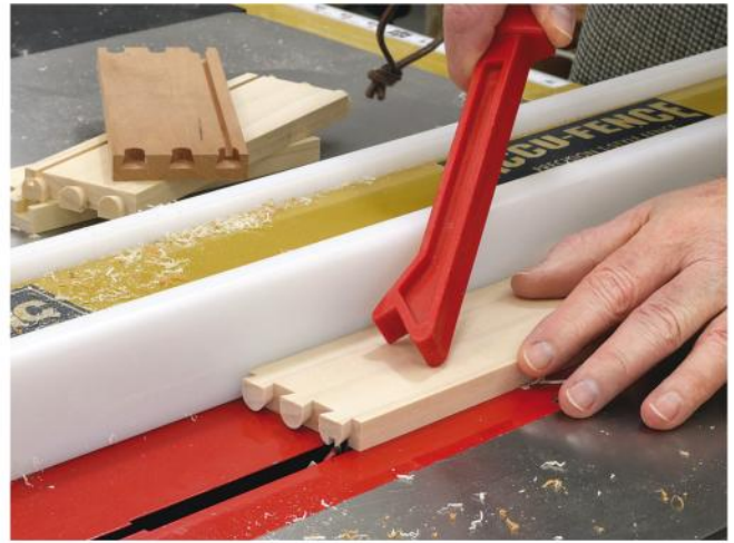
Cut the grooves for the drawer bottoms so they fall within the bottom tail. Once assembled, the groove will be invisible.
