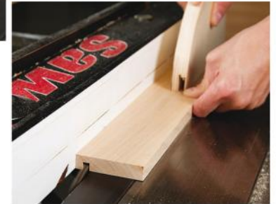
When cutting dados, make sure to hold the workpiece flat against the saw table. On narrow parts, such as shown in the inset photo, use a push stick to keep your fingers clear of the blade.
