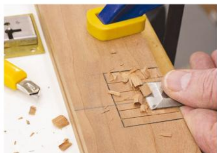
With the top rail clamped to your work surface, create the initial mortise for the desk lock.
