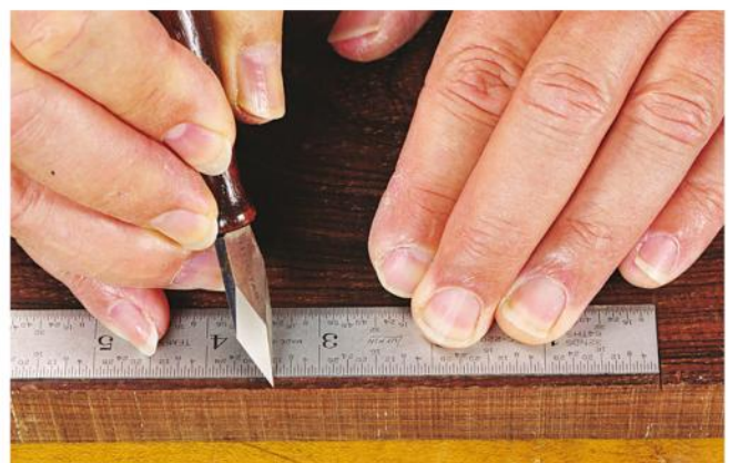
Use a quality rule with machine-cut (not just photo-etched) graduations to make dead-on precise knife marks.
