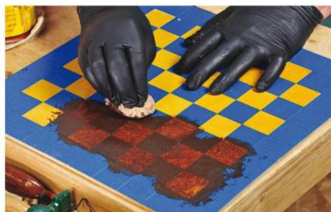
Using stain? Daub instead of scrubbing or wiping, if possible. Here, the author is using a dark pigment stain. Note that the borders are masked.
