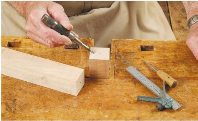
Find exact center with a center finder and a scribe (don't use a pencil, it is not as accurate) and center punch for accurate centering. This will give consistent major diameters just by turning.
