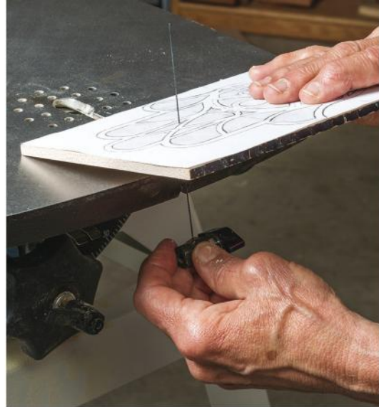
A spring-loaded arm provides easy access to the underside of projects like fretwork.
