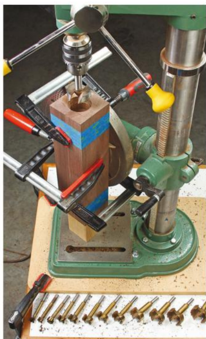
Drilling deep holes into the end grain of the corner block bundle is tough going. Work up in bit sizes if you have a modest drill press like this.
