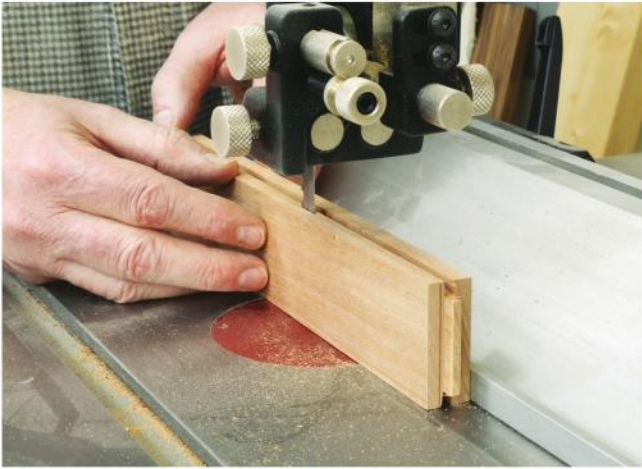
Resaw most of the back side of the center stile on the band saw, then follow up with a hand plane and/or sander.
