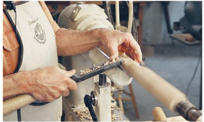
By lightly touching your fingers to the back of the work, you can sense when the spindle is just round with no flat spots. This technique creates a consistent diameter without the use of calipers.
