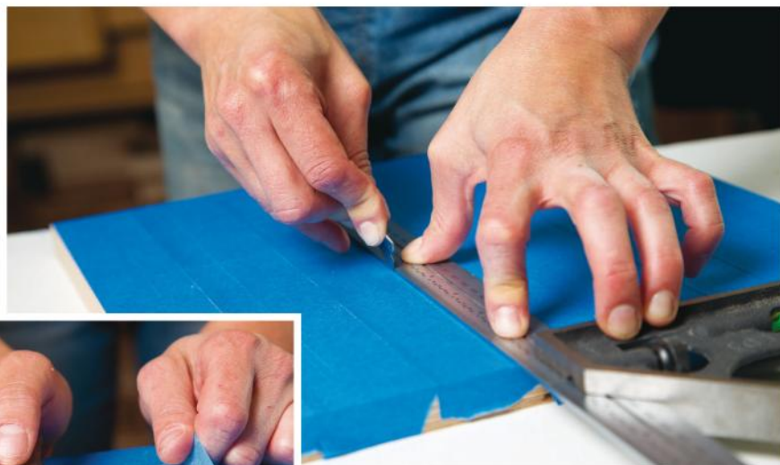
The author used finishing expert Michael Dresdner's process of masking off with tape (see page 82) in order to create the chessboard squares with spray paint.
