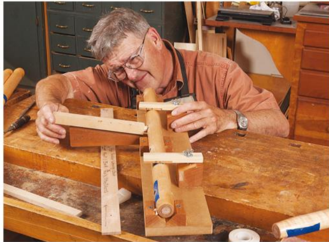
For his drilling fixture, the author glued V blocks to a base and secured them with drywall screws through a hole at the edge. The clamping arms are secured with 1/4"-20 threaded rod epoxied into the block.
