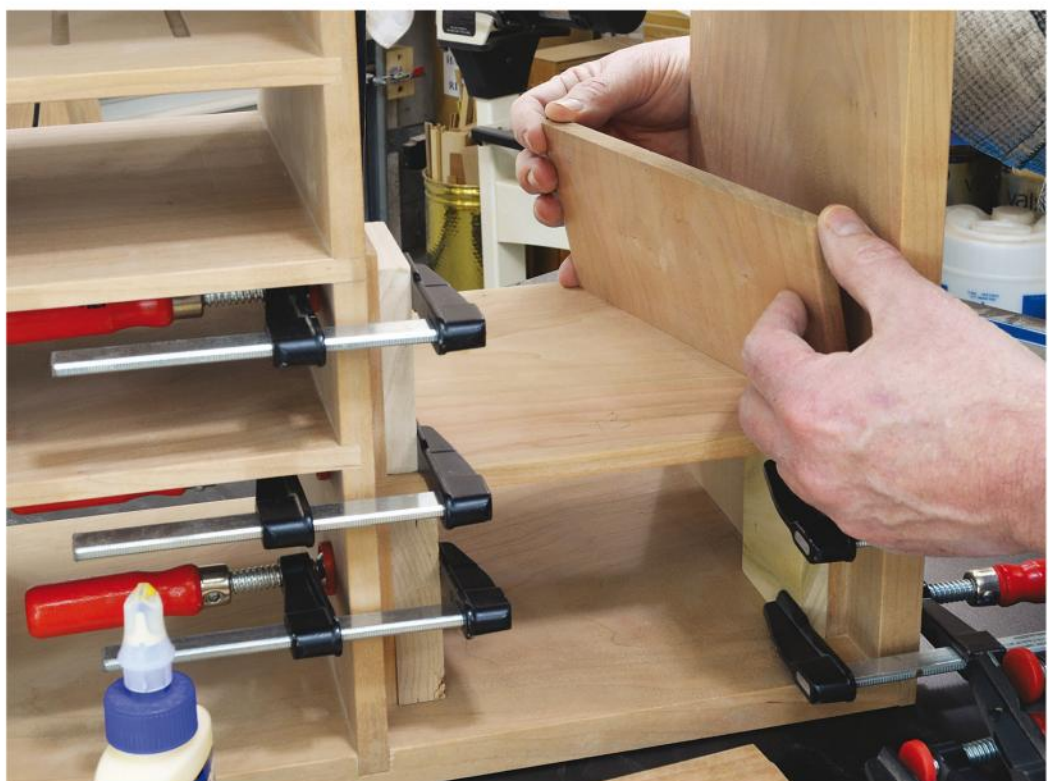
Creating the "shelf stack" is simply a matter of gluing and stacking the shelves and side pieces. Start by gluing the two bottom side pieces in place. Top with the first shelf and follow with the next set of sides.
