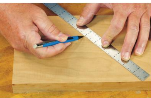
To divide a workpiece into equal thirds, slant a rule so 0 is at one edge of the piece and 9" at the other, then mark the 3" and 6" points.
