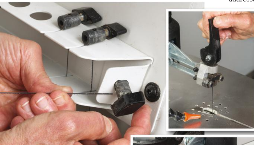
In assessing the JET 22" Scroll Saw's blade change capabilities, the author used features like a built-in wrench (left photo, above), a cam lever that secures and tensions the blade (right photo, above) and set screws for the upper clamp (photo at right).
