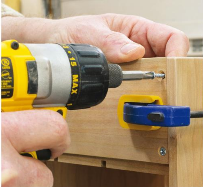
Glue and screw the back of the upper storage compartment into place. This creates a rabbet underneath that will later accept the desk back.
