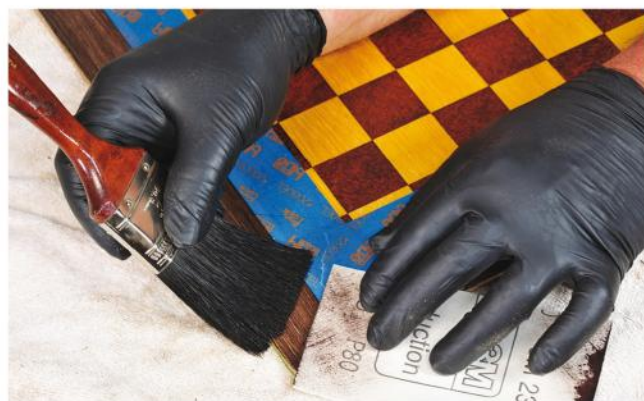
To create a "faux miter," lay a piece of 80-grit sandpaper at 45° on the corner, grit side down. Start with the bristles on the paper and drag the brush away from it, through the stain.
