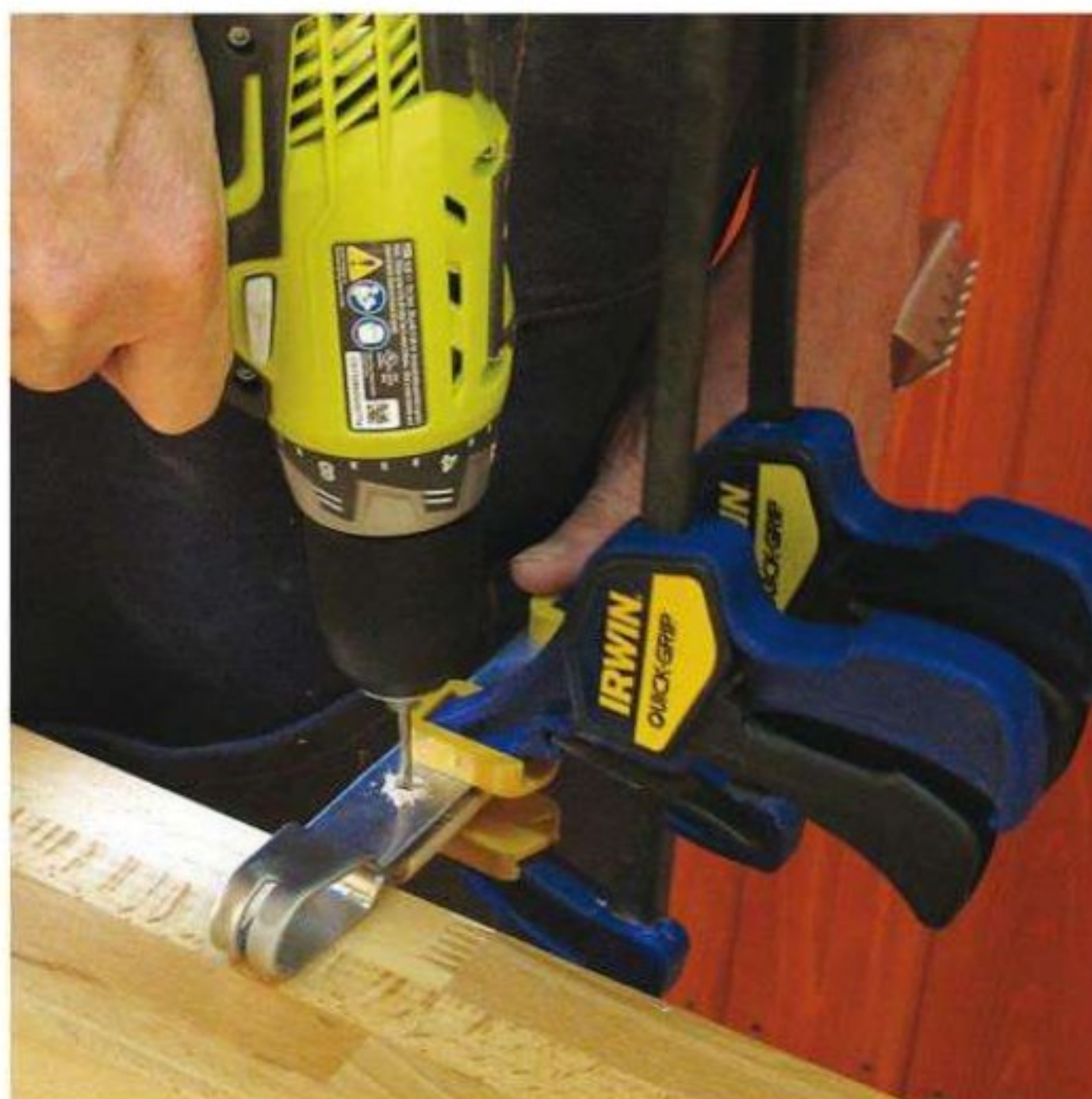
After the epoxy has cured, drill the pin holes through the handle using the predrilled holes in the tongs as a guide (keep it clamped as you do).
