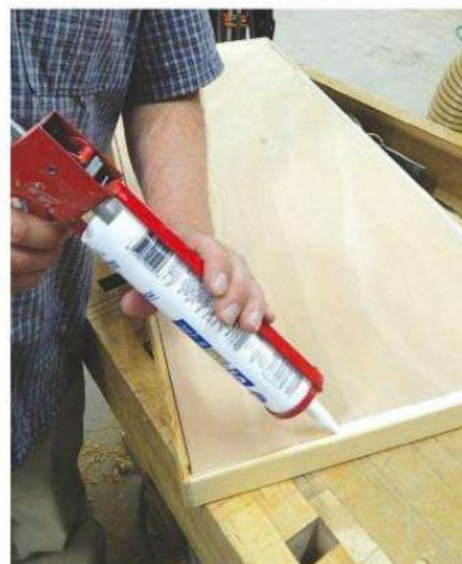
Seal any gaps around the lid frame and panel with a thick bead silicone caulk, for added insurance against leaks or insect pests.
