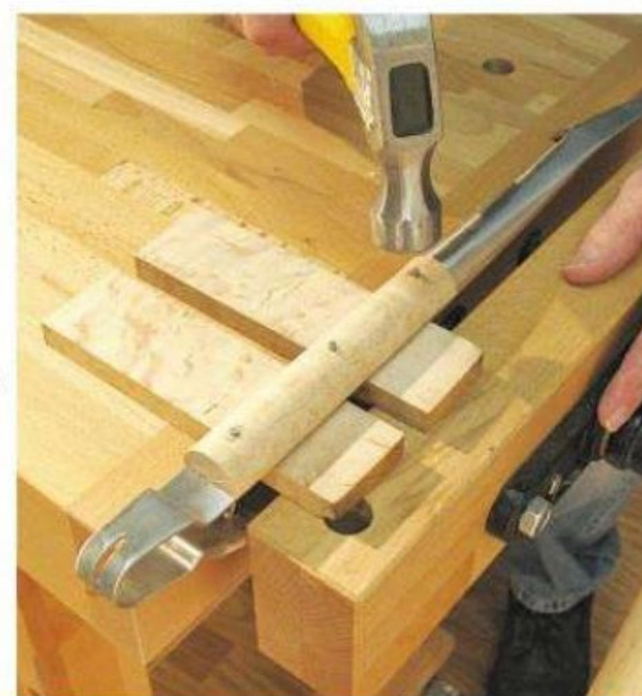
Drive the pins into their holes and then file them flush to the wood surface. Now sand and apply finish, and the tongs are ready to go to work.
