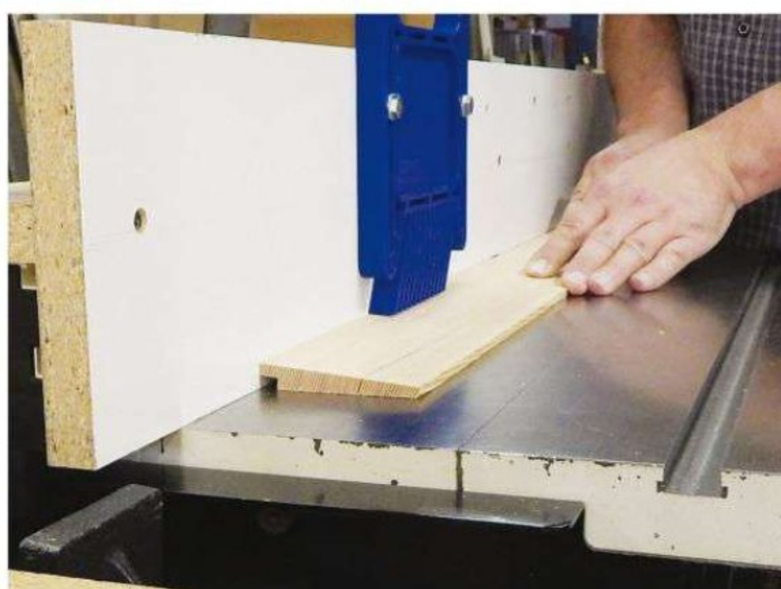
Start the roof lap-siding by making a tilted resaw cut at the band saw to form two siding pieces (left). Trim the bottom edges at the table saw to square them up again, then rabbet them to form lap joints with a dado blade tipped to 85°.
