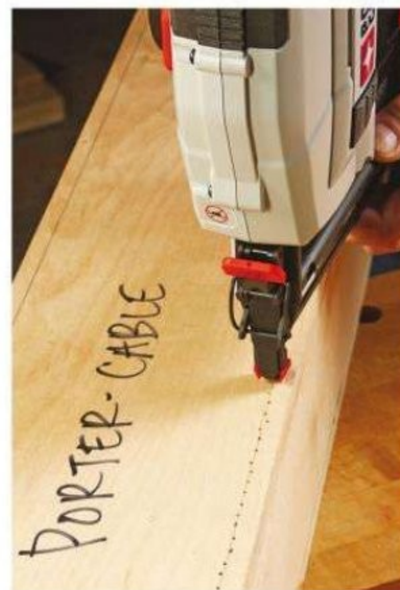
PORTER-CABLE's front-oriented nailing tip made it easy to sight and sink brads along a pencil line. The contact element is behind it.
