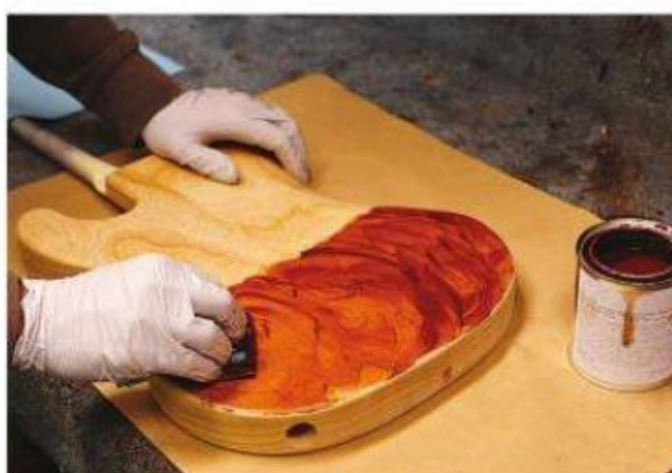
You need pore filler for open pore wood or exposed end grain to prevent visible defects on your guitar.
