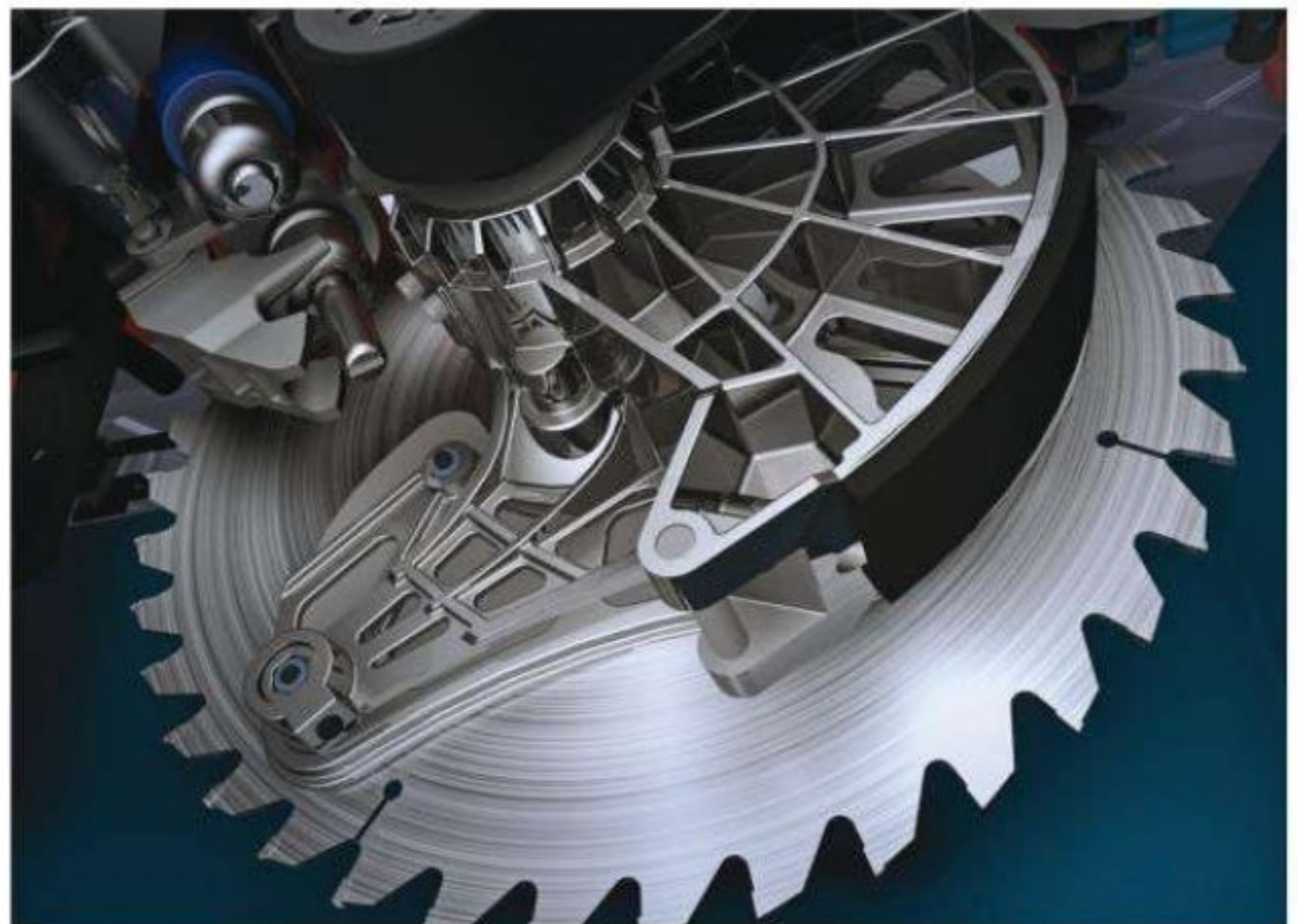
When the saw's computer detects that the blade has contacted skin during use, the cartridge drives the arbor below the table at a high rate of speed.
