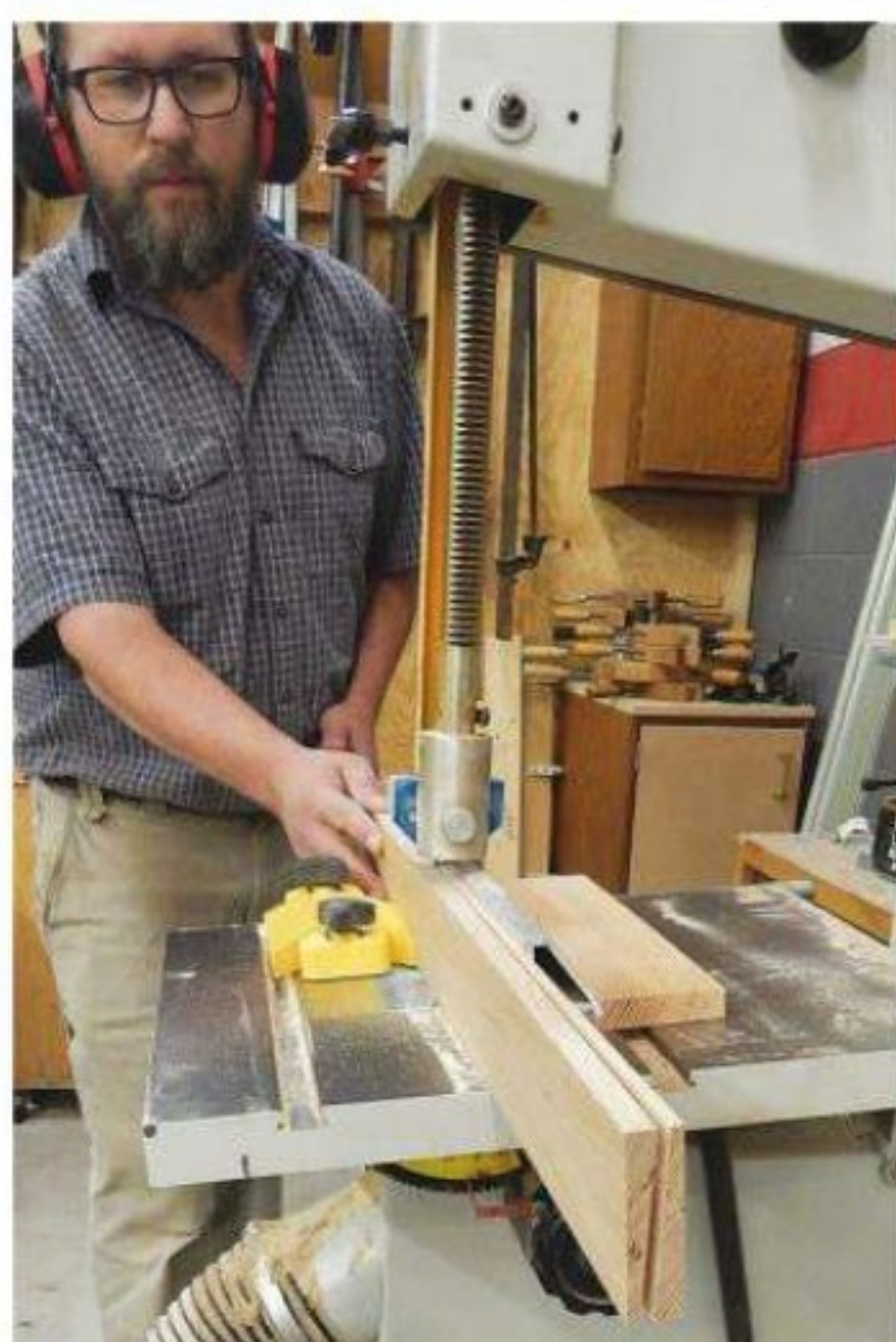
Start the roof lap-siding by making a tilted resaw cut at the band saw to form two siding pieces (left). Trim the bottom edges at the table saw to square them up again, then rabbet them to form lap joints with a dado blade tipped to 85°.
