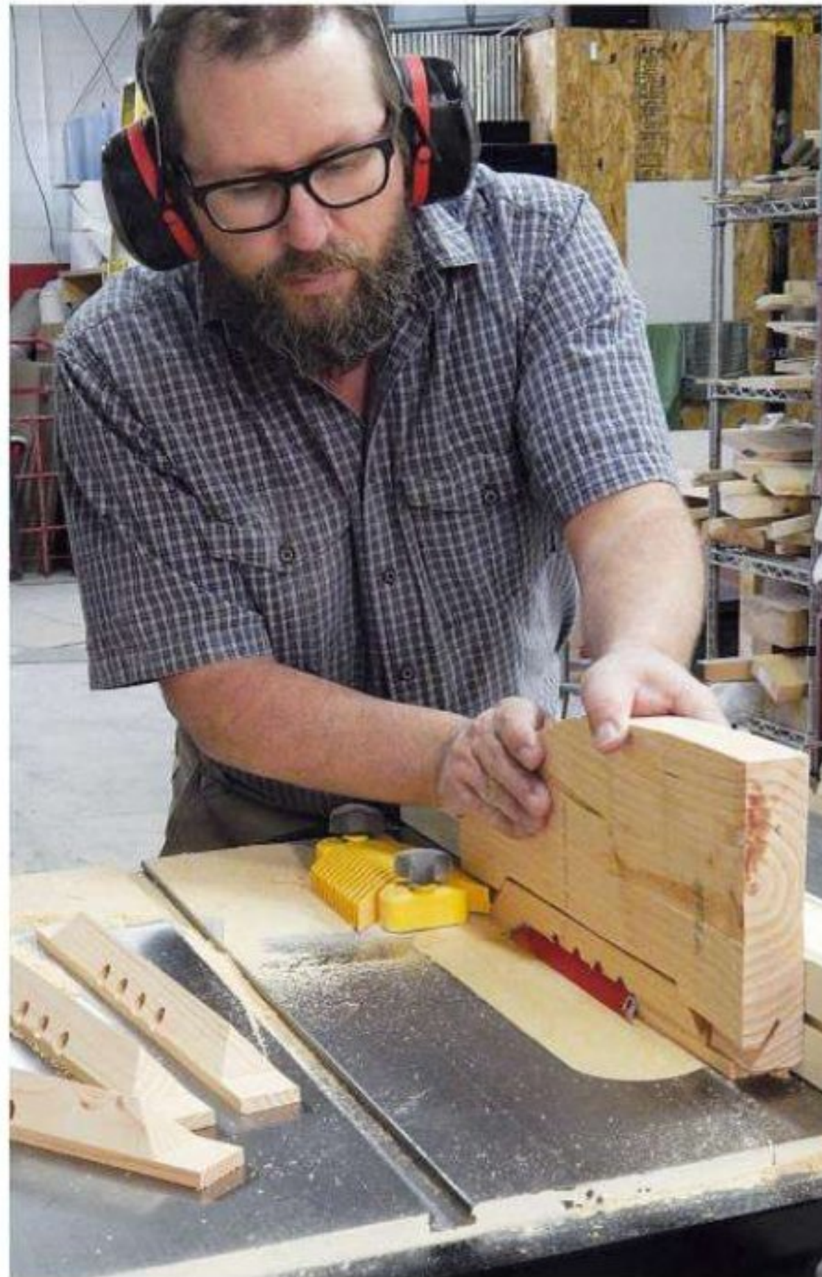
To create the long beveled edges on the top bars, the author used a special push block that fits around the top bar blanks and holds their lapped ends down against the saw table. It has a cutout area in the middle to accommodate the taller part of the upturned bars. Two cuts, with the saw blade tipped to 55½° and passing through a zero-clearance throatplate, did the job.
