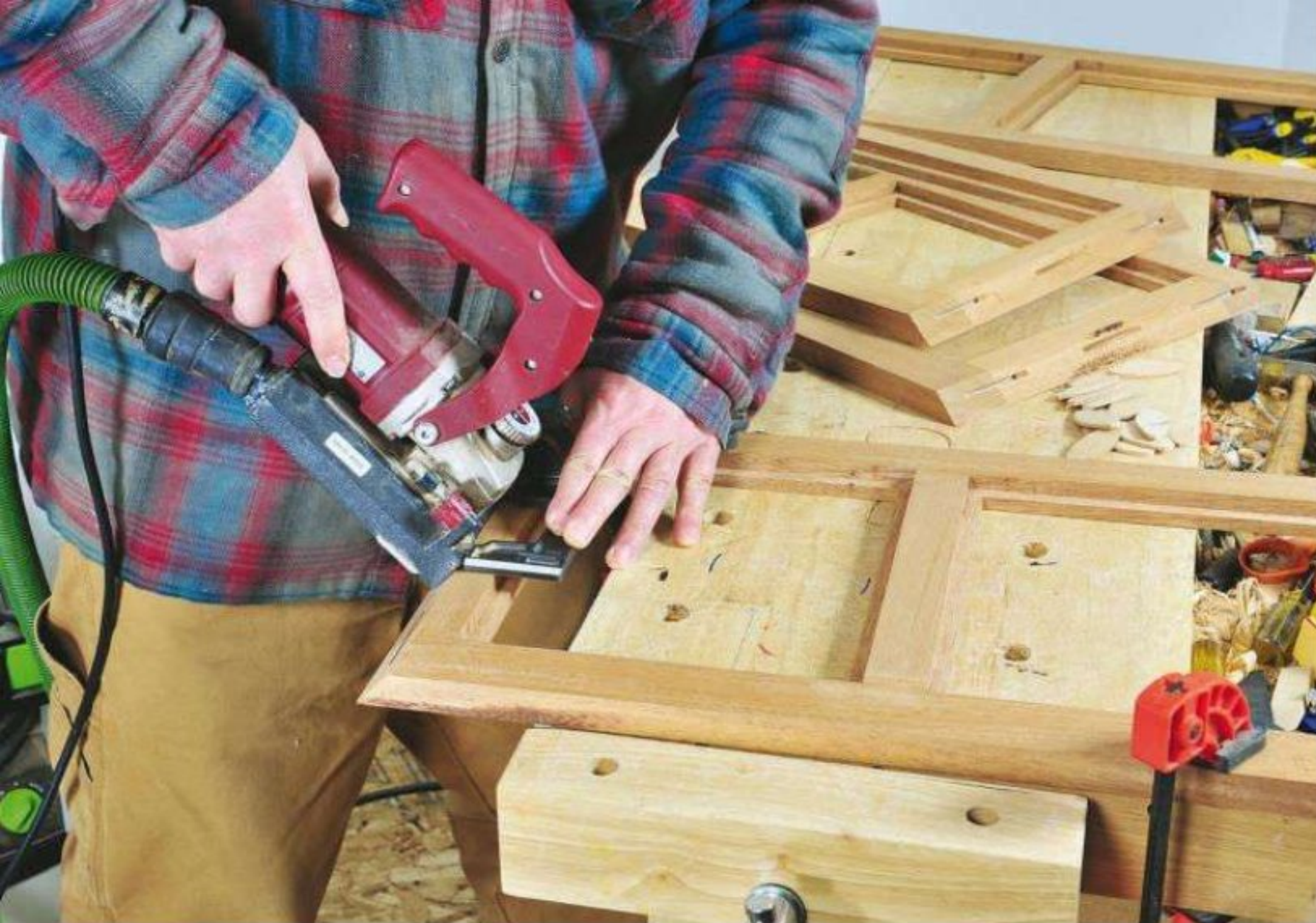
A biscuit joiner with the fence tilted to 45° cuts slots in the beveled ends of the frames for the #20 plate joinery biscuits that will join the sub-assembled frames together to form the ottoman's carcass.
