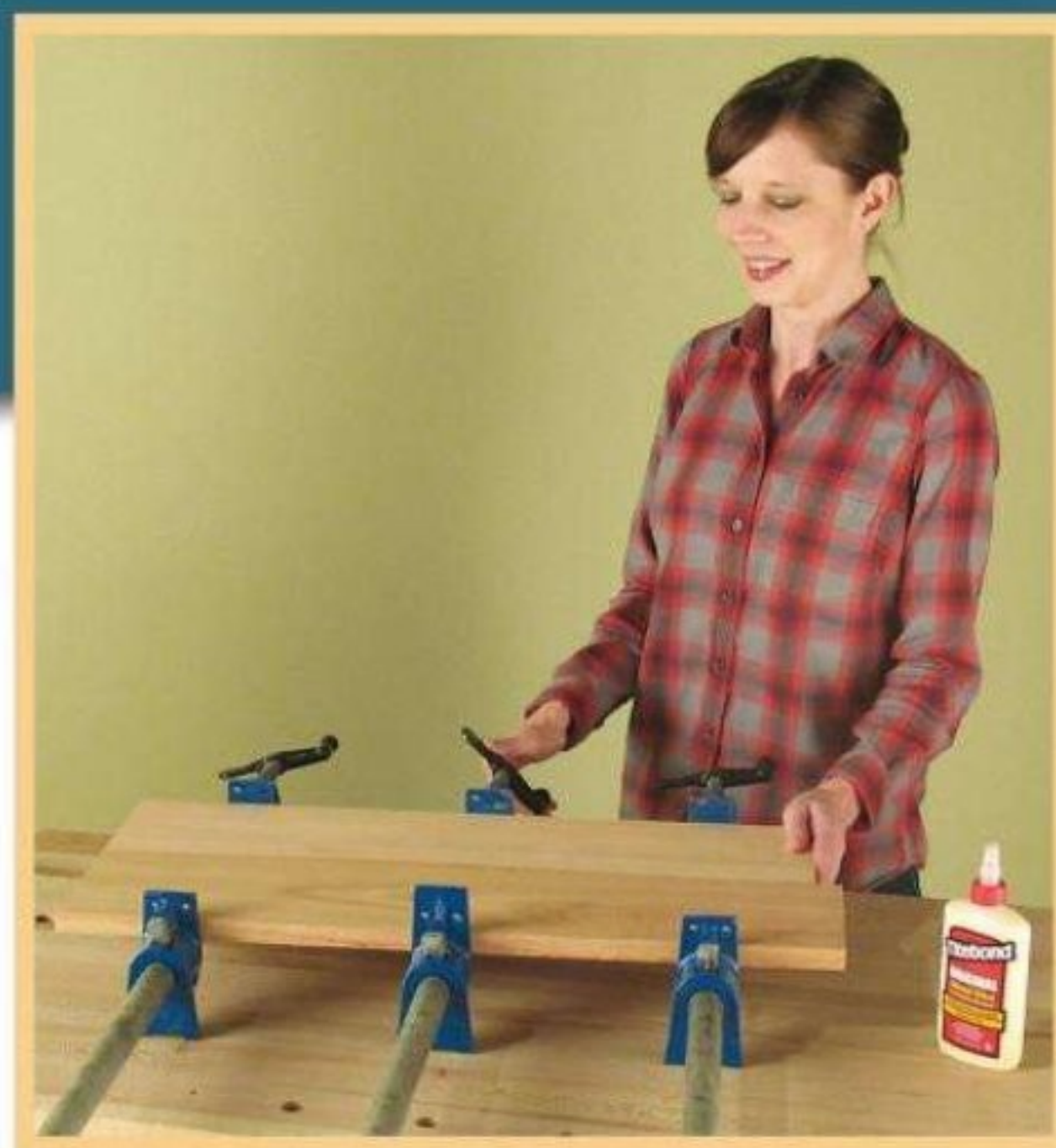
Gluing up enough 10"-wide stock for the main shelf components is the first step in the process. You'll need three wide pieces.
