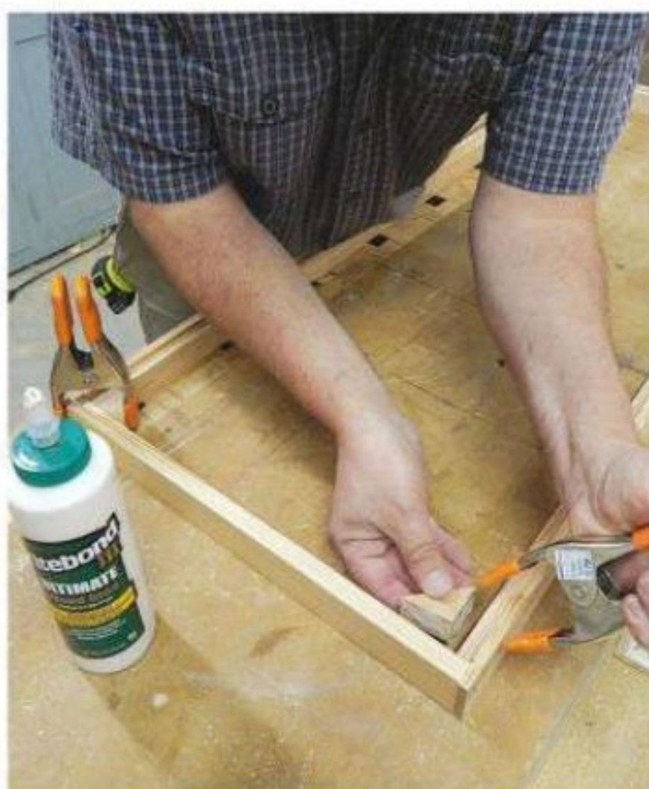
Assemble the lid frame and corner blocks with glue, screws and clamps. These blocks fit around the hive handles so the lid rests flat.
