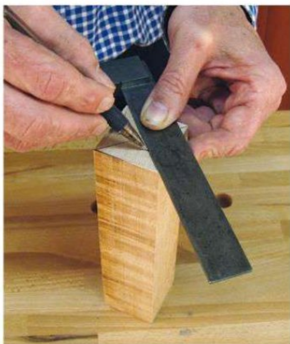
After squaring the ends of the blank to each other, mark the exact center of both ends. To do so, just draw an X from corner to corner.
