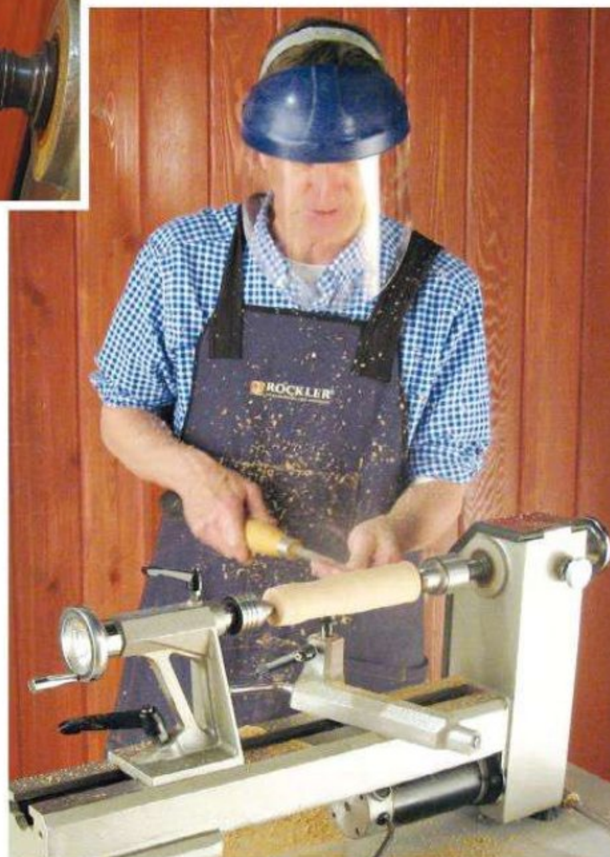
Once the blank has been threaded onto the lathe mandrel (inset), it is time to rough it round and then shape the handle to suit your needs and to please your eye. Let creativity be your guide.
