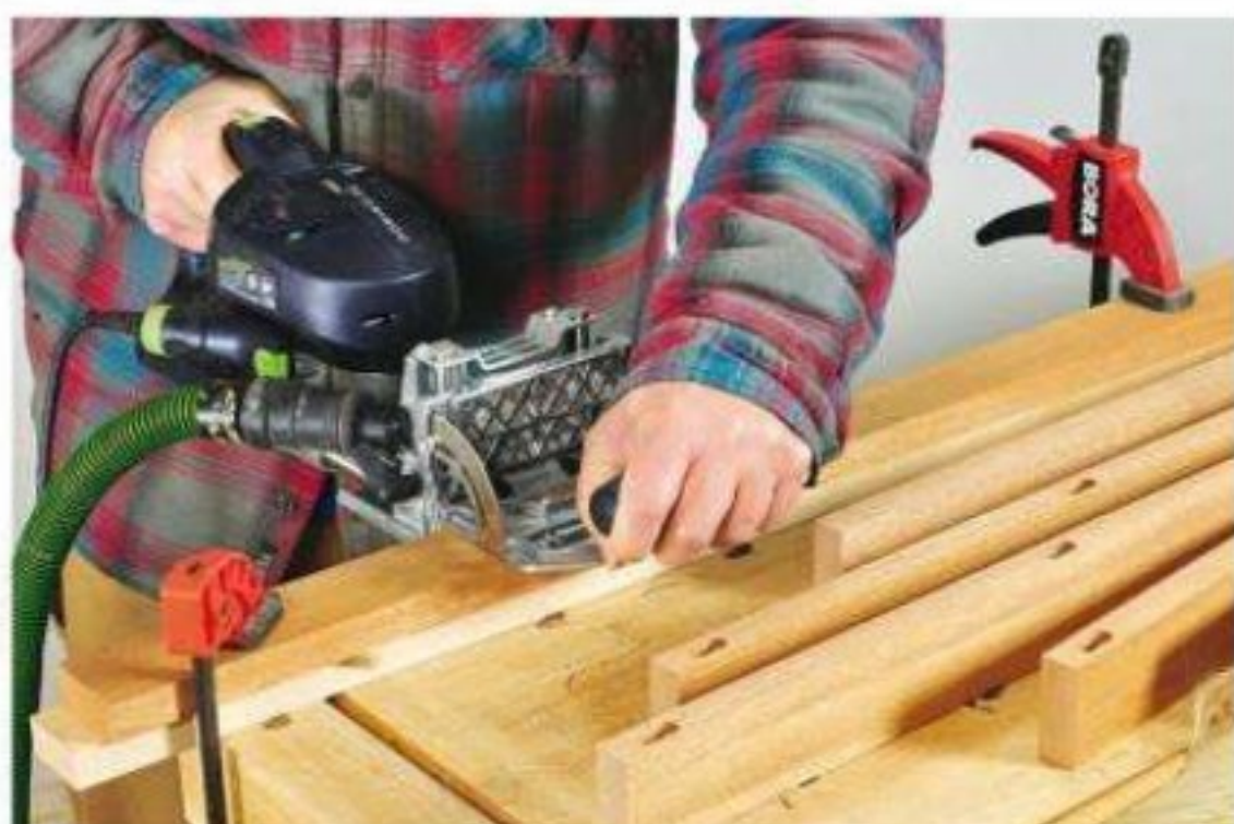
The author uses the Festool Domino system loose tenons to join the frame members of the ottoman.
