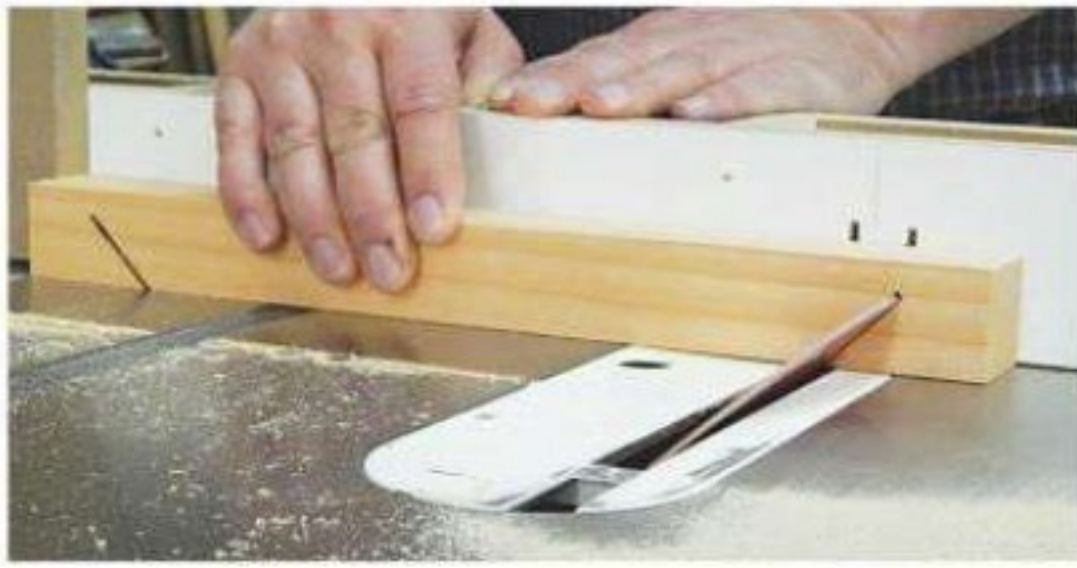
Cut the non-through end angles on the top bars at the table saw. Use your miter gauge and a stop block to control these cuts. Tilt the saw blade to 45°.
