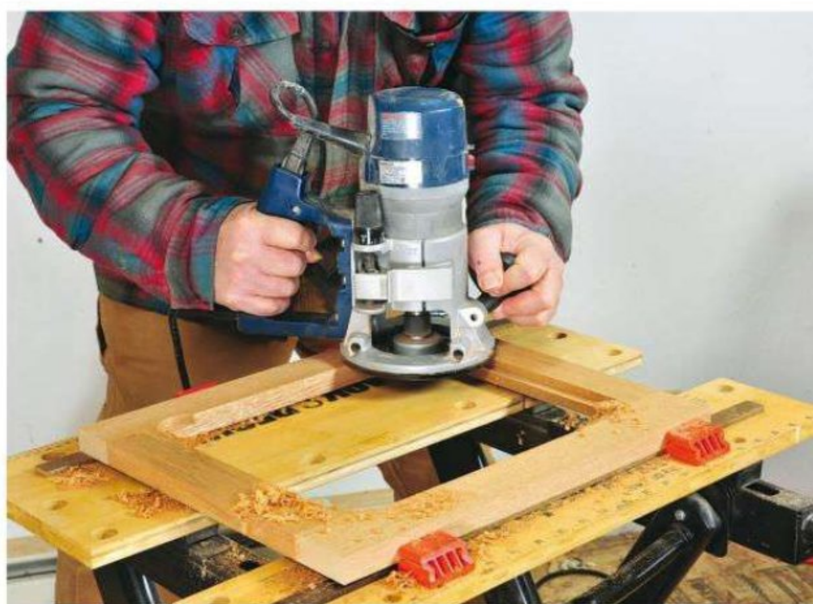
Rout the inside edges of a frame opening with a piloted rabbet bit.
