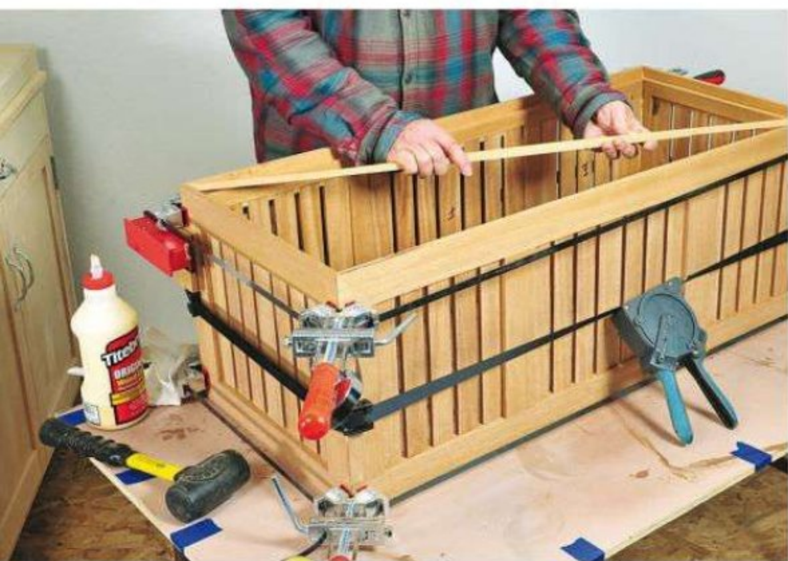
Band clamps hold the frame subassemblies together during glue-up.
