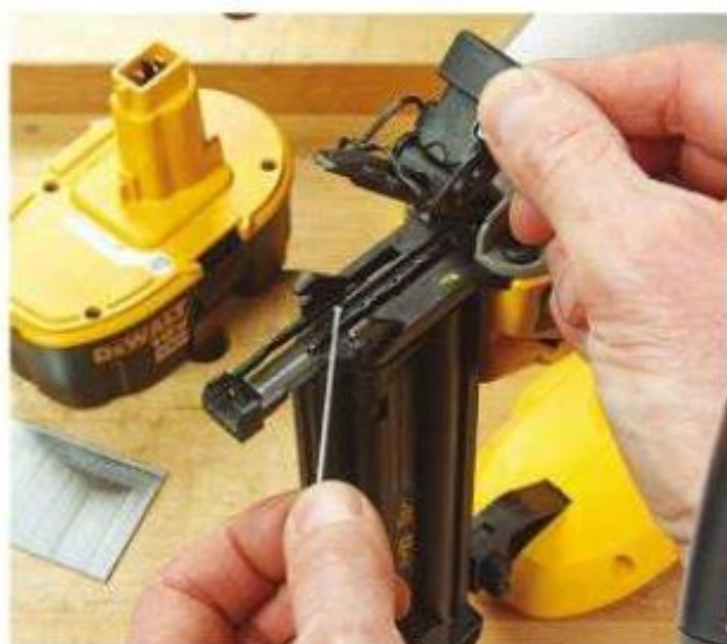
Flipping a lever releases the nose cover on this DeWALT and several other nailers for clearing jams.
