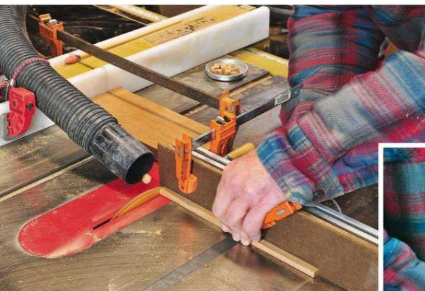
A shop vacuum hose nozzle, clamped atop the saw table, collects the small spacer blocks as they are cut, thus preventing them from being flung by the blade and lost.
