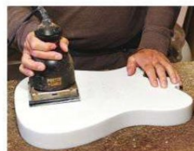
Apply several coats of automotive primer. If you sand through to the wood, apply more primer.
