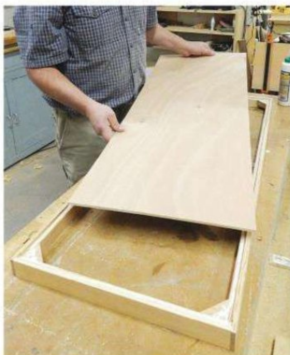
Cut the lid panel to size, then glue it into the rabbets in the frame assembly. The author used pin nails as fasteners.
