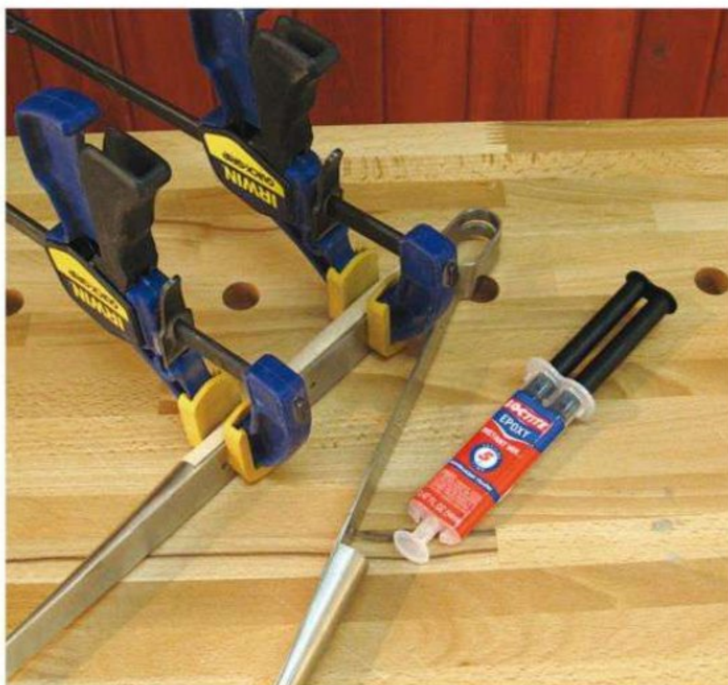
Quick-setting epoxy is a good adhesive choice for bonding the wood to the tongs. Wipe the excess off before it cures.
