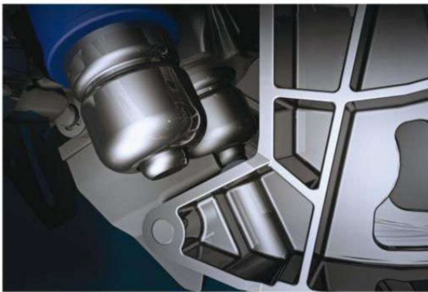
Bosch's easily removable, pressurized activation cartridge responds to two skin-sensing incidents before replacement is necessary.
