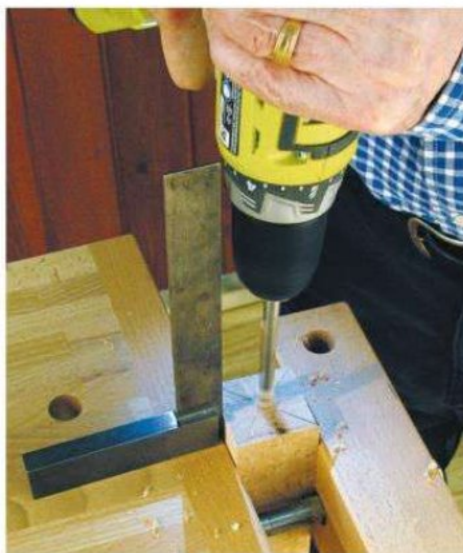
When drilling the hole to accept the threaded insert, make sure you are drilling straight into the wood. A square beside your drill can help.
