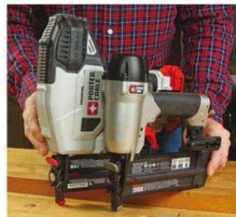
Cordless brad nailers are heavier and larger than their pneumatic counterparts, but self-contained.
