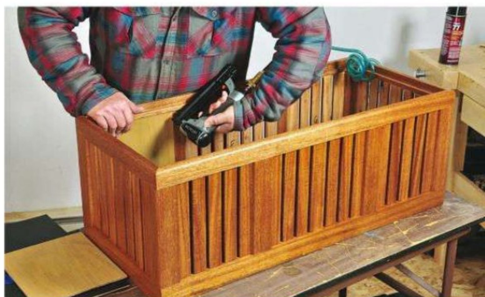
A pin nailer with 1/2" pins secured the backing panels into their frame openings. The "good" side of each panel is covered in black vinyl.
