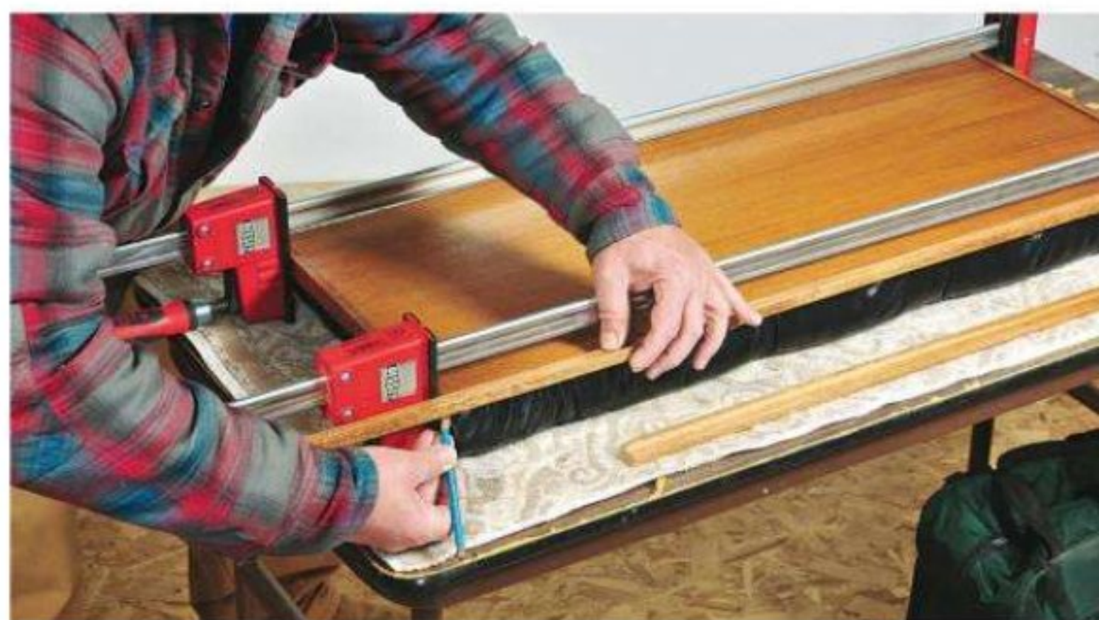
The author marks the outside length of the long trim pieces against the two pieces clamped to the short edges of the lid.
