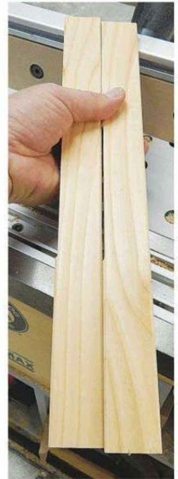
Each top bar receives a narrow vent, milled at the router table, along one edge. These vents provide air circulation between the combs but are thin enough to prevent the bees from crawling through.
