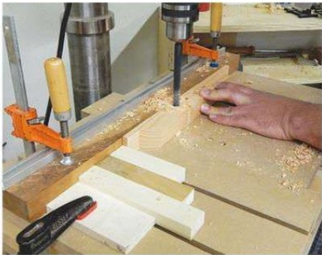
A stop block clamped to the drill press table, and three spacers, make it easy to drill the top bars' three through holes so they're evenly spaced.
