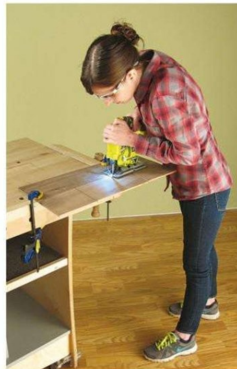
Two large rectangular sections are cut out of the lower two laminations of the shelf. Use a handheld jigsaw to remove the material.
