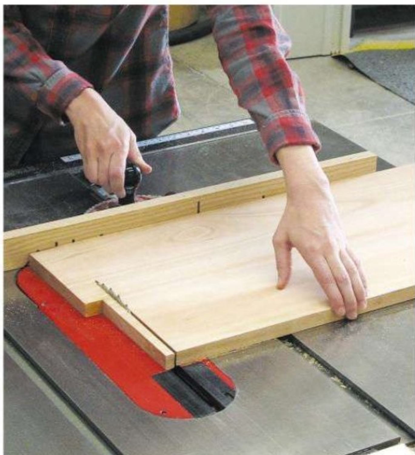
Crosscut the stock to length on the table saw with a miter gauge. A circular saw or a sliding miter saw could also handle this task.
