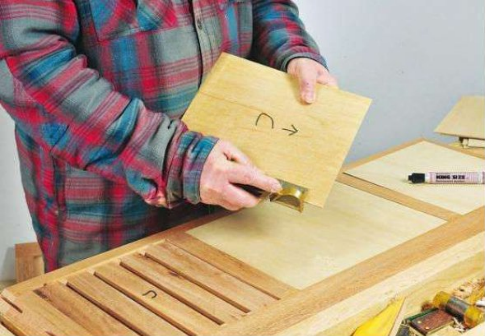
The author uses a small hand plane to trim each 1/8" plywood backing panel for a snug fit in its frame opening. Each is labeled, so it can be returned to the correct frame opening later.
