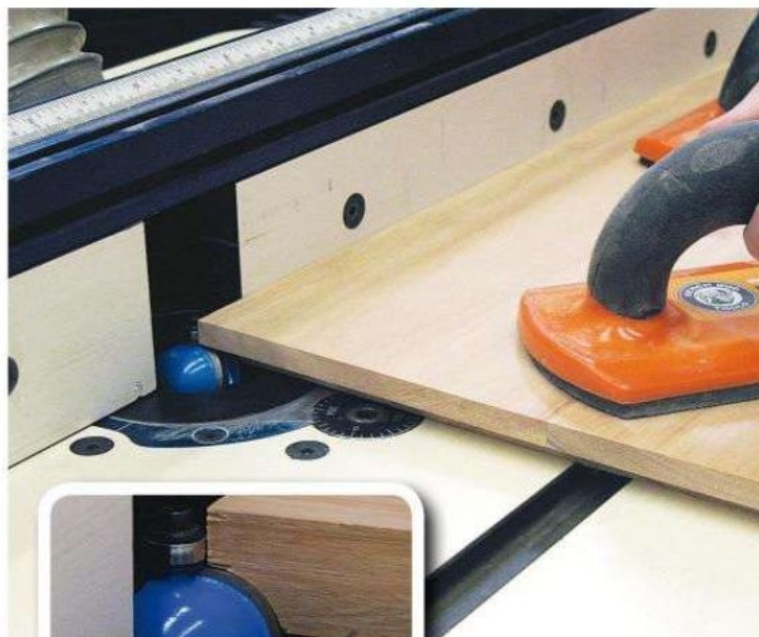
To add shape and shadows to the shelf, a 3/8" cove is routed into the edges and ends of the 3/4" stock. This works best on a router table but can also be done with a handheld router.
