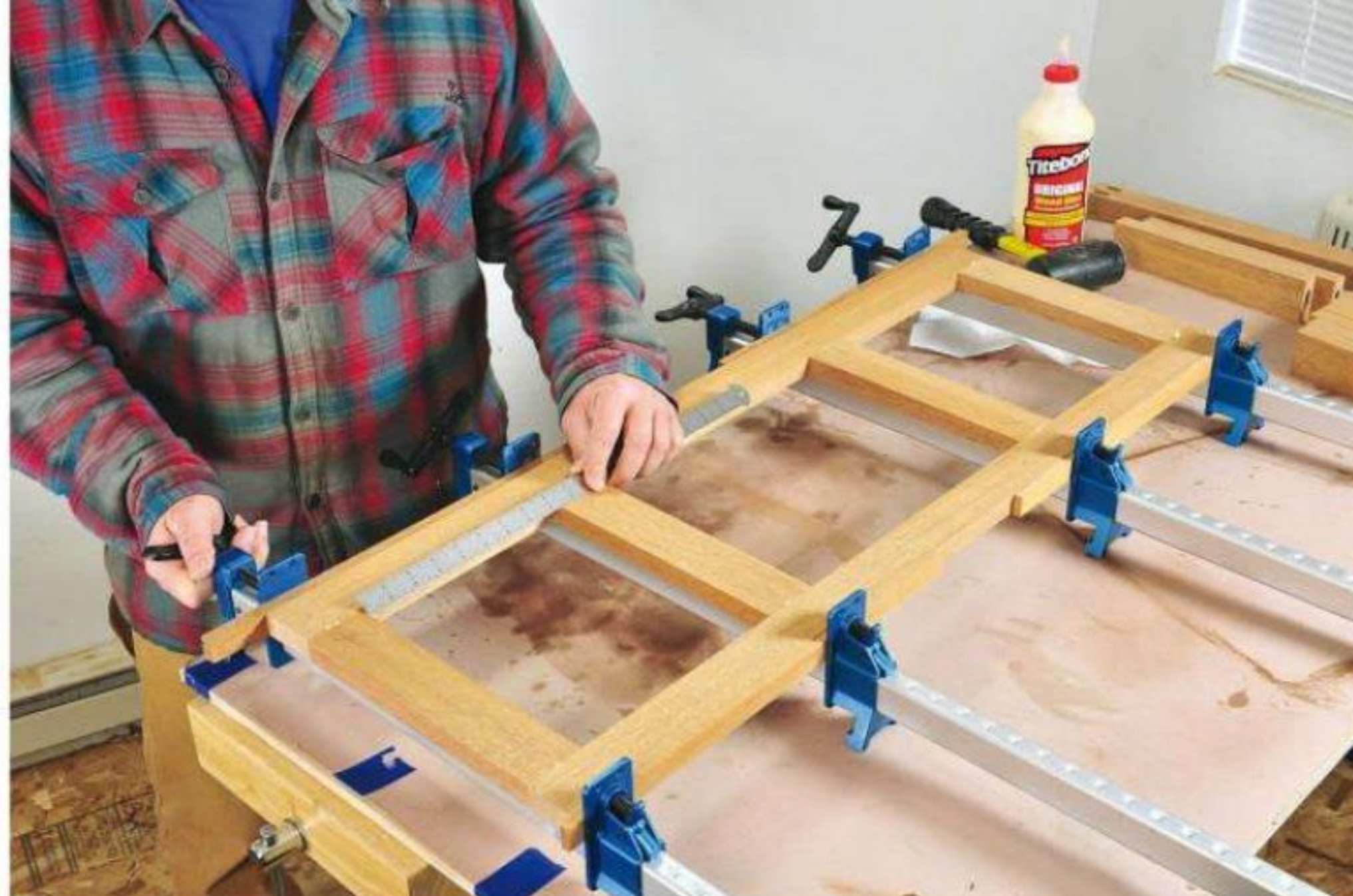
Use a ruler to make sure that the spaces for open panels on the long sides of the ottoman are even.
