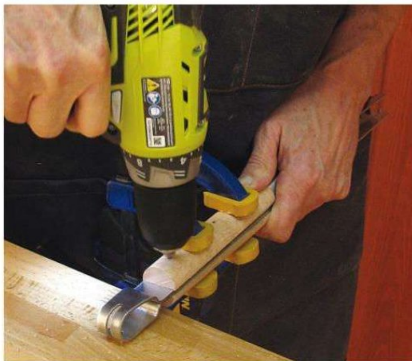
With the second handle glued in place, extend the pin holes from the first handle through it. Keep these holes perpendicular as you drill them.
