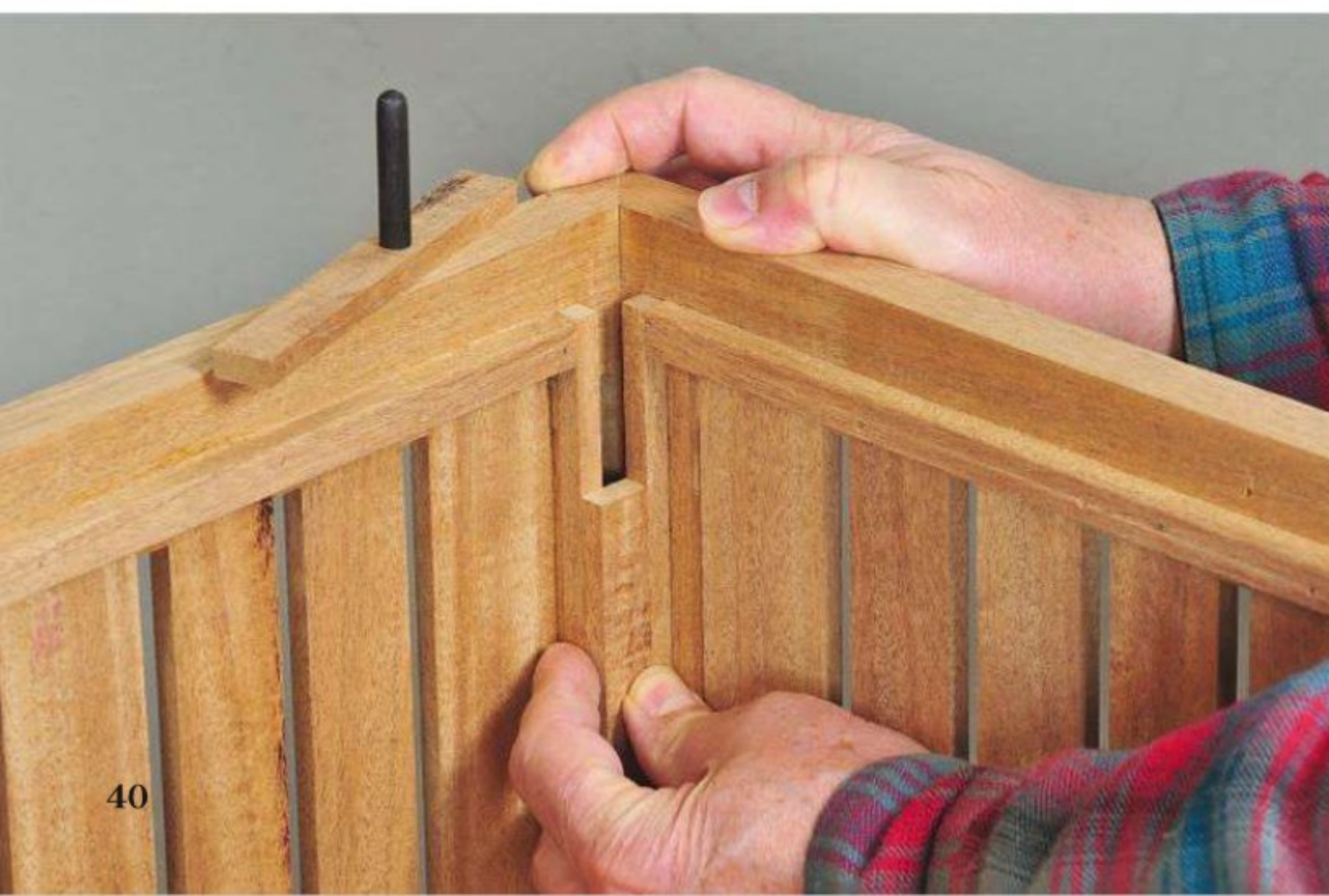
The lid lifter housing is comprised of three pieces fit to the rear left corner of the carcass.
