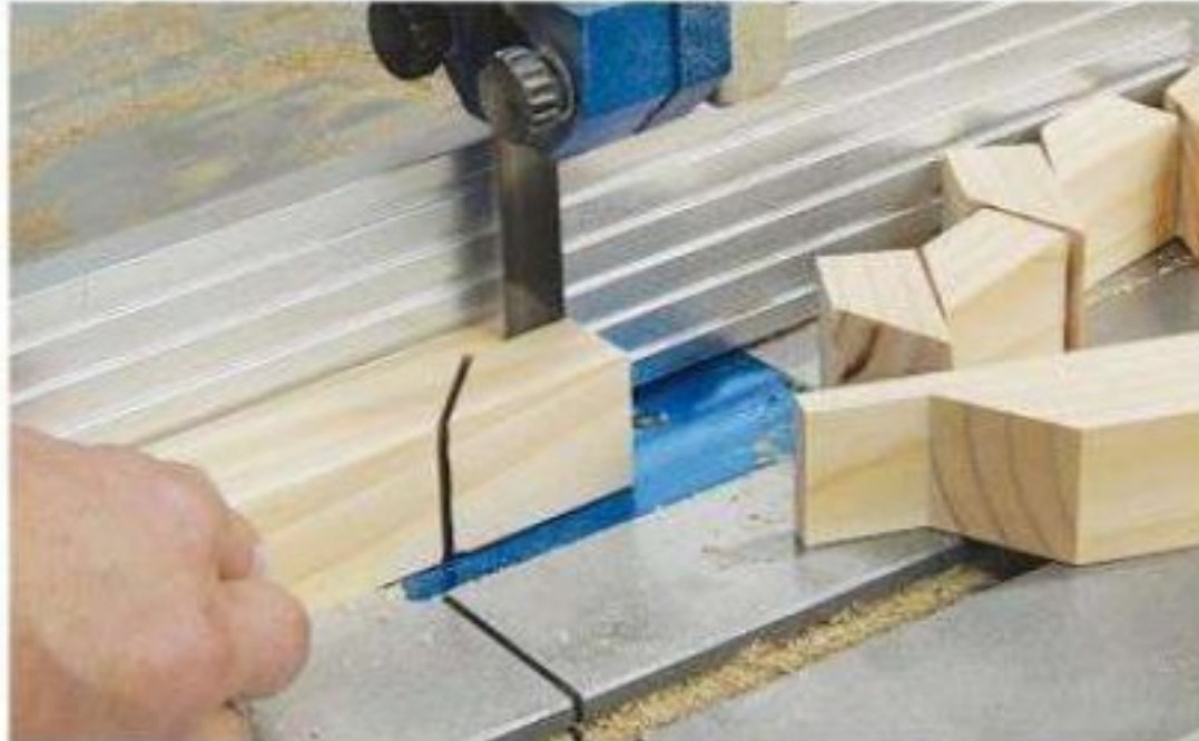
Trim the waste pieces free at the band saw to complete the "lapped" ends of the cross bars. It's a faster, safer method than using a tenoning jig at the table saw.
