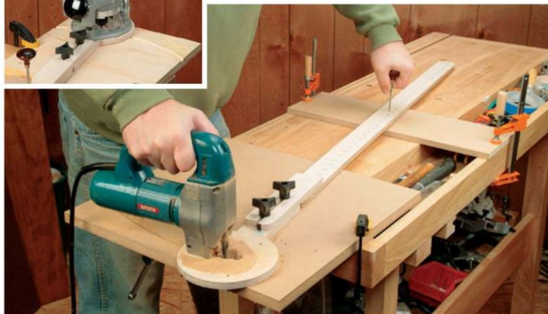
A scratch awl inserted in one of the pivot strip's holes acts as a pivot point, for either cutting or routing circles and arcs.
