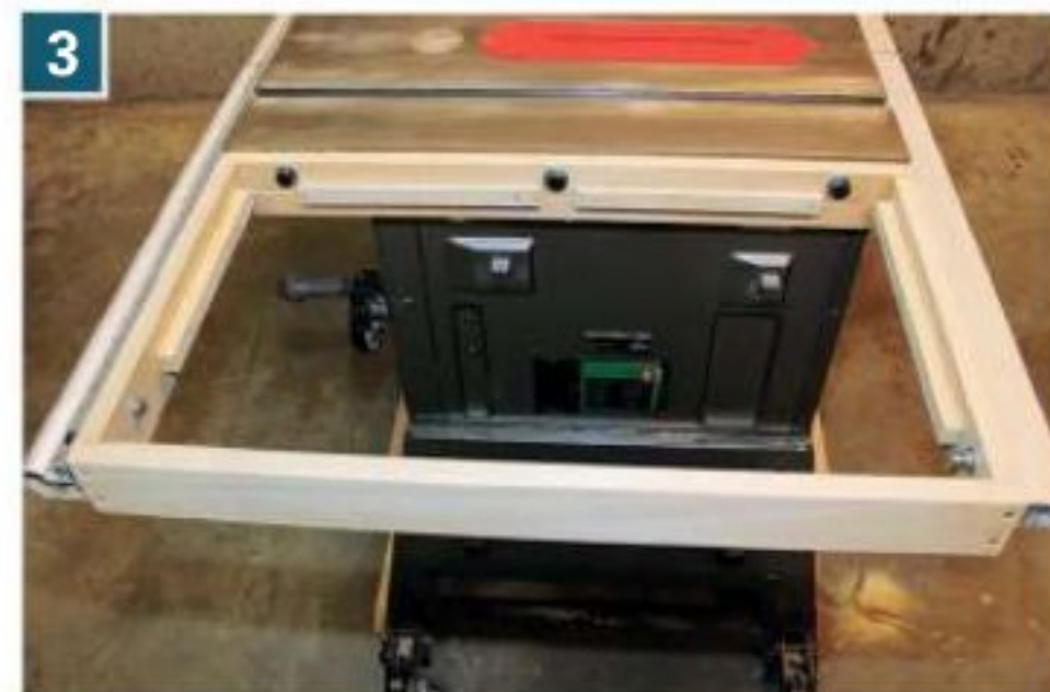
3 Bolt the frame to the saw table and rip fence rails to check its fit. The bolt holes should be large enough to allow for some fine-tuning.
