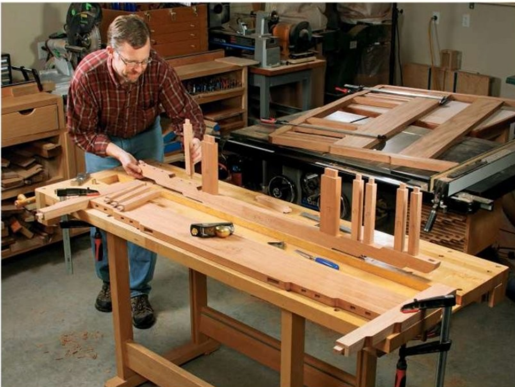
Once the rails have shaped edges, their length, weight and contour makes tenoning them on the table saw more difficult. A "wraparound" jig and a handheld router with guide collar offer a good alternative for this task.
