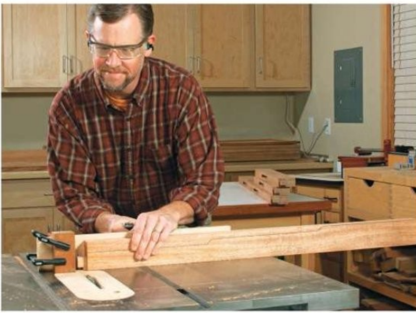
Raise tenons on the top ends of the legs before you cut their contoured edges, while the workpiece edges are still flat. A dado blade, miter gauge and stop block make this process quick and accurate.
