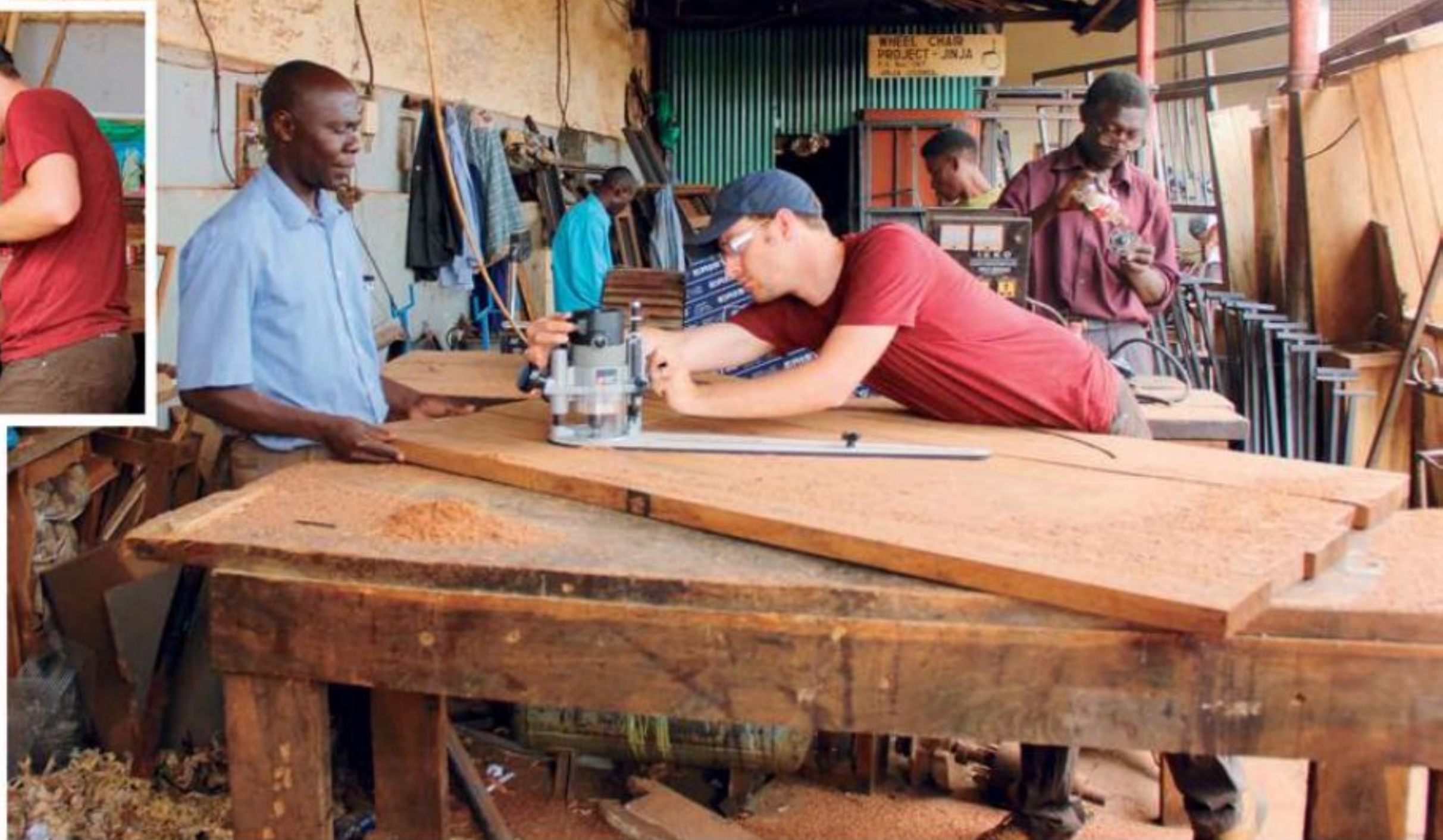
Ugandan carpenter Robert Machi (left) provided support as Brice Aarrestad routed a mugavu wood tabletop using a circle cutting jig.
