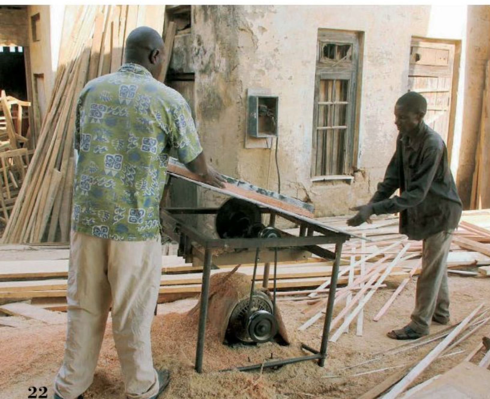
With this Ugandan tilt-top table saw, the lower the angle, the deeper the cut.
