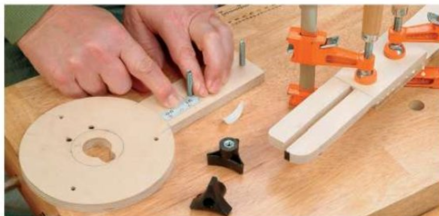
A short length of stick-on measuring tape allows fine-tuning of the distance between the jigsaw blade (or router bit) and the jig's pivot hole.
