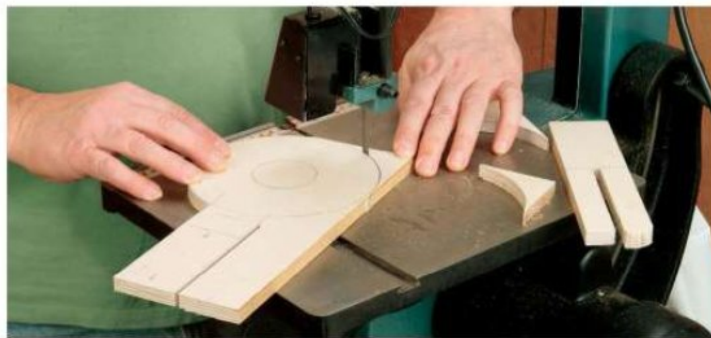
Next, using a band saw (or jigsaw), cut a 6"-diameter circle on the area of the baseplate opposite the tongue cut on the table saw in the last step.
