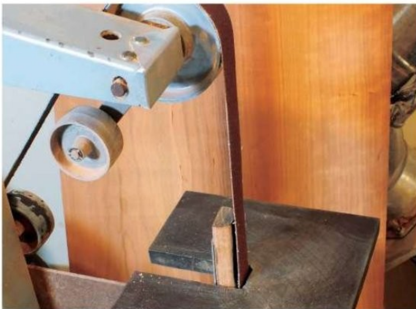
Figure 1: The author bent the platen back on his 1"-wide edge sander and screwed half of a 1" dowel to it. It enables easier sanding of inside curves.
