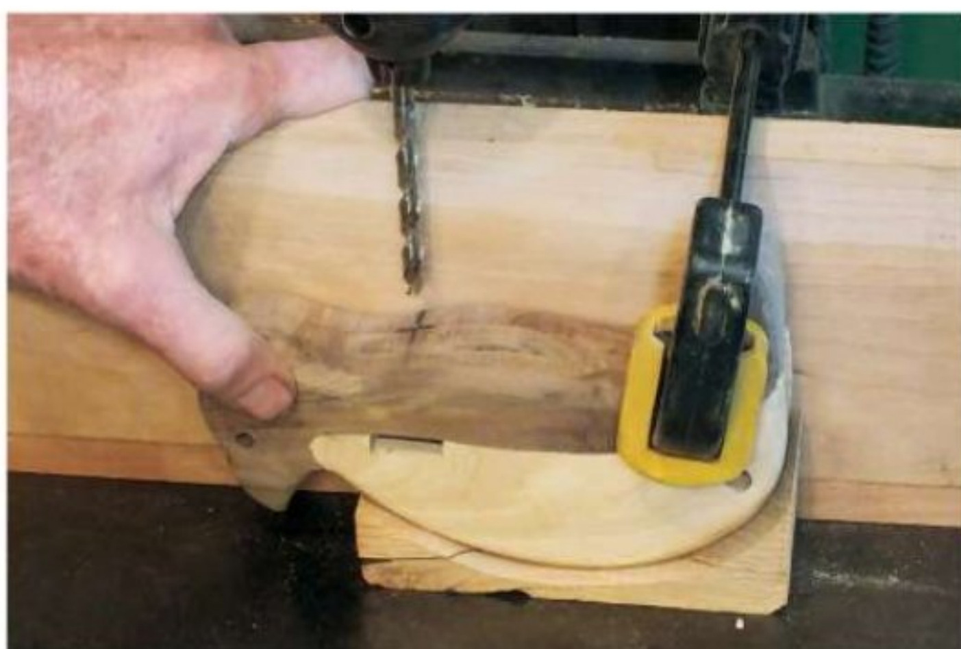
Figure 5: Support the penguin's body for drilling with a shaped block under the belly and a right-angle fence behind. The goal is to hold the body perpendicular to the drill bit and parallel to the drill press table for boring the flipper assembly's pivot hole.
