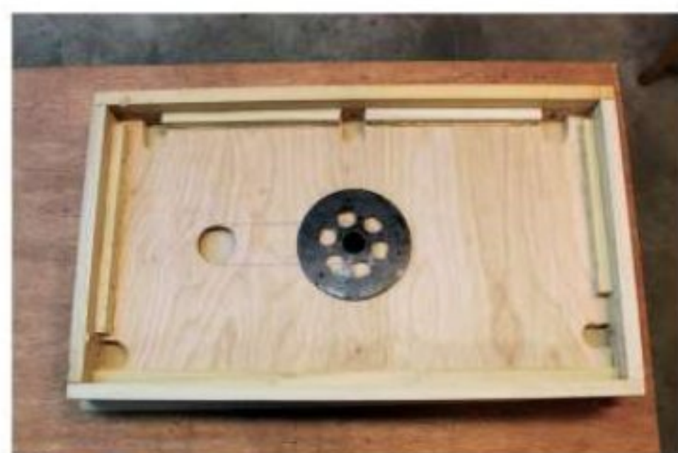
Your router's baseplate makes an excellent template for determining where to drill the attachment screws for the router base.
