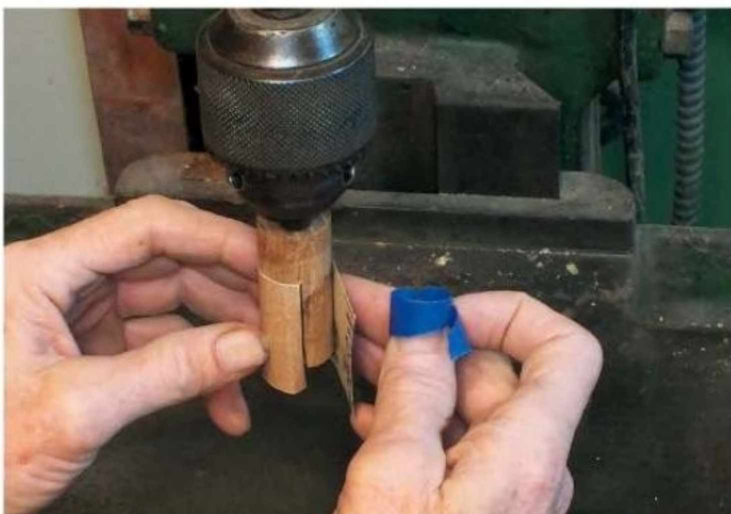
Figure 3: Make a drum sander for tight inside curves if you don't have one. Just cut a slot in a dowel and wrap some sandpaper around the dowel, using the slot to hold it in place. Secure the paper with a strip of tape.
