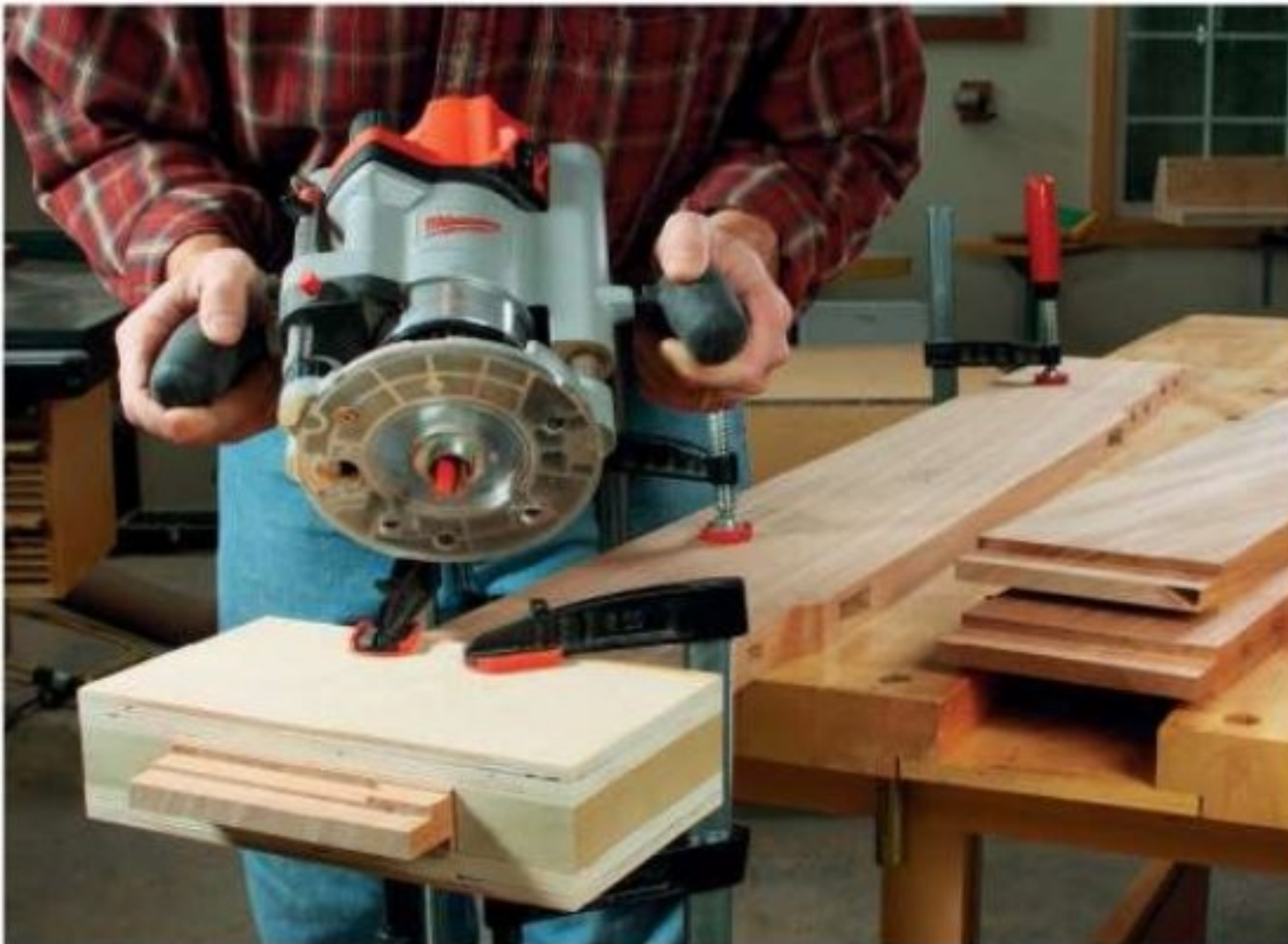
Once the rails have shaped edges, their length, weight and contour makes tenoning them on the table saw more difficult. A "wraparound" jig and a handheld router with guide collar offer a good alternative for this task.
