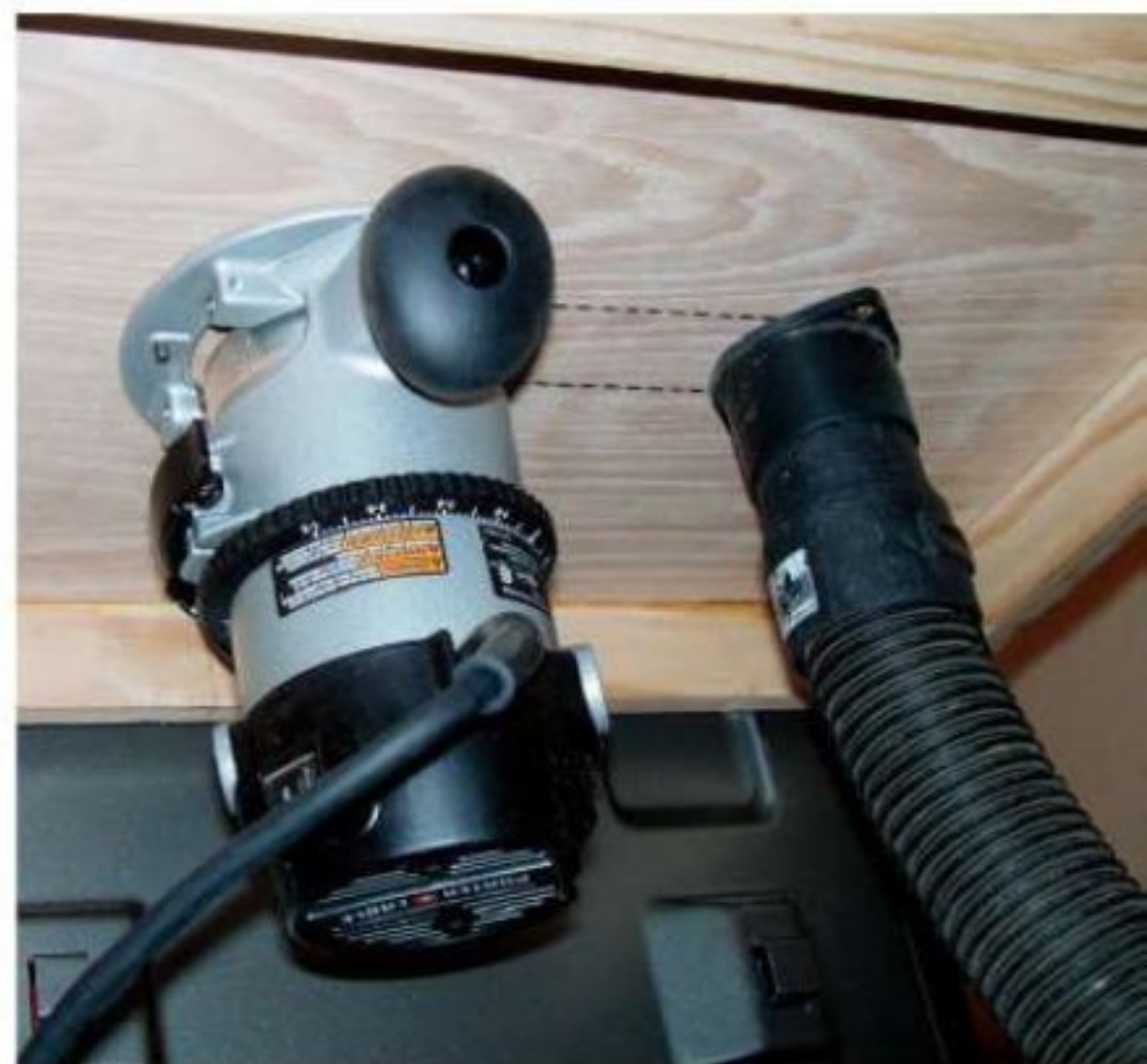
The internal chamber allows a shop vac to draw debris away from close to the router with no hose obstructions above the table.
