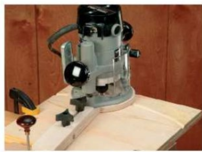
A scratch awl inserted in one of the pivot strip's holes acts as a pivot point, for either cutting or routing circles and arcs.
