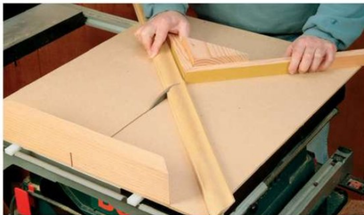
Using a miter jig on a table saw is one of the best ways to ensure perfectly matching mitered corners when you're making picture frames.
