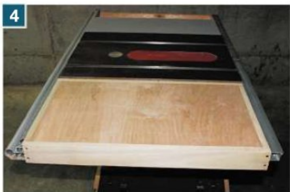
4 Cut a piece of 3/4" birch plywood for the table's bottom layer. Once set into place, its top surface should be flush with the top of the frame.
