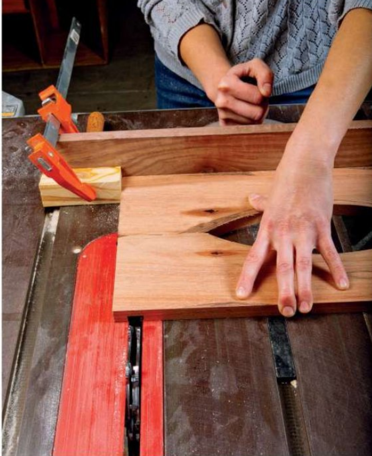
A stop block clamped to the miter gauge fence enables the shelf dados to be cut accurately. Our author held the sides in alignment to cut both dados at once, but you could cut one dado at a time if you prefer.
