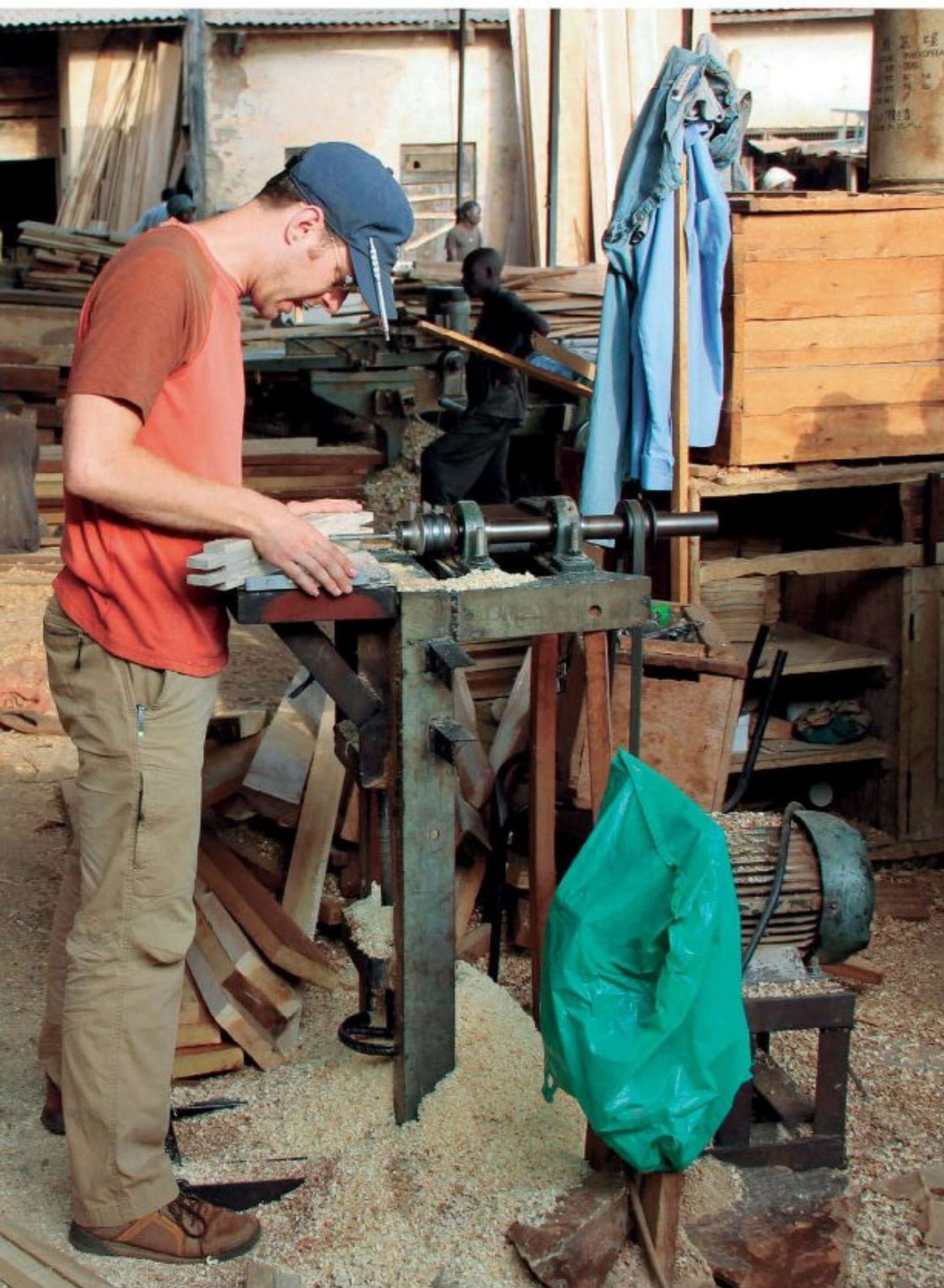
Brice Aarrestad used a Ugandan “locally made” mortising machine (a motor on one end with a shaft connected to a drill chuck) to bore holes in a bench frame.
