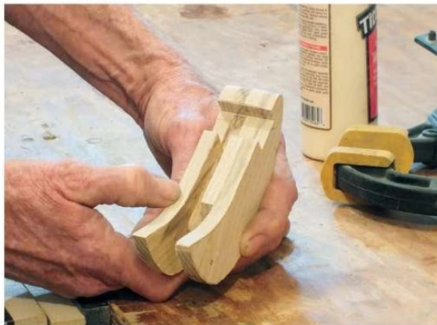
Figure 2: Organize the four pieces of the body carefully before gluing and clamping them together. Keep the front edges aligned.
