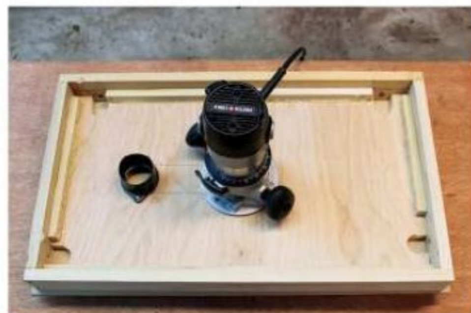
Orient your router on the table so you'll have easy access to its On/Off switch and depth-setting controls once it's installed.
