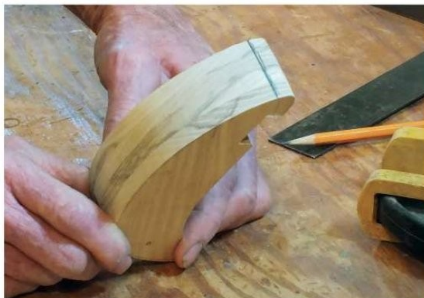
Figure 4: The author marked the top of the belly piece with a pencil line to avoid spreading glue too far forward on the front edge. The glue should stop just short of the penguin's beak.
