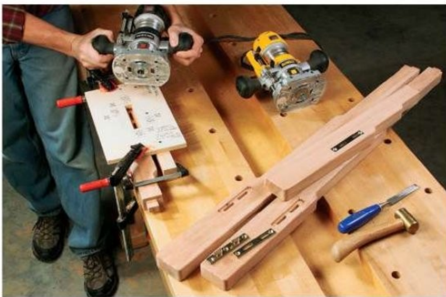
The author clamped a shop-made, slotted mortising jig to the legs, then used two different guide collars and bit sizes to rout the bed rail hardware mortises and prong slots. Chisel the shallow mortises square.
