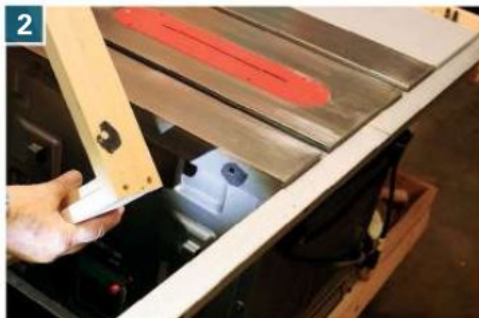
2 The author dabbed black paint on the hole locations of his saw table to mark the router frame for drilling matching holes.
