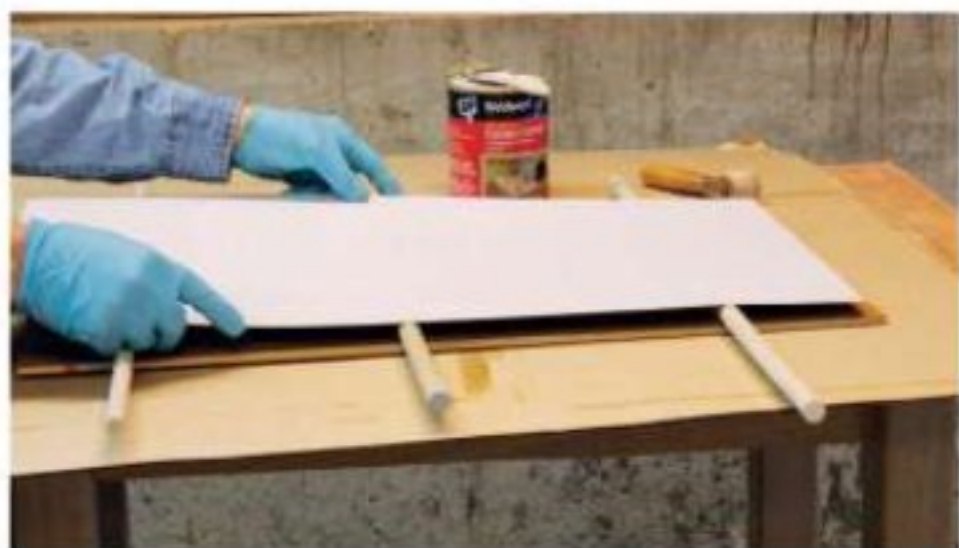
Bond the top laminate to the middle MDF layer with contact cement. Dowel spacers make it easier to position the laminate accurately.
