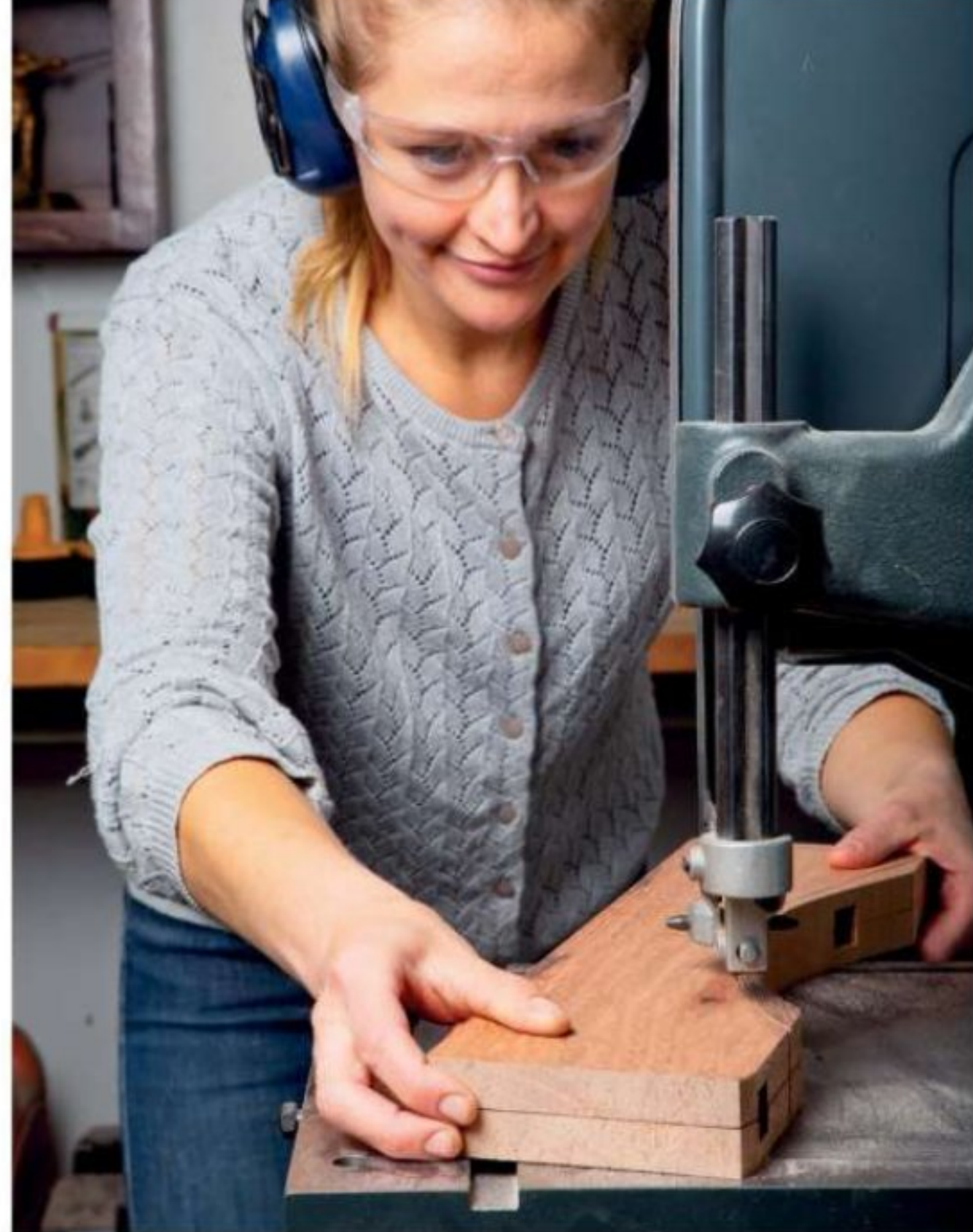
Stacking and securing the side pieces together with double-sided tape, the author could make the open-ended branch cuts at the same time on the band saw.
