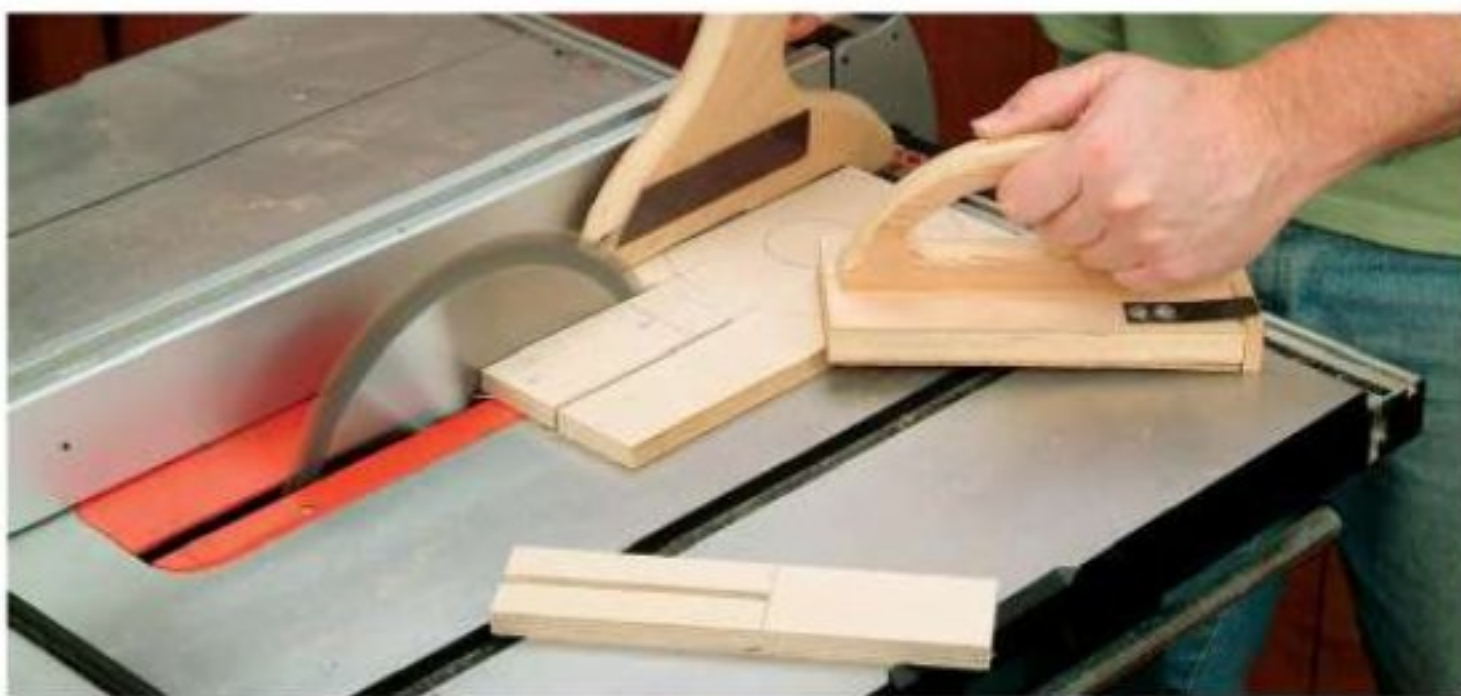
Using a table saw and rip fence, make two 5"-long stopped cuts to form a 2"-wide tongue that's centered on the jig's base, widthwise.
