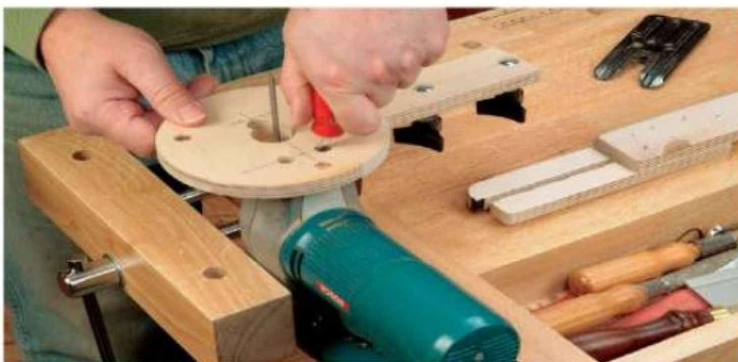
Counterbored holes bored through the circle jig's round baseplate provide the means for mounting either a jigsaw or a router.
